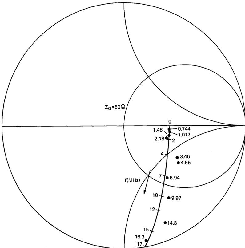
Fig. 9—Comparison of experimental (solid dots) and theoretical (solid curve) frequency dependence of the small-signal impedance  $Z_i$ . GaAs diode,  $I_o = 120 \text{ mA}$ ,  $f_o = 4.7 \text{ GHz}$ , output power = 1 watt,  $R_- = 143.6 \Omega$ ,  $R_{sc} = 33.6 \Omega$ , and  $\gamma = 59 \times 10^6$  radians per second.
