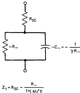
Fig. 7—Low-frequency equivalent circuit of an oscillating IMPATT diode neglecting thermal effects.  $R_{sc}$  is the space-charge resistance of the diode,  $\gamma$  and  $R_-$  are defined in the text.
