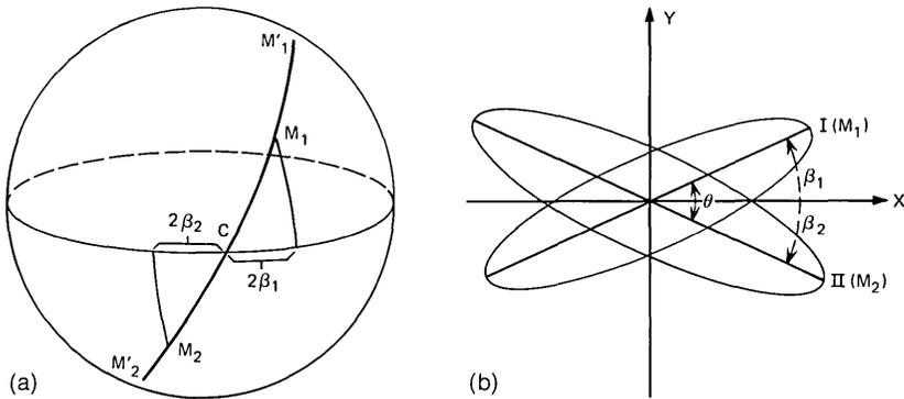
Fig. 1—Orthogonalization by differential attenuation.
