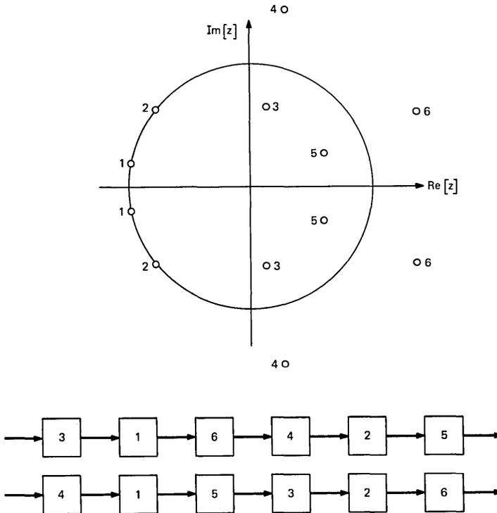
Fig. 3—Two orderings with equal output noise variances.
