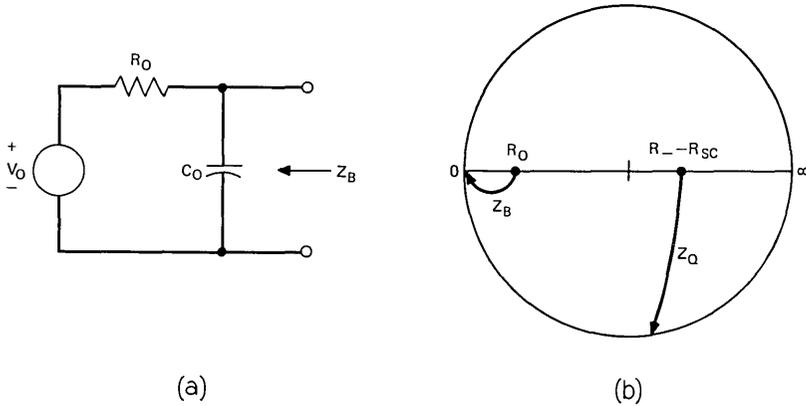
Fig. 13—Stability considerations for constant-voltage supply: Section 6.2.3.
