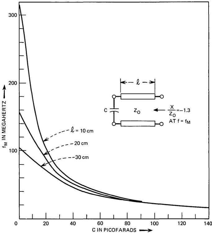
Fig. 17—Depicting the effect of a length of line,  $l$ , between the diode (having maximum bias-circuit oscillation frequency  $f_M$ ) and a shunt capacity  $C$ , for the GaAs diode terminal impedance shown in Fig. 2.
