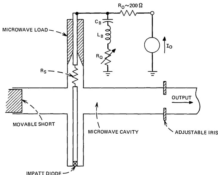
Fig. 1—Microwave cavity and bias configuration. The IMPATT diode is mounted at the end of a coax line which is coupled to the microwave cavity. The bias circuit includes a stabilizing resistor  $R_s$ , a resonant circuit  $C_B$ ,  $L_B$ ,  $R_Q$  used to induce bias-circuit oscillations, and a resistor  $R_0$  to isolate the bias circuit from the constant current supply  $I_0$ .
