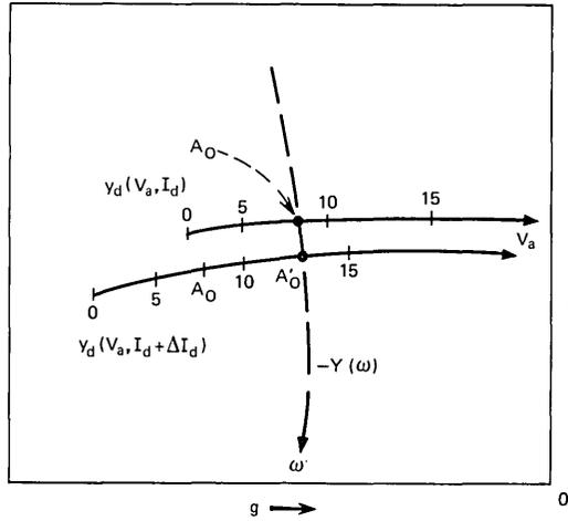
Fig. 5—Schematic admittance-plane description of the microwave large-signal device admittance,  $y_d(V_a, I_d)$ , and the negative of the microwave circuit admittance,  $-Y(\omega)$ . The intersection of  $y_d$  with  $-Y$  determines the amplitude of the microwave oscillation  $A_o$  and the frequency  $\omega$ . An increase in  $I_d$  requires an increase in  $V_a$  from  $A_o$  to  $A'_o$  as shown.
