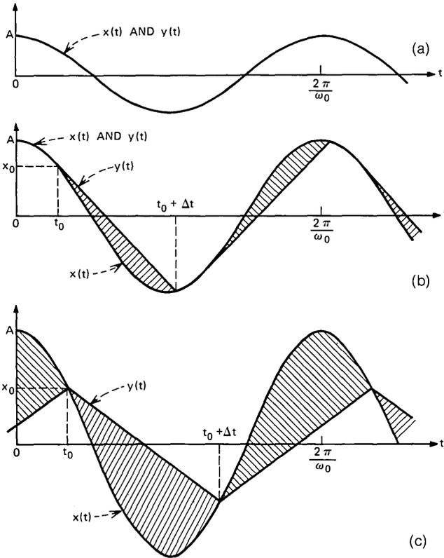
Fig. 4—The three regions of sinewave amplitude. (a)  $0 \leq A \leq x'_0/\omega_0$  (no noise). (b)  $(x'_0/\omega_0) < A < (x'_0/\omega_0)\sqrt{1 + \pi^2/4}$  (primary noise). (c)  $A \geq (x'_0/\omega_0)\sqrt{1 + \pi^2/4}$  (secondary noise).
