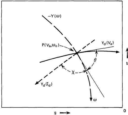
Fig. 6—Illustrating the definitions of the angles  $\theta$  and  $\chi$  at the intersection of the device admittance  $y_d(V_a)$  and the circuit admittance  $-Y(\omega)$ . The intersection angle is  $\theta$  for microwave voltage variations and is  $\chi$  for bias-current variations. The angle  $\theta + \chi$  is determined by the device alone.
