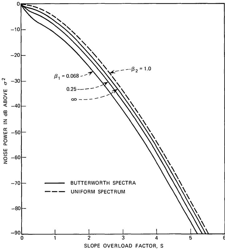
Fig. 13—Noise power results for several spectra.
