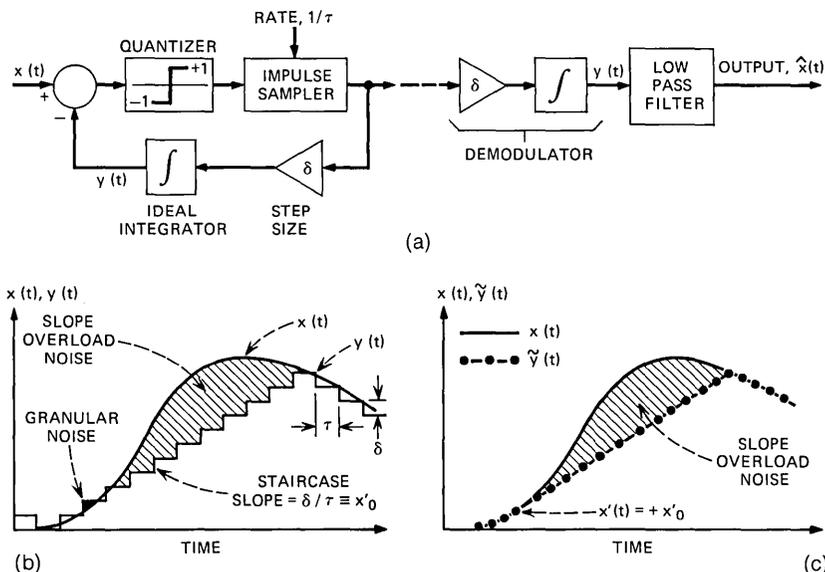
Fig. 1—Linear  $\Delta M$  codec with perfect feedback integrator. (a) Equivalent block diagram. (b) Input and feedback signals. (c) Model used.
