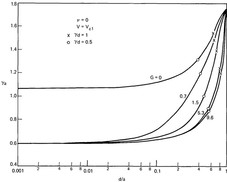
Fig. 8—This figure shows the parameter  $\gamma a$  as a function of  $d/a$  for several values of  $G$ .  $V$  is taken equal to the cutoff value  $V_{c1}$  of the mode  $\nu = 1$ .
