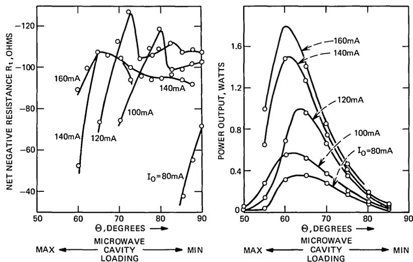
Fig. 3—Output power and induced net small-signal negative resistance as a function of bias current and microwave loading for GaAs. Microwave frequency was 4.7 GHz, bias-circuit frequency was  $\sim 5$  MHz.
