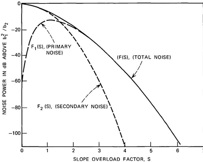
Fig. 6—Normalized noise powers for the two-band process.
