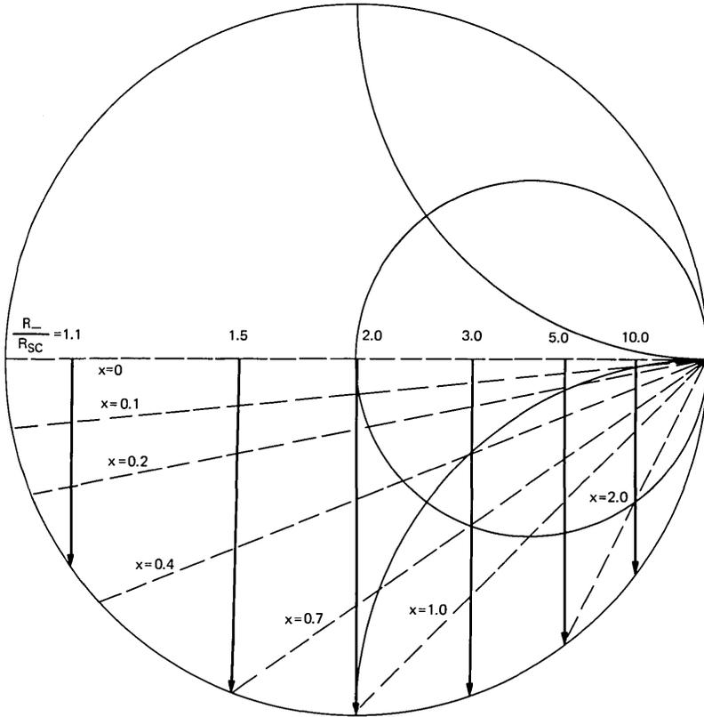
Fig. 8—The negative of the equivalent circuit impedance,  $Z_t/R_{sc}$ , normalized to the space-charge resistance, versus normalized frequency  $x = \omega/\gamma$ . The straight line characteristics of this plot make it useful in estimating the ratio of  $f_M$  from the values of  $R_-$ ,  $R_{sc}$ , and  $\gamma$ .
