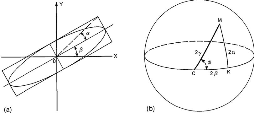
Fig. 5—Poincaré spherical representation of a polarization ellipse.
