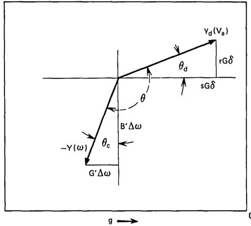
Fig. 18—Defining the angles  $\theta_c$ ,  $\theta_d$ , and  $\theta$  in the microwave large-signal admittance plane of the diode.
