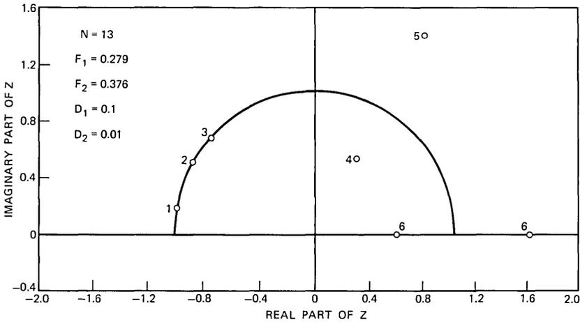
Fig. 5—Positions of the zeros of one filter.
