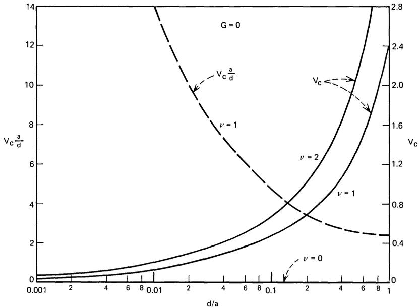
Fig. 2—The cutoff value of the normalized frequency  $V$  for  $G = 0$  as a function of the ratio of wall thickness  $d$  to tube (outer) radius  $a$ . The cutoff value for the mode  $\nu = 0$  is  $V = 0$ .
