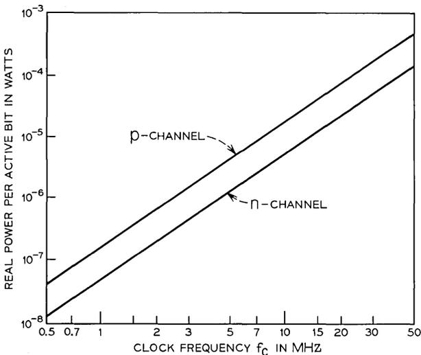
Fig. 22—Theoretical power dissipation per bit versus clock frequency for a poly-phase charge-coupled device.
