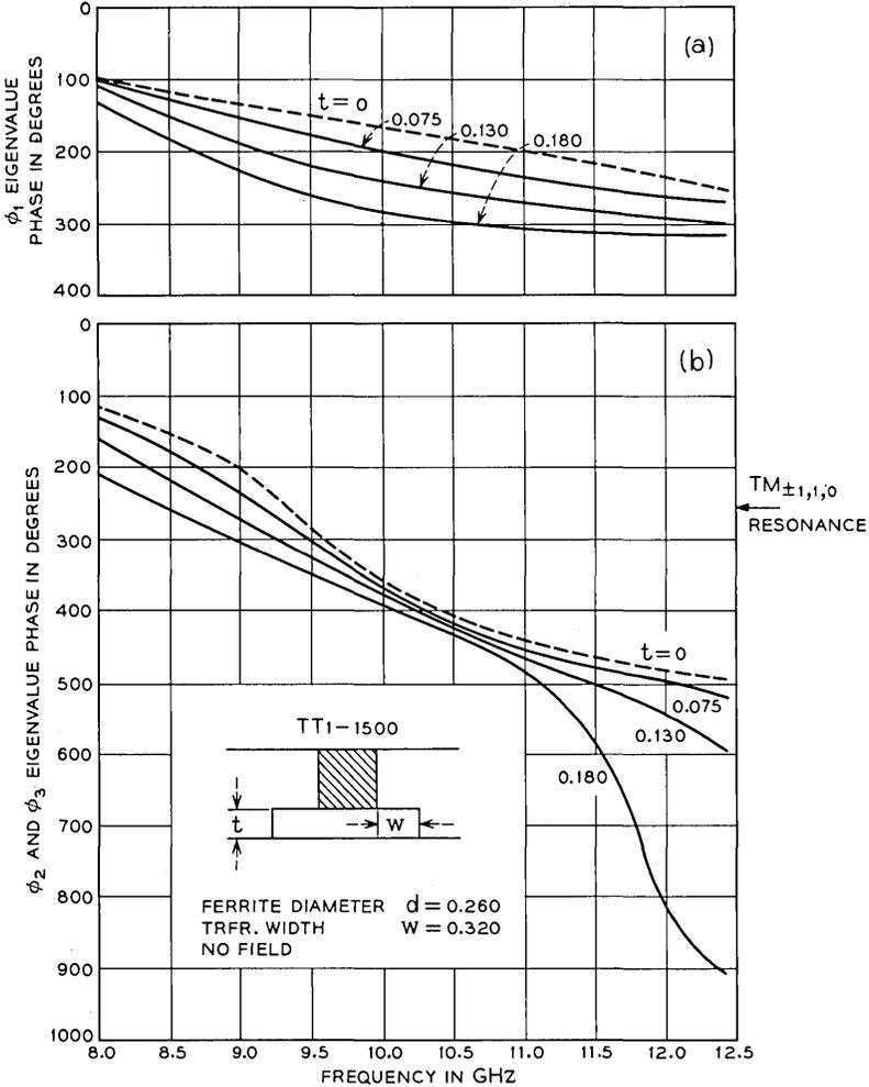
Fig. 20—The eigenvalue-phase frequency response of a junction with a full height ferrite post and different height transformers. The results show (a) the curvature in  $\angle\phi_1$  as the transformer height is increased and (b) the linearization of  $\angle\phi_2$  and  $\angle\phi_3$  in the vicinity of the  $TM_{\pm 1,1,0}$  resonance.
