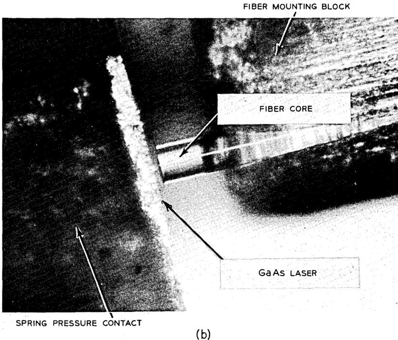
Fig. 4—(a) The Gaussian light beam emanating from a laser aperture (typical dimensions:  $1 \mu\text{m} \times 13 \mu\text{m}$ ) is injected into the core of an optical fiber. In its far field the beam diverges at an angle,  $\alpha_y$ , perpendicular to the junction plane. (b) Photograph taken through a microscope shows the 0.5-mil air gap across which light is coupled from a GaAs laser into the core of a 10-micron fiber.
