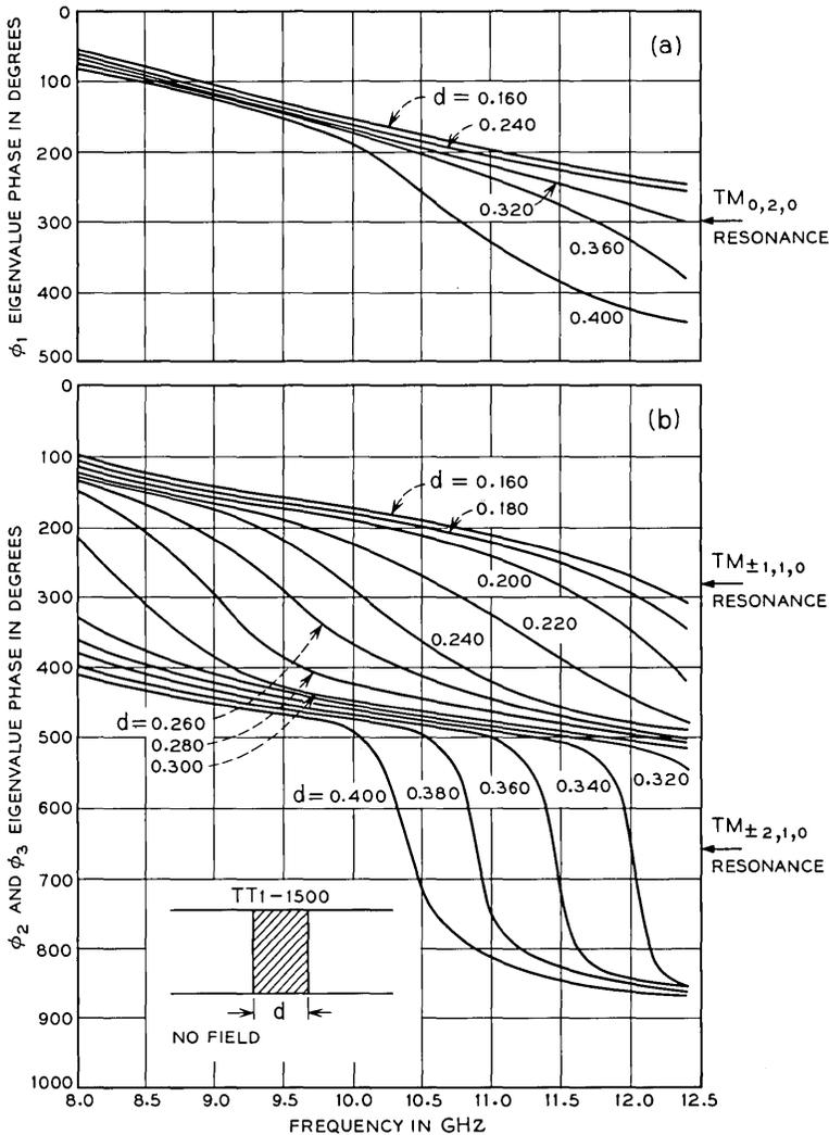
Fig. 11—The eigenvalue phase-frequency response of a junction with a full height ferrite post of various diameters. The results display (a) the lower-order  $TM_{0,n,0}$  modes in  $\angle\phi_1$ , (b) the lower-order  $TM_{\pm m,n,0}$  modes in  $\angle\phi_2$  and  $\angle\phi_3$ .
