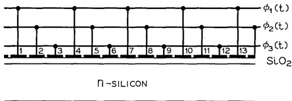
Fig. 2—Simple three-phase charge-coupled device.
