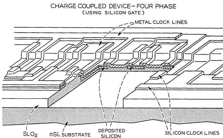
Fig. 8—Sectional drawing of a multilevel charge-coupled device.
