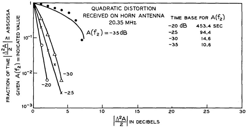
Fig. 14—Conditional quadratic distortion distributions for 20.35 MHz.
