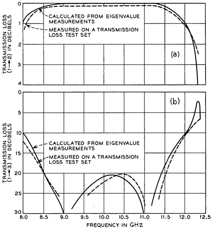
Fig. 24—Transmission loss from (a) ports 1 to 2 and (b) ports 1 to 3 for the junction in Fig. 23. The losses calculated from the eigenvalue phase are compared with those measured on a loss test set.
