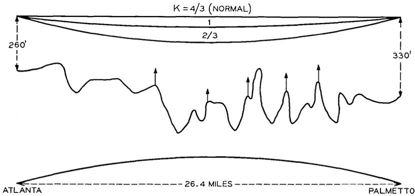
Fig. 2—Atlanta-Palmetto path profile and line-of-sight radio path for the normal (an equivalent earth radius factor  $k = 4/3$ ) and the less frequent ( $k = 1, 2/3$ ) atmospheric configurations. Clearance is adequate even for the extreme case of  $k = 2/3$ .
