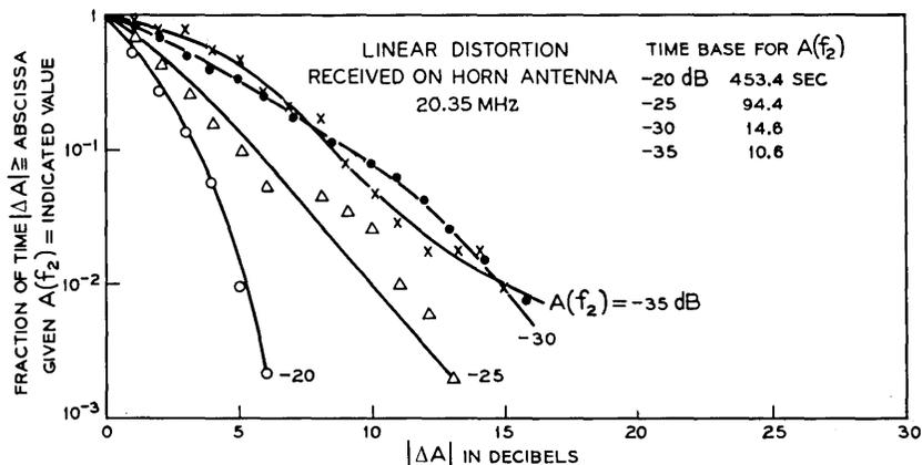
Fig. 13—Conditional linear distortion distributions for 20.35 MHz.
