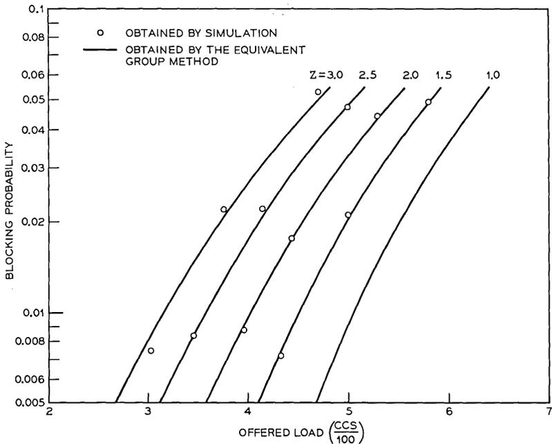
Fig. 3—Load service relations for the 25-trunk graded multiple with 40 selectors.
