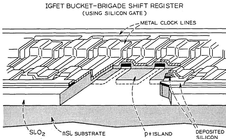
Fig. 5—Cutaway view of integrated bucket-brigade register—silicon gate technology.
