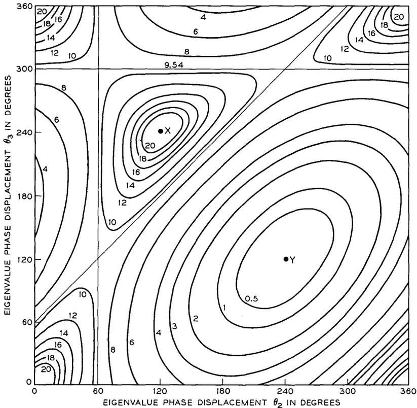
Fig. 2—The transmission loss in decibels from port 1 to port 2 is shown as a function of the phase angles between the eigenvalues. The curves are the loci of constant loss.
