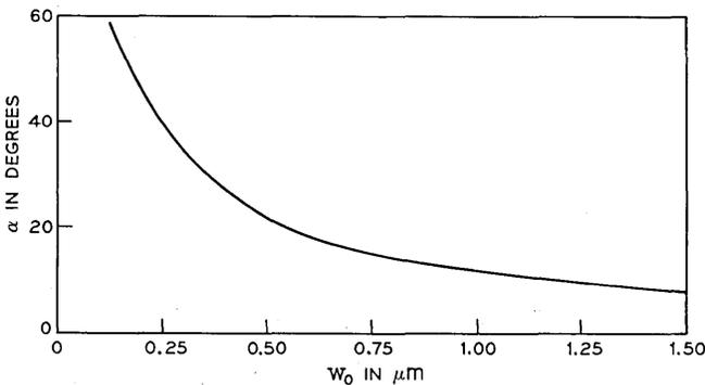
Fig. 9—The far field divergence angle,  $\alpha$ , of a Gaussian power distribution is plotted versus the half-width,  $w_o$ , of the electric field at the beam waist ( $\lambda = 9000 \text{ \AA}$ ).  $\alpha = \tan^{-1} \lambda / \sqrt{2} \pi w_o$ .
