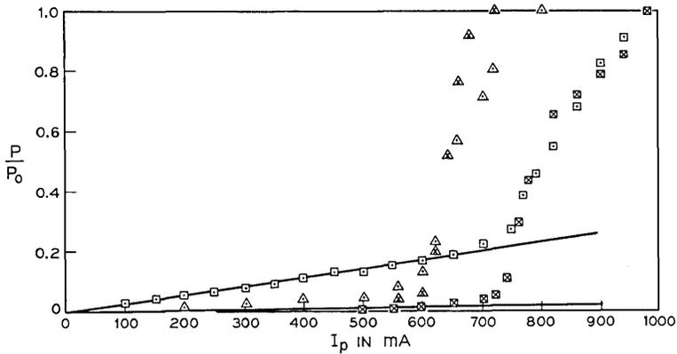
Fig. 6—Normalized power radiated from the laser surface versus pump current:  $\square$  L-352 #1, DH laser with oxide-masked stripe;  $\triangle$  L-363 #1, DH laser with proton-bombarded stripe. Normalized power leaving the end of a  $3.2\text{-}\mu\text{m}$  fiber versus pump current:  $\boxtimes$  L-352 #1, DH laser;  $\blacktriangle$  L-363 #1, DH laser.
