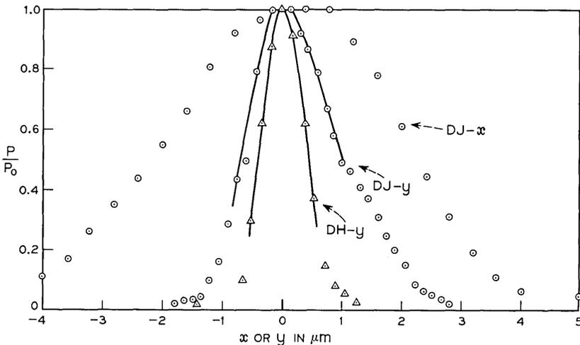
Fig. 3—Near field power distributions on the surface of junction lasers. Legend:  $\circ$  L-229 #1, DJ laser with stripe width =  $6 \mu\text{m}$ .  $\triangle$  L-363 #1, DH laser with stripe width =  $13 \mu\text{m}$ . Normalized power,  $P/P_0$ , is plotted versus distance,  $x$ , along the junction and distance,  $y$ , perpendicular to the junction.
