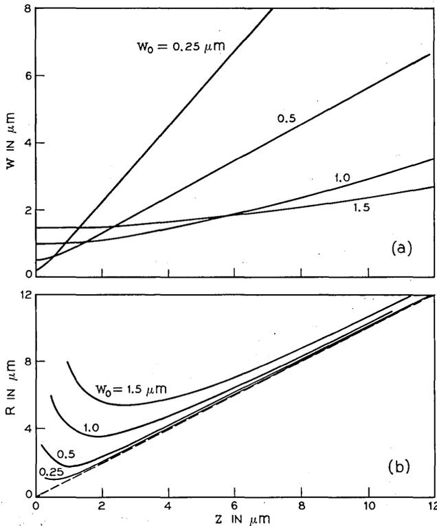
Fig. 10—(a) The half-width,  $w$ , of a Gaussian beam is plotted versus  $z$ , the separation of the reference plane from the plane of the beam waist ( $\lambda = 9000 \text{ \AA}$ ). The half-width,  $w_0$ , of the electric field at  $z = 0$  is the parameter. (b) The wavefront radius of curvature,  $R$ , is plotted versus  $z$  ( $\lambda = 9000 \text{ \AA}$ ).  $w_0$  is the parameter.
