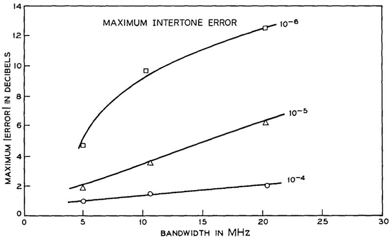
Fig. 22—A crossplot of Fig. 21 showing the observed MAX |ERROR| as a function of bandwidth for  $10^{-4}$ ,  $10^{-5}$ , and  $10^{-6}$  fractions of the time.
