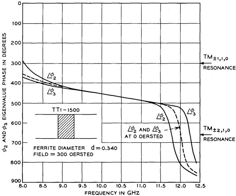
Fig. 12—The eigenvalue phase-frequency response of a junction with a full height ferrite post showing the  $TM_{\pm 1,1,0}$  and  $TM_{\pm 2,1,0}$  resonant modes splitting in opposite directions with field.
