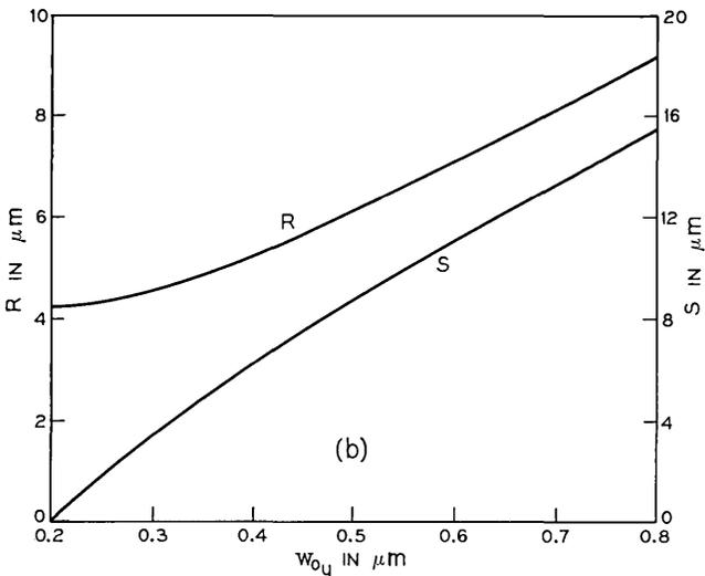
Fig. 7—(a) Cylindrical lens arrangement for collimating the laser beam perpendicular to the junction plane. (b) The radius of curvature,  $R$ , of a cylindrical lens and its axial offset,  $s$ , from the surface of a laser are plotted versus  $w_{0y}$ , the mode width perpendicular to the junction plane. The lens is designed to collimate the beam ( $\lambda = 9000 \text{ \AA}$ ) to a  $6\text{-}\mu\text{m}$  half-width perpendicular to the junction plane.
