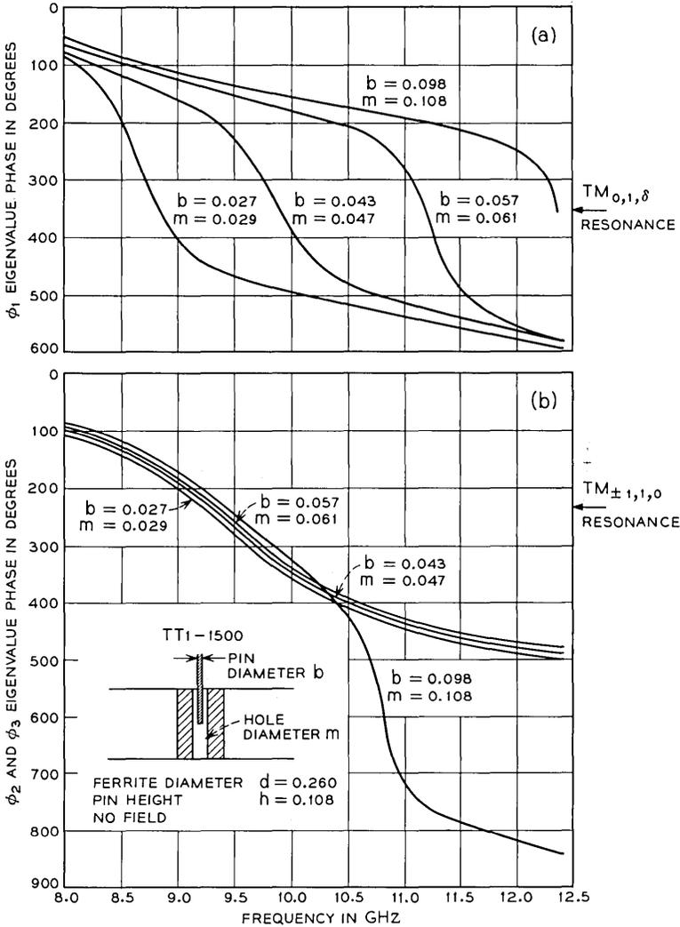
Fig. 14—The eigenvalue phase-frequency response of a junction with a full height ferrite post and containing various diameter holes and various diameter axial pins. In (a), the  $TM_{0,1,\delta}$  resonance in  $\angle\phi_1$  increases in frequency as the pin diameter is made larger. In (b),  $\angle\phi_2$  and  $\angle\phi_3$  are unaffected until the pin is sufficiently large to excite axially resonating  $HE_{\pm m,n,z}$  modes.
