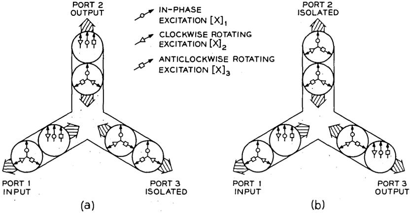
Fig. 4—A phase displacement of 120 degrees between the eigenvalues results in circulation. In (a),  $\phi_2$  is phase retarded and  $\phi_3$  phase advanced for clockwise circulation. In (b),  $\phi_2$  is phase advanced and  $\phi_3$  phase retarded for anticlockwise circulation.
