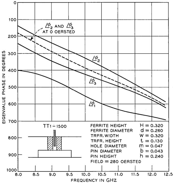
Fig. 22—The eigenvalue phase-frequency response of a junction with a transformer and pinned, full height ferrite. The eigenvalues have been linearized by the transformer in the vicinity of the  $TM_{\pm 1,1,0}$  and  $TM_{0,1,8}$  resonances. The field and pin have been adjusted for circulation.
