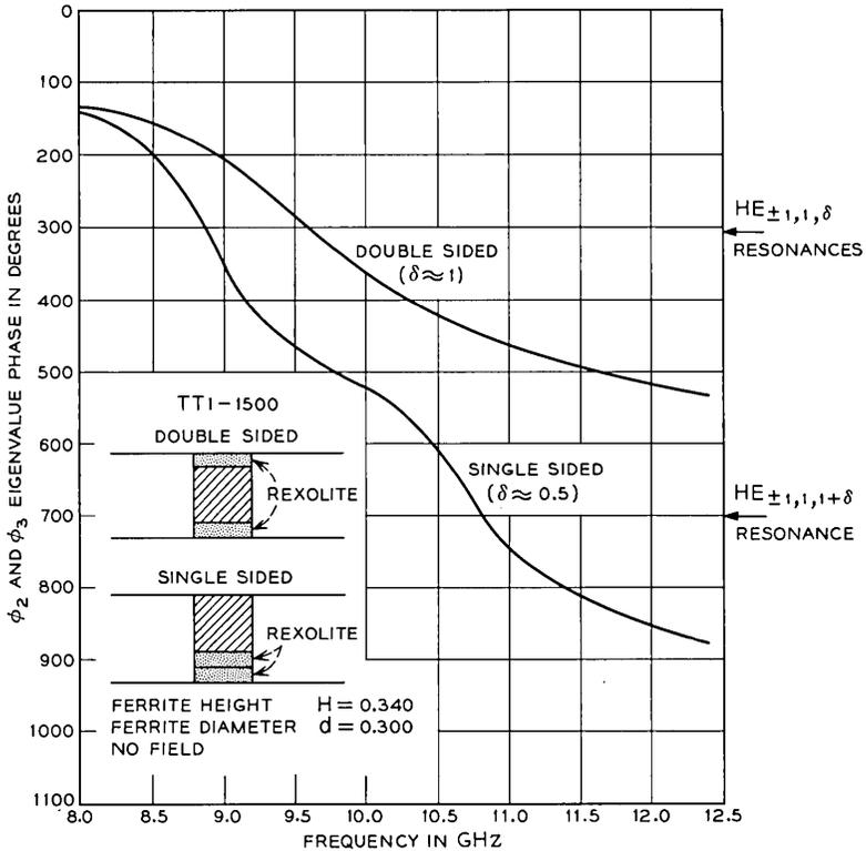
Fig. 19—The phase-frequency response of  $\phi_2$  and  $\phi_3$  for a junction with a partial height ferrite of both the single- and double-sided type. In the single-sided case, the HE resonances occur when the ferrite is approximately an integral number of quarter wavelengths long ( $\delta \approx 0.5$ ). In the double-sided case, they occur when the ferrite is approximately an integral number of half wavelengths long ( $\delta \approx 1$ ).
