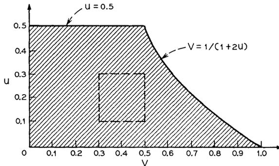
Fig. 2—Dimensional restrictions for the shielded pair. Typical values of  $u$  and  $V$  for existing shielded balanced-pair cables and equivalent  $u$  and  $V$  for multipair cables generally lie within the dashed square.
