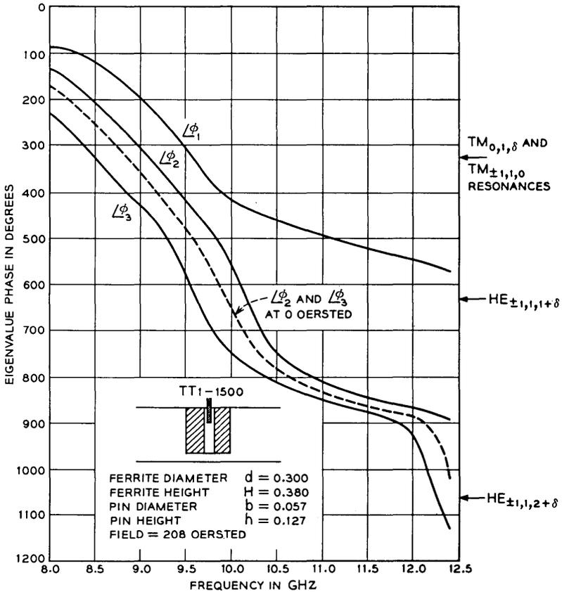
Fig. 18—The eigenvalue phase-frequency response of a junction with a partial height and pinned ferrite. The ferrite height and diameter have been selected to "stagger" the  $TM_{\pm 1,1,0}$  and  $HE_{\pm 1,1,1+\delta}$  modes, and the  $TM_{0,1,\delta}$  pin-induced resonance has been adjusted for circulation at 9.3 GHz.
