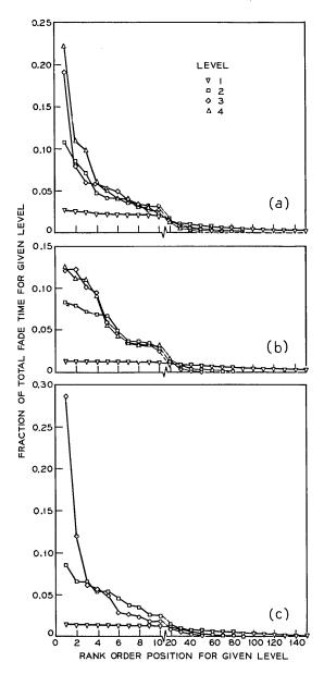
Fig. 14a—4-GHz rank order of hourly fade times, 1966 West Unity. Fig. 14b—6-GHz rank order of hourly fade times, 1966 West Unity. Fig. 14c—11-GHz rank order of hourly fade times, 1966 West Unity.
