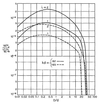
Fig. 3—The normalized first two eigenvalues  $\alpha^{(i)}d/(\bar{\sigma}^2k^2)$  (i = 1 and i = 2) are shown as functions of D/d for the 10- and 21-mode case. The lowest-order eigenvalue, i = 1, is the steady state power loss of the multimode waveguide.
