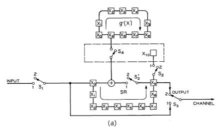
Fig. 6a—Serial encoding for the (30,20) code.
