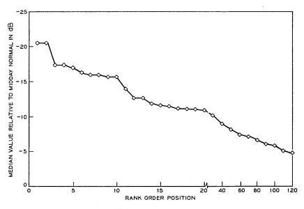
Fig. 17-4-GHz rank order of hourly median (channel 4-7).
