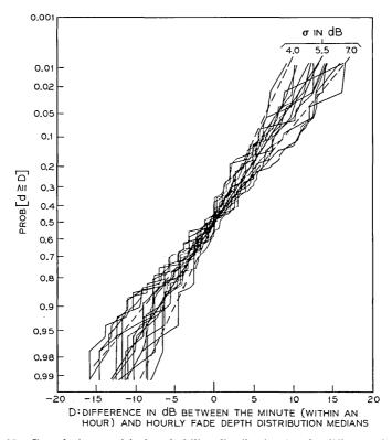
Fig. 23—Cumulative empirical probability distribution for the difference between the minute and hourly fade depth distribution medians. Data samples of five hours for 4, 6, and 11 GHz.
