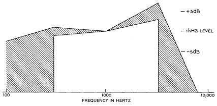
Fig. 1-Microphone response design objective.
