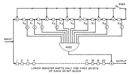
Fig. 9-Conventional single-error correcting decoder with (30,20) code.
