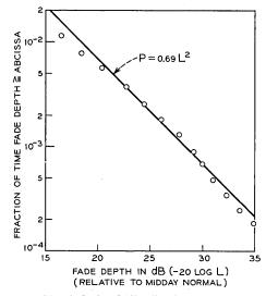
Fig. 3—11-GHz fade depth distribution, 1966 West Unity.
