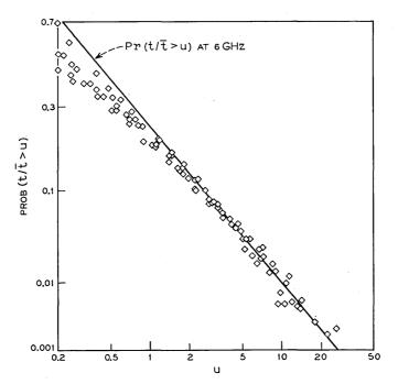
Fig. 6—11-GHz fade duration distribution: probability that the fade duration, normalized to its mean for a given fade depth, is longer than a given number. Data pooled for all fade depths greater than 10 dB.
