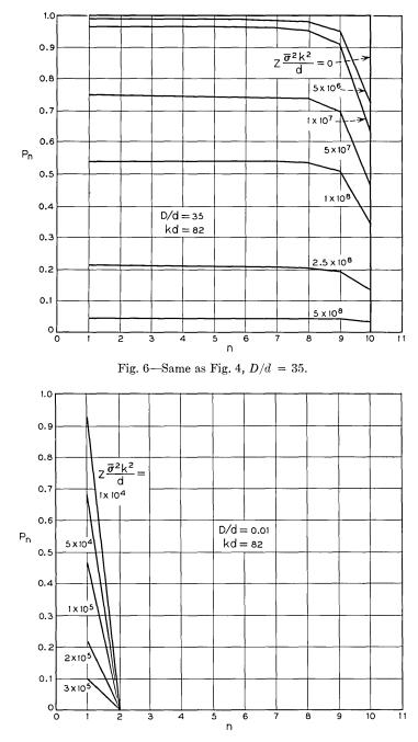
Fig. 7—Power distribution versus mode number for several values of the normalized length along the guide. Only mode 1 is excited at z = 0. D/d = 0.01.
