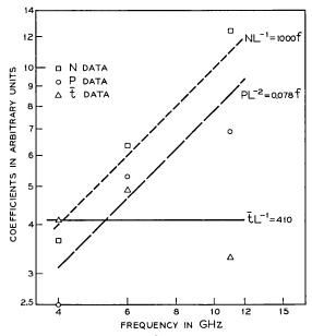
Fig. 7—Coefficients of P, N, and  $\overline{i}$  characteristics versus frequency.
