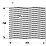
Fig. 1-Cross section of rectangular waveguide.
