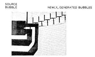
Fig. 3—Generation of bubbles in field access propagation.
