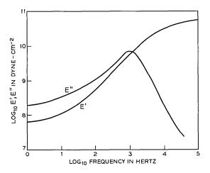
Fig. 4—Complex extensional modulus, polybutadiene, T = 20 °C.
