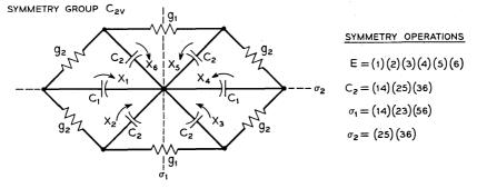
Fig. 4—Network with  $C_{2v}$  symmetry and symmetry operations.
