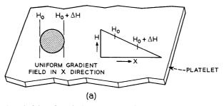
Fig. 2a-A cylindrical domain located in a uniform gradient field.
