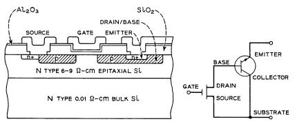
Fig. 1-BIGFET device schematic and structure.
