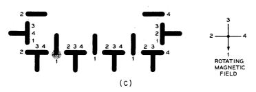
Fig. 2c-Field access propagation of bubbles.
