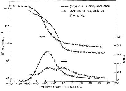
Fig. 5—E' and tan  $\delta$  vs temperature.
