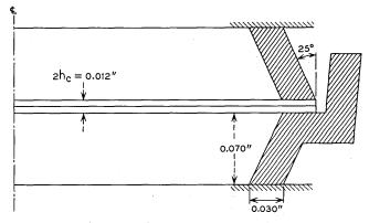
Fig. 3-Conical washer configuration.
