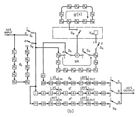
Fig. 6b—A complete serial encoder for the (30,20) code.
