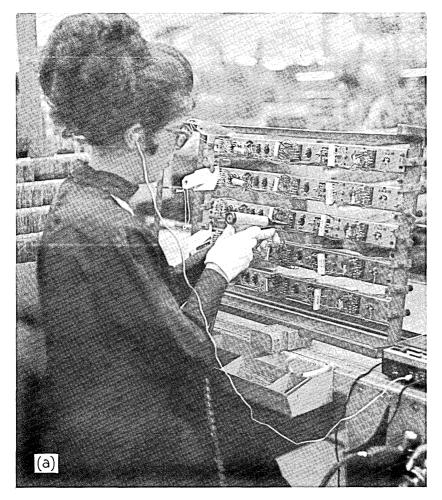
Fig. 3a—Wireman on production line at Western Electric Company plant in Oklahoma City. The wireman is fabricating crossbar-4 equipment from the computer-spoken wire list.
