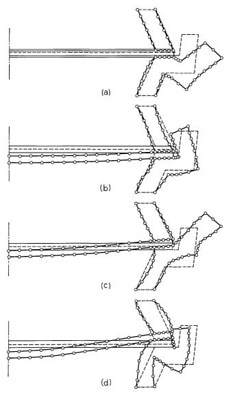
Fig. 9a—Resonant mode shape,  $f_0 = 2250$  Hertz,  $E_R = 40 \times 10^6$  dynes/cm<sup>2</sup>. Fig. 9b—Resonant mode shape,  $f_0 = 2700$  Hertz,  $E_R = 40 \times 10^6$  dynes/cm<sup>2</sup>. Fig. 9c—Resonant mode shape,  $f_1 = 5400$  Hertz,  $E_R = 60 \times 10^6$  dynes/cm<sup>2</sup>. Fig. 9d—Resonant mode shape,  $f_2 = 8500$  Hertz,  $E_R = 80 \times 10^6$  dynes/cm<sup>2</sup>.
