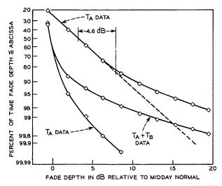
Fig. 26—4-GHz fade depth distribution, 1966 West Unity, probabilities for measurement intervals  $T_A$  (0.78  $\times$  10<sup>6</sup> seconds),  $T_B$  (4.48  $\times$  10<sup>6</sup> seconds), and  $T_A + T_B$  (5.26  $\times$  10<sup>6</sup> seconds).
