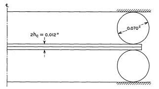
Fig. 2—"O"-ring support configuration.
