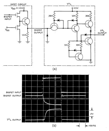
Fig. 6—(a) Circuit schematic of BIGFET-T<sup>2</sup>L interface. (b) Typical waveforms for BIGFET-T<sup>2</sup>L interface.
