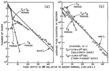
Fig. 29a-6-GHz number of fades for the entire test period. Fig. 29b-6-GHz average fade duration for the entire test period.
