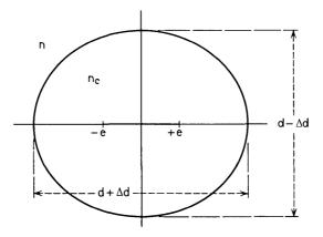
Fig. 2-Cross section of elliptically deformed fiber.
