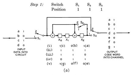
Fig. 5a—Encoding for a (7,4) block cyclic code with generator function  $g(X) = 1 + X^2 + X^3.$
