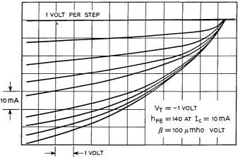
Fig. 2-BIGFET current-voltage characteristics.
