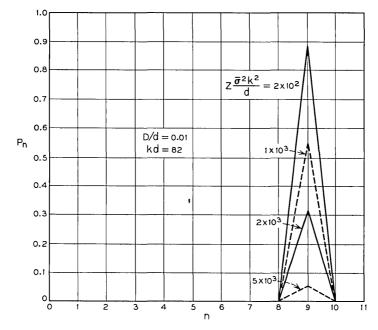
Fig. 10—Power distribution versus mode number for several values of the normalized distance along the guide. Only mode 9 is excited at z = 0. D/d = 0.01.
