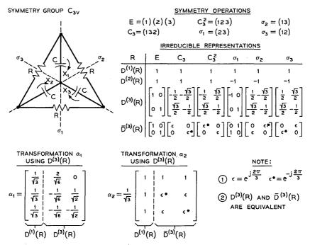
Fig. 3—Network with  $C_{3*}$  symmetry, including symmetry operations, irreducible representations, and transformation matrix  $\alpha$ .
