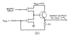
Fig. 7—Circuit schematic for BIGFET-T<sup>2</sup>L (CDI) interface: (a) resistor ladder output. (b) single emitter resistor.
