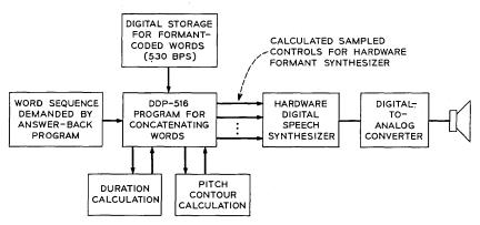
Fig. 2—DDP-516 computer system for automatic synthesis of spoken wiring instructions.
