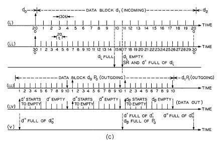
Fig. 6c-Timing diagram for encoder shown in Fig. 6b.
