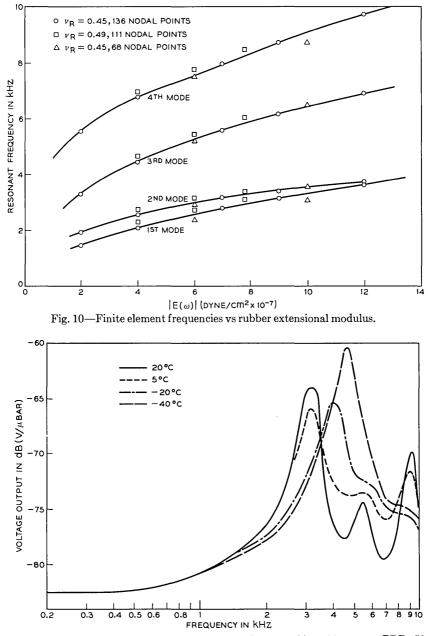
Fig. 11—Frequency response vs temperature change, rubber: 50 percent PBD, 50 percent SBR.
