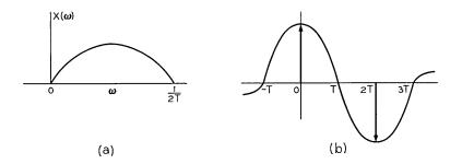
Fig. 2-Class IV partial response: (a) spectrum; (b) sampled impulse response.
