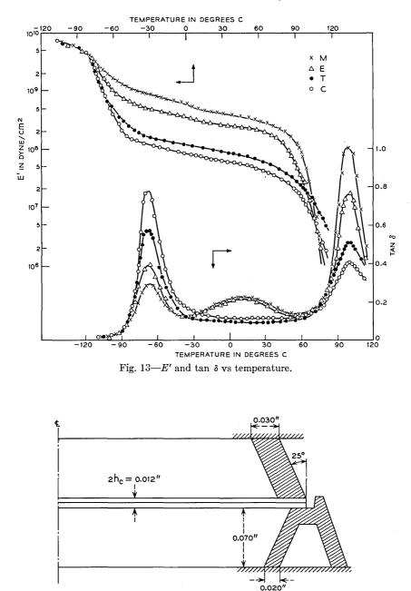
Fig. 14-Modified conical washer design.
