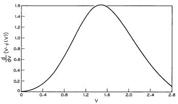
Fig. 4—The normalized delay distortion  $d (v \cdot \psi(v))/dv$ .
