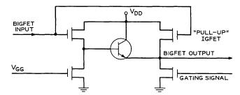
Fig. 8-IGFET "pull-up" circuit for BIGFET-IGFET interface.
