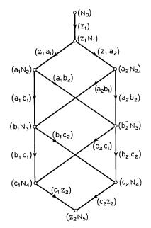
Fig. 11—Transition graph  $G^T$  corresponding to Fig. 10.
