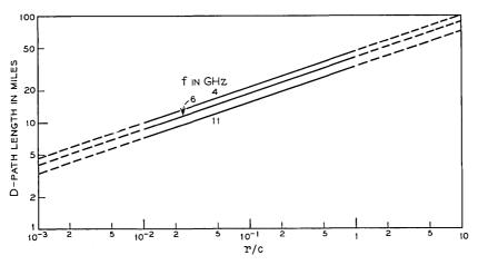
Fig. 8—Worst month multipath fading:  $P = rL^2 = c(f/4) D^3L^2$ .
