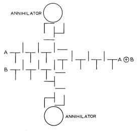
Fig. 4—Exclusive-or operation in field access propagation.
