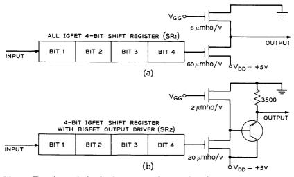
Fig. 3-Experimental circuits for comparative speed performance measurements.
