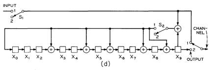
Fig. 5d—Conventional encoder configuration for the (30,20) code with same generator used in Fig. 5c.
