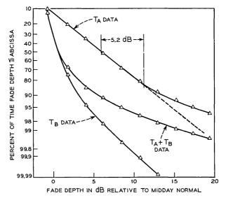
Fig. 27—6-GHz fade depth distribution, 1966 West Unity, probabilities for measurement intervals  $T_A$  (0.78 × 10<sup>6</sup> seconds),  $T_B$  (4.48 × 10<sup>6</sup> seconds), and  $T_A + T_B$  (5.26 × 10<sup>6</sup> seconds).
