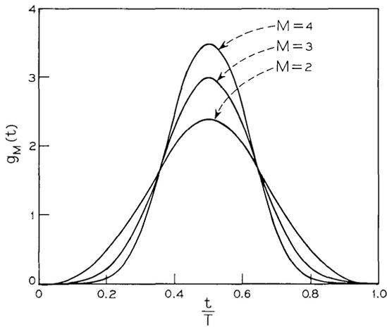
Fig. 9 — Time response of the Class III weighting functions.
