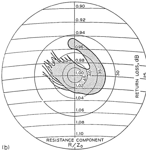
Fig. 16—Return loss for the  $8 \times 8$  array from dc to 100 MHz: (a) with 8200-ohm shunt resistance, (b) with 2740-ohm shunt resistance.
