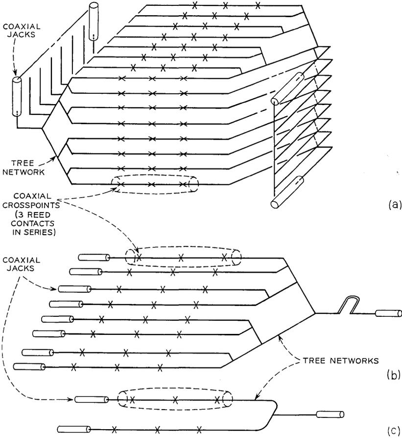
Fig. 1 — Array schematic: (a)  $8 \times 8$ , (b)  $1 \times 8$ , (c)  $1 \times 2$ .
