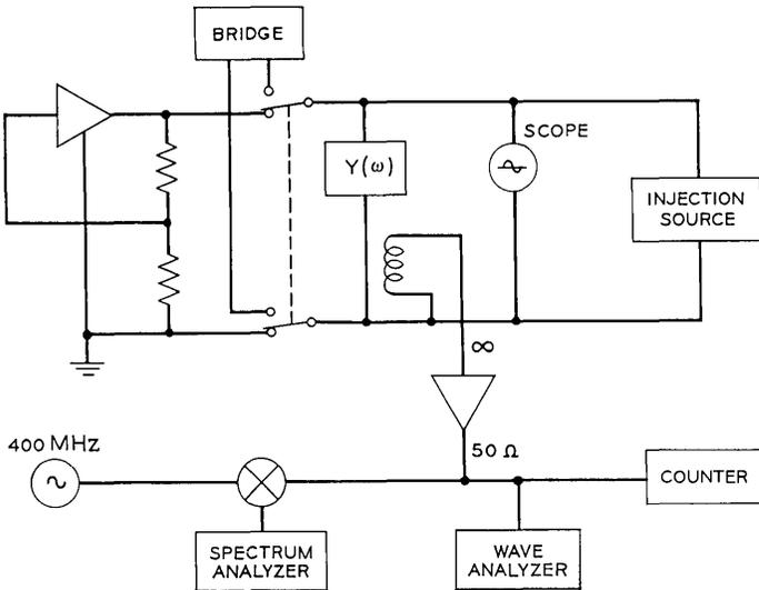
Fig. 5 — Schematic of low-frequency experiment.
