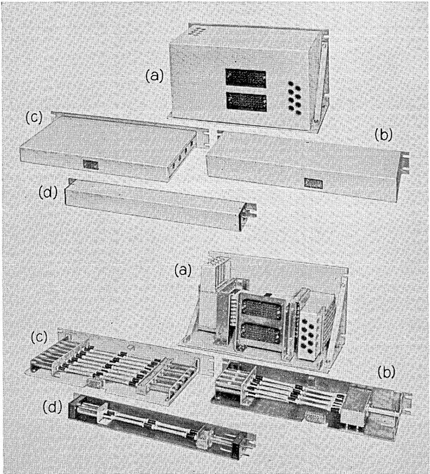
Fig. 2—Photograph of switch arrays: (a) 8 × 8, (b) 1 × 8, (c) 1 × 2 (4 switches per package), (d) 1 × 2 (1 switch).
