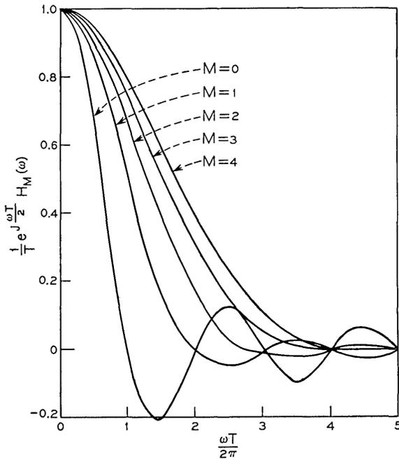
Fig. 2 — Spectra of the Class I weighting functions.
