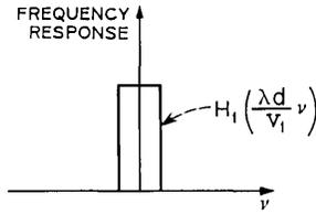
Fig. 4 — Frequency response of the filter  $H_1[(\lambda d/v_1)\nu]$ .
