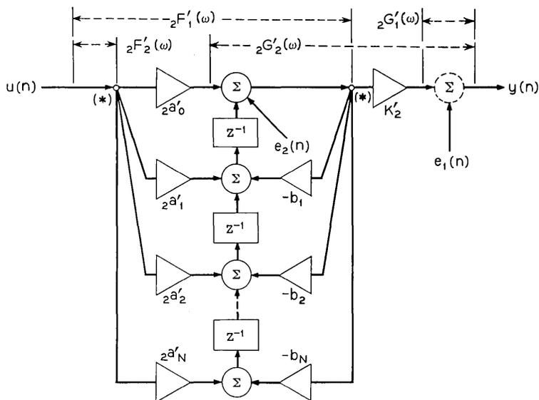
Fig. 4 — Direct form 2 with scaling.
