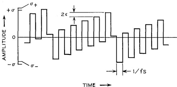
Fig. 1—Asymmetrical integrator output for an idle-channel input, shown for  $|\sigma_+| > |\sigma_-|$ .
