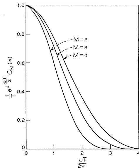
Fig. 7—Spectra of the Class III weighting functions.
