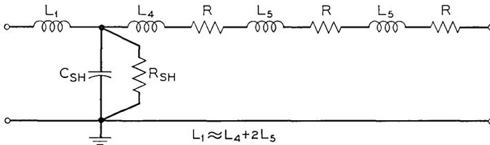
Fig. 13 — Low-frequency approximation of a tuned path through a  $1 \times 8$  matrix. ( $L_1$ ,  $L_4$ ,  $L_5$  = equivalent inductance of high impedance transmission lines;  $C_{SH}$  = equivalent lumped capacitance of open-circuited stubs;  $R$  = contact resistance of the 237G contact;  $R_{SH}$  = shunt resistance to adjust real-part of input impedance.)
