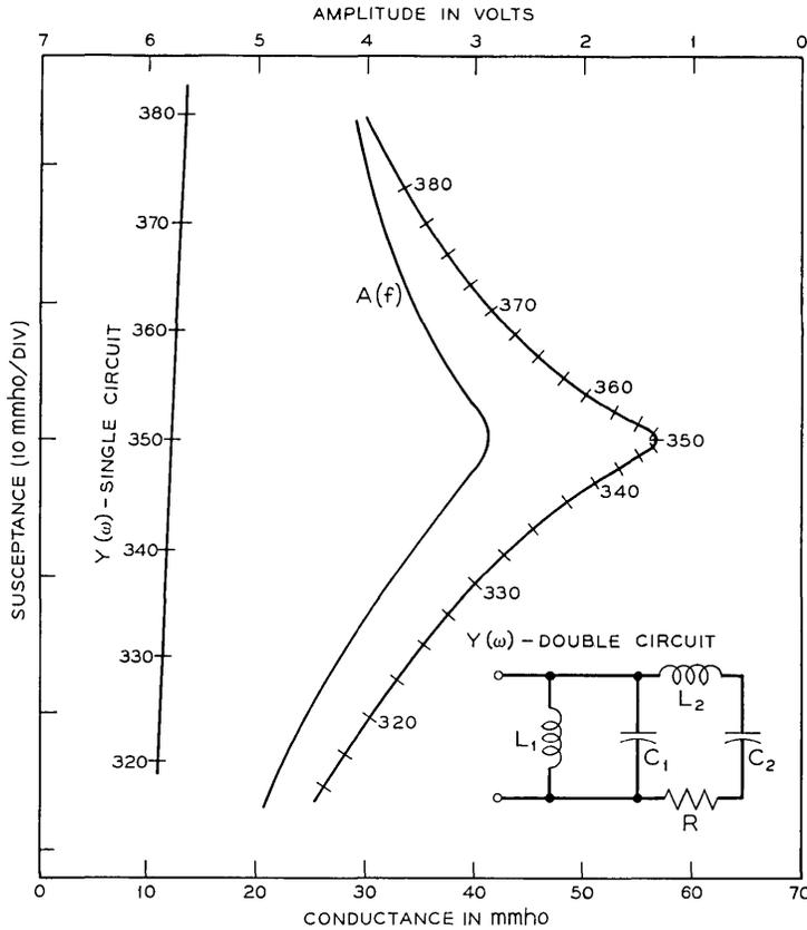
Fig. 9 — Double-tuned circuit behaviour.
