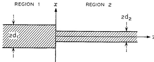
Fig. 2 — Abrupt step in a dielectric slab waveguide.
