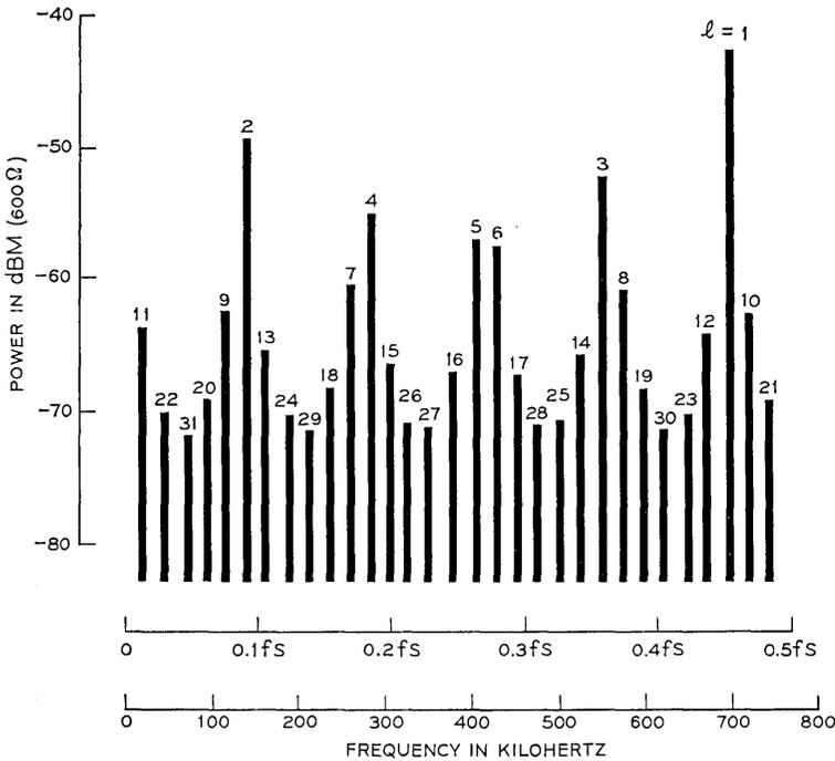
Fig. 4 — Calculated idle-channel noise spectrum,  $f_s = 1.56$  MHz,  $\vartheta = 0.0937$ .
