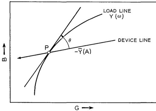
Fig. 1 — Definition of  $\theta$  at oscillation point.
