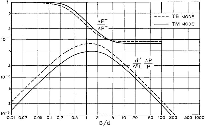
Fig. 9 — Comparison of TM loss (solid line) and TE loss (dotted line) caused by a random distortion of one waveguide wall.  $B$  = correlation length,  $A$  = r.m.s. wall distortion,  $d$  = half width of slab,  $L$  = length of distorted guide section.  $n = 1.5, kd = 1.3$ .
