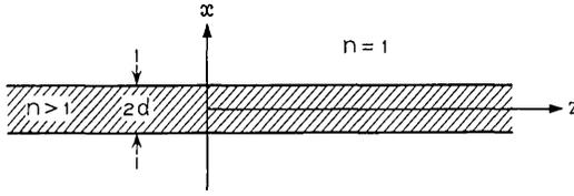
Fig. 1 — Dielectric slab waveguide.
