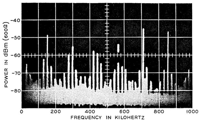
Fig. 2 — Observed idle-channel noise spectrum,  $f_s = 1.56$  MHz,  $\vartheta = 0.0937$ .
