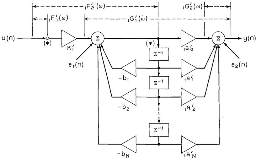
Fig. 3 — Direct form 1 with scaling.
