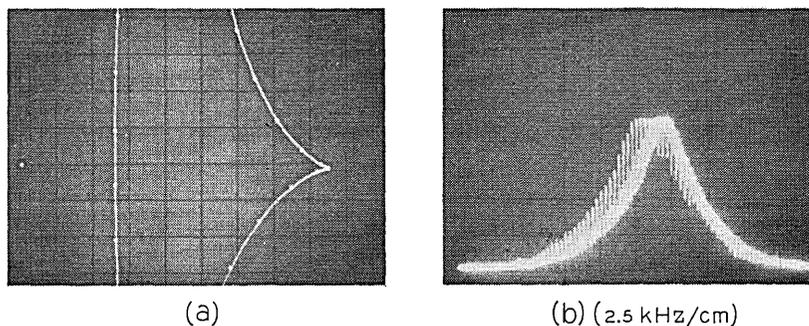
Fig. 11 — Circuit admittance for  $Q_2 = 0$  and  $Q_2 = Q_1$  cases.
