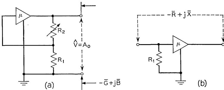
Fig. 4 — Negative admittance and impedance circuits.
