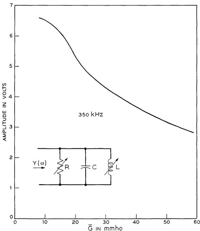
Fig. 7 — Conductance saturation curve at 350 kHz.
