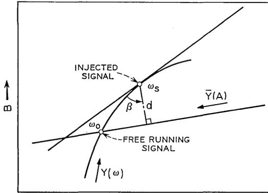
Fig. 3 — Injection locking conditions.
