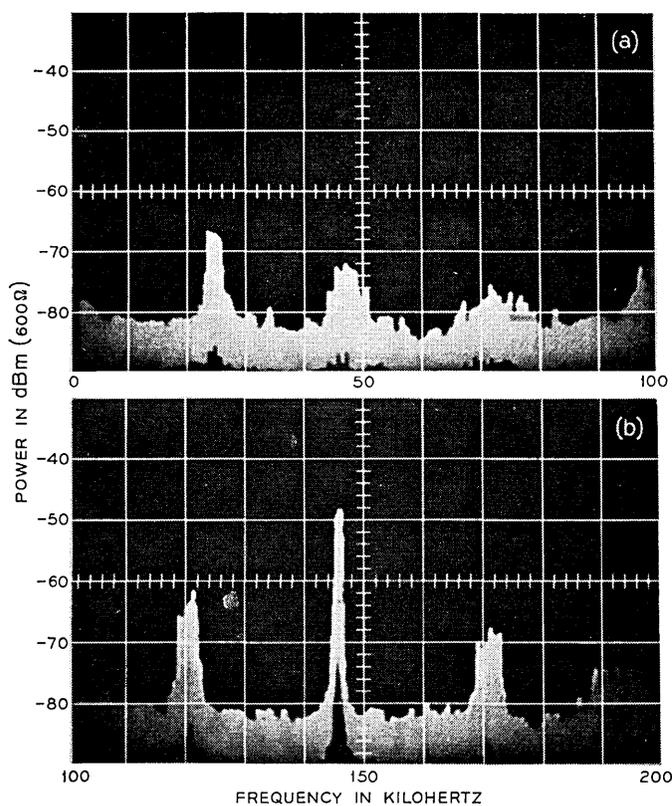
Fig. 3 — Expanded idle-channel noise spectrum: (a) 0 — 100 kHz, (b) 100 — 200 kHz.
