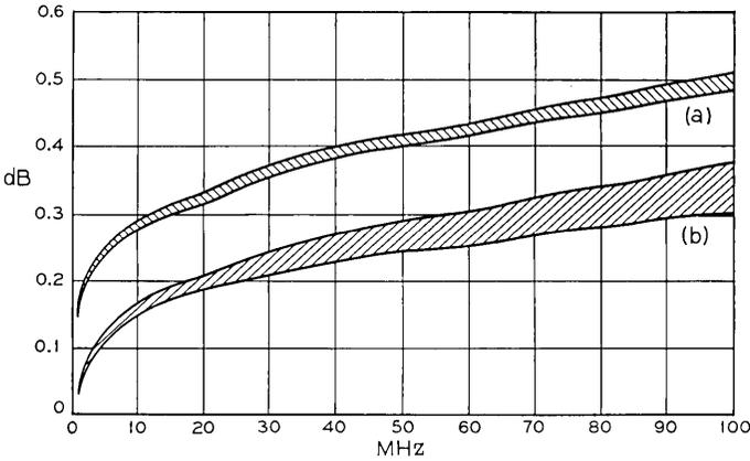
Fig. 20—Insertion loss from dc to 100 MHz: (a)  $1 \times 8$  array, (b)  $1 \times 2$  array.
