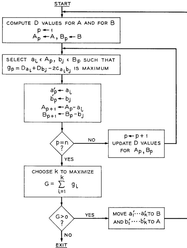
Fig. 1 — Flowchart of phase 1 optimization procedure.
