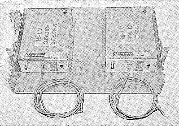
Fig. 40 — Transmitting bay—power separation filter shelf.
