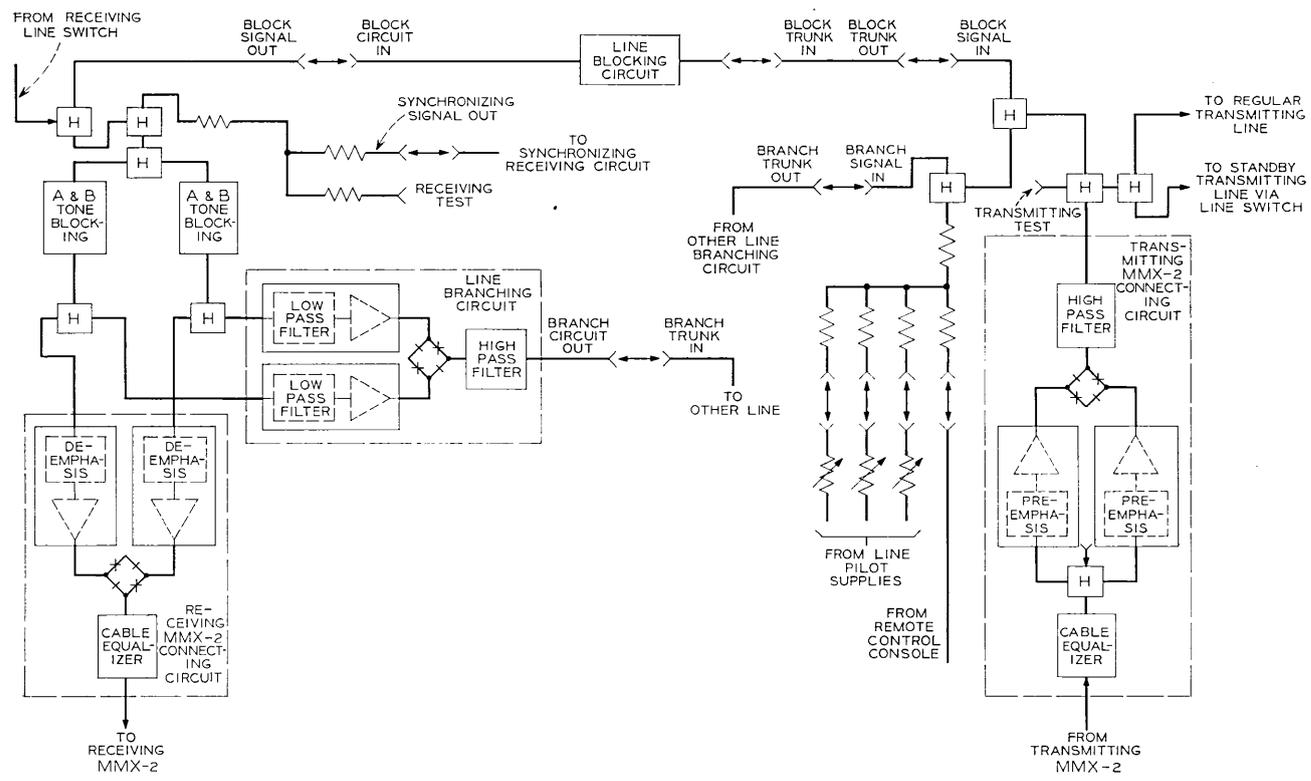
Fig. 16 — Line connecting circuits.
