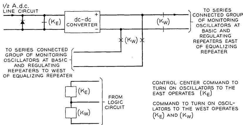
Fig. 23 — Monitoring oscillator power and switching circuit.
