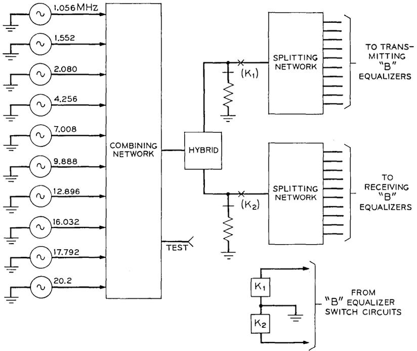
Fig. 35 — B test oscillator and oscillator connecting circuit.
