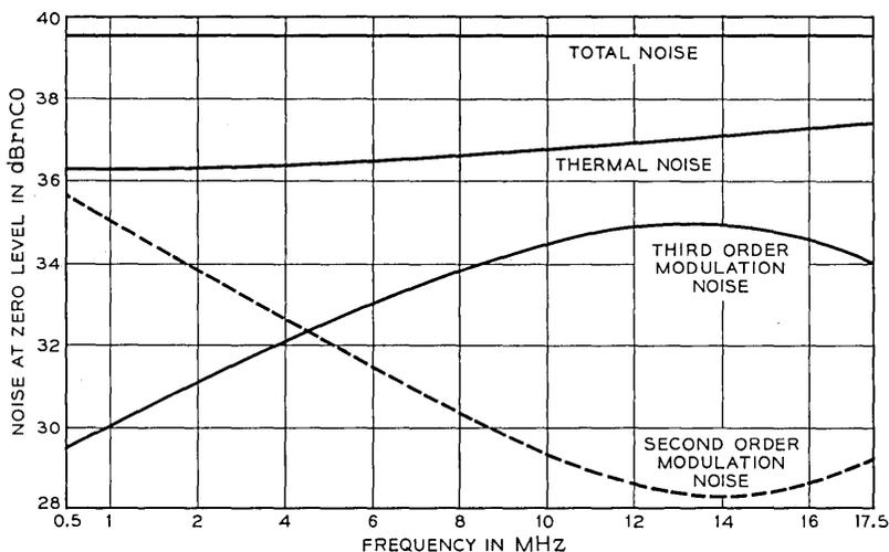
Fig. 4—Zero level message channel noise for 4,000-mile L-4 high-frequency line.
