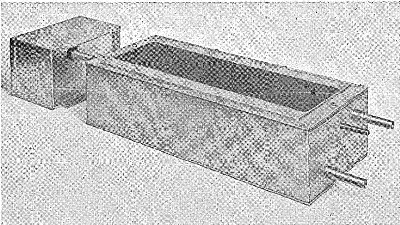
Fig. 3 — Basic repeater assembly with line build-out network (at left) detached.
