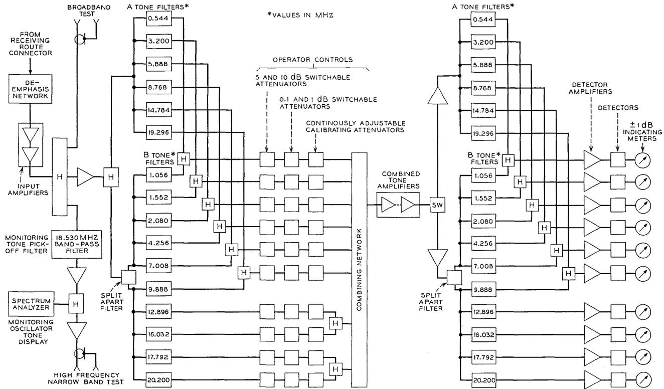
Fig. 4—Receiving circuit block diagram.
