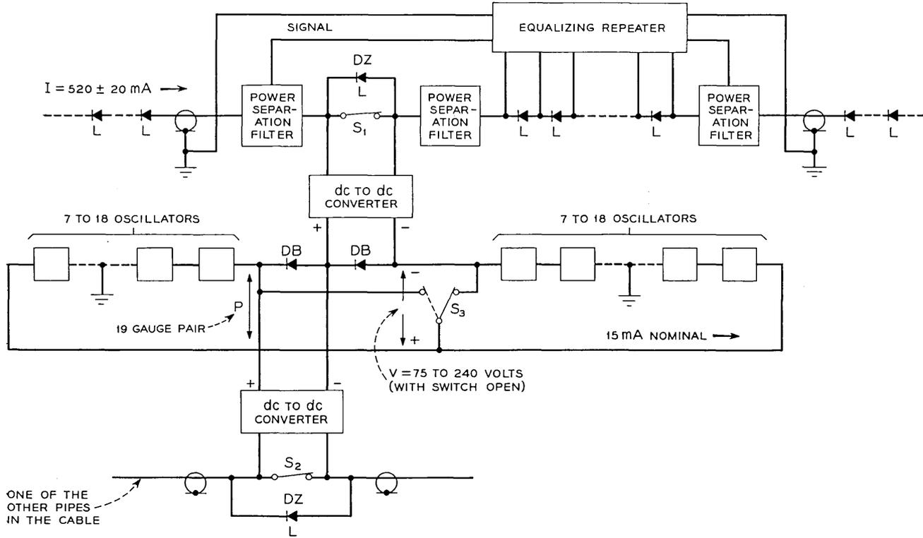
Fig. 6 — Monitoring oscillator power arrangements.
