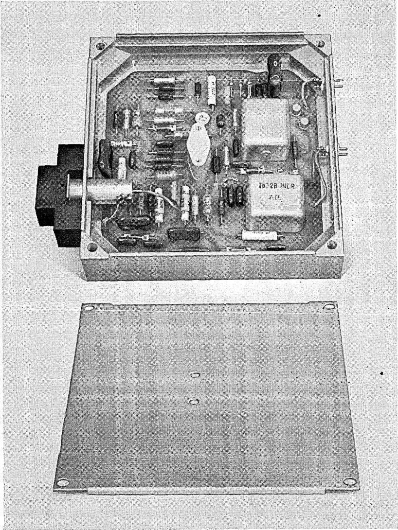
Fig. 4 — Top view of preamplifier with cover removed.
