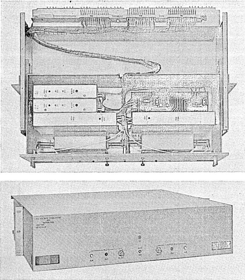
Fig. 49— 512 kHz pilot stabilization and distribution unit. Top view (top) and front view.
