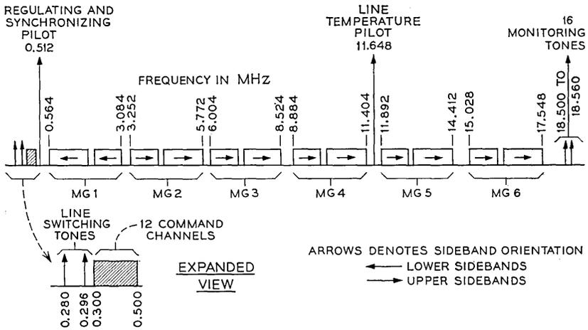
Fig. 1 — L-4 frequency allocations.
