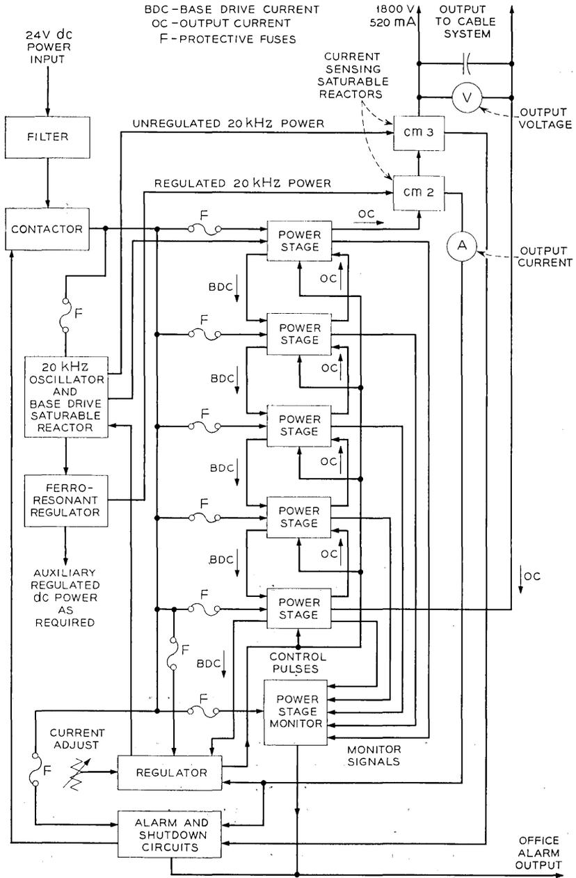
Fig. 4 — Power converter block diagram.
