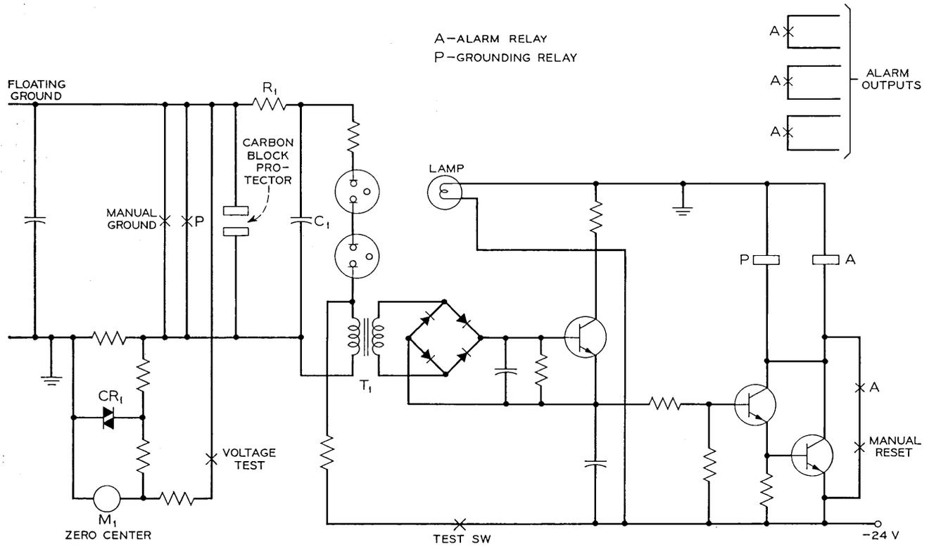
Fig. 2 — Ground circuit simplified schematic.
