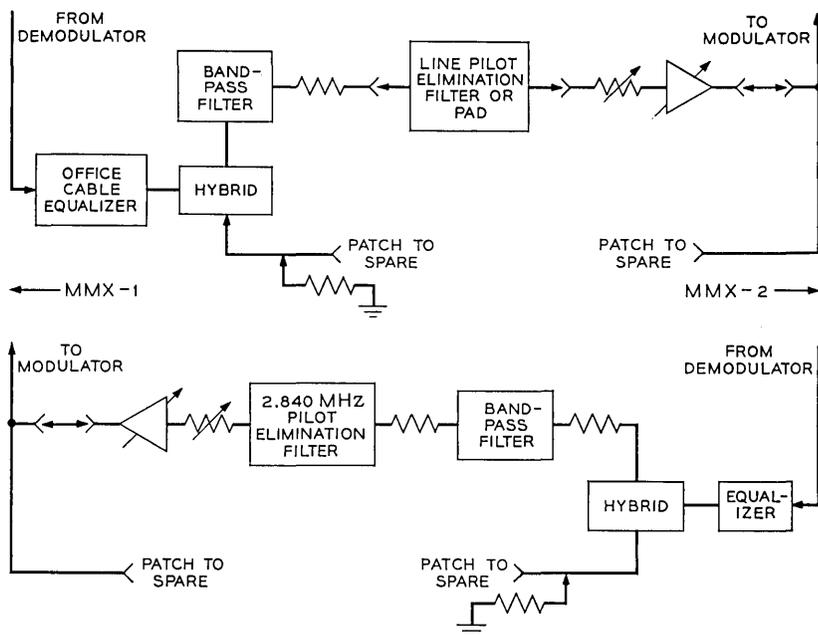
Fig. 20—Mastergroup connector, MMX-1 to MMX-2 (two-way).
