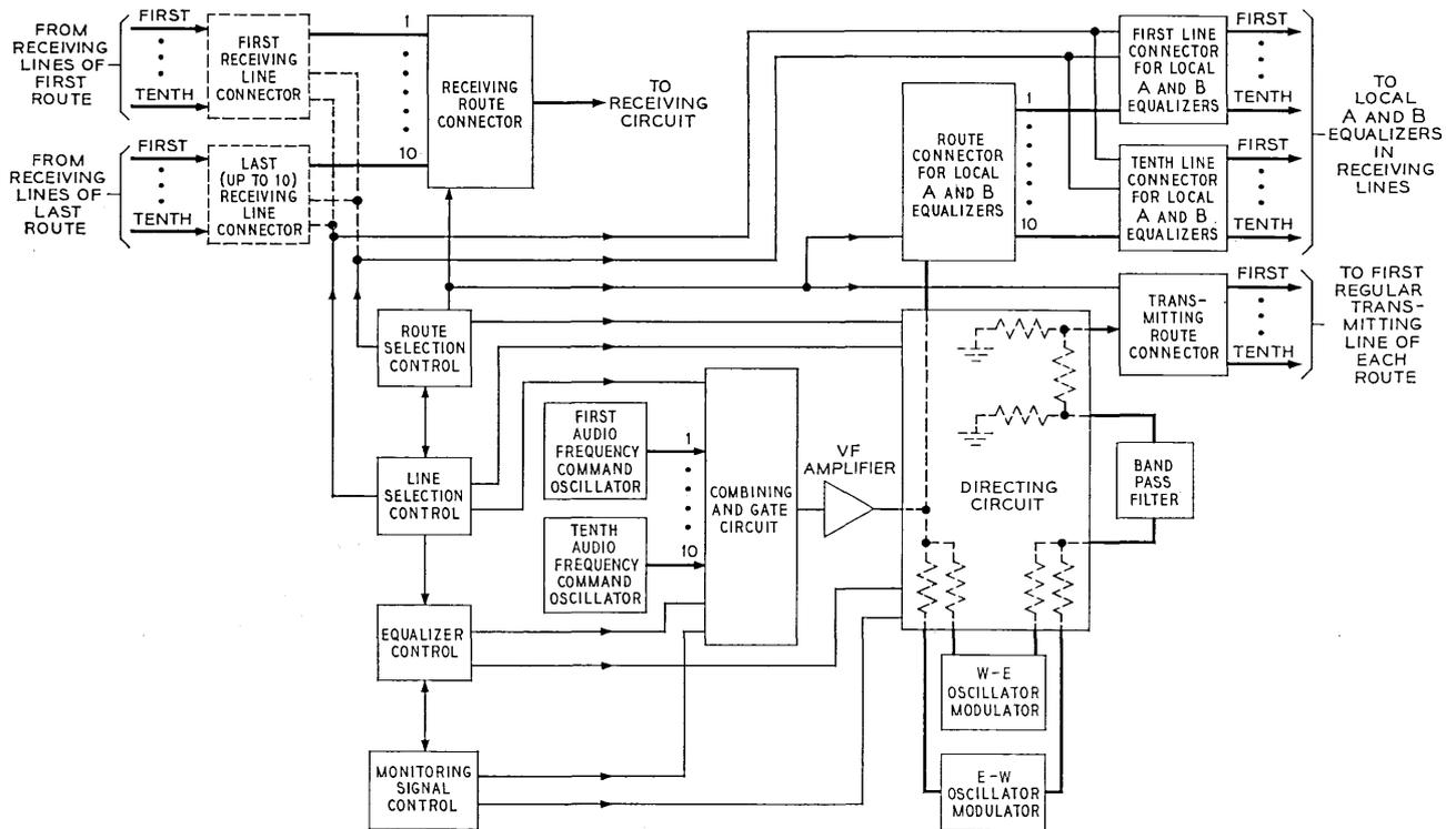
Fig. 3—Sending circuit block diagram.
