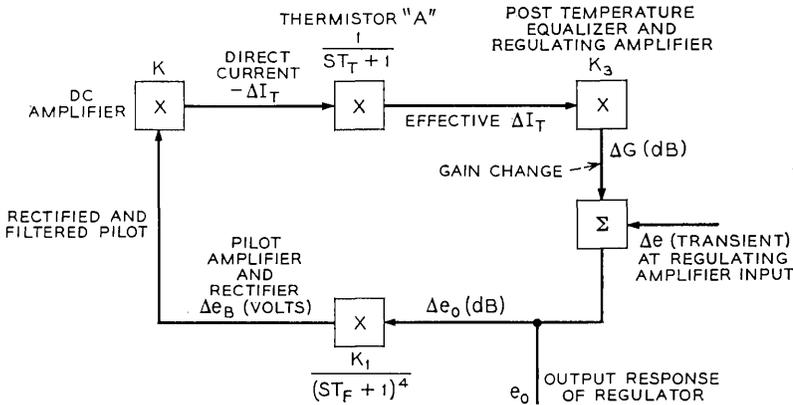
Fig. 35 — Mathematical model of the pilot-controlled postregulator.
