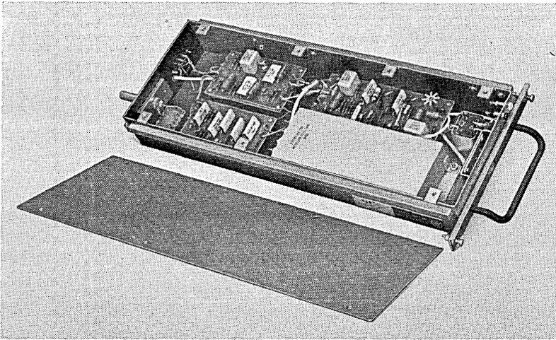
Fig. 27 — Command receiver assembly.
