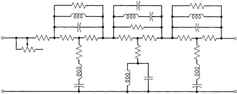
Fig. 18 — Configuration of the A trim equalizer.
