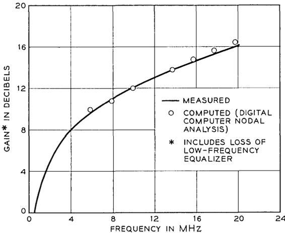
Fig. 9 — Measured and computed insertion gain of pre-amplifier.
