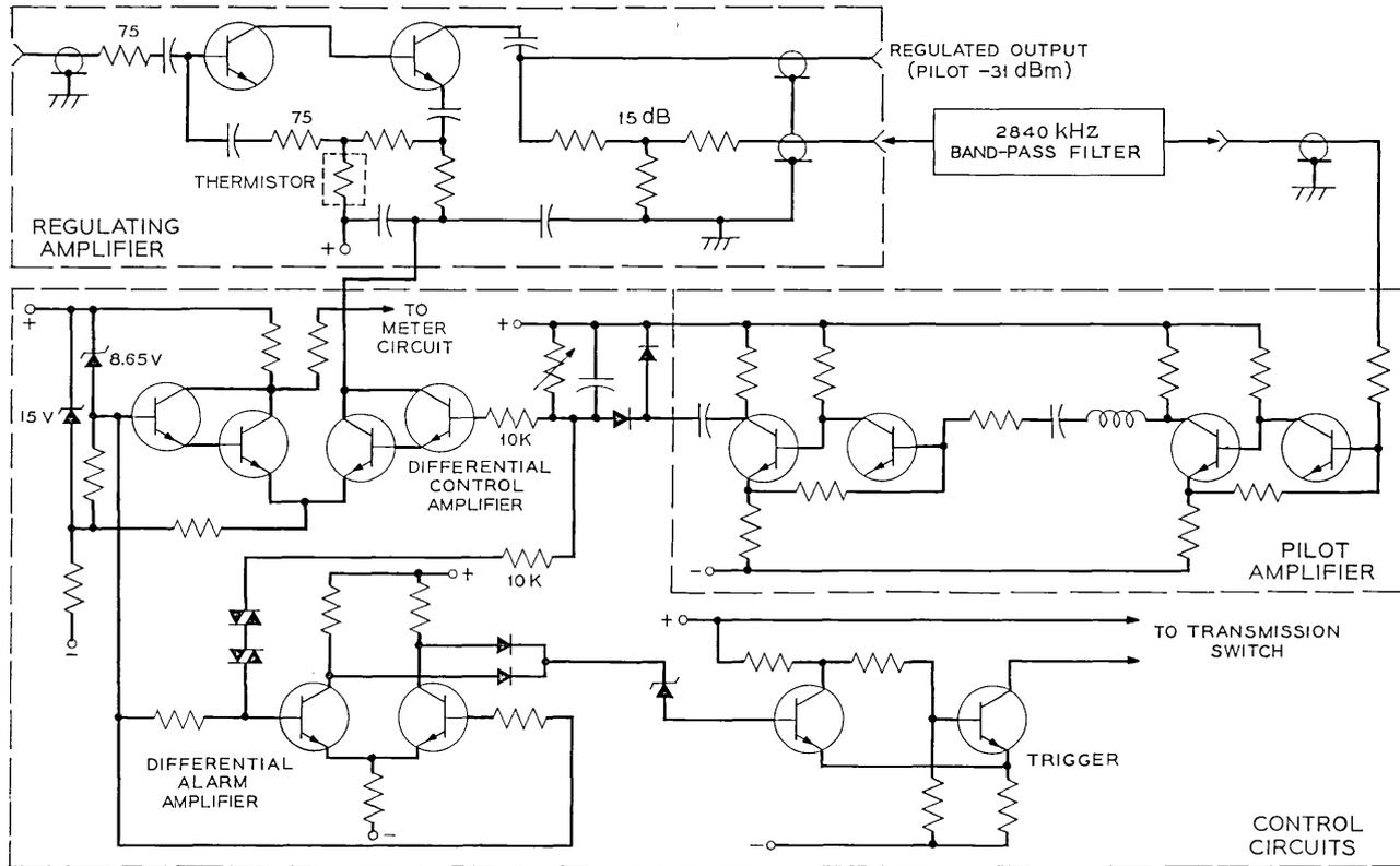
Fig. 5—Mastergroup transmission regulator circuit.
