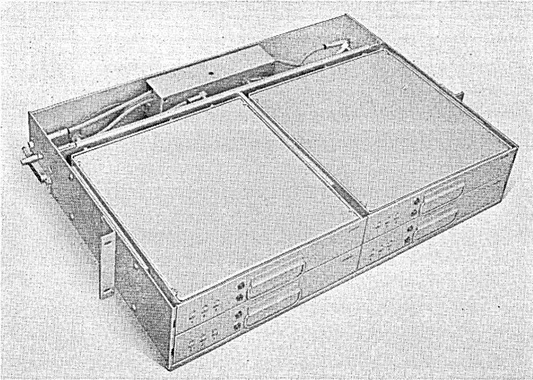
Fig. 43 — B equalizer assembly.
