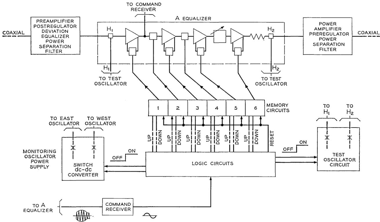
Fig. 1 — Functional block diagram of the equalizing repeater.
