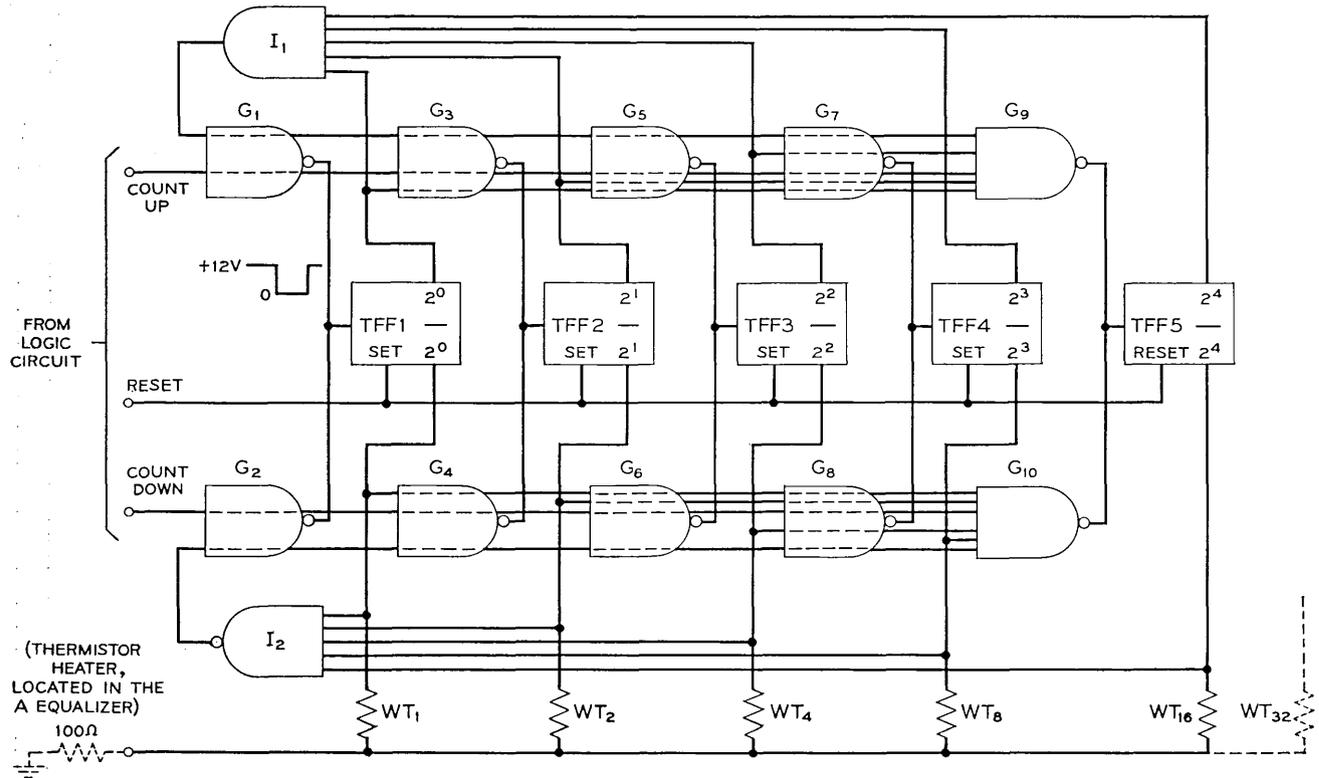
Fig. 22 — Memory circuit for the equalizers. This circuit is used throughout the system for the control of A and B equalizer settings.
