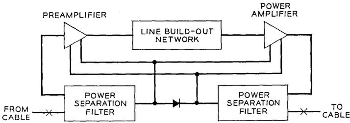
Fig. 1 — Simplified block diagram of basic repeater.
