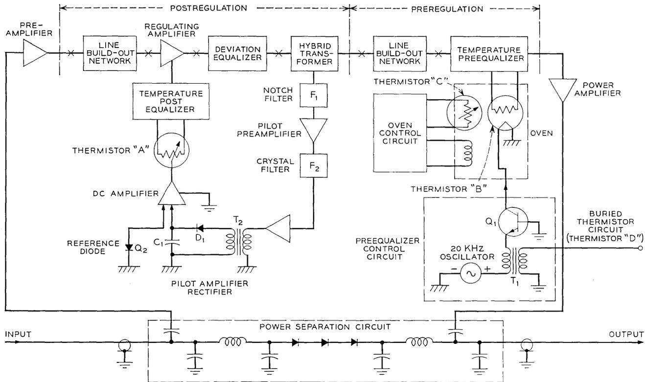
Fig. 19 — Complete block diagram of regulating repeater.
