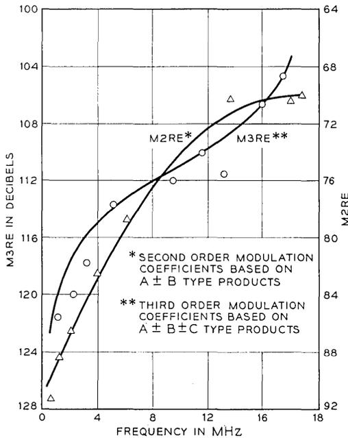
Fig. 12 — Second and third order modulation coefficients for power amplifier.
