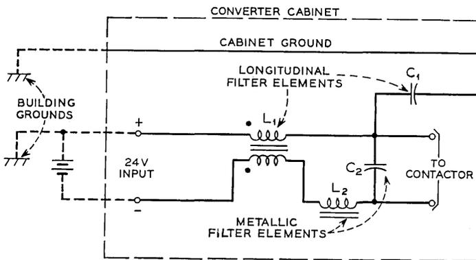
Fig. 5 — Input filter circuit.
