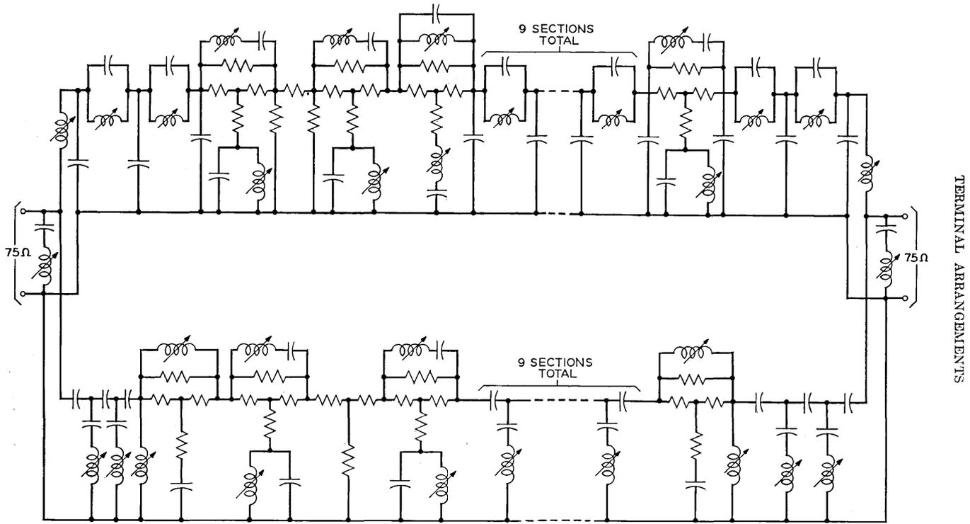
Fig. 17 — Schematic of typical mastergroup blocking filter arrangement.
