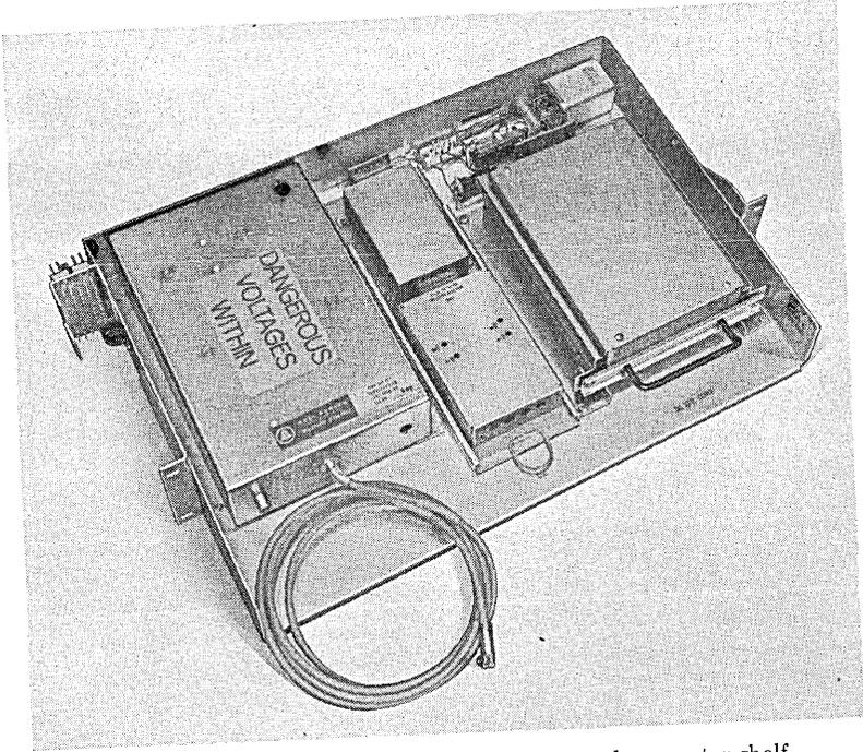
Fig. 46 — Receiving bay—power separation and converter shelf.
