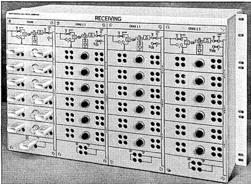
Fig. 11 — MMX-2 receiving patch and test unit.
