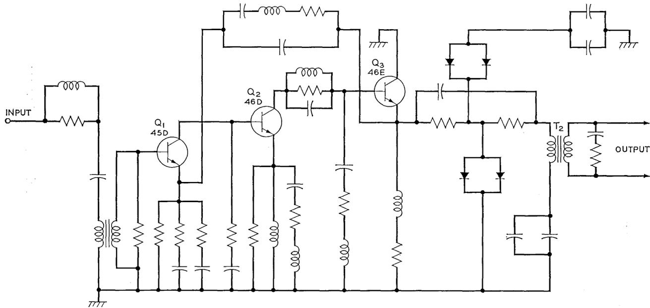
Fig. 11 — Schematic diagram of power amplifier (less bias circuitry).
