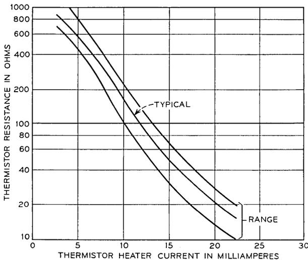
Fig. 16 — Thermistor *R-I* characteristics. Shown are the typical, maximum, and minimum characteristics.
