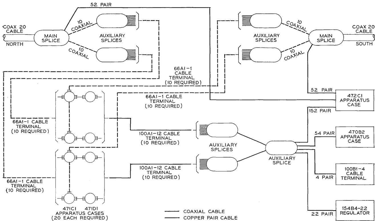
Fig. 15 — L-4 equalizing station schematic.
