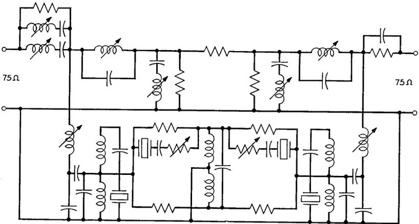
Fig. 19—Schematic of typical low frequency A- or B-tone band-elimination filter.
