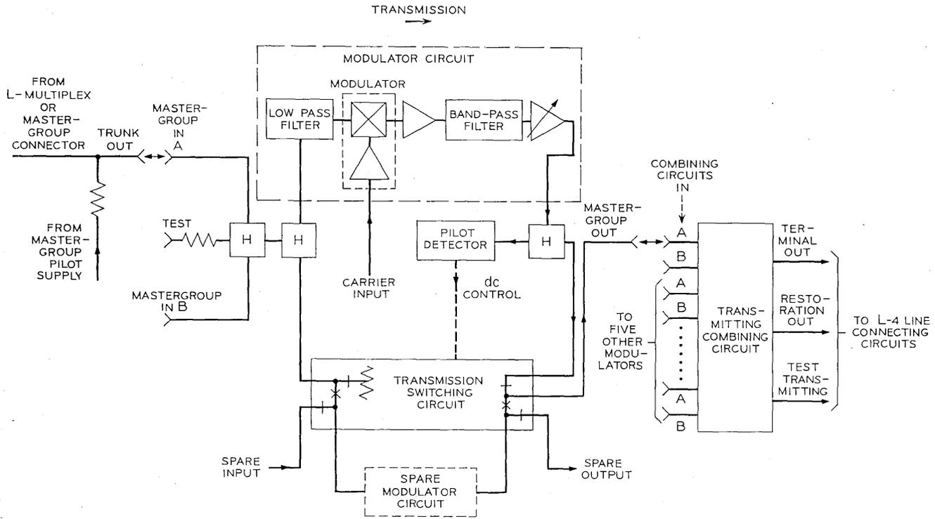
Fig. 4 — MMX-2 transmitting circuits.
