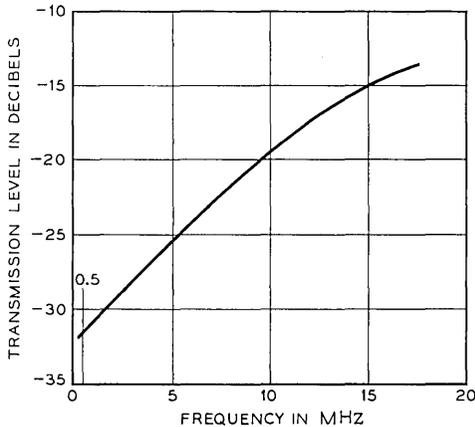
Fig. 5 — Transmission level at repeater output.
