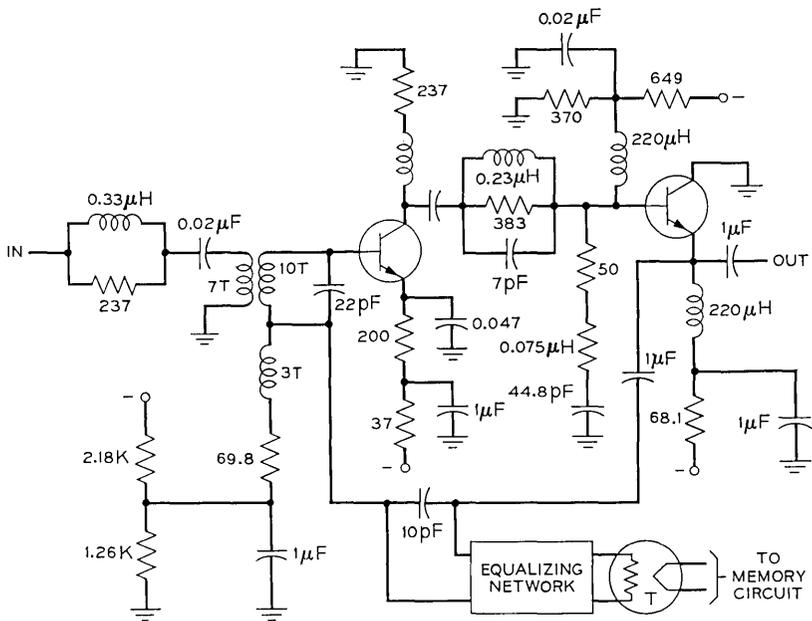
Fig. 8—Schematic diagram of a typical equalizer amplifier. The circuit shown is that of  $A_4$  in Fig. 6.
