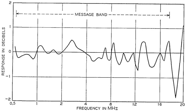
Fig. 52 — Response of L-4 main section after the adjustment of the A and B equalizers.
