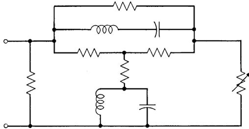
Fig. 15 — Ideal A equalizer Bode section.
