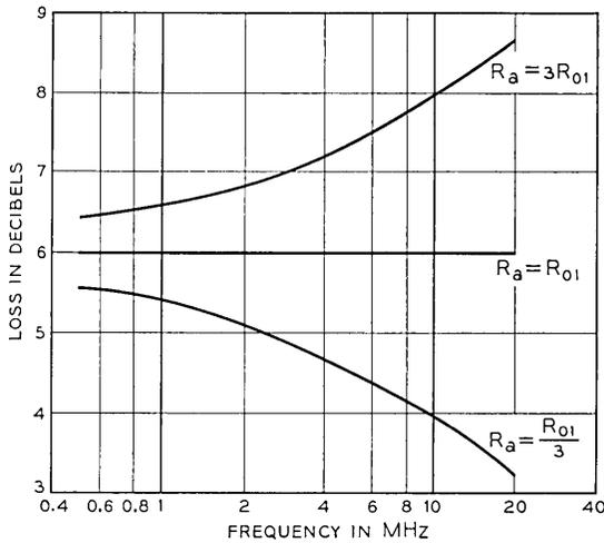
Fig. 25 — Insertion loss characteristic of preregulator network.
