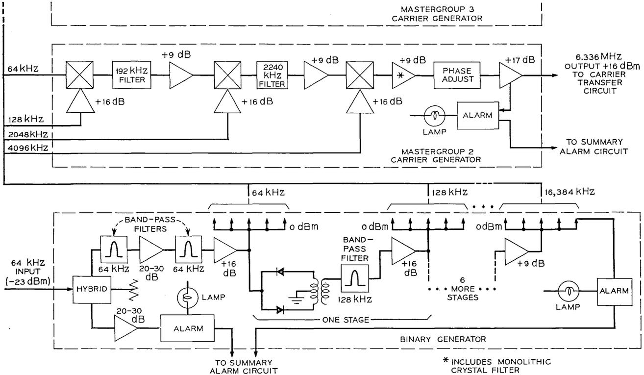
Fig. 6 — Carrier supply circuits.
