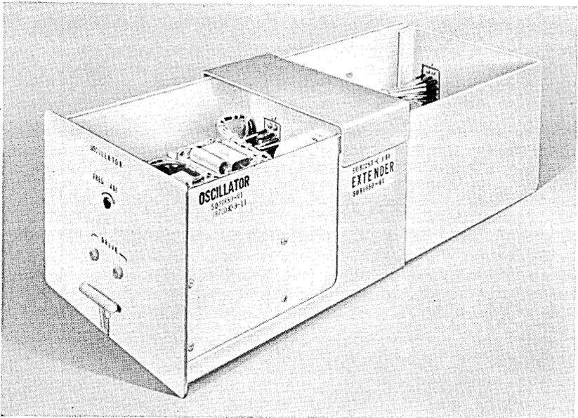
Fig. 9—Extender for oscillator and converter (power stage) units—oscillator in position.
