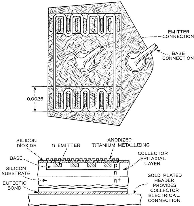
Fig. 1 — The 45D transistor.
