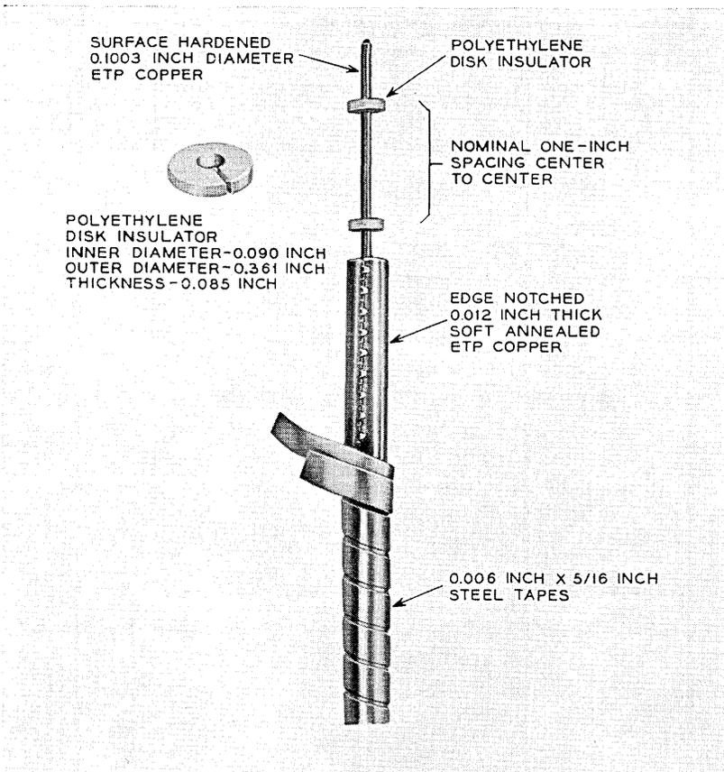
Fig. 1—Air dielectric disk-insulated 0.375 inch serrated-seam coaxial.
