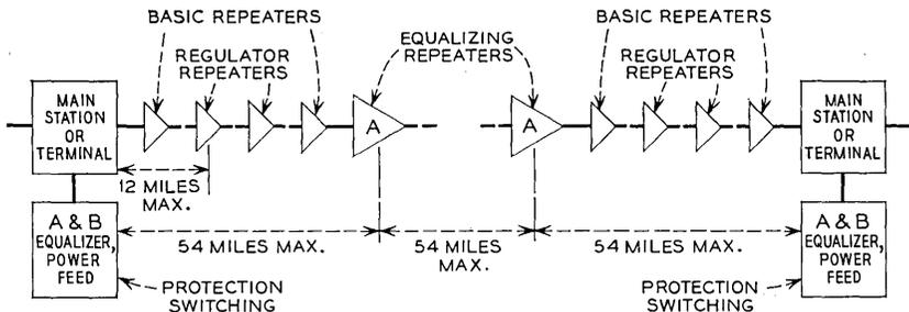
Fig. 2 — Typical L-4 repeated line layout: maximum distance between main stations is 150 miles.
