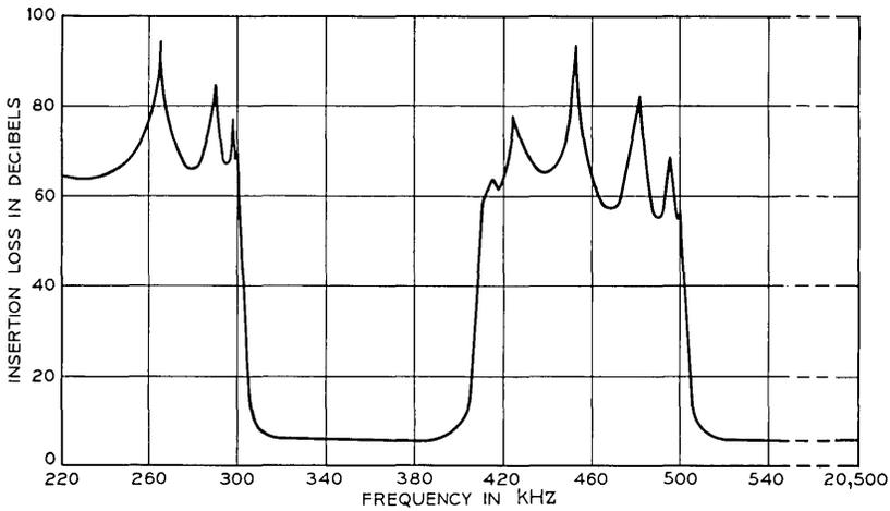
Fig. 18 — Command and line switching tone blocking filter.
