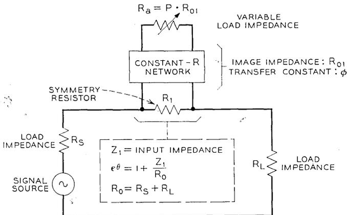
Fig. 23 — Series-type Bode regulator network.
