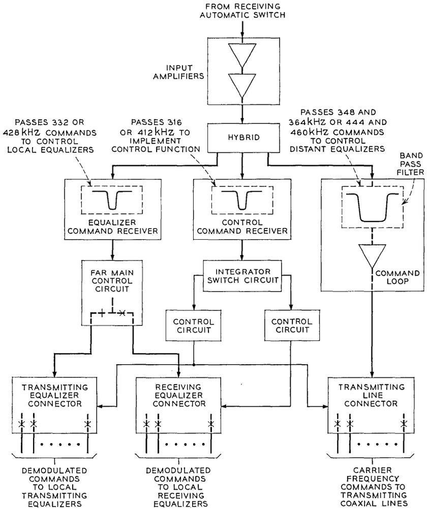
Fig. 5 — Loop-back circuit for unattended main station.
