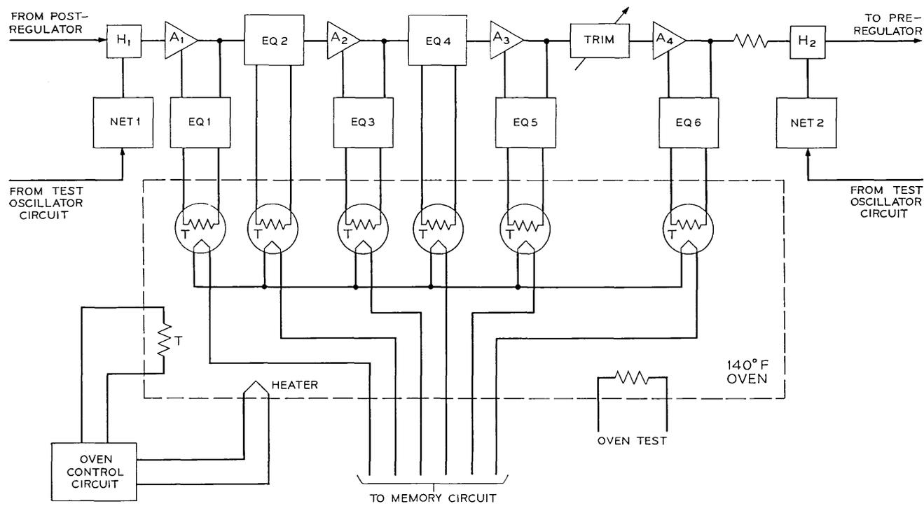
Fig. 6—Block schematic diagram of the A equalizer. For clarity the two ovens and oven control circuits actually used are shown as one.
