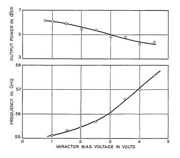
Fig. 3 - Performance of the varactor-tuned oscillator.
