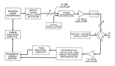
Fig. 6 — Circuit block diagram for the error rate measurement.
