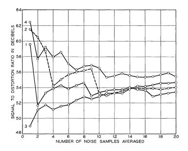
Fig. 8—Fluctuations in SDR of single pole filter as a function of number of sets of computations. Ten sine waves in baseband; SDR computer in slot 4; bandwidth expansion factor k = 10;  $\sigma = 0.2$  MHz;  $\omega_c/W = 1.223$ .
