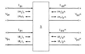
Fig. 2—Small-signal terminal behavior of a harmonic generator of order 2". m is the AM index and  $\theta$  is the PM index of the multiplier.
