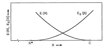
Fig. 11—Typical behavior of  $E_s(R)$  and E(R) near their zero value.
