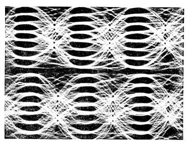
Fig. 16 — Bilateral pulse transmission over phase-linearized NIB line.
