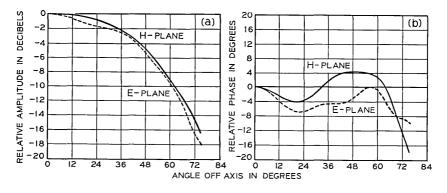
Fig. 2 – Subreflector illumination,  $TE_{11}$  and  $TM_{11}$  modes, freq. =  $f_0$ .
