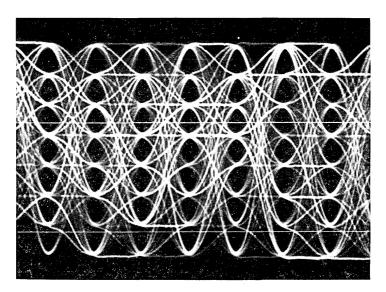
Fig. 15 — Eight-level pulses received over phase-linearized NIB line.
