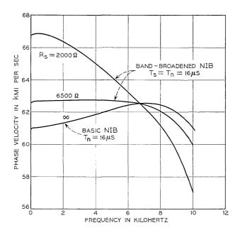
Fig. 14 — Effect of band broadening upon phase velocity of NIB line; 22-gauge BSA cable, 12,000-foot spacing.
