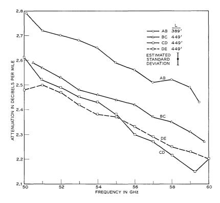
Fig. 3 — Measured attenuation of short length waveguide sections.
