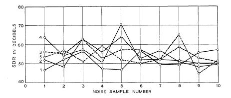
Fig. 9—FM SDR in a single pole filter. 50 sine waves in baseband; SDR computed in slot 19; bandwidth expansion factor k = 10;  $\sigma = 0.2$  MHz;  $\omega_o/W = 1.223$ .
