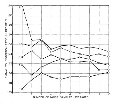
Fig. 11 — Fluctuations in SDR of single pole filter as a function of number of sets of computations. 50 sine waves in baseband; SDR computed in slot 19; bandwidth expansion factor k = 10;  $\sigma = 0.2$  MHz;  $\omega_c/W = 1.223$ .
