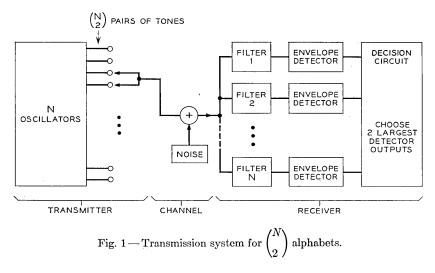
signal out is M simultaneous pulses of energy, one pulse on each of M distinct frequencies, lasting for T seconds. White gaussian noise is added in the channel. Filters, matched to the pulse shape, are tuned to each of the N possible frequencies. The filter outputs are envelope-detected and all N envelope samples are intercompared at the end of the pulse period. The largest M of these outputs determine the transmitted character.\*
