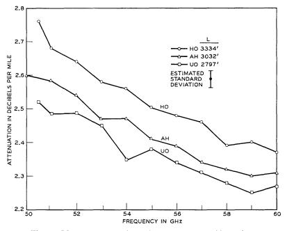
Fig. 5 — Measured attenuation of long length waveguide sections.
