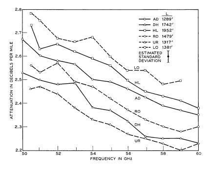
Fig. 4 - Measured attenuation of medium length waveguide sections.
