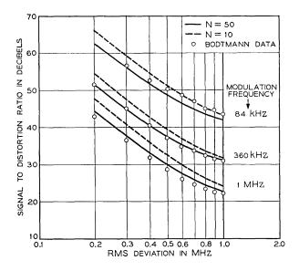
Fig. 5 — Bodtmann's measured results compared with noise samples.
