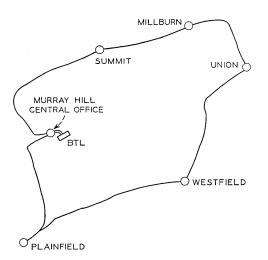
Fig. 9 — Cable route in field test of negative impedance boosting. The line was 32 miles long, mostly buried 22 gauge cable, and it had 16 NIB sections.
