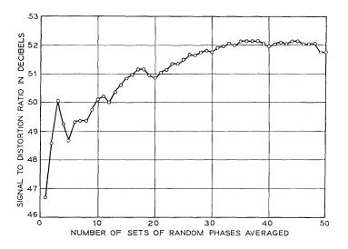
Fig. 10 — Fluctuations in SDR of single pole filter as a function of number of sets of computations. 50 sine waves in baseband; SDR computed in slot 19; bandwidth expansion factor k = 10;  $\sigma = 0.2$  MHz;  $\omega_c/W = 1.223$ .
