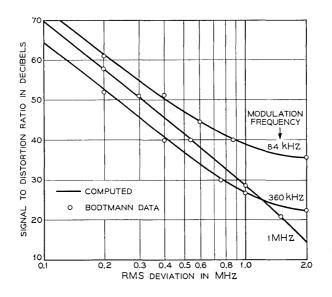
Fig. 4 — Third harmonic distortion in single pole filter.
