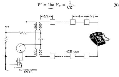
Fig. 3—Negative impedance boosted subscriber line and central office terminating circuit.
