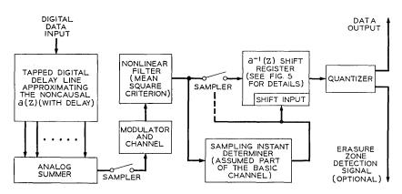
Fig. 4—One possible general arrangement for unadaptive stationary (shift-register) linear-real encoders and decoders. For multilevel signals, a Gray encoder can be used before the analog summer, and the quantizer would incorporate a Gray decoder.
