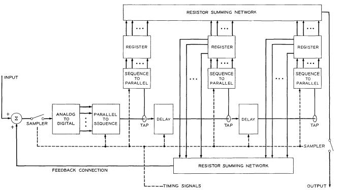
Fig. 5-A possible arrangement for implementing the decoding shift register.
