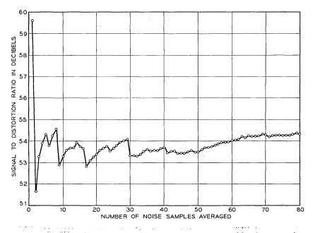
Fig. 7 — Fluctuations in SDR of single pole filter as a function of number of sets of computations. Ten sine waves in baseband; SDR computed in slot 4; bandwidth expansion factor k = 10;  $\sigma = 0.2$  MHz;  $\omega_c/W = 1.223$ .
