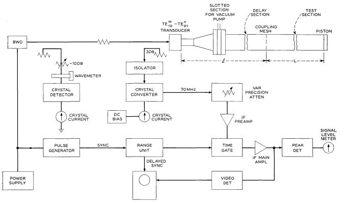
Fig. 2 — Block diagram of measuring setup.
