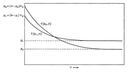
Fig. 14—Two members of the family of curves:  $f(x,n) = x + (A - x)K_2 \exp(-Bnx^2)$ .
