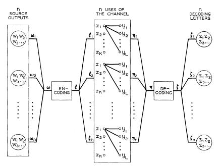
Fig. 3 — Block diagram of the encoding and decoding.
