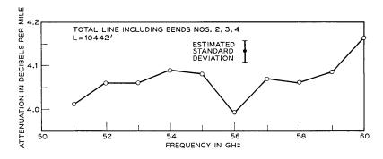
Fig. 7 — Measured attenuation of total line including bends.
