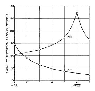
Fig. 19—FM and AM SDR in three-pole transitional Butterworth-Thomson filters. W = 7 MHz; loss 256 MHz from midband = 20 db; N = 10; k = 30; no carrier offset;  $\sigma/W = 3.12$ ; slot 10.
