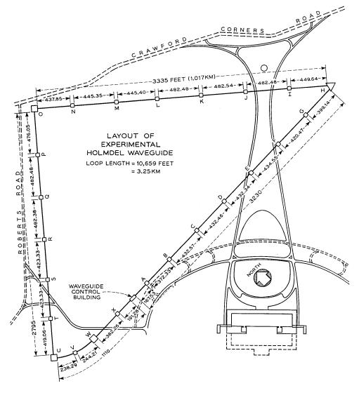
Fig. 1-Layout of experimental Holmdel waveguide.
