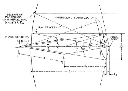
Fig. 1—Geometry of cassegrain antenna.
