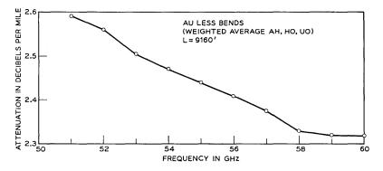
Fig. 6 - Measured attenuation of total straight waveguide.
