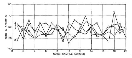
Fig. 6 – FM SDR in a single pole filter. Ten sine waves in baseband; SDR computed in slot 4; bandwidth expansion factor k = 10;  $\sigma = 0.2$  MHz;  $\omega_c/W = 1.223$ .
