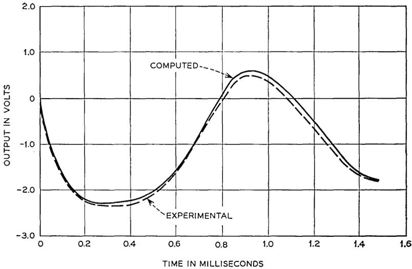
Fig. 2— Comparison of computed and experimental response of the oscillator shown in Fig. 1.
