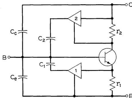
Fig. 7.—Two-pole transistor self-analogue.
