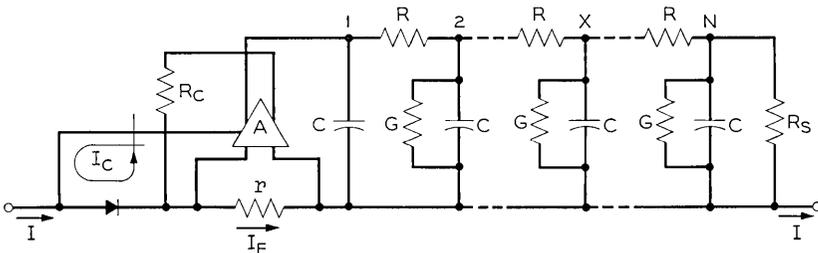
Fig. 3 — Physical realization of Linvill model as a diode self-analogue.
