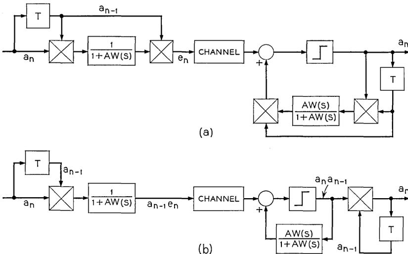
Fig. 5—Equivalent binary one-tap systems. (a) Equivalent system. (b) Simplified equivalent.
