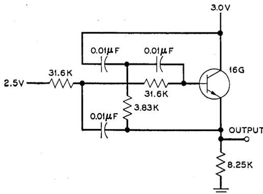
Fig. 1 — One-kilocycle oscillator using a 16G "100 megacycle" transistor.
