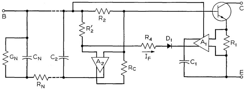
Fig. 9 — Separation of active and saturation region storage.
