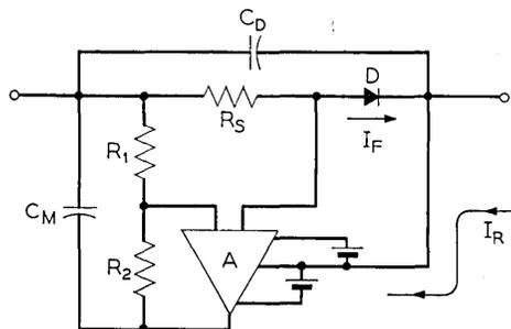
Fig. 1 — Diode self-analogue with scaling of charge storage.
