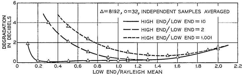
Fig. 3 — Degradation resulting from limited dynamic range.
