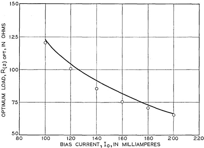
Fig. 10 — Measured (plotted points) and computed values (curve) of  $R_{(2)opt}$  as a function of bias current,  $I_o$ , using a Western Electric 20J transistor with  $R_s = 500$  ohms and  $V_o = 25$  volts.
