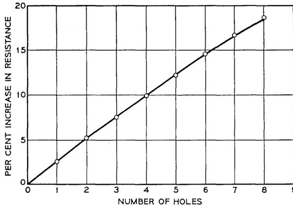
Fig. 12 — Resistor trimming by spot material removal.
