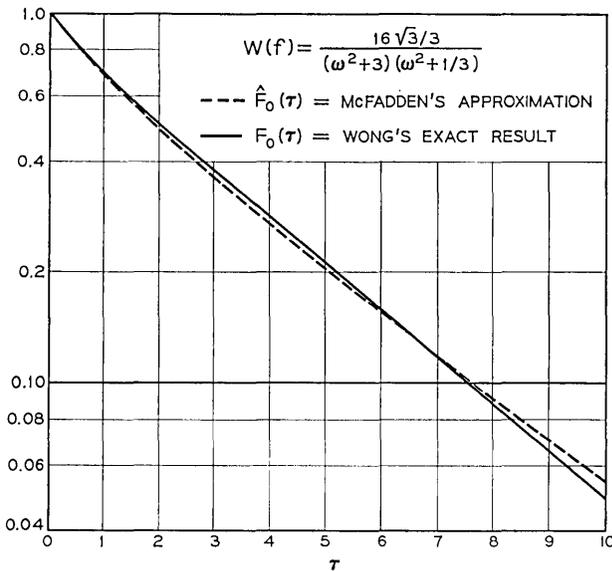
Fig. 2—Comparison of approximate and exact results for  $F_0(\tau)$ , the probability that a zero-crossing interval lasts longer than  $\tau$ .
