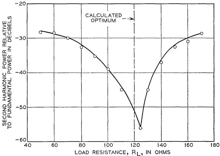
Fig. 3 — Experimental null in second harmonic distortion as a function of  $R_L$ , using a Western Electric 20J transistor with  $V_o = 30$  volts,  $I_o = 100$  milliamperes, and  $R_e = 500$  ohms.
