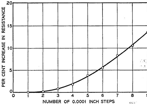
Fig. 13 — Resistor trimming by edge material removal.
