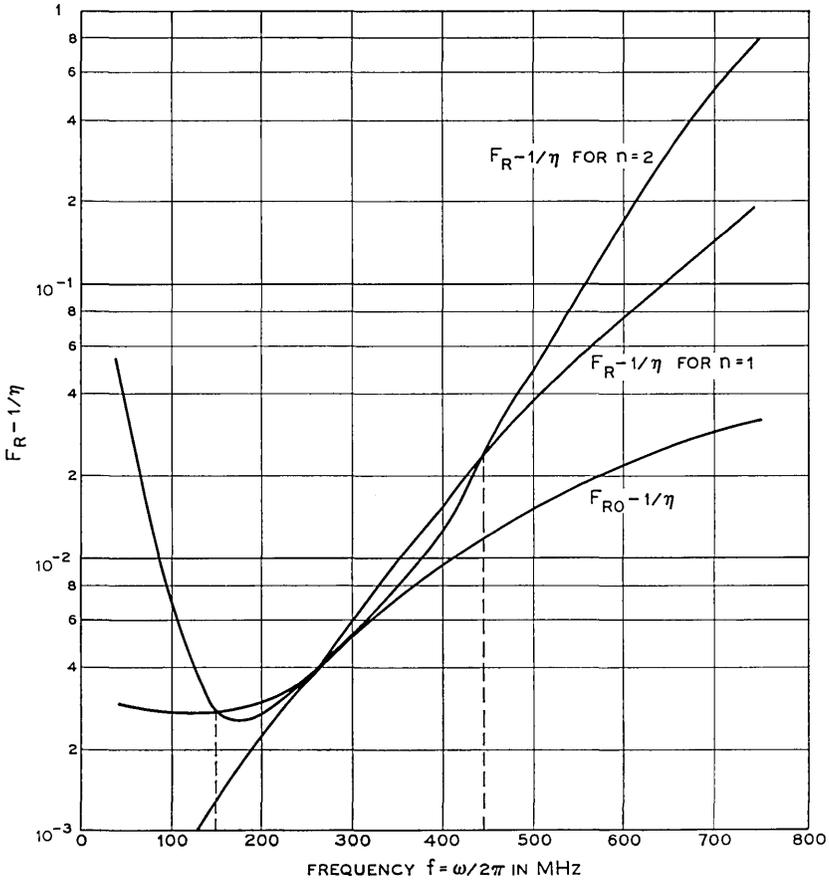
Fig. 7—Butterworth approximations of order  $n = 1, 2$ . It is assumed that  $f_o = 31.83$  GHz,  $\eta = 0.70$ ,  $T_d = 290^\circ\text{K}$ ,  $I_o = 500 \mu\alpha$ ,  $F_o = 2.0833$ , and  $\epsilon^2 = 1$ .
