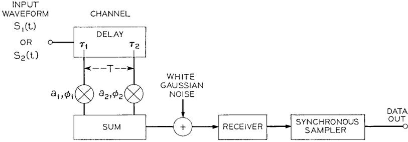
Fig. 1—Data transmission system model.
