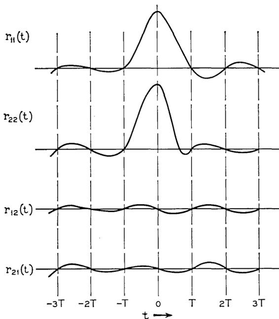
Fig. 5—Required time domain responses for distortionless transmission.
