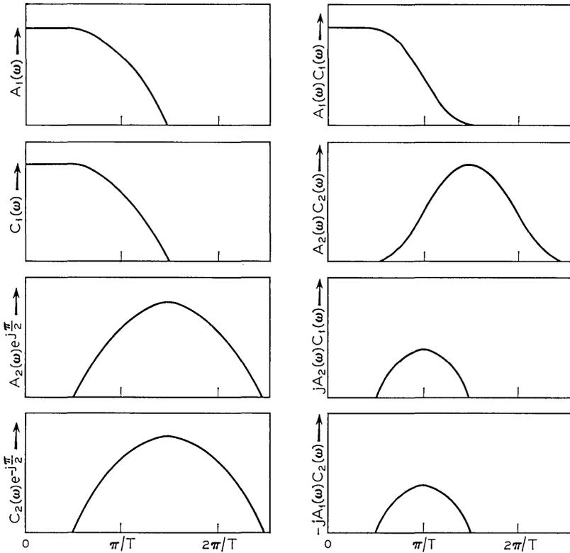
Fig. 6 — A possible two-channel system assuming  $B(\omega) = 1$ .
