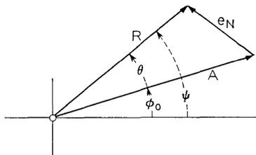
Fig. 3 — Angular perturbation caused by noise.
