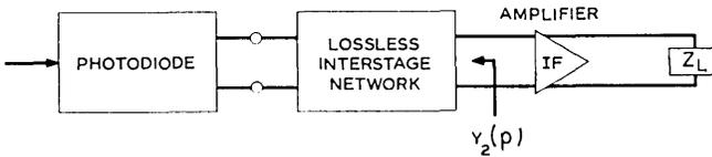
Fig. 1—A double detection optical receiver. The input to the photodetector is the sum of the local oscillator beam and the incoming signal beam.
