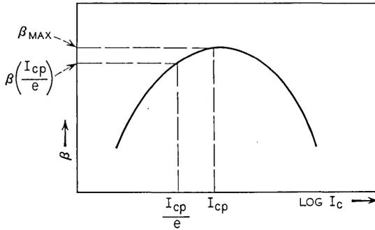
Fig. 8— Current gain nonlinearity as a function of the bias current,  $I_c$ .
