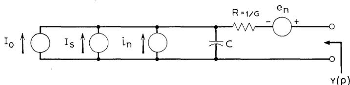
Fig. 2—Equivalent circuit of photodiode. The physical sources of noise that are present in the diode are also shown. The conductance  $G_p$  which appears in parallel with  $C$  is usually so small (around  $10^{-7}$  mho) that it can be neglected for all practical purposes if  $\omega \gg 0$ .
