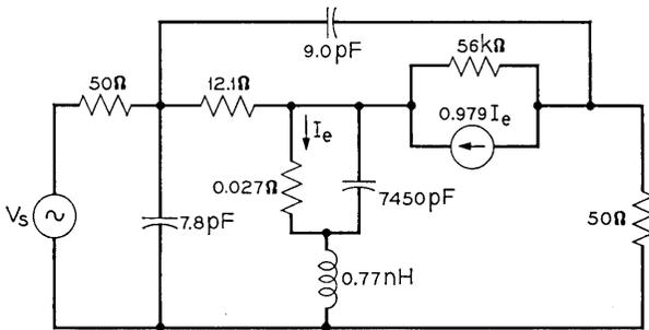
Fig. 4 — Linear model for  $I_e = 150$  mA,  $V_{cb} = 10$  V. With the indicated element values, this model matches the measured  $h$ -parameters shown in Fig. 5. The quality of the match at this bias point ( $I_e = 150$  mA,  $V_{cb} = 10$  V) is typical.
