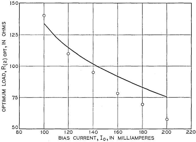
Fig. 9 — Measured (plotted points) and computed values (curve) of  $R_{(2)opt}$  as a function of bias current,  $I_o$ , using a Western Electric 20J transistor with  $R_s = 500$  ohms and  $V_o = 29$  volts.
