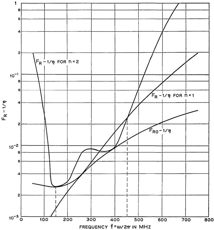
Fig. 10 — Noise factor  $F_R$  as a function of  $\omega$  for Chebyshev approximations of order  $n = 1, 2$ . It is assumed that  $f_c = 31.83$  GHz,  $\eta = 0.70$ ,  $T_o = 290^\circ\text{K}$ ,  $I_o = 500 \mu\alpha$ ,  $F_o = 2.0833$ , and  $\epsilon^2 = 1$ .
