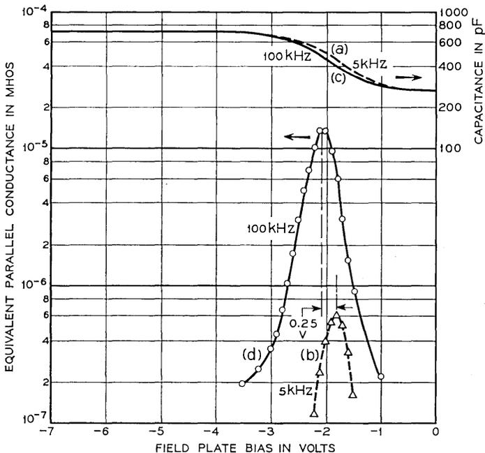
Fig. 1—Capacitance and equivalent parallel conductance measured at 5 kHz and 100 kHz on a p-type sample having an acceptor density of  $2.08 \times 10^{18} \text{ cm}^{-3}$  and interface state density in the  $10^{11} \text{ cm}^{-2} \text{ eV}^{-1}$  range. Interface state time constants and densities are given in Fig. 14 and Fig. 15 for this sample.
