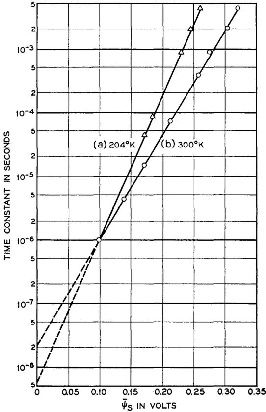
Fig. 16—Log  $\tau_m$  vs  $\bar{\psi}_s$  for p-type sample of Fig. 14: (a) measured at 204°K and (b) at 300°K. (b) Replot of (a) in Fig. 14. Curves show that experimentally obtained points satisfy temperature dependence of (22). (a) is the only one in this experiment measured at a temperature other than 300°K.
