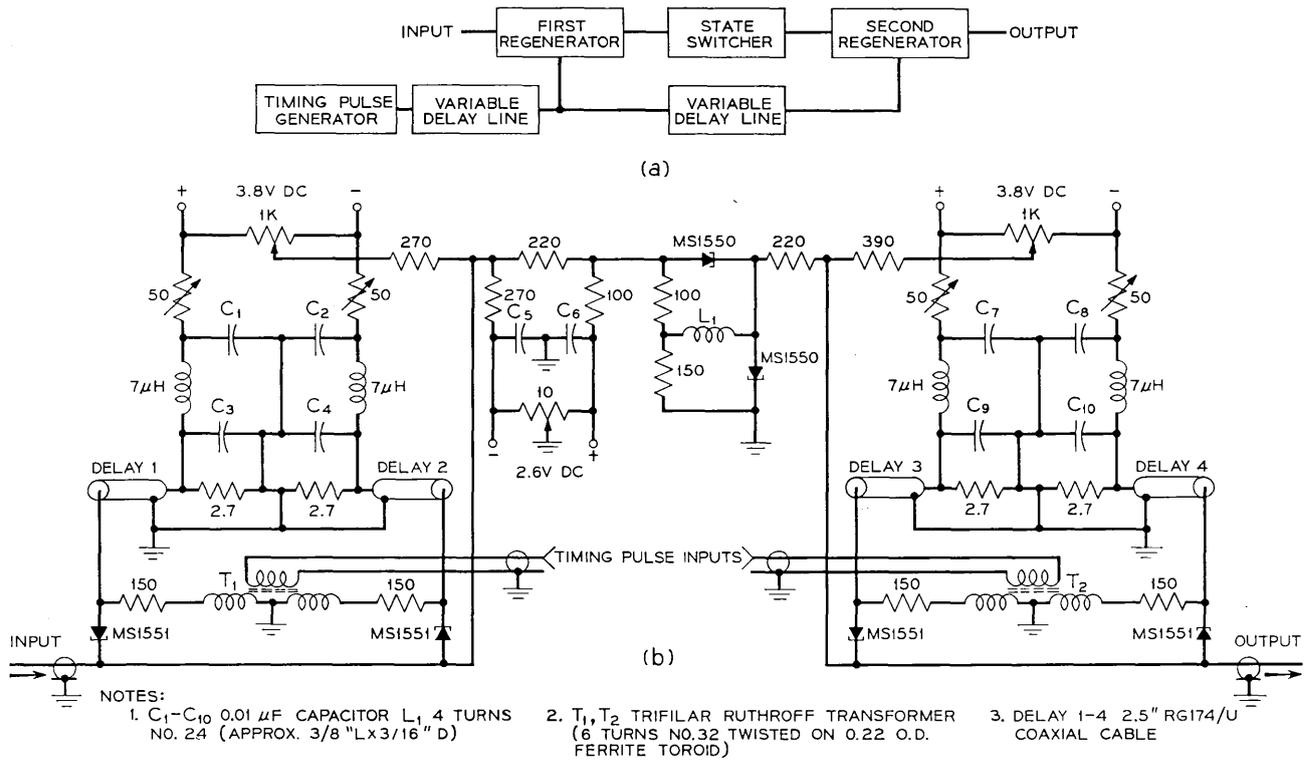
Fig. 7 — (a) Baseband regenerator; (b) baseband regenerator-schematic.
