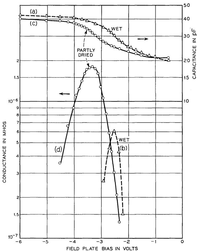
Fig. 3—(a) capacitance and (b) equivalent parallel conductance vs field plate bias before drying; (c) capacitance and (d) equivalent parallel conductance vs field plate bias of the same capacitor after heating in dry nitrogen for 17 hours at 350°C. Field plate diameter is  $3.8 \times 10^{-2}$  cm, silicon resistivity 1  $\Omega$ -cm, p-type, crystal orientation [111], oxide thickness 910 Å grown in steam, and measurement frequency 100 kHz.
