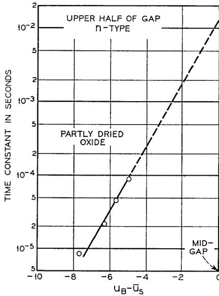
Fig. 19 — Log  $\tau_m$  vs  $u_B - \bar{u}_s$  after partial drying of n-type sample in Fig. 4. Measured points still fit (22). Donor density is  $1.4 \times 10^{18} \text{ cm}^{-3}$ ,  $u_B = 13.7$ , and  $C_{ox} = 5.96 \times 10^{-2} \text{ farads/cm}^2$ .
