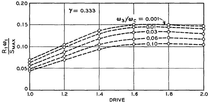
Fig. 14—Input resistance at  $\omega_1$ , for a graded-junction varactor. These results become inaccurate for high loss (high  $\omega_3/\omega_c$ ) and  $\omega_3 \neq 8\omega_1$ . Accurate values of  $R_1\omega_1/S_{max}$  may be obtained by subtracting the quantity
