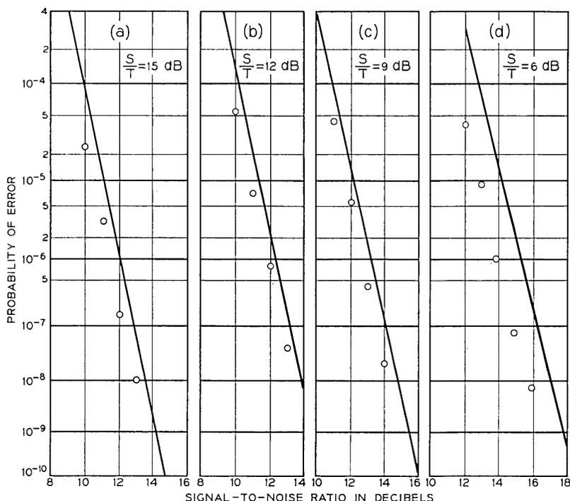
Fig. 13 — Error rate vs S/N for band-limited pulses. Points represent experimental values, curves are theoretical values from Ref. 5 evaluated  $\rho_r = 22.5$  dB (the experimentally determined value for this waveform).
