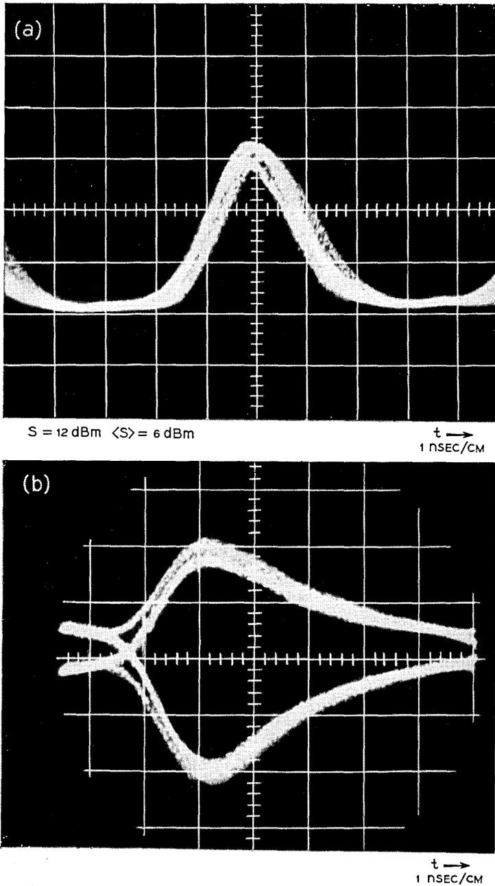
Fig. 10—Narrow pulse experiment wave forms. (a) Envelope-detected RF pulse. (b) Eye-diagram (output to differential phase detector, input to regenerator).
