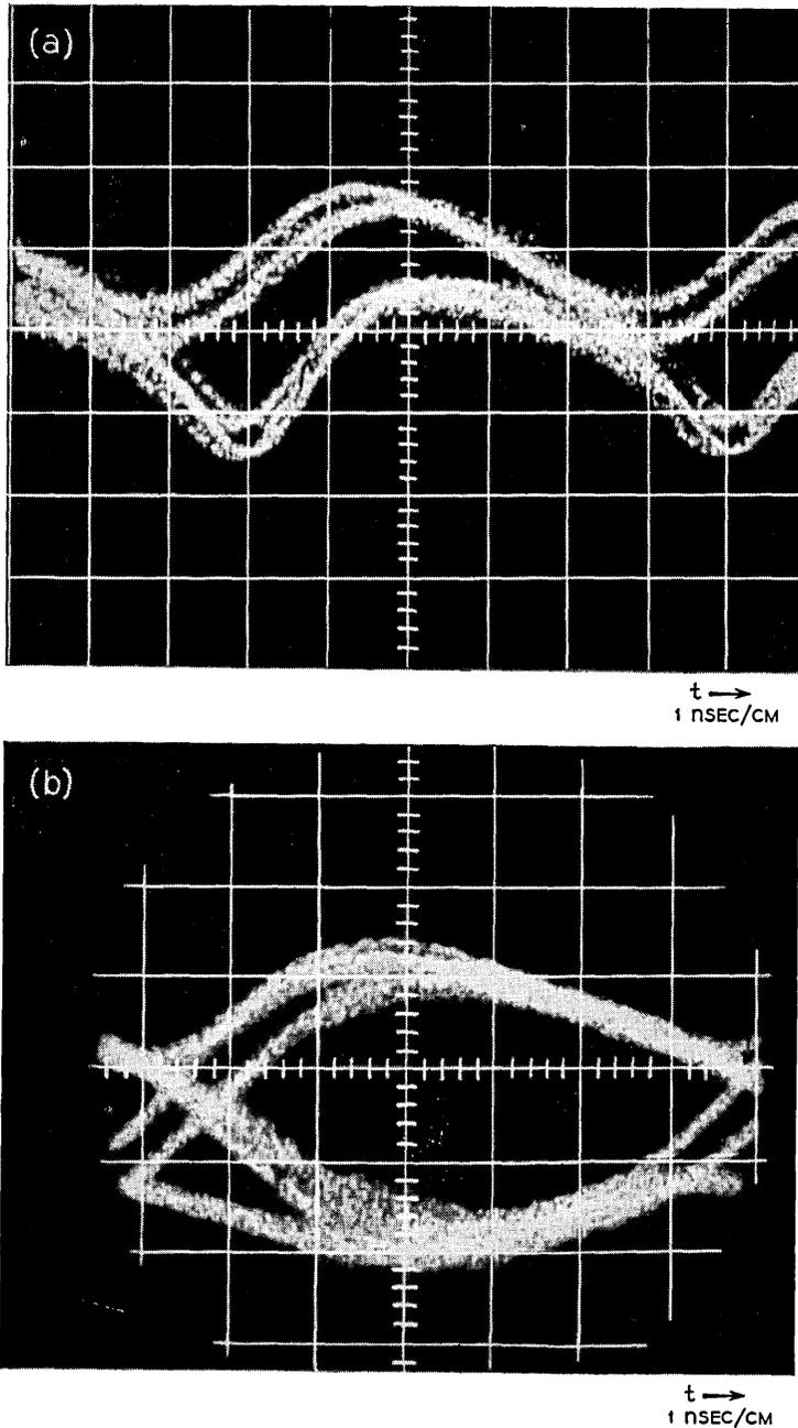
Fig. 12—Widened pulse experiment wave forms. (a) Envelope-detected RF pulse. (b) Eye-diagram (output to differential phase detector, input to regenerator).
