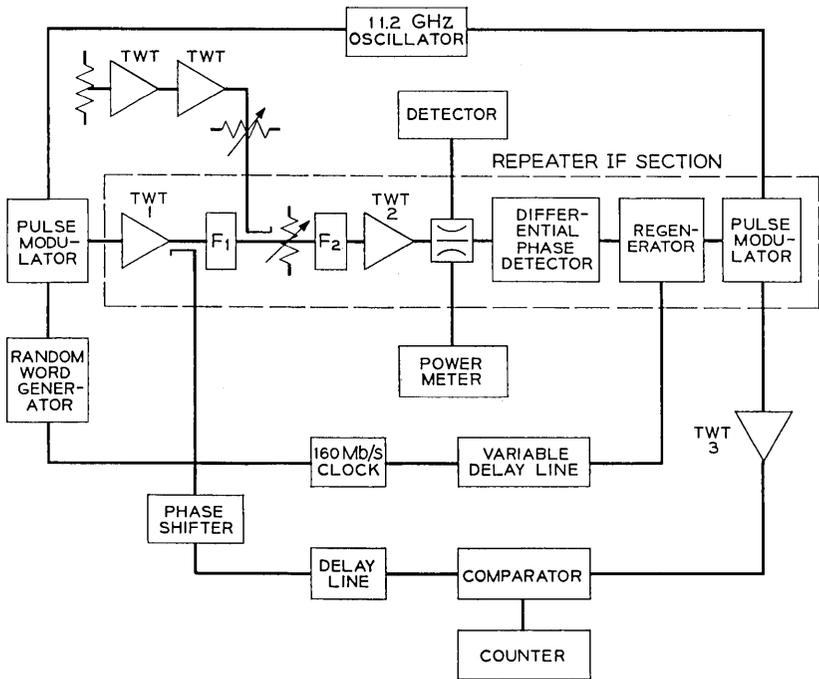
Fig. 2 — Block diagram of the AM-DCPSK model repeater.
