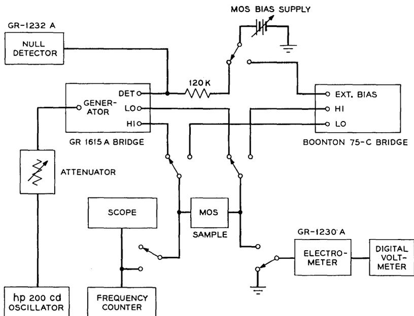
Fig. 10 — Block diagram of measuring apparatus.
