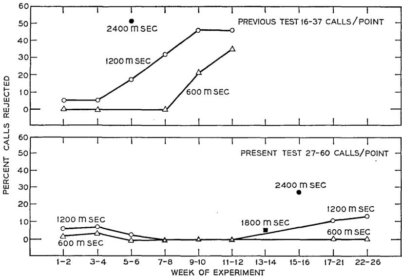
Fig. 1—Rate of rejection of circuits as a function of weeks of the experiment from Riesz and Klemmer<sup>6</sup> and for the present experiment. Combined data from 18 and 20 subjects, respectively.
