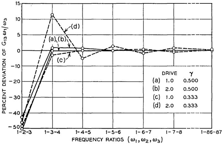
Fig. 4—Variation of normalized upconversion gain as a function of the three upconverter frequencies. Percent deviations are calculated with respect to the 1-86-87 case.  $\omega_3/\omega_c = 0.001$ .
