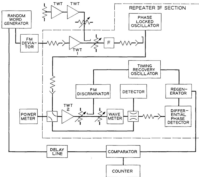
Fig. 3—Block diagram of the FM-DCPSK model repeater.
