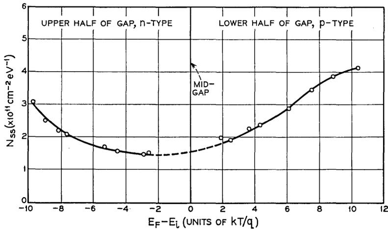
Fig. 15— $N_{ss}$  from (59) vs  $E_F - E_i$  measured in units of  $kT/q$  for same two samples in Fig. 14. Flat band is 14.1 in lower half of the gap and 13.5 in upper half.  $E_F$  is position of the Fermi level and  $E_i$  is mid-gap.
