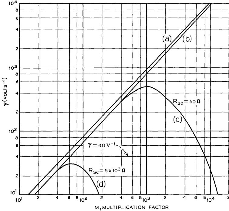
Fig. 1— $\gamma$  versus multiplication factor. (a)  $p$ - $n$  junction in silicon with background doping  $5 \times 10^{16} \text{ cm}^{-3}$  and without space-charge effect. (b)  $p$ - $n$  junction in silicon with background doping  $1.5 \times 10^{17} \text{ cm}^{-3}$  and without space-charge effect. (c) Same as (a) with 50-ohms space-charge resistance. (d) Same as (a) with 5000 ohms space-charge resistance.
