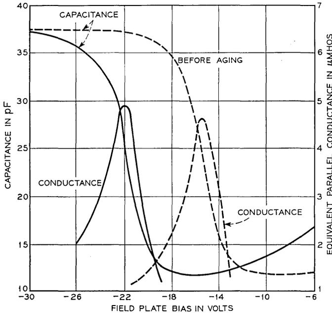
Fig. 2—Measured capacitance and equivalent parallel conductance as functions of field plate bias before and after aging at 150°C in room air. Field plate diameter is  $3.8 \times 10^{-2}$  cm, silicon resistivity 50  $\Omega$ -cm, p-type, crystal orientation [111], oxide thickness 1200 Å, and measurement frequency 100 kHz.
