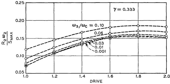
Fig. 16—Input resistance at  $\omega_2$  for a graded-junction varactor. These results become inaccurate for high loss (high  $\omega_3/\omega_c$ ) and  $\omega_3 \neq 8\omega_1$ . Accurate values of  $R_2\omega_2/S_{max}$  may be obtained by adding the quantity
