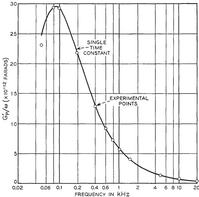
Fig. 25 —  $G_p'/\omega$  vs frequency showing how experimental points fit (17).  $C_s = 5.14 \times 10^{-8}$  farads/cm<sup>2</sup> and  $\tau = 1.7 \times 10^{-8}$  seconds are used in (17) to get this fit.  $G_p'$  is equivalent parallel conductance in mhos derived from measurements. Experimental points are measured at a bias of -3.3 volts ( $\bar{u}_s = 19.8$ ) in the weak inversion region on the n-type sample of Fig. 14.
