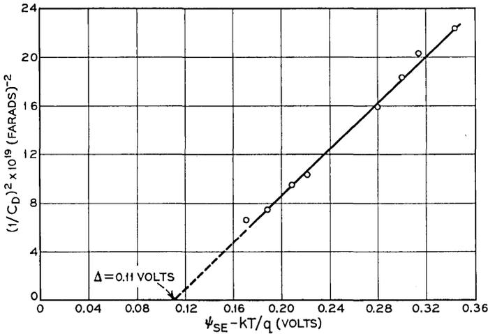
Fig. 12— $1/C_D^2$  vs  $\psi_{se}-kT/q$  where  $C_D$  in farads is obtained from measurements in the depletion region of an n-type sample ( $N_D = 1.15 \times 10^{15} \text{ cm}^{-3}$ ) and  $\psi_{se}$  from the integral in (52). Field plate diameter is  $3.8 \times 10^{-2}$  cm.
