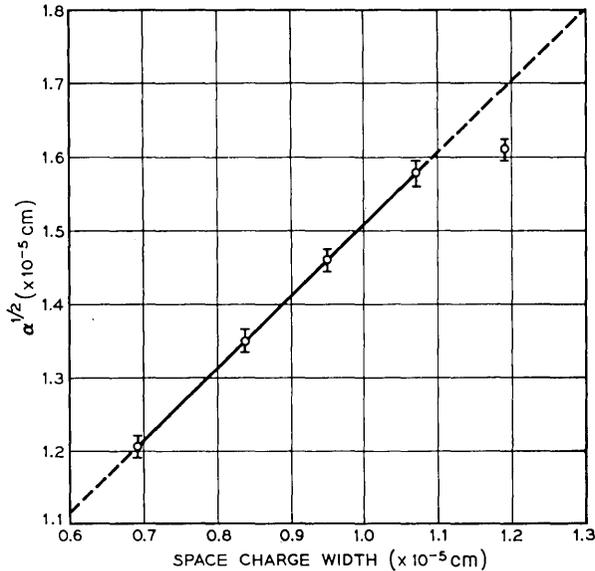
Fig. 22 —  $\alpha^{1/2}$  vs space-charge width where  $\alpha$  is obtained by finding the best fit of (39) to experimental points taken on p-type sample in Fig. 14.  $\alpha^{1/2}$  can have any value within vertical bars through each point. Bars indicate precision with which (39) can be fitted to measured  $G_p/\omega$  vs frequency points. No reason why the point at the largest  $W$  does not lie on the straight line is known.
