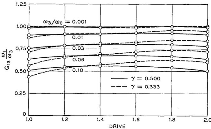
Fig. 9— Upconversion gain for varactor upconverters operating at maximum power output. These results become inaccurate for high loss (high  $\omega_3/\omega_c$ ) and  $\omega_3 \neq 8\omega_1$ . Accurate values of gain may be obtained from the values plotted by dividing by the correction factor
