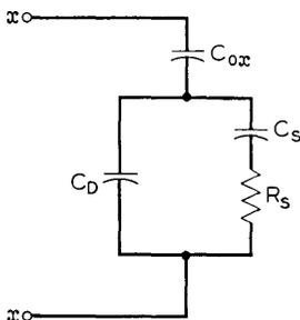
Fig. 6—Equivalent circuit of MIS capacitor for capture and emission of majority carriers by a single level interface state.  $C_{ox}$  is the oxide capacitance per unit area,  $C_D$  the depletion layer capacitance per unit area,  $C_s$  the interface state capacitance per unit area, and  $R_s$  the majority carrier capture resistance. Bulk generation-recombination is zero.
