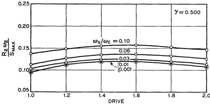
Fig. 15—Input resistance at  $\omega_2$  for an abrupt-junction varactor. These results become inaccurate for high loss (high  $\omega_3/\omega_c$ ) and  $\omega_3 \neq 8\omega_1$ . Accurate values of  $R_2\omega_2/S_{max}$  may be obtained by adding the quantity
