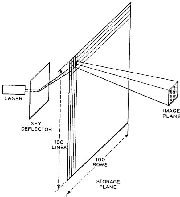
Fig. 2 — Schematic of optical memory system.
