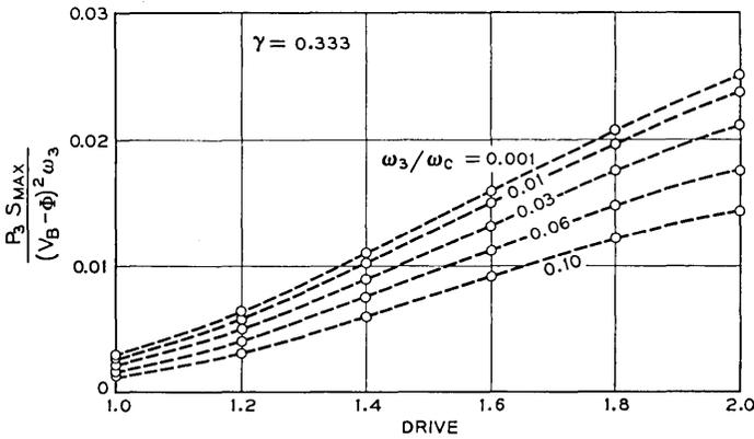
Fig. 8— Maximum power output for graded junction varactors.
