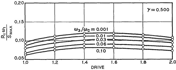
Fig. 13 — Input resistance at  $\omega_1$  for an abrupt-junction varactor. These results become inaccurate for high loss (high  $\omega_3/\omega_c$ ) and  $\omega_3 \neq 8\omega_1$ . Accurate values of  $R_1\omega_1/S_{MAX}$  may be obtained by subtracting the quantity
