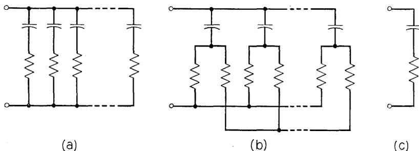
Fig. 31 — (a) Schematic of interface state branch of equivalent circuit in depletion-accumulation region where  $\bar{u}_s < u_B$ . (b) Schematic of interface state branch of equivalent circuit in mid-gap region where  $\bar{u}_s = u_B \pm a \text{ few } kT/q$ . (c) Schematic of interface state branch of equivalent circuit in weak inversion region where  $u_B < \bar{u}_s < 2u_B$ .
