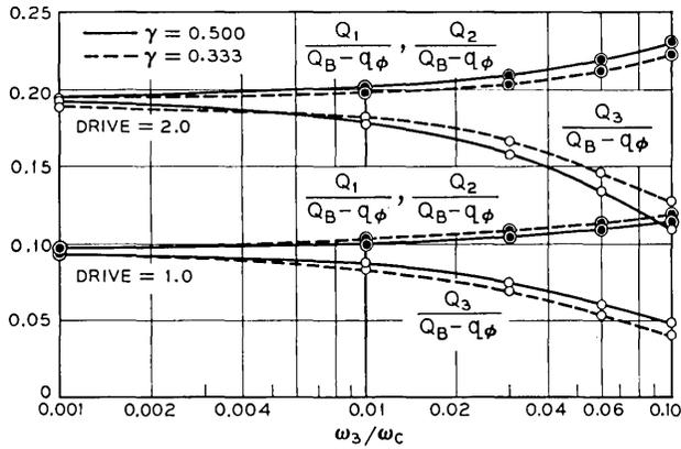
Fig. 6—Normalized charge amplitude coefficients for maximum power output.
