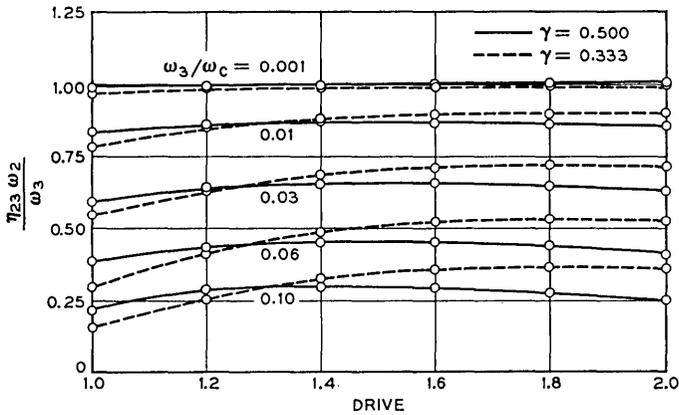
Fig. 10 — Microwave conversion efficiency for varactor upconverters operating at maximum power output. These results become inaccurate for high loss (high  $\omega_3/\omega_c$ ) and  $\omega_3 \neq 8\omega_1$ . Accurate values of efficiency may be obtained from the values plotted by dividing by the correction factor
