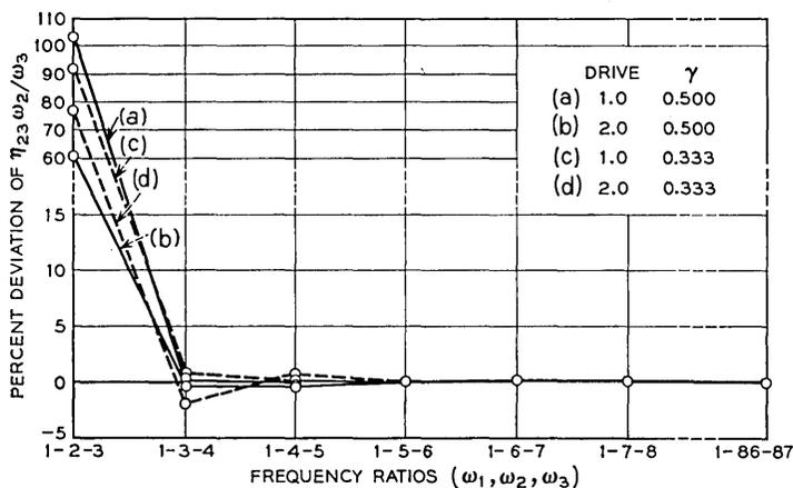
Fig. 3—Variation of normalized microwave conversion efficiency as a function of the three upconverter frequencies. Percent deviations are calculated with respect to the 1-86-87 case.  $\omega_3/\omega_c = 0.001$ .
