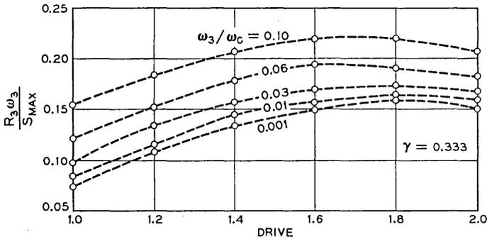
Fig. 18— Load resistance for a graded-junction varactor.
