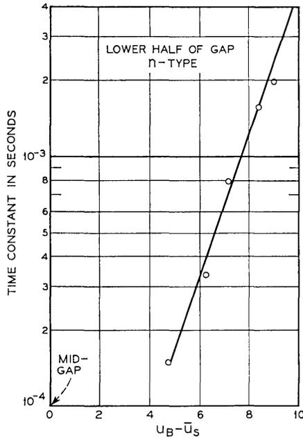
Fig. 26—Log  $\tau_m$  vs  $u_B - \bar{u}_s$  for n-type sample in Fig. 14 in weak inversion region. Curve shows that equivalent parallel conductance in weak inversion is dependent on majority carrier density at the silicon surface.
