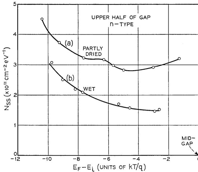
Fig. 20 —  $N_{ss}$ , from (59) vs  $E_F - E_t$ . (a) n-type sample in Fig. 19 and (b) replot of n-type sample from Fig. 15 for comparison. For (a), flat band is 13.7 and for (b), flat band is 13.5.
