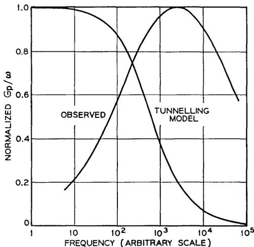
Fig. 33—Normalized  $G_p/\omega$  vs  $\log$  frequency for tunnelling calculated from (104) and normalized  $G_p/\omega$  vs  $\log$  frequency obtained for measurement. Frequency scale is arbitrary to compare the shapes of two curves.
