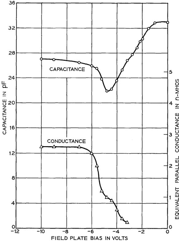
Fig. 29—Capacitance and equivalent parallel conductance measured at 50 Hz vs field plate bias. Field plate diameter is  $3.8 \times 10^{-2}$  cm, silicon resistivity 1 ohm-cm, n-type, [100] oriented, and  $C_{ox} = 2.8 \times 10^{-8}$  farads/cm<sup>2</sup>. Oxide is grown in steam then H<sub>2</sub> annealed as described in text to produce low  $N_{ss}$ .
