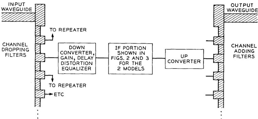
Fig. 1 — Block diagram of a complete repeater.
