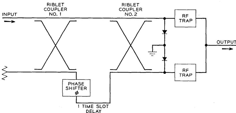
Fig. 5—Differential phase detector ( $D\phi D$ ).
