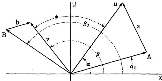
Fig. 9—Phasor diagram for the differential detection process.
