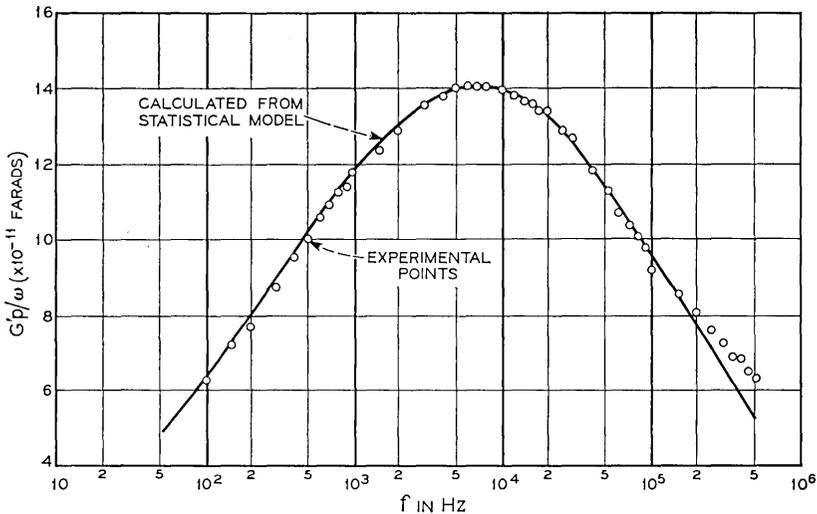
Fig. 21— $G_p/\omega$  vs frequency showing how experimental points fit (39). An  $\alpha$  of  $2.5 \times 10^{-10} \text{ cm}^2$  is used in (39) to get this fit.  $G_p'$  is equivalent parallel conductance in mhos derived from the measurements. Experimental points are measured at a bias of  $-1.9$  volts ( $\bar{u}_s = 8.1$ ) in depletion region on the p-type sample of Fig. 14.
