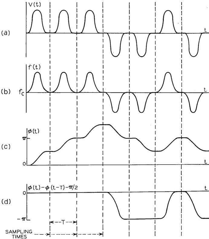
Fig. 15—FM-DCPSK signal; (a) modulating voltage vs time; (b) frequency vs time; (c) phase vs time; (d) differential phase vs time.
