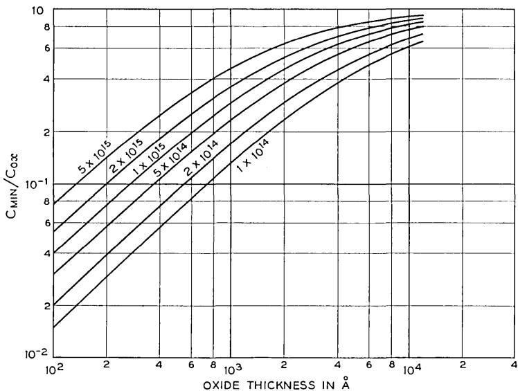
Fig. 43 — Minimum capacity vs oxide thickness. Doping density as parameter
