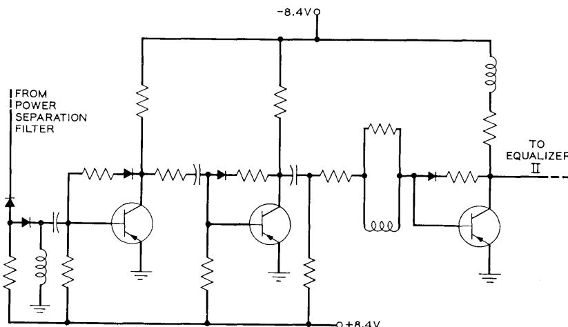
Fig. 24 — Preamplifier circuit.
