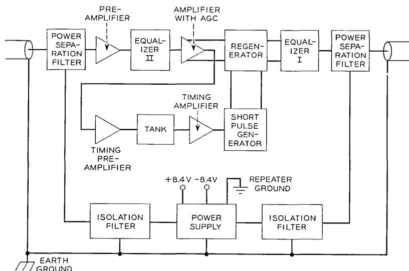
Fig. 21.—Functional block diagram of the repeater.
