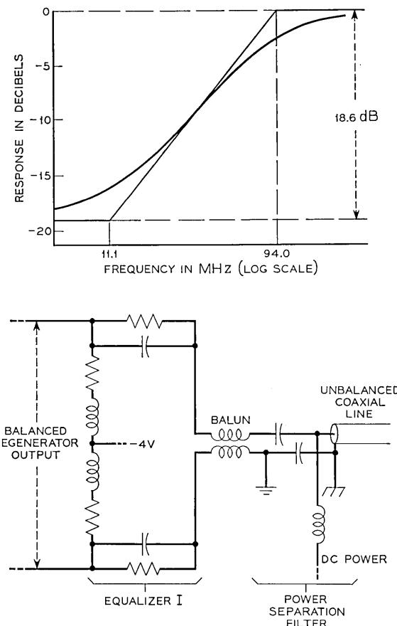
Fig. 22 — Equalizer I—attenuation characteristic and circuit configuration.
