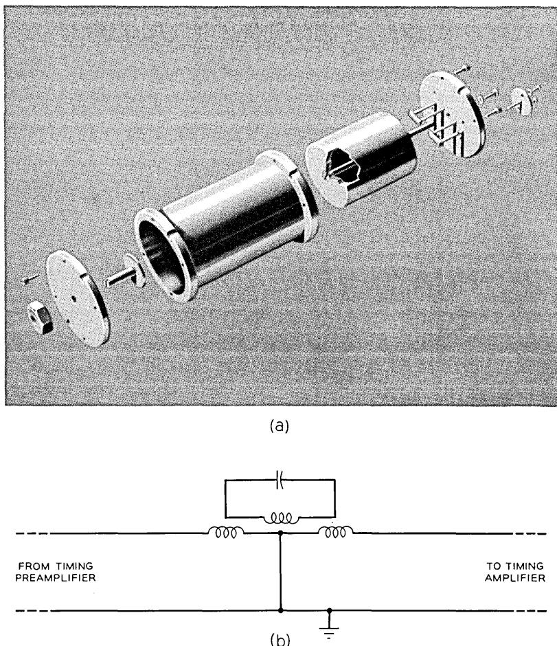
Fig. 26—The resonant tank; (a) exploded view; (b) equivalent circuit.
