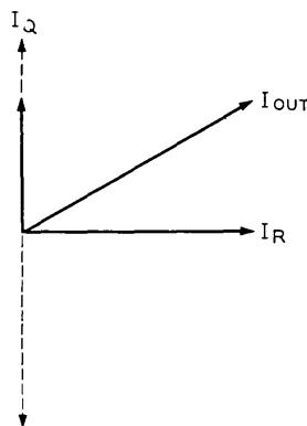
Fig. 31 — Vector diagram for phase adjustment circuit.
