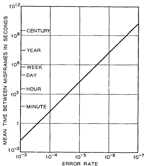
Fig. 6 — Misframes due to random line errors.
