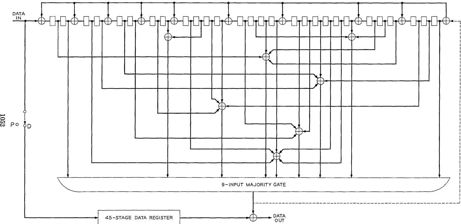
Fig. 2 — Decoder for  $(73, 45)$ ,  $d = 10$ , binary difference-set cyclic code.
