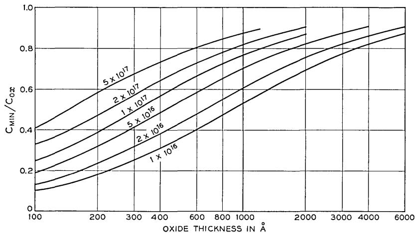
Fig. 44 — Minimum capacity vs oxide thickness. Doping density as parameter
