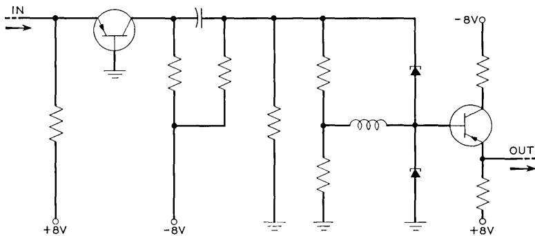
Fig. 9—Goto pair binary counter using two Esaki diodes.
