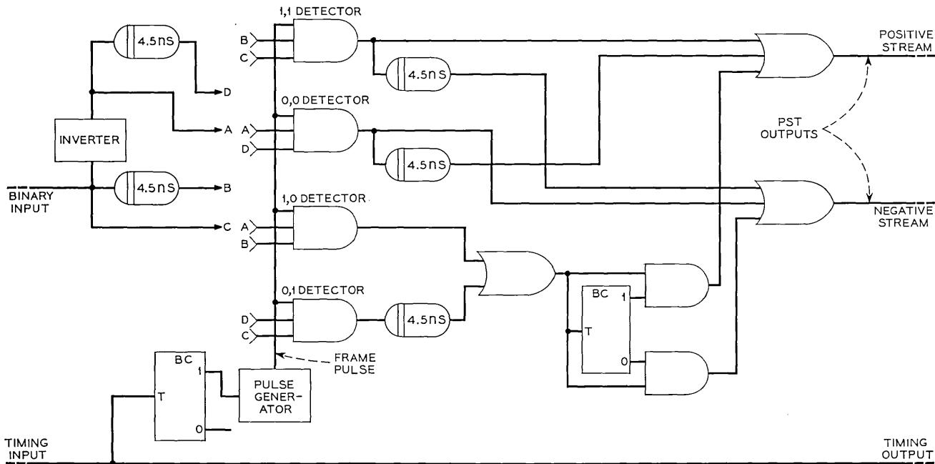
Fig. 3 — Logical diagram of the binary-to-PST translator.
