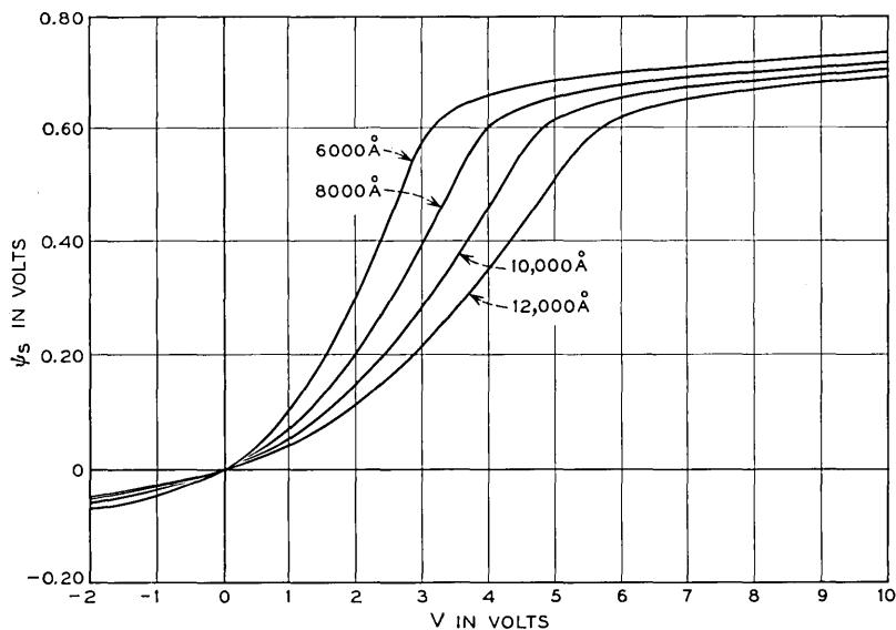
Fig. 24 — Surface potential vs voltage. Oxide thickness 6000–12,000 Å. ( $N_A = 1.0 \times 10^{15} \text{ cm}^{-3}$ )
