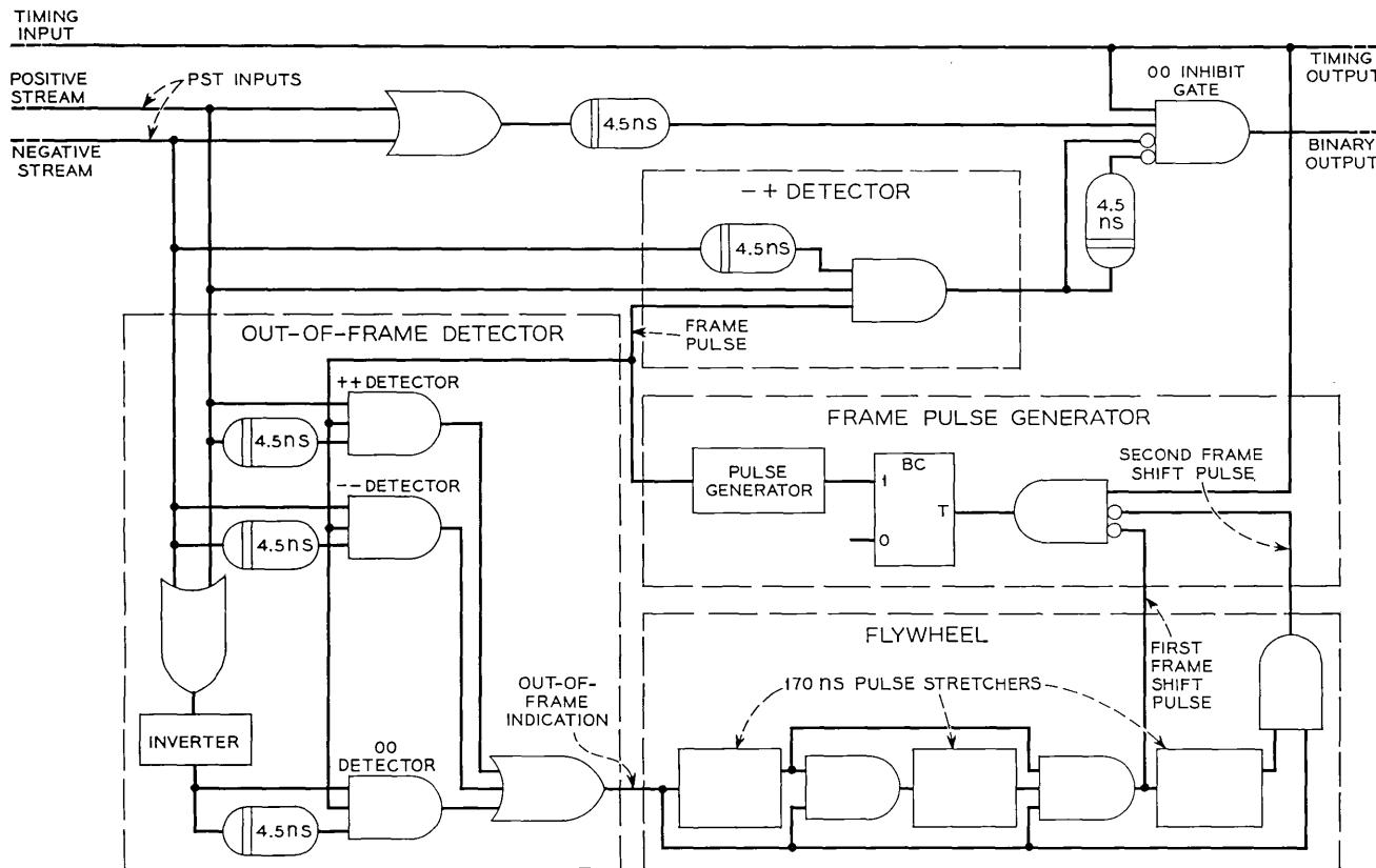
Fig. 4—Logical diagram of the PST-to-binary translator.
