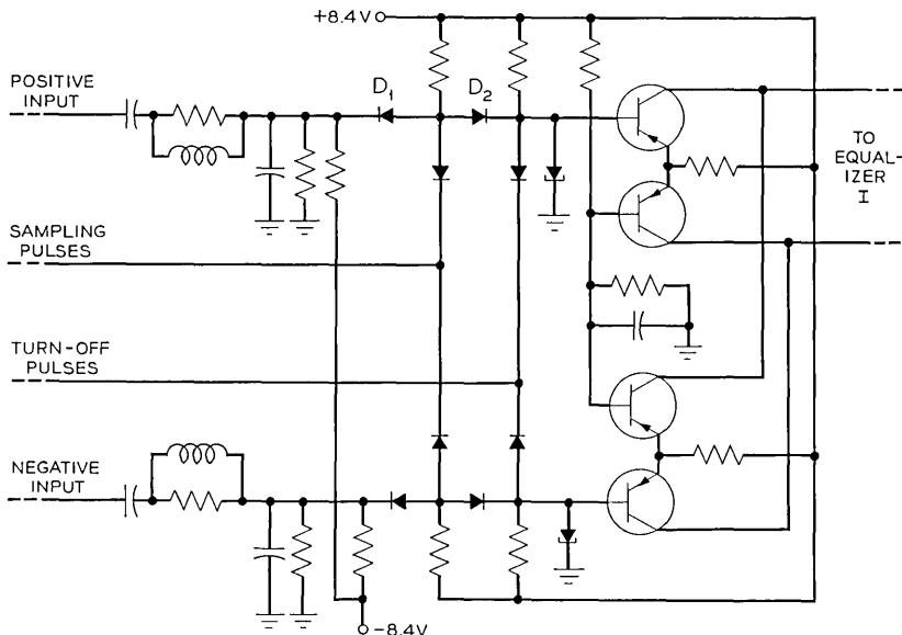
Fig. 33 — Regenerator circuit.
