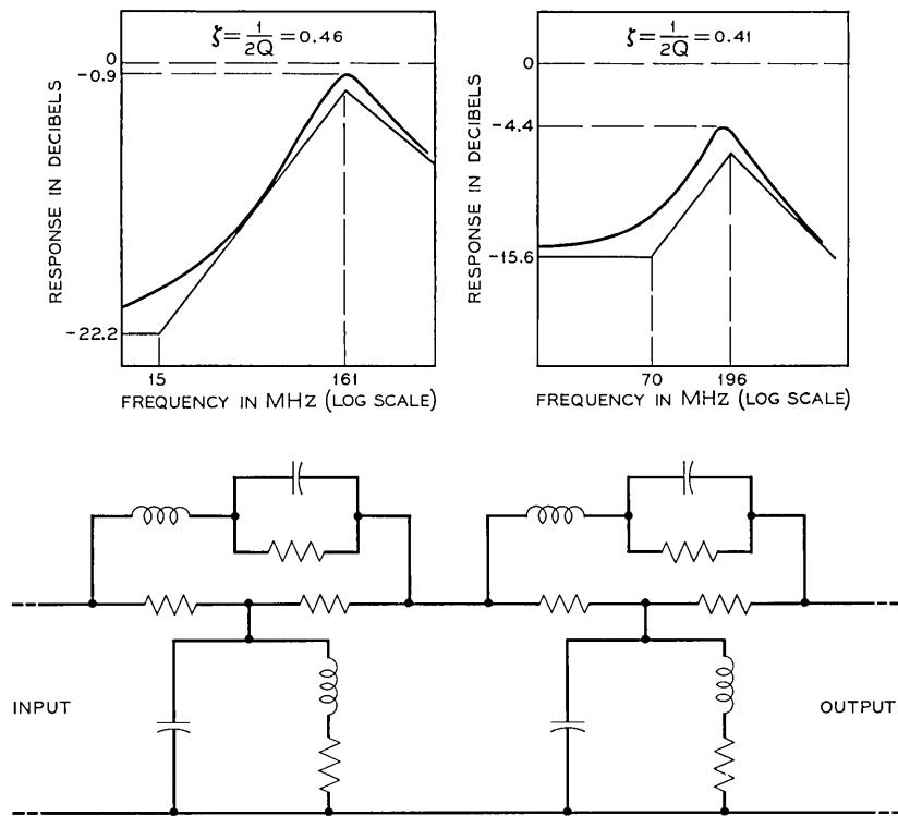
Fig. 23—Equalizer II — attenuation characteristic and circuit configuration.
