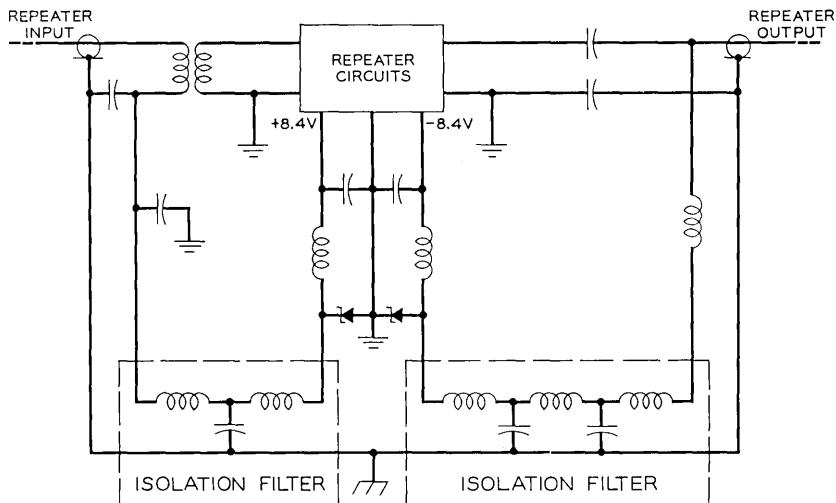
Fig. 36 — Repeater powering circuit.
