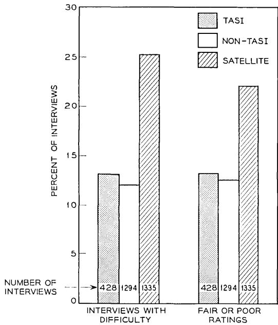
Fig. 14 — Comparison of cable and satellite circuits.
