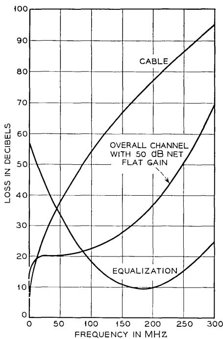
Fig. 14—Cable, equalization, and overall channel loss characteristics.
