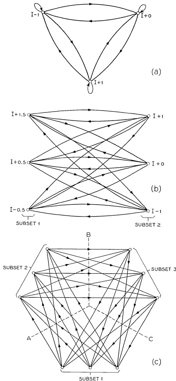
Fig. 11—(a) Midtread case;  $A = -\frac{1}{2}$ ,  $M = 1$ . (b) Midriser case;  $A = 0$ ,  $M = 2$ . (c)  $A = -\frac{1}{6}$ ,  $M = 3$ .
