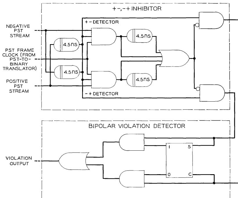
Fig. 7—Logical diagram of the PST violation monitor.
