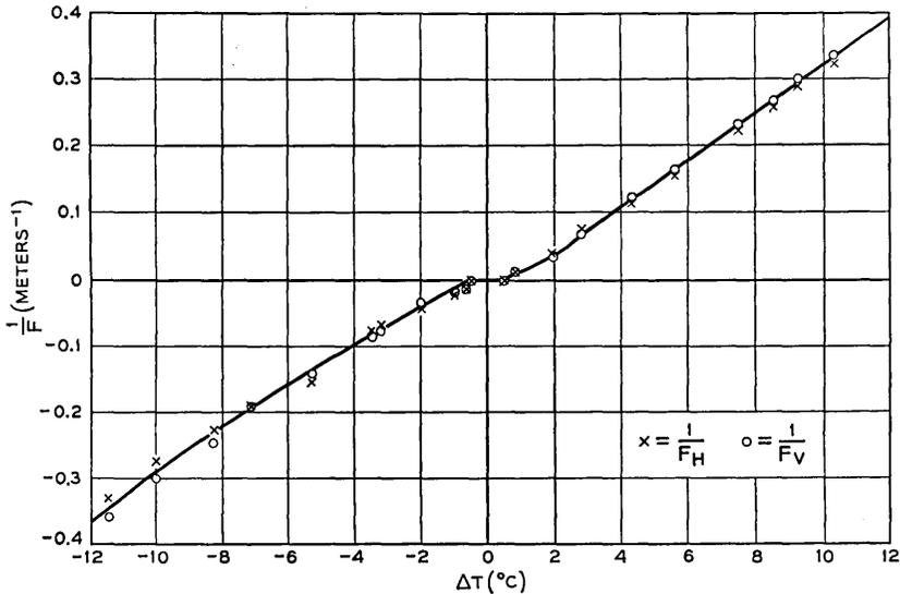
Fig. 2 — Reciprocal focal length, or convergence in vertical plane ( $1/F_V$ ) and in horizontal plane ( $1/F_H$ ), vs temperature of inner helix minus temperature of outer tube for the lens shown in Fig. 1 with CO<sub>2</sub> at one atmosphere pressure. The difference between horizontal and vertical convergence is a measure of astigmatism.
