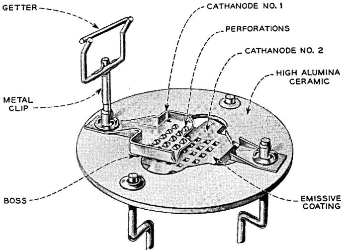
Fig. 11 — Structural features of the 458A tube.
