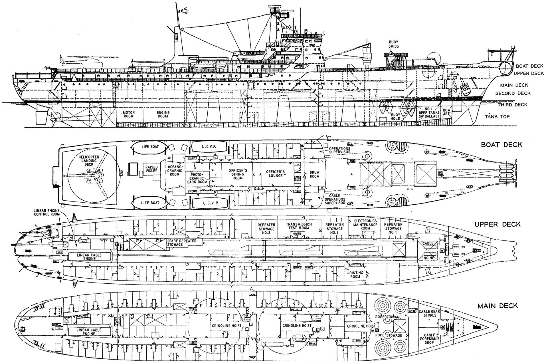
Fig. 4 — General arrangement of decks.
