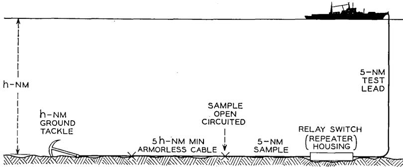
Fig. 12 — Cable arrangement for sea trial.
