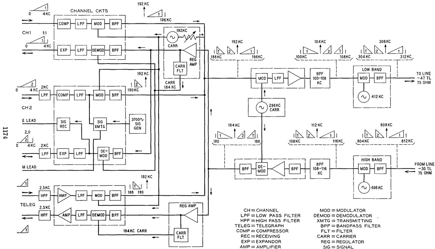
Fig. 14 — Order wire block schematic.
