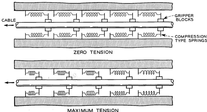
Fig. 3 — Shear limiting.
