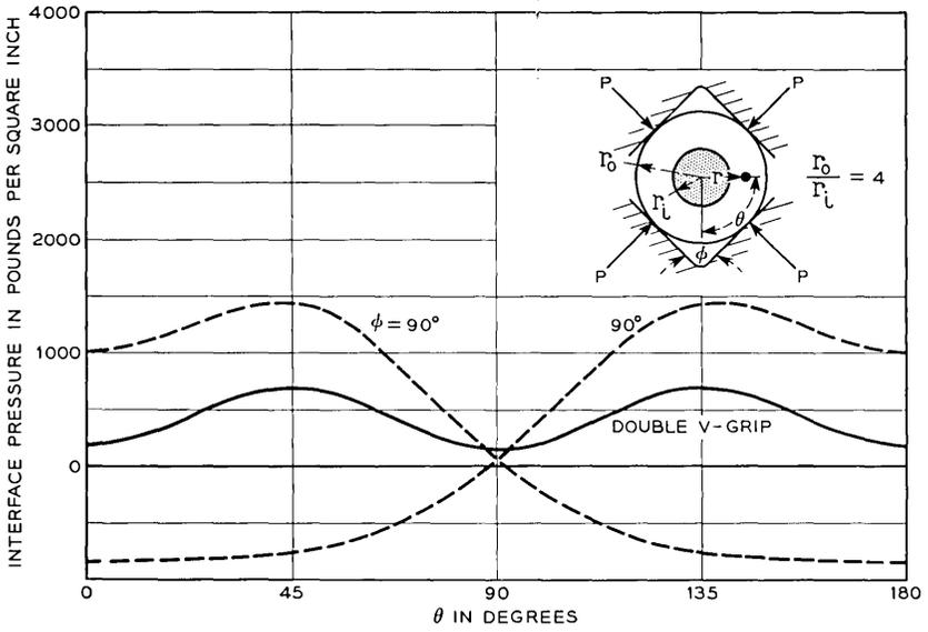
Fig. 21 — Center conductor normal stress — two V blocks.
