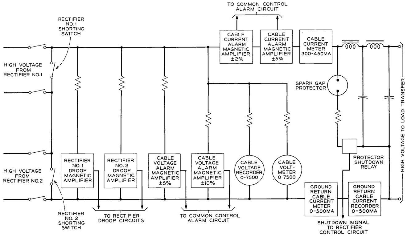
Fig. 11 — Common control functional circuit.
