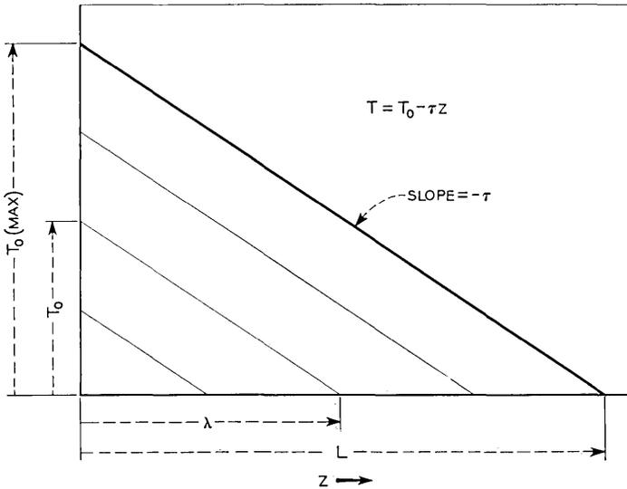
Fig. 19 — Uniformly dissipated cable tension distribution.
