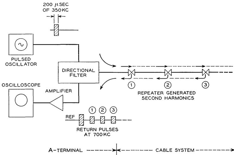
Fig. 15 — Repeater fault locating test set.
