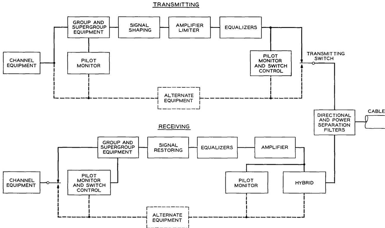
Fig. 5 — Shore terminal block schematic.
