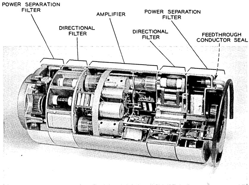
Fig. 11 — Repeater unit — cutaway view.
