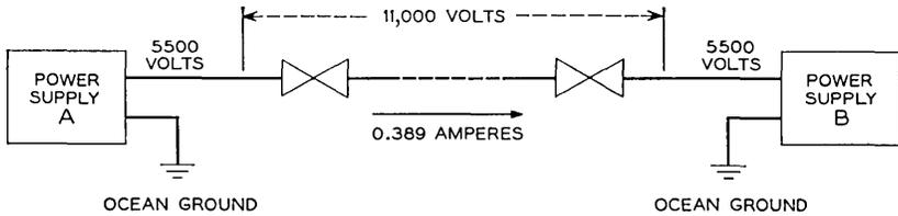
Fig. 1 — Basic power feed arrangement.
