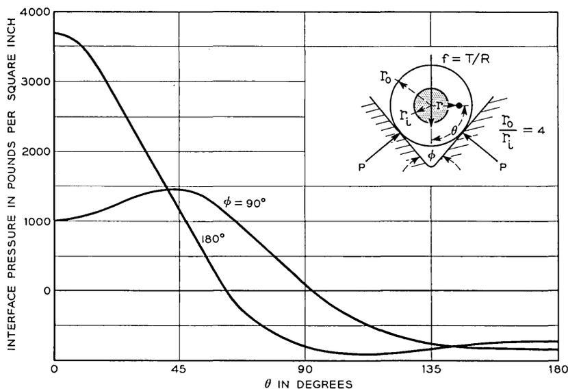
Fig. 20 — Center conductor normal stress — one V-block.
