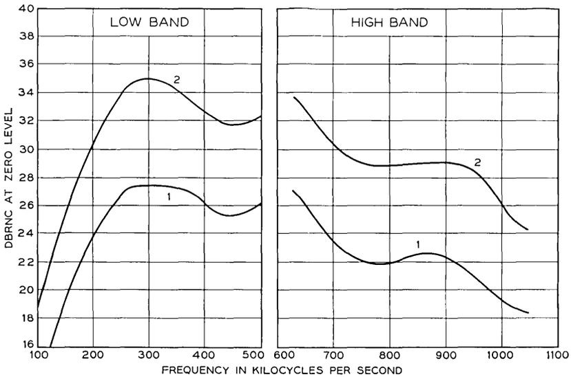
Fig. 22 — Computed modulation noise — TAT-3 system. Load assumptions: talker volume,  $-10.8$  VU; standard deviation,  $5.8$  db; activity,  $0.75$ . Curve 1 shows average modulation noise; curve 2 shows noise level that will be exceeded only 1 per cent of the time.
