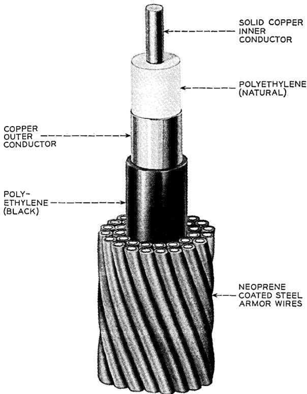
Fig. 3 — SD cable for shallow water, maximum protection.
