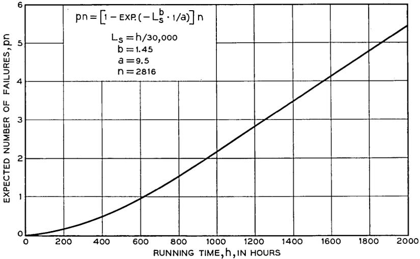
Fig. 24 — Expected number of failures in  $h$  hours.
