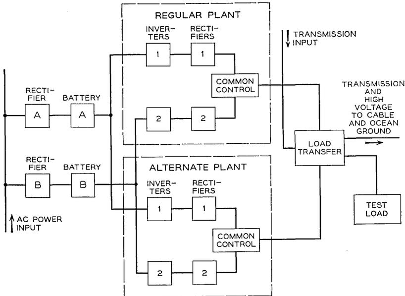
Fig. 2 — Power system functional block diagram.
