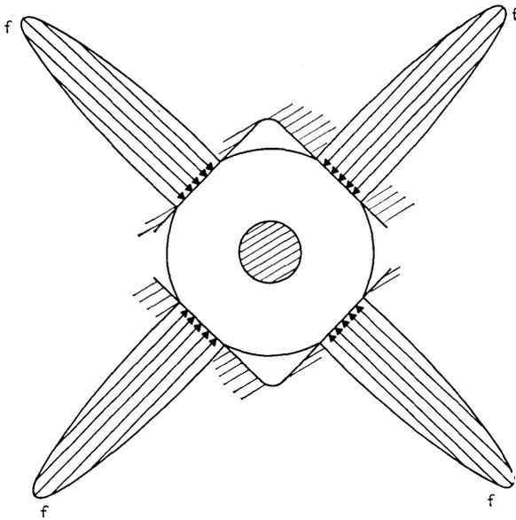
Fig. 22 — Contact stress distribution — two V-blocks.
