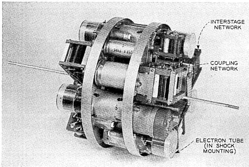
Fig. 13 — Assembled amplifier.
