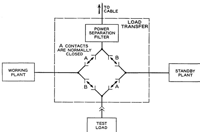
Fig. 12 — Load transfer circuit.
