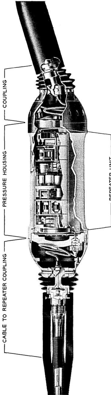
Fig. 8 — Repeater — cutaway drawing.
