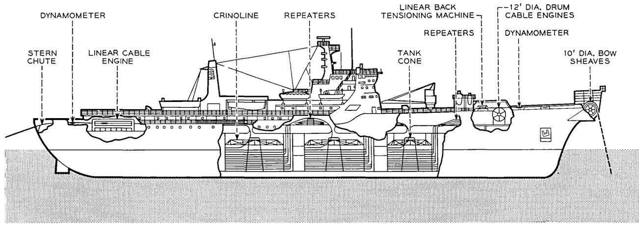
Fig. 1 — General layout of the cable laying system.
