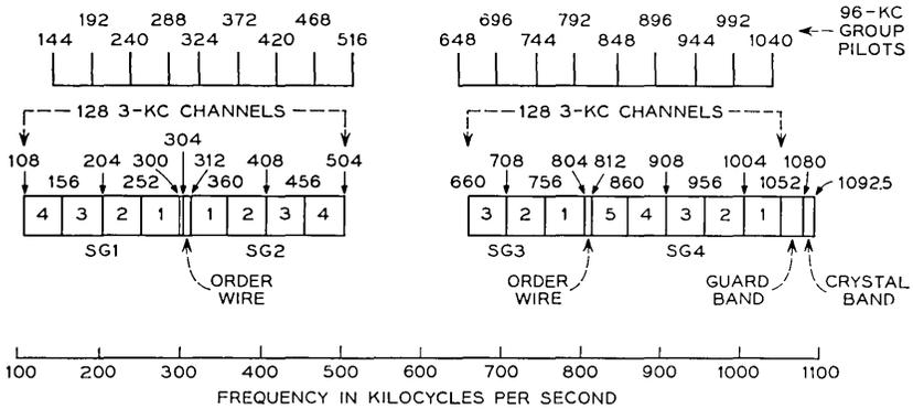
Fig. 2 — Frequency allocations for 128 3-kc message channels.
