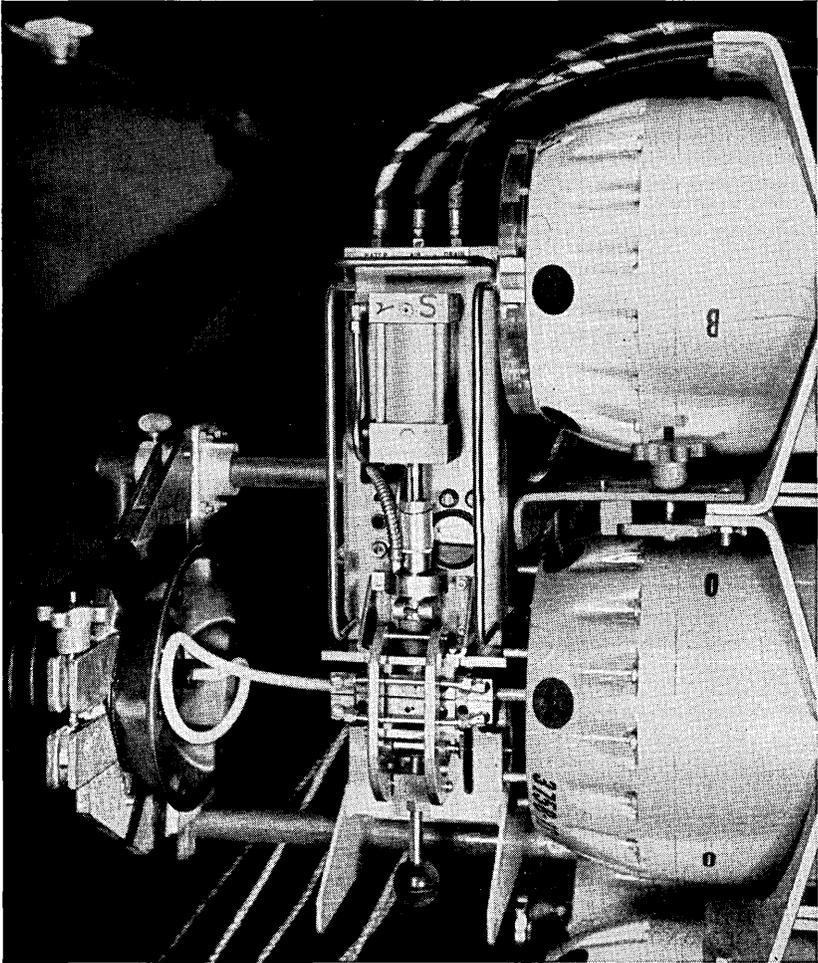
Fig. 12 — Mounting jig with molding machine in position.
