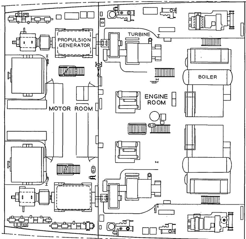
Fig. 5 — Layout of main machinery spaces.
