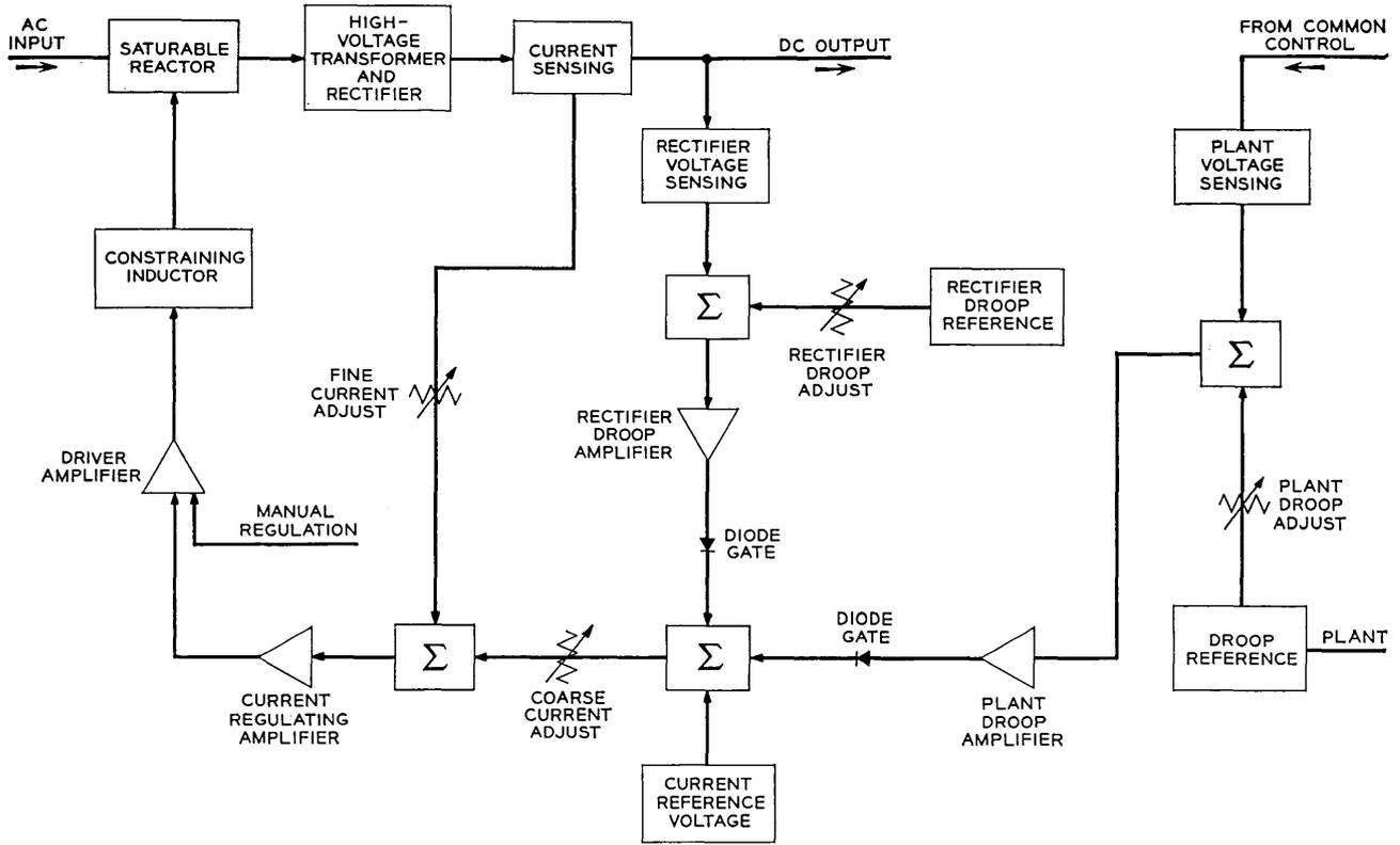
Fig. 8 — Rectifier feedback regulator functional block diagram.
