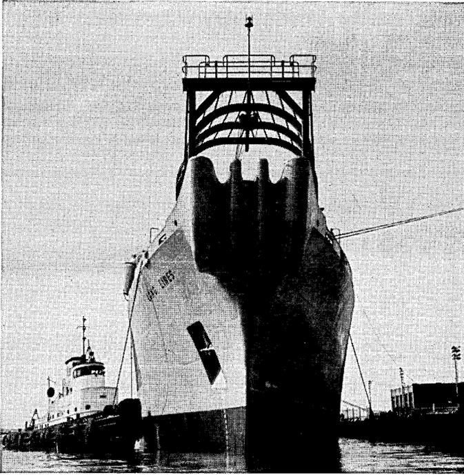
Fig. 10 — Bow sheaves of C.S. *Long Lines*.
