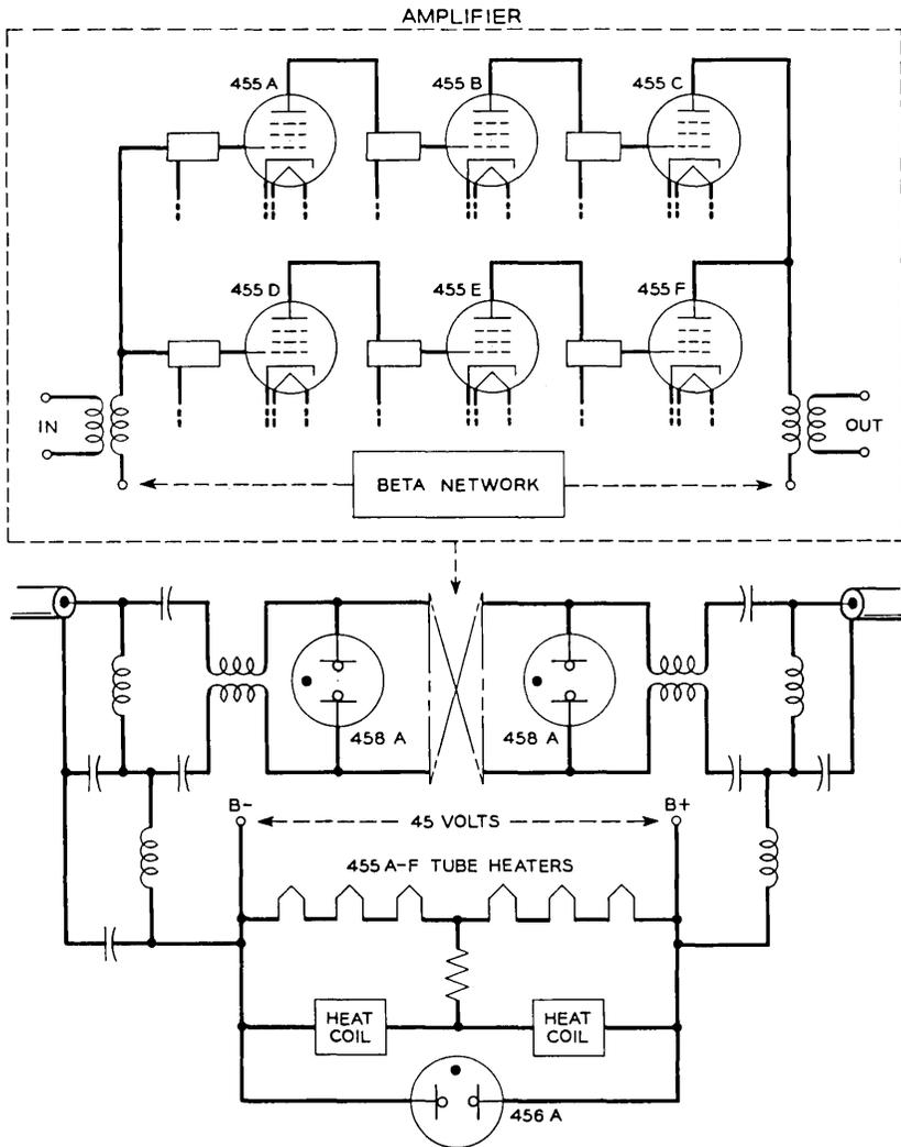
Fig. 5 — Functional location of the electron tubes in the SD submarine cable system repeater.
