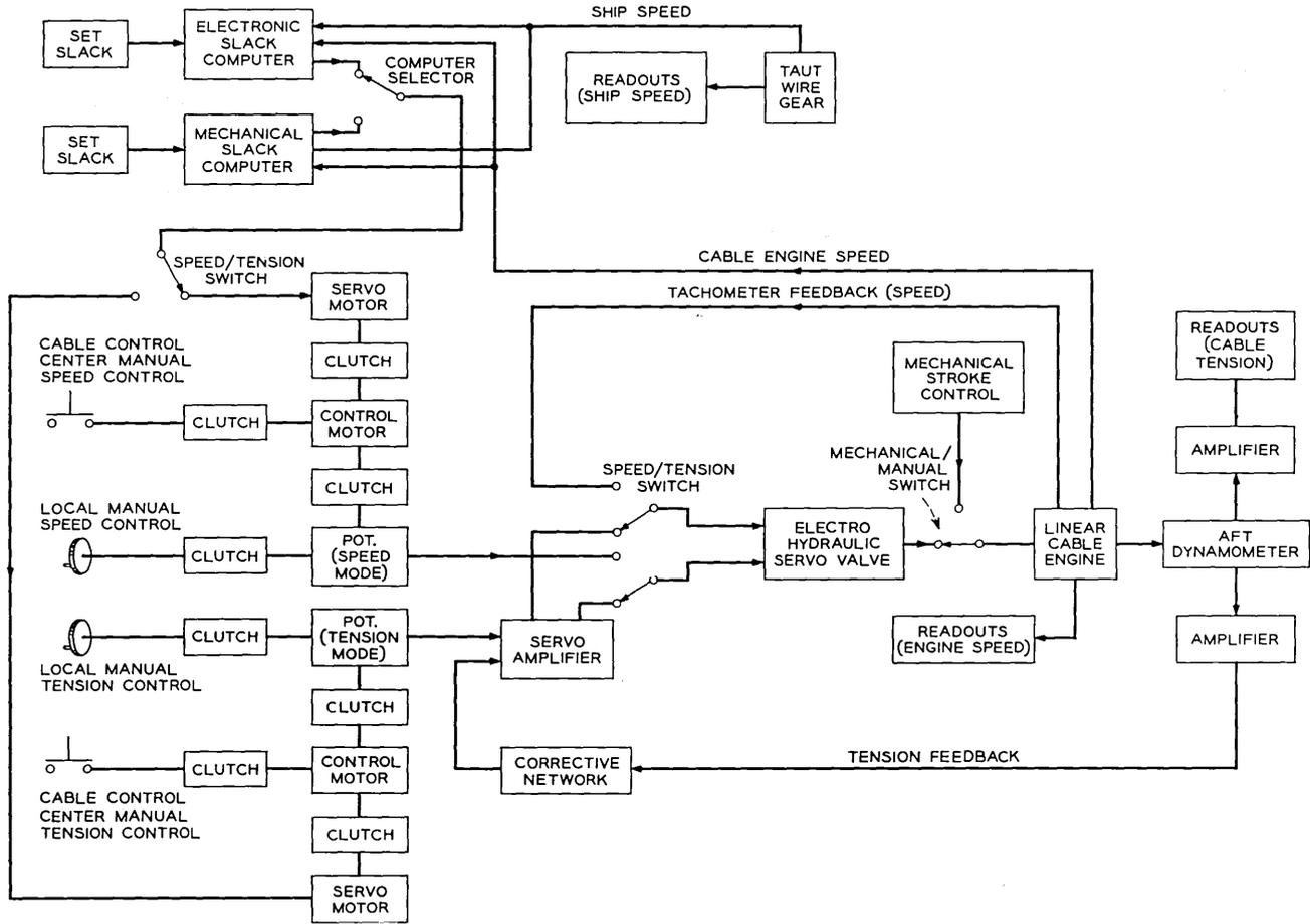
Fig. 18 — Cable engine control system.
