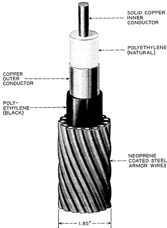
Fig. 2 — SD cable for shallow water.
