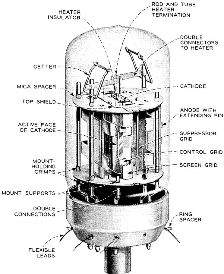
Fig. 1 — Structural details of the 455A-F electron tube.
