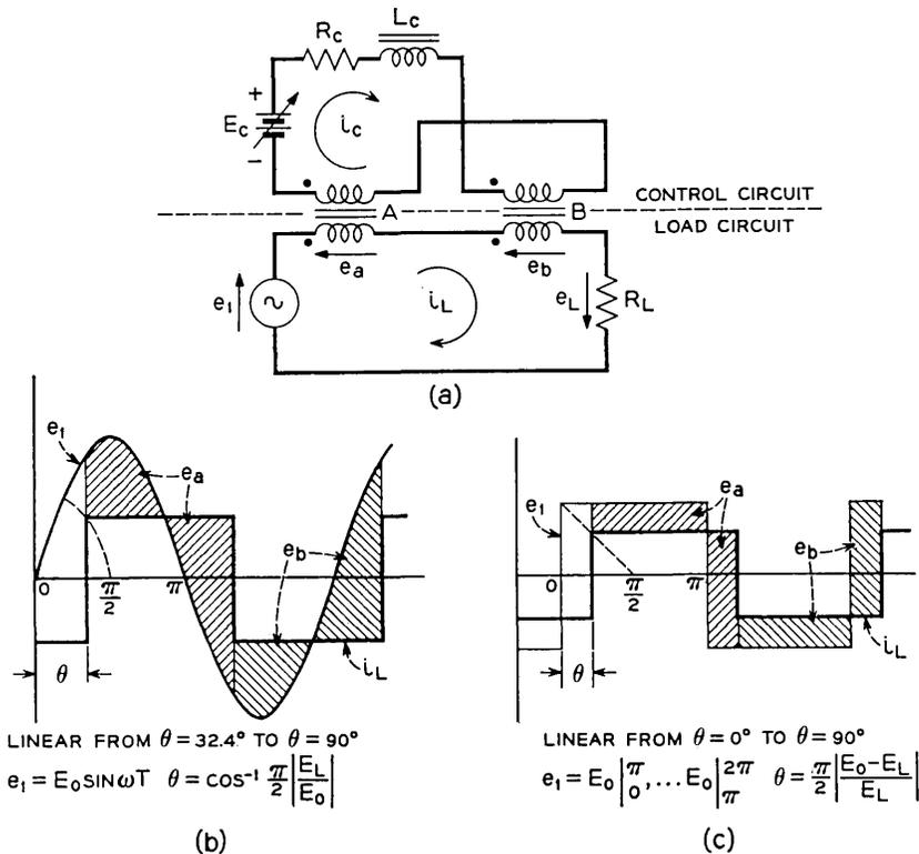
Fig. 5 — Saturable reactor regulator circuit: (a) schematic, (b) waveforms with sinusoidal excitation, (c) waveforms with square-wave excitation.
