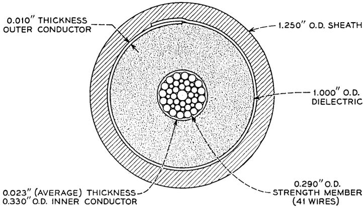
Fig. 6 — Cross section of armorless ocean cable.
