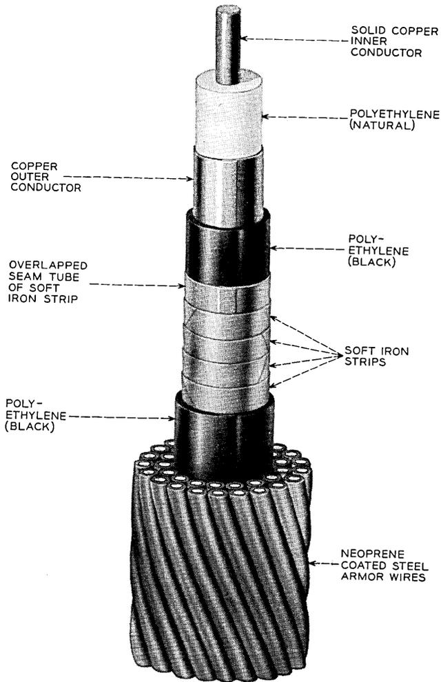
Fig. 5 — SD cable for shore ends, maximum protection.
