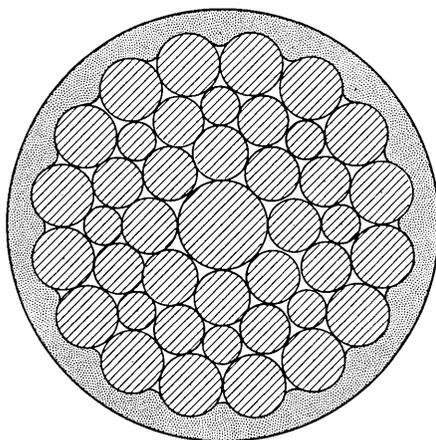
Fig. 4 — Cross section of finished conductor.
