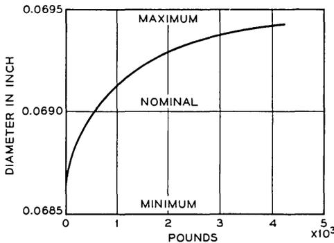
Fig. 2 — Wire diameter changes due to die wear.
