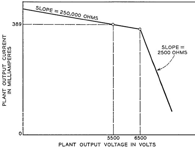
Fig. 9 — Power plant voltage-current characteristic curve.
