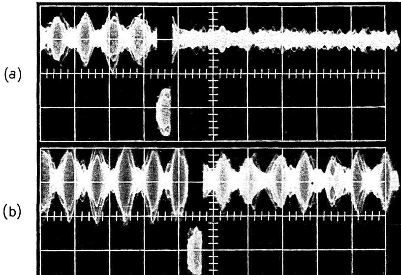
Fig. 16 — Repeater fault locating test set displays: (a) pulse returns from repeaters 178-182 — the pulse from the last repeater in the system (182) has been displaced for identification; (b) returns from repeaters 165-178 — repeater 171 has been displaced for identification.
