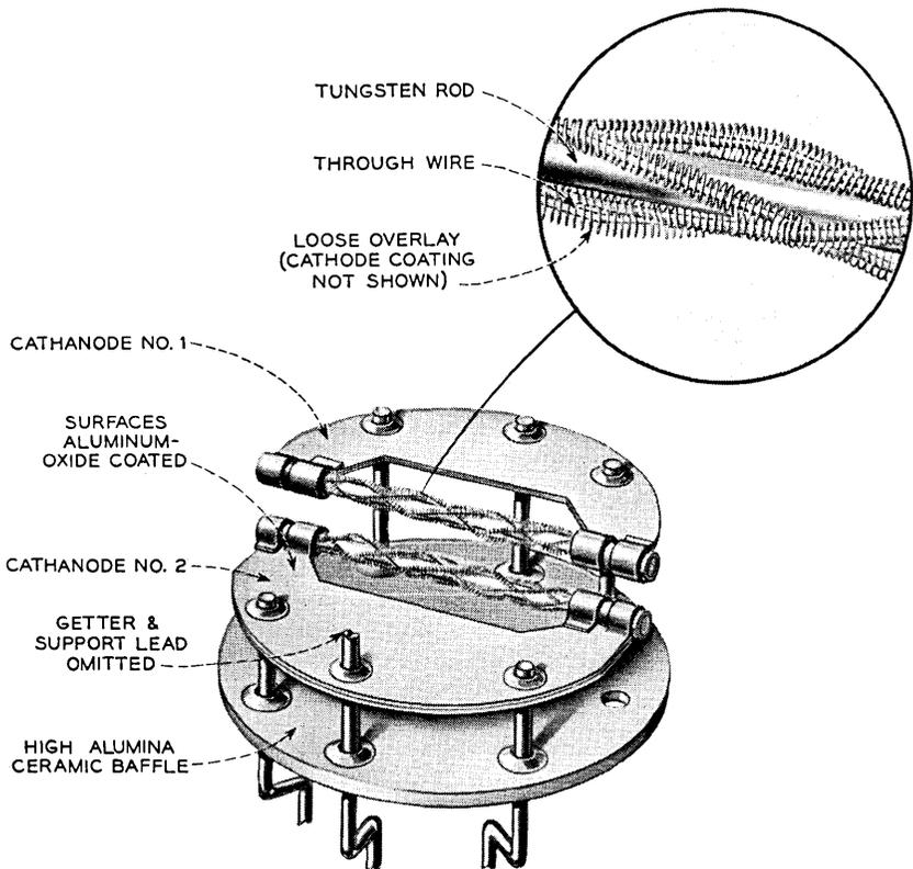
Fig. 10 — Structural features of the 456A tube.
