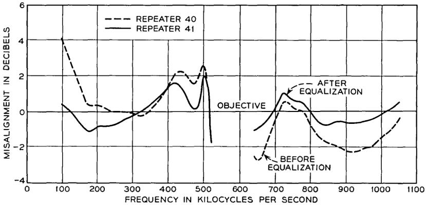
Fig. 11 — Reduction of misalignment by an ocean-block equalizer.
