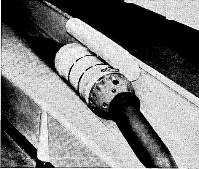
Fig. 8 — Repeater ready for launching with attached parachute.
