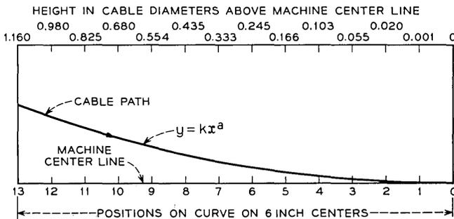
Fig. 13 — Path of cable through forming mill.
