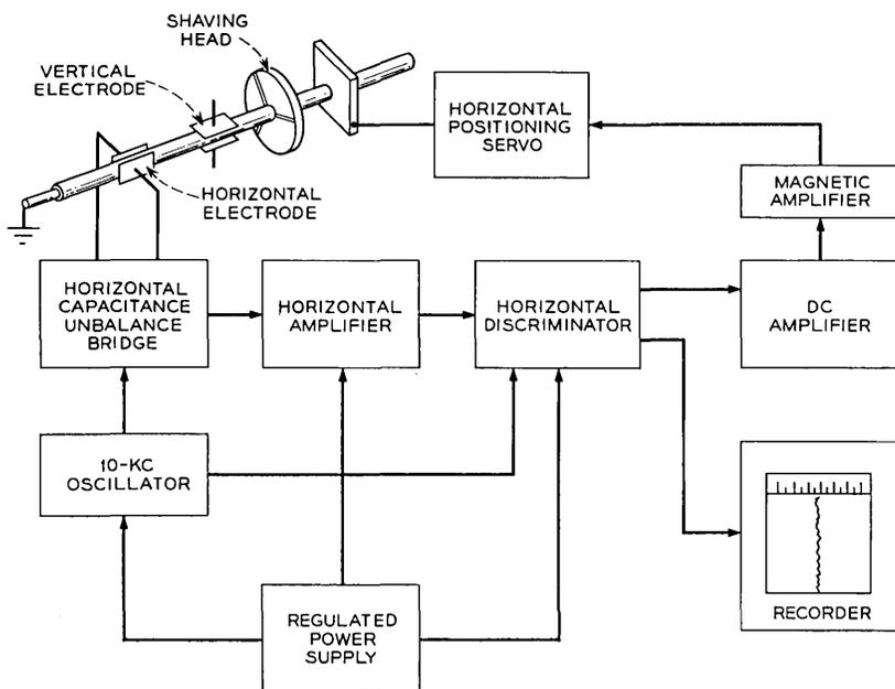
Fig. 12 — Shaver eccentricity control system — horizontal half.
