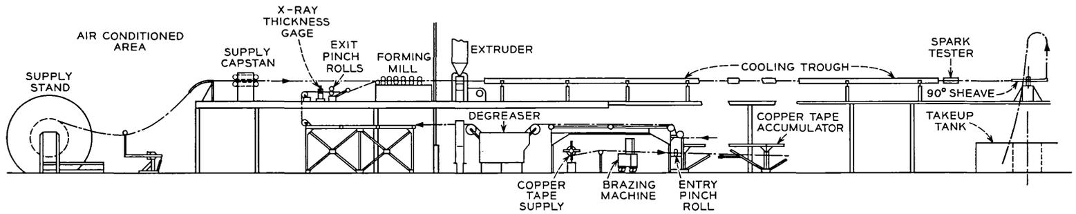
Fig. 15 — Elevation of outer conductor forming and jacketing line.
