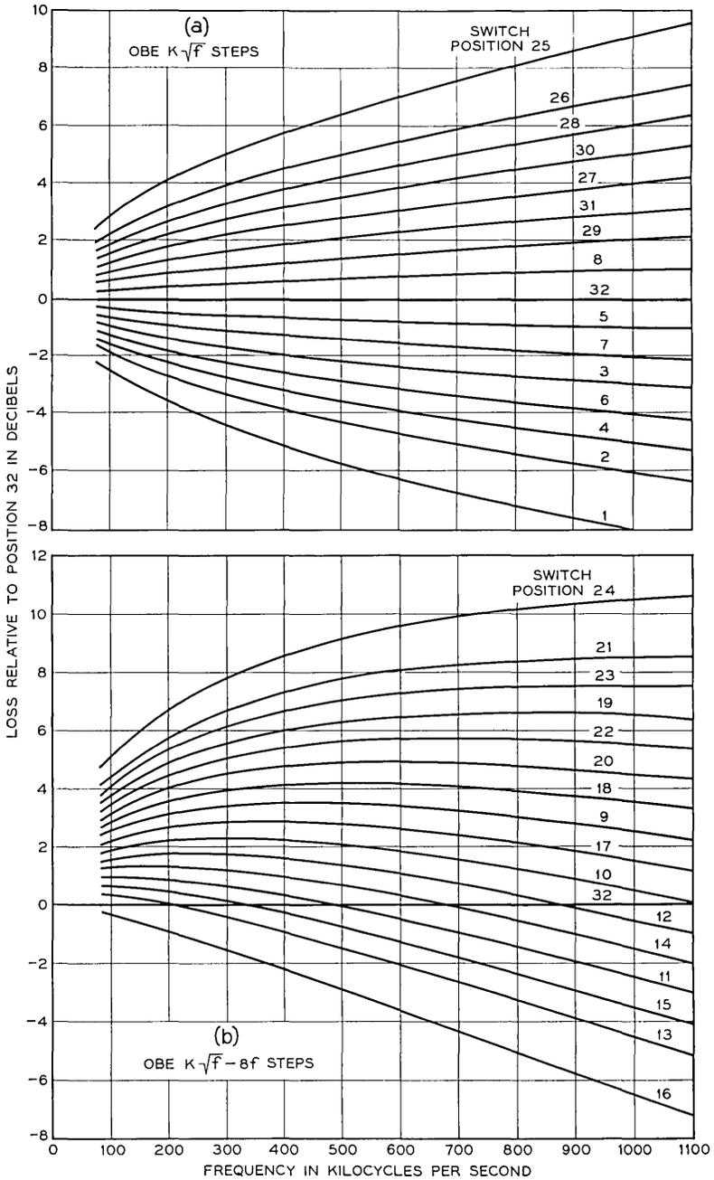
Fig. 10 — Ocean-block equalizer shapes.
