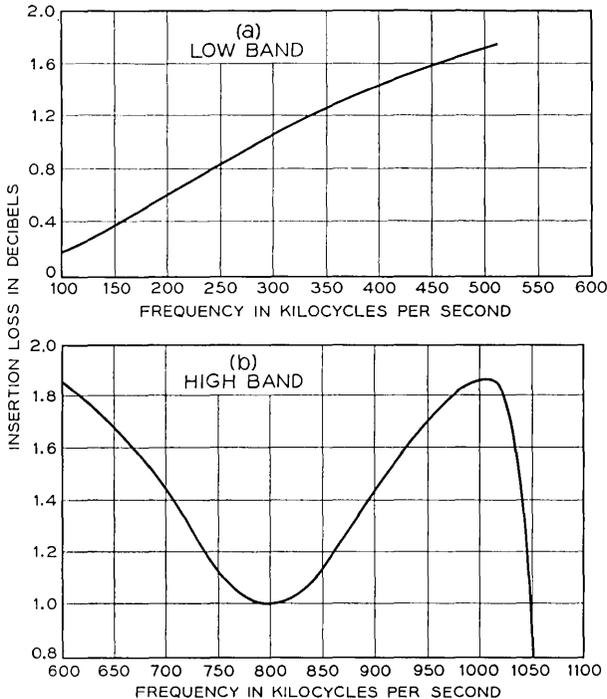
Fig. 12 — Transmitting basic equalizer shape.
