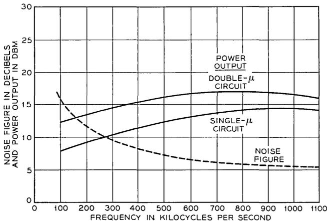
Fig. 6 — Repeater power output and noise figure.
