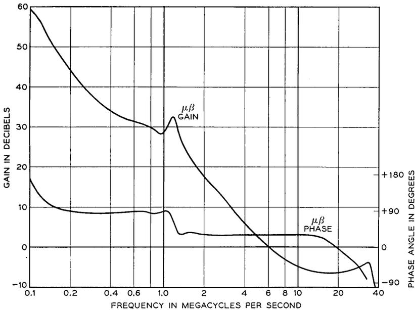
Fig. 4 — Amplifier feedback characteristics.
