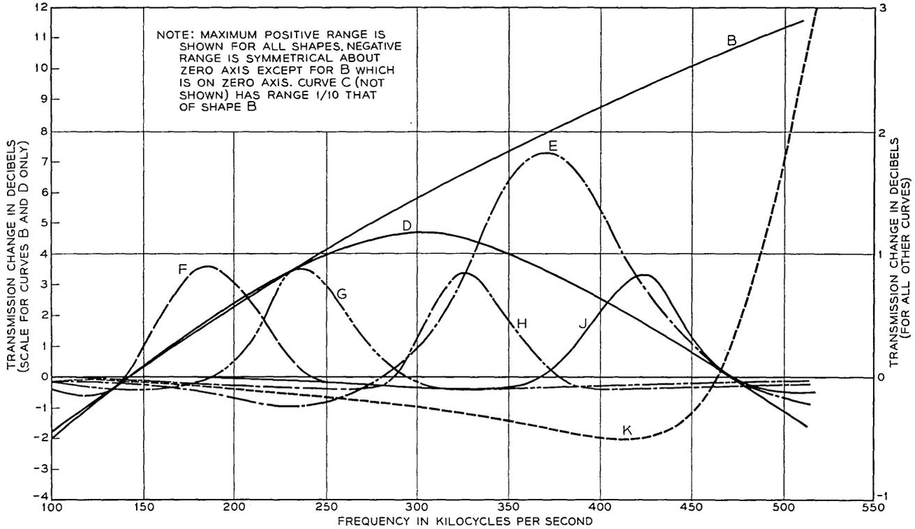
Fig. 13 — Transmitting general equalizer shape.
