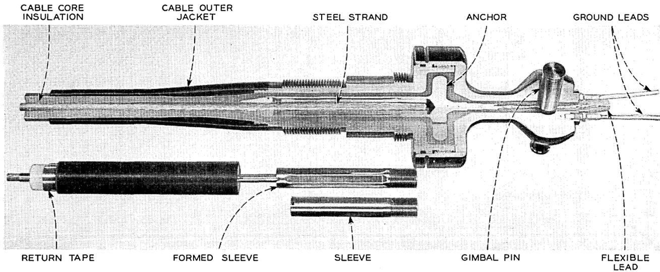
Fig. 17 — Repeater-cable coupling.
