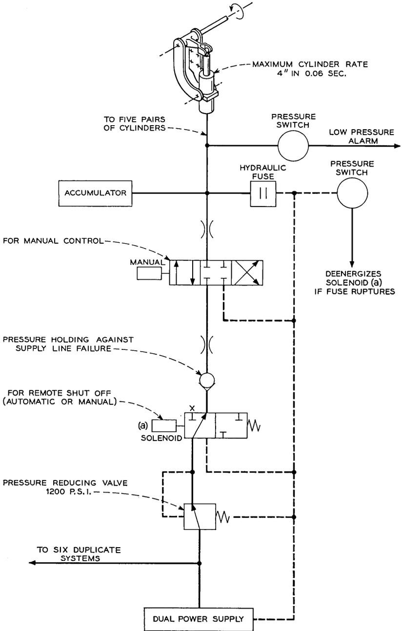
Fig. 10 — Schematic of hydraulic squeezing system.
