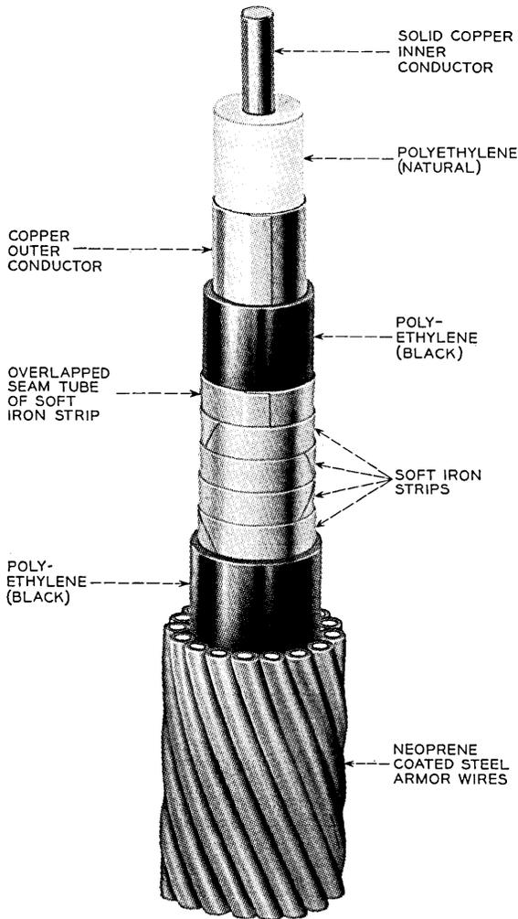
Fig. 4 — SD cable for shore ends.
