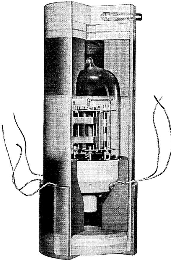
Fig. 2 — 455A-F tube cushioned in a methacrylate housing.
