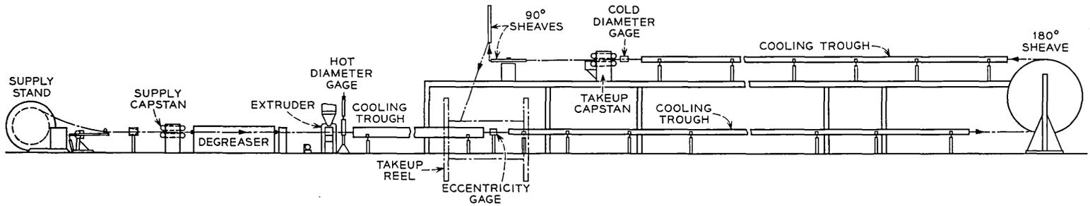
Fig. 9 — Elevation of ocean cable dielectric line.
