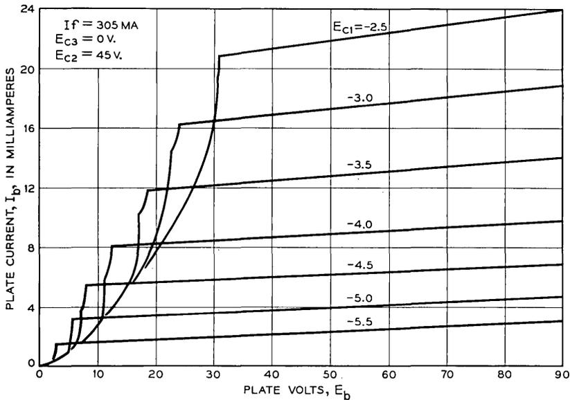
Fig. 6 — Plate current-plate voltage characteristics for the 455A-F electron tube.
