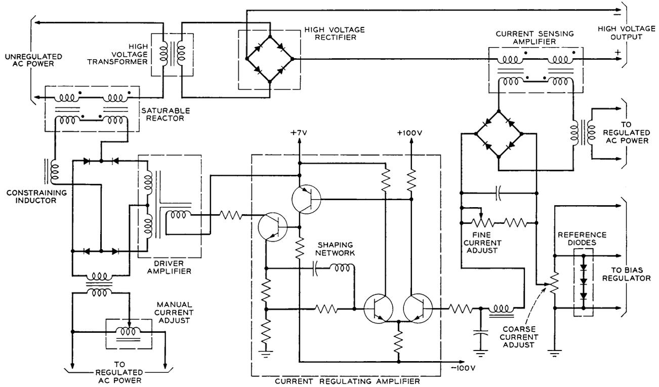
Fig. 7 — Current regulating feedback circuit.
