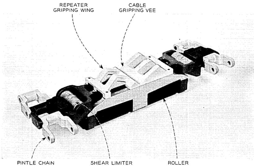
Fig. 6 — Model of roller carriage.
