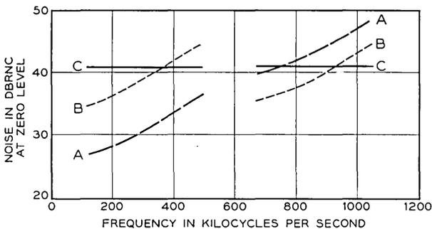
Fig. 8 — Effect of signal shaping on random noise.
