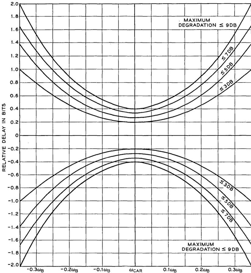
Fig. 25 — Design curve no. III. Maximum allowable delay for  $\alpha_{ps}/K = 8$  to give indicated degradation:
