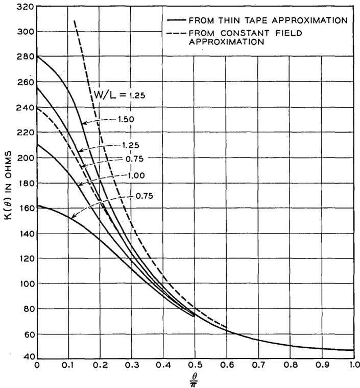
Fig. 2 — The impedance of the finger vs  $\theta$ . It is assumed that  $L - l = l = d$ .
