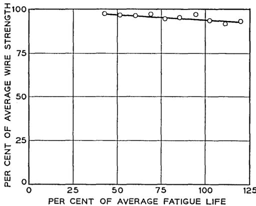
Fig. 18 — Ultimate strength as a function of bending fatigue life for percussive welded connections, test number 15 (without insulation).
