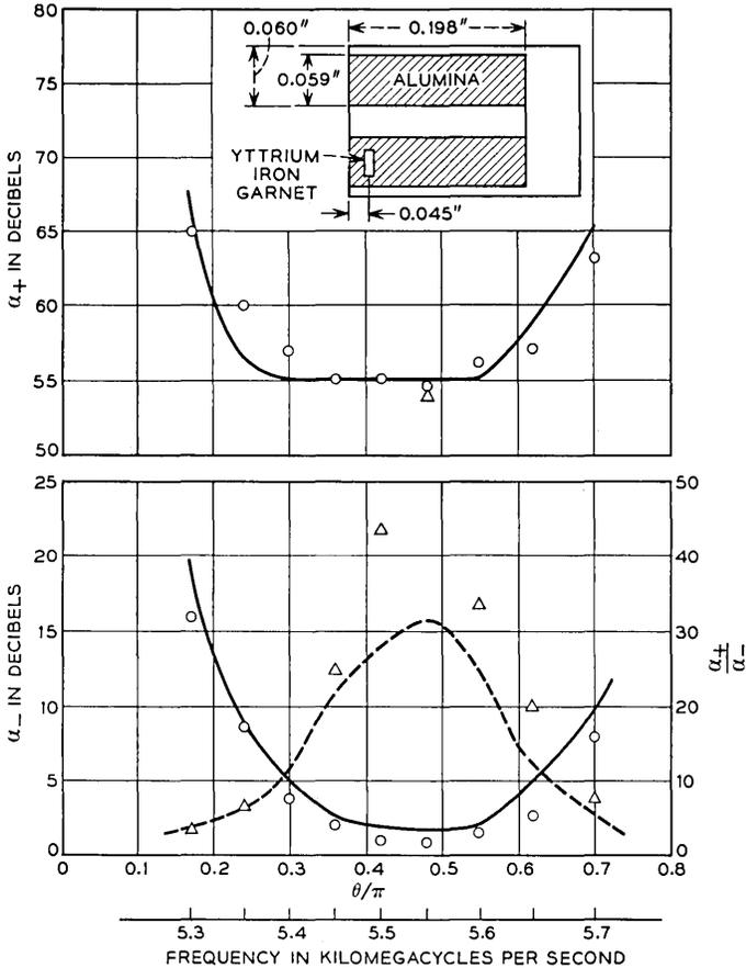
Fig. 15 — Measured and calculated forward and reverse losses. Ferrite disks  $0.02 \times 0.02 \times 0.002$  inch (71 pieces).  $L = 0.08$  inch,  $D = 0.06$  inch,  $l = 0.04$  inch,  $a = 0.016$  inch,  $\Delta H = 223$  oe,  $4\pi M = 1750$  oe. Solid lines are the calculated  $\alpha_{\pm}$  and the circled points are measured. Broken line is the calculated  $\alpha_+/\alpha_-$  and the triangles are measured points.
