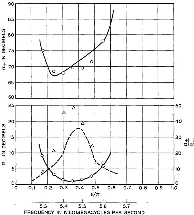
Fig. 16 — Measured and calculated forward and reverse absorption. Ferrite size:  $0.02 \times 0.02 \times 0.002$  inch (71 pieces).  $L = 0.08$  inch,  $D = 0.06$  inch,  $l = 0.04$  inch,  $a = 0.01$  inch,  $\Delta H = 223$  oe,  $4\pi M = 1750$  oe. Solid lines are the calculated  $\alpha_{\pm}$  and the circled points are measured. Broken line is the calculated  $\alpha_{+}/\alpha_{-}$  and the triangles are measured points.
