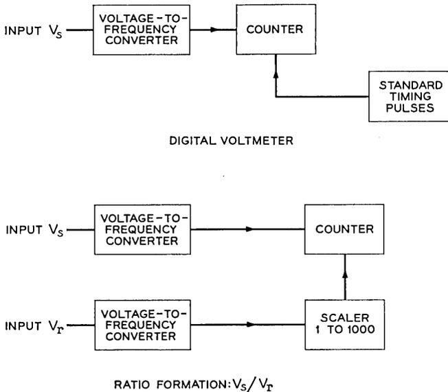
Fig. 5 — Method of ratio formation.
