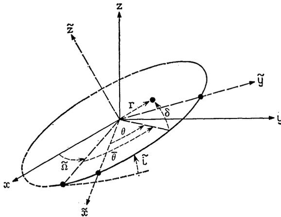
Fig. 4 — Rotating spherical orbital coordinates.
