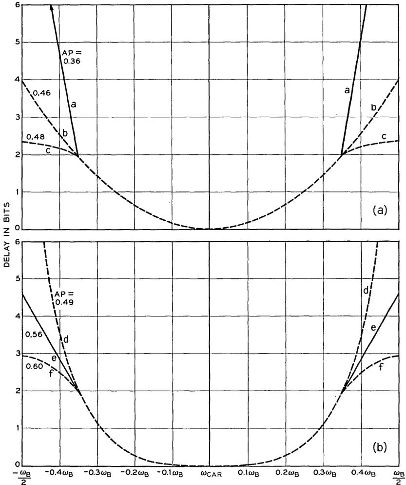
Fig. 22 — Bandwidth requirements, all curves symmetric about  $\omega_{car}$ : (a) quadratic delay, (b) fourth-power delay.
