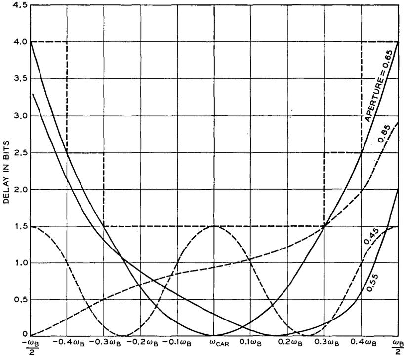
Fig. 21 — Examples of performance range meeting classical delay requirements; frequency in multiples of bit speed from carrier.
