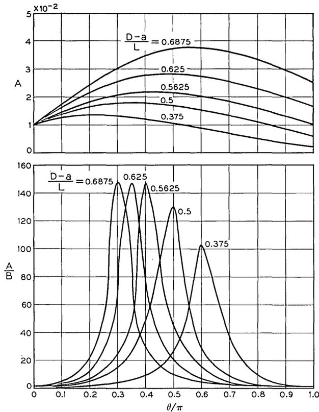
Fig. 12 —  $A$  and  $A/B$  vs  $\theta/\pi$  for the following parameters:  $D/L = 0.75$ ,  $l/L = 0.5$ ; ferrite size,  $(b - a)/L = (d - c)/L = 0.125$  ( $0.01 \times 0.01$  inch);  $(d + c)/L = 1.0$  (ferrite on an axis midway between the adjacent fingers).
