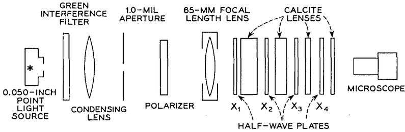
Fig. 8 — Pictorial diagram of four-unit deflection system.
