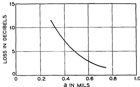
Fig. 6 — Loss vs radius of aperture at  $f/15$  and  $6943 \text{ \AA}$ .
