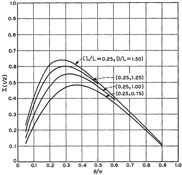
Fig. 3 —  $\Sigma(\frac{1}{2})$  vs  $\theta/\pi$  for  $l/L = 0.25$  and four values of the parameter  $D/L$ .
