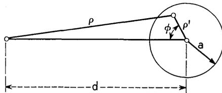
Fig. 17 — Circle of integration for determining crosstalk ratio and loss.
