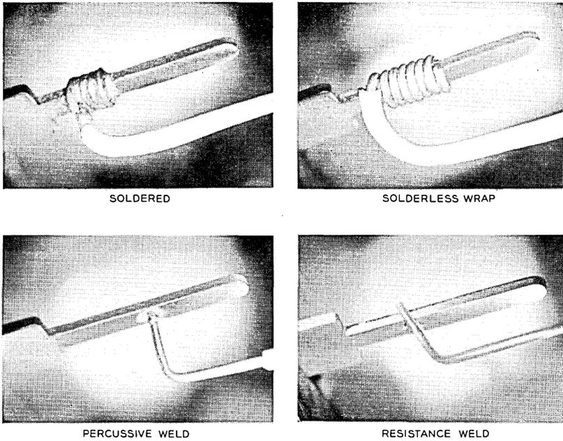
Fig. 3 — Typical examples of general wiring connections.
