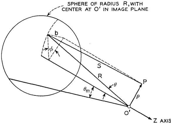
Fig. 16 — Angles and dimensions used to determine  $E(\rho)$ .
