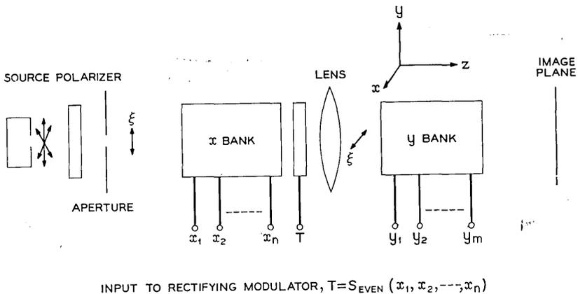
Fig. 4 — Incorporation of  $x$  bank and  $y$  bank into lens system.
