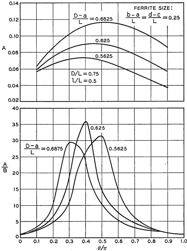
Fig. 13 —  $A$  and  $A/B$  vs  $\theta/\pi$ :  $D/L = 0.75$ ,  $l/L = 0.5$ ; ferrite size,  $(b - a)/L = (d - c)/L = 0.25$  ( $0.02 \times 0.02$  inch).
