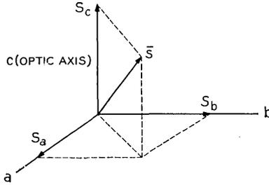
Fig. 14 — Wave normal and the crystallographic direction in the uniaxial media.
