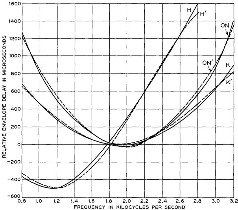
Fig. 16 — Representations of some typical lines by sinusoidal approximations (primes are approximations). K = 2 links K carrier, ON = 3 links ON carrier, and H = 300 miles of H44 loaded cable.
