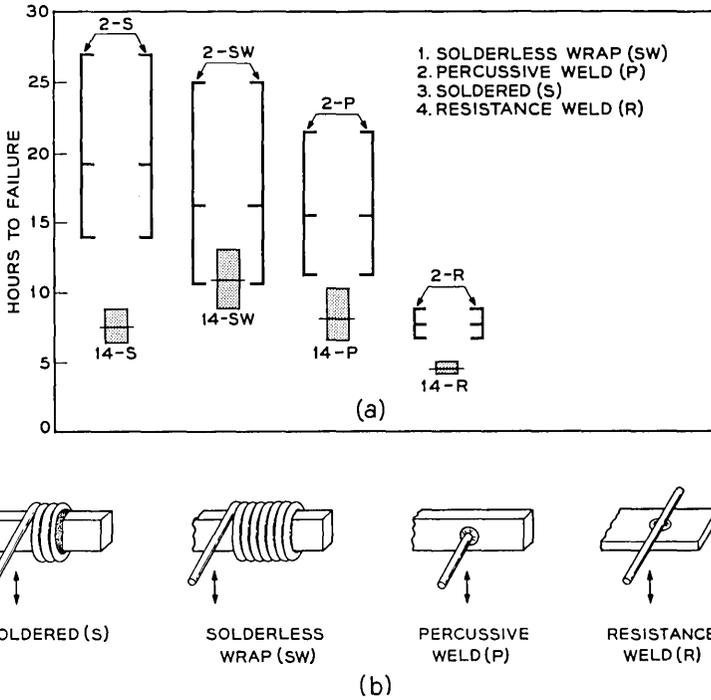
Fig. 17 — (a) Vibration fatigue life with configuration omitting 90° bend in the lead-off wire, test number 14 (with insulation); order of merit, based on vibration fatigue life. (b) Vibration configuration omitting 90° bend.
