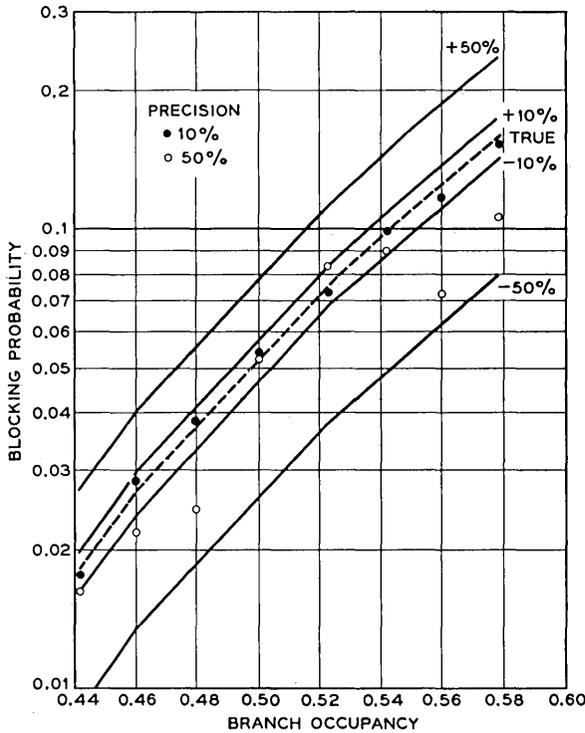
Fig. 10 — NEASIM blocking estimates for GRAPH of Fig. 3 vs branch occupancy  $p = p_2$ .
