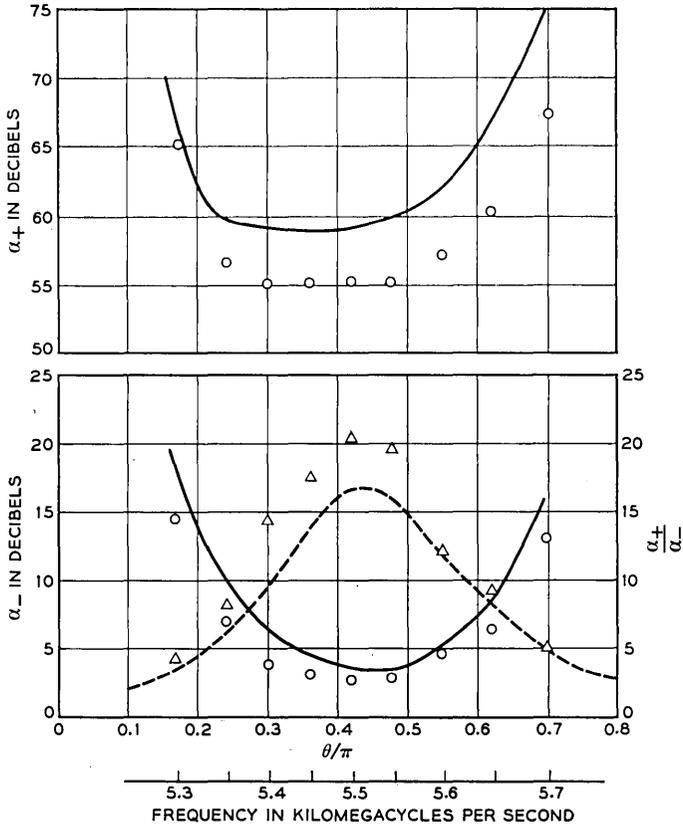
Fig. 17 — Measured and calculated forward and reverse absorption. Ferrite disks =  $0.03 \times 0.03 \times 0.002$  inch (35 pieces).  $L = 0.08$  inch,  $D = 0.06$  inch,  $l = 0.04$  inch,  $a = 0.009$  inch,  $\Delta H = 251$  oe,  $4\pi M = 1750$  oe. Solid lines are the calculated  $\alpha_{\pm}$  and the circled points are measured. Broken line is the calculated  $\alpha_+/\alpha_-$  and the triangles are measured points.
