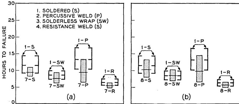
Fig. 10 — Vibration fatigue life after temperature tests. (a) Test number 7 (central office conditions); (b) test number 8 (outside plant conditions). The order of merit, based on vibration fatigue life, was the same for both tests.
