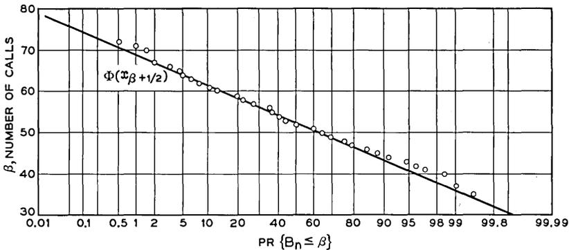
Fig. 8 — Cumulative distribution for GRAPH of Fig. 3 ( $p = p_2 = 0.5$ ) in a run of 201,600 calls in which the number of blocked calls was noted for every 1,008 calls run. The points are experimental data; the line is the theoretical distribution,  $\Phi(x_{\beta+\frac{1}{2}})$
