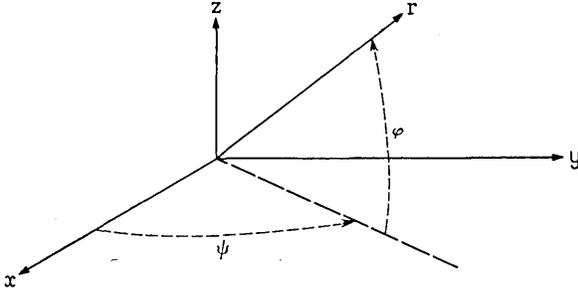
Fig. 2 — Equatorial spherical coordinate system.
