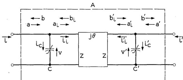
Fig. 1 — Basic configuration of the unilateral parametric amplifier.
