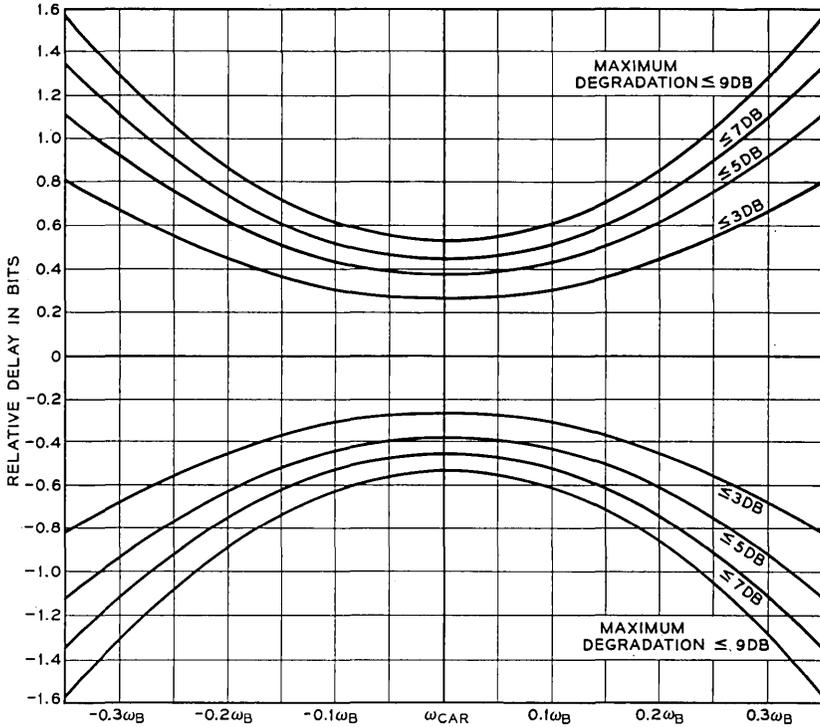
Fig. 24 — Design curve no. II. Maximum allowable delay for  $\alpha_{ps}/K = 4$  to give indicated degradation:
