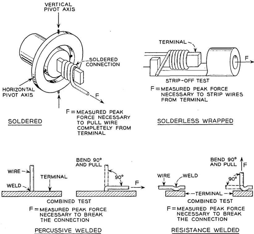
Fig. 23 — Destructive tests.
