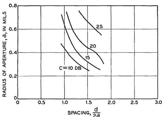
Fig. 5 — Radius of aperture vs center-to-center spacing at constant crosstalk,  $f/15$  and  $6943 \text{ \AA}$ .
