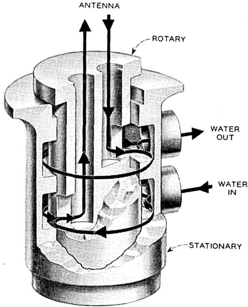
Fig. 11 — Rotary joint for chilled water system.
