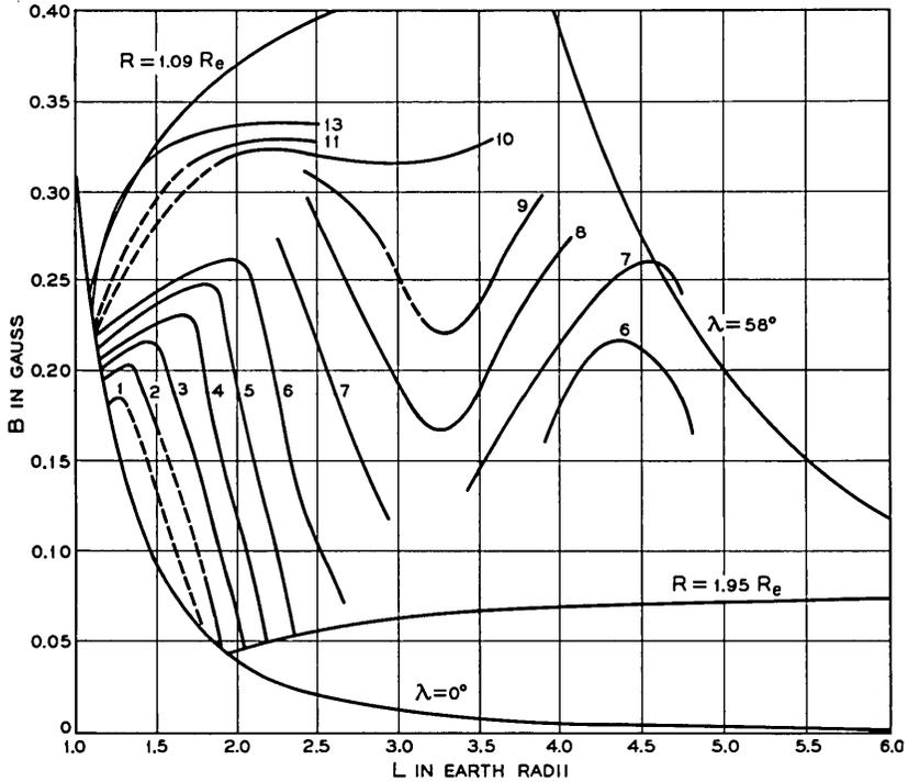
Fig. 10 — Contours of constant  $OCR$ , electron channel 3, days 203 to 207, 1962, plotted in  $B$ - $L$  coordinates. Dashed lines indicate extrapolations and interpolations. The lines  $R = 1.09 R_e$ ,  $R = 1.95 R_e$  and  $\lambda = 58^\circ$  define the approximate boundaries of the space swept out by the Telstar orbit.  $\Phi$  ranges are defined in Table I.
