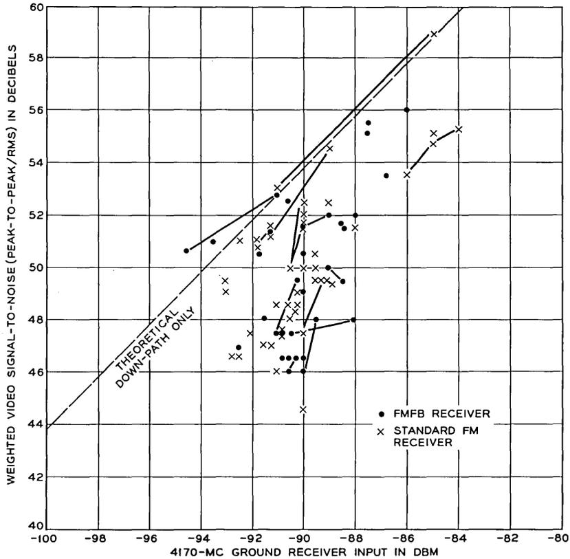
Fig. 24 — Video noise vs received carrier power.
