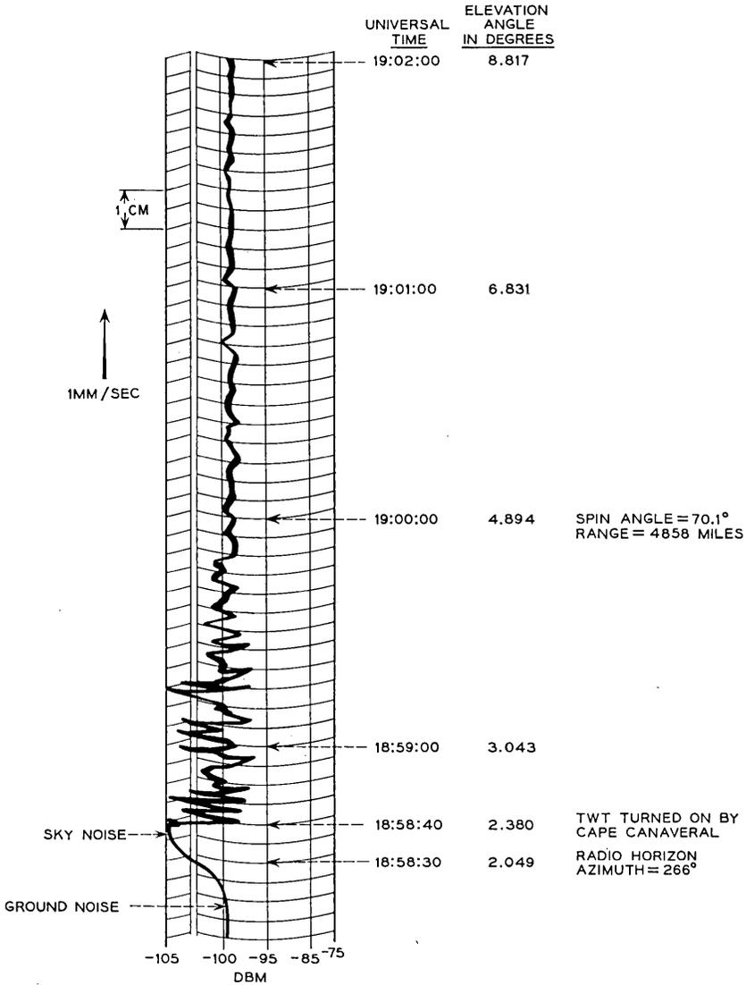
Fig. 8 — Low-angle fading at 4170 mc; pass 470, Aug. 30, 1962.
