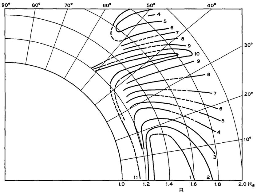
Fig. 8 — Contours of constant  $OCR$ , electron channel 3, days 263 to 267, 1962, plotted in  $R$ - $\lambda$  coordinates. Dashed lines indicate interpolations and extrapolations.  $\Phi$  ranges are defined in Table I.
