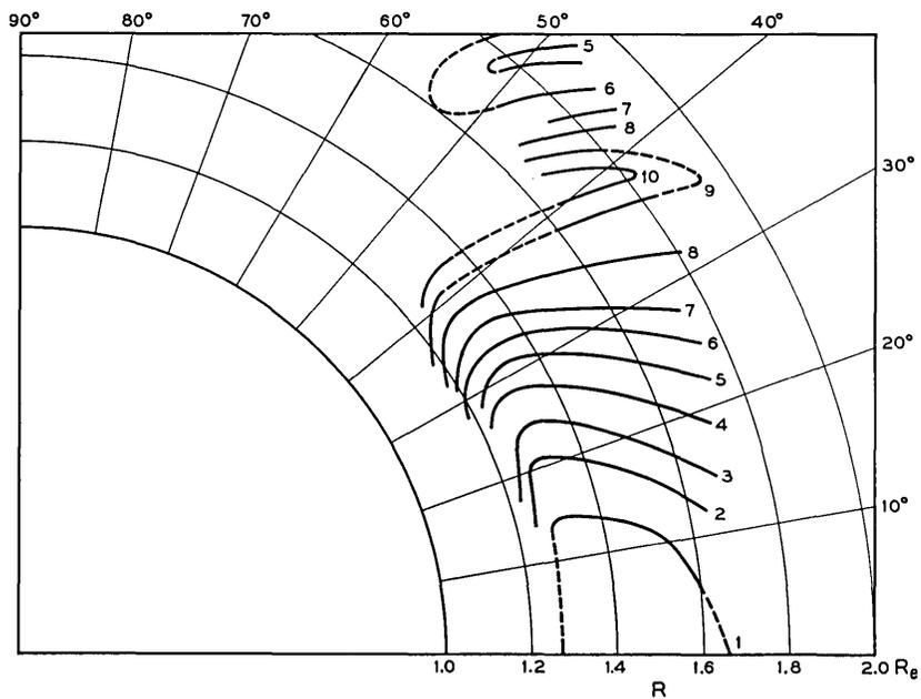
Fig. 7 — Contours of constant  $OCR$ , electron channel 3, days 238 to 242, 1962, plotted in  $R$ - $\lambda$  coordinates. Dashed lines indicate interpolations and extrapolations.  $\Phi$  ranges are defined in Table I.
