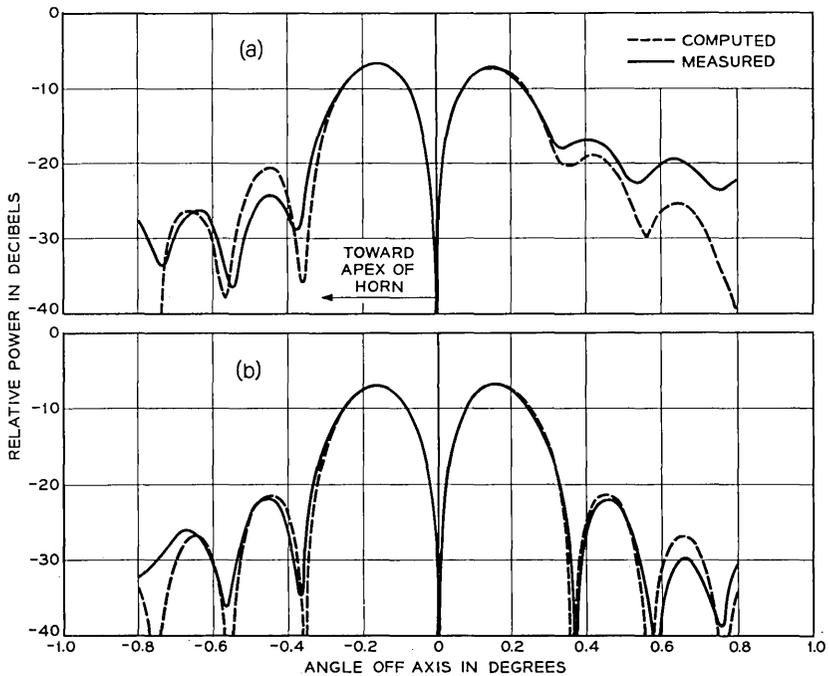
Fig. 13 — Radiation patterns of the full size antenna for  $TM_{01}$  mode: (a) in the longitudinal plane for the longitudinal component of the aperture field (the dashed curve is computed for the reduced range); (b) in the transverse plane for the transverse component of the aperture field (the dashed curve is the computed far-field pattern).
