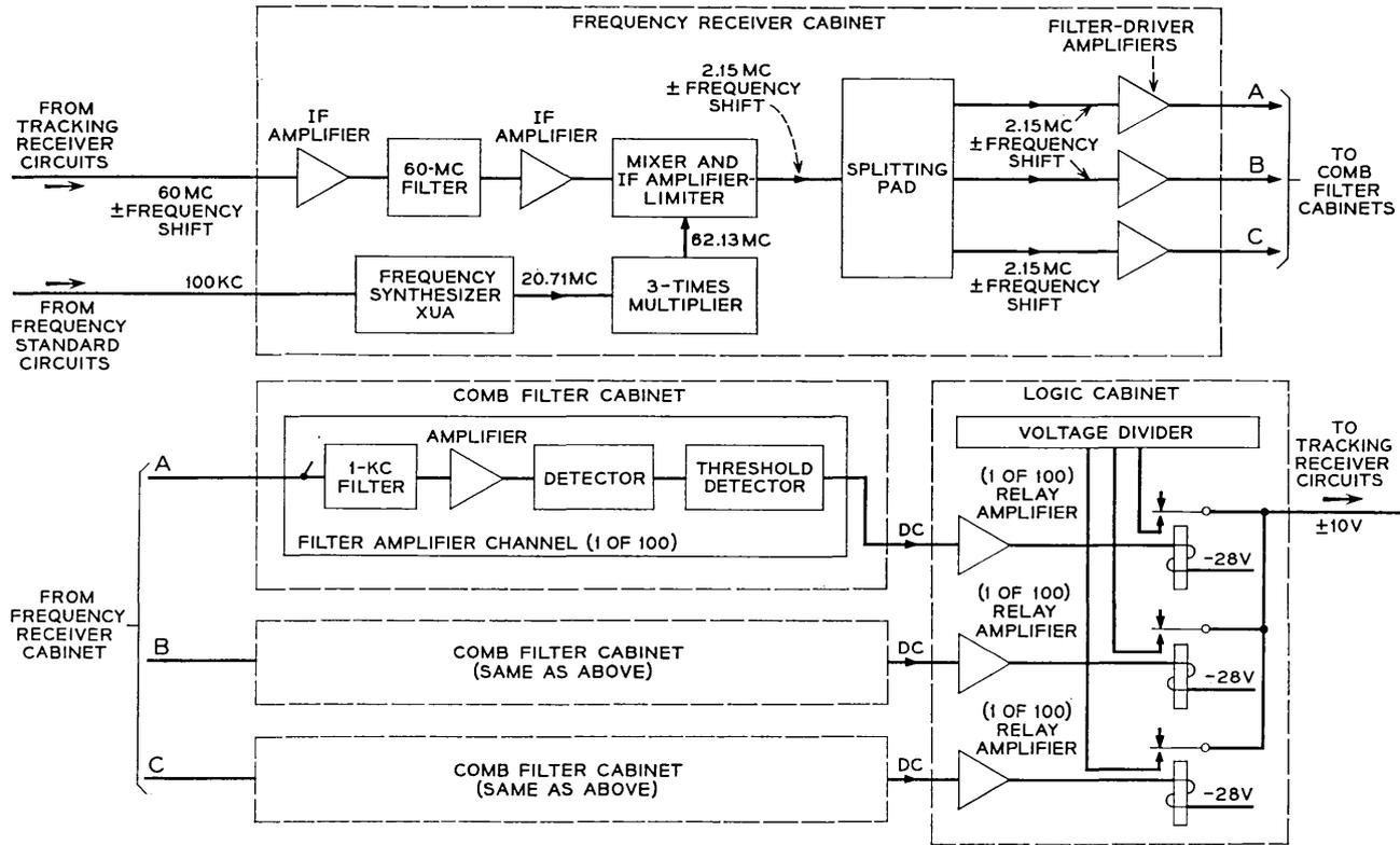
Fig. 17 — Acquisition receiver, block diagram.
