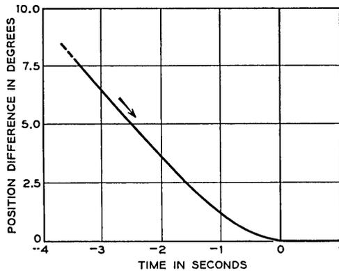
Fig. 18 — Servo system response in slew mode — azimuth.
