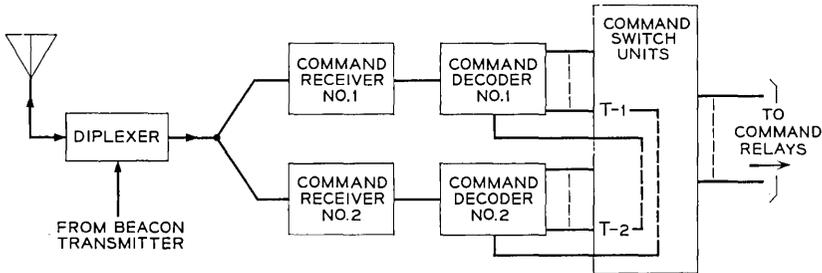
Fig. 1 — Block diagram of command system.
