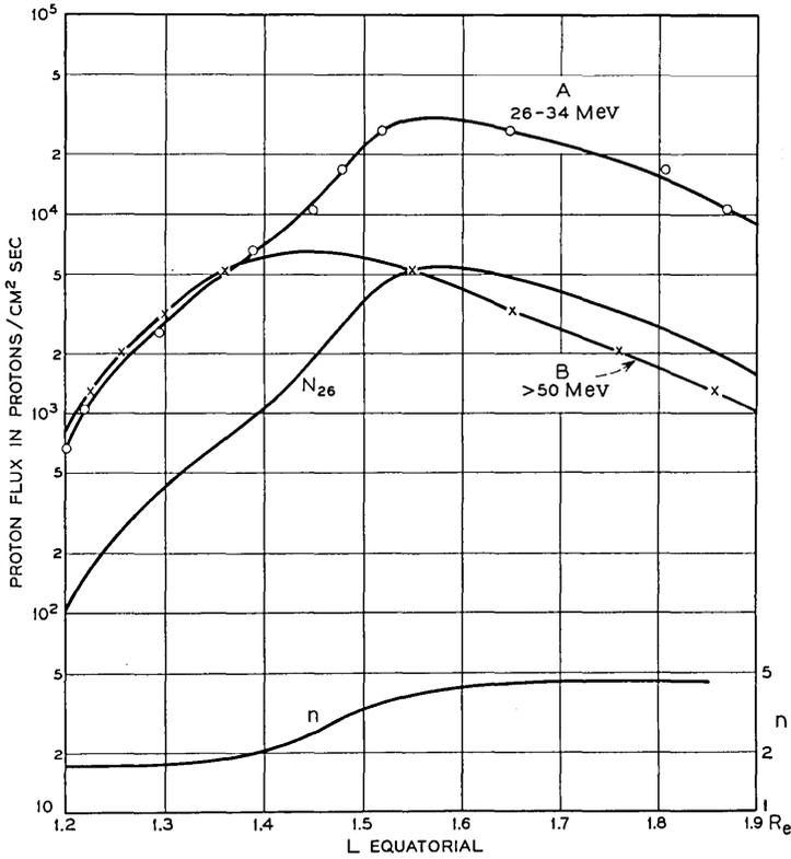
Fig. 19 — Equatorial proton flux. Curve A is for protons in the energy range 26 to 34 Mev, and curve B for protons with energies >50 Mev. *n* and *N*<sub>26</sub> are defined in the text.
