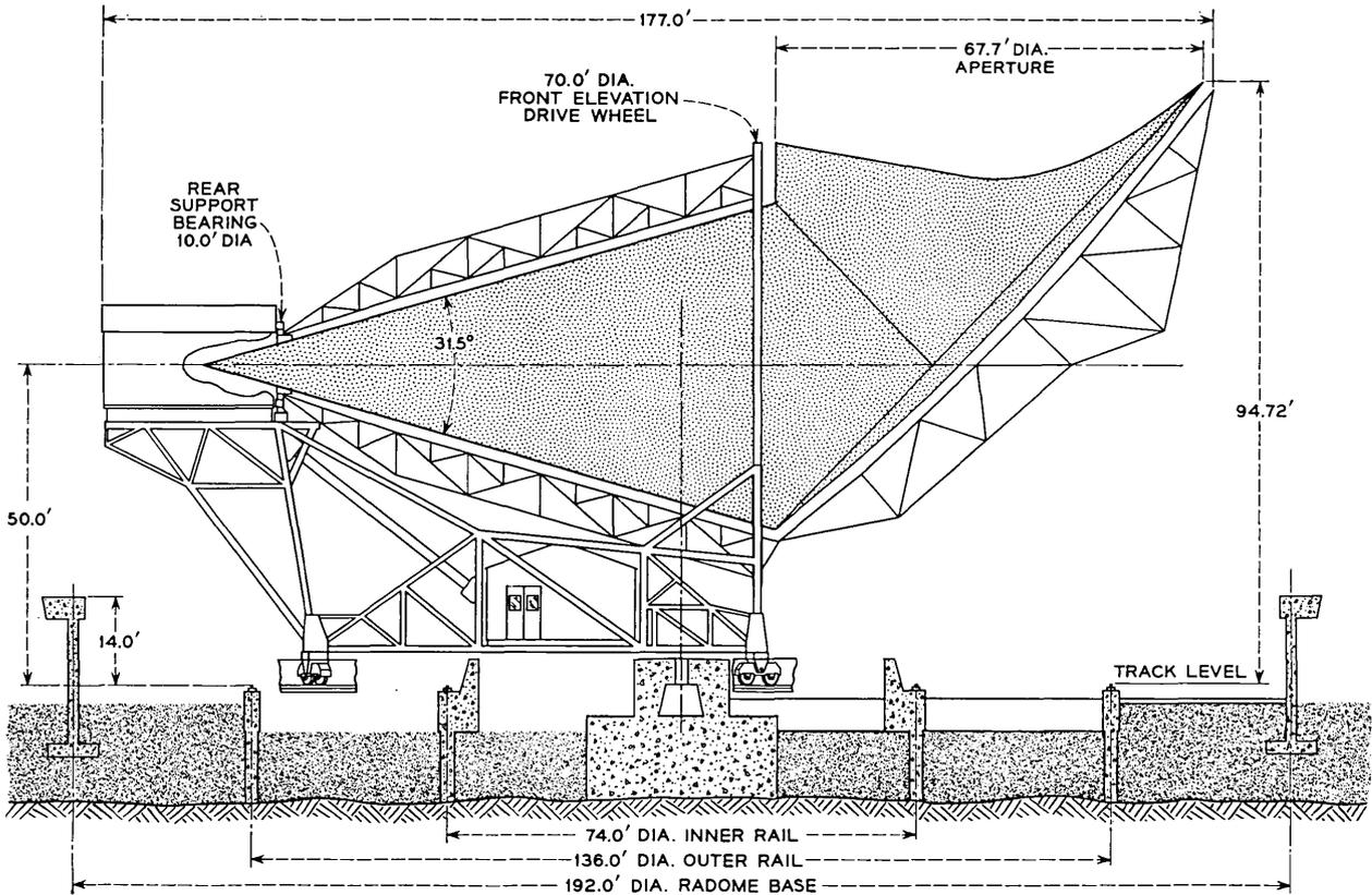
Fig. 6 — Outline drawing of horn-reflector antenna.
