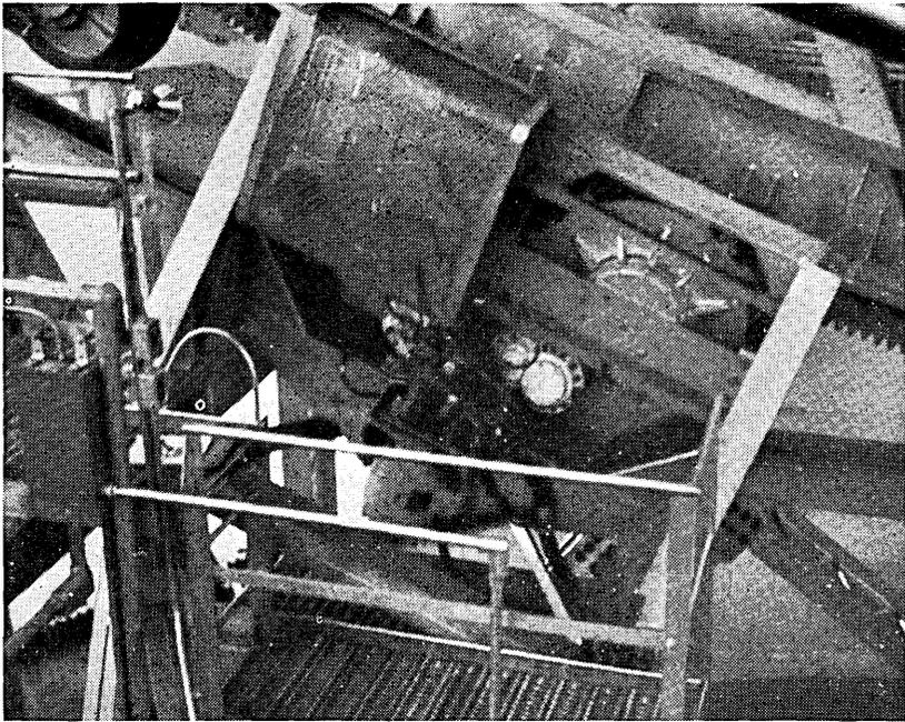
Fig. 21 — Left-hand elevation drive mounted on antenna structure.
