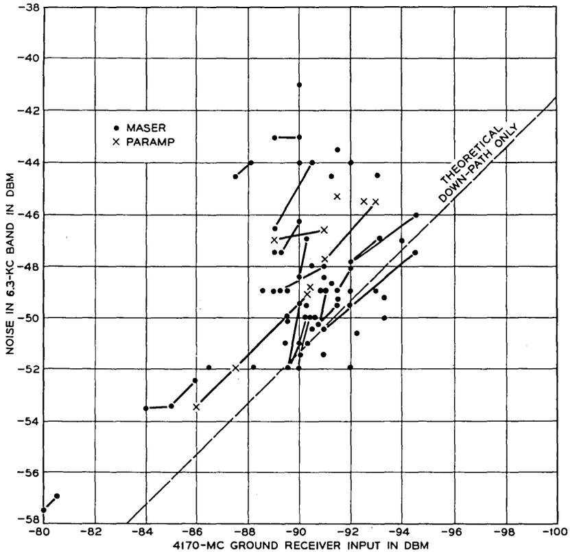
Fig. 23 — 6-mc noise vs received carrier power.
