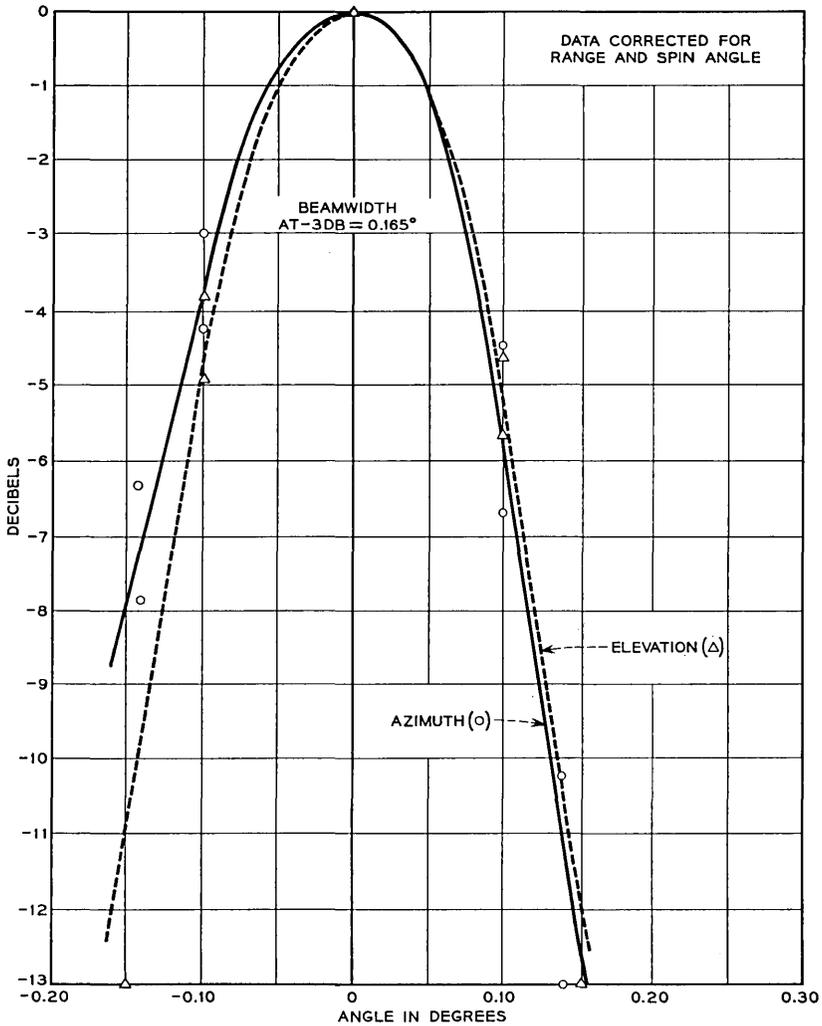
Fig. 13 — 6-kmc horn antenna pattern; pass 105, July 21, 1962.
