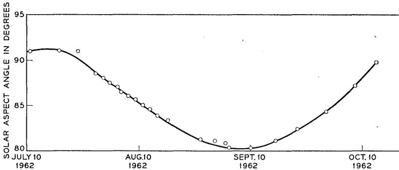
Fig. 1 — Telstar spacecraft — solar aspect angle versus time.
