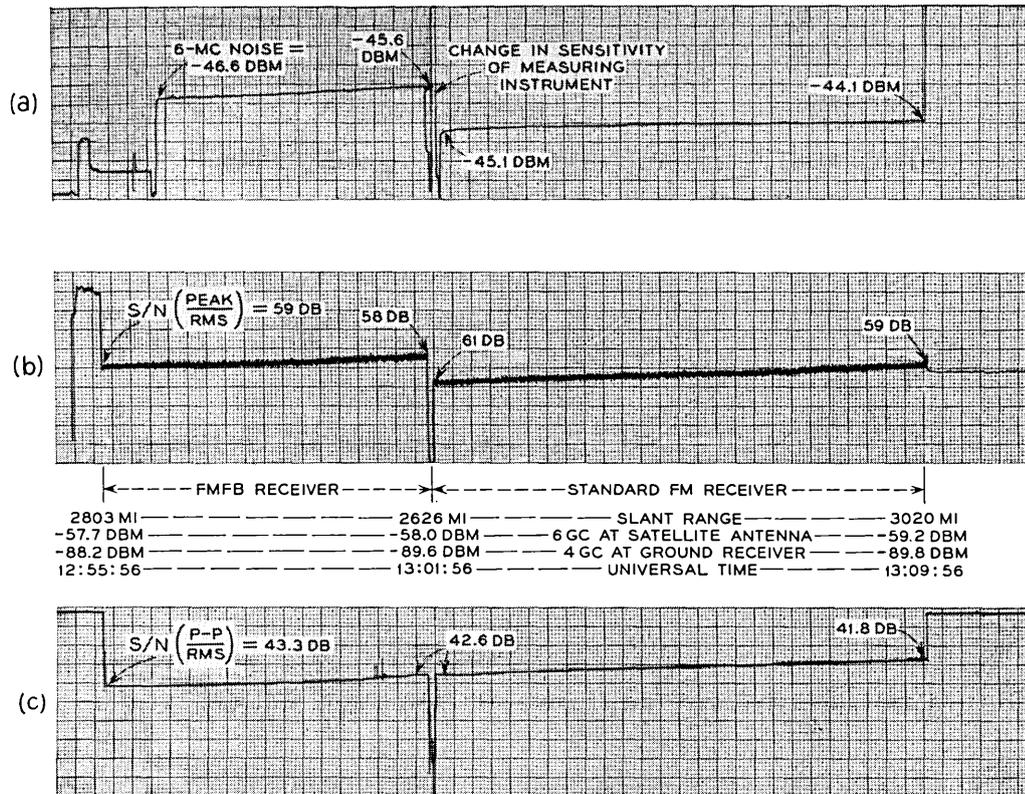
Fig. 22 — Baseband noise recordings; pass 988, Oct. 26, 1962. (a) Noise at 6 mc in 6.3-ke band; (b) weighted audio noise; (c) weighted video noise.
