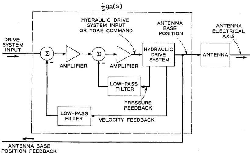
Fig. 2 — Functional diagram of drive system.
