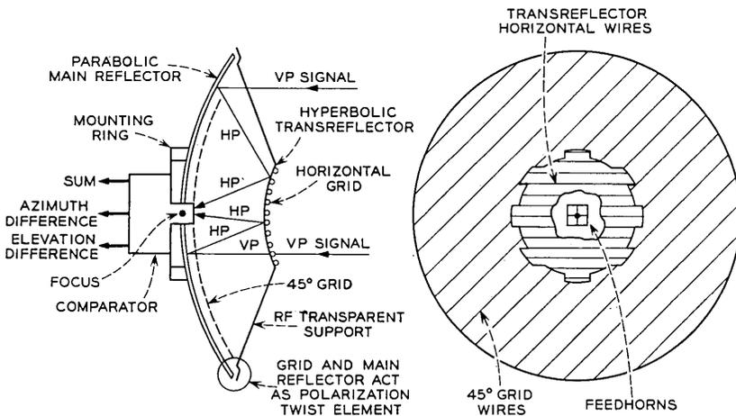
Fig. 4 — Cassegrainian antenna and twist reflector.
