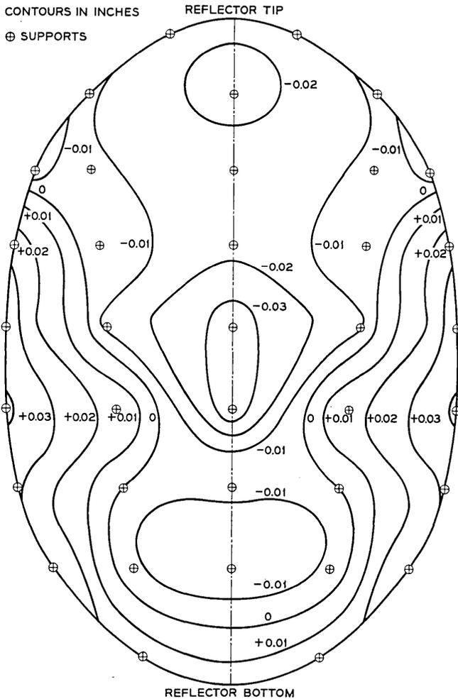
Fig. 10 — Elastic reflector contours.
