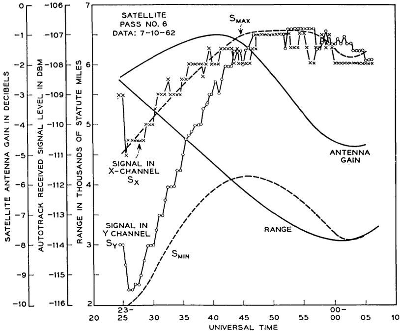
Fig. 17 — Received signal levels for Telstar satellite pass 6.
