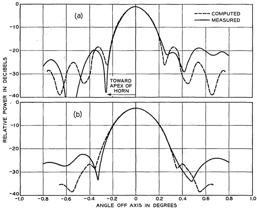
Fig. 11 — Principal radiation patterns of the full size antenna for  $TE_{11}$  mode in the longitudinal plane: (a) longitudinal polarization  $(TE_{11})_x$ ; (b) transverse polarization  $(TE_{11})_y$ . (The dashed curves are computed far-field patterns.)
