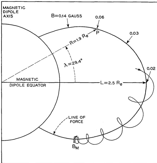
Fig. 2 — The motion of a charged particle trapped in a dipole magnetic field. The particle is confined near the magnetic shell  $L = 2.5 R_e$  and is mirroring at field strength  $B_m$ . The  $B$ - $L$  coordinates of the point  $P$  are  $B = 0.06$  gauss and  $L = 2.5 R_e$ . The  $R$ - $\lambda$  coordinates of the point  $P$  are  $R = 1.9 R_e$  and  $\lambda = 29.4^\circ$ . Distances are measured in units of earth radii,  $R_e$ .
