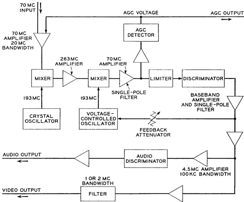
Fig. 2 — Block diagram of frequency compression demodulator.
