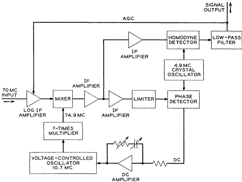
Fig. 3 — Block diagram of phase-locked loop.
