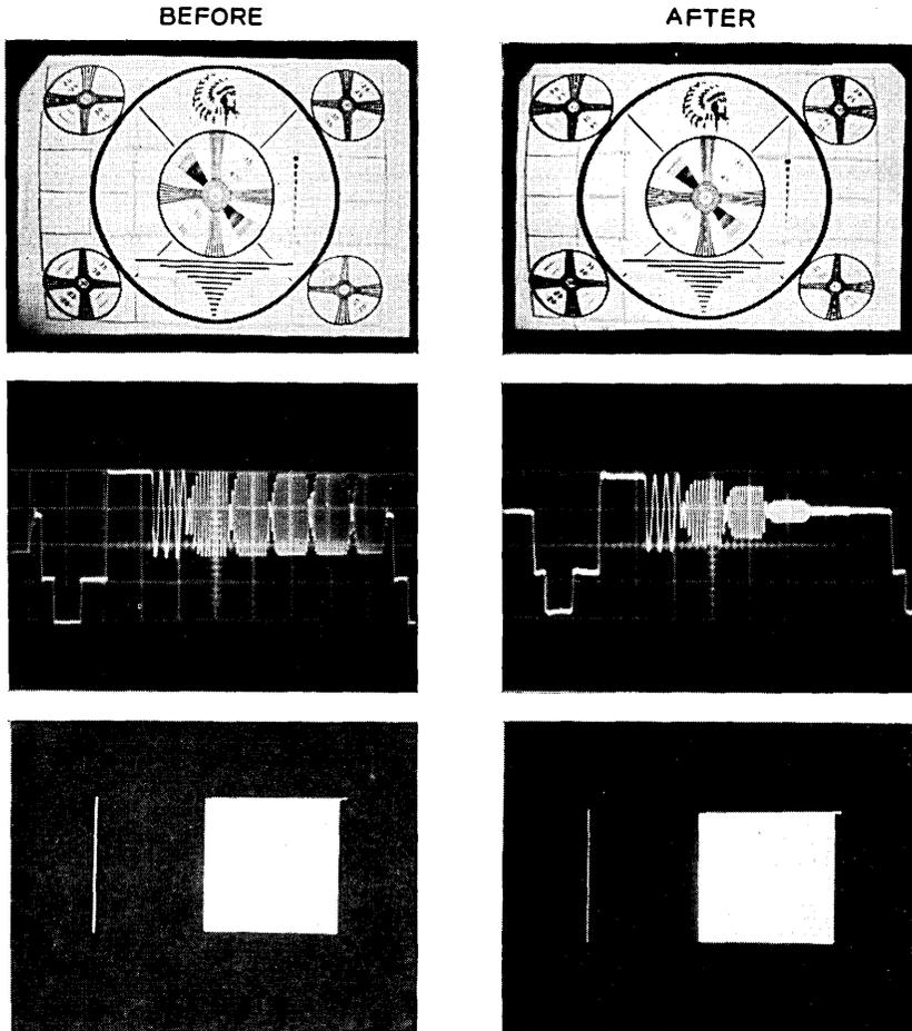
Fig. 18 — Effect of transmission on various test signals.
