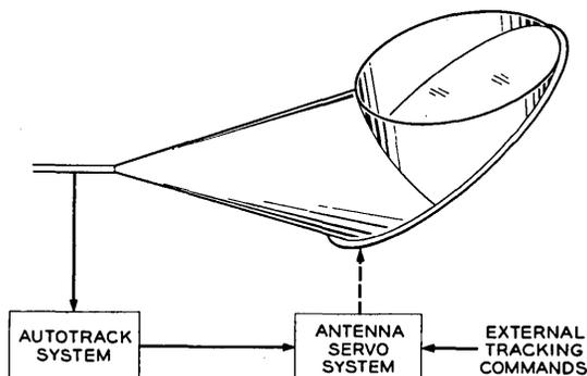
Fig. 1 — Autotrack connection with the antenna servo system.
