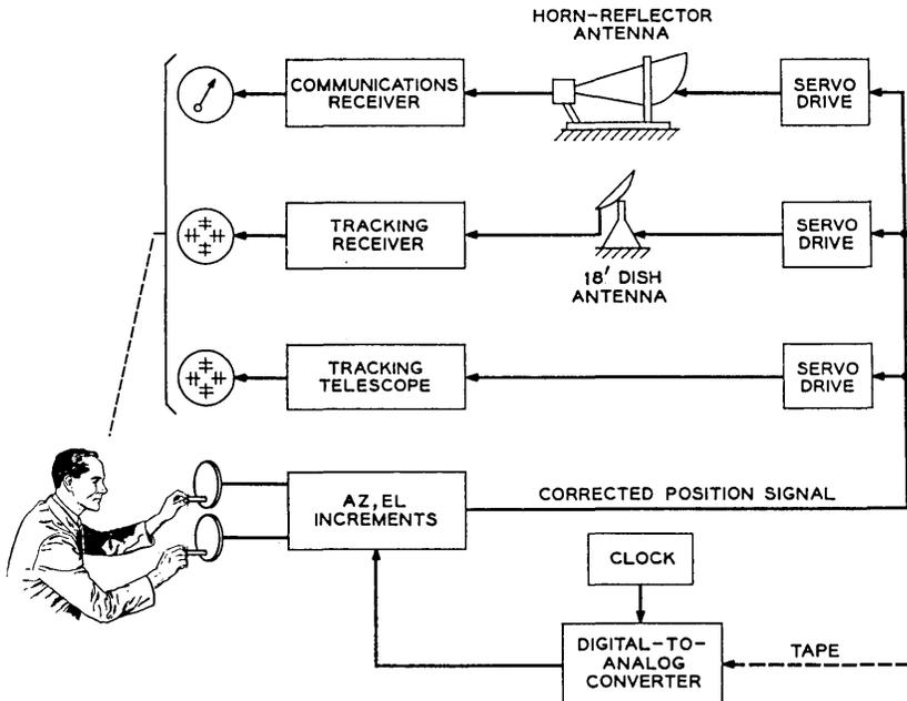
Fig. 4 — Block diagram of tracking modes at Holmdel.
