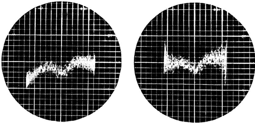
Fig. 29 — Envelope delay distortion of equalized loop through Telstar satellite; pass 925, Oct. 19, 1962. Left: FMPB receiver. Right: standard FM receiver. Scales same as Fig. 27.
