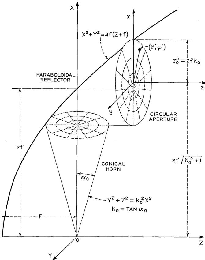
Fig. 1 — Geometry of the conical horn-reflector antenna.
