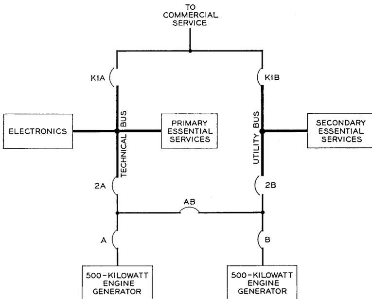
Fig. 9 — General plan for distribution of power.
