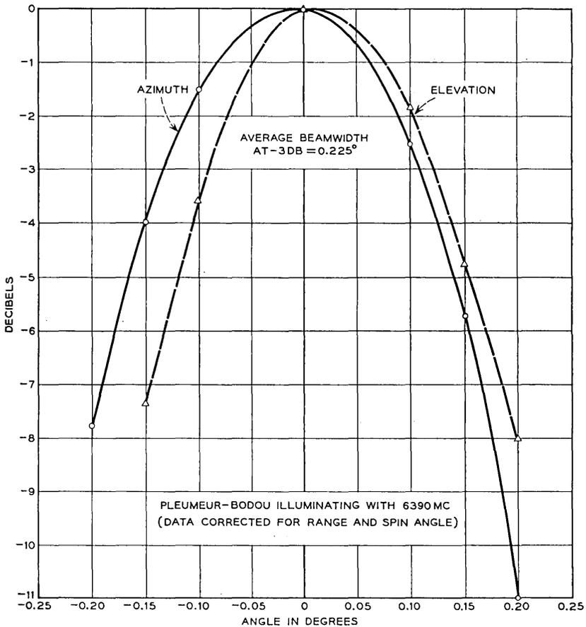
Fig. 12 — 4-kmc horn antenna pattern; pass 132, July 24, 1962.
