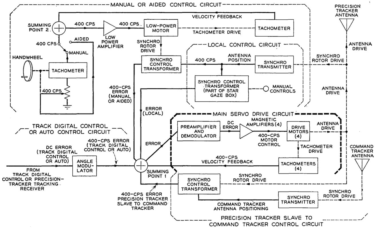
Fig. 15 — Antenna positioning circuits, azimuth or elevation.
