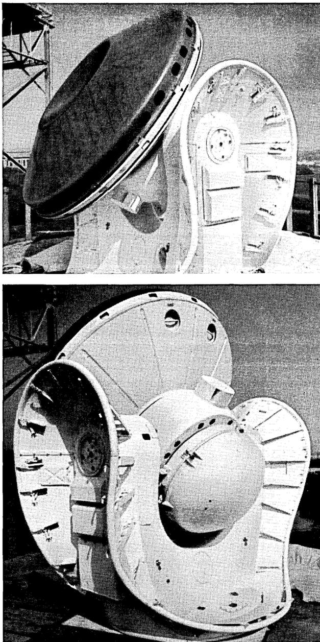
Fig. 3 — Precision tracker antenna, front and rear views.
