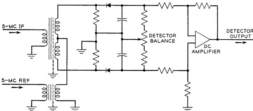
Fig. 11 — Phase detector.
