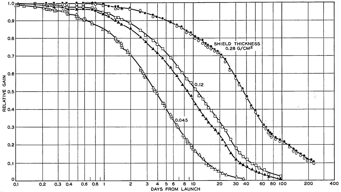
Fig. 30 — The relative gains of the radiation damage transistors as a function of time.
