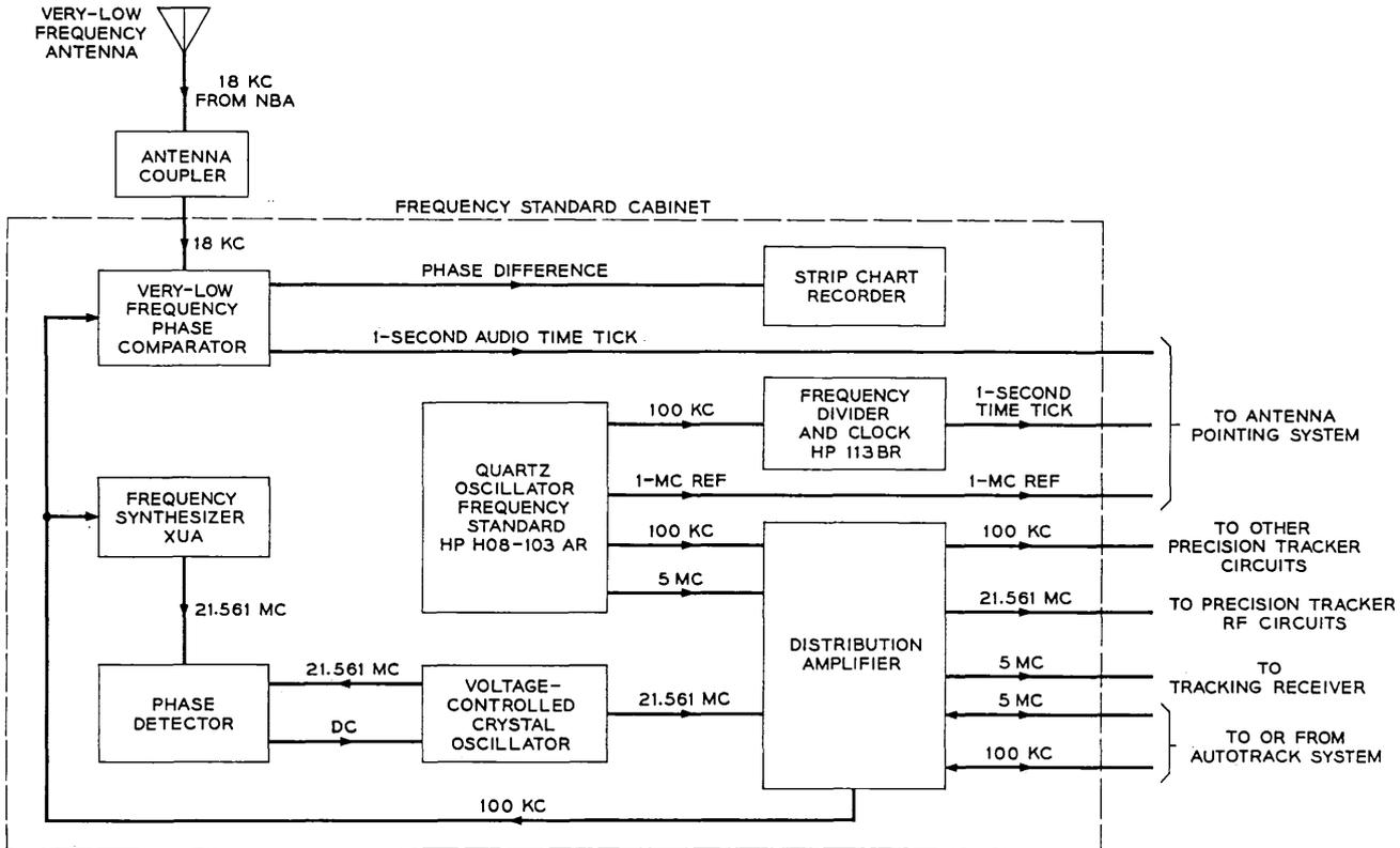
Fig. 18 — Frequency standard circuits, block diagram.
