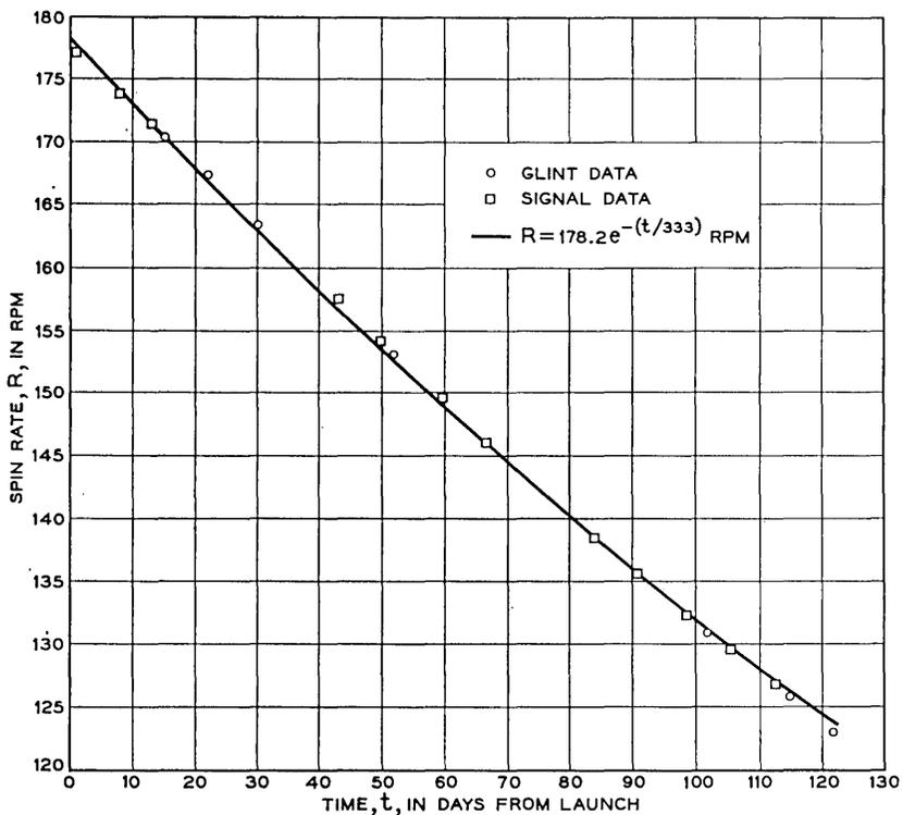
Fig. 8 — Change of satellite spin rate with time.
