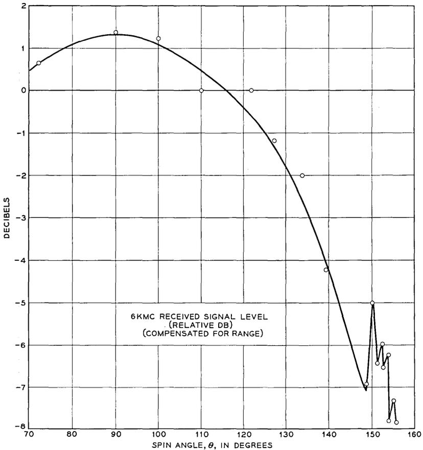
Fig. 11 — 6-kmc satellite antenna pattern; pass 125.
