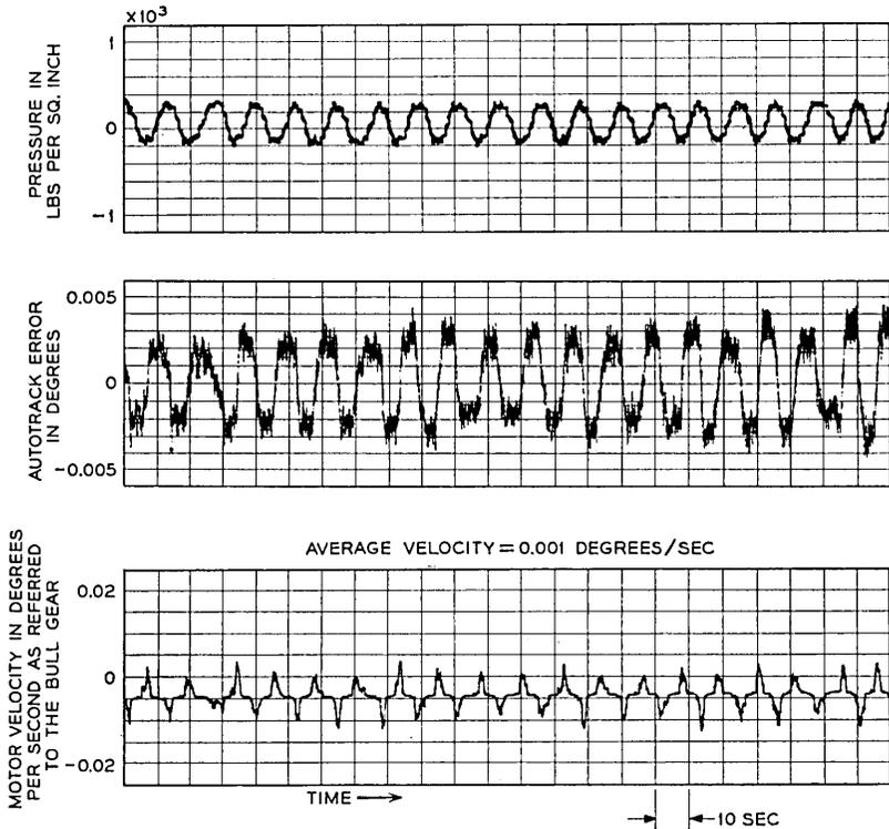
Fig. 26 — Small amplitude hunting in combined mode — azimuth.
