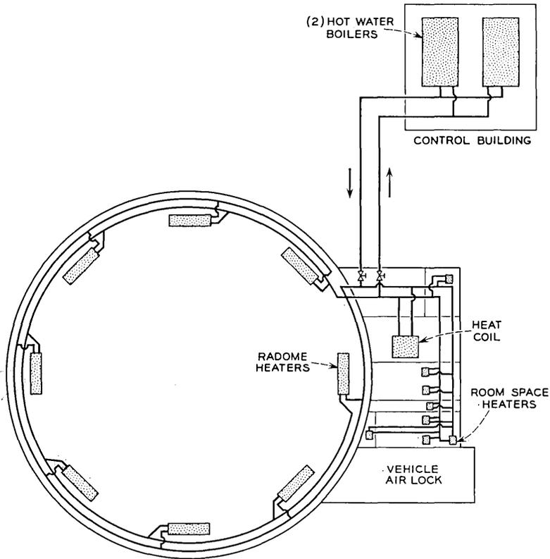
Fig. 10 — Schematic diagram of closed hot water system.
