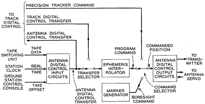
Fig. 4 — Antenna digital control block diagram.
