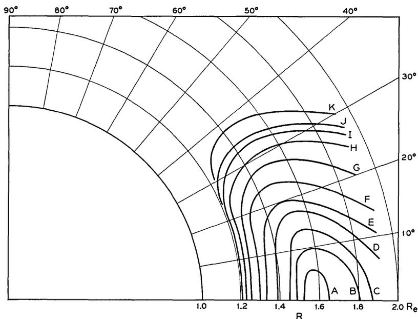
Fig. 17 — Contours of constant  $OCR$ , protons in the energy range 26 to 34 Mev, days 191 to 294, 1962, plotted in  $R$ - $\lambda$  coordinates. To convert  $OCR$  to omnidirectional flux ( $1/\text{cm}^2 \text{ sec}$ ), add 0.32 to  $\Phi$ . The range of  $\Phi$  associated with the contours is: A, 4.0-4.2; B, 3.8-4.0; C, 3.6-3.8; D, 3.4-3.6; E, 3.2-3.4; F, 3.0-3.2; G, 2.8-3.0; H, 2.6-2.8; I, 2.4-2.6; J, 2.2-2.4; K, 2.0-2.2.
