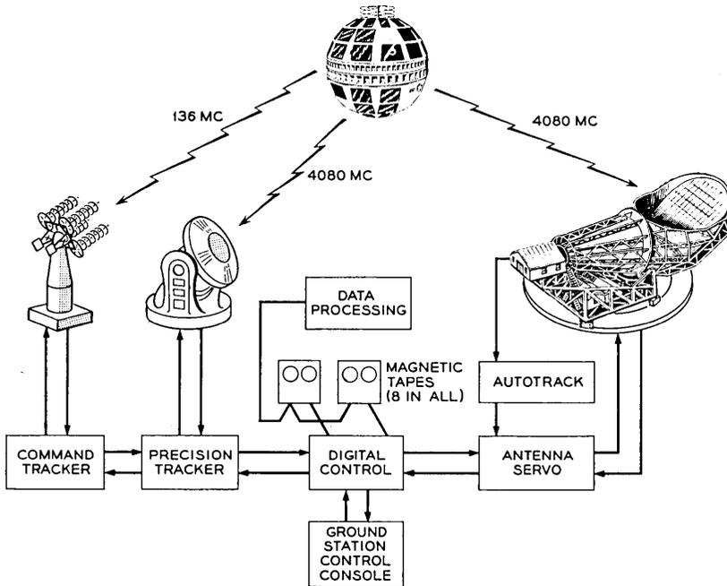
Fig. 1 — Block diagram of pointing system.
