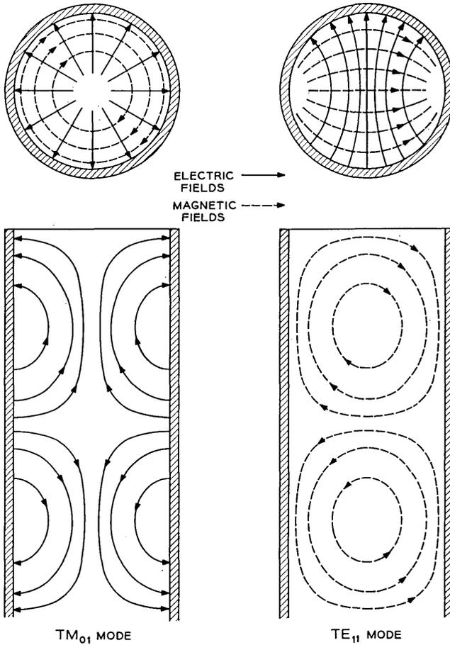
Fig. 2 — Circular waveguide mode field configurations.
