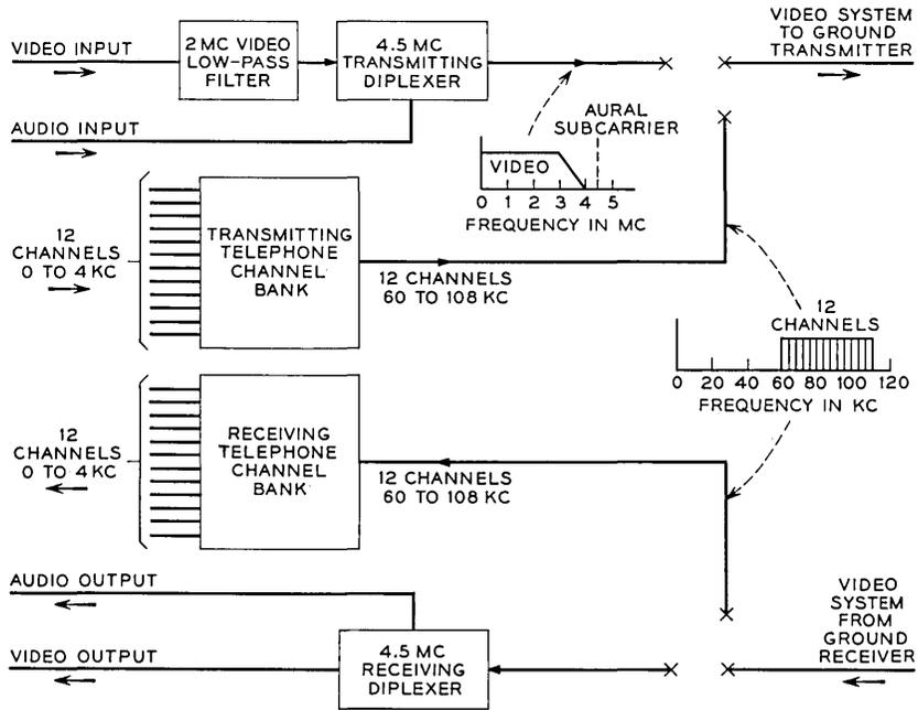
Fig. 2 — Arrangements for television and two-way message transmission.
