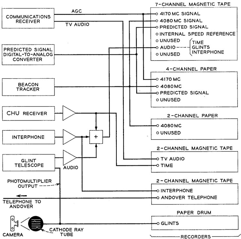
Fig. 5 — Block diagram of data recording facilities.
