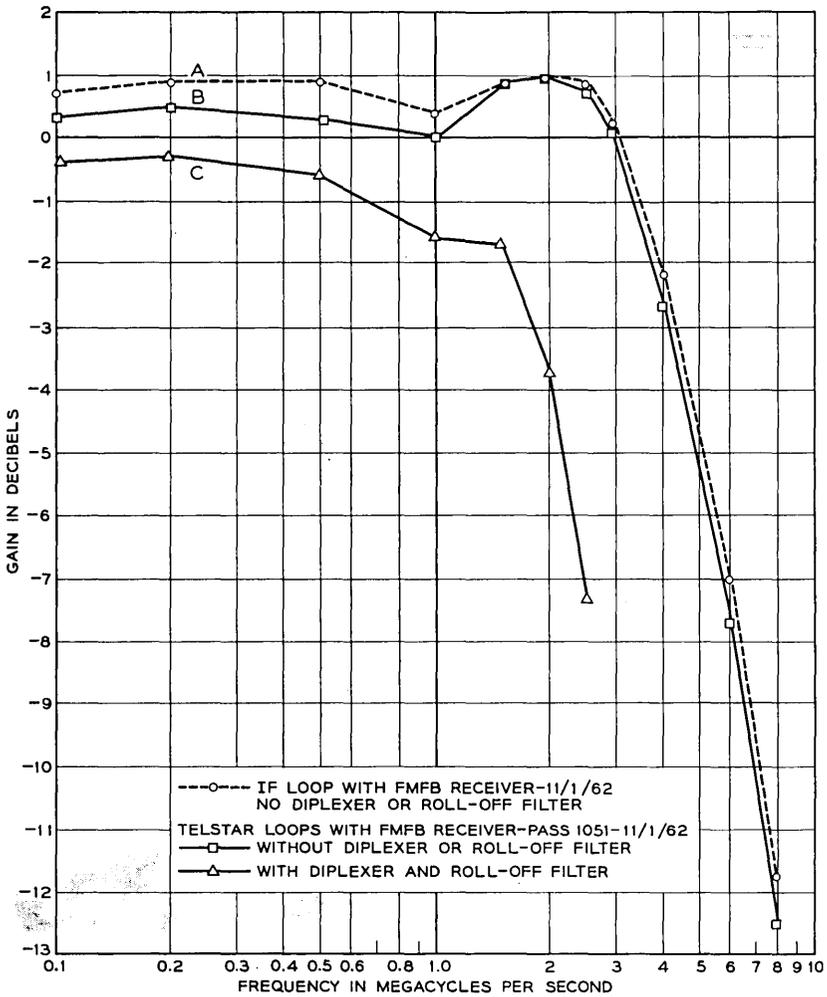
Fig. 17 — Baseband frequency response (FMFB receiver).
