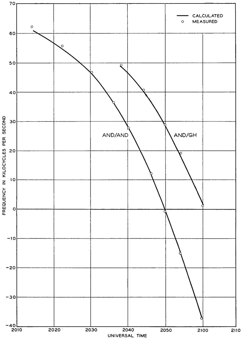
Fig. 52 — Doppler shift of communications carrier; pass 443, Aug. 27, 1962.
