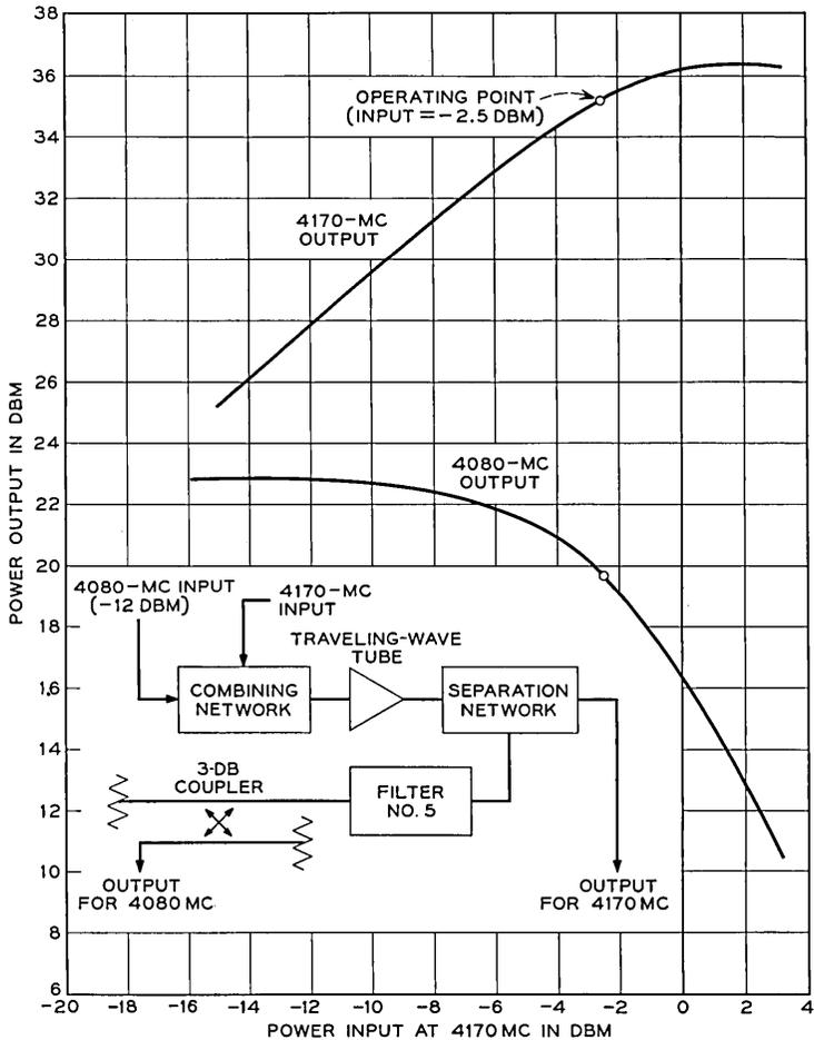
Fig. 18 — Operating characteristics of the traveling-wave amplifier.
