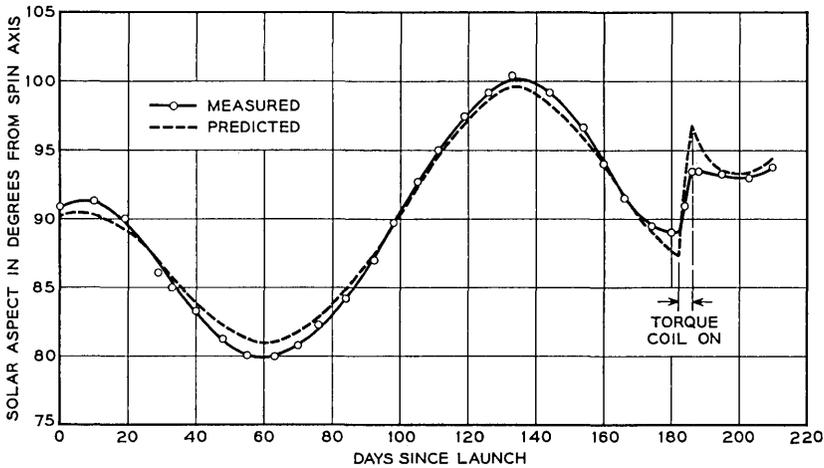
Fig. 27 — The time variation of  $\alpha$ , the angle between the spin axis of the satellite and the satellite-sun line, from launch until February 5, 1963. The angle is measured from the telemetry antenna end of the satellite.
