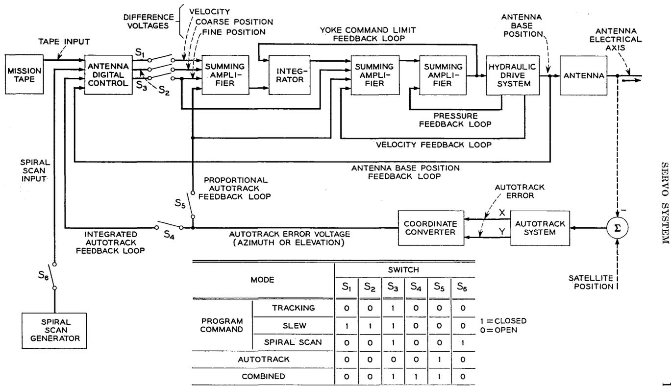
Fig. 11 — Over-all functional diagram of the servo system.
