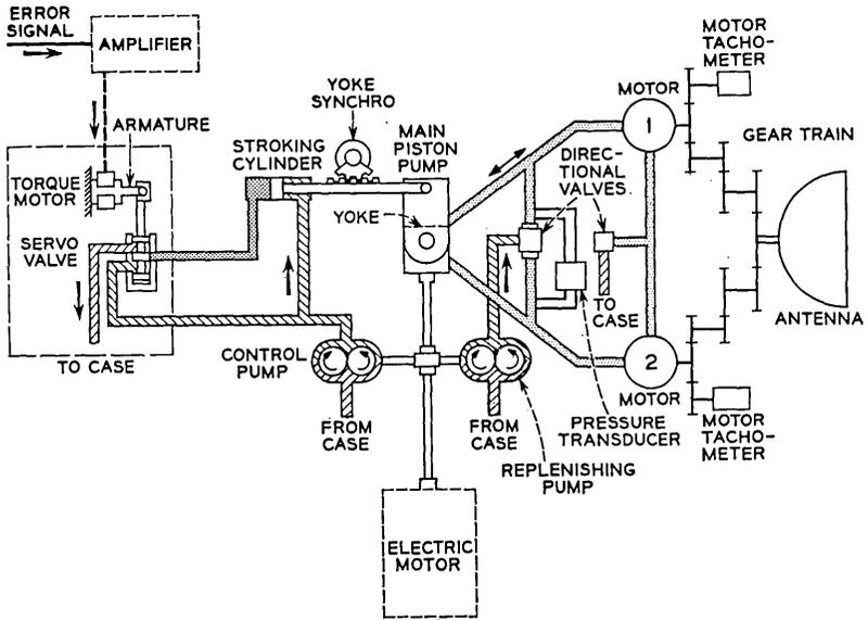
Fig. 23 — Simplified schematic of basic hydraulic drive circuit.
