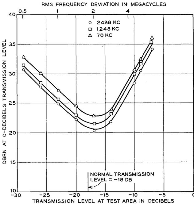
Fig. 34 — Baseband loop noise loading measurements, Sept. 27, 1962.
