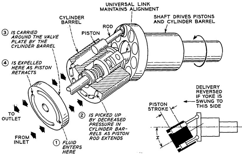
Fig. 24 — Mechanical schematic of piston pump.
