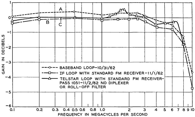
Fig. 16 — Baseband frequency response (standard FM receiver).
