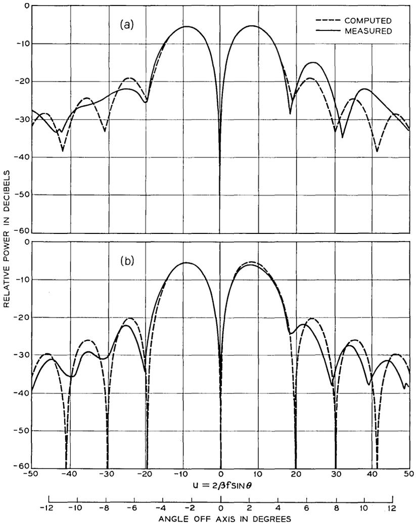
Fig. 8 — Radiation patterns for  $TM_{01}$  mode (model two): (a) in the longitudinal plane for the longitudinal component of the aperture field; (b) in the transverse plane for the transverse component of the aperture field.
