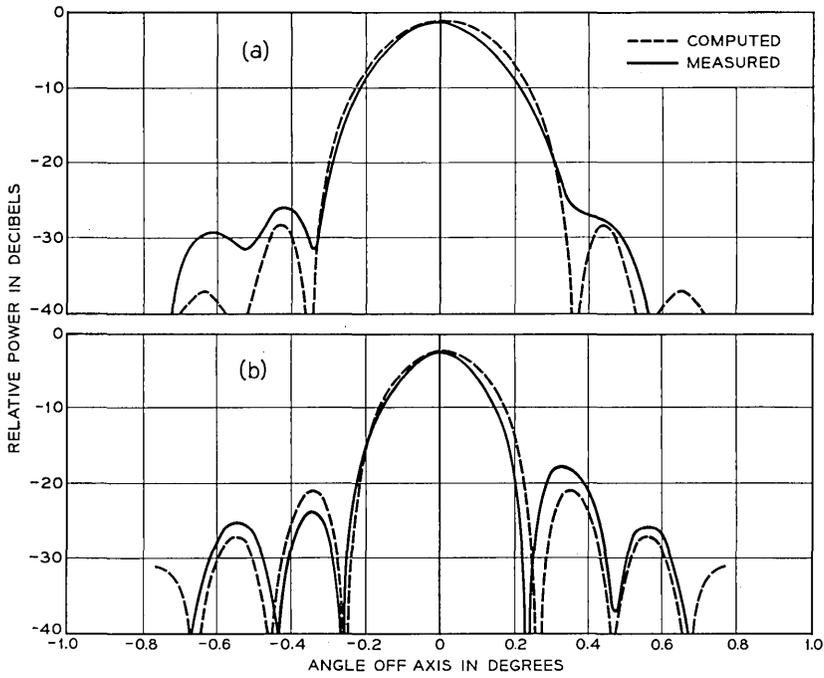
Fig. 12 — Principal radiation patterns of the full size antenna for  $TE_{11}$  mode in the transverse plane: (a) longitudinal polarization  $(TE_{11})_x$ ; (b) transverse polarization  $(TE_{11})_y$ . (The dashed curves are computed far-field patterns.)
