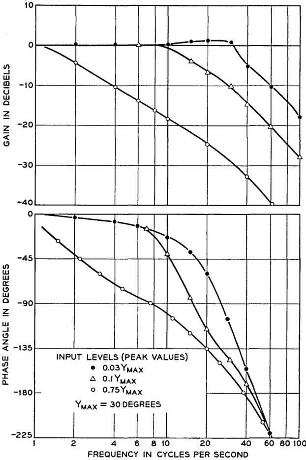
Fig. 6 — Closed-loop frequency response of yoke position — azimuth.
