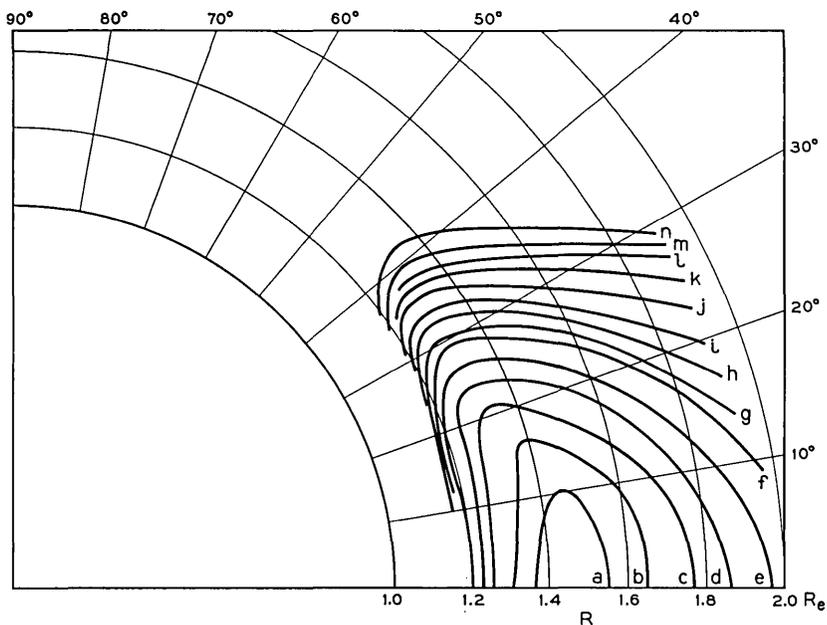
Fig. 18 — Contours of constant  $OCR$ , protons with energies  $>50$  Mev, days 191 to 294, 1962, plotted in  $R$ - $\lambda$  coordinates. To convert  $OCR$  to omnidirectional flux ( $1/\text{cm}^2 \text{ sec}$ ), add  $0.42$  to  $\Phi$ . The range of  $\Phi$  associated with the contours is: a, 3.2-3.4; b, 3.0-3.2; c, 2.8-3.0; d, 2.6-2.8; e, 2.4-2.6; f, 2.2-2.4; g, 2.0-2.2; h, 1.8-2.0; i, 1.6-1.8; j, 1.4-1.6; k, 1.2-1.4; l, 1.0-1.2; m, 0.8-1.0; n, 0.4-0.6.
