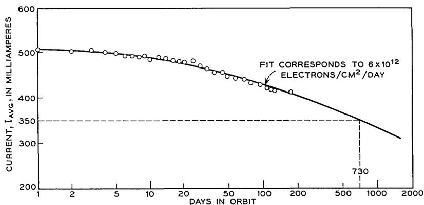
Fig. 28 — The average over the angle  $\phi$  of the output current of the solar power plant from launch until February, 1963. Corrections have been made for mean solar distance. No detailed temperature corrections or corrections for solar aspect angle have been made in these data. Such corrections are expected to reduce the scatter of the points.
