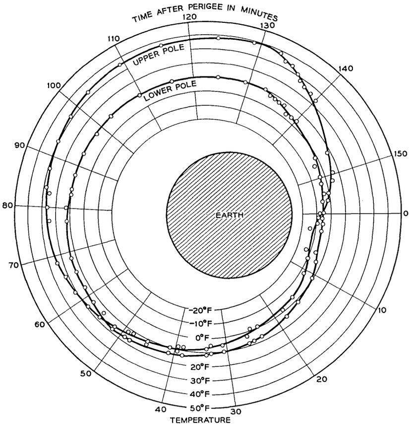
Fig. 11 — Skin temperature versus orbital position.
