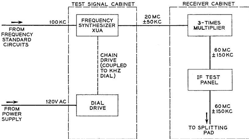
Fig. 20 — 60-mc IF test signal circuits, block diagram.
