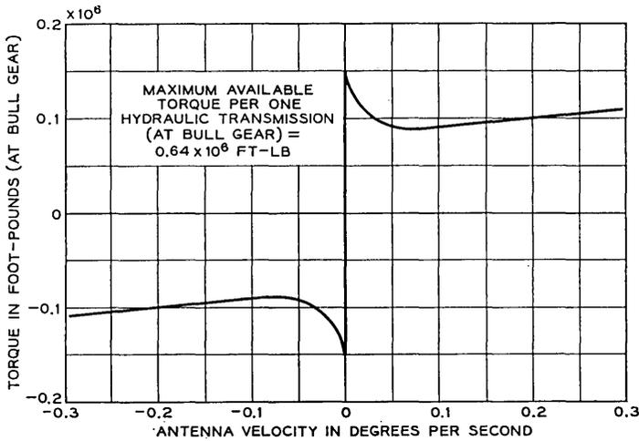
Fig. 3 — Average friction torque at constant velocity — azimuth.
