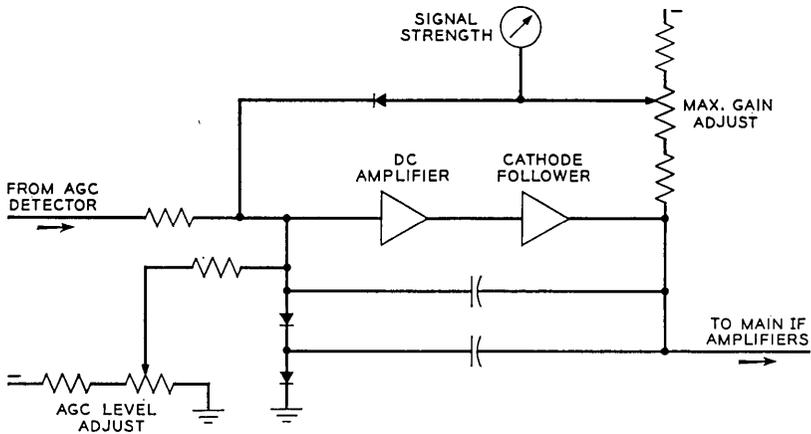
Fig. 13 — AGC amplifier and loop filter.
