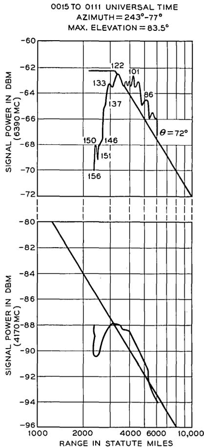
Fig. 9 — Received carrier power vs range; pass 125.
