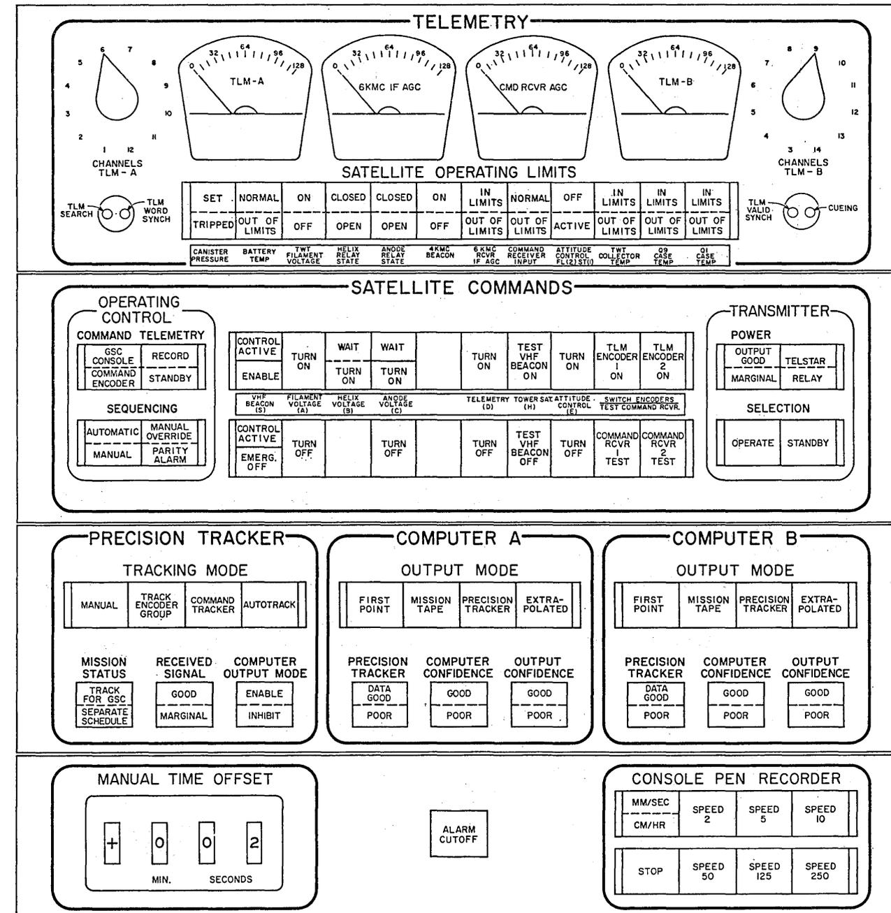
Fig. 8 (This page and overleaf)—Front panel layout of ground station control console.
