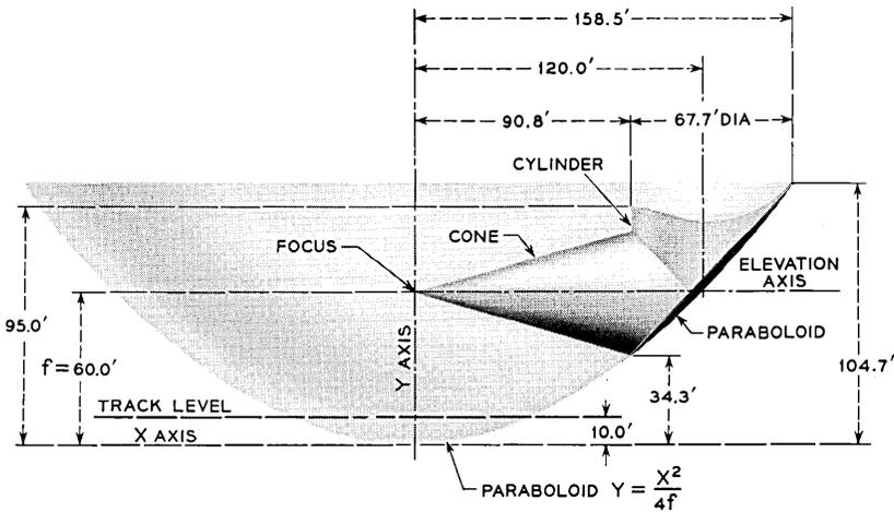
Fig. 7 — Relationship between horn, shield, and reflector surfaces.
