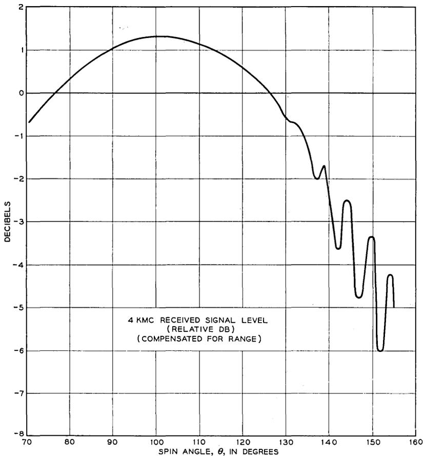
Fig. 10 — 4-kmc satellite antenna pattern; pass 125.
