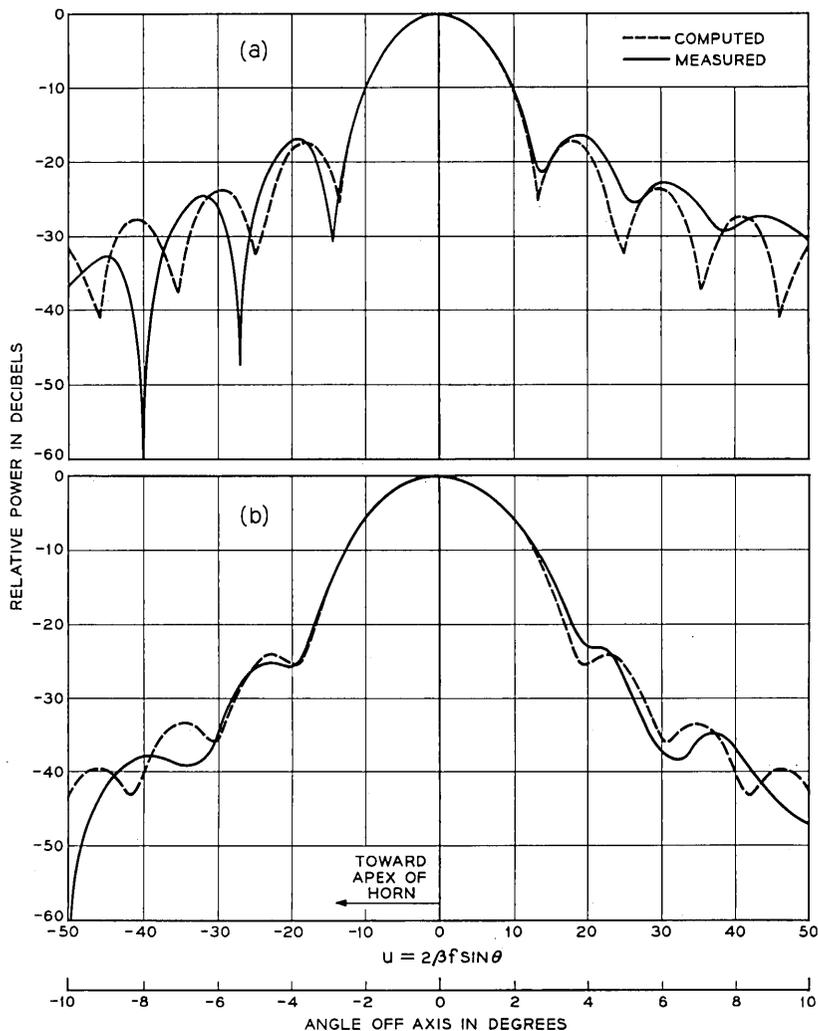
Fig. 5 — Radiation patterns for  $TE_{11}$  mode in the longitudinal plane (model one): (a) longitudinal polarization; (b) transverse polarization.
