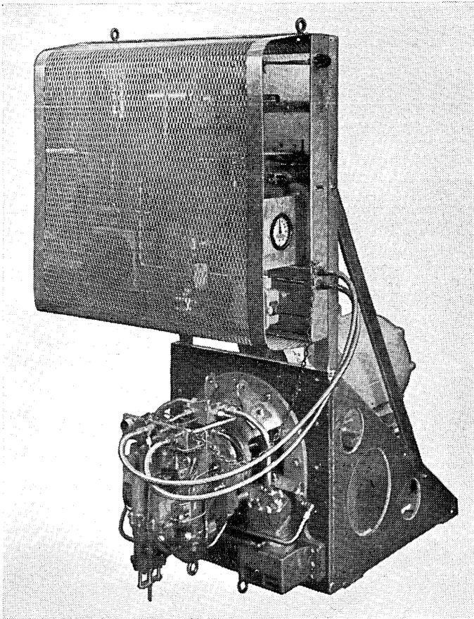
Fig. 22 — Vickers 25-horsepower azimuth drive unit.
