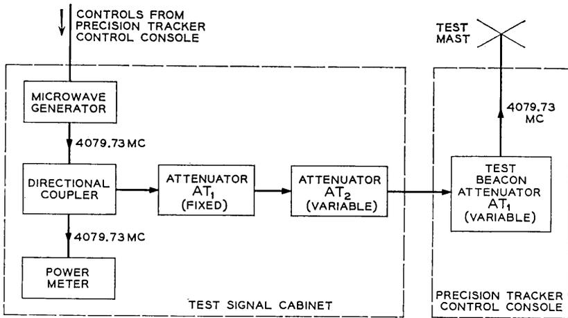
Fig. 19 — 4-kmc test signal circuits, block diagram.
