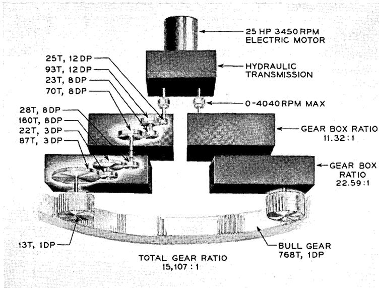
Fig. 16 — Schematic of azimuth gear train.
