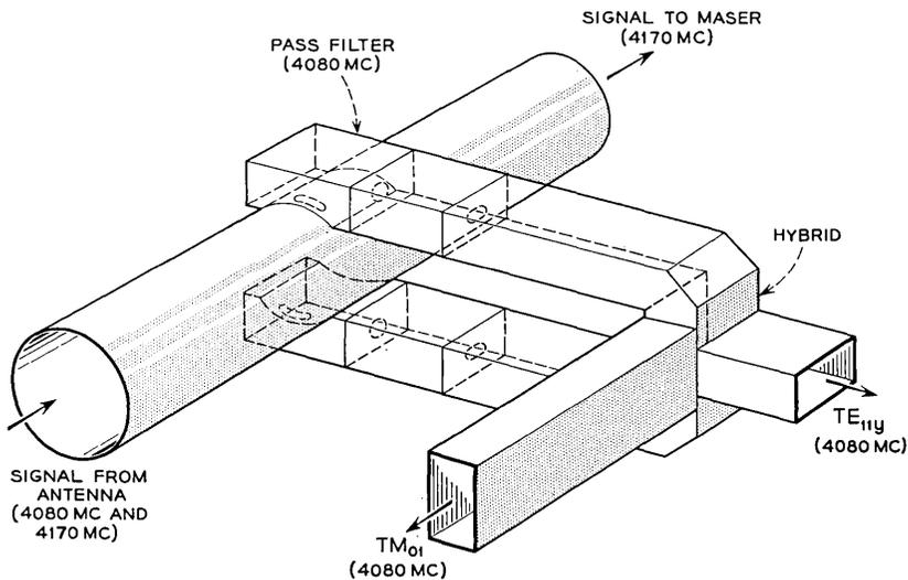
Fig. 15 — Conceptual version of the sampling coupler.
