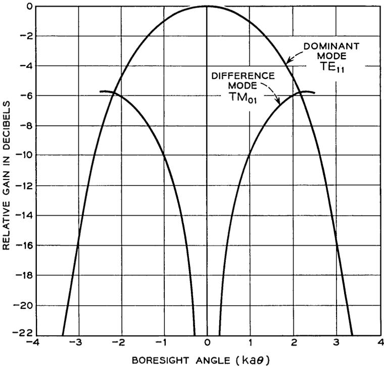
Fig. 3 — Radiation patterns for an open-end circular waveguide.
