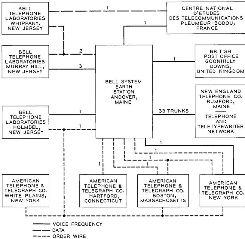
Fig. 12 — Voice-frequency, data and order wire connections with Andover.
