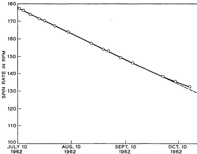
Fig. 4 — Telstar satellite — spin rate versus time.
