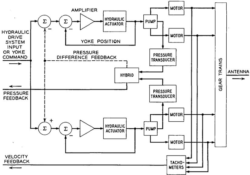
Fig. 5 — Functional diagram of hydraulic drive system.
