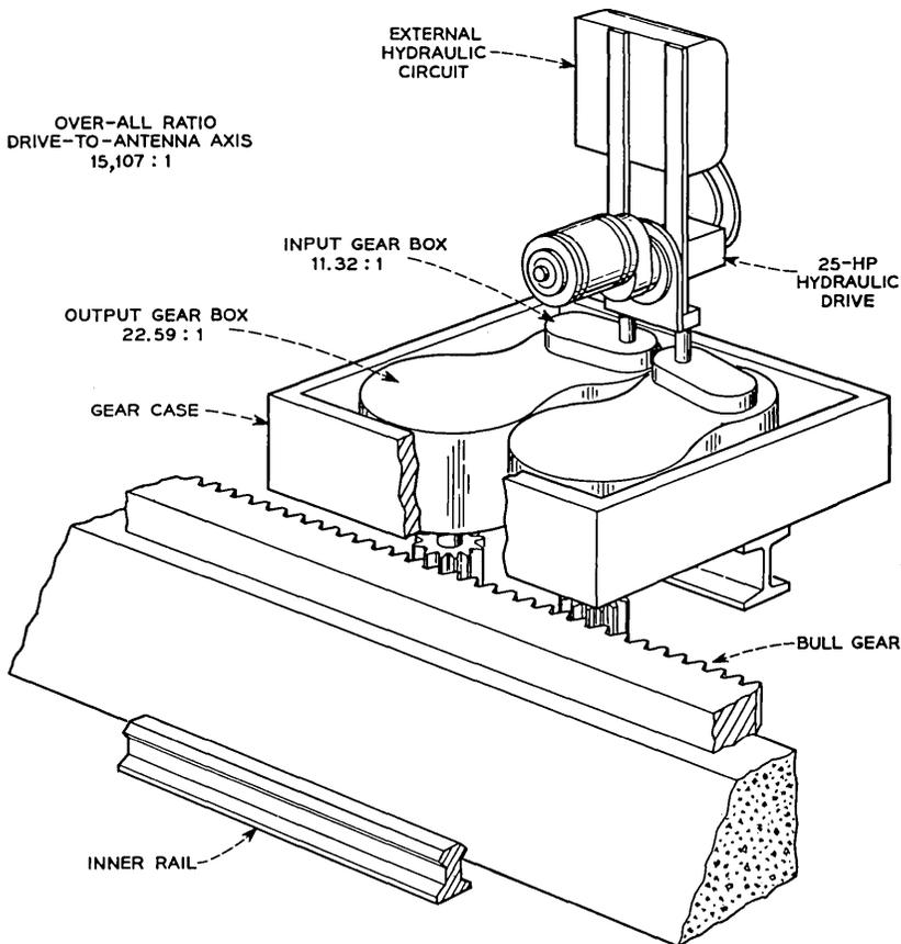
Fig. 15 — Schematic showing arrangement of one azimuth drive.
