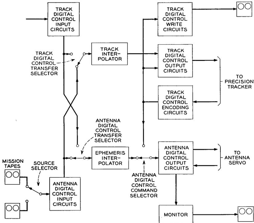
Fig. 8 — Normal mode operation block diagram.
