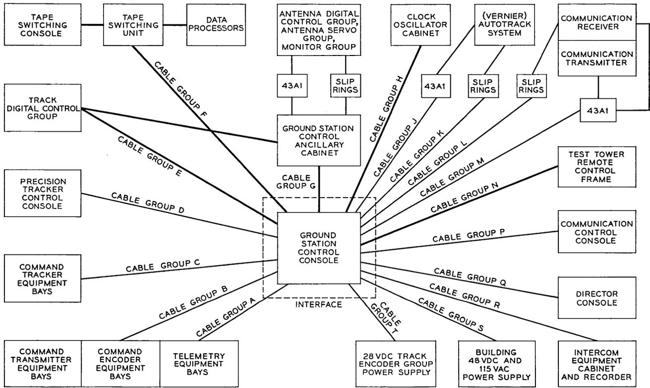
Fig. 7 — Connections to ground station control console (GSCC).
