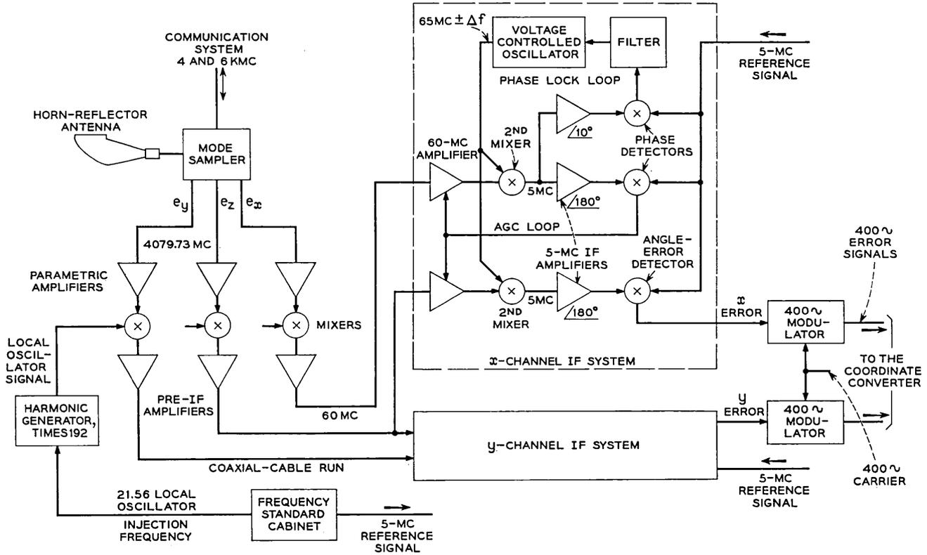
Fig. 12 — Standard four-channel autotrack system arrangement.
