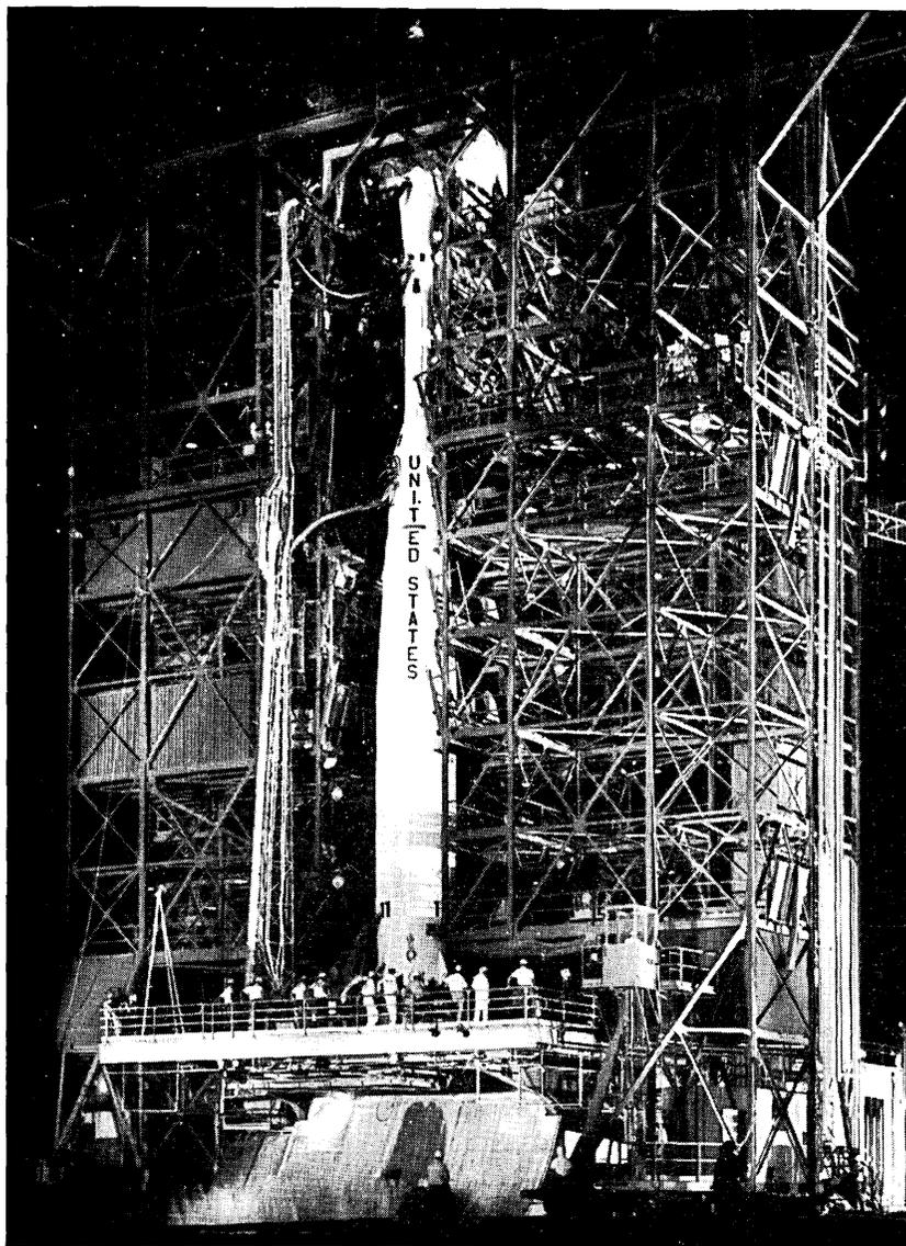
Fig. 12 — Delta vehicle and Telstar spacecraft in gantry.
