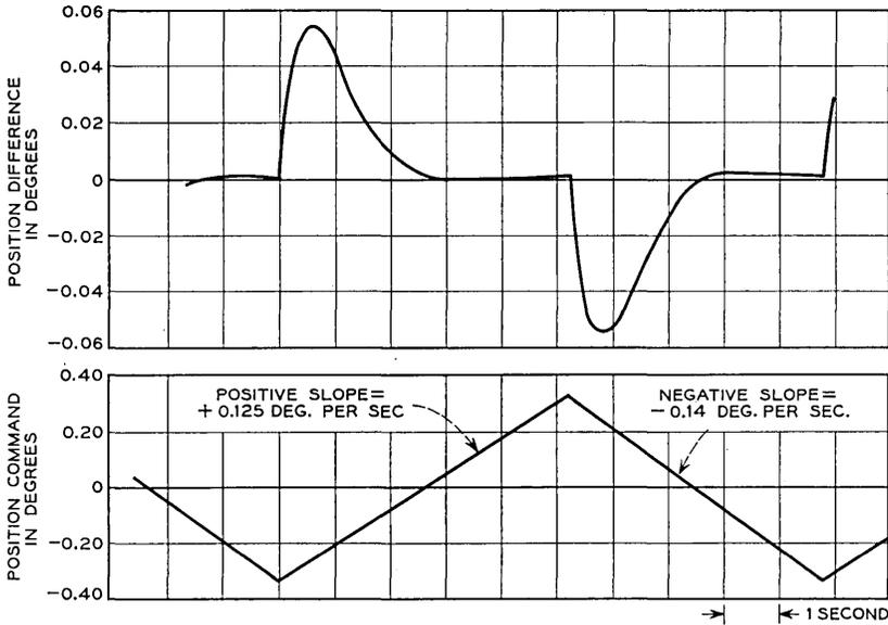
Fig. 15 — Ramp response of program command mode — azimuth.
