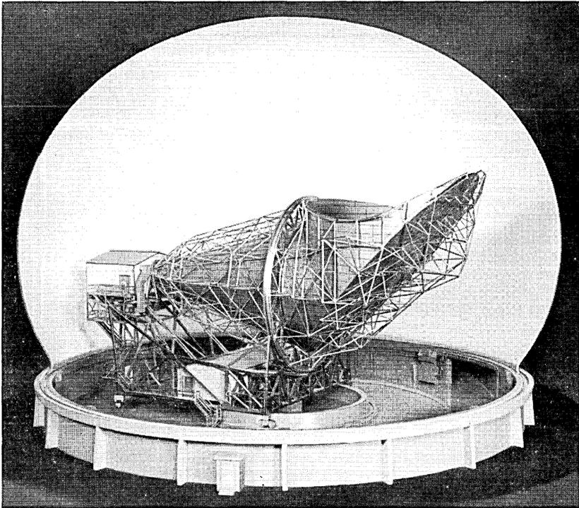
Fig. 5 — Model of Telstar horn-reflector antenna.
