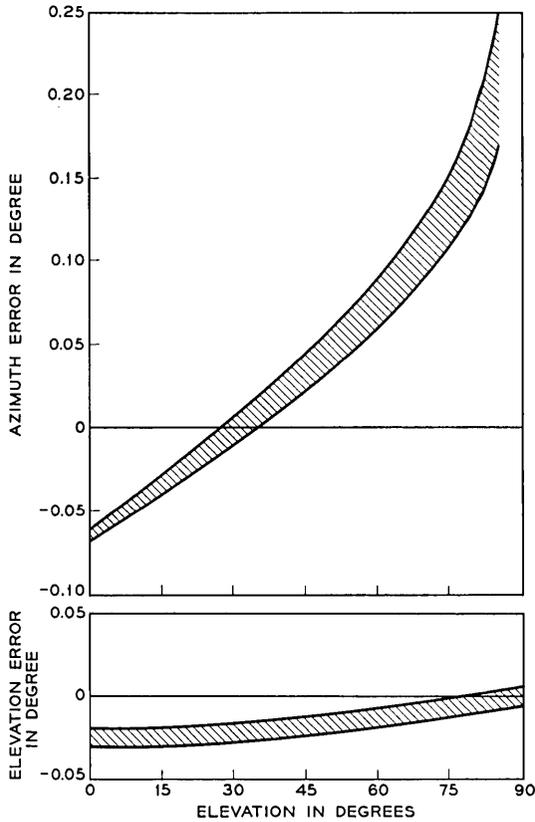
Fig. 4 — Calculated structural variable pointing errors.
