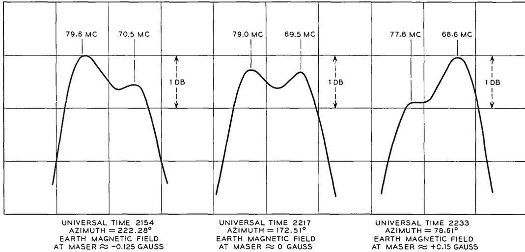
Fig. 19 — IF-RF transmission characteristics; pass 188, July 30, 1962.
