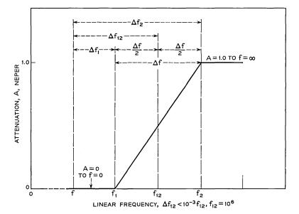
Fig. 2 — Unit attenuation line segment.
