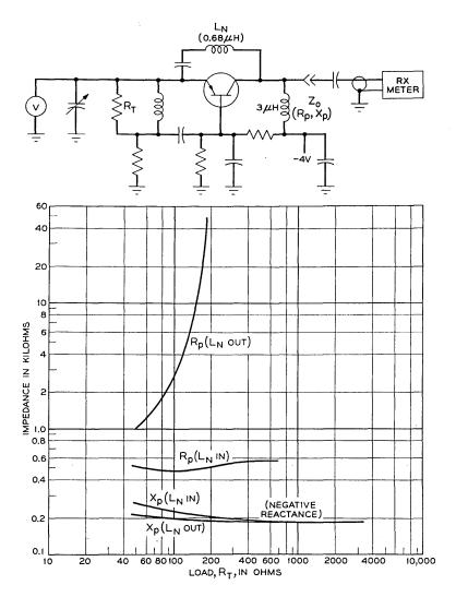
Fig. 10 — RF amplifier, neutralization effect on output impedance.
