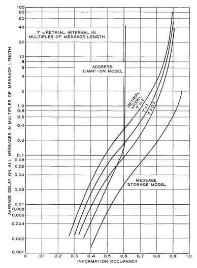
Fig. 5 — Average delay on all messages vs information occupancy; 10 lines per group, 3 addresses per message.
