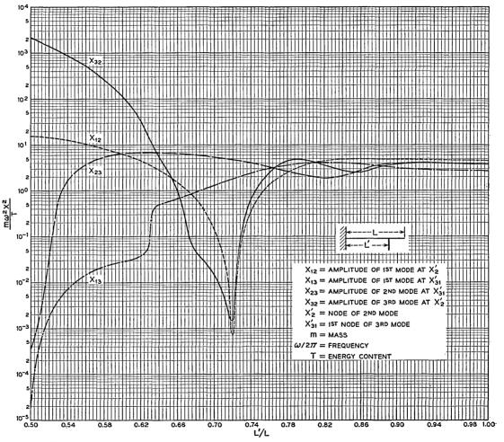
Fig. 5 — Propped cantilever: energy content in terms of amplitudes at specific locations.
