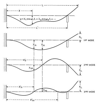
Fig. 1 — Flexural vibrations of a propped cantilever.
