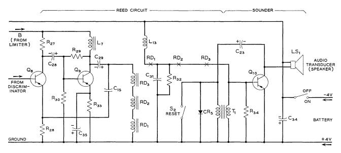
Fig. 4 — Reed circuit and sound oscillator.
