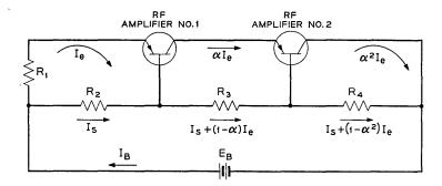
Fig. 12 - 55A receiver — RF amplifiers transistor bias circuit.
