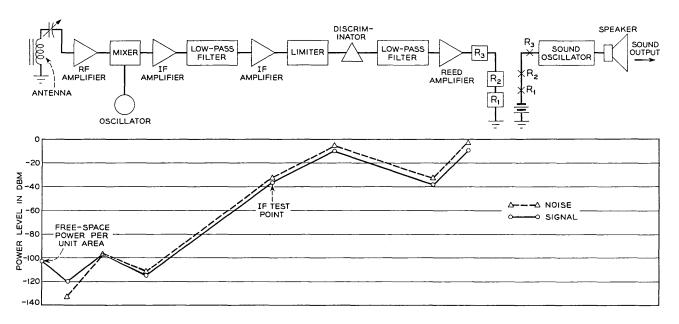
Fig. 7 — Receiver power level diagram.
