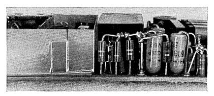
Fig. 14 — Component wiring for space conservation.
