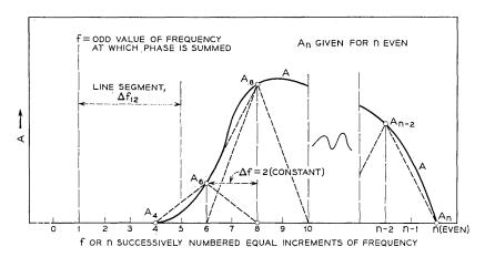
Fig. 3 — Phase summation using wedge element.
