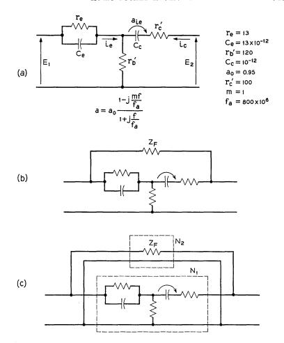
Fig. 8 — (a) Assumed equivalent circuit for RF amplifier transistor; (b) assumed equivalent circuit with neutralizing impedance added; (e) component networks used in analysis of neutralization.
