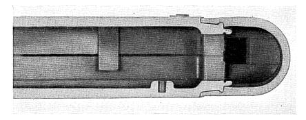
Fig. 18 — Snap fastener of case.
