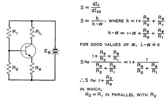
Fig. 11 — 55A receiver — bias stabilization, single stage.
