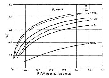
Fig. 9 — Upper and lower bounds (solid and dashed curves, respectively) on fractional loss in rate,  $r/\bar{r}$ , due to finite encoding. Loss plotted vs R/W for fixed n and  $P_{\epsilon}$ .
