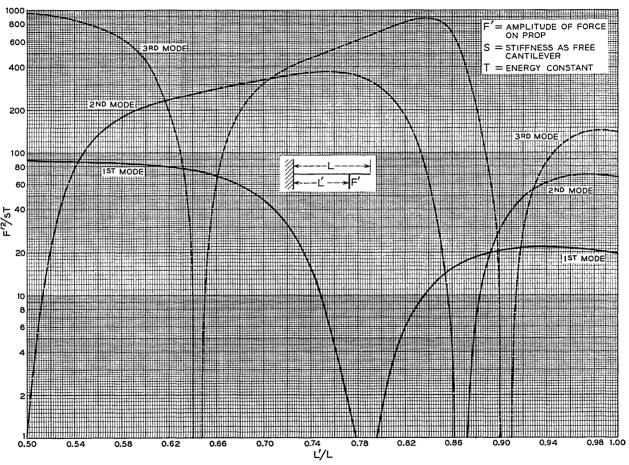
Fig. 6 — Propped cantilever: force on prop.
