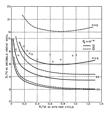
Fig. 2 — Upper and lower bounds (dashed and solid curves, respectively) on S/N needed to achieve word-error probability of  $10^{-4}$  for various values of n=2WT. Circle, triangles, and crosses give performance of some known codes.
