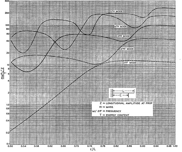
Fig. 7 — Propped cantilever: slide amplitude at prop.
