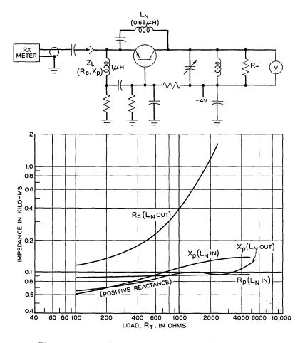
Fig. 9 — RF amplifier, neutralization effect on input impedance.
