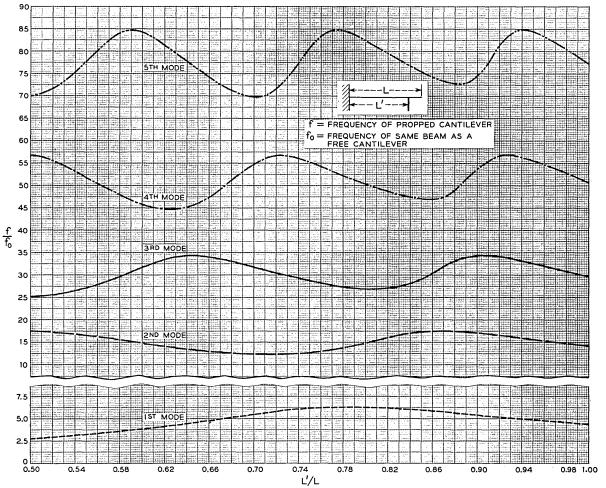
Fig. 2 — Frequency of a propped cantilever.
