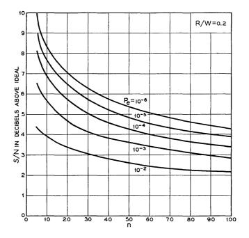
Fig. 7 — Cross-plot of Figs. 4, 5 and 6 showing (for R/W=0.2) decrease in S/N needed to achieve a given word-error probability as n is increased.
