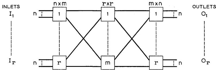
Fig. 1 — Three-stage Clos network  $N(m, n, r)$ .
