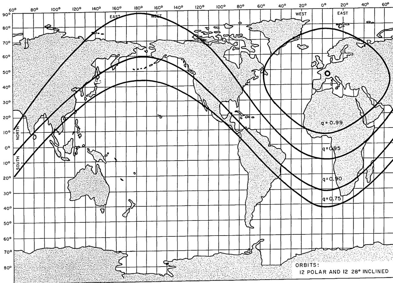
Fig. 17 — Qualities of service from a West-European point for a system of 24 satellites in 6000-mile orbits (12 polar and 12 28°-inclined).
