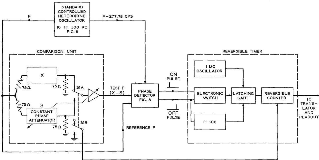
Fig. 4 — Block diagram of phase measurement circuits.
