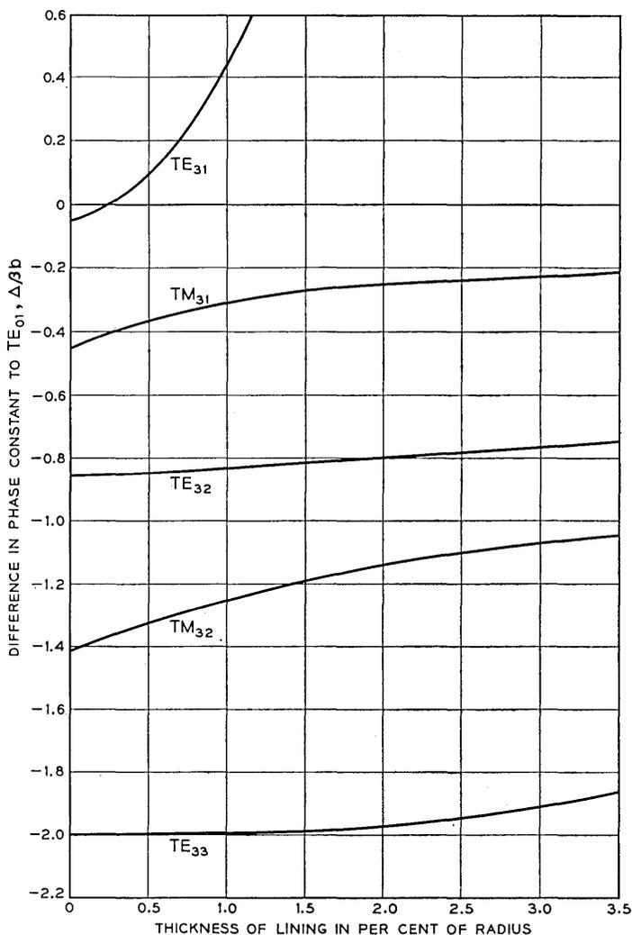
Fig. 4 — Phase constants of TE<sub>3n</sub> and TM<sub>3n</sub> modes in lined waveguide.  $b/\lambda = 4.70$ ,  $\epsilon_r = 2.5$ .
