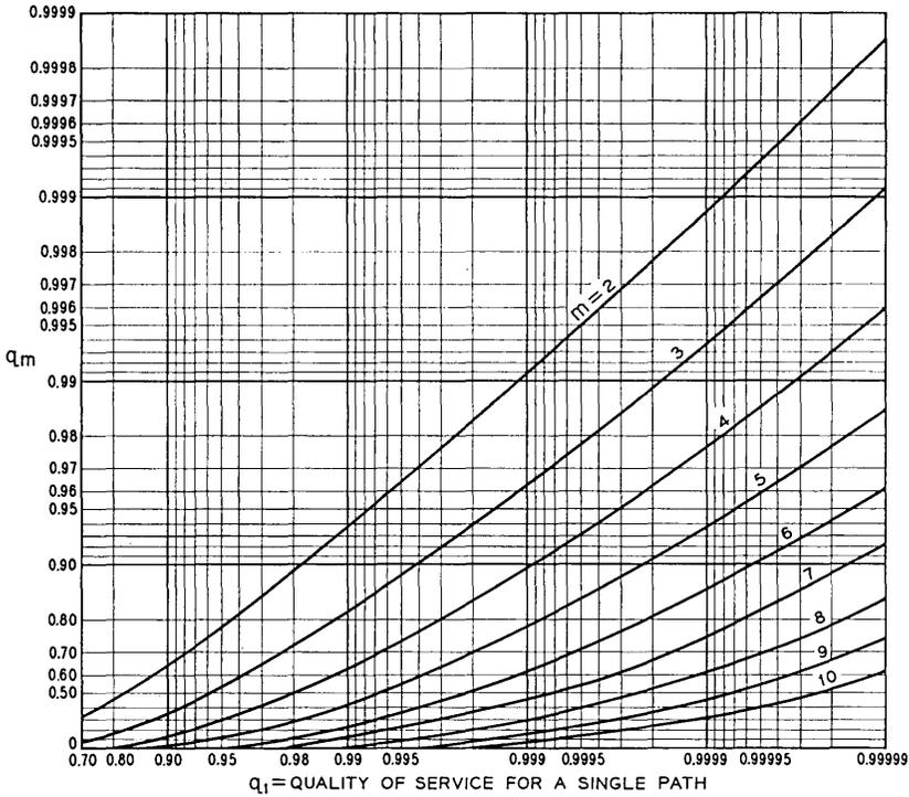
Fig. 9 — Fraction of time  $q_m$  that  $m$  or more satellites are visible. In a system with multiple paths between two ground stations  $q_m$  is the quality of service on a path with priority  $m$ . The number of satellites needed to furnish  $q_m$  is found by entering Fig. 8 with  $q_1$  and  $p$ .
