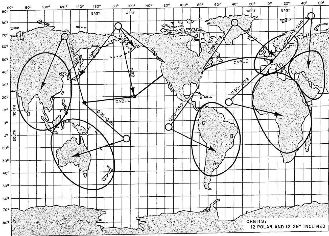
Fig. 18 — A world-wide network which uses satellites and submarine cables. The ranges of qualities of service shown for each region would be provided by 24 satellites in 6000-mile orbits (12 polar and 12 28°-inclined).
