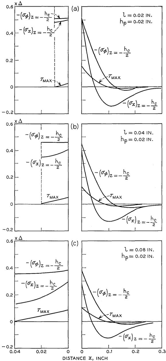
Fig. 9 — Stress distributions showing the effect of varying the length,  $l$ , of the intermediate cylinder in an axially unbalanced seal. Note the difference in scale for long (right side) and short (left side) cylinders.
