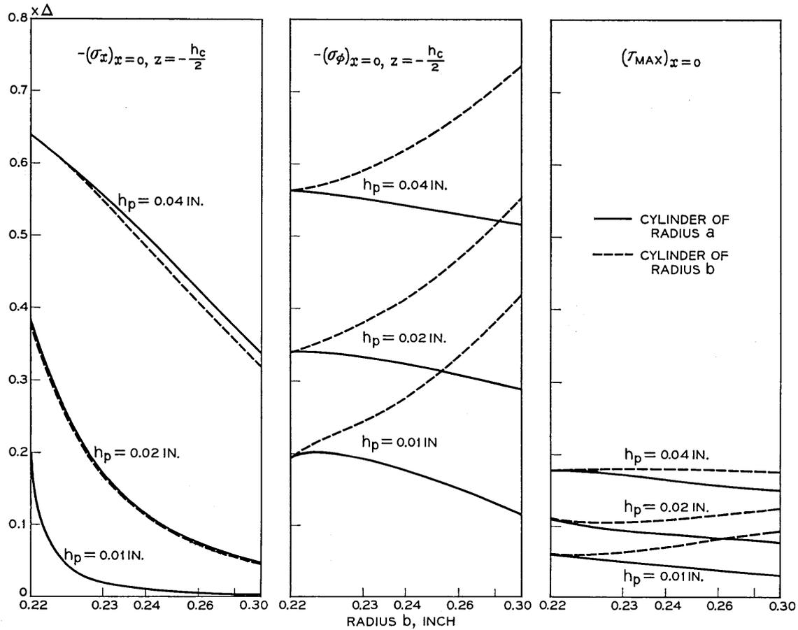
Fig. 6 — Stresses at the junctions of radially unbalanced seals. The values for both cylinders are shown as the radius,  $b$ , of the balancing seal is varied.
