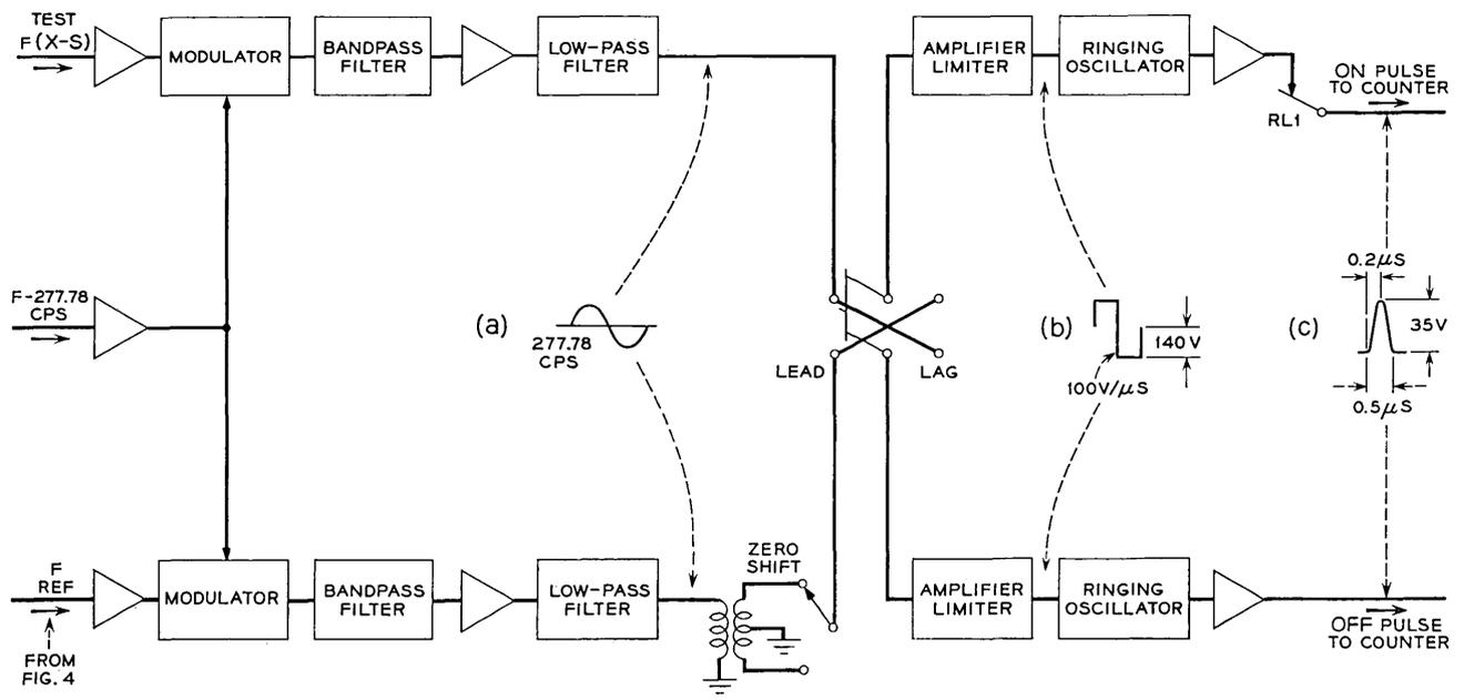
Fig. 7 — Block diagram of phase detector.
