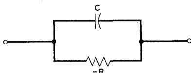
Fig. 1 — “C, -R” model of the tunnel diode.
