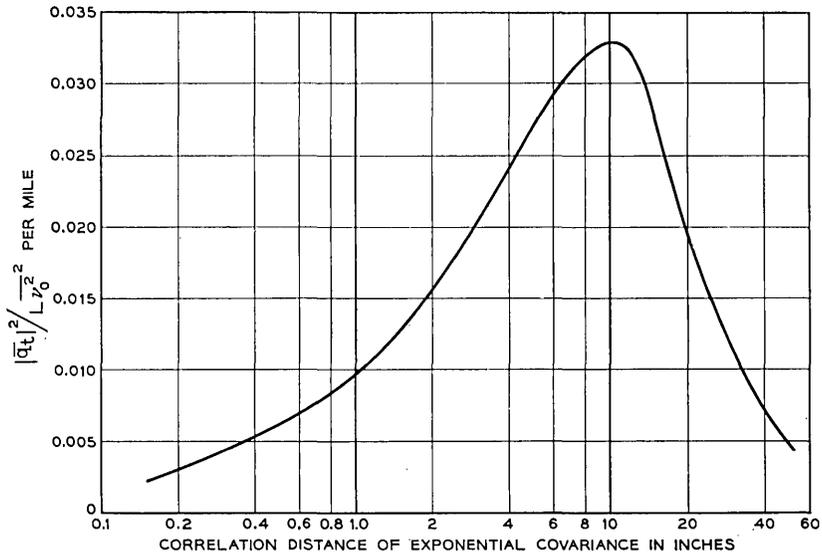
Fig. 13 —  $TE_{01}$  — pulse distortion in lined waveguide with random imperfections of the lining. Mode conversion causes a reconversion tail of rms amplitude  $\sqrt{|q_t|^2}$  to follow the pulse.  $b/\lambda = 4.70$ ,  $\epsilon_r = 2.5$ ,  $\delta = 1$  per cent.
