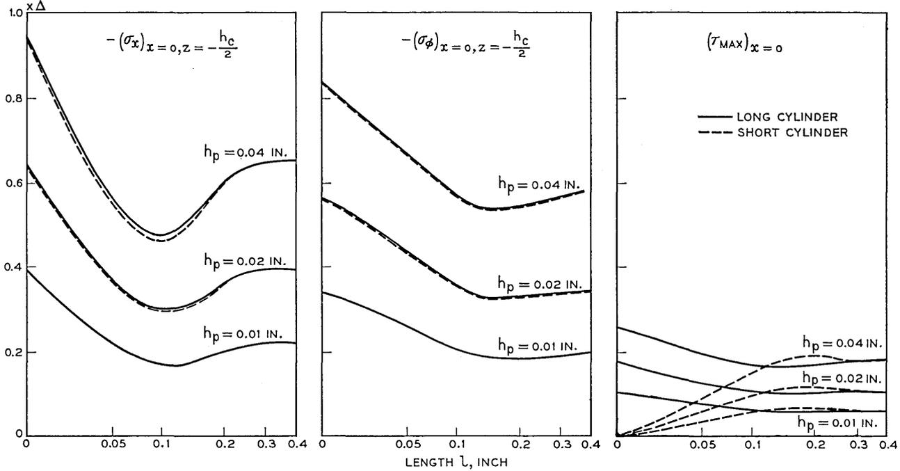
Fig. 8 — Stresses at the junctions of axially unbalanced seals. The values for both cylinders are shown as the length,  $l$ , of the intermediate cylinder is varied.
