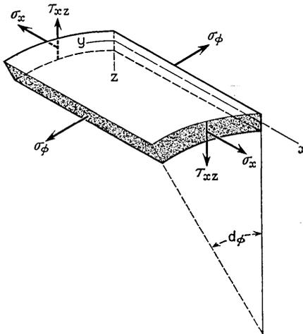
Fig. 4 — Cylindrical element showing stress directions.
