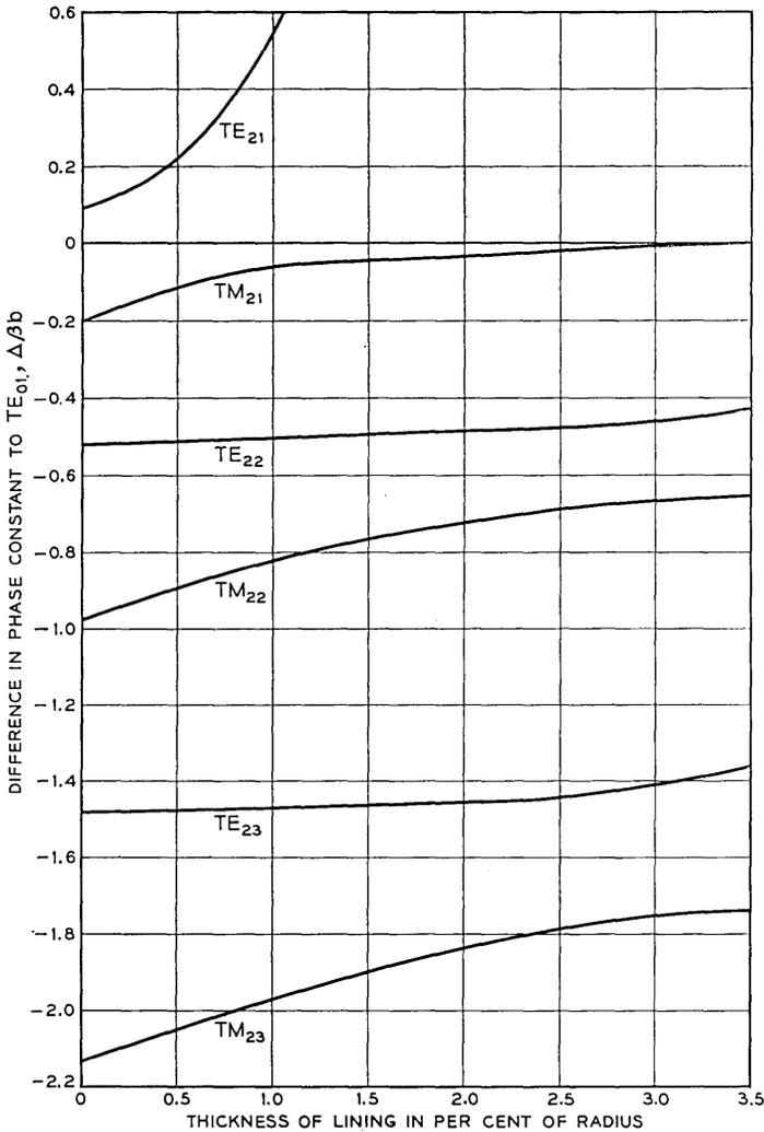
Fig. 3 — Phase constants of  $TE_{2n}$  and  $TM_{2n}$  modes in lined waveguide.  $b/\lambda = 4.70$ ,  $\epsilon_r = 2.5$ .
