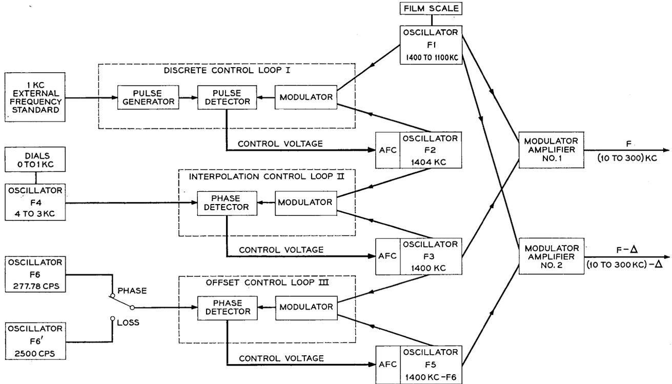
Fig. 6 — Block diagram of standard controlled heterodyne oscillator (SCHO).
