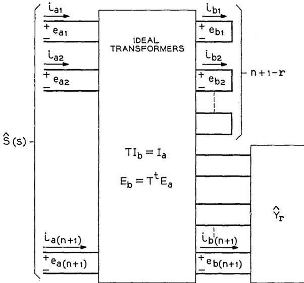
Fig. 4 — Realization of  $\hat{S}(s)$  when the normal rank of  $[1_{n+1} + \hat{S}(s)]$  is  $r$ .
