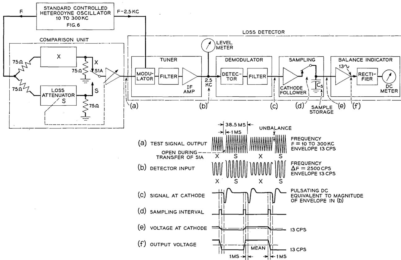
Fig. 3 — Block diagram of loss measurement circuits.
