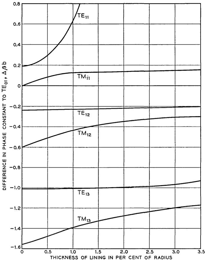
Fig. 2 — Phase constants of TE<sub>1n</sub> and TM<sub>1n</sub> modes in lined waveguide.  $b/\lambda = 4.70$ ,  $\epsilon_r = 2.5$ .
