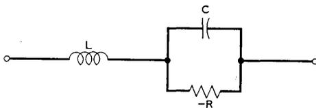
Fig. 2 — “LC, -R” model of the tunnel diode.
