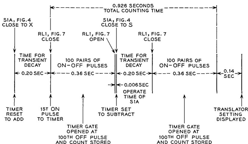
Fig. 8 — Time diagram of phase measurement circuit operation.
