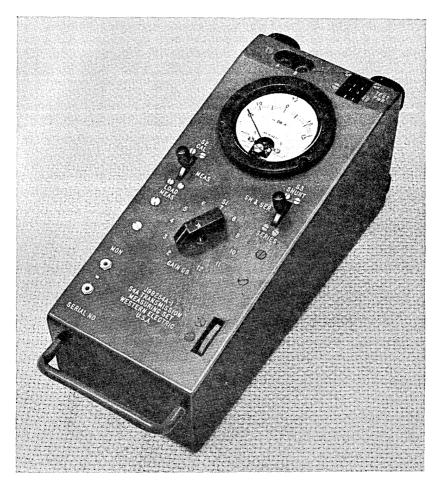
Fig. 40 — 54A transmission measuring set.
