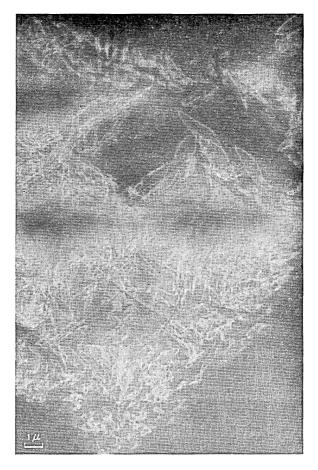
Fig. 6 — Dark-field micrograph. Some of the loops in the upper part of the figure have sides that are parallel to (110) and (310) planes.
