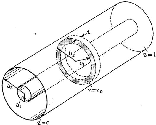
Fig. 2 — Circular coaxial cavity with ferrite ring of thickness  $t$  placed at  $z = z_0$ ;  $a_1$  and  $a_2$  are inner and outer radii of cylinders;  $b_1$  and  $b_2$  are inner and outer radii of ferrite ring.
