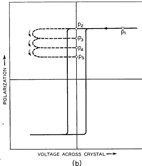
Fig. 1 — (a) Circuit for switching small amounts of charge through a ferroelectric crystal; (b) diagram of crystal's hysteresis loop showing path traced by circuit of (a).
