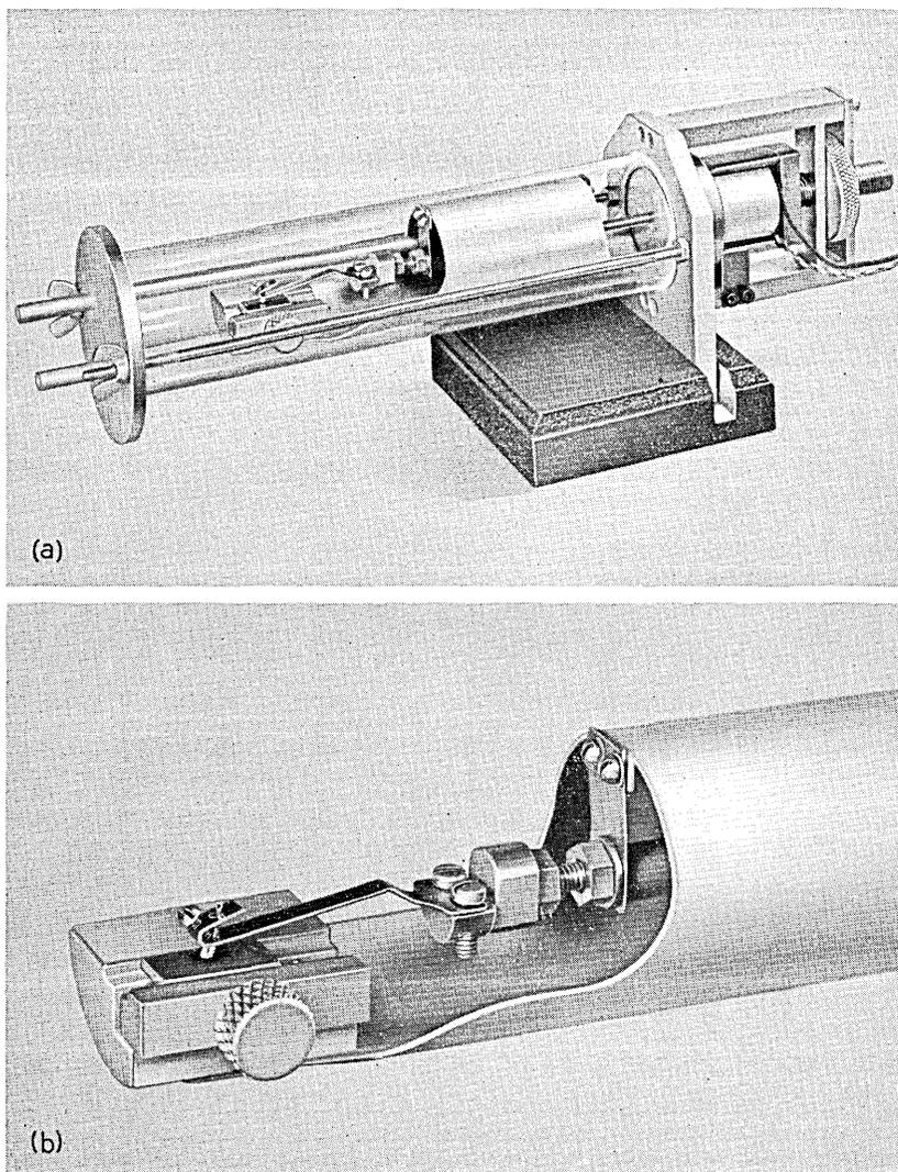
Fig. 5 — Close-up views of electromagnetically driven friction device.
