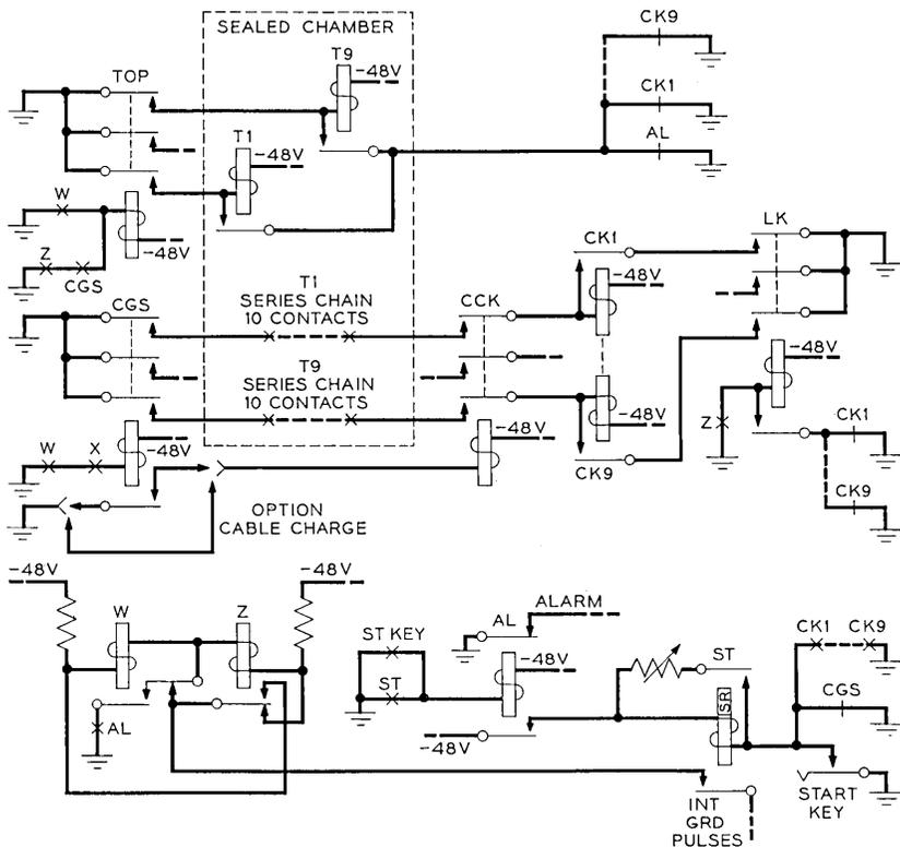
Fig. 18 — Simplified schematic of the OCTM.
