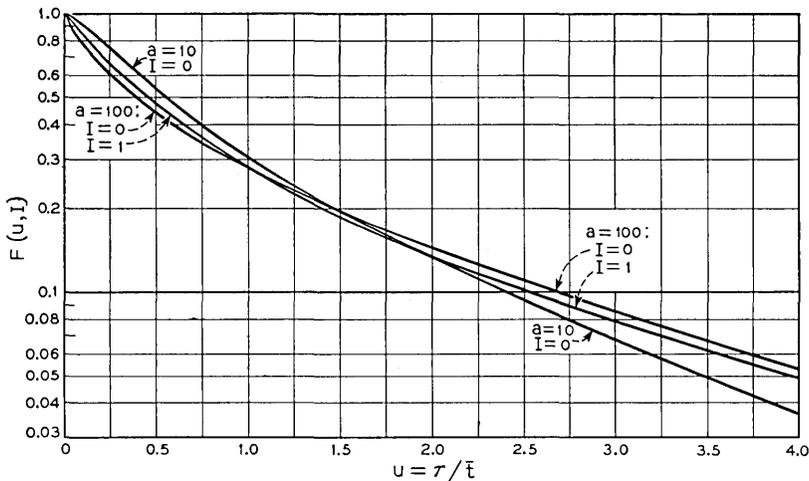
Fig. 13 — The probability  $F(u, I)$  that  $I(t) > I$  for an interval lasting longer than  $\tau$ .  $I(t)$  has the power spectrum given by equation (131) and  $\bar{t}_0$  is  $\pi a^{-1} \sqrt{2a + 1}$ .
