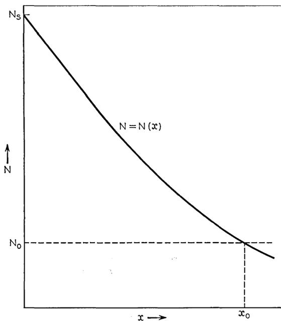
Fig. 1 — Assumed impurity distribution, with  $N_0$  representing the impurity concentration of the original material.
