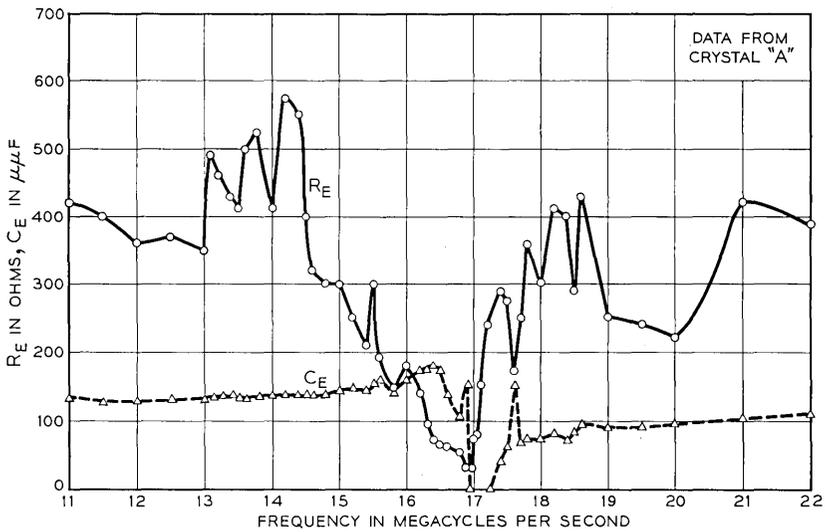
Fig. 4 — Admittance of an unbonded BaTiO<sub>3</sub> single crystal near zero average polarization in the vicinity of its resonant frequency.
