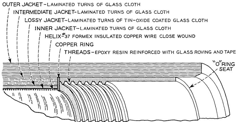
Fig. 4 — Cross-sectional delineation of mode filter.
