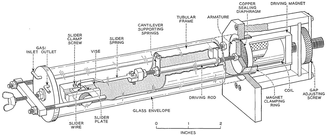
Fig. 4 — Electromagnetically driven friction device.
