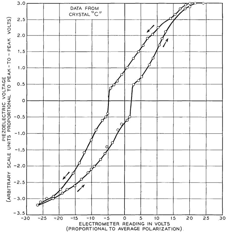
Fig. 12 — Piezoelectric output voltage vs. average polarization of a BaTiO<sub>3</sub> single crystal subjected to constant amplitude strain waves.
