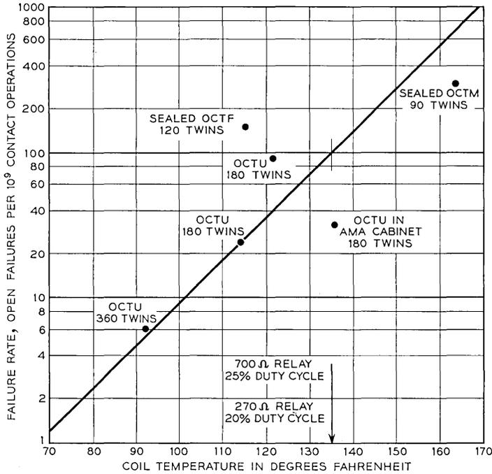
Fig. 10 — Effect of relay coil temperature.
