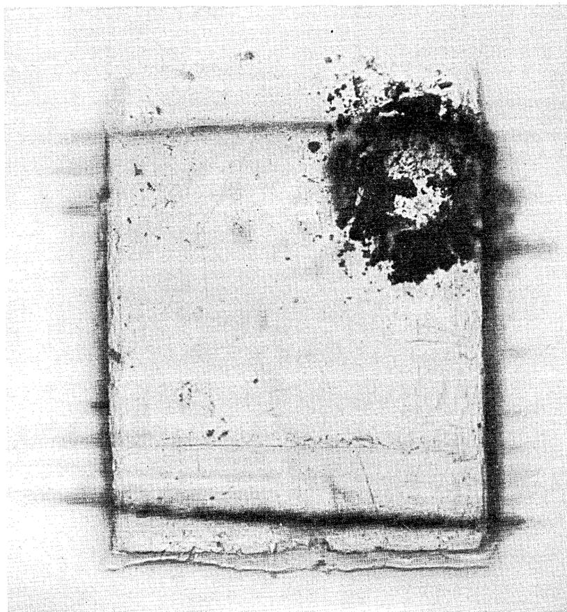
Fig. 3 — Replica of a palladium contact with all inorganic components, showing organic deposit from hexane vapors after 10<sup>6</sup> closures. (Magnified 75 times.)
