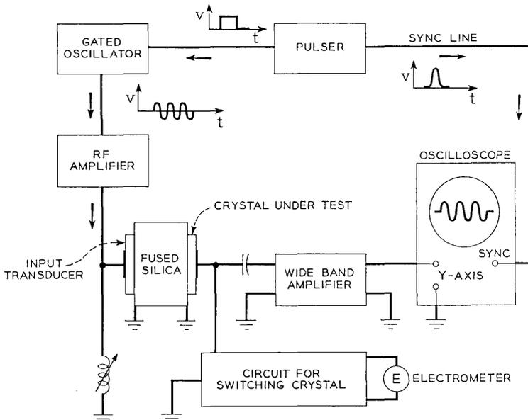
Fig. 11 — Block diagram of apparatus for measuring piezoelectric output voltage of a BaTiO<sub>3</sub> single crystal as a function of its average polarization.
