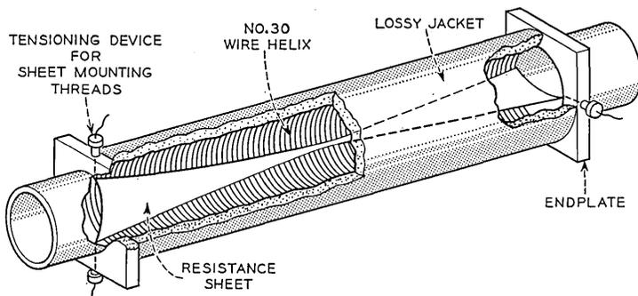
Fig. 10 — A resistance-sheet helix mode filter.
