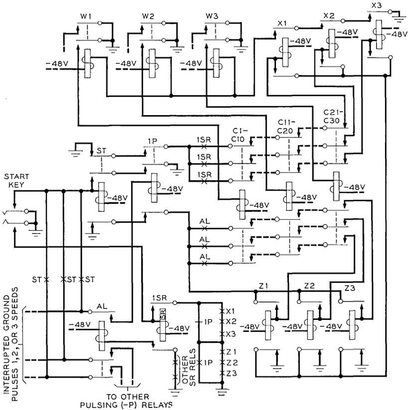
Fig. 19 — Simplified schematic of the octu.
