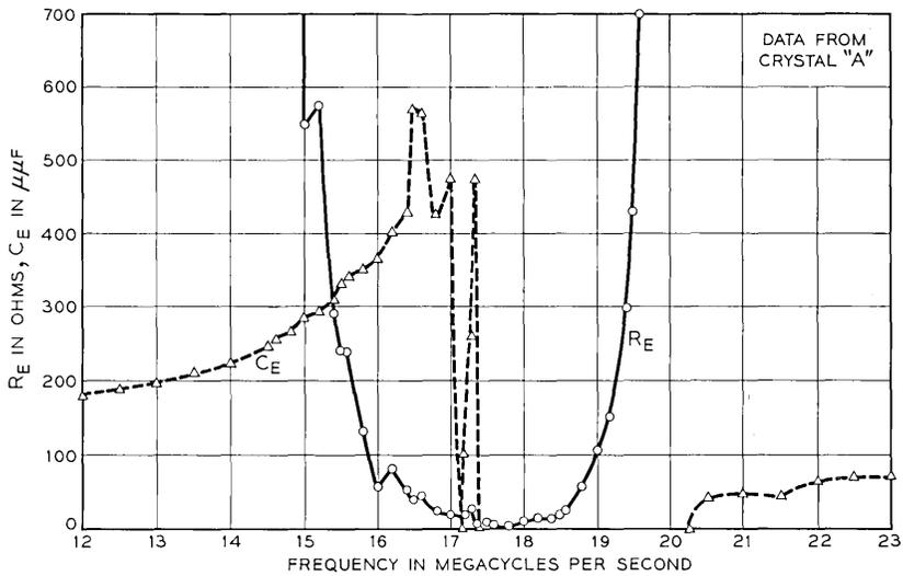
Fig. 3 — Admittance of an unbonded BaTiO<sub>3</sub> single crystal at maximum polarization near its resonant frequency.
