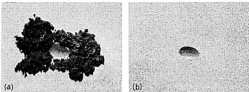
Fig. 8 — (a) Palladium wear products generated in the absence of organic vapors after about  $4 \times 10^6$  wipes; (b) deposit removed, showing deep pit in absence of lubrication by the organic deposit. (Magnified 25 times.)
