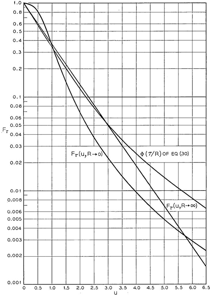
Fig. 4 — Plots of  $F_r(u, R)$  for special cases.  $F_r(u, R \rightarrow \infty)$  is given by (22).  $F_r(u, R \rightarrow 0)$  corresponds to fixed values of the median and fading rate, and is given by (23).  $\Phi(\tau/R)$  of (30) corresponds to fixed median but variable fading rate.
