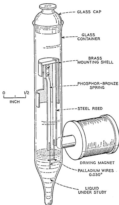
Fig. 14 — Device for generating frictional polymer in liquids.
