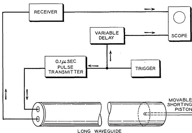
Fig. 1 — Block diagram of pulse transmission test equipment.
