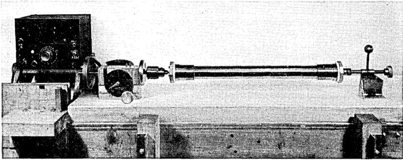
Fig. 3 — Mandrel and machine for winding mode filters.
