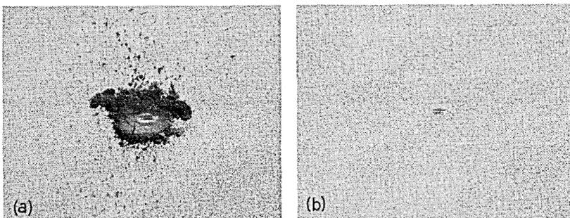
Fig. 9 — (a) Organic deposit formed from benzene vapors after  $4 \times 10^6$  wipes; (b) deposit removed, showing greatly reduced wear due to lubrication by the vapors and deposit. (Magnified 25 times.)
