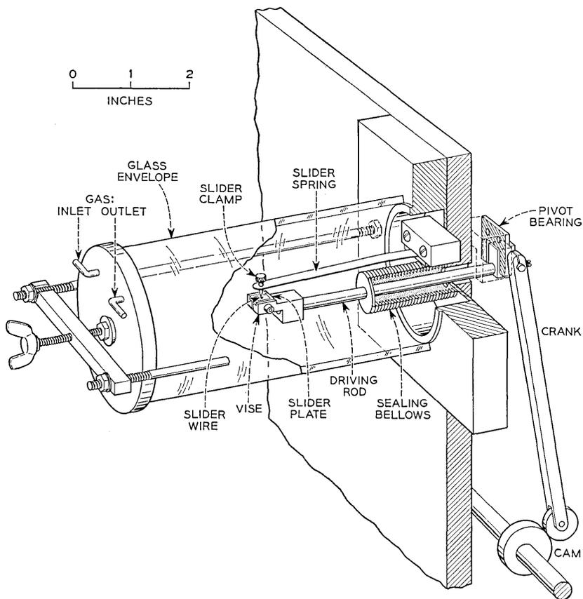
Fig. 6 — Cam-driven friction device.
