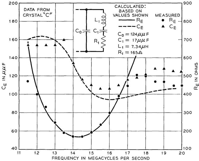
Fig. 7 — Admittance of a bonded BaTiO<sub>3</sub> single crystal near zero average polarization in the vicinity of its resonant frequency.
