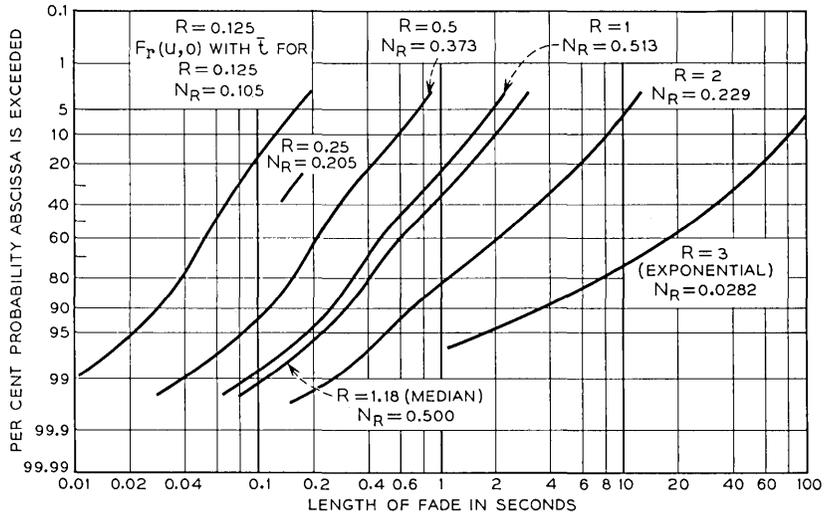
Fig. 3 — Distribution of the duration of fades.  $R(t)$  is the envelope of narrow-band noise. The time scale is chosen so that fades below the median value of  $R(t)$  have an average length of one second.
