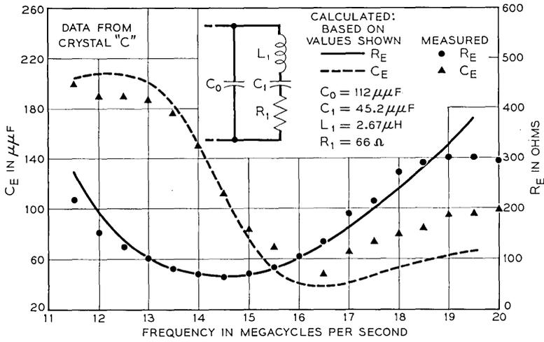
Fig. 6 — Admittance of a bonded BaTiO<sub>3</sub> single crystal at maximum polarization near its resonant frequency.
