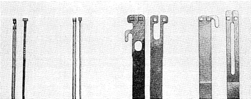
Fig. 14 — Mating twin contact pairs of AF, M24, U and UB relays. The AF and M24 twin contacts are coined to a cylindrical shape, the other contacts have flat surfaces. The AF and M24 twins are made up of two singles which are relatively closer together than in the U and UB relays. Also, the AF and M24 have a common fixed contact, while the U and UB have individual contacts.
