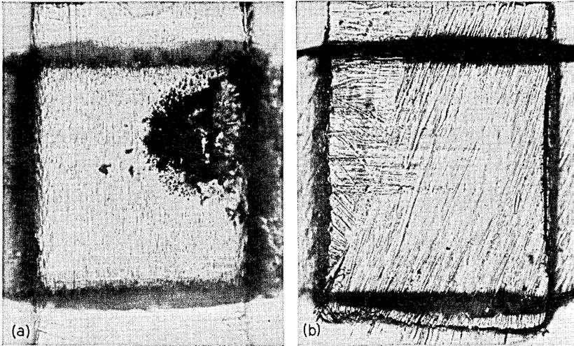
Fig. 1 — (a) Vinylite replica of a palladium relay contact, showing organic deposit formed from vapors of organic structural parts after  $10^6$  closures; (b) replica of a silver relay contact after  $10^6$  closures, showing complete absence of organic deposit. (Both magnified 75 times.)
