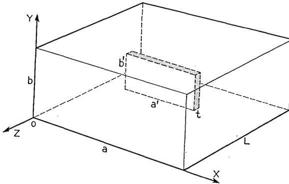
Fig. 3 — Rectangular cavity containing rectangular ferrite slab.
