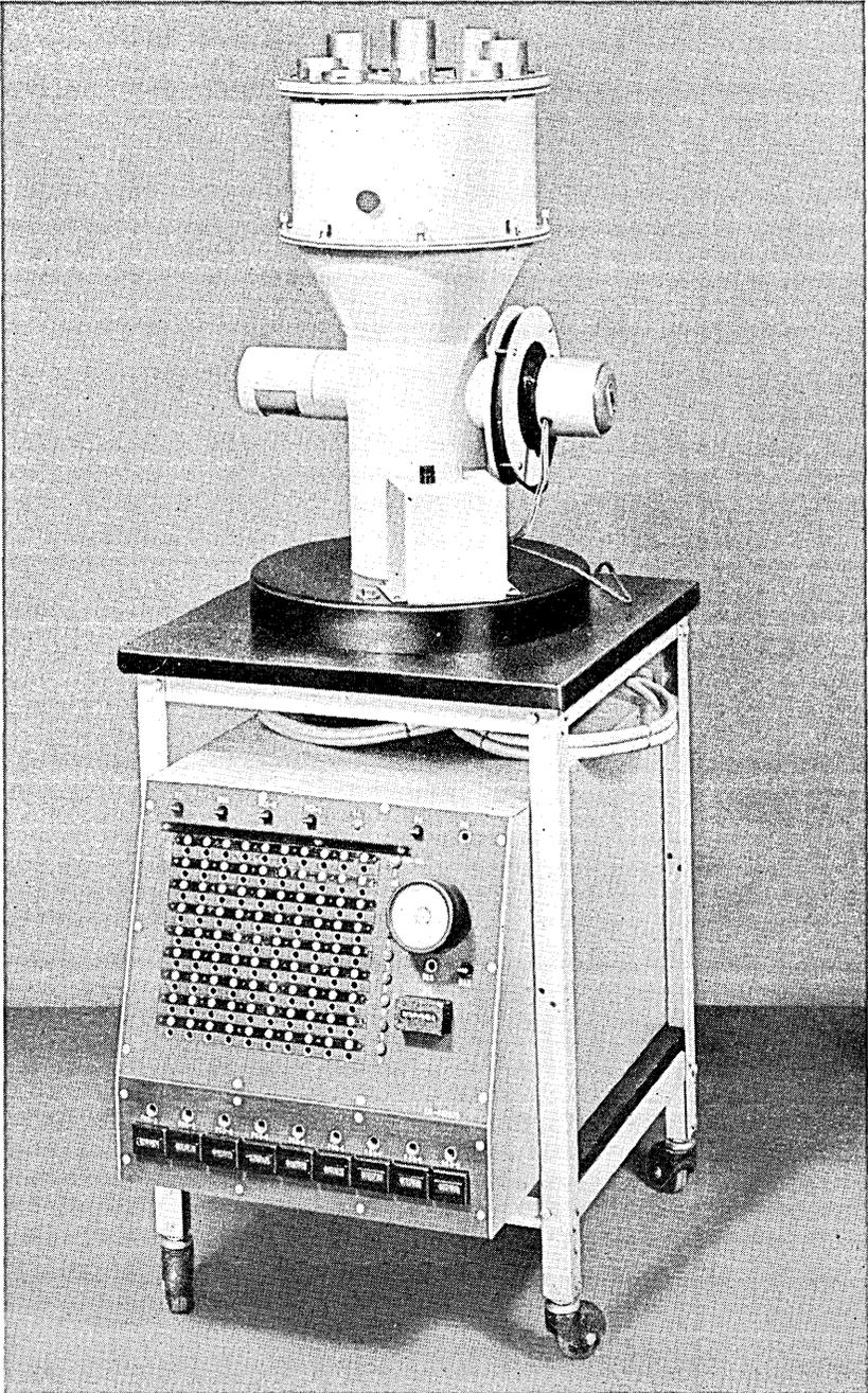
Fig. 2(a) — Open Contact Test Machine (OCTM) is used for exploratory tests of short duration. Single contacts are used instead of twins to increase the failure rate, with usually only one parameter being varied for each test.
