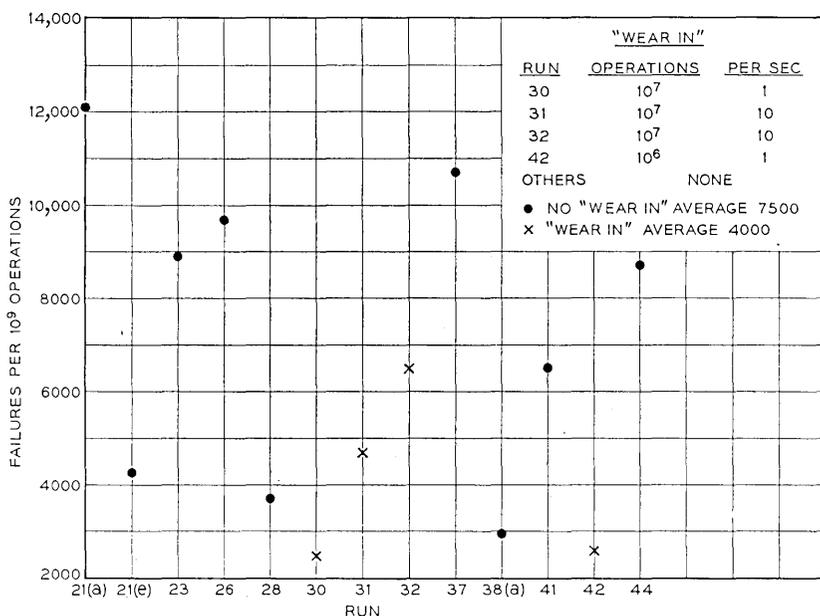
Fig. 8 — Effect of mechanical wearing-in of contacts.
