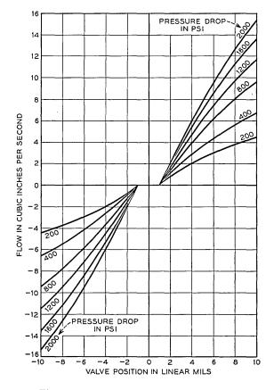
Fig. 12 - Flow characteristics of J-7 valve.
