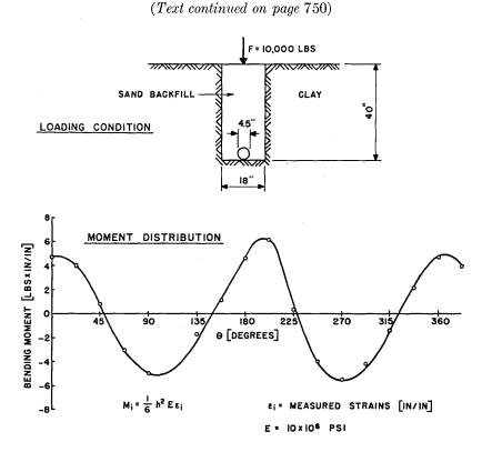
Fig. 8 - Moment distribution in a thin-walled tube, using sand backfill.
