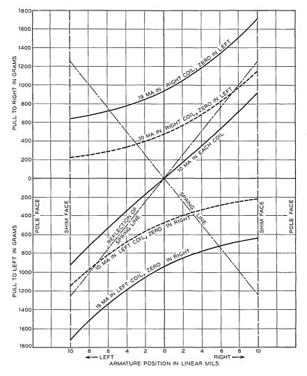
Fig. 10 — Spring and magnetic forces on armature of J-7 valve.
