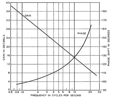
Fig. 19 - Frequency characteristics of J-7 valve.
