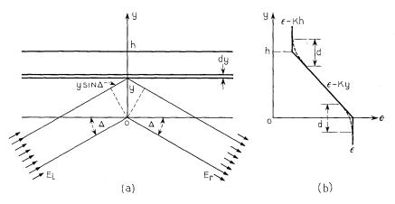
Fig. 3 — Plane-wave reflection at an incremental layer dy within a stratified medium extending from y = 0 to y = h.
