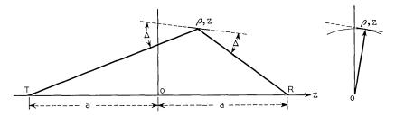
Fig. 6 — Grazing angle  $\Delta$  at a layer.
