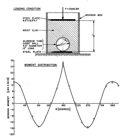
Fig. 9 — Moment distribution in thin- walled tube resting on steel plate and covered with moist elay.
