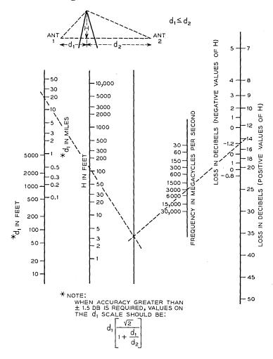
FIG. 7 -Knife-edge diffraction loss relative to free space.
