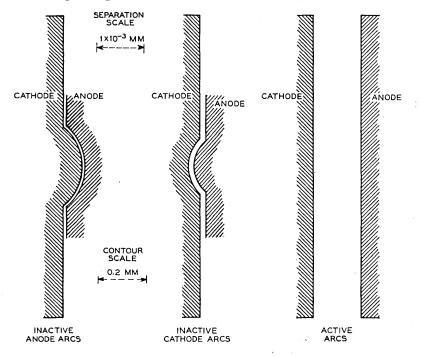
Fig. 8 — Erosion produced by anode arcs at clean surfaces, by inactive cathode arcs and by active arcs of either type, the total energy in each case being 10<sup>8</sup> ergs. The electrode separations at which these arcs strike correspond to 50 volts and are represented here on a greatly expanded scale.
