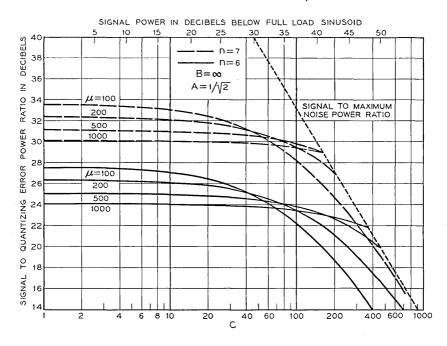
Fig. 20 — Curves illustrating the comparison of signal to quantizing error power ratios with the ratio of signal to background noise. The line representing the signal to maximum noise ratios corresponds to the hypothetical case where the maximum background noise is determined by the requirement that the signal to noise ratio be 20 db for a signal 50 db below full sinusoidal modulation.
