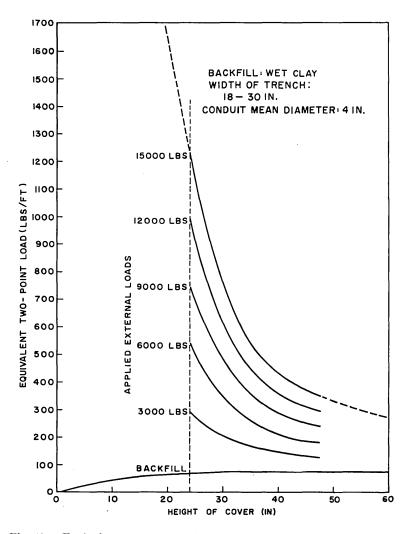
Fig. 12 - Equivalent two-point load versus height of cover for clay backfill.
