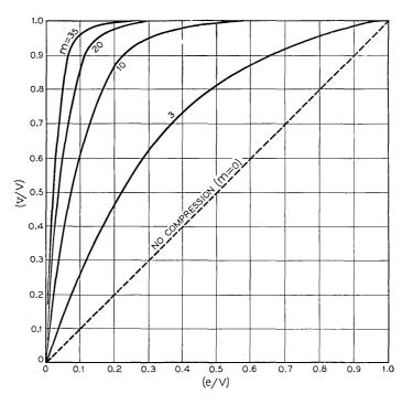
Fig. 21 — Typical *m*-ensemble compression characteristics determined by equation (A-7). Note the strong emphasis on weak signal amplitudes. These curves may be compared with those for the  $\mu$ -ensemble in Fig. 3.
