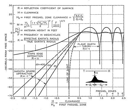
FIG. 8 — Transmission loss versus clearance.
