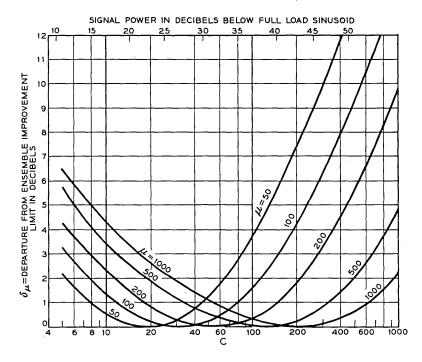
Fig. 14 — Improvement selectivity, i.e., departures from the ensemble upper limit of improvement due to the use of a single value of  $\mu$  rather than the ensemble of  $\mu_c$  values. The minima at  $\delta_{\mu} = 0$  locate the signals (C) for which  $\mu$  and  $\mu_c$  coincide. All curves correspond to the case where the "dc component",  $e_0$ , is zero.
