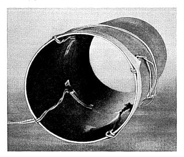
Fig. 1 — Thin-walled tube with SR-4 strain gages.
