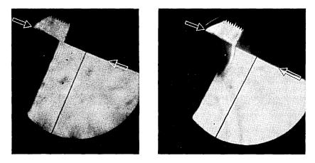
Fig. 15 — Oil flow through simple port.
