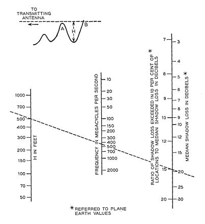
FIG. 11 — Estimated distribution of shadow losses.
