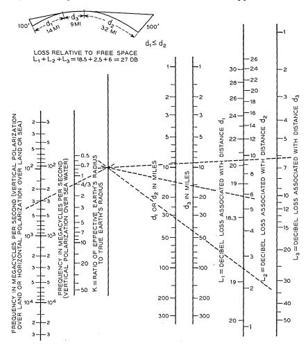
FIG. 6 — Diffraction loss relative to free space transmission at all locations beyond line-of-sight over a smooth sphere.
