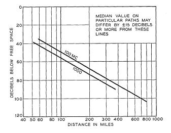
FIG. 9 — Beyond-horizon transmission — median signal level versus distance.
