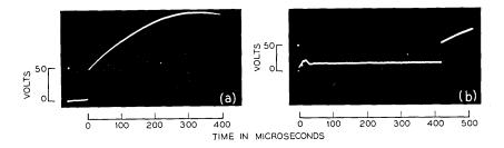
Fig. 1 — Oscilloscope traces of the voltage across relay contacts breaking a current of half an ampere through an inductive relay load. In each case a standard protective network of a  $0.5 \,\mu$ f capacitor in series with 100 ohms is in parallel with the contacts. (a) Clean or "inactive" contacts, with no observable arc. (b) Active contacts, with a sustained arc lasting 400 microseconds.
