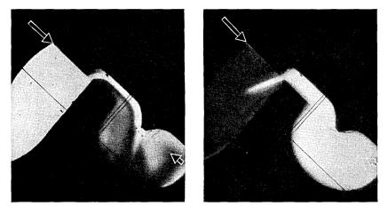
Fig. 17 — Flow through port with decreased Bernoulli effect and increased flow.
