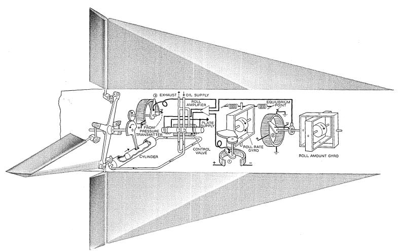
The roll system's reference is an "Amount Gyro," which is a free-free gyro oriented on the ground prior to missile launch. The brush of a fourtap potentiometer (Item 2 in Fig. 1) is connected to the outer gimbal and provides a dc signal whose sign and magnitude indicate the roll position with respect to the stable equilibrium point. This signal is the principal input to the servo amplifier that drives the valve.
