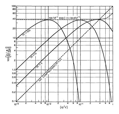
Fig. 23 — Pulse sample to step size ratios as a function of relative sample amplitude, for various compandors in the *m*-ensemble. The maxima exhibited by these curves occur at  $e/V = m^{-1}$ ;  $M = 1 - \exp(-m)$ . Compare with Fig. 5.
