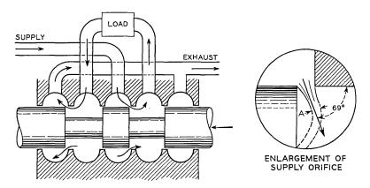
Fig. 13 — Simple valve with rectangular lands.
