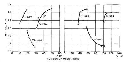
Fig. 3 — Measurements of arc voltage at cathode arcs between a carbon-platinum pair of electrodes, and between a carbon tungsten pair — at successive reversals of striking potential.
