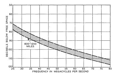
FIG. 18 — Median signal levels for ionospheric scatter transmission.
