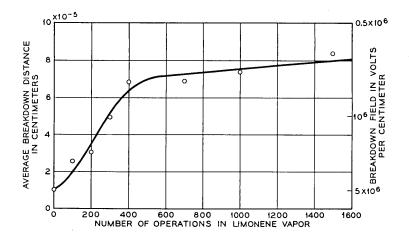
Fig. 2 — Breakdown distance, and apparent striking field, for arcing at relay contacts on closure in the presence of limonene vapor, plotted against number of operations. Each closure discharges a very small capacitor charged to 50 volts. Contacts are clean and inactive at the beginning of the test.
