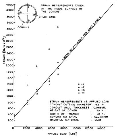
Fig. 3 — Strain measurements versus applied load.
