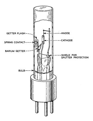
Fig. 5 — A talking-path switching diode.
