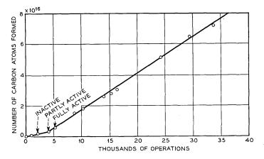
Fig. 10 — Measurements by P. Kisliuk of the amount of carbon formed at arcing platinum contacts, each arc 1,250 ergs. The final slope represents the production of  $3.5 \times 10^{-14}$  gm of carbon per erg of arc energy, or one benzene molecule decomposed for every 150 electrons flowing in the arc.
