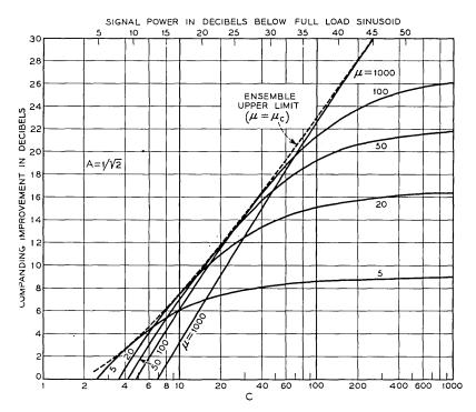
Fig. 8 — Companding improvement (in db), as calculated from equation (37), for various values of  $\mu$ . The saturated improvement for weak signals (relatively constant ordinate for large C values) is identical with the asymptotic behavior for weak signals which is predicted by Fig. 9.
