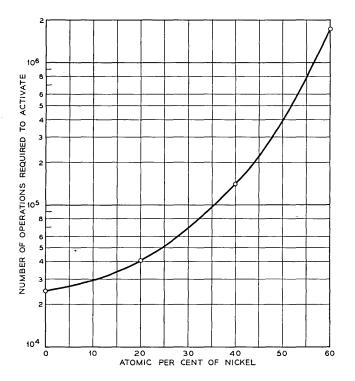
Fig. 11 — Resistance to activation of various alloys of nickel and palladium.
