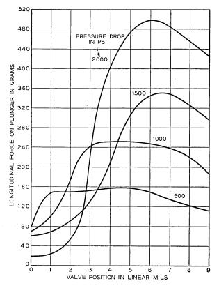
Fig. 18 — Force on plunger of J-7 valve due to Bernoulli effect.
