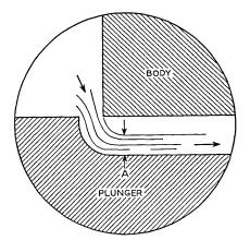
Fig. 14 - A compensated valve orifice.
