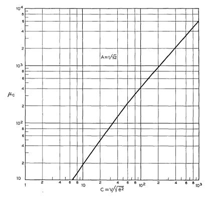
Fig. 7 — Critical compression parameters,  $\mu_e$ , required to minimize the quantizing error power as a function of relative signal strength, as determined by equation (36). Each point on the curve defines a compandor in the optimum compandor ensemble. It must be understood that such an ensemble provides the best performance consistent with equation (8) rather than the absolute minimum quantizing error discussed in the Appendix.
