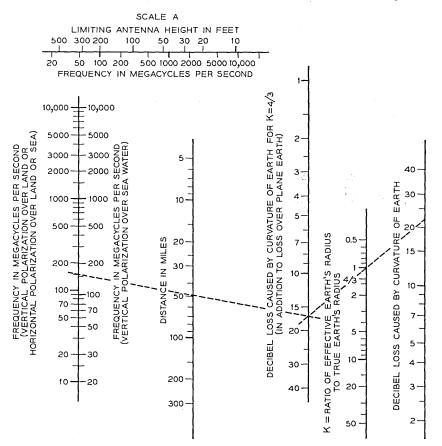
FIG. 5 — Diffraction loss around a perfect sphere.
