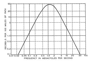
FIG. 17 — Typical values of midday ionospheric absorption.
