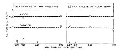
Fig. 6 — Results of measurement by weighing of the erosion of palladium electrodes produced by active arcs in limonene vapor (a) and in napthalene vapor (b).
