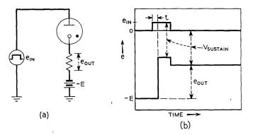
Fig. 1 — Simplified gas diode switching circuit.
