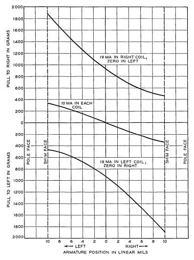
Fig. 11 — Resultant forces on armature of J-7 valve.
