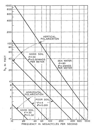
FIG. 3 — Minimum effective antenna height.
