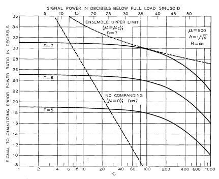
Fig. 17 — Signal to quantizing error power ratios (in db) as a function of relative signal power for companding corresponding to  $\mu = 500$ . Symbols have the same significance as in Fig. 15.  $B = \infty$  throughout.
