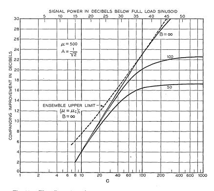
Fig. 12 — The effect of a "dc component" on companding improvement for  $\mu = 500$ . For further details, see the caption of Fig. 10.
