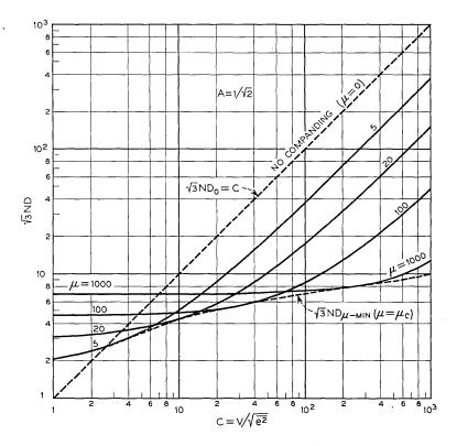
Fig. 6 — Variation of the rms error to signal voltage ratio (D) with relative signal strength,  $C = V/\sqrt{\frac{e}{e^2}}$ , as given by equation (27) for various degrees of logarithmic companding.
