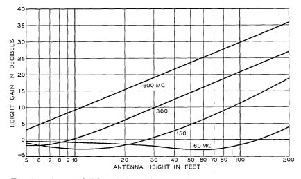
FIG. 15 - Antenna height gain factor for vertical polarization over sea water.
