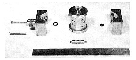
Fig. 7 — Hydraulic parts of the J-7 valve.
