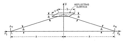
Fig. 1 — Reflection by a layer.
