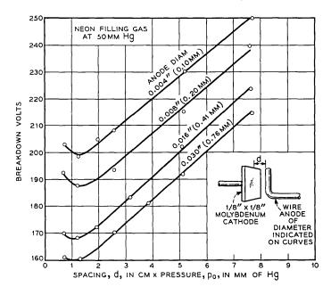
Fig. 4 — Breakdown voltage as a function of spacing and pressure for small wire anodes parallel to cathode surface.
