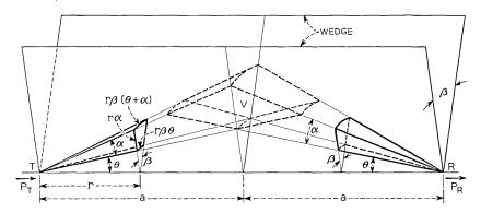
Fig. 7 — Idealized antenna patterns used in this study.
