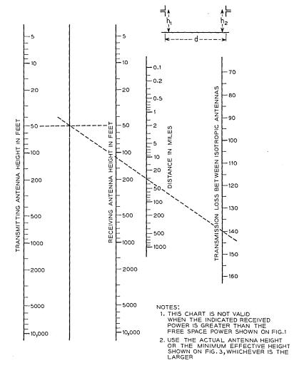
FIG. 2 — Transmission loss over plane earth.
