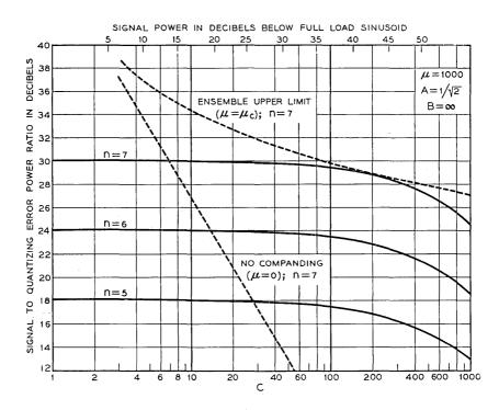
Fig. 18 — Signal to quantizing error power ratios (in db) as a function of relative signal power for companding corresponding to  $\mu = 1,000$ . Symbols have the same significance as in Fig. 15.  $B = \infty$  throughout.
