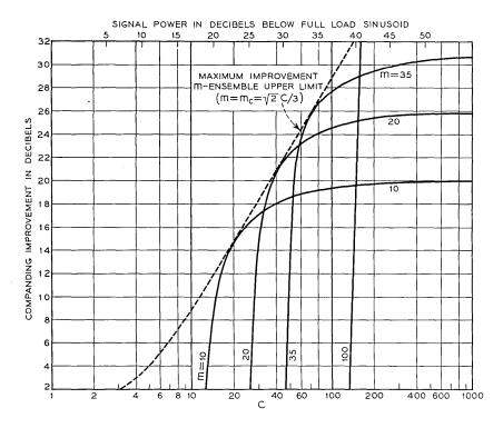
Fig. 25 — Companding improvement curves for representative members of the *m*-ensemble. These curves are to be compared with those for the  $\mu$ -ensemble in Fig 8. Note the important difference between the two ensembles for strong signals (small values of C).
