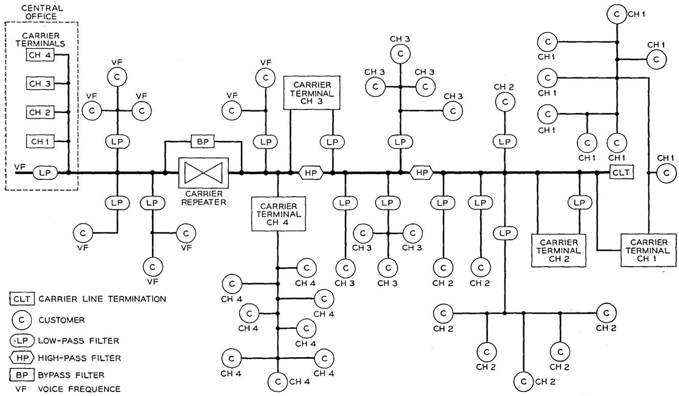
Fig. 26 — Typical P1 carrier application schematic.
