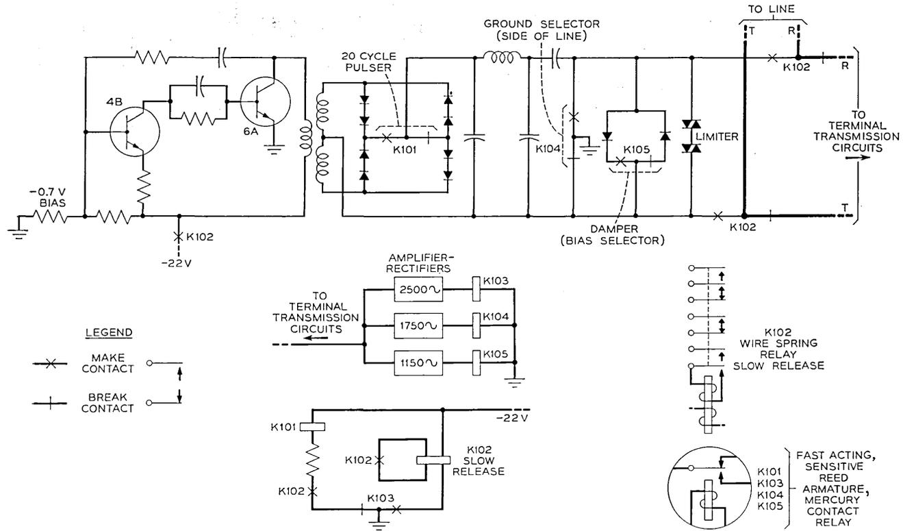
Fig. 6 — Remote terminal 20-cycle ringing generator.
