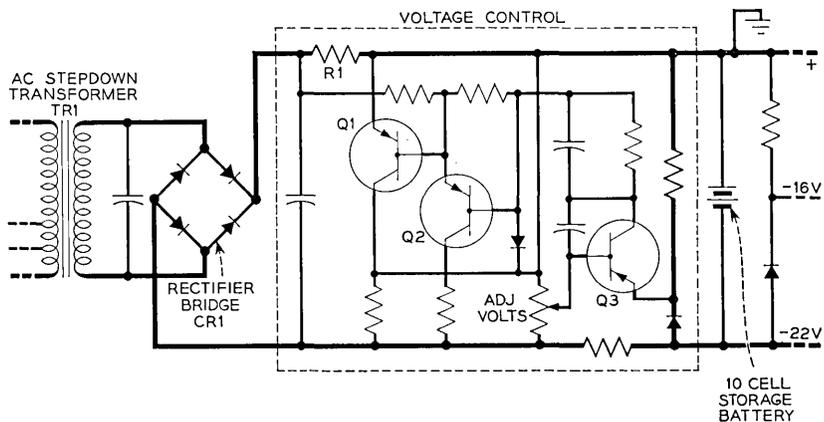
Fig. 21 — Schematic of ac rectifier-battery power supply.
