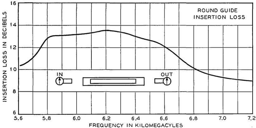
Fig. 7 — Insertion loss of 6-kmc coupler.
