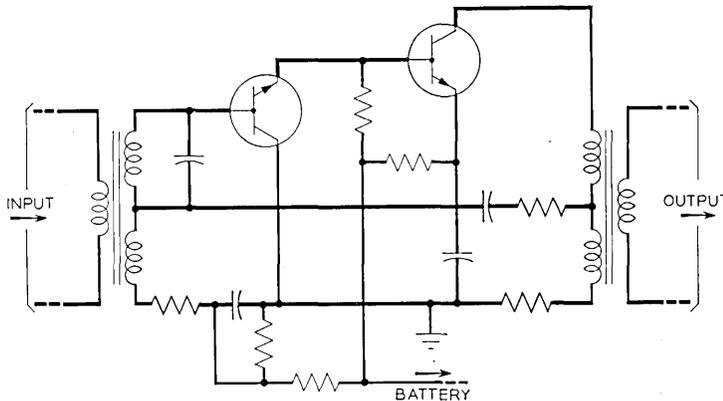
Fig. 3. — P1 transistor transmitting amplifier circuit.
