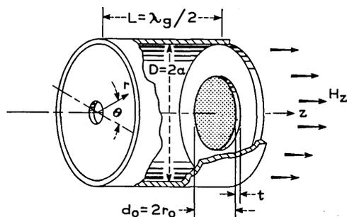
Fig. 3 — Degenerate  $TE_{111}$  cylindrical cavity with ferrite disc.
