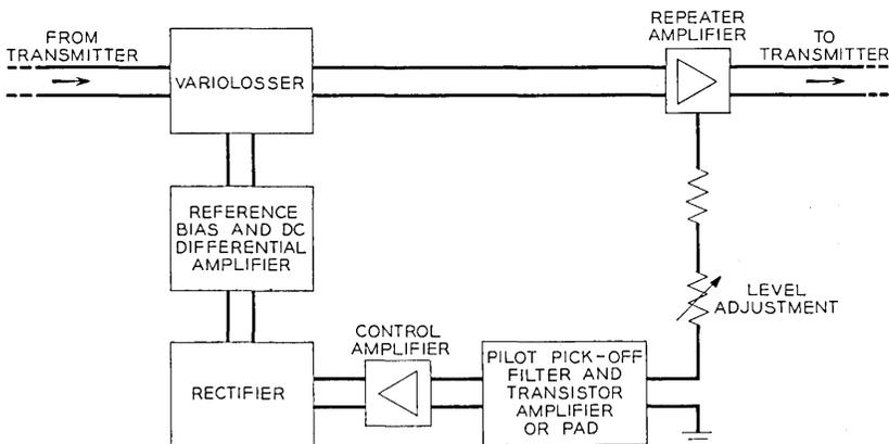
Fig. 10 — P1 Repeater regulator block schematic.
