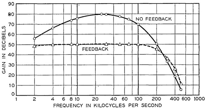
Fig. 9 — P1 Repeater amplifier gain-frequency characteristic.
