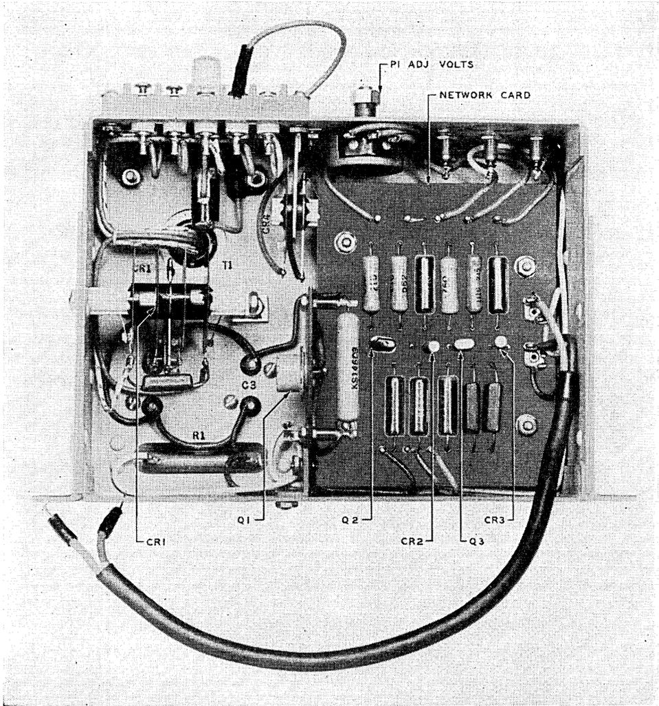
Fig. 24 — Close-up of bottom of rectifier chassis.
