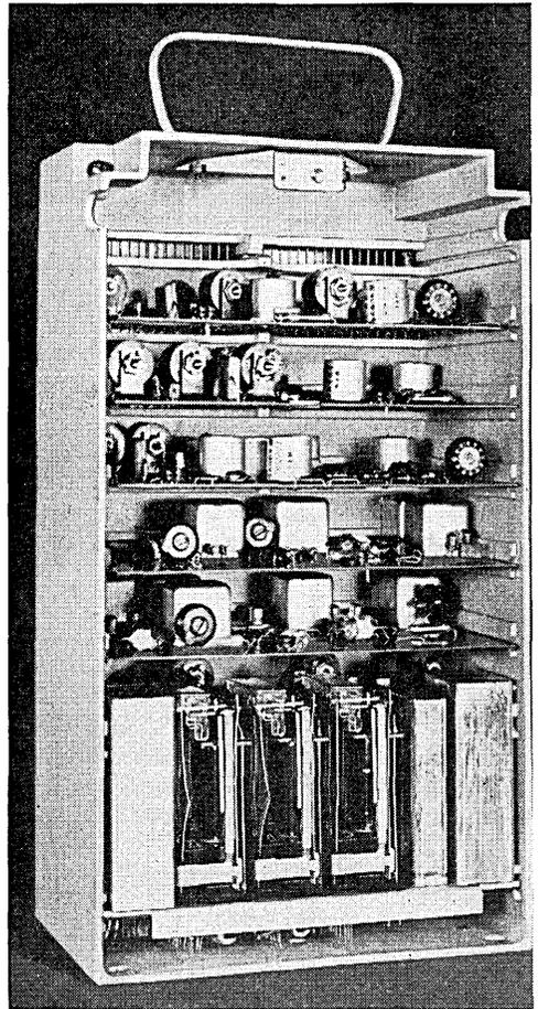
Fig. 18 — Typical terminal networks mounted in a prototype connector box.
