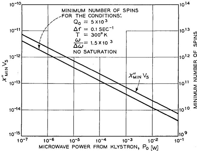
Fig. 5 — Minimum RF susceptibility and number of electrons which should be observable under thermal noise limitations. The conditions for the minimum number of spins correspond closely to those under which the experimental set-ups were tested.
