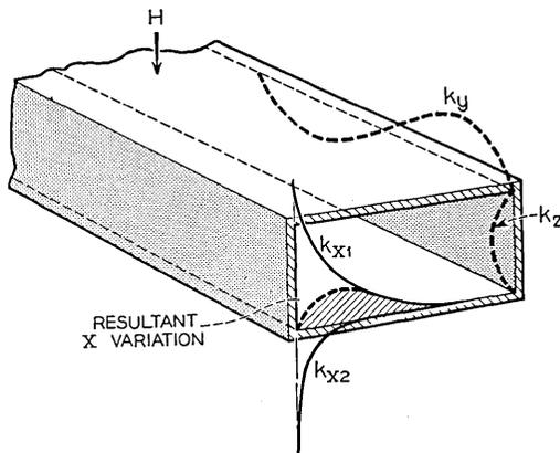
Fig. 2 — Mode in ferrite filled rectangular guide.
