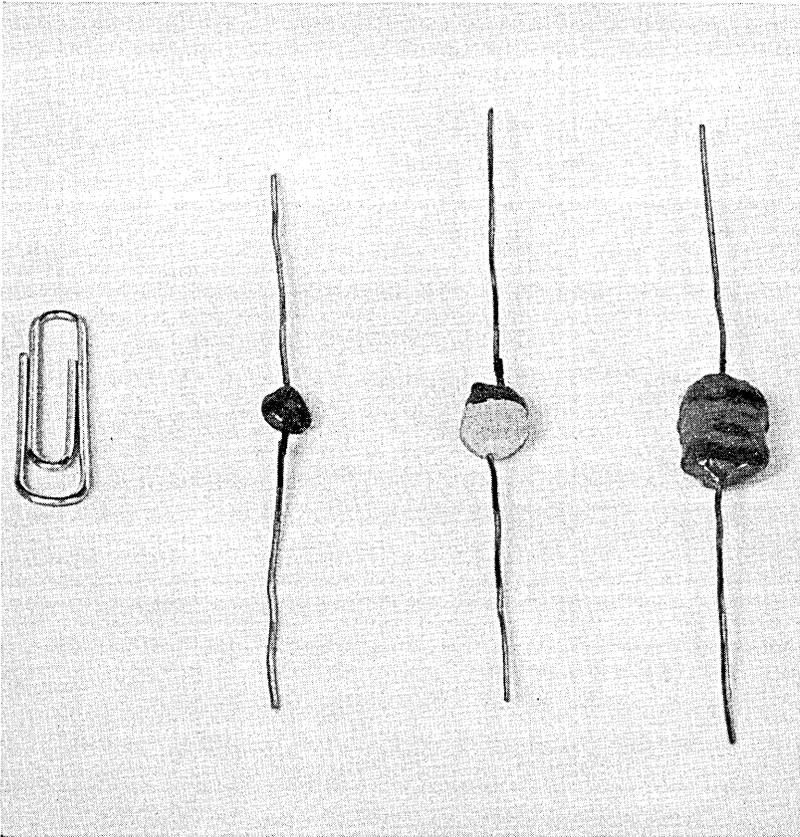
Fig. 12 — Prototype solid tantalum capacitors for P1 carrier.
