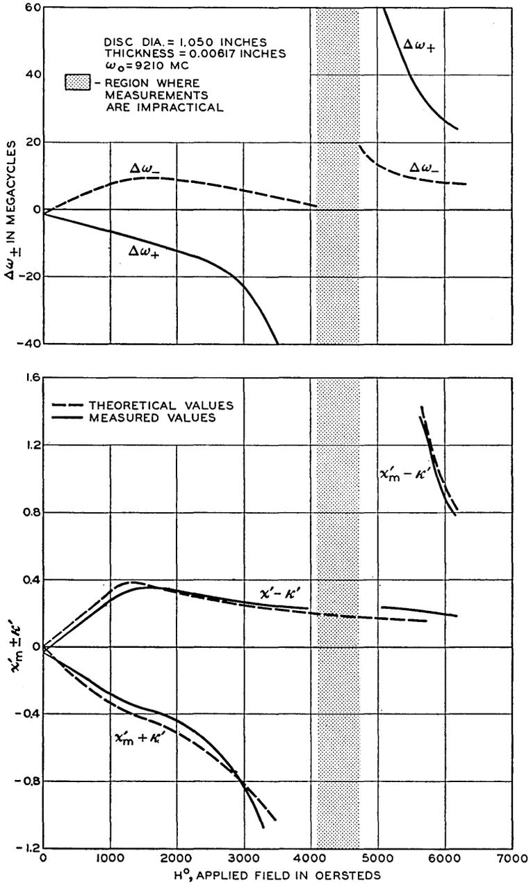
FIG. 6 — Evaluation of  $\chi'_m \pm \kappa'$  from measurements of frequency shift  $\Delta\omega_{\pm}$  and comparison with Polder's theory. Low-loss BTL ferrite, saturation magnetization 1300 oersted.
