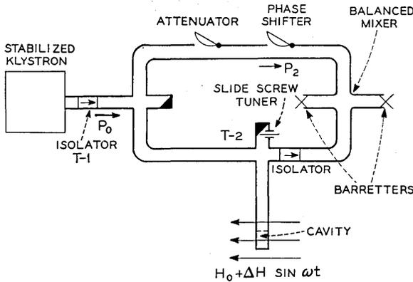
Fig. 8 — Barretter system with balanced mixer.
