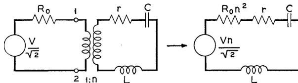
Fig. 2 — Equivalent circuit for a reflection cavity.
