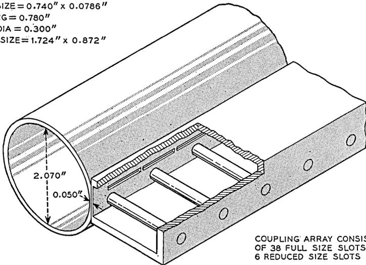
COUPLING ARRAY CONSISTS OF 38 FULL SIZE SLOTS & 6 REDUCED SIZE SLOTS
