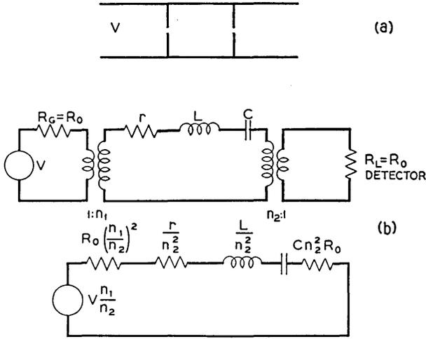
Fig. 3 — Equivalent circuit for a transmission cavity.
