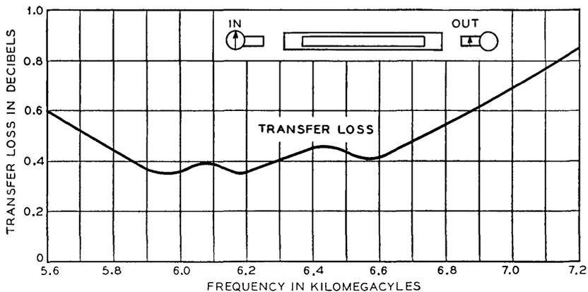
Fig. 6 — Transfer loss of 6-kmc coupler.
