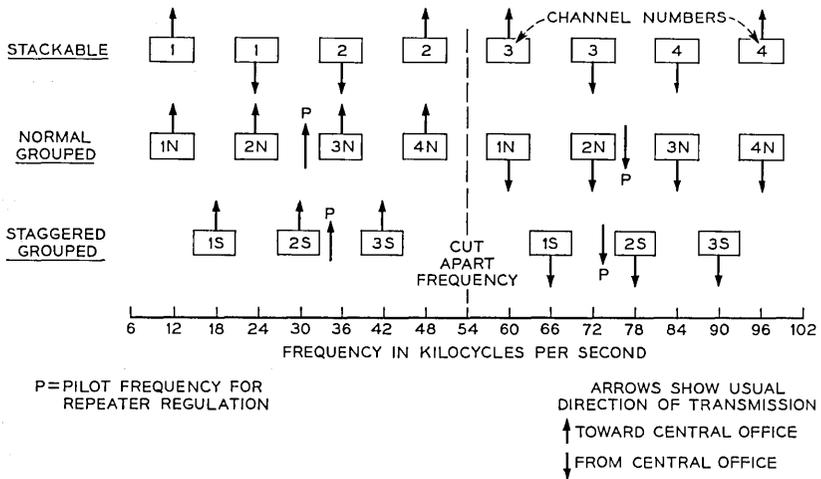
Fig. 1 — Type P1 Carrier Frequency Plan.
