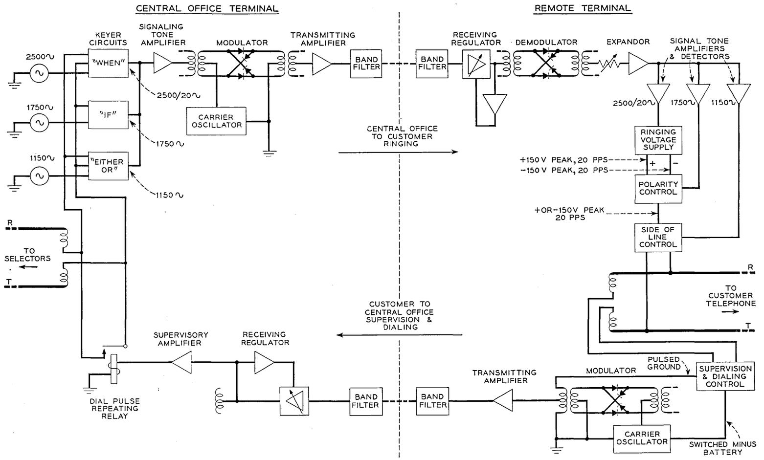
Fig. 5 — P1 signaling block schematic.
