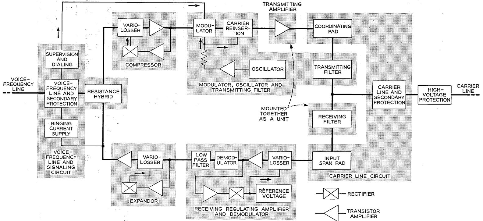
Fig. 2 — P1 Carrier remote terminal block diagram.
