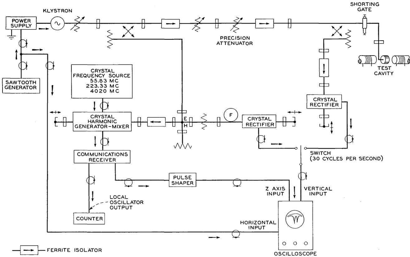
Fig. 5 — Microwave circuit for measuring ferrite parameters.
