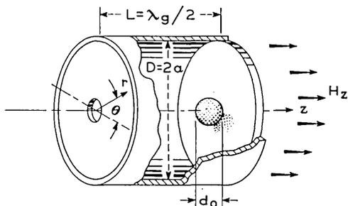
Fig. 2 — Degenerate  $TE_{111}$  cylindrical cavity with ferrite sphere.
