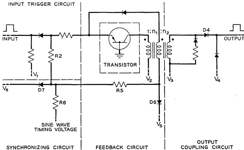
Fig. 11 — Shunt connection of output and feedback.
