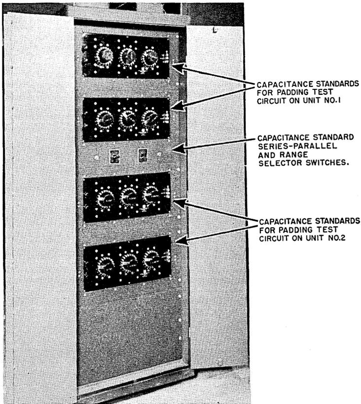
Fig. 6 — Control panels for capacitance circuits.
