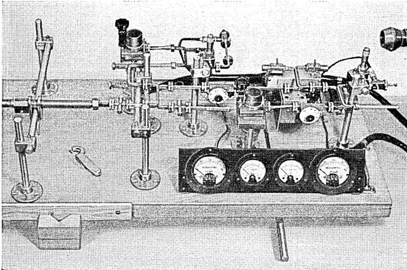
Fig. 2 — Waveguide portion of millimeter wave measuring set.
