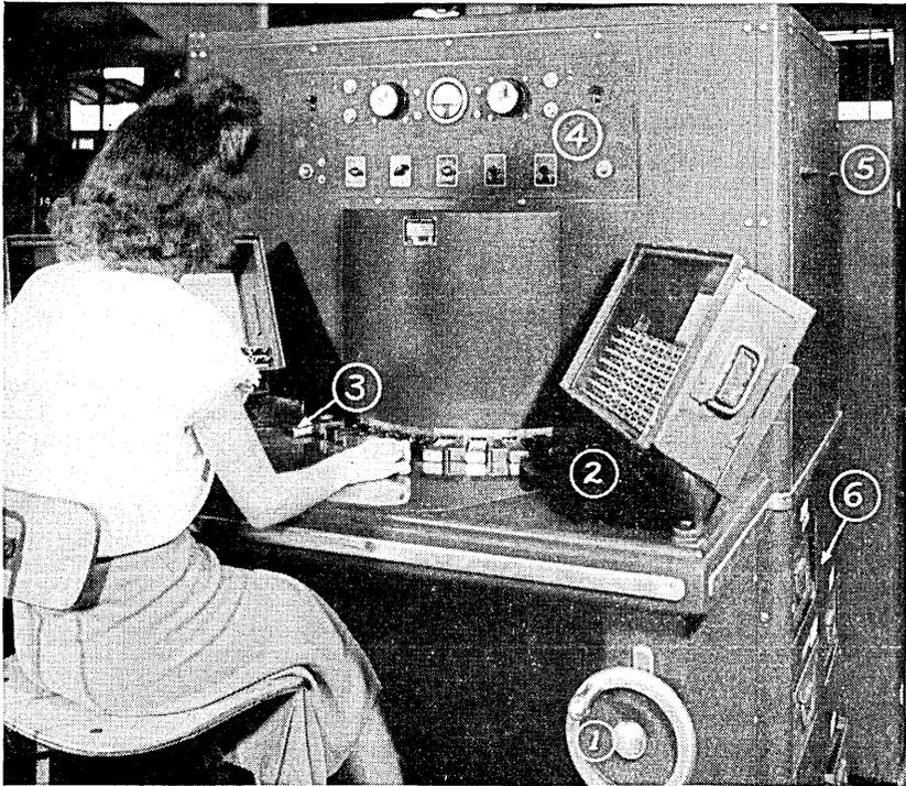
1. HANDWHEEL FOR POSITIONING TEST FIXTURES.
