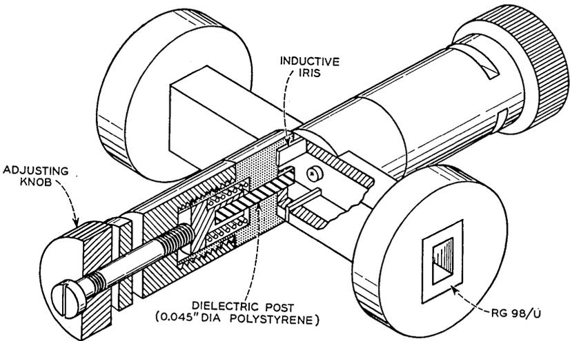
Fig. 4 — Structure of impedance matching tuner.
