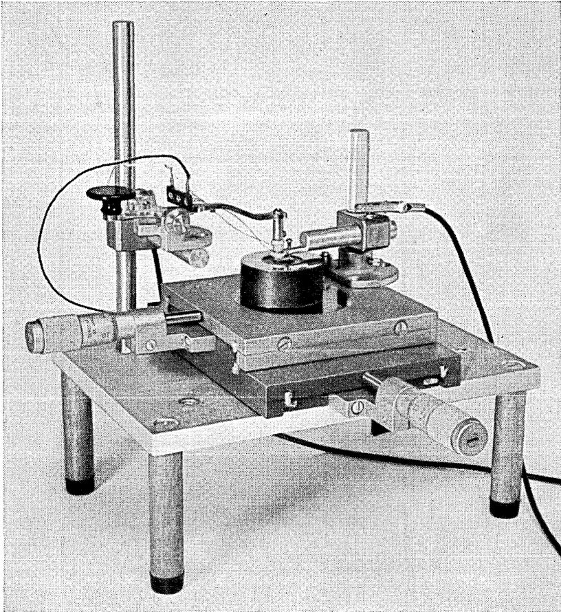
Fig. 2 — Apparatus for locating and marking  $p$ - $n$  junctions.
