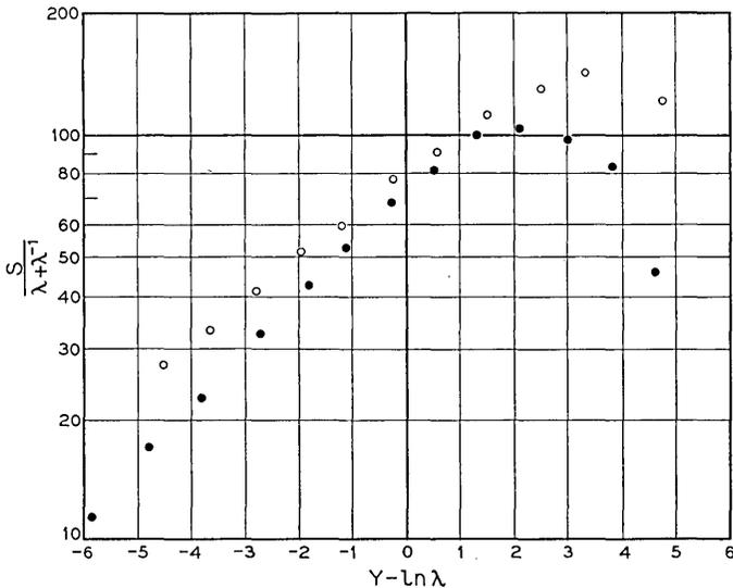
Fig. 7 — Surface recombination velocity versus surface potential. The curves show  $s/(\lambda + \lambda^{-1})$  plotted against  $Y - \ln \lambda$ . Dots:  $p$ -type; circles:  $n$ -type.
