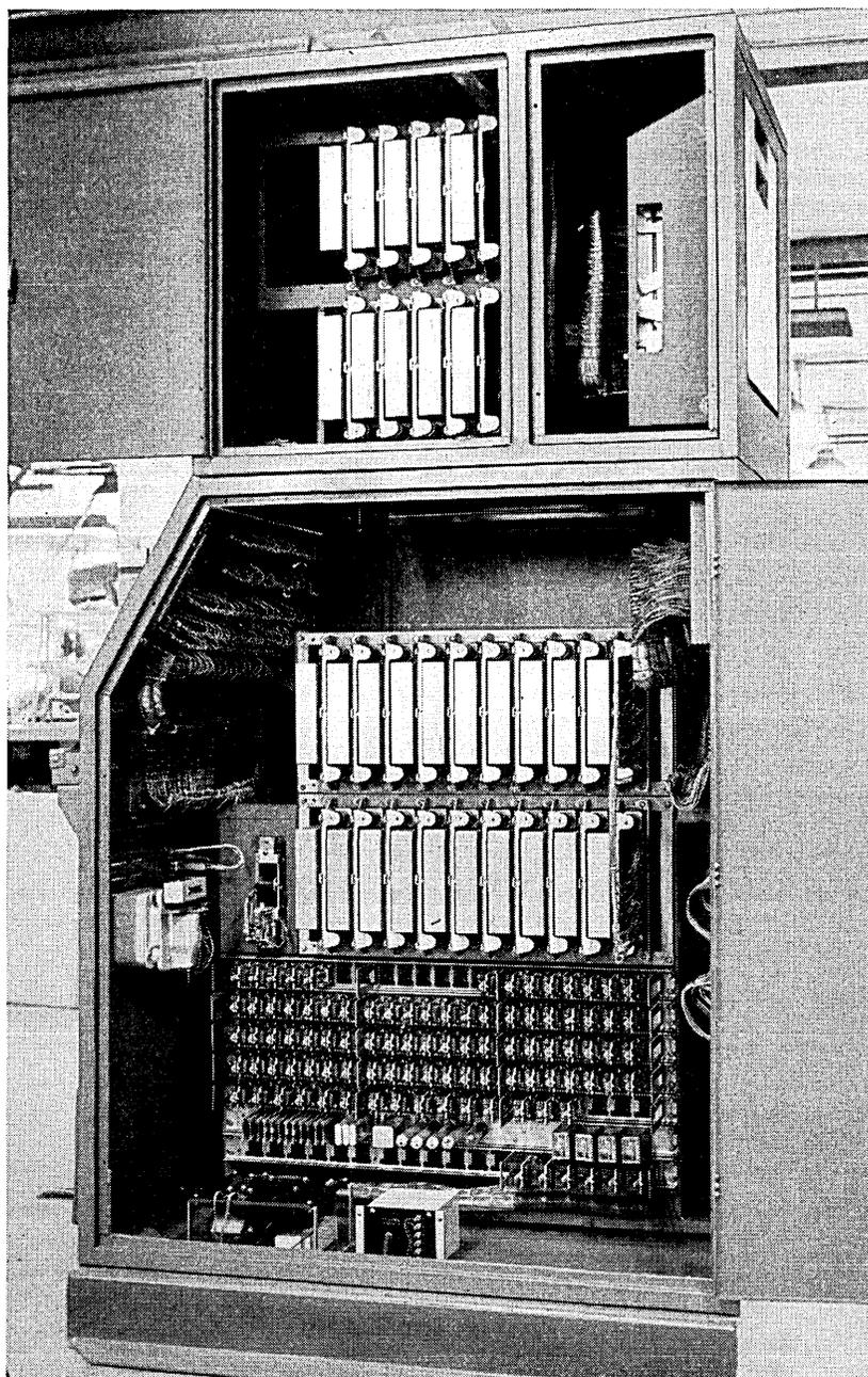
Fig. 7 — Interior of Card-O-Matic test set.
