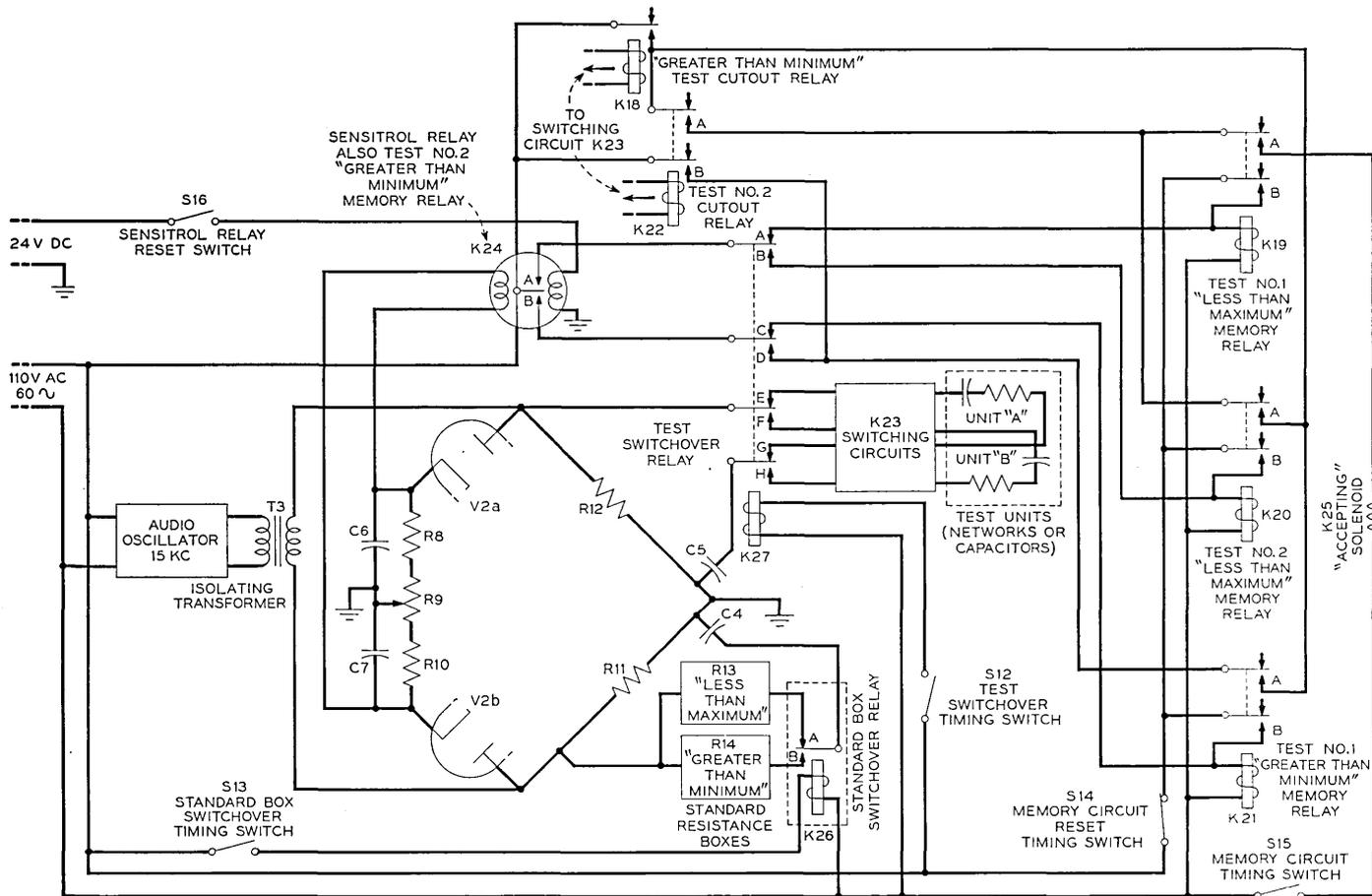
Fig. 9 — Simplified schematic of impedance test circuits.
