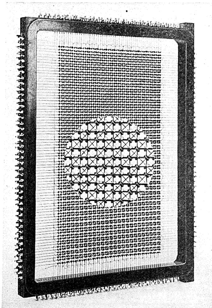
Fig. 18 — Magnetic core array (Courtesy of IBM).
