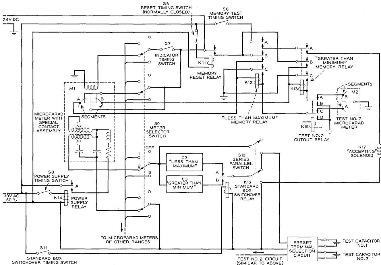
Fig. 11 — Simplified schematic of capacitance test circuits.
