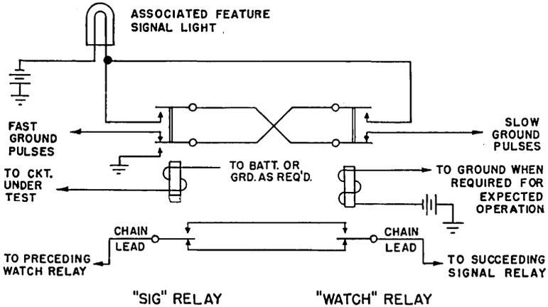
Fig. 9 — Chain circuit showing watching relay function.
