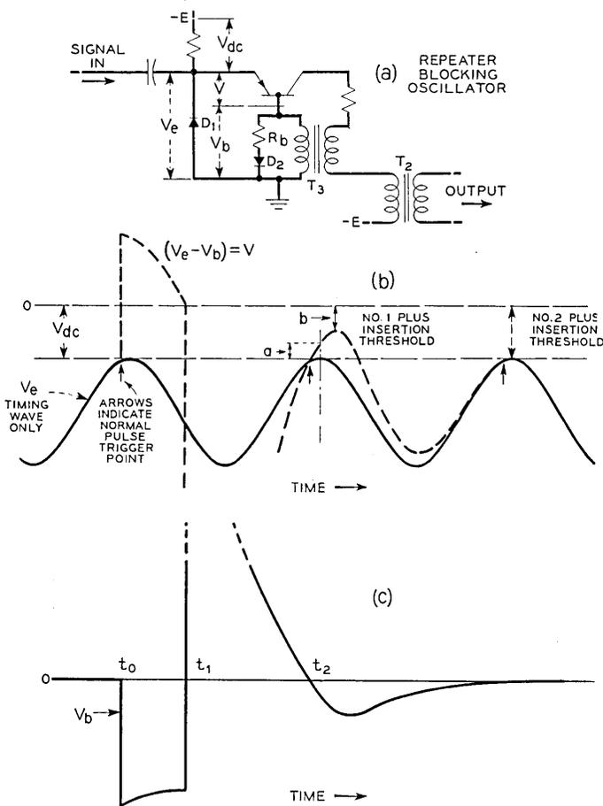
Fig. 10 — (a) Circuit diagram of blocking oscillator showing various components of the effective bias. (b) The effective bias as a function of time. (c) Inhibiting voltage  $V_b$  produced by a regenerated pulse.
