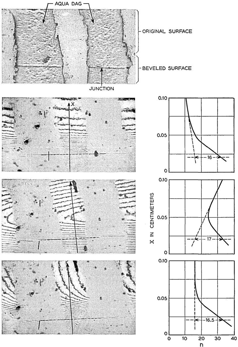
Fig. 8 — Evaluation of the interference fringe pattern on a scribed  $p-n$  junction.
