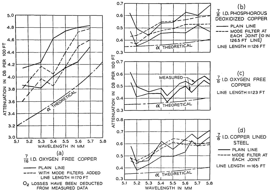
Fig. 8 — Measured and theoretical loss of the four lines studied.
