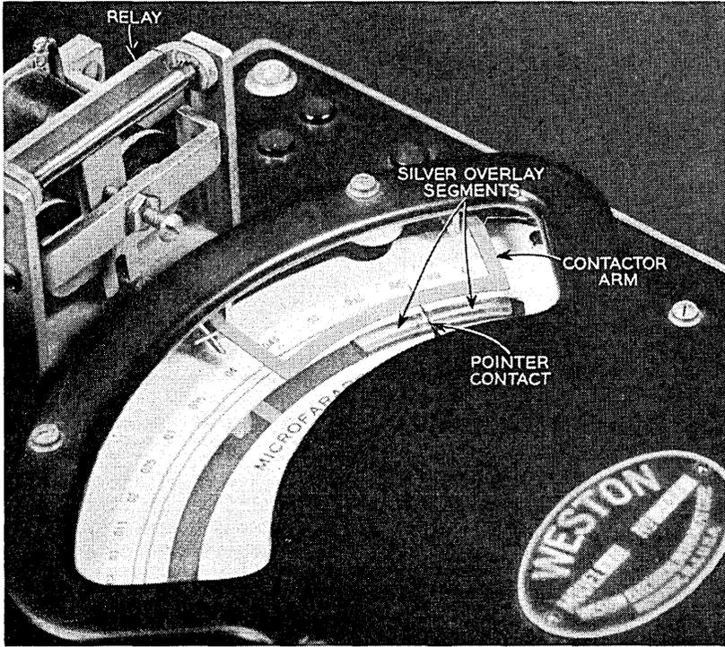
Fig. 10 — Details of modified microfarad meter.
