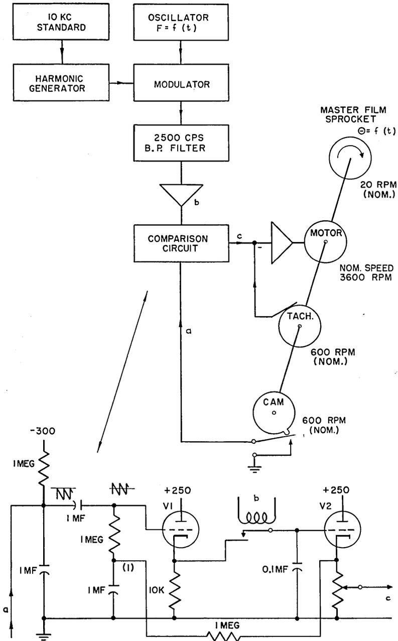
Fig. 10 — Block diagram of film scale calibrator with schematic of comparison circuit.
