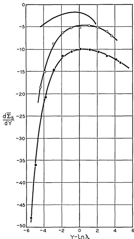
Fig. 6 — Differential charge in fast states versus surface potential. The graphs show  $(\partial\bar{\Sigma}_s/\partial Y)$  plotted against  $Y - \ln \lambda$ . Dots: p-type; circles: n-type. A typical result of Brown and Montgomery, using 28 ohm-cm p-type germanium, is also shown.
