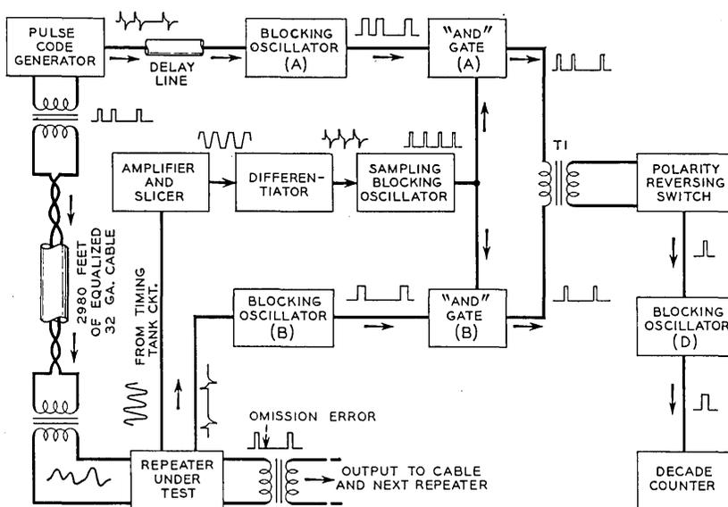
Fig. 7 — Block diagram of error detecting circuit.
