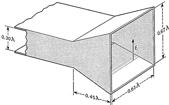
Fig. 6 — Feed horn dimensions.
