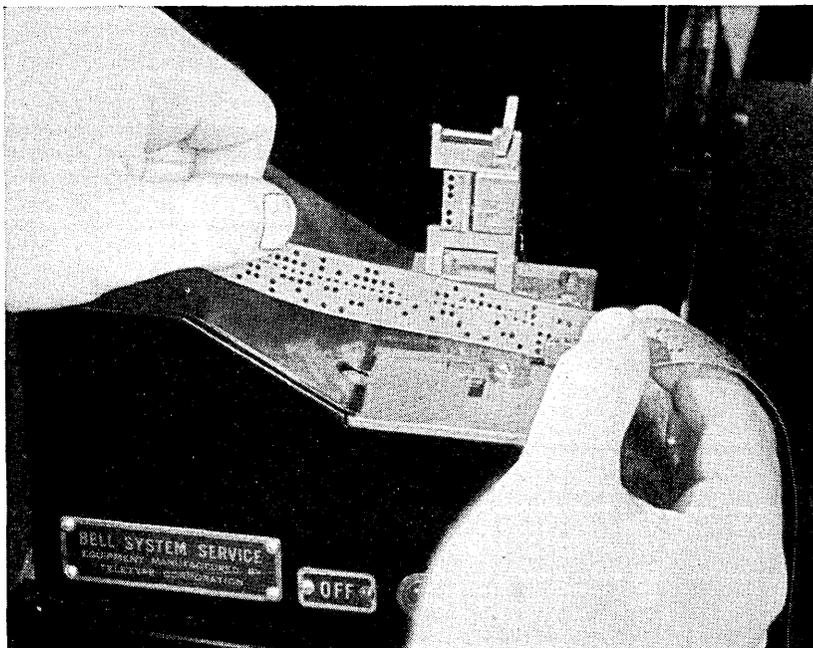
Fig. 15 — Perforated tape being inserted in reader.
