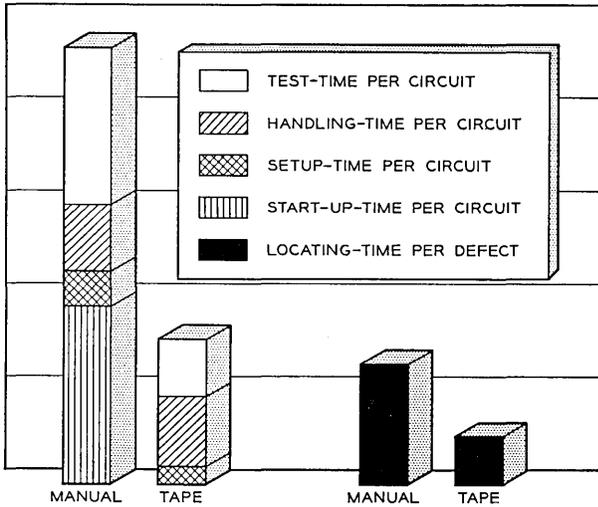
Fig. 16 — Comparison of manual and Tape-O-Matic test operation times.
