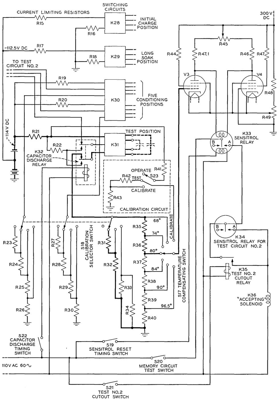
Fig. 12 — Simplified schematic of insulation resistance test circuits.
