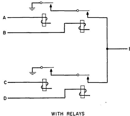
Fig. 25 — A logic function with relays.
