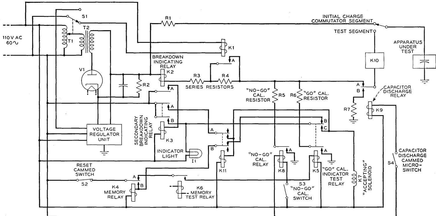
Fig. 7 — Simplified schematic of dielectric strength test circuits.
