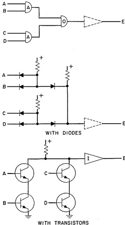
Fig. 26 — A logic function with diodes or transistors.
