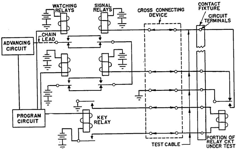
Fig. 3 — Simplified circuit sketch for automatic test operation.
