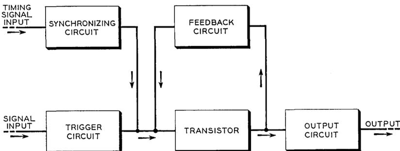
Fig. 2 — Regenerative amplifier block diagram.
