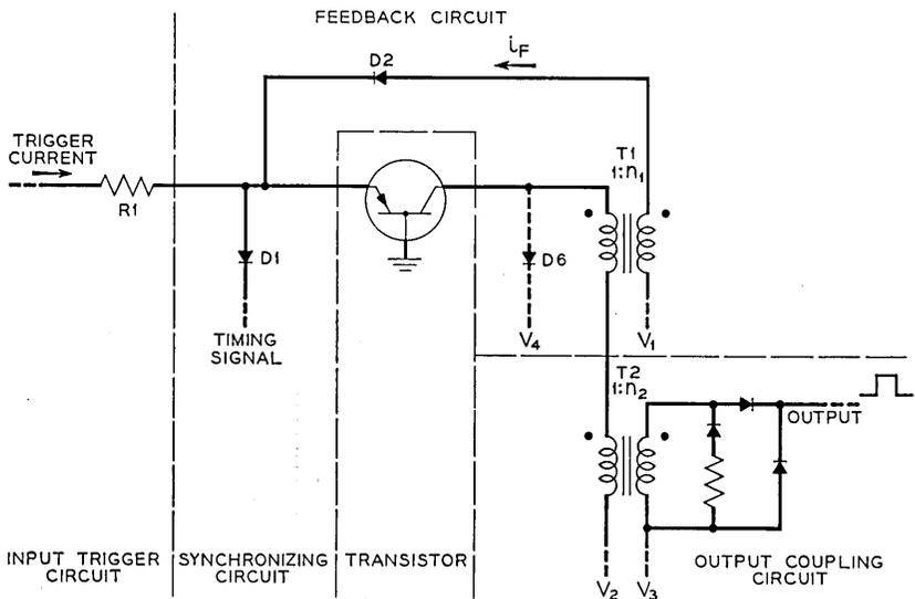
Fig. 12 — Series connection of output and feedback.
