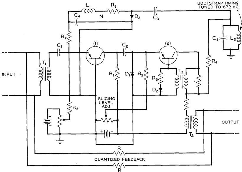
Fig. 3 — Circuit diagram of the regenerative repeater.
