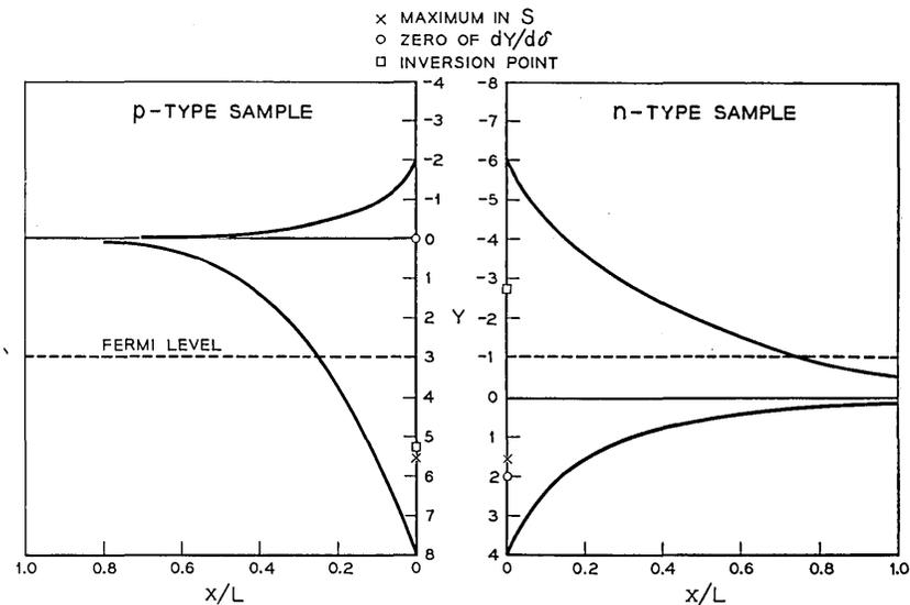
Fig. 10 — The shapes of the surface space-charge regions for the *p*-type and *n*-type samples in the extremes of gaseous environment. The two surfaces are to the center of the figure. The solid curves show the center of the gap (intrinsic Fermi level) plotted against distance, in units of an intrinsic Debye length. Also shown are the positions of the zeros of  $(dY/d\delta)$ , the maxima of  $s$ , and the minima of surface conductivity.
