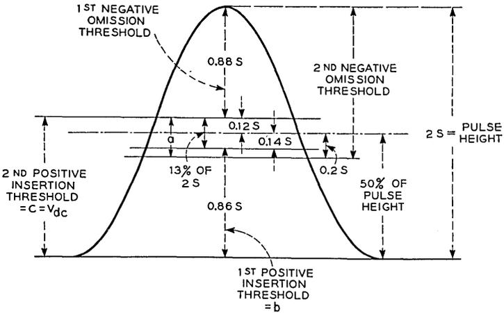
Fig. 12 — Bias levels used in calculating repeater errors.
