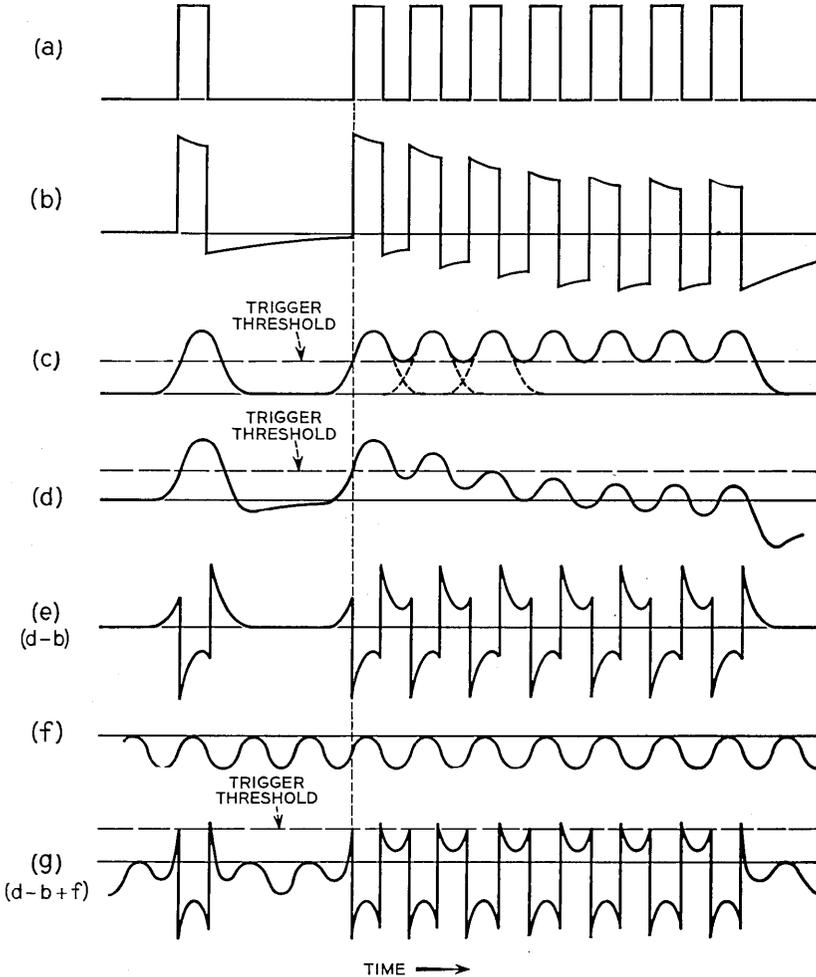
Fig. 1 — (a), a perfectly regenerated pulse train; (b) showing the effect of low-frequency cutoff; (c), showing (a) after passing over equalized line; (d), showing (b) after passing over equalized line; (e), effect of (d) minus (b); (f), inverted pedestal timing wave; (g), composite wave at input to repeater, namely, (d) minus (b) plus (f).
