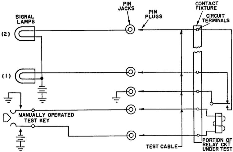
Fig. 2 — Simplified circuit sketch for manual test operation.
