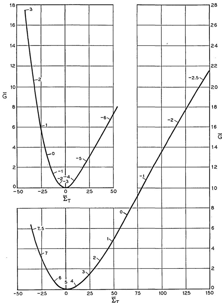
Fig. 5 — Curves showing  $\Delta \bar{G}$  (surface conductivity, in units of  $e\mu_p n_i \mathcal{L}$ ) and  $\bar{\Sigma}$  surface charge, in units of  $en_i \mathcal{L}$  for the 22.6 ohm-cm sample (upper curve) and for the 8.1 ohm-cm sample (lower curve). Values of  $Y$ , deduced from the surface conductivity, are indicated on the curves.
