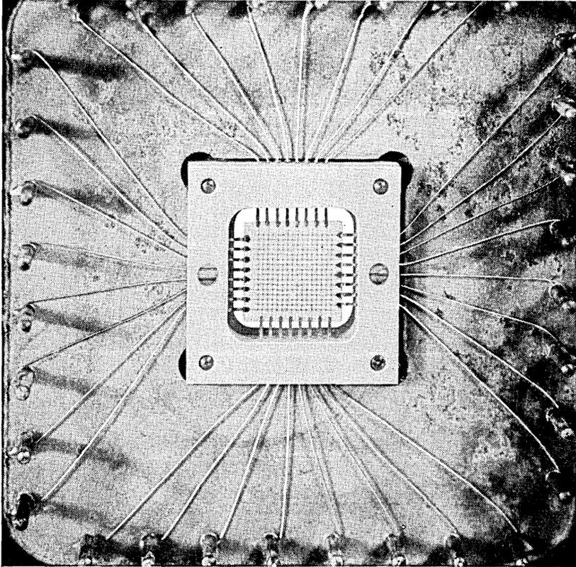
Fig. 20 — Ferroelectric array.
