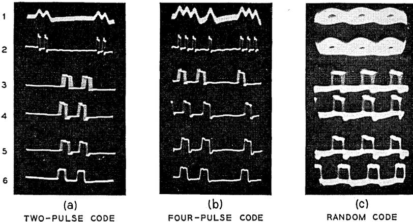
Plate III — (a), set code having 2 pulses out of possible 8; (b), set code having 4 pulses out of possible 8; (c), random code having an average of 4 pulses out of a possible 8.1 (a and b), input signal plus interference; 2 (a and b), regenerated output of 1; 3, expanded section of 2; 4, output of 2nd repeater; 5, output of 3rd repeater; 6, output of 4th repeater. 1(c), input signal alone; 2(c), input signal plus interference.
