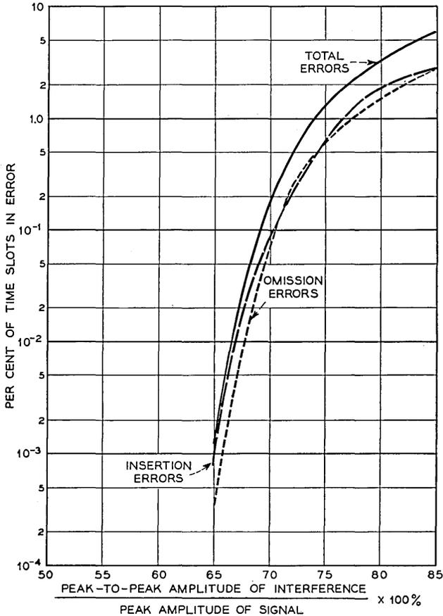
Fig. 13 — Repeater errors as a function of interferences level for sinusoidal interference.
