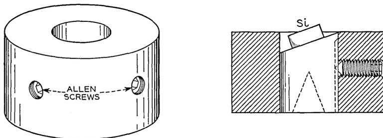
Fig. 1 — Jig for lapping a bevel.
