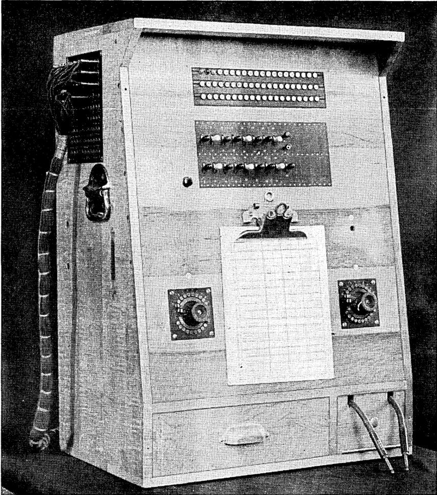
Fig. 1 — Manual wired unit test set.
