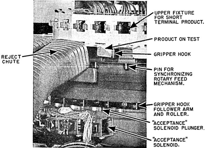
Fig. 3 — View of rejection and acceptance mechanisms.
