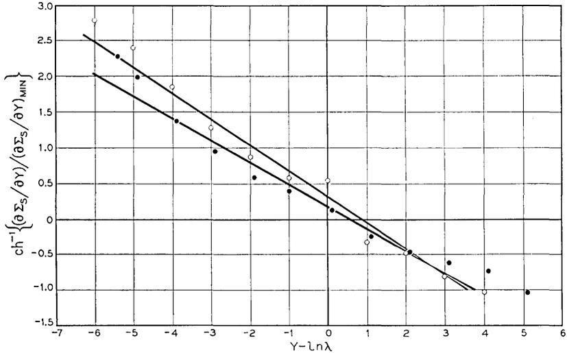
Fig. 1 — The fit between Equations (13) and (14) and the experimental data. The circles and dots give the experimental data for the *n* and *p*-type samples respectively and the solid straight lines represent Equations (13) and (14).
