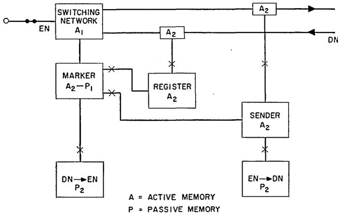
Fig. 11 — Memory in typical electromechanical switching system.
