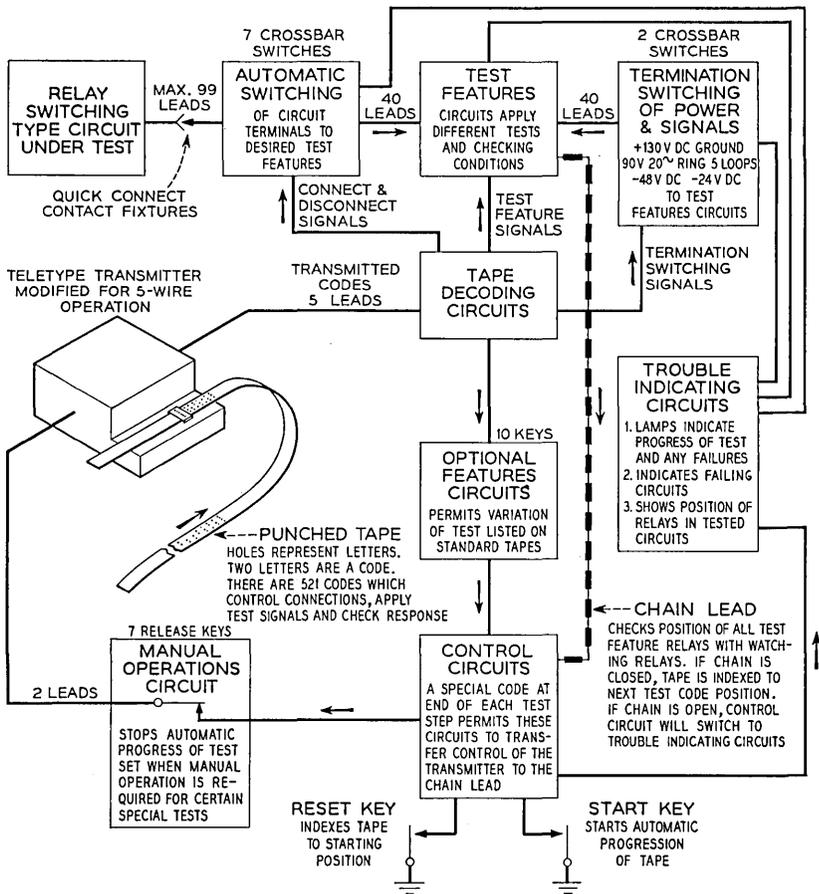
Fig. 13 — Block schematic.
