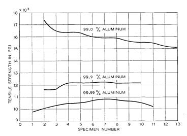
Fig. 19 — Tensile strength of extruded aluminum pipe.
