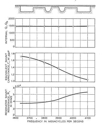
Fig. 9 — Variation of internal cavity parameters over the mechanical tuning range. Using a scaled-up brass model of the cavity shown in Fig. 6 (b), the curves for internal  $Q,\,Q_0$ , and for the equivalent gap capacitance, C, were determined experimentally by independent methods and the third curve calculated from the first two using the relation,  $R=Q_0/\omega C$ .
