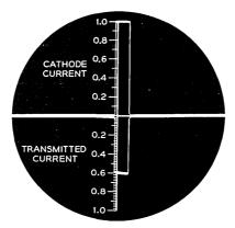
Fig. 5 — Oscilloscope display obtained with electron-gun-transmission test set. The special reticule permits the cathode current pulse to be adjusted for unit height; thus the height of the transmitted current pulse gives transmission efficiency directly.
