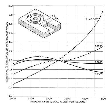
Fig. 8 — Variation in cavity loading (i.e., external Q) for various lengths, L, of the output transformer. The curve for L=0.860'' shows the least variation and was chosen for M1805 design. The above curves were obtained experimentally using scaled-up, 4,000-mc brass models.
