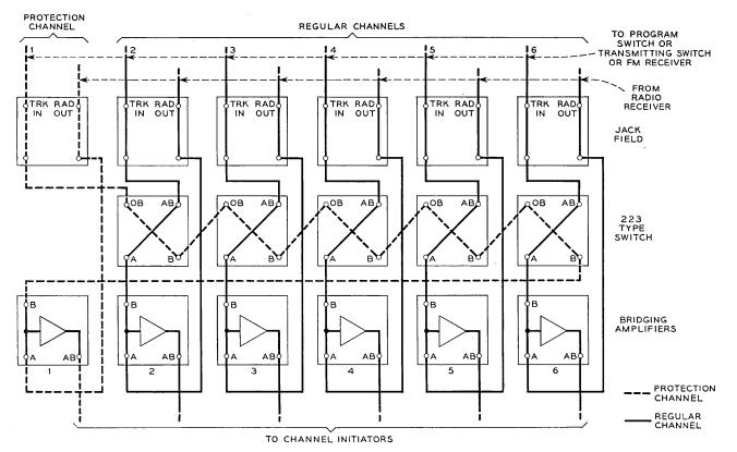
Fig. 9 — TD-2 automatic switching receiving switch.
