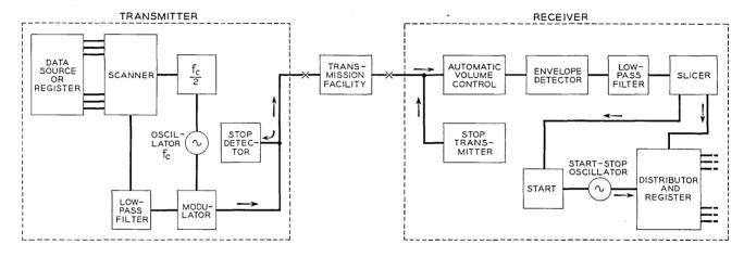
Fig. 5 — Block diagram of signaling system.
