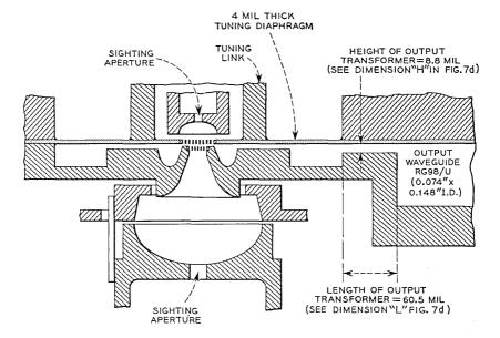
Fig. 17 — M1805, electrically significant contours. This drawing shows the interrelationship and the combination of the essential tube elements. More detailed data on these elements were contained in Fig. 4 for the gun, Fig. 6 for the passive circuit and Fig. 16 for the repeller.
