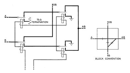
Fig. 7 — 223-type coaxial switch.
