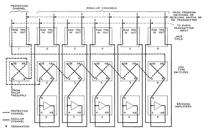
Fig. 8 — TD-2 auto switching t ransmitting switch.
