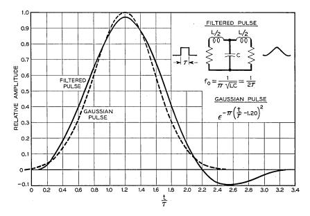
Fig. 4 — Filtered rectangular pulse and Gaussian pulse.
