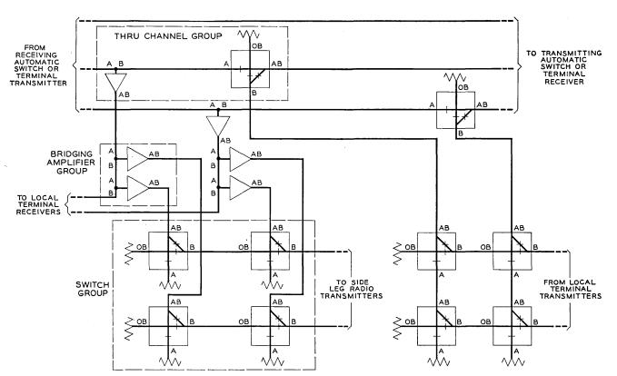
Fig. 19 — Example of program switching.
