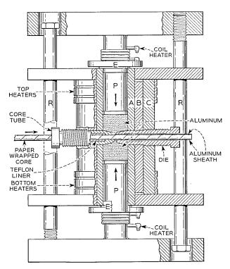
Fig. 5 — Diagram of experimental press assembly.
