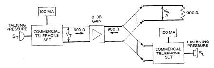
Fig. 2 — Additive property of transmission ratings. Transmitting rating:  $R_T = -20 \, \log_{10} \, V_T/S_T$ . Receiving rating:  $R_L = -20 \, \log_{10} \, (S_L/(V_W/2))$ . Since  $V_w/2 = V_T$ , over-all rating,  $R_0 = -20 \, \log_{10} \, S_L/S_T = R_T + R_L$ .
