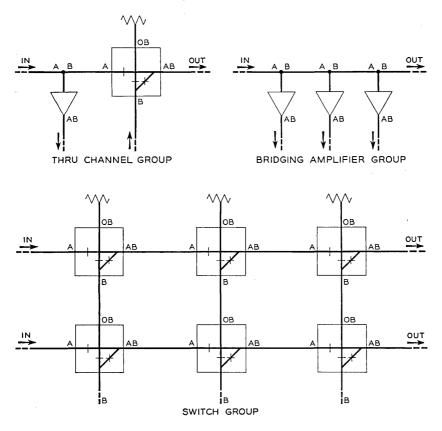
Fig. 18 — Basic circuits for program switching.
