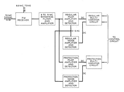
Fig. 12 — Simplified block schematic-protection initiator.
