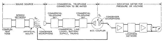
Fig. 4 — Measurement of over-all rating of a telephone connection.
