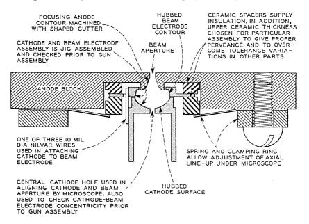
Fig. 2 — The demountable electron gun structure shown in this figure was originally used in an experimental study aimed at adapting the Heil gun for use in the MI805 millimeter wave reflex klystron. The reproducibility and mechanical stability, however, proved so satisfactory that this structure was incorporated in the final tube design essentially without change.
