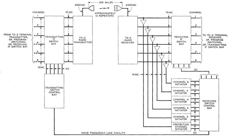
Fig. 4 — Automatic switching.
