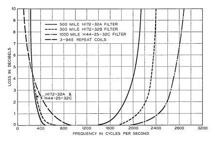
Fig. 1 — Transmission frequency characteristics of typical voice-frequency telephone circuits.
