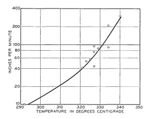
Fig. 12 — Effect of temperature on extrusion rate at constant pressure of  $65,000~\mathrm{psi}$ .
