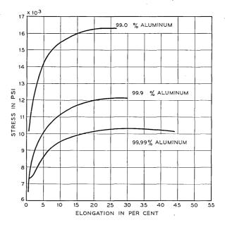
Fig. 20 — Stress-strain curves for extruded aluminum pipe.
