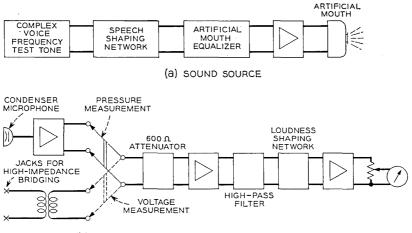
(b) INDICATING METER FOR PRESSURE OR VOLTAGE
