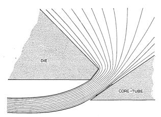
Fig. 11 — Schematic representation of flow of aluminum through a section of the extrusion orifice.
