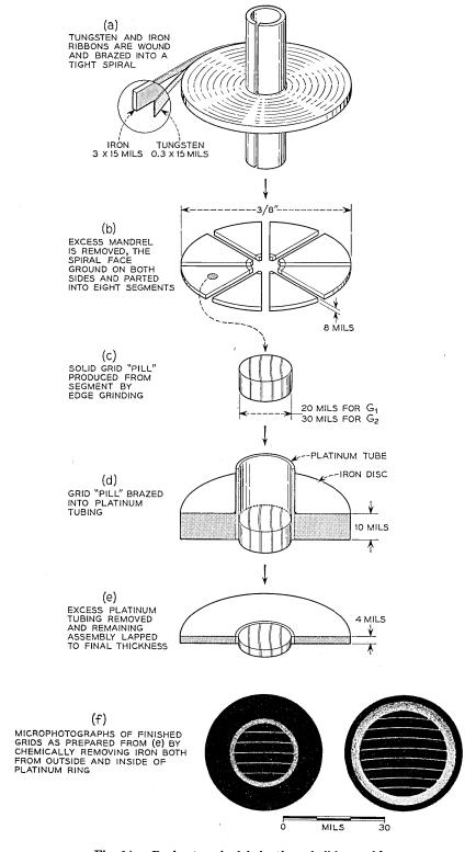
Fig. 14 — Basic steps in fabrication of ribbon grid.
