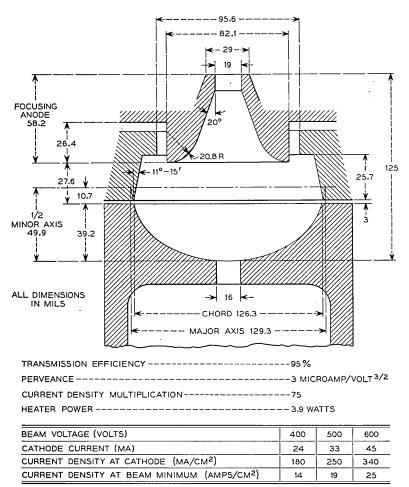
Fig. 4 — Modified Heil electron gun as used in M1805 millimeter wave reflex klystron. The performance data tabulated above, only apply to a unidirectional electron beam as produced in gun testers. Both perveance and cathode loading will be somewhat lower in an operating reflex klystron due to electrons returned into cathode region.
