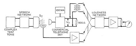
Fig. 5 — Measurement of transmitting rating of a telephone set.
