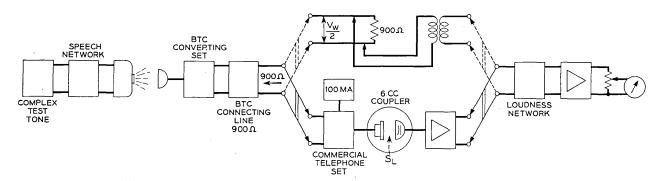
Fig. 6 — Measurement of receiving rating of a telephone set.
