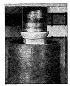
Fig. 25 — Start, middle, and end of shaving operation for removing outer surface of cast aluminum billets.
