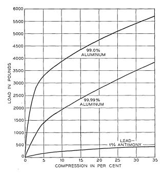
Fig. 1 — Compression tests at 265°C.
