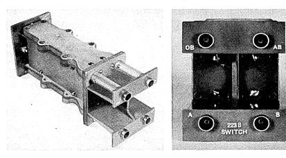
Fig. 6 — 223-type IF coaxial switch.
