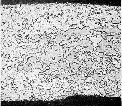
Fig. 23 — Transverse microsection of extruded aluminum sheath. Above, charge weld — line of demarcation is plainly visible. Below, charge weld — the new charge material appears darker because the grains have a different orientation. Both at  $150 \mathrm{x}$ .
