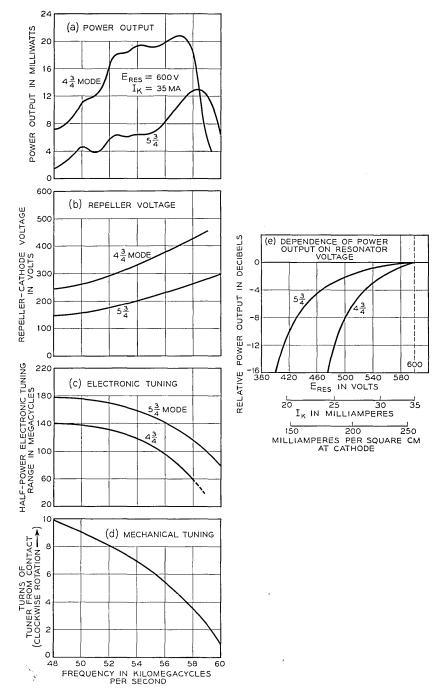
Fig. 20 — Typical M1805 performance characteristics.
