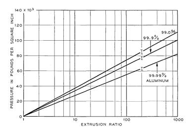
Fig. 27 — Effect of degree of reduction on extrusion pressure at constant speed.
