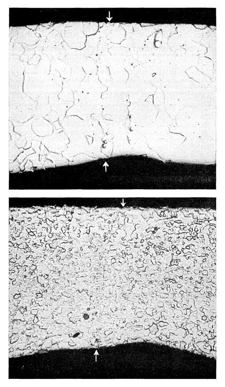
Fig. 22 — Transverse microsection of extruded 99.99 per cent aluminum sheath. Above, seam weld coarse grained material, and below, seam weld fine grained material, both at 150x.
