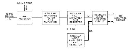
Fig. 11 — Simplified block schematic of regular initiator.
