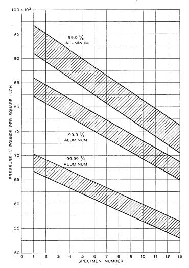
Fig. 14 — Effect of charge length and purity on extrusion pressure at constant rate.
