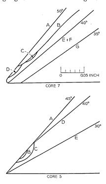
Fig. 8 — Longitudinal sections through upper tip of core-tubes at various stages of modification.
