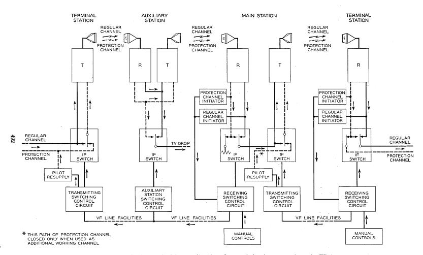
Fig. 13 — Control circuits required for one direction of transmission for two sections of a TD-2 system.
