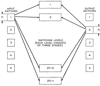
Fig. 4 — Five-stage switching array.
