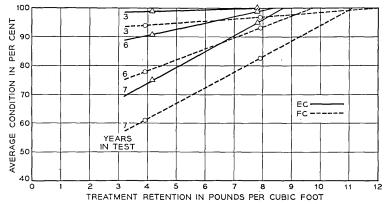
Fig. 26—Theoretical lines for estimating threshold retention for creosote No. 5285A; ¾-inch southern pine sapwood stakes.
