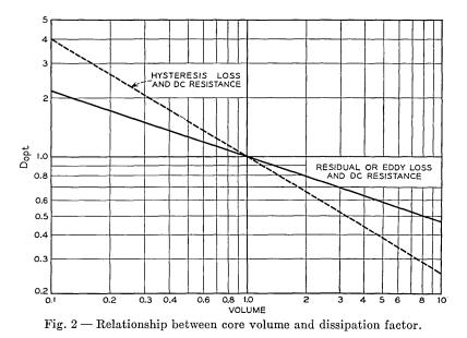
deviations from optimum up to about 20 per cent the penalty in dissipation is not severe, but beyond this point the dissipation factor increases rapidly.
