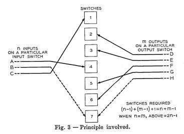
is made via levels, a level consisting of three intermediary switching stages. The number of levels required is  $(2N^{1/3} - 1)$ . Each level has  $N^{2/3}$  inputs and the same number of outputs. The number of crosspoints for a three-stage non-blocking array for  $N^{2/3}$  inputs and  $N^{2/3}$  outputs can be obtained from equation (2) by substituting  $N^{2/3}$  for N in that equation. The total number of crosspoints required for the five-stage array is:
