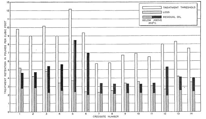
Fig. 34—Soil-block tests of fourteen creosotes against *Lentinus lepideus*; weathered southern pine sapwood blocks; comparison of treatment thresholds, losses during weathering and reconditioning, and gross characteristics of residual creosotes in terms of calculated amounts remaining of fractions above and below 355°C; based on Madison data. See Table XXXV.
