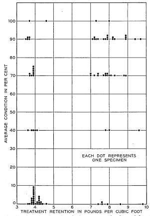
Fig. 18—Distribution of ratings in relation to retention by weight at treatment; creosote No. 5283, full-cell treatment (toluene dilution), seven years exposure.
