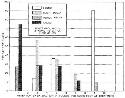
Fig. 28—The relation of creosote retention in lb/cu ft at treatment by toluene extraction, and the rated condition of pole-diameter test posts, by retention groups; 1950 inspection; Gulfport test plot. See text and Table XVI.
