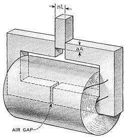
Fig. 9 — Inductance adjustment by constriction in magnetic cross section.
