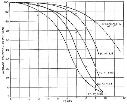
Fig. 19—Depreciation curves for ¾-inch southern pine sapwood stakes treated with creosote, BTL No. 5283, empty-cell and full-cell (toluene dilution) processes, and with greensalt K; Gulfport test plot. See text, Tables XII–XIII, and companion Figs. 20, 21 and 22.
