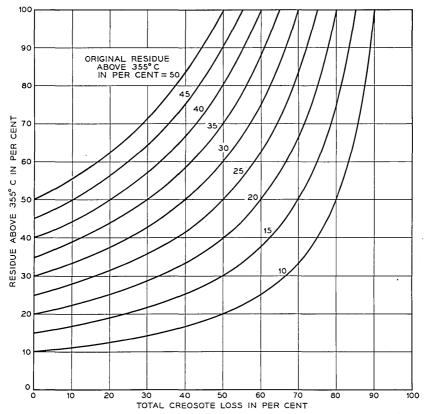
Fig. 31—Theoretical relation of the per cent increases in the residue above  $355^{\circ}$ C and the per cent losses of total creosote.
