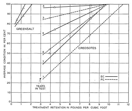
Fig. 23—Theoretical lines for estimating threshold retention for creosote No. 5283, in  $\frac{3}{4}$ -inch southern pine sapwood stakes, empty-cell and full-cell (toluene dilution) treatments, and for greensalt K; Gulfport test plot. See text, Tables XI and XIII, and companion Figs. 24, 25 and 26.
