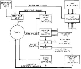
Fig. 11-Block diagram of the time system.
