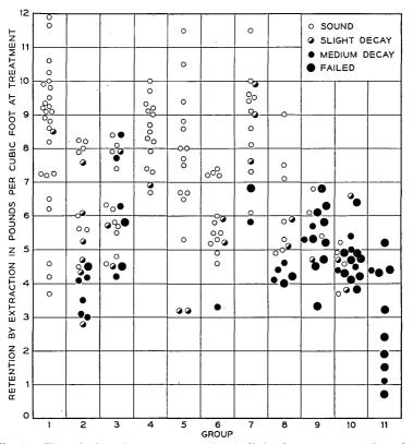
Fig. 27—The relation of creosote retention in lb/cu ft at treatment, by toluene extraction, and the rated condition of pole-diameter southern pine test posts, by post groups; 1950 inspection; Gulfport test plot. See text and Table XIV.
