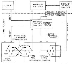
Fig. 12-Block diagram of marker progress circuits.
