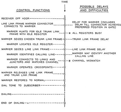
\* MARKER MUST TAKE ALTERNATIVE ACTION IF IT ENCOUNTERS THIS CONDITION Fig. 3—Establishing a dial tone call.
