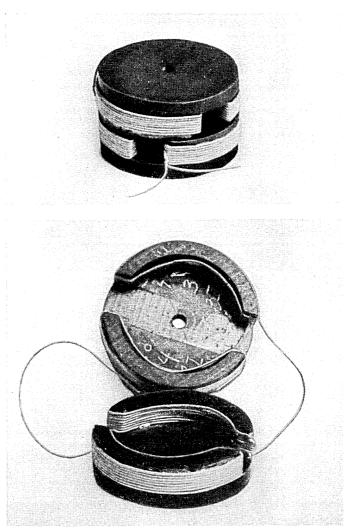
Fig. 14 — Magnetic variometer. Inductance adjustment by variation in mutual inductance.
