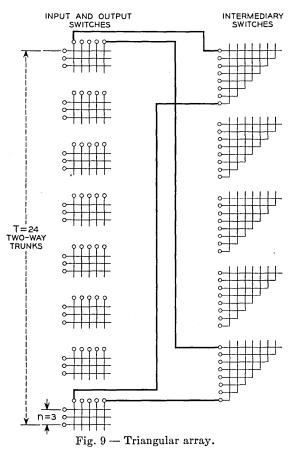
one-way outgoing and two-way trunks can be freely interconnected without blocking. The number of crosspoints for this case is:
