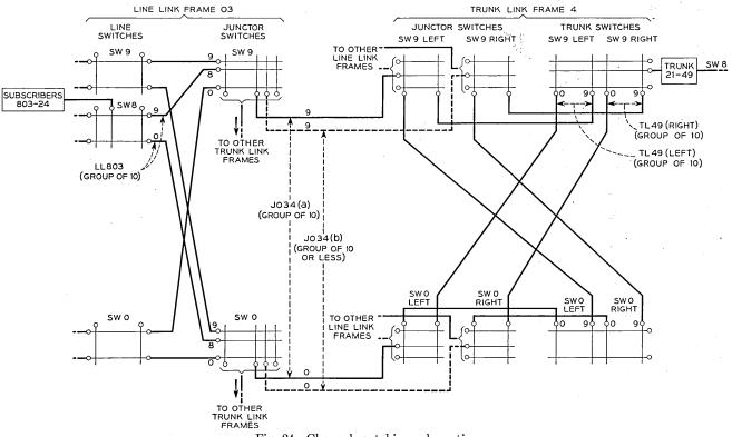
Fig. 24-Channel matching schematic.
