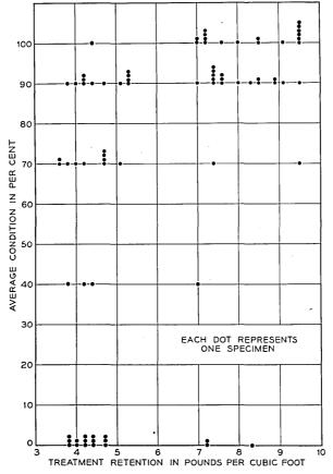
Fig. 16—Distribution of ratings in relation to retention by weight at treatment; creosote No. 5283, empty-cell treatment, seven years exposure.
