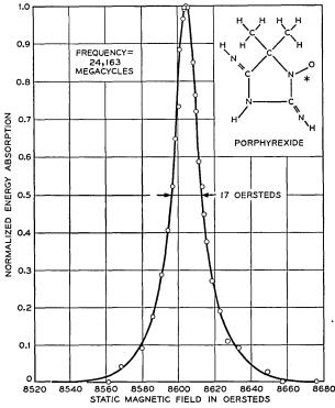
Fig. 2. — Electron resonance of porphyrexide. This is one of the strongest and sharpest peaks of electron-resonance yet observed. The g-value is  $2.0064 \pm 0.0002$ , which makes it slightly but significantly different from the ideal case. In the structural diagram, the asterisk signifies a three-electron bond. (A. N. Holden, W. A. Yaeger and F. R. Merritt).
