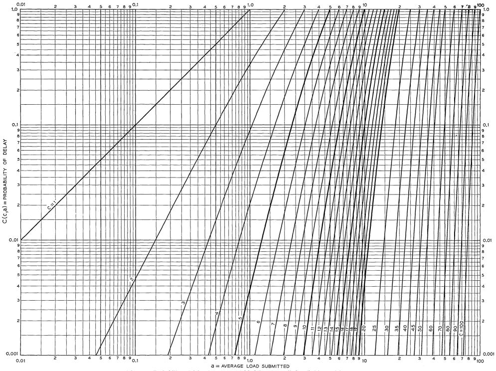
Fig. 21 — Probability of delay for exponential holding time calls handled in a "delayed" basis.
