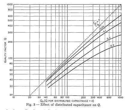
maintain small values of distributed capacitance. It will be necessary to increase the separation of windings from each other and from the core and this will result in a lower winding efficiency and a higher dc resistance.
