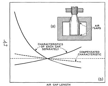
Fig. 12 — Inductance adjustment with partially compensating air gaps.
