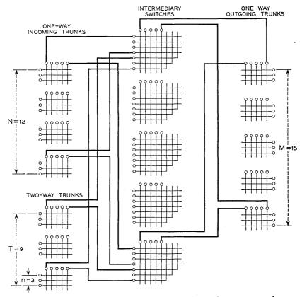
Fig. 10 — One-way incoming, one-way outgoing and two-way trunks.
