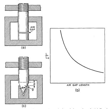
Fig. 11 — Inductance adjustment by variation of air gap length. (a) Gap formed by parallel plane surfaces. (b) Adjustment characteristic. (c) Cone or wedge shaped gaps.
