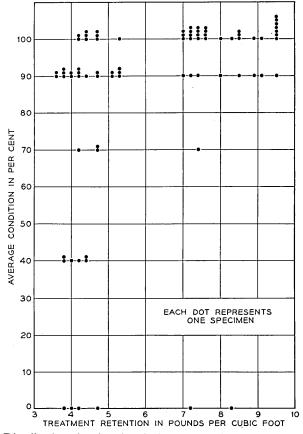
Fig. 15—Distribution of ratings in relation to retention by weight at treatment; creosote No. 5283,  $\frac{3}{4}$ -inch southern pine sapwood stakes; 1941 series, empty-cell treatment; six years exposure; Gulfport test plot. See text and companion Figs. 16, 17 and 18.
