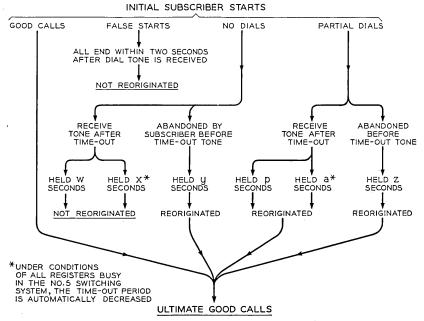
Fig. 6-Simplified characteristic action of subscribers in converting initial subscriber starts to ultimate good calls.
