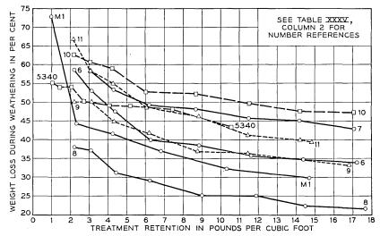
Fig. 33—Creosote losses in weathered,  $\frac{3}{4}$ -inch cubc, southern pine sapwood test blocks; relation of per cent loss of total creosote to original residue abovo 355°C and retention at treatment, lb/cu ft. All treatments were made with toluene creosote solutions. The total elapsed time from treatment to final reconditioned weight was about 105 days, including 60 days outdoor exposure on the Laboratory roof at Madison, Wis. See Table XXXV for number references.
