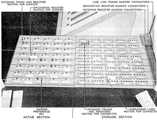
Fig. 18—The gate for control of marker connector preference.
