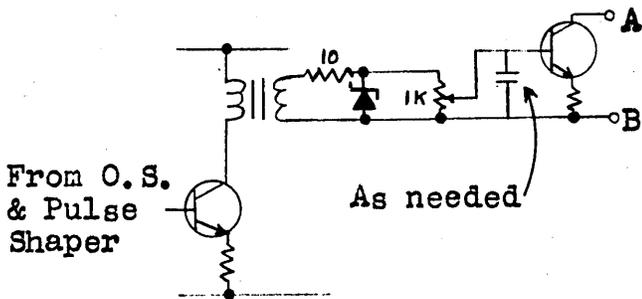
This circuit has the advantage that it can pass a constant current from either the positive or negative voltages. For positive, A goes to a positive voltage and B is the output. For negative, B goes to a negative and A is the output. Any number can be connected to the same output terminal.
