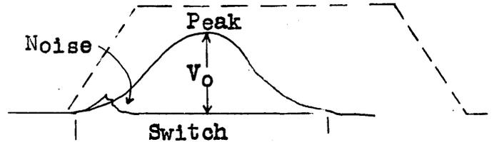
The value of current which, when increased, produces an output (first appearing at the noise position), is the value of the knee.
