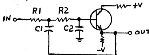
This is an active low-pass filter, so presumably it produces a pure delay below the cutoff frequency. However, a lot of sections would be needed if a good pulse shape is to be preserved.  $R_1C_1$  should be made equal to  $R_2C_2$ , and the  $C_1/C_2$  ratio is a critical parameter.
