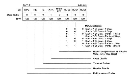
Figure 8. ASCI Control Register A (Ch. 1)
