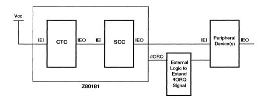
Figure 79. Peripheral Device as Part of the Daisy Chain
