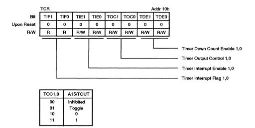
Figure 27. Timer Control Register
