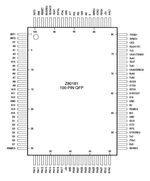
Figure 2. Z80181 Pin-out Assignment
