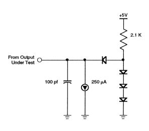
Figure 59. Standard Test Circuit
