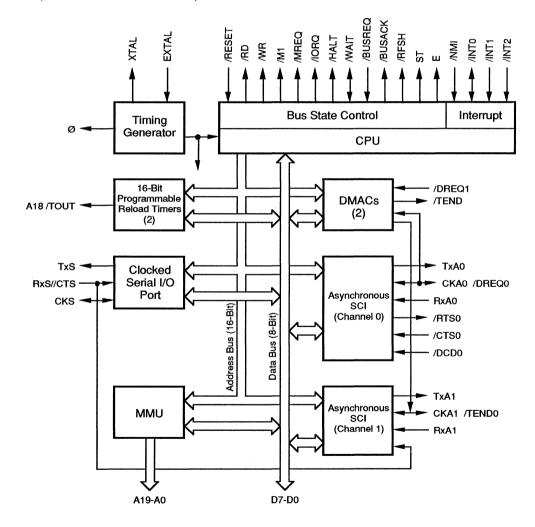
Figure 3. Z181 MPU Block Diagram
