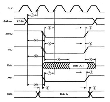
Figure 75. Read/Write External BUS Master Timing
