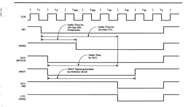
Figure 78. Interrupt Acknowledge Cycle Timing
