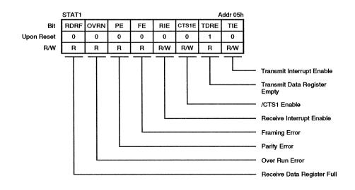
Figure 12. ASCI Status Register (Ch. 1)
