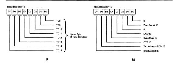
Figure 49. SCC Read Register Bit Functions (Continued)
