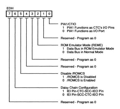
Figure 58. System Configuration Register
