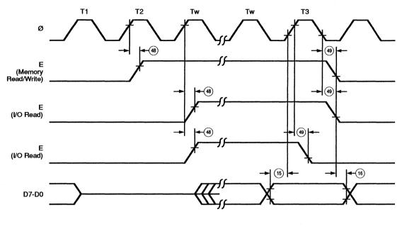
a) E Clock Timing (Memory Read/Write Cycle, I/O Read/Write Cycle)
