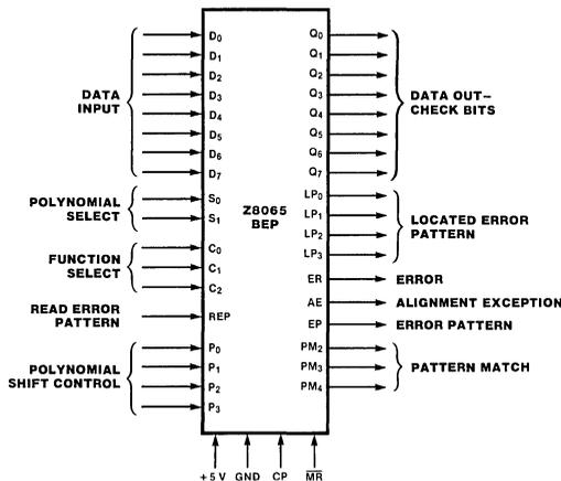
Figure 1. Pin Functions
