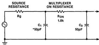
$$\text{MULTIPLEXER TIME CONSTANT} = (R_g + R_{on}) C_2$$
