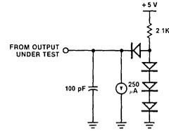
All ac parameters assume a load capacitance of 100 pF max, except for parameter 6 (50 pF max). Timing references between two output signals assume a load difference of 50 pF max.
