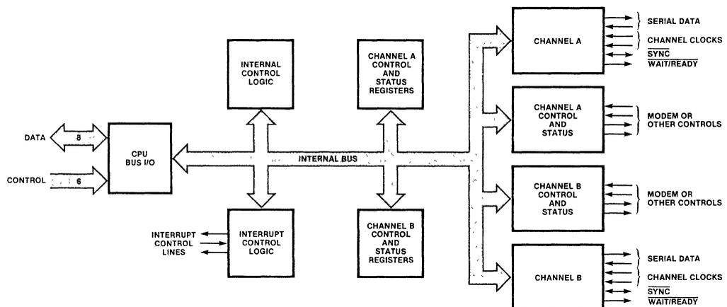
Figure 7. Block Diagram
