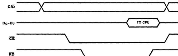
Figure 9. Non-Z-BUS Read Cycle Timing
