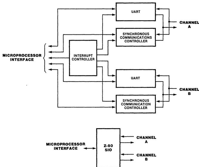
Figure 8. Conventional Devices Replaced by the Z-80 SIO
