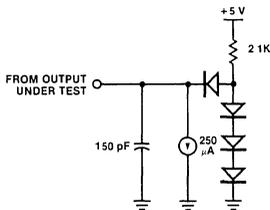
Figure 15. Test Load 1
