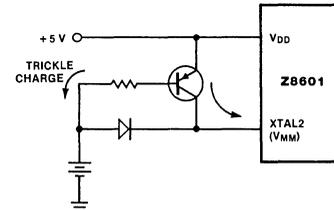
Figure 10. Recommended Driver Circuit for Power Down Operation
