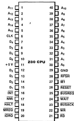
Figure 2. Pin Assignments
