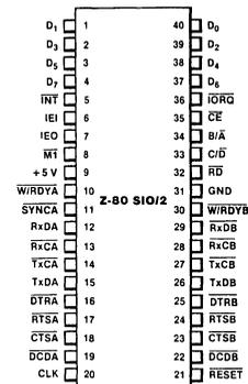
Figure 2. Z-80 SIO/2 Pin Assignments
