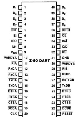
Figure 2. Pin Assignments
