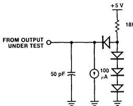
Figure 16. Test Load 2
