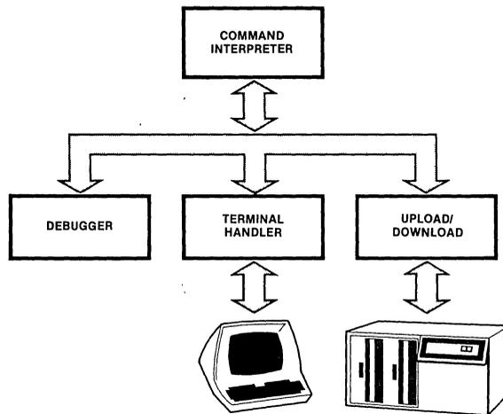
Figure 1. Monitor Block Diagram
