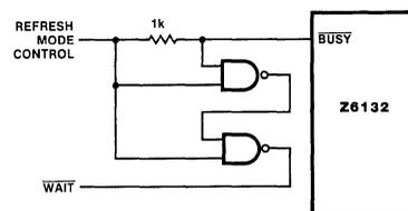
Figure 4. External  $\overline{\text{WAIT}}$  Generation
