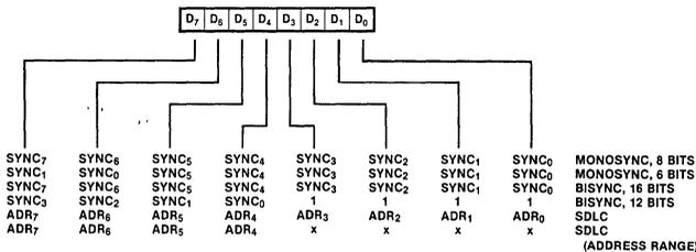
Figure 11. Write Register Bit Functions
