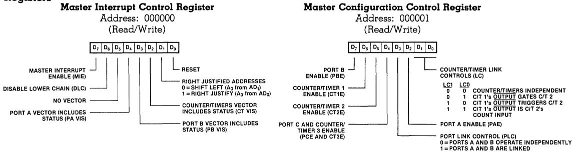
Figure 11. Master Control Registers
