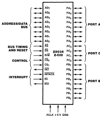
Figure 1. Pin Functions
