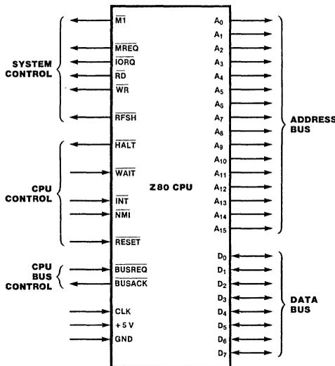
Figure 1. Pin Functions
