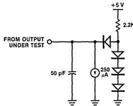
Figure 18. Test Load 1
