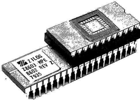
Figure 12. The Z8613 Microcomputer Protopack Emulator
