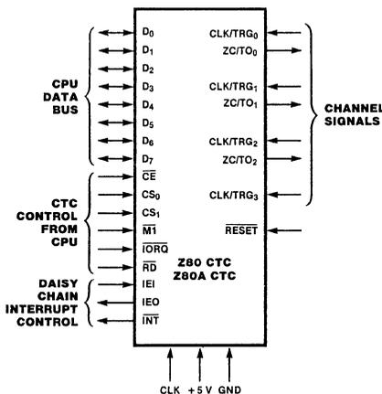
Figure 1. Pin Functions
