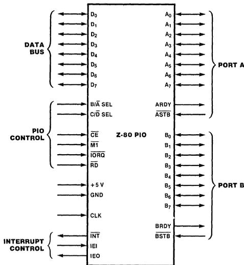
Figure 1. Pin Functions
