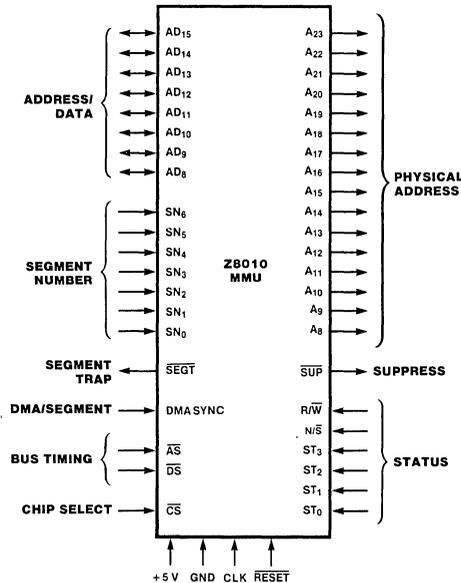
Figure 1. Pin Functions
