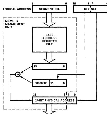
**Figure 6. Logical-to-Physical Address Transformation**
