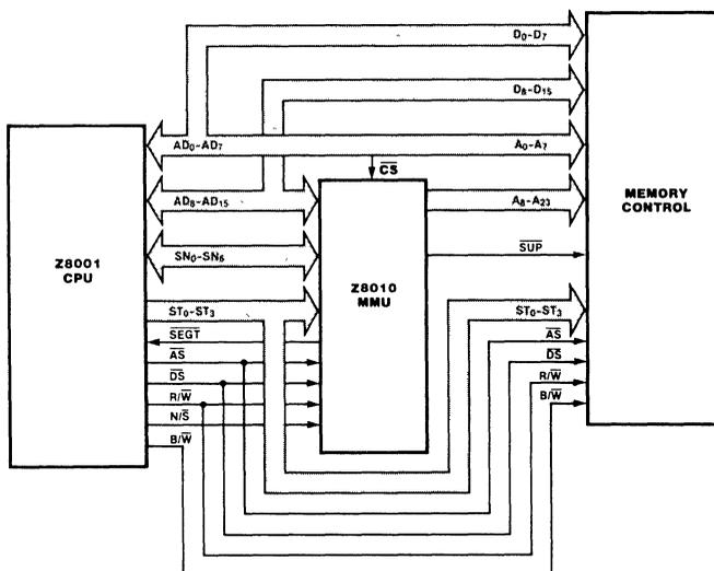
Figure 13. The MMU in a Z8001 System
