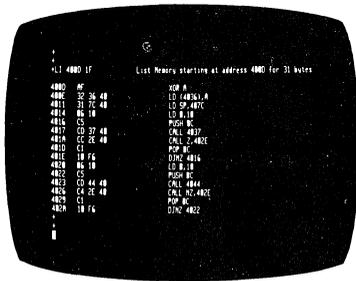
**Disassembly Capability.** User memory, system memory, and the trace memory of the development system may be displayed in the hexadecimal or disassembled format. In disassembled format,
