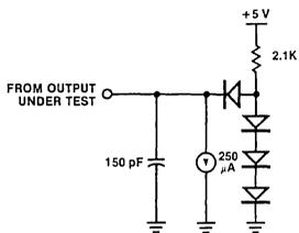
Figure 15. Test Load 1
