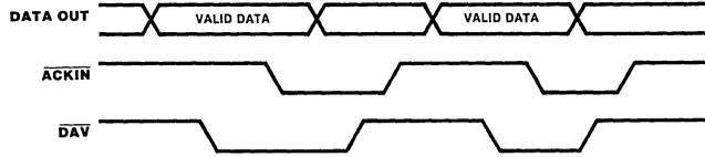
Figure 22. Interlocked Handshake Timing (Output) Port 2 Side Only
