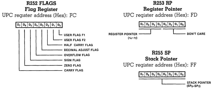
Figure 15. UPC Control Registers
