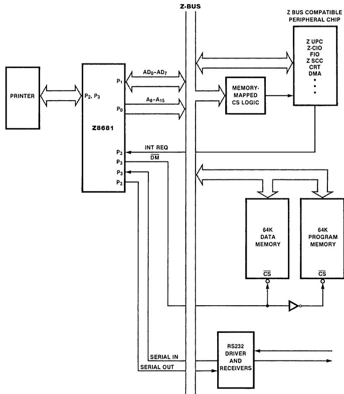
Figure 4. Z8681 Interfacing to External Memory
