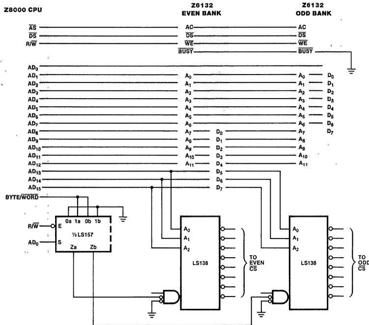
Figure 6. Connection Diagram
