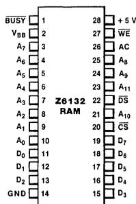
Figure 2. Pin Assignments
