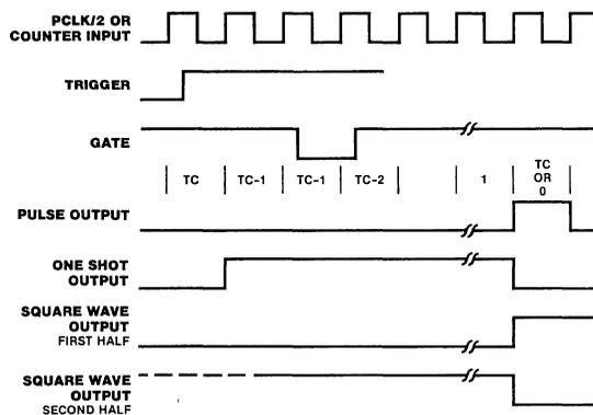
**Figure 10. Counter/Timer Waveforms**
