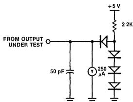
Figure 22. Standard Test Load
