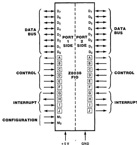
Figure 1. Pin Functions
