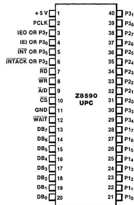
Figure 2. Z8590 UPC Pin Assignments
