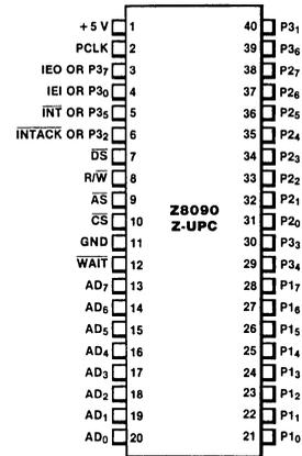
Figure 2. Z8090 Z-UPC Pin Assignments
