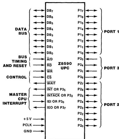
Figure 1. Z8590 UPC Pin Functions
