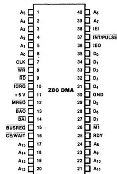
Figure 2. Pin Assignments
