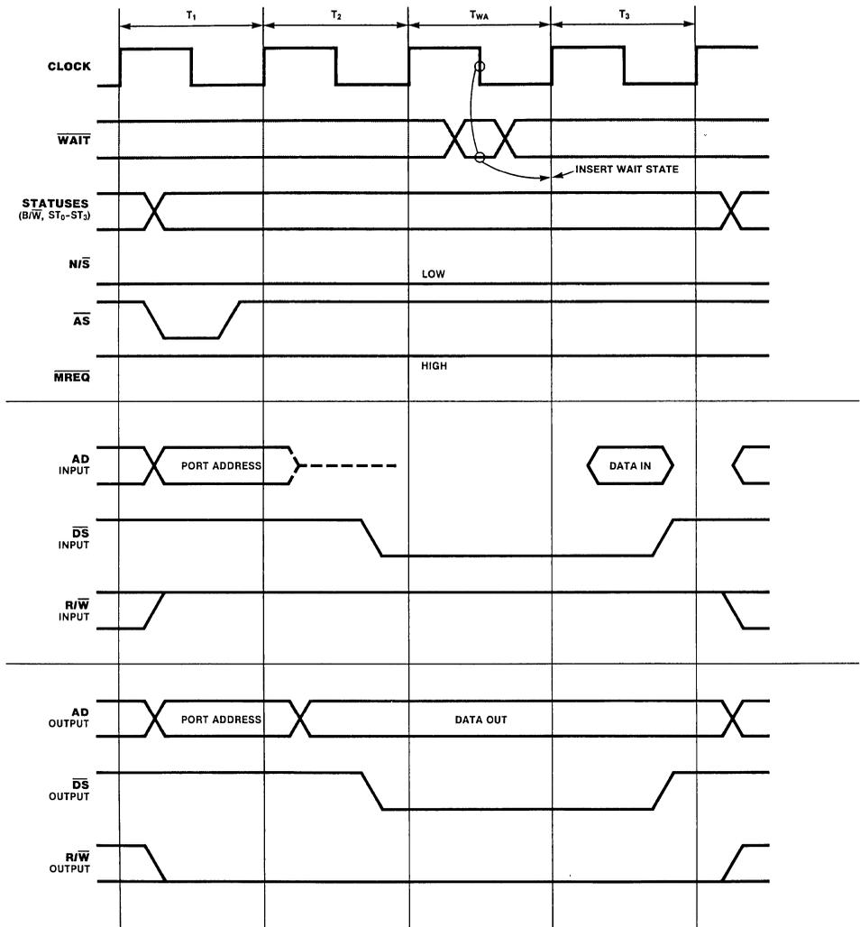
Figure 13. Input/Output Timing
