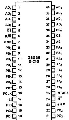
Figure 2. Pin Assignments
