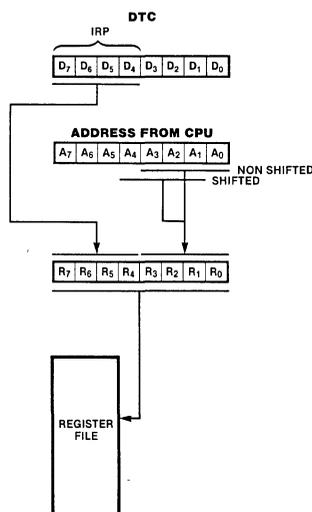
Figure 7. DSC Register Addressing Scheme
