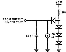
Figure 19. Test Load 2
