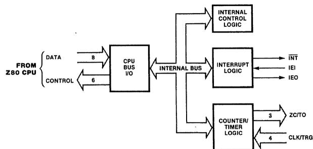
Figure 3. Functional Block Diagram
