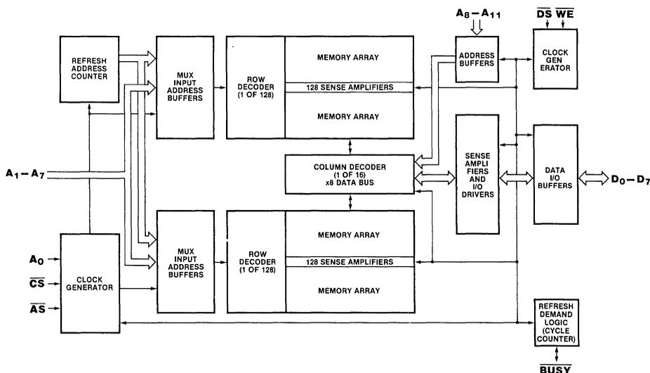
Figure 3. Z6132 Block Diagram
