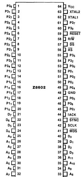
Figure 11. Z8602 Pin Assignments
