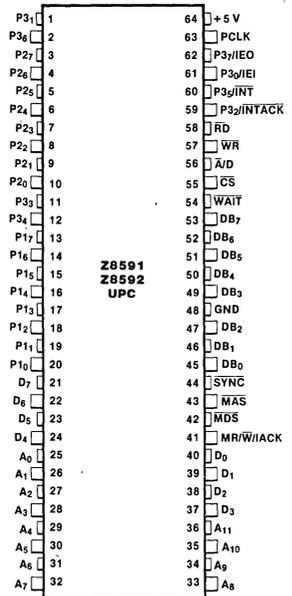
Figure 10. Z8591/Z8592 UPC Pin Assignments
