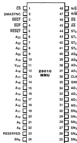
Figure 2. Pin Assignments
