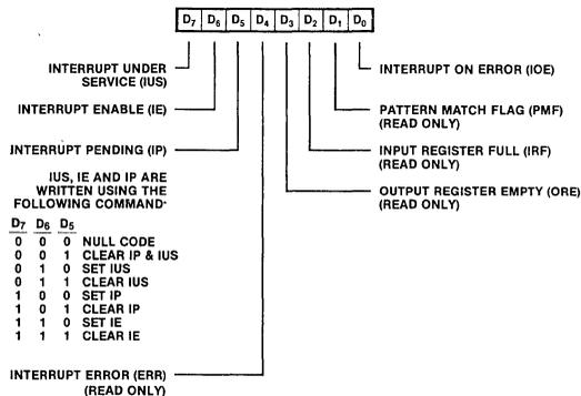
Figure 13. Port Specification Registers
