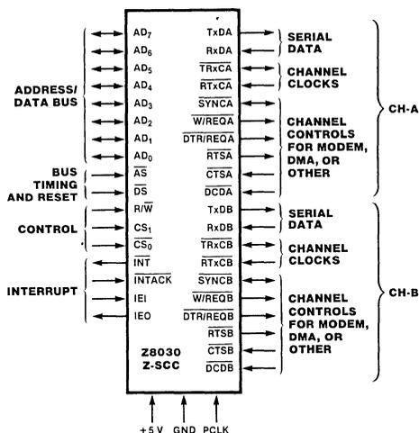
Figure 1. Pin Functions
