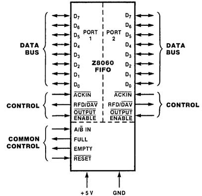
Figure 1. Pin Functions
