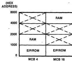
**Figure 1. Memory Addressing for MCB/4 and MCB/16**
