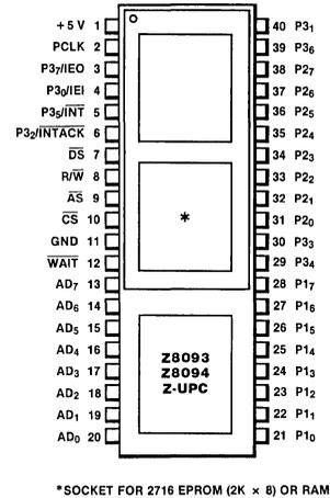
Figure 11. Z8093/Z8094 Prototack Pin Assignments
