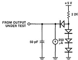
Figure 18. Test Load 1
