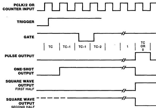
**Figure 10. Counter/Timer Waveforms**
