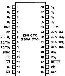
Figure 2. Pin Assignments
