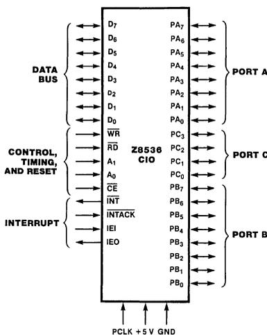
Figure 1. Pin Functions
