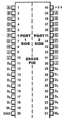
Figure 2. Pin Assignments
