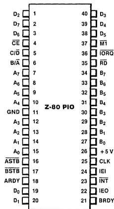
Figure 2. Pin Assignments
