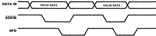
Figure 21. Interlocked Handshake Timing (Input) Port 2 Side Only
