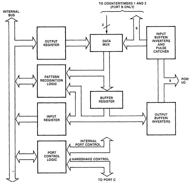
Figure 4. Ports A and B Block Diagram
