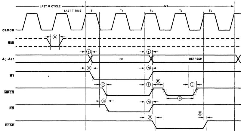
\* Although  $\overline{\text{NMI}}$  is an asynchronous input, to guarantee its being recognized on the following machine cycle,  $\overline{\text{NMI}}$ 's falling edge
