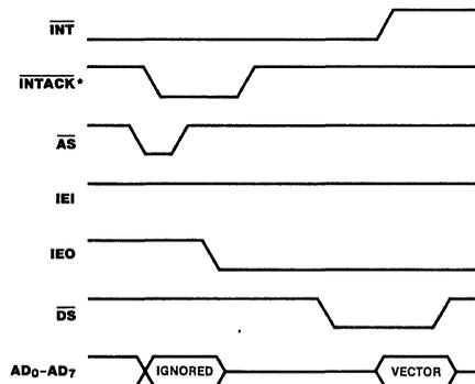
\* $\overline{INTACK}$  is decoded from Z8000 status.
