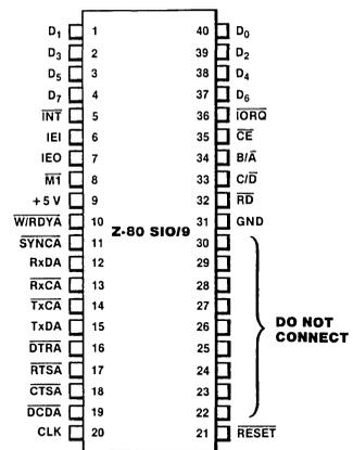
Figure 2. Z-80 SIO/9 Pin Assignments
