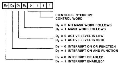
\*NOTE THE PORT IS NOT ENABLED UNTIL THE INTERRUPT ENABLE IS FOLLOWED BY AN ACTIVE MI
