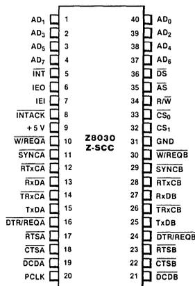
Figure 2. Pin Assignments
