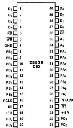
Figure 2. Pin Assignments
