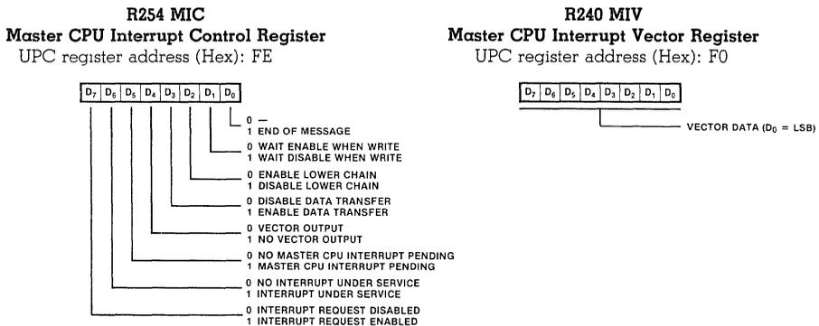
Figure 14. Master CPU Interrupt Registers
