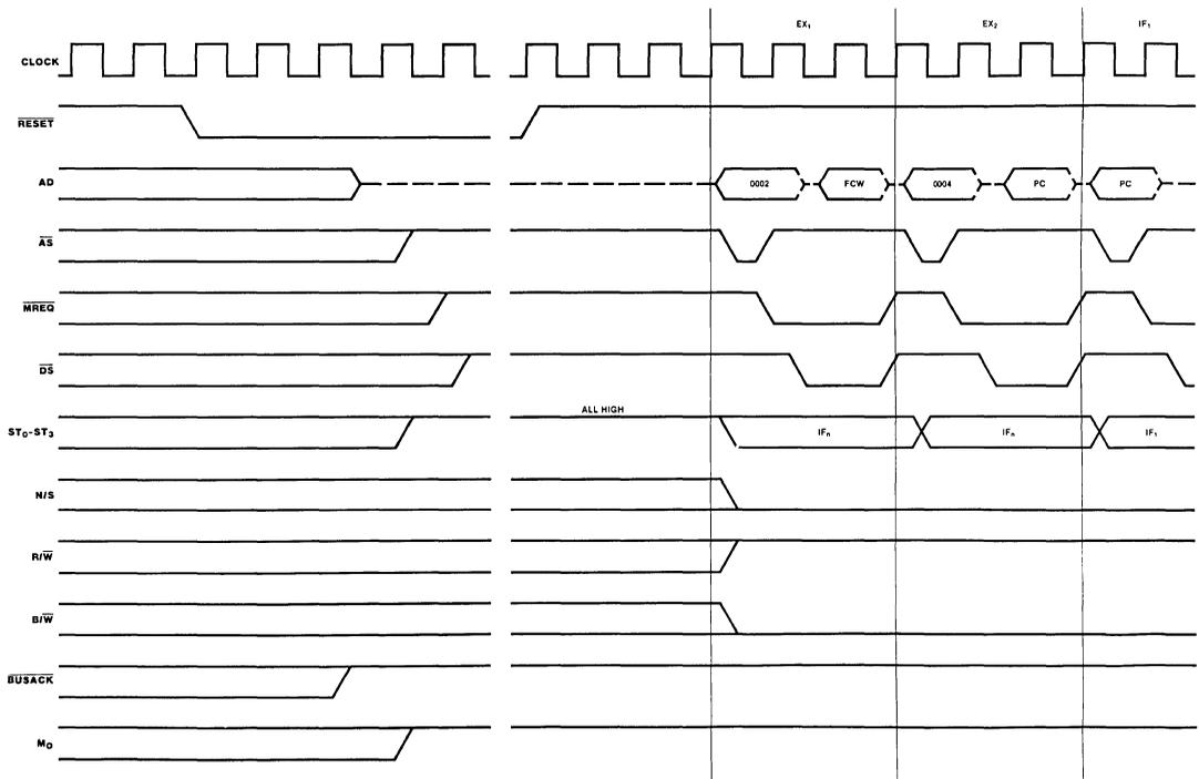
Figure 19. Reset Timing
