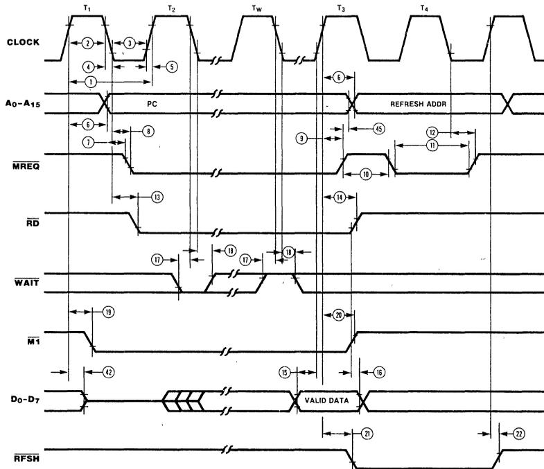
NOTE:  $T_w$ —Wait cycle added when necessary for slow ancillary devices
