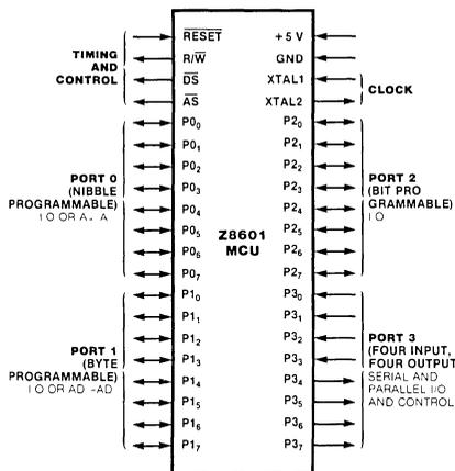
Figure 1. Z8601 MCU Pin Functions
