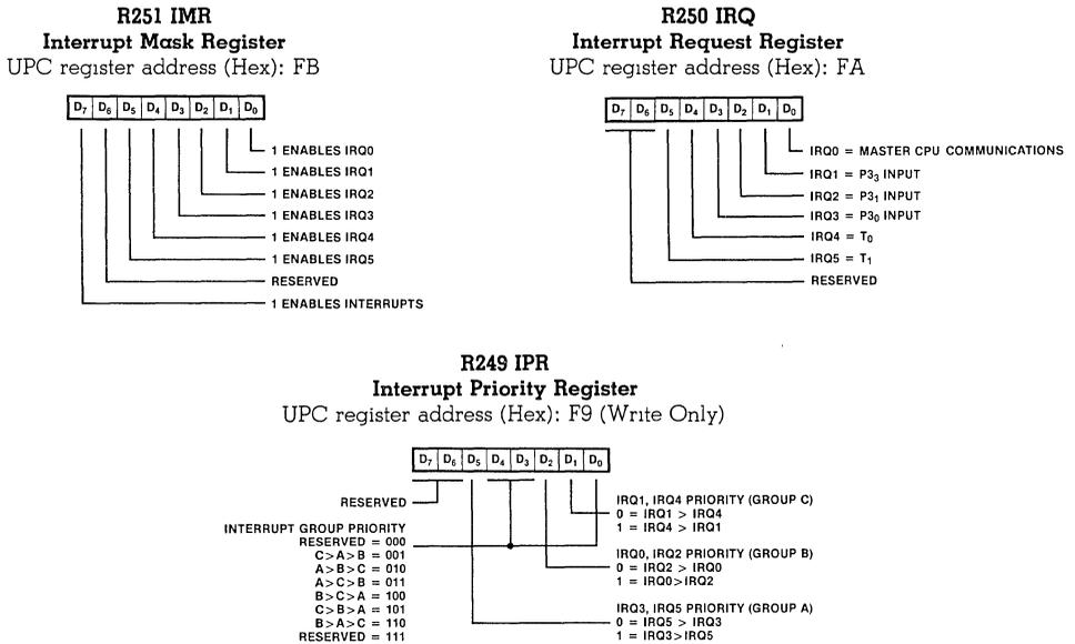
Figure 13. Interrupt Control Registers
