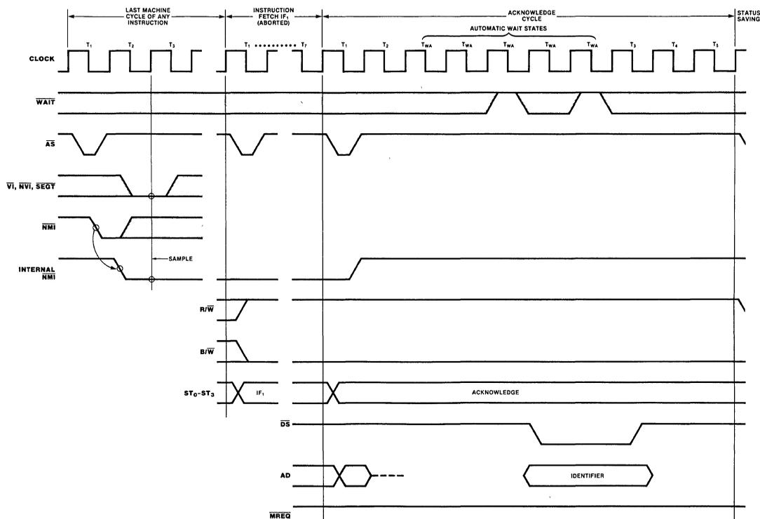
Figure 14. Interrupt and Segment Trap Request/Acknowledge Timing
