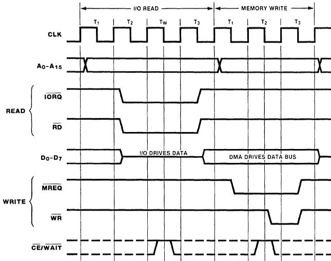
Figure 13. I/O-to-Memory Transfer
