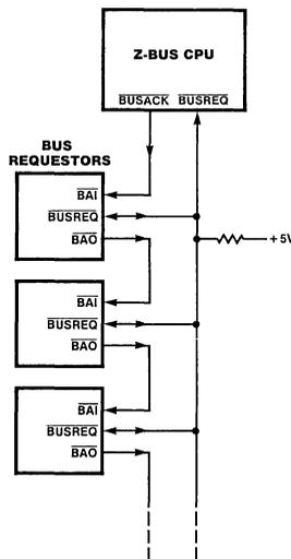
Figure 6. Bus Request Connections
