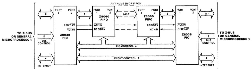
Figure 2. Using FIFOs to Extend FIOs
