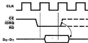
Figure 11. CPU-to-DMA Read Cycle
