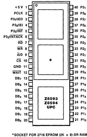
Figure 11. Z8593/Z8594 UPC Prototack Pin Assignments
