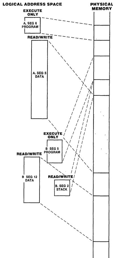
Figure 2. Mapping Logical Segments to Physical Memory
