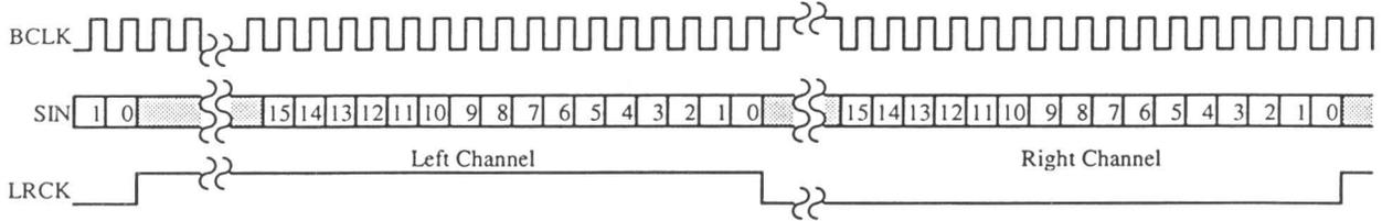
Fig.6-1 Conventional DAC Interface Format for OPL4-ML
