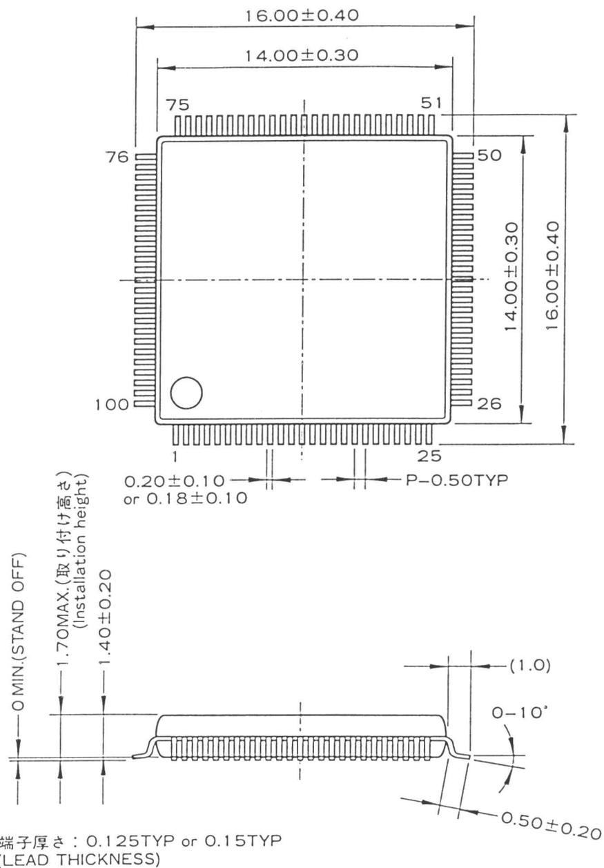
The shape of the molded corner may slightly different from the shape in this diagram.
