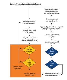
Figure 3 - Demonstration system upgrade process.
