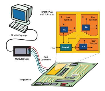
Figure 1 - Integrated Logic Analyzer (ILA) block diagram.
