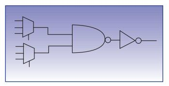
Figure 1 - CoolRunner Fast Zero Power AND gate.
