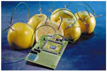
Figure 2 - The CoolRunner XPLA3 Development Kit uses only 60 µa (powered here by six grapefruit).
