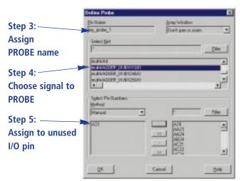
Figure 2 - Assigning signals to probes.
