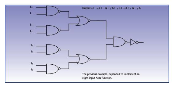
Figure 3 - Expanding the number of inputs.
