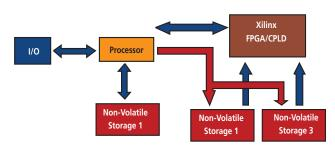
Figure 4 - Basic system architecture.
