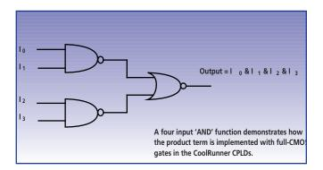
Figure 2 - Representation of a 4-input product-term using the CoolRunner FZP design technique.
