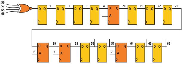
Figure 6 - Example of an LFSR counter.
