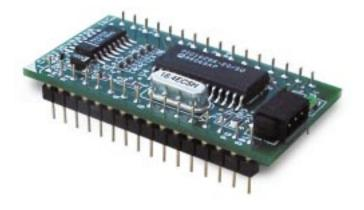
Figure 1 - Configurator 32-pin DIP module.
