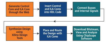
Figure 2 - ChipScope ILA flow.
