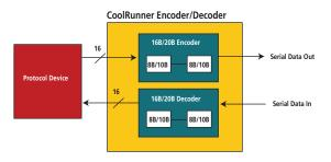
Figure 1 - 16B/20B block diagram.
