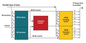
Figure 2 - 8B/10B encoder logic block diagram.
