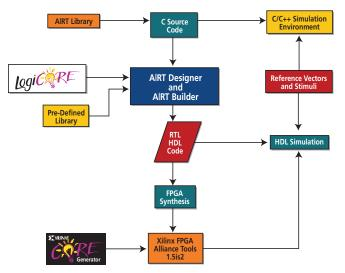
Figure 1 - AIRT design flow.
