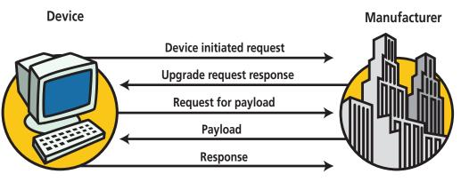
Figure 1 - The remote upgrade process.
