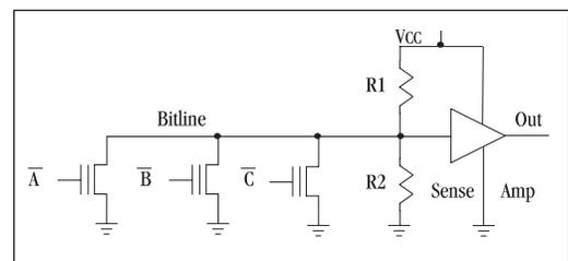
Figure 2: Simplified CPLD Programmable Structure
