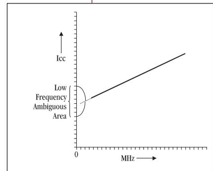
*Figure 5: I<sub>cc</sub> VS Frequency*
