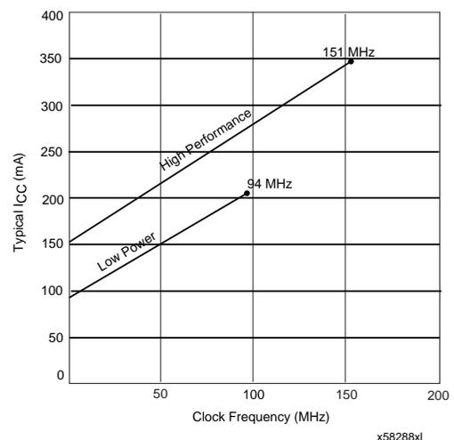
Figure 1: Typical  $I_{CC}$  vs. Frequency for XC95288XL
