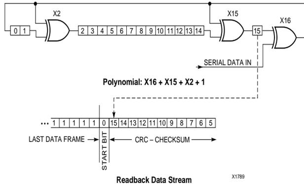
Figure 46: Circuit for Generating CRC-16
