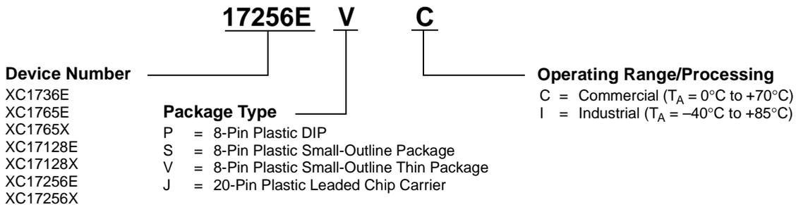
**Note:** When marking the device number on the EL parts, an X is used in place of an EL.
