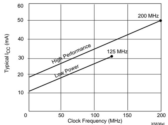
Figure 1: Typical  $I_{CC}$  vs. Frequency for XC9536XL
