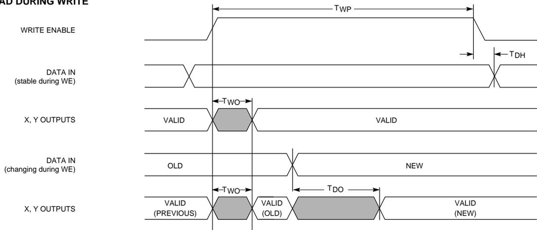
**READ DURING WRITE, CLOCKING DATA INTO FLIP-FLOP**
