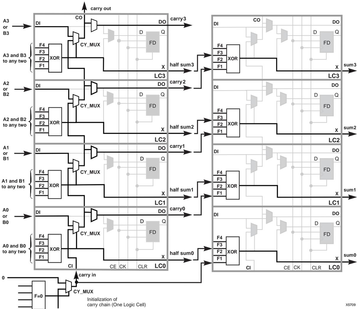
Figure 6: XC5200 CY\_MUX Used for Adder Carry Propagate
