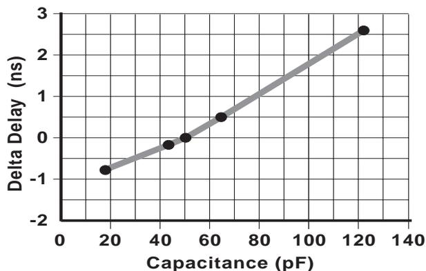
Figure 1: Delay Factor at Various Capacitive Loads X8257
