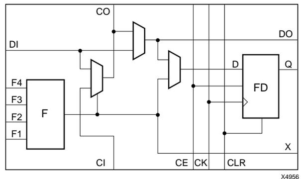
Figure 3: XC5200 Logic Cell (Four LCs per CLB)
