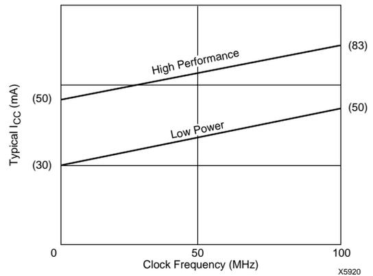
Figure 1: Typical  $I_{CC}$  vs. Frequency For XC9536
