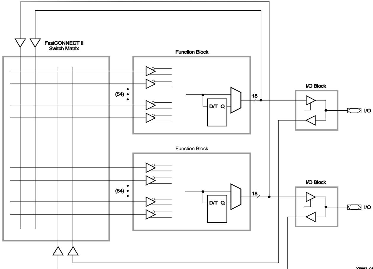
Figure 9: FastCONNECT Switch Matrix
