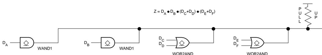
**Figure 22: Open-Drain Buffers Implement a Wired-AND Function**
