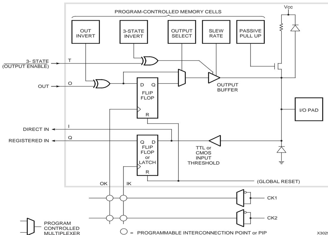
**Figure 4: Input/Output Block.**
