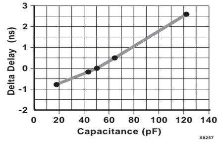
**Figure 32: Delay Factor at Various Capacitive Loads**
