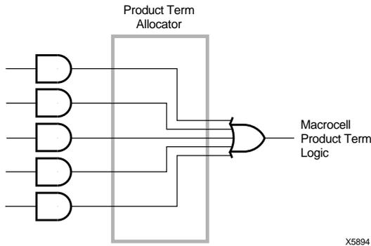
**Figure 5: Macrocell Logic Using Direct Product Term**
