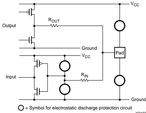
Figure 3: Input/Output Protection Circuitry
