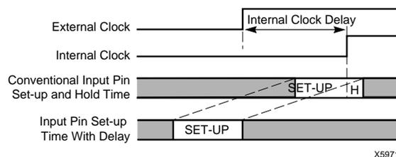
Figure 1: Set-up and Hold Times
