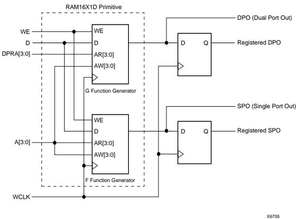
Figure 7: XC4000 Series Dual-Port RAM, Simple Model
