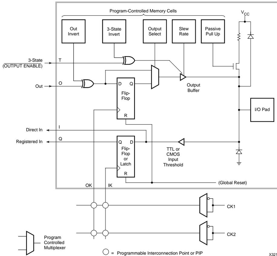
Figure 3: Input/Output Block (IOB)
