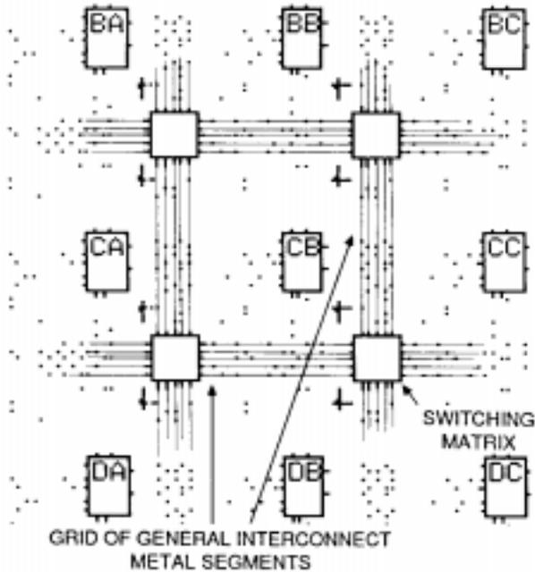
**Figure 10: FPGA General-Purpose Interconnect.**
