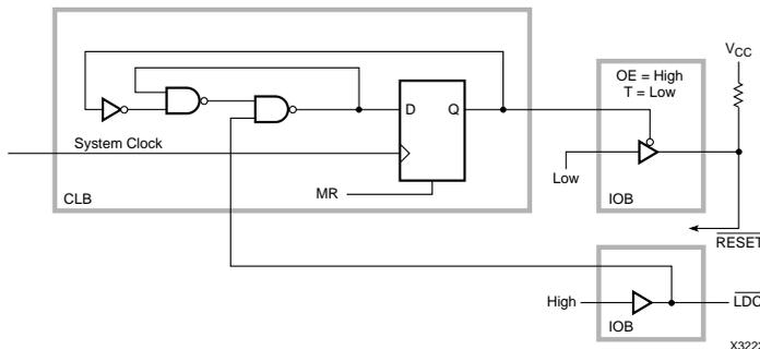
Figure 10: Synchronous Reset
