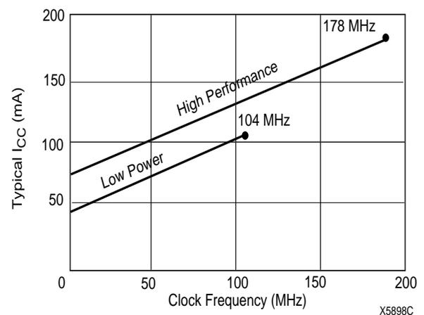
Figure 1: Typical  $I_{CC}$  vs. Frequency for XC95144XL
