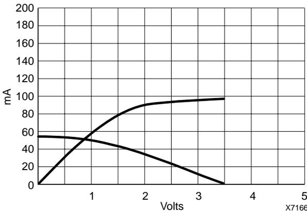
**Figure 3: Output Voltage/Current Characteristics (default for XC4000XL, XC4000XV and Spartan-XL)**
