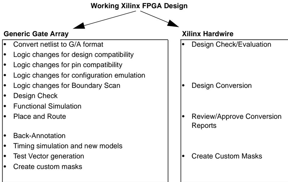
**Figure 2: Steps Involved in Converting a PLD Design to a Gate Array as Compared to a HardWire Device**
