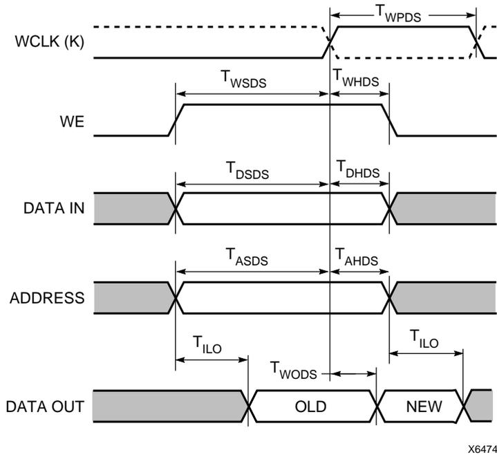
**XC4000EX CLB RAM Asynchronous (Level-Sensitive) Write and Read Operation Guidelines**
