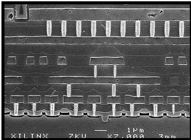
**Figure 1: Cross Section of Xilinx 0.25 micron, 5 layer metal XC4000XV FPGA.** Visible features are five layers of metallization, tungsten plug vias and trench isolation. The small gaps above the lowest layer are 0.25 micron polysilicon MOSFET gates. The excellent planarity of each metal layer is due to the use of “chemical-mechanical polishing” or CMP. In effect, each layer is ground flat before a new layer is added.
