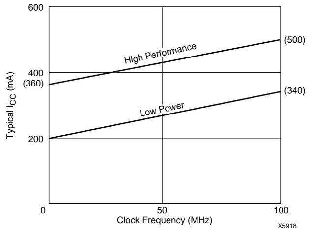
Figure 1: Typical I<sub>CC</sub> vs. Frequency For XC95216
