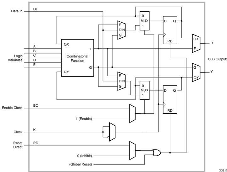
Figure 1: Configurable Logic Block (CLB)
