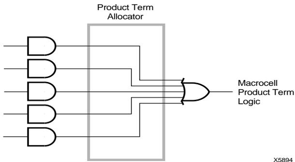
Figure 5: Macrocell Logic Using Direct Product Term
