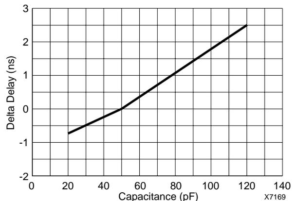
**Figure 4: Additional Delay at Various Capacitive Loads**
