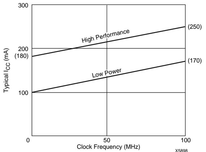
Figure 1: Typical  $I_{CC}$  vs. Frequency for XC95108
