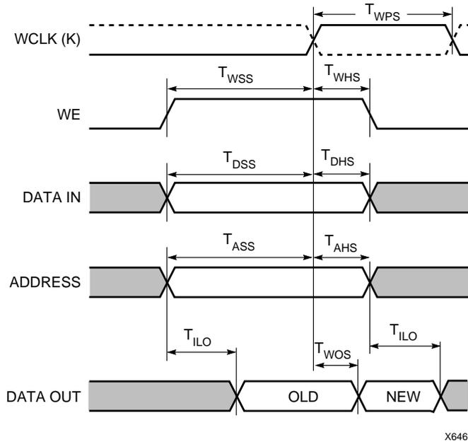
**XQ4000E CLB Dual-Port RAM Synchronous (Edge-Triggered) Write Timing**
