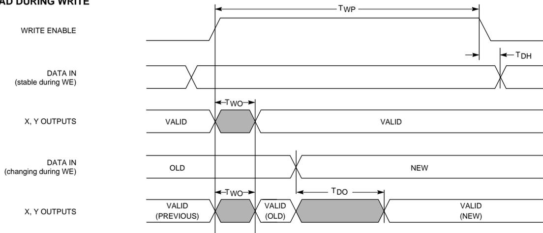
**READ DURING WRITE, CLOCKING DATA INTO FLIP-FLOP**
