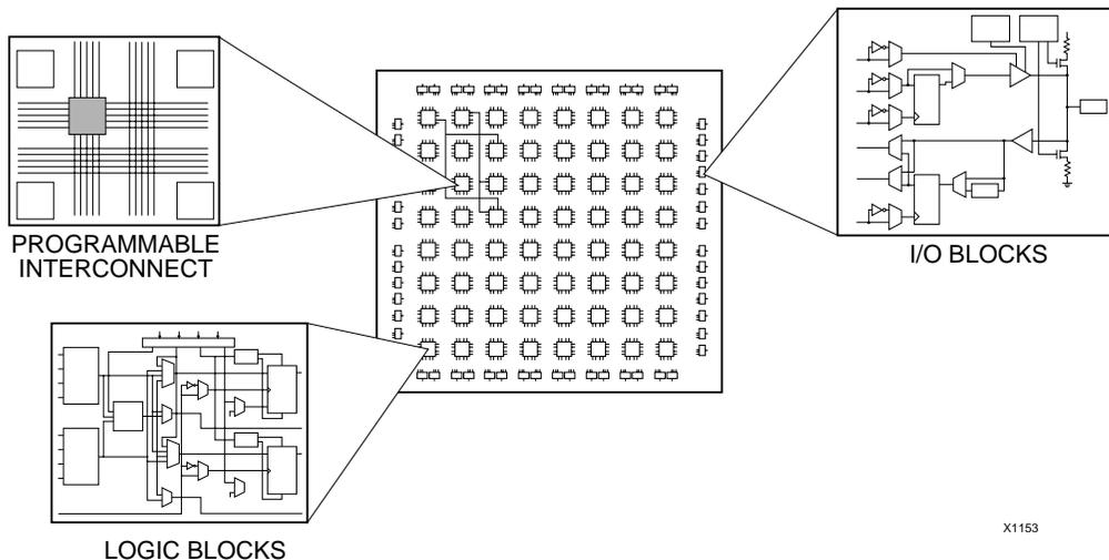
Figure 3: FPGA Architecture
