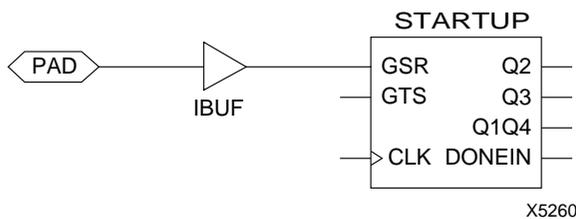
**Figure 3: Schematic Symbols for Global Set/Reset**
