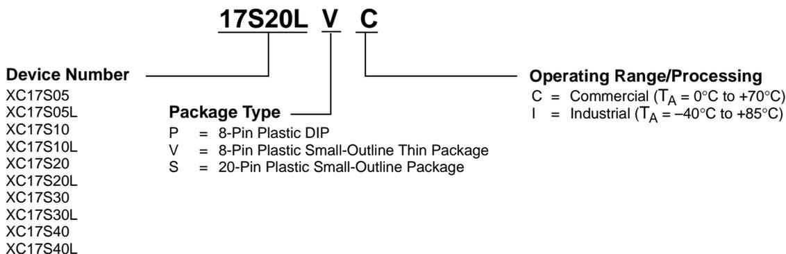
**Note:** When marking the device number on the XL parts, an L is used in place of an XL.
