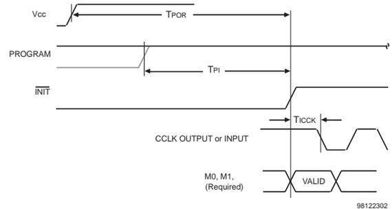
Figure 17: Power-up Timing Configuration Signals
