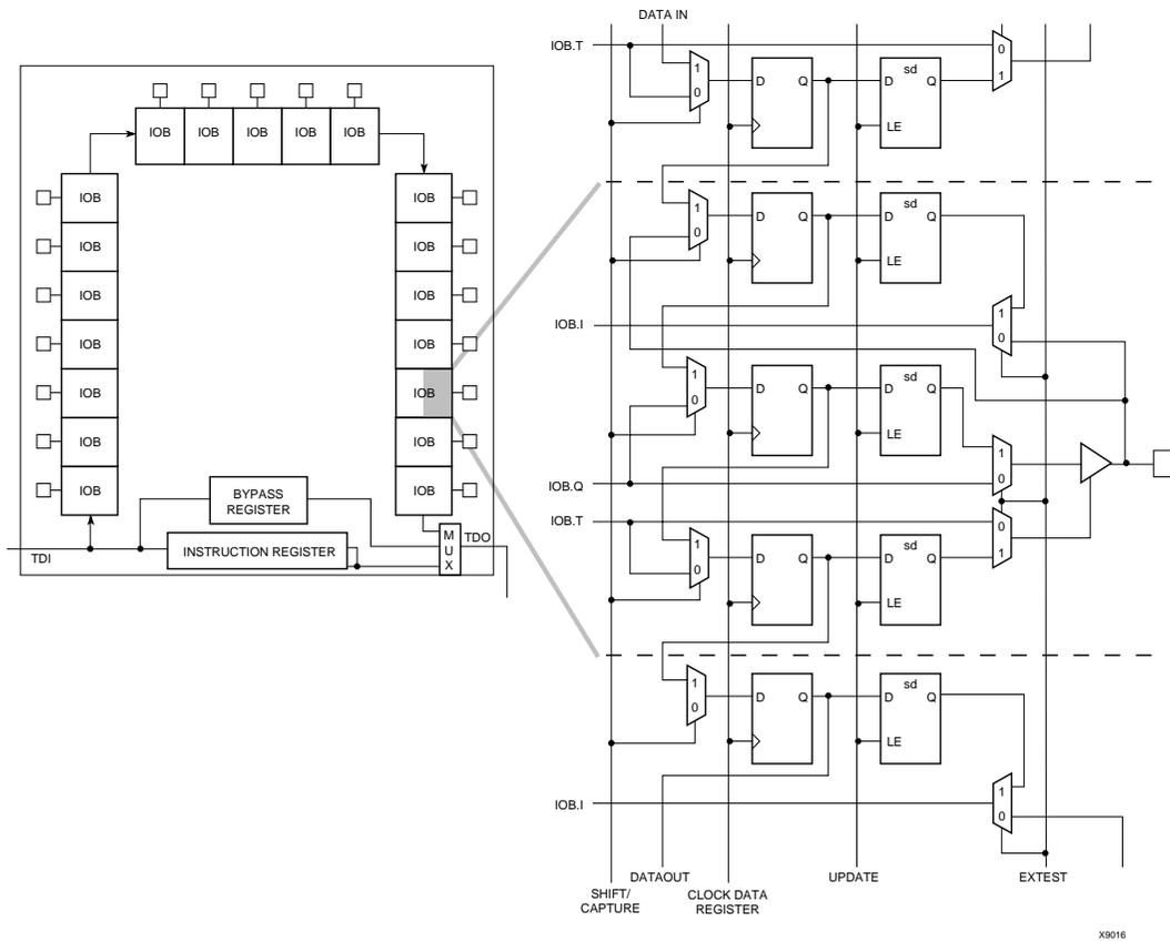
Figure 42: XC4000 Series Boundary Scan Logic
