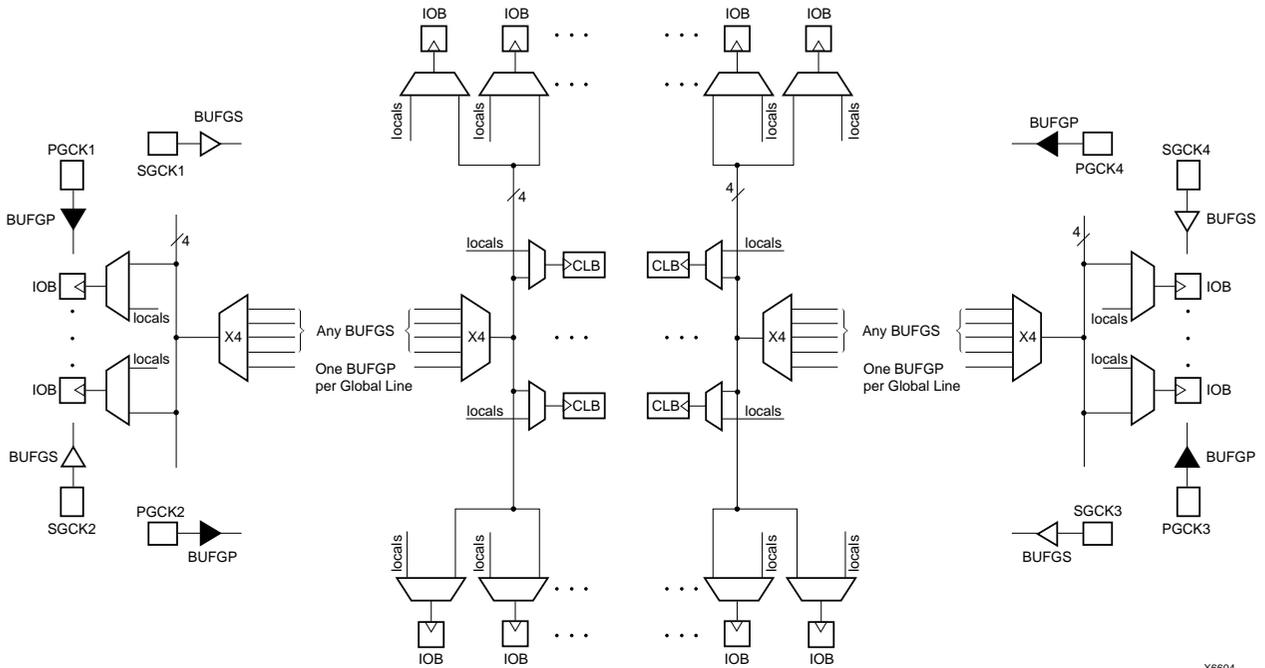
**Figure 11: 5V Spartan Series Global Net Distribution**
