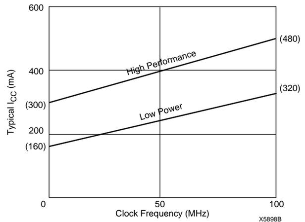
Figure 1: Typical  $I_{CC}$  vs. Frequency for XC95144
