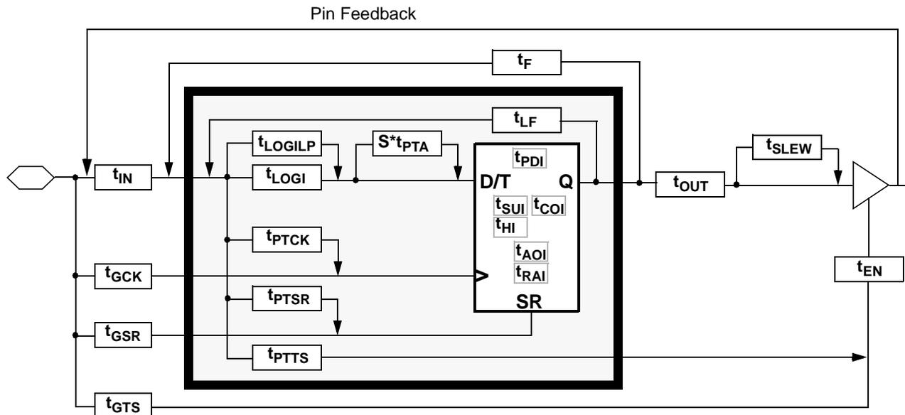
Figure 15: Detailed Timing Model
