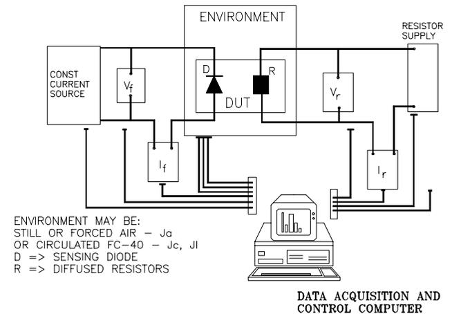
**Figure 2: Thermal Measurement Set-Up (Schematic for Junction to Reference)**
