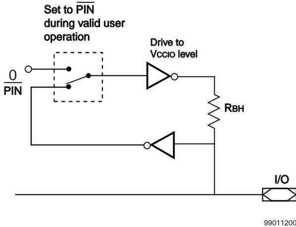
Figure 13: Bus-Hold Logic
