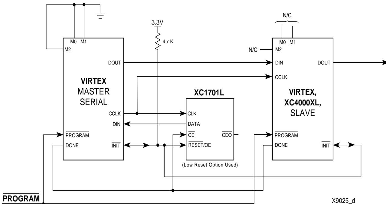
Figure 10: Master/Slave Serial Mode Circuit Diagram
