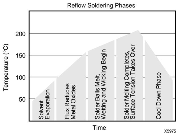
Figure 3: Soldering Sequence
