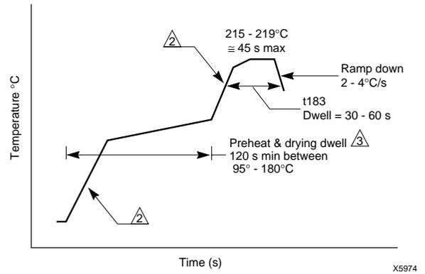
**Figure 5:** Typical Conditions for IR Reflow Soldering
