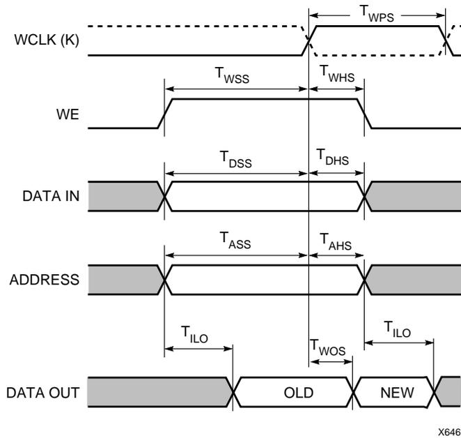
**XQ4000EX CLB Dual-Port RAM Synchronous (Edge-Triggered) Write Timing**
