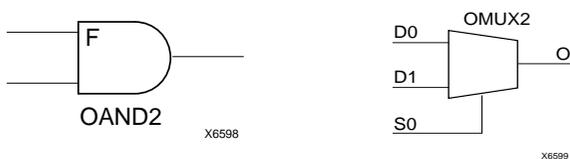
**Figure 21: AND & MUX Symbols in XC4000X IOB**
