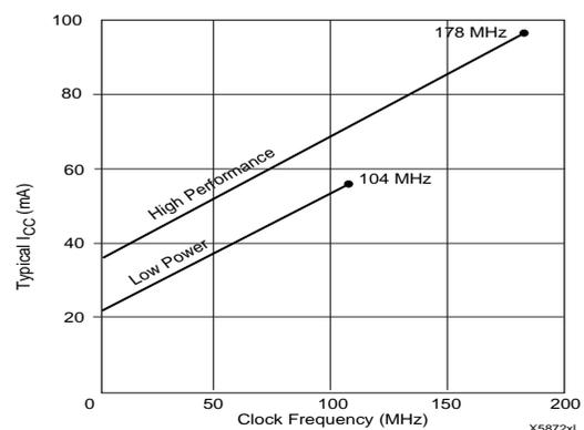
Figure 1: Typical  $I_{CC}$  vs. Frequency for XC9572XL
