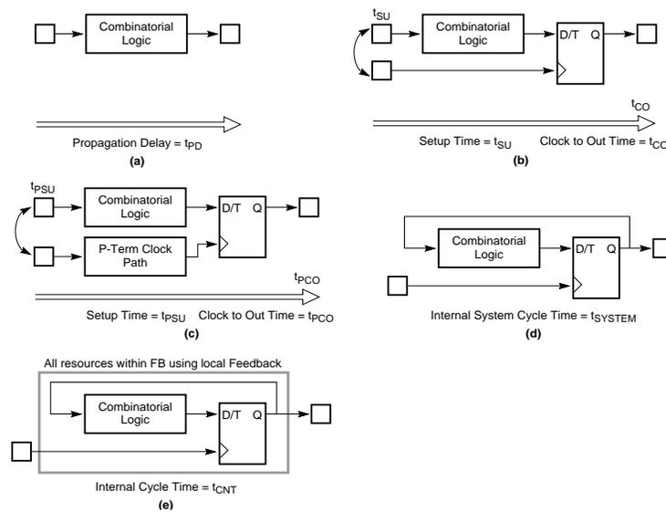
Figure 14: Basic Timing Model
