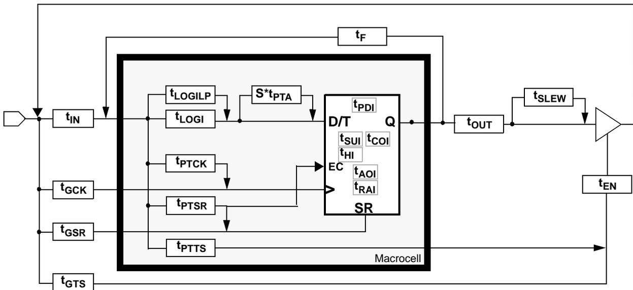
Figure 16: Detailed Timing Model
