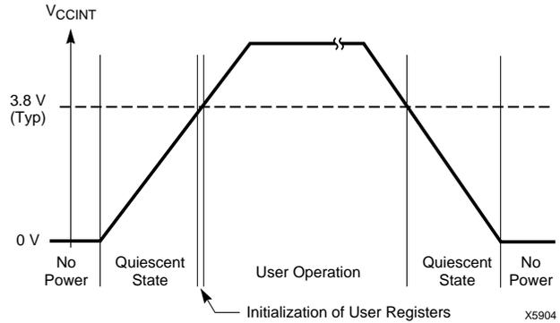
**Figure 16: Device Behavior During Power-up**
