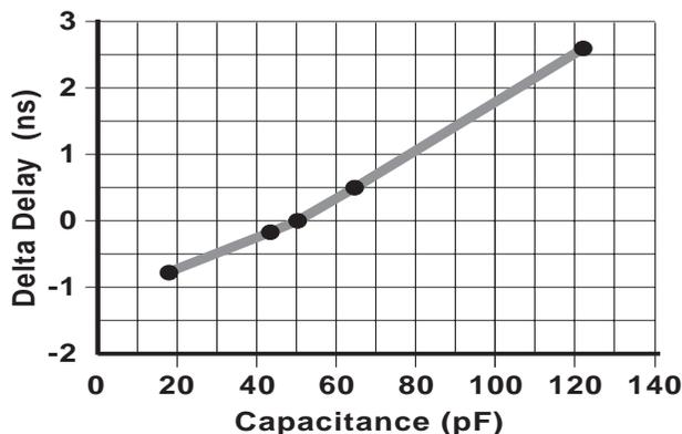
Figure 8: Delay Factor at Various Capacitive Loads
