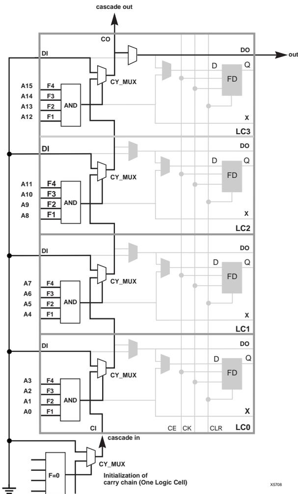
**Figure 7: XC5200 CY\_MUX Used for Decoder Cascade Logic**
