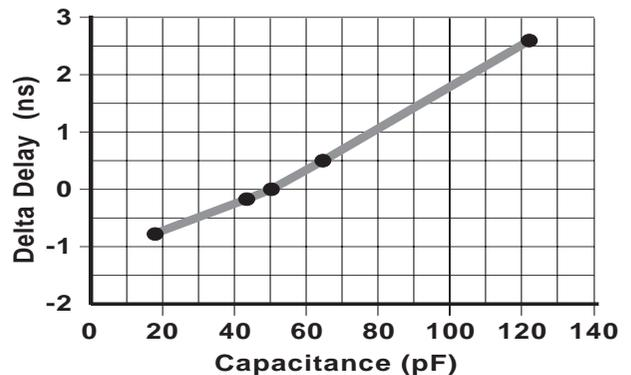
Figure 61: Delay Factor at Various Capacitive Loads X8257
