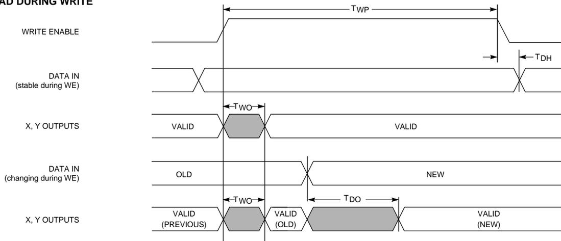
**READ DURING WRITE, CLOCKING DATA INTO FLIP-FLOP**
