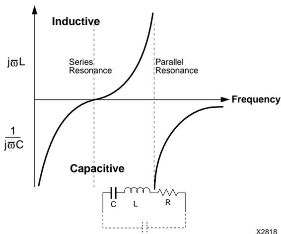
**Figure 6: Reactance as a Function of Frequency**
