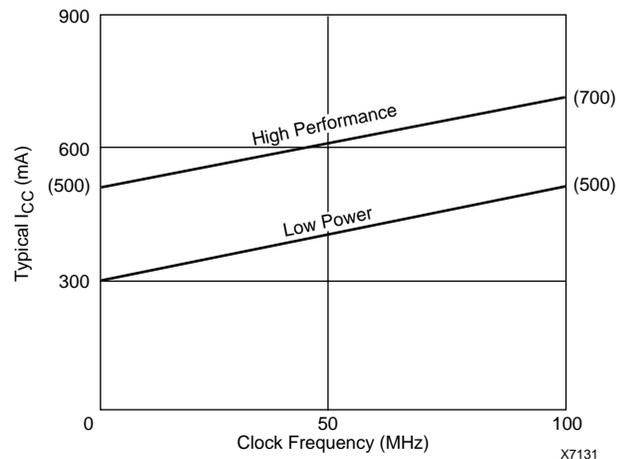
Figure 1: Typical I<sub>CC</sub> vs. Frequency For XC95288
