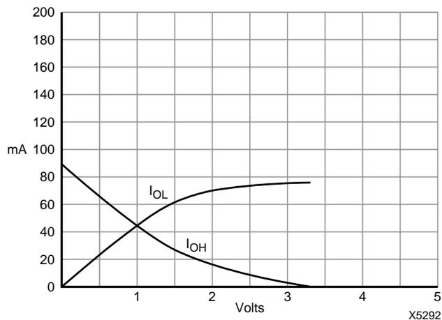
Figure 2: Output Voltage/Current Characteristics for XC4000XL
