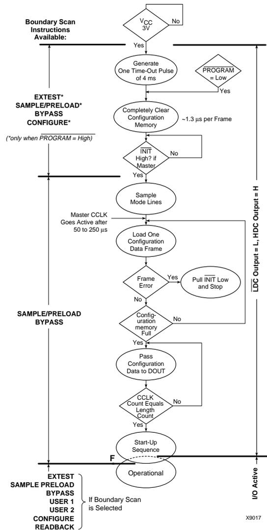
Figure 24: Configuration Sequence
