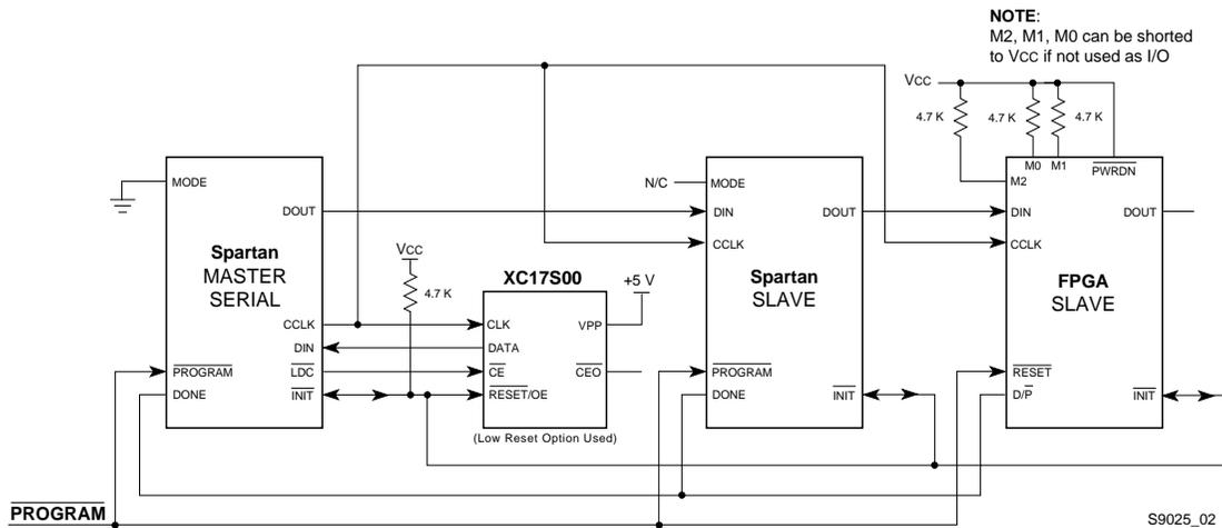
Figure 24: Master/Slave Serial Mode Circuit Diagram
