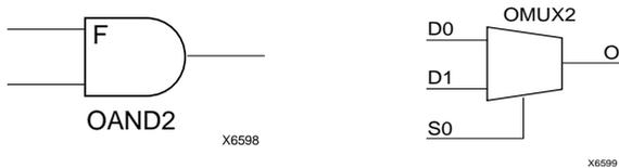
**Figure 7: AND & MUX Symbols in SpartanXL IOB**
