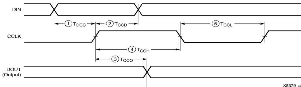
Figure 11: Slave Serial Mode Programming Switching Characteristics
