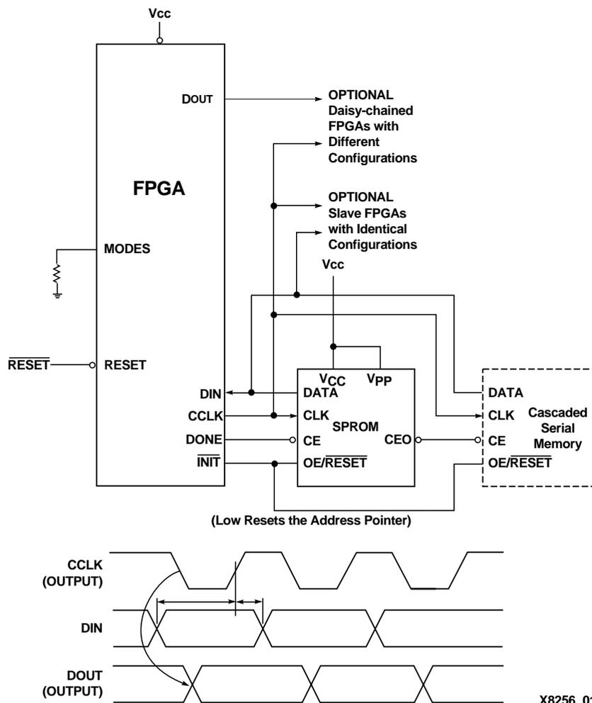
**Figure 2: Master Serial Mode.** The one-time-programmable SPROM supports automatic loading of configuration programs. Multiple devices can be cascaded to support additional FPGAs. An early DONE inhibits the PROM data output one CCLK cycle before the FPGA I/Os become active.
