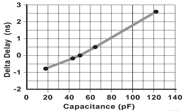
Figure 7: Delay Factor at Various Capacitive Loads X8257
