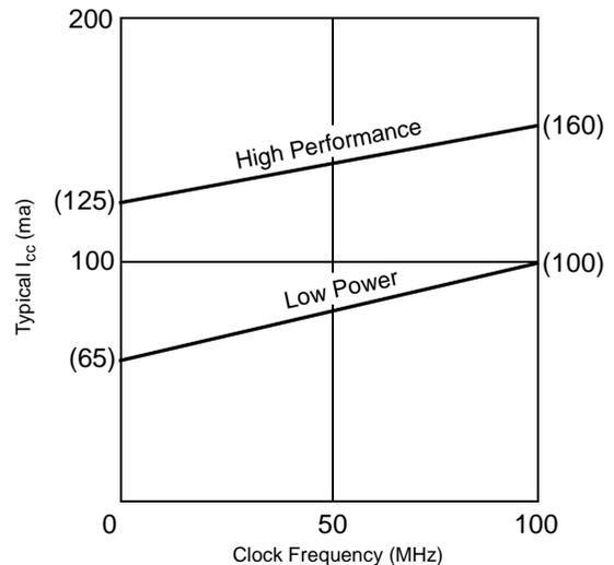
Figure 1: Typical  $I_{CC}$  vs. Frequency for XC9572
