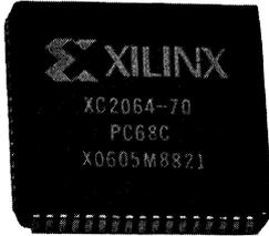
The XC2000 series of LCA devices was introduced in 1985. Price reductions since that time have reflected steadily increasing production volumes. The family includes two compatible arrays: the XC2064 with 1200 gates, and the XC2018 with 1800 gates.
