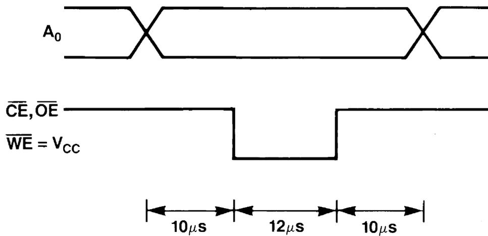
Figure 10: Static life test bias diagram
