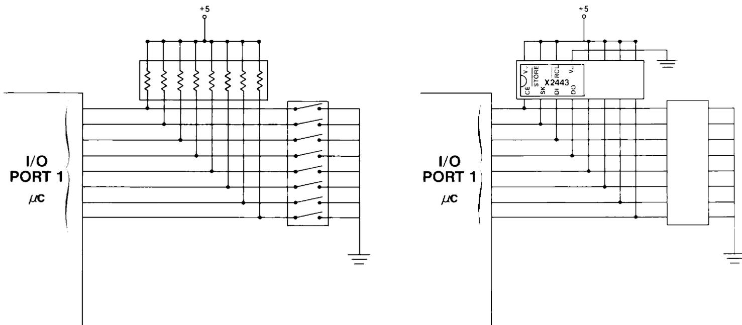
**Figure 2. Microcomputer without Internal Pullups**
