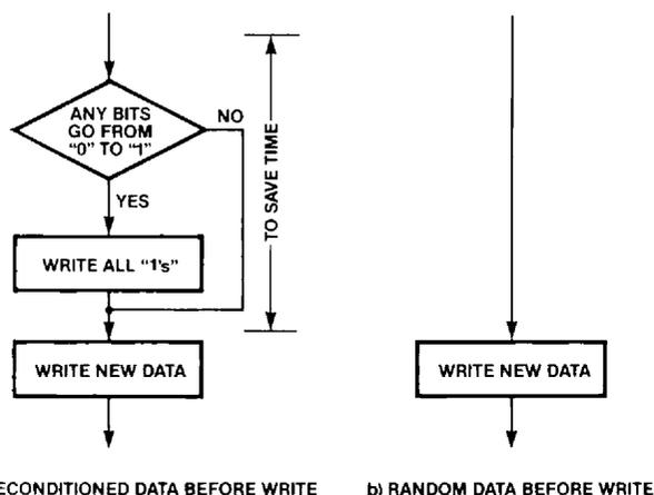
Figure 9) Comparison of software requirements for minimum write time systems between a) preconditioned data and b) random data prior to the write cycle.
