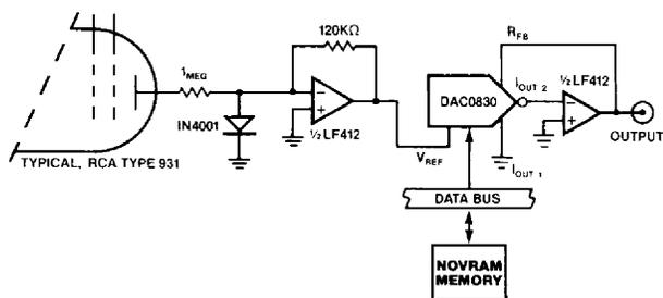
Figure 15) Gain trimming for photomultiplier tubes.
