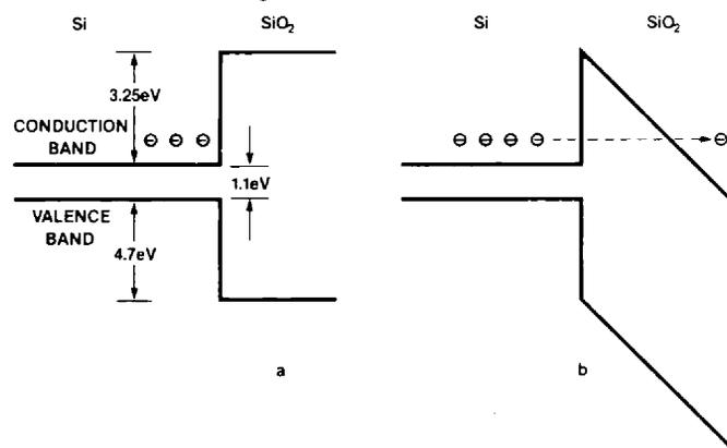
Figure 7. Energy band diagrams of the Si/SiO<sub>2</sub> system in the neutral state (a), and during the store operation (b).
