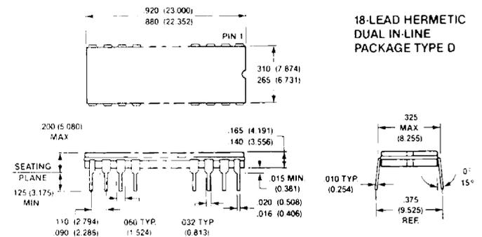
Figure 3. Package outline drawing for memories in cerdip
