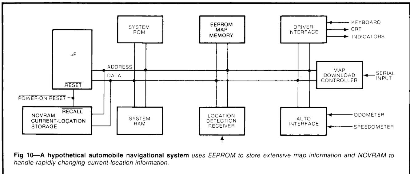
Fig 10—A hypothetical automobile navigational system uses EEPROM to store extensive map information and NOVRAM to handle rapidly changing current-location information.
