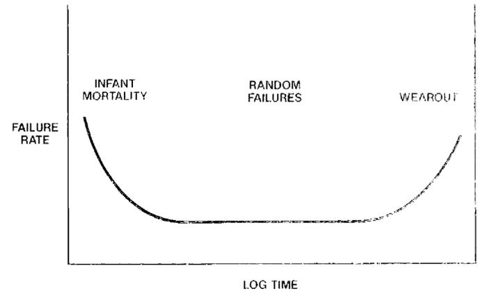
Figure 17. Illustration of bathtub curve of failure rates showing regions in which infant mortality, random failures, and wearout mechanisms dominate the failure rate.
