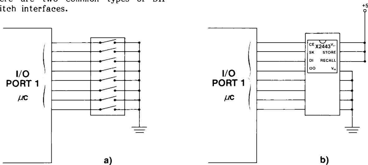
**Figure 1. Microcomputer with Internal Pullups**
