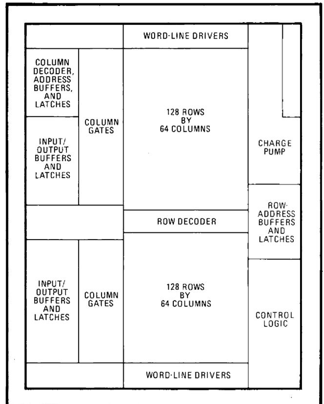
**1. All aboard.** This 16-K electrically erasable programmable read-only memory integrates all its support circuits. A charge pump generates the programming voltage from a 5-V supply; latches hold addresses and data during the internally timed write cycle.
