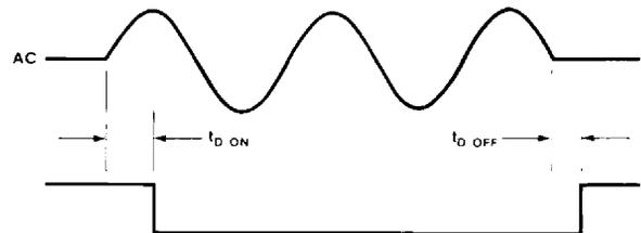
Figure 11) Waveforms for the MID400.
