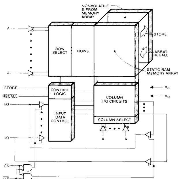
Figure 1) Block diagram of the XICOR NOVRAM family
