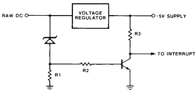
Figure 14) A Zener diode in series with a base-emitter diode establishes the trip point of this dc detector.
