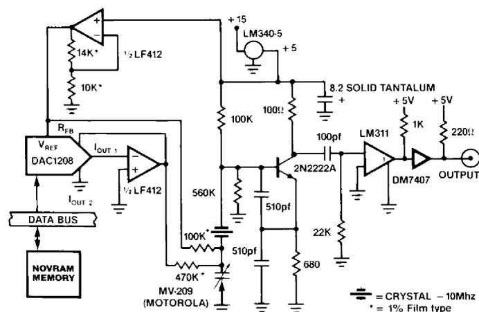
Figure 10) Tuneable crystal oscillator.
