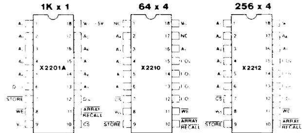
Figure 3) Pin configuration of the XICOR NOVRAM family.
