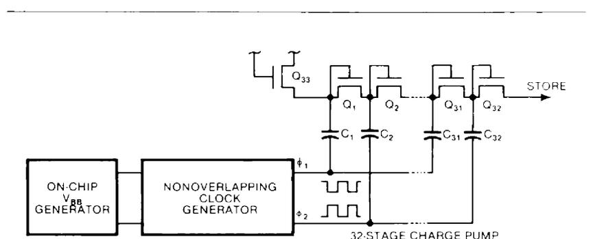
**Fig B—A 32-stage charge pump** internally generates a NOVRAM's high Store voltage, allowing the device's NOVRAM and EEPROM sections to operate from 5V.
