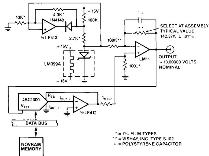
Figure 12) Software programmable voltage reference.
