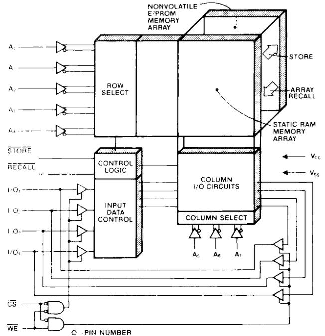
Figure 2. Functional diagram of X2212 memory
