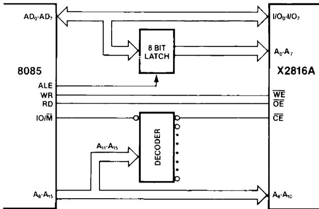
Figure 11) Interfacing the X2816A to the 8085 microprocessor.
