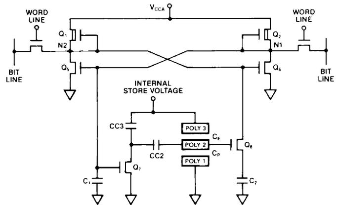
Figure 6. Schematic diagram of a NOVRAM memory cell showing how a standard six-transistor static RAM cell is merged with a floating gate E<sup>2</sup>PROM cell.
