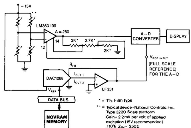
Figure 14) Automatic scale calibration.
