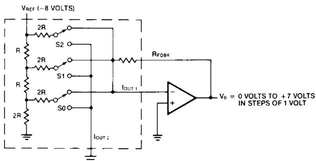
Figure 7) A simplified 3-switch CMOS DAC.
