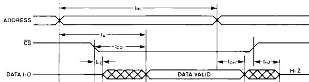
Figure 5) Timing diagram for Reading from the RAM.
