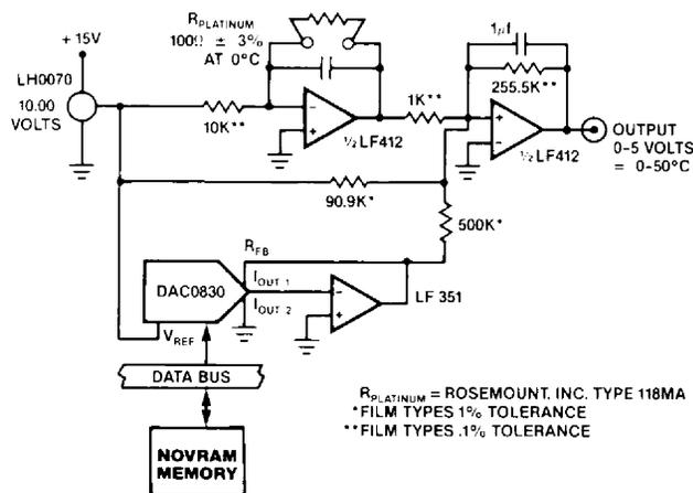
Figure 13) Self-calibrating, interchangeable probe thermometer.
