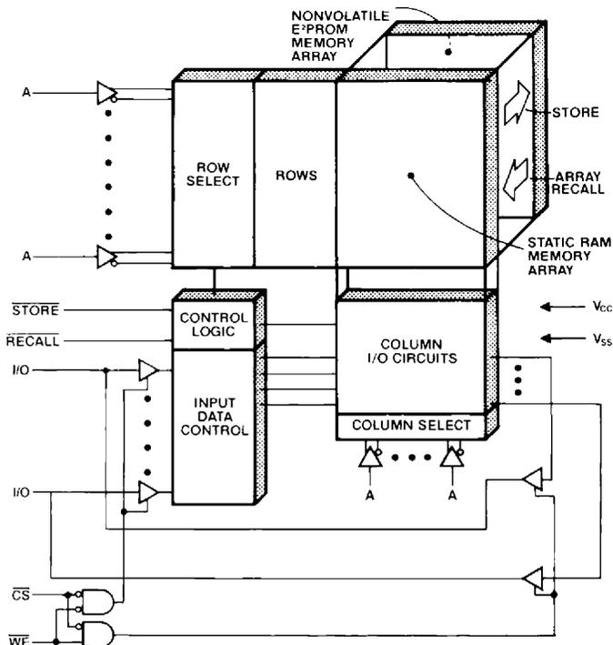
Figure 1) NOVRAM memory block diagram.
