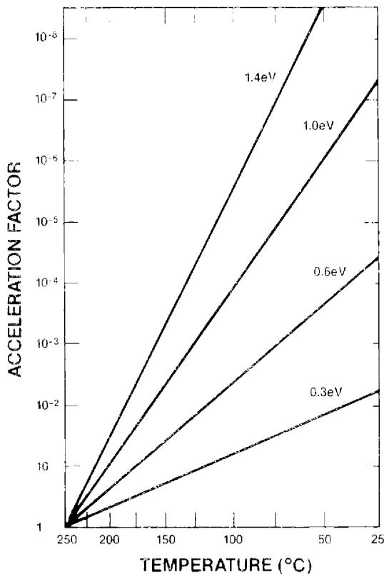
Figure 18. Acceleration factor vs. temperature calculated for various activation energies from Arrhenius relation.
