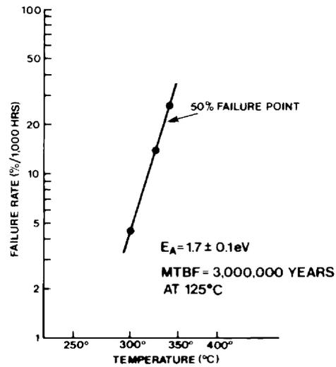
Figure 8:  $E^2$  cell endurance data for a typical cell
