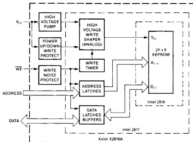
Figure 8) Evolution of easy-to-use EEPROMs from the Intel 2816 and 2817 to the Xicor X2816A.
