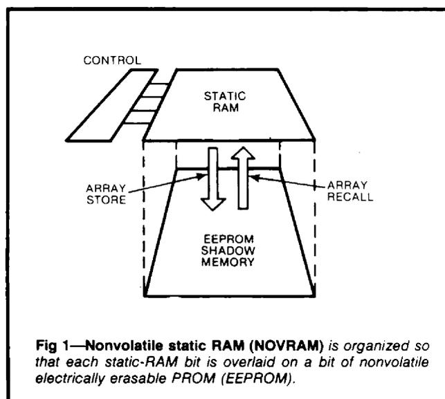
**Fig 1—Nonvolatile static RAM (NOVRAM) is organized so that each static-RAM bit is overlaid on a bit of nonvolatile electrically erasable PROM (EEPROM).**
