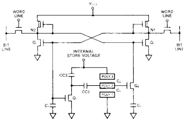
Figure 2) Circuit diagram of a NOVRAM cell.
