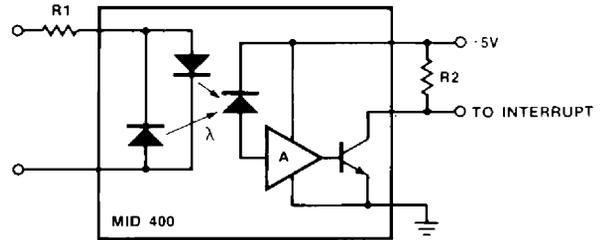
Figure 10) The MID400 requires only two resistors to connect directly to the ac power line.
