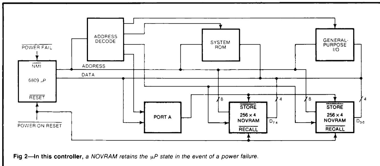
Fig 2—In this controller, a NOVRAM retains the μP state in the event of a power failure.
