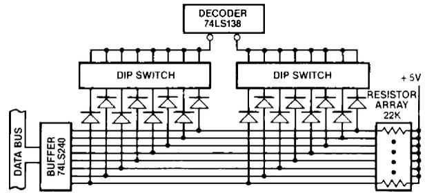
Figure 2) Typical DIP switch interface for multiple packages.
