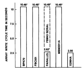
Figure 2: Array Write Cycle Times
