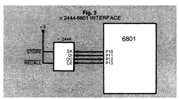
lines and software. Housed in an eight-pin mini-DIP, the X2444 provides inexpensive non-volatile data storage for both operational and configuration parameters. Its low cost (less than \$4.00 in unit quantities) makes it the least expensive non-volatile storage on the market, even rivalling the DIP switch in unit cost, while providing the equivalent of 32 DIP switches in terms of data capacity.
