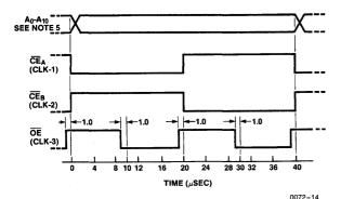
Figure 8b: X2804A/2816A (DIP) Burn-In Timing
