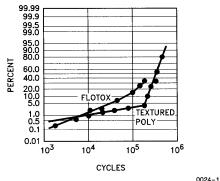
Figure 1: Percent fail vs. number of cycles at room temperature for FLOTOX (2816A, 2817A) and Textured Poly (2864).
