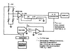
Figure 14) Automatic scale calibration
