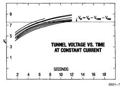
Figure 7: This is a record of tunnel voltage (expressed as trap-up voltage) vs time. The end of endurance is reached when the tunnel voltage reaches a value  $V_{Qf}$ . The time associated with that voltage can be read off this chart.
