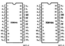
Figure 1: X2804A and X2816A Pin configurations.
