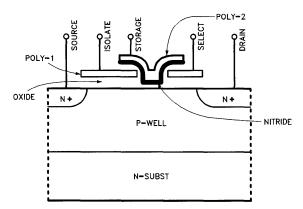
Figure 1c: Cross sectional structure of a MNOS memory cell.8
