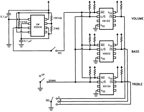
Figure 11: Switch Network for Manual Operation
