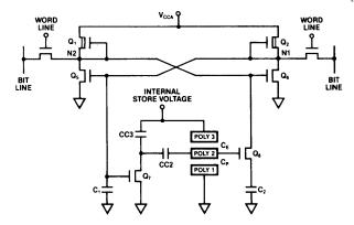
Figure 5: Schematic diagram of a NOVRAM memory cell.
