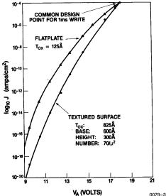
Figure 5: Comparison of calculated tunneling J-V curves for emission from a planar and a textured structure. The devices were designed to have the same emission in the high current regime where programming takes place.
