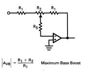
Figure 7: Bass Portion of Active Preamp Circuit
