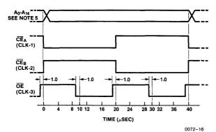
Figure 9b: X2864A/2864B/2864H/28256 (DIP) Burn-In Timing
