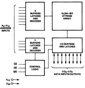
Figure 2: X2816A Functional block diagram.
