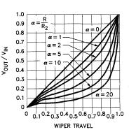
Figure 9: Utilizing External Resistors to Vary Potentiometers Trim (EDN Nov. 13)
