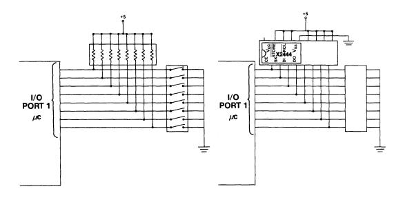
Figure 2. Microcomputer without Internal Pullups
