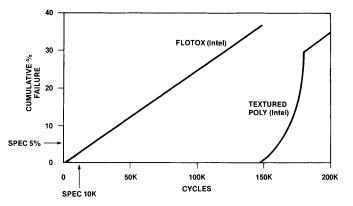
Figure 1: Endurance of two E<sup>2</sup> technologies. FLOTOX and textured poly processed at Intel (16K arrays).
