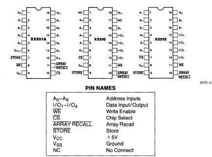
Figure 1: X2201A, X2210, and X2212 pin assignment drawings.
