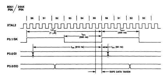
Figure 1. 12 MHz 8051 Serial Port Mode 0 and X2444 Timing
