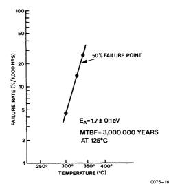
Figure 16: Log data loss rate vs. inverse temperature for X2210's.
