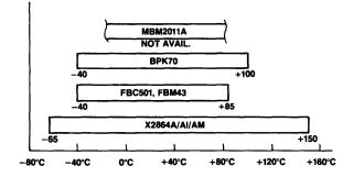
Figure 5: Nonvolatile Storage Temperature
