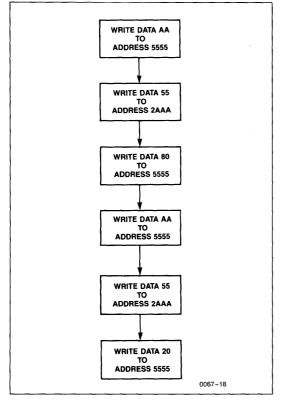
In the event the user wants to deactivate the software data protection feature for testing or reprogramming in an E<sup>2</sup>PROM programmer, the following six step algorithm will reset the internal protection circuit. After t<sub>WC</sub>, the X28C256 will be in standard operating mode.
