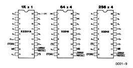
Figure 3) Pin configuration of the XICOR NOVRAM family.
