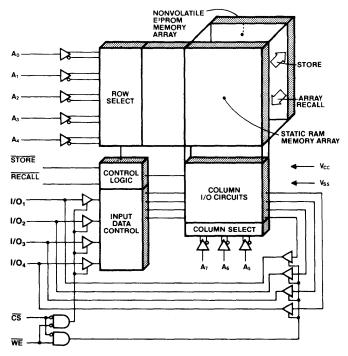
Figure 2: Functional diagram of X2212 memory.
