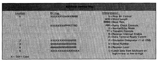
device, with the associated data stored in each of the 16-bit locations. The end results of replacing the DIP switch with the NOVRAM are increased design flexibility, as well as reduced manufacturing and testing costs.
