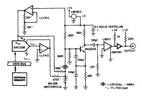
Figure 10) Tuneable crystal oscillator.
