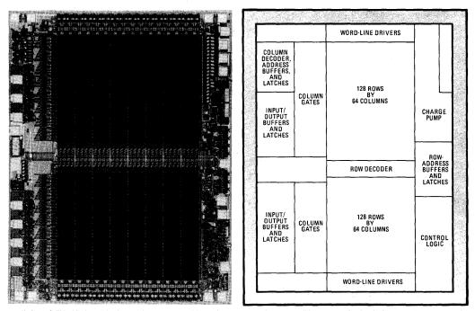
1. All aboard. This 16-K electrically erasable programmable read-only memory integrates all its support circuits. A charge pump generates the programming voltage from a 5-V supply; latches hold addresses and data during the internally timed write cycle.
