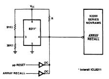
Figure 3: Power-up/Power-down Write Protection Circuit
