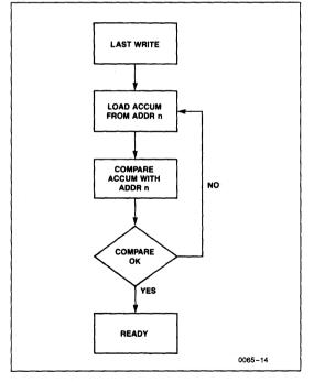
The Toggle Bit can eliminate the software housekeeping chore of saving and fetching the last address and data written to a device in order to implement  $\overline{DATA}$  Polling. This can be especially helpful in an array comprised of multiple X28C256 memories that is frequently updated. The timing diagram in Figure 3a illustrates the sequence of events on the bus. The software flow diagram in Figure 3b illustrates a method for testing the Toggle Bit.
