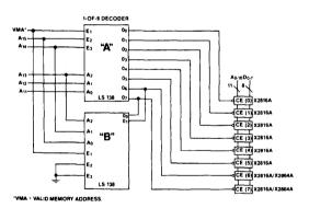
Figure 4. 74LS138 Decode Wiring Option
