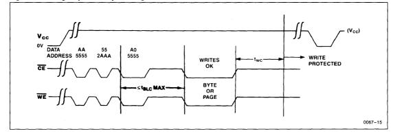
Figure 4b: Write Sequence for Software Data Protection
