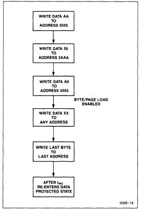
Regardless of whether the device has previously been protected or not, once the software data protected algorithm is used and data has been written, the X28256 will automatically disable further writes unless another command is issued to cancel it. If no further commands are issued the X28256 will be write protected during power-down and after any subsequent power-up.
