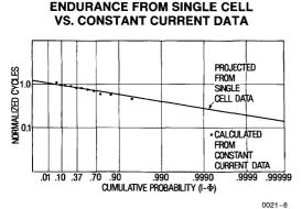
Figure 8: This is again a Log Extreme Value probability plot. The points are those calculated from the times measured via Figure 7. The straight line represents the endurance predicted from the single cell data in Figure 5.
