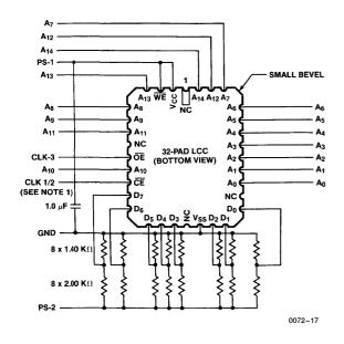
Figure 10a: X2816A/2816B/2864A/2864B/2864H/28256 (LCC) Burn-In Circuit
