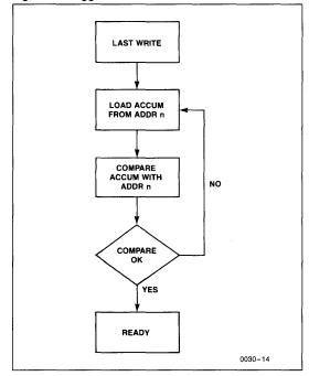
Figure 3b: Toggle Bit Software Flow
