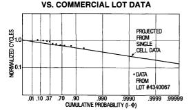
0021-6 Figure 6: This is a Log Extreme Value probability plot of the endurance of a lot of X2212 NOVRAMs. The points are measured values, the straight line represents endurances predicted from the single cell data shown in Figure 5.
