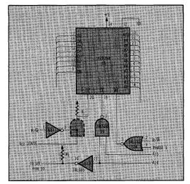
Fig 5 The EEPROM control logic uses the processor's high order address lines to map the device into the proper address range and enable it at the same time.
