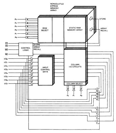
Figure 2: X2004 functional block diagram.
