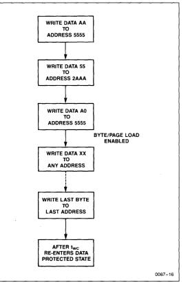
Regardless of whether the device has previously been protected or not, once the software data protected algorithm is used and data has been written, the X28C256 will automatically disable further writes unless another command is issued to cancel it. If no further commands are issued the X28C256 will be write protected during power-down and after any subsequent power-up.
