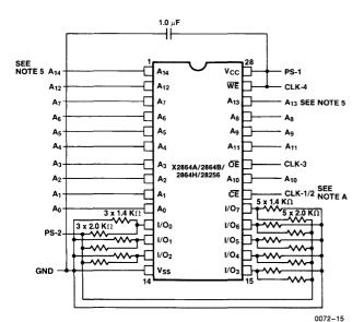
Note A: CLK-1: Rows 1, 3, 5 . . . (odd rows $-\overline{CE}_A$ ) CLK-2: Rows 2, 4, 6 . . . (even rows $-\overline{CE}_B$ ) Such that: CLK-2 =  $\overline{CLK-1}$
