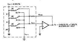
Figure 7) A simplified 3-switch CMOS DAC.
