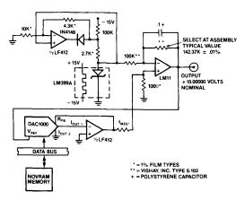
Figure 12) Software programmable voltage reference.
