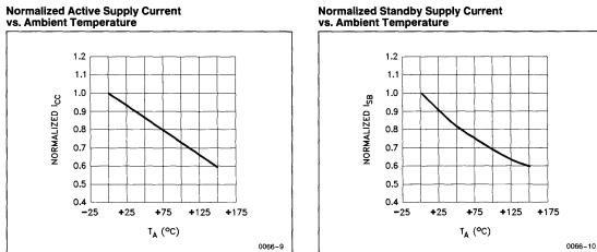
Normalized Standby Supply Current vs. Ambient Temperature
