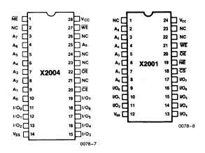
Figure 1: X2004 and X2001 pin configurations.
