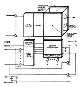
Figure 1) NOVRAM memory block diagram.
