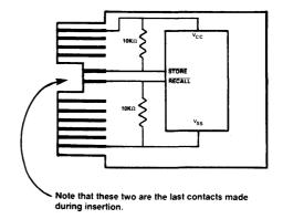
Figure 5: Typical Cartridge Write Protect Scheme
