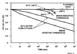
Figure 3: Data Retention: Floating gate, no intrinsic charge retention problem; MNOS, continuous charge loss and window closure tending to become worse after cycling.
