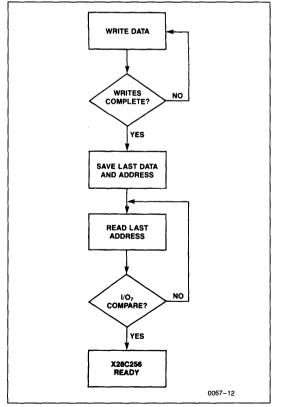
DATA Polling can effectively halve the time for writing to the X28C256. The timing diagram in Figure 2a illustrates the sequence of events on the bus. The software flow diagram in Figure 2b illustrates one method of implementing the routine.
