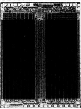
ide floating gates are relative- 1. SMALL DIE. Equivalent in size to many thin-oxide 64-K parts, ly easy to manufacture, but Xicor's 256-K EEPROM die measures about 64,000 mils2.
