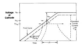
Figure 4: Voltage vs. Time Relationships at Floating Gate
