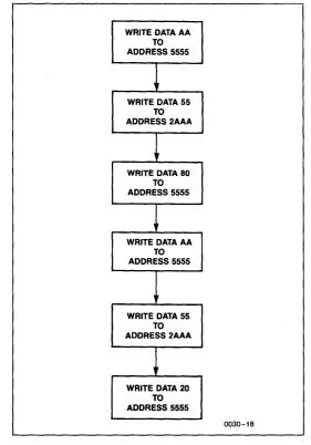
In the event the user wants to deactivate the software data protection feature for testing or reprogramming in an E<sup>2</sup>PROM programmer, the following six step algorithm will reset the internal protection circuit. The next time the X28256 is powered-up the device will be in the standard operating mode.
