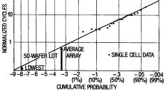
Figure 5: This shows the Log Normal probability plot of individual single cell endurance data. The right half of the plot is quite standard, as marked by typical cumulative percentages. The left half represents an extension of the standard chart to much lower probabilities, in order to permit predictions for specific members of a much larger population.
