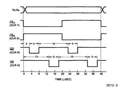
Notes: (1)  $A_0$ - $A_8$ : binary sequencing cycle period: 40  $\mu$ s. (2) NE disabled (tied to V<sub>CC</sub> at device).
