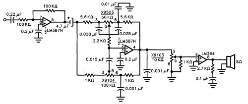
Figure 10: E<sup>2</sup>PREAMP with Three X9MME—No Digital Controls Shown
