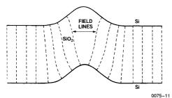
Figure 11: Sketch illustrating the manner in which field lines converge near convex feature and diverge near concave feature.
