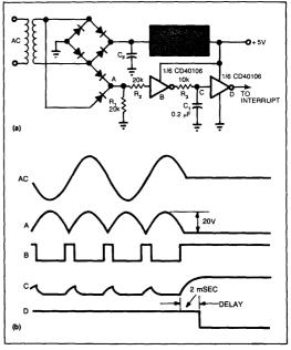
Fig 6—When you use two Schmitt triggers to detect ac loss (a), the delay produced by  $R_i$  and  $C_i$  must be longer than the first gate's output pulse width. The timing diagram (b) shows the circuit waveforms.
