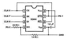
Notes: (1) STO (Pin 7) must be hardwired to V<sub>CC</sub> (Pin 9) at device as shown.
