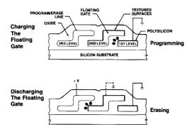
Figure 1: TPFG Cell Operation
