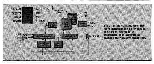
read operation, the processor supplies the read instruction, and then gives the X2443 16 clock cycles, which the device uses to output the data to be read. The NOVRAM also includes several non-data types of instructions to control the nonvolatile operation of the part, the part's power consumption, and the write/store lockout feature.
