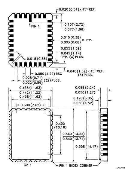
32-PAD CERAMIC LEADLESS CHIP CARRIER (GLASS FRIT SEAL) PACKAGE TYPE G
