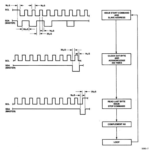
X2404 Burn-in timing diagram and program flow.
