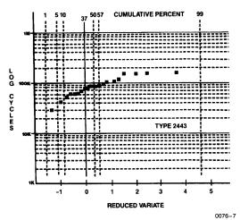
Figure 7: Endurance data from a lot of Xicor X2443 Serial NOVRAMs.
