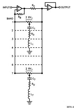
Figure 3: Graphic Equalizer Configuration
