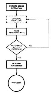
Figure 2: Early Write Completion Flowchart
