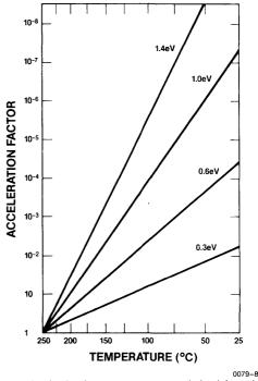
Figure 10: Acceleration factor vs. temperature calculated for various activation energies from Arrhenius relation.
