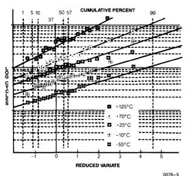
Figure 4: The effect of temperature on endurance: the endurance doubles for every increase in temperature by 50°C.
