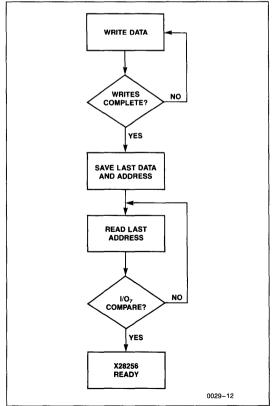
DATA Polling can effectively halve the time for writing to the X28256. The timing diagram in Figure 2a illustrates the sequence of events on the bus. The software flow diagram in Figure 2b illustrates one method of implementing the routine.
