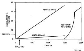
Figure 2: Endurance of 3 E<sup>2</sup> Technologies: FLOTOX and textured poly processed at Intel (16K arrays), MNOS data from Hitachi (prorated to 16K).
