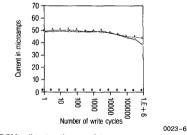
Figure 5: E<sup>2</sup>PROM cell test endurance data.
