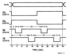
Notes: (1) A<sub>0</sub>-A<sub>8</sub>: binary sequencing cycle period: 40  $\mu$ s.
