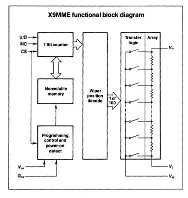
erasable ( $E^2$ ) device called the X9MME digitally controls resistance trimming. The device has three-wire TTL control and operates from a standard. 5-V power supply. Packaged in the dip is a 99-resistor array. Tap points are between the resistive elements and at the ends of the array. A tap point can be connected to the wiper output  $V_W$ .
