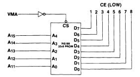
Figure 6. Bipolar PROM Mapping for Memory Expansion
