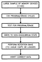
These flows will work for either FLOTOX or Textured Poly. Intermediate readouts may be performed in the oxide breakdown flow, but the test/bake/verify sequence should be repeated at each readout.
