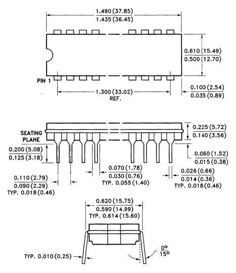
28-LEAD HERMETIC DUAL IN-LINE PACKAGE TYPE D
