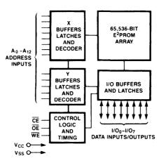
Figure 2: X2864A Functional block diagram.
