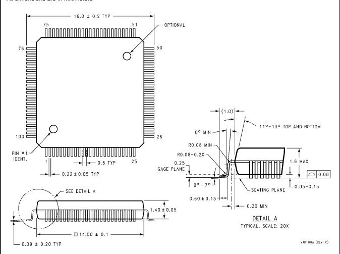
Thin Quad Flatpack (TQFP), JEDEC Order Numbers 87391D2, 87392D2, 87393FD2
