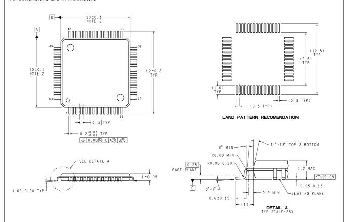
64-Pin Thin Quad Flatpack (TQFP) Order Number 87384MG/K1
