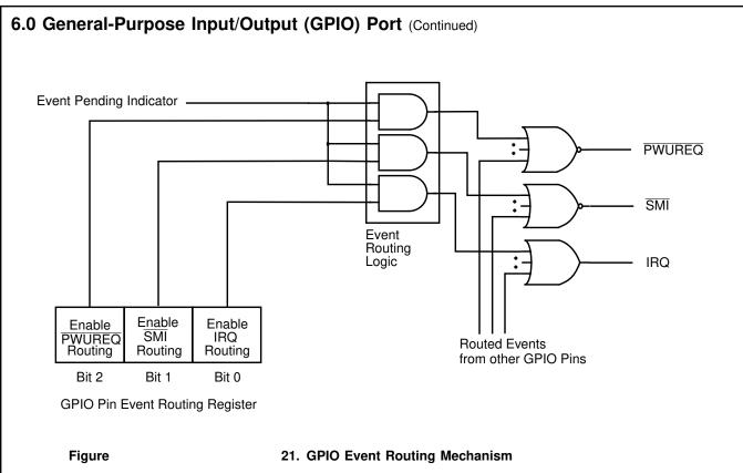
The GPEVST register is a general-purpose edge detector that may be used to reflect the event source pending status for edge-triggered events.
