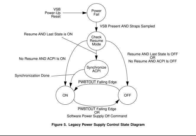
When V<sub>SB</sub> is first applied, the PSC state machine is initialized to Power Fail state. In this state, the mechanism waits for the PC87364 to be initialized according to strap options. Then the PSC enters Check Resume Mode state. In this state, the PSC checks if Resume to Last PSON state is enabled.
