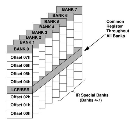
Figure 29. SP2 Register Bank Architecture
