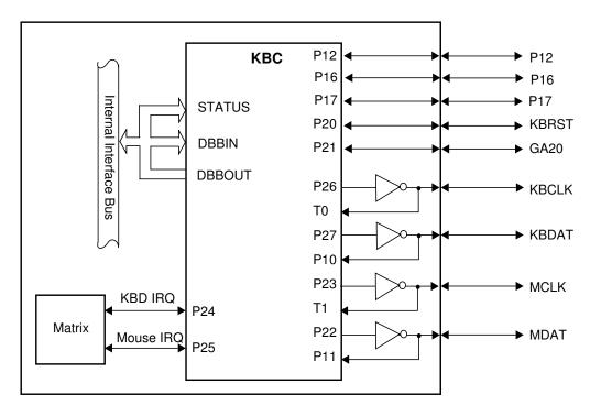
Figure 6. Keyboard and Mouse Interfaces
