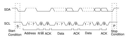
Figure 27. A Complete ACCESS.bus Data Transaction
