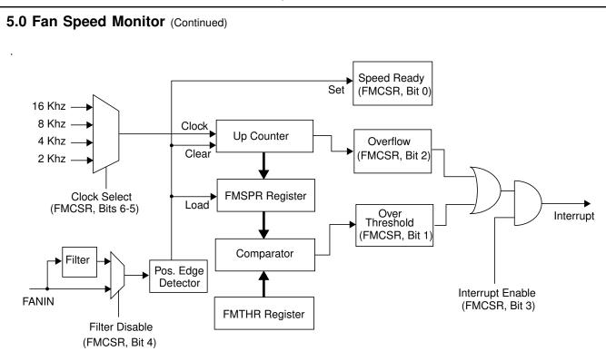
Figure 17. Fan Speed Monitor
