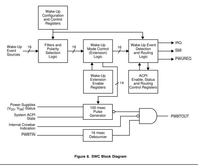
In addition to the event detection and system notification capabilities, the SWC operates several general-purpose I/O pins powered by  $V_{SB}$ . These pins can be used to perform various tasks while  $V_{SB}$  is present and  $V_{DD}$  is not.
