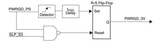
Figure 24. PWRGD\_3V Generation (Simplified Diagram)
