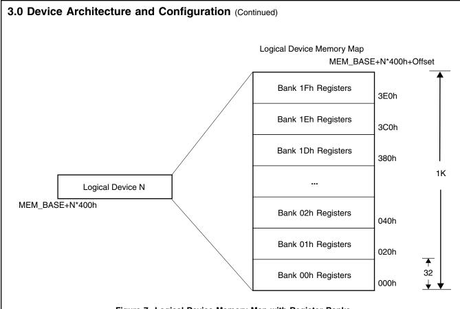
Figure 7. Logical Device Memory Map with Register Banks
