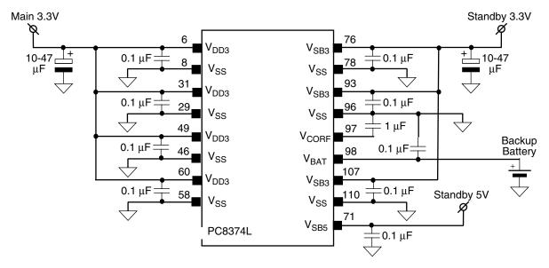
Figure 2. Decoupling Capacitors Connection
