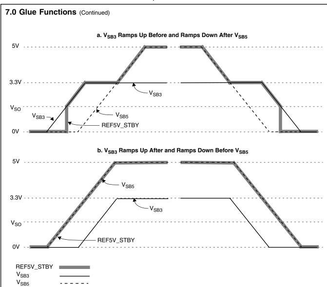
Figure 22. REF5\_STBY as a Function of  $V_{SB3}$  and  $V_{SB5}$
