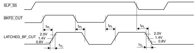
Figure 55. BKFD\_CUT and LATCHED\_BF\_CUT (AC Characteristics)
