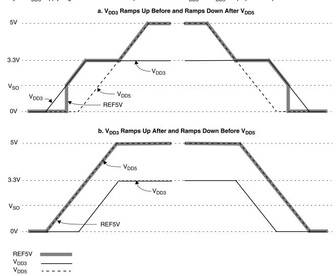
Figure 20. REF5 as a Function of V<sub>DD3</sub> and V<sub>DD5</sub>
