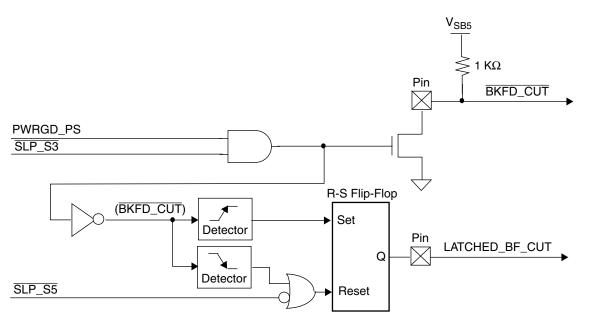
Figure 25. BKFD\_CUT and LATCHED\_BF\_CUT Generation (Simplified Diagram)
