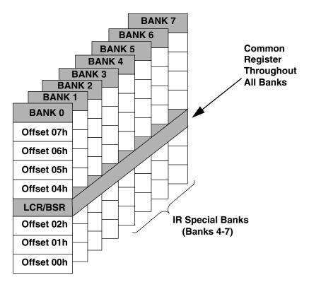
Figure 39. SP2 Register Bank Architecture
