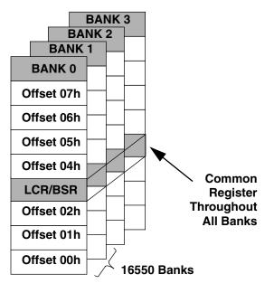
Figure 38. Register Bank Architecture
