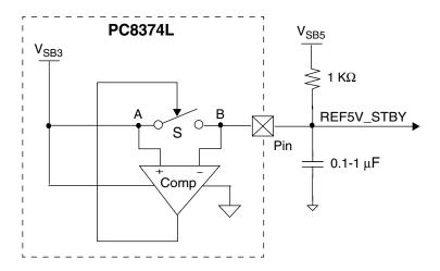
Figure 21. REF5\_STBY Generation (Simplified Diagram)
