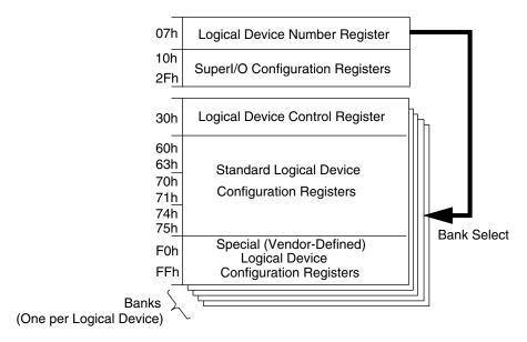
Figure 4. Structure of Standard Configuration Register File
