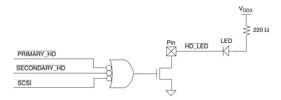
Figure 27. HD\_LED Generation (Simplified Diagram)
