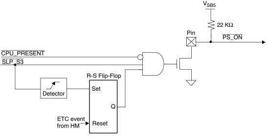
Figure 26. PS ON Generation (Simplified Diagram)
