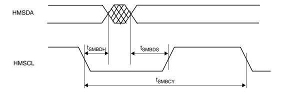
Figure 59. SMBus Data Bit Timing
