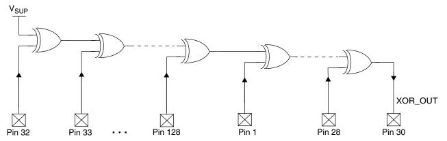
Figure 3. XOR Tree (Simplified Diagram)
