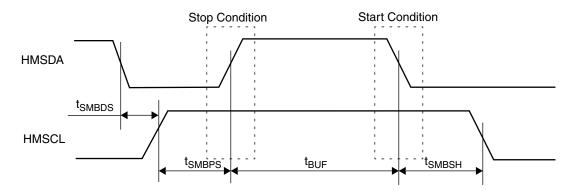
Figure 60. SMBus Start and Stop Condition Timing
