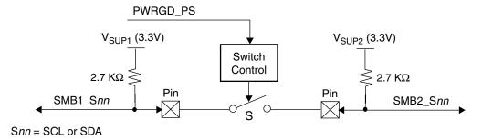
Figure 29. SMBus Isolation (Simplified Diagram)
