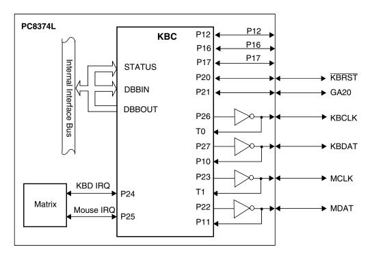
Figure 41. Keyboard and Mouse Interfaces
