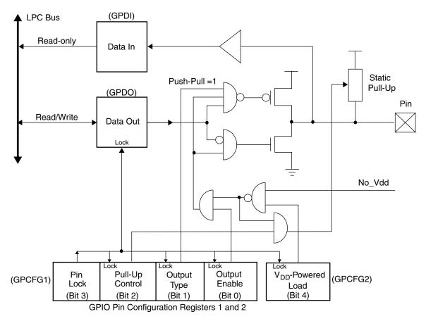
Figure 16. GPIO Basic Functionality
