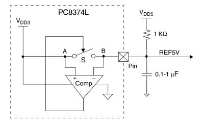
Figure 19. REF5 Generation (Simplified Diagram)
