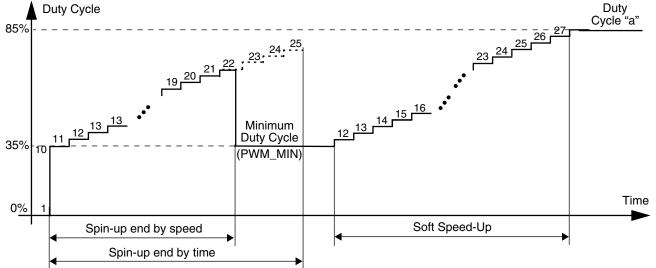
Figure 33. Soft Spin-Up and Soft Speed-Up Example
