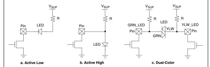
Figure 14. LED Connection Configurations
