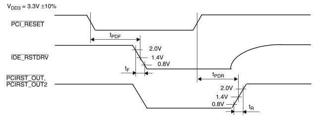
Figure 54. Reset Outputs
