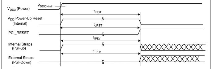
Figure 47. Internal  $V_{DD}$  Power-Up Reset
