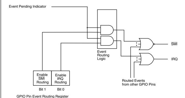
Figure 18. GPIO Event Routing Mechanism for System Notification
