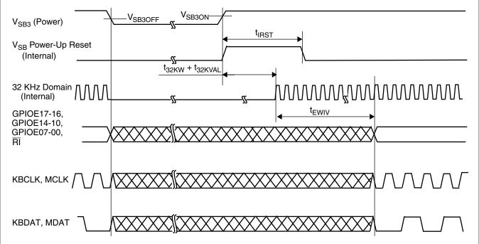
Figure 56. Inputs at V<sub>SB3</sub> Power Switching
