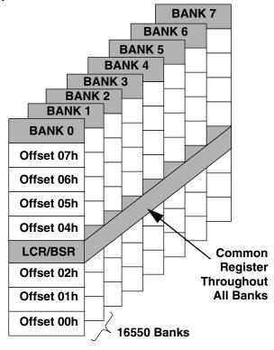
Figure 40. Register Bank Architecture
