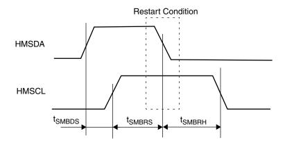
Figure 61. SMBus Restart Condition TIming
