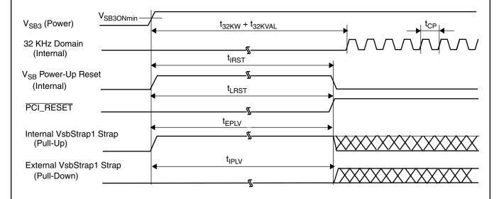
Figure 46. Internal  $V_{SB}$  Power-Up Reset - Ended by  $\overline{PCI\_RESET}$
