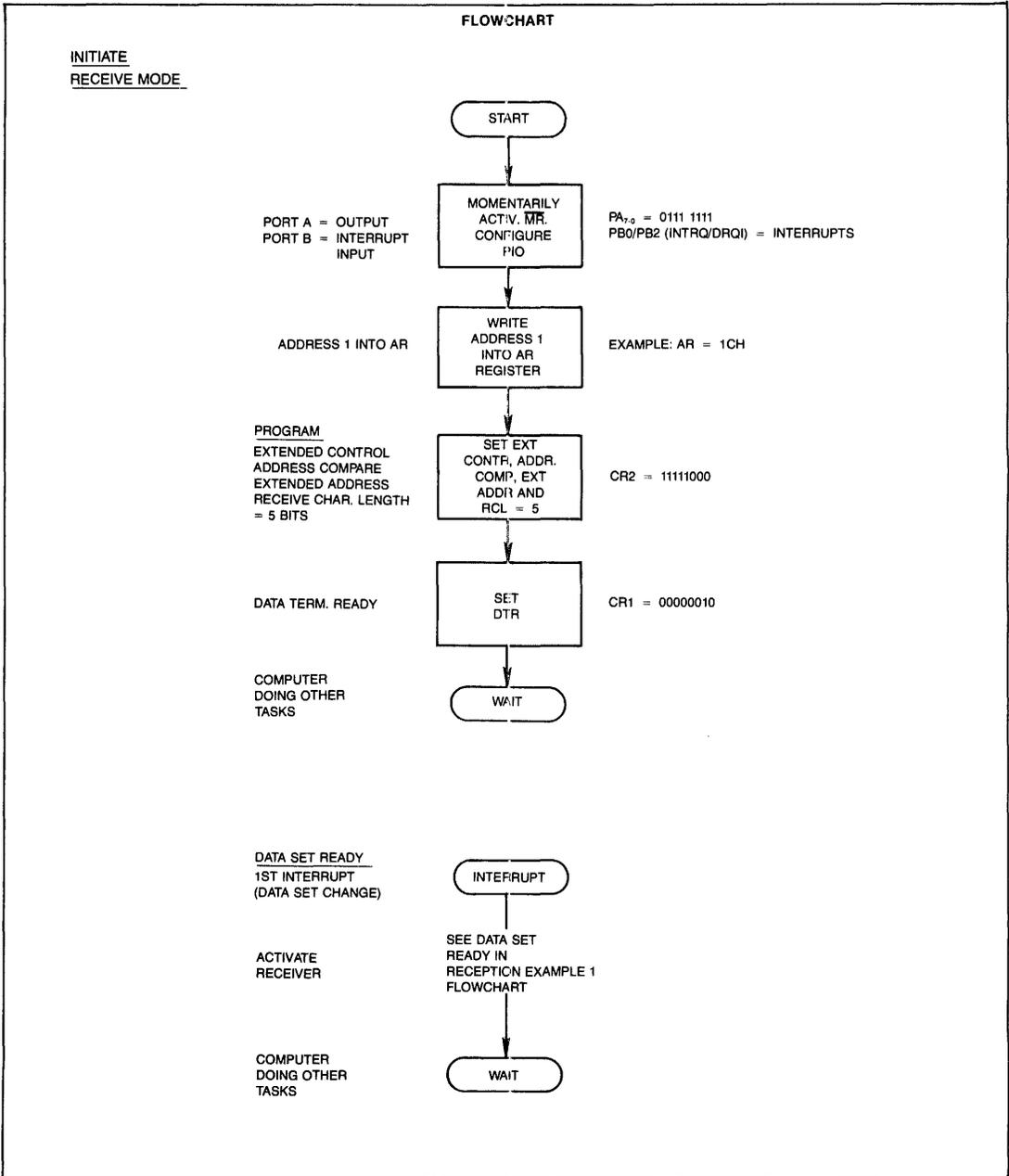
Figure 23. FLOW DIAGRAM OF FRAME RECEPTION (EXAMPLE NO. 2)
