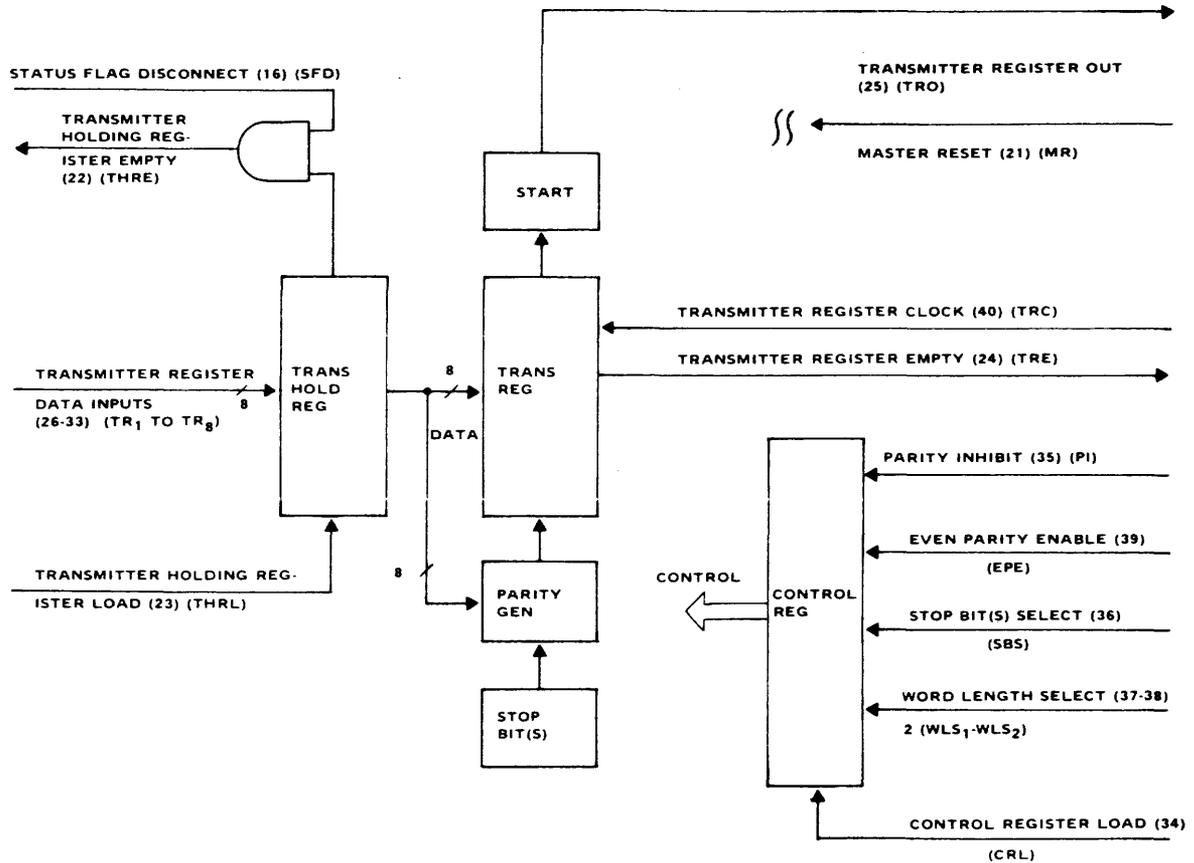
Figure 6. Transmitter Block Diagram
