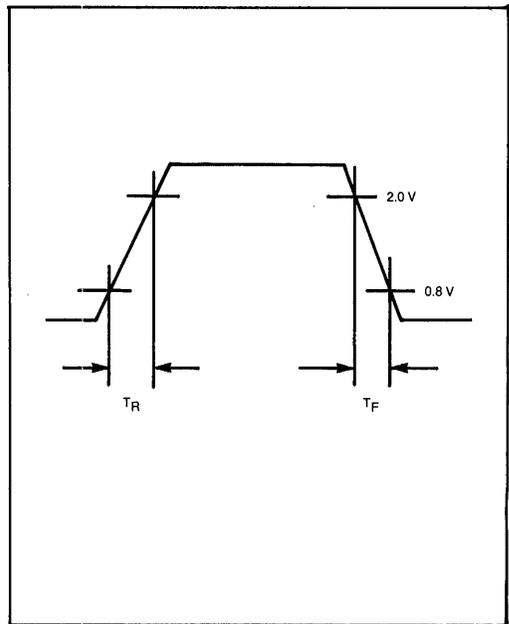
Figure 12. WD193X RISE AND FALL TIMING DIAGRAM
