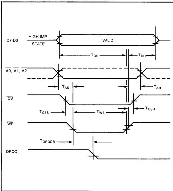
Figure 11. WD193X WRITE TIMING DIAGRAM
