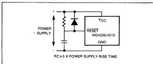
Figure 4 POWER-UP CLEAR CIRCUITS
