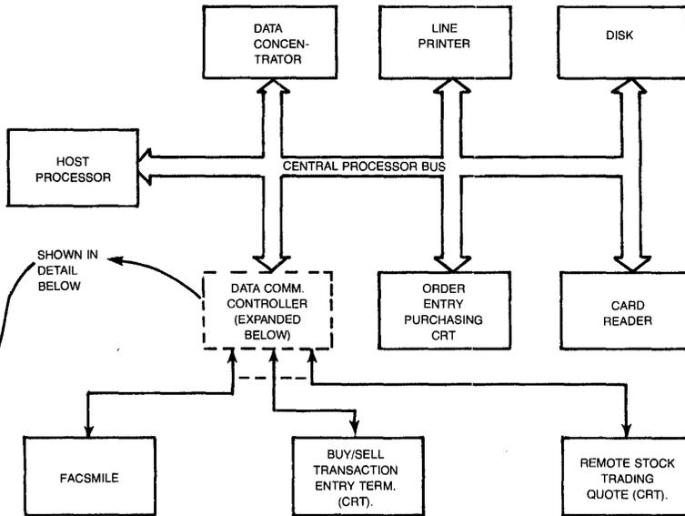
Figure 5. STOCK BROKERAGE SYSTEM
