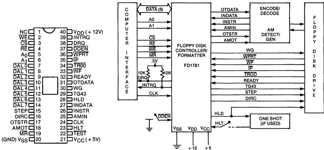
Figure 1. 1781 SYSTEM BLOCK DIAGRAM
