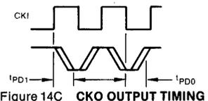
**Figure 14C CKO OUTPUT TIMING**
