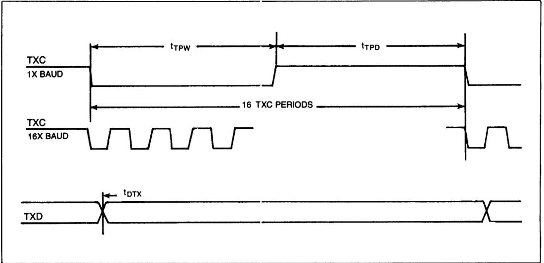
Figure 7 TRANSMITTER CLOCK AND DATA TIMINGS
