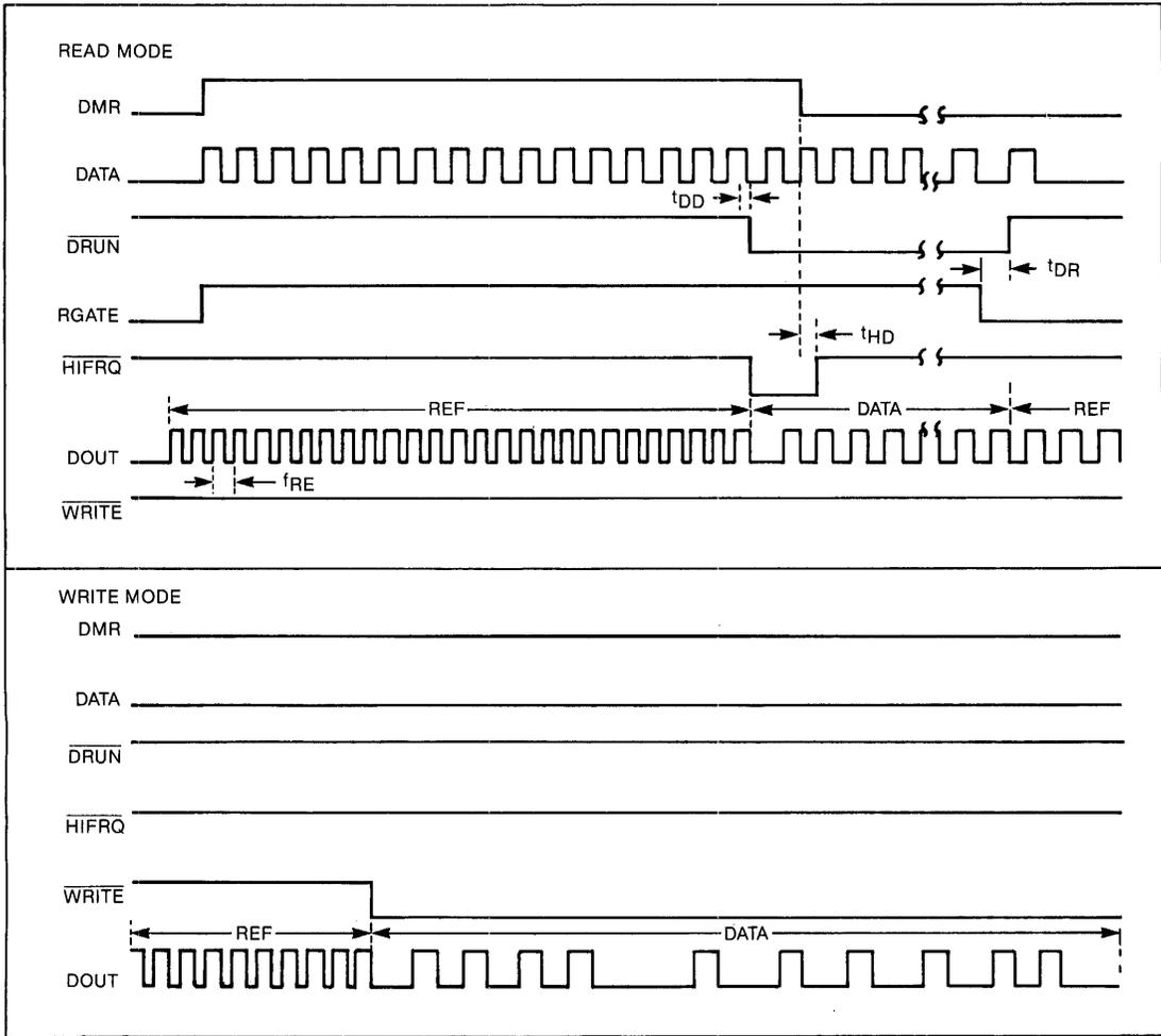
AC Electrical Characteristics  $T_A = 0^\circ\text{C to } 50^\circ\text{C}; V_{CC} = +5\text{V} \pm 10\%; V_{SS} = 0\text{V}$
