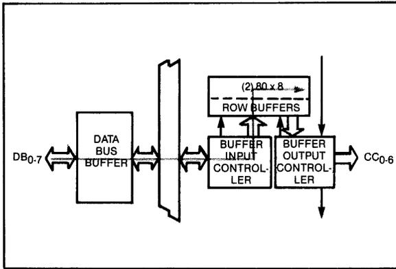
**Figure 5.** FIRST ROW BUFFER FILLED
