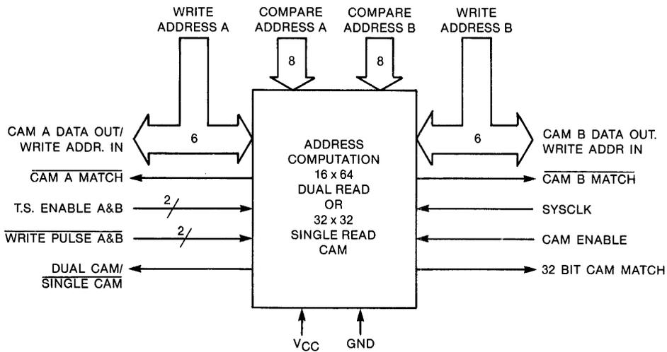
**Figure 1 — WD5010 CAM OVERVIEW BLOCK DIAGRAM**
