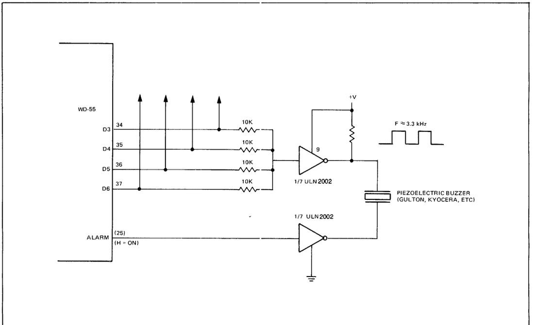
**FIGURE 9. WD-55 USED WITH PIEZOELECTRIC BUZZER**
