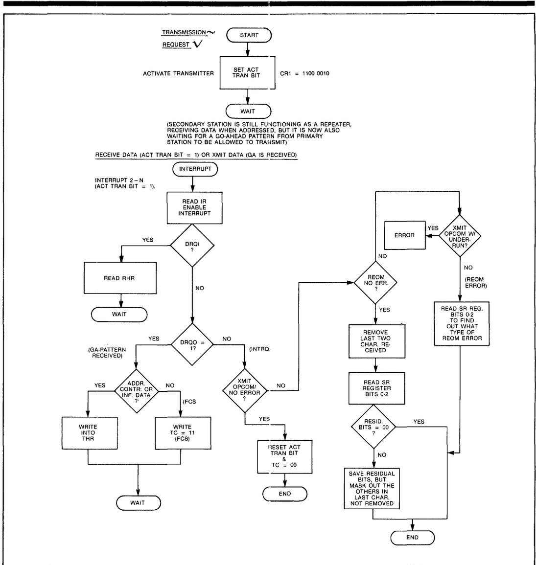
Figure 25. FLOW DIAGRAM OF SDLC LOOP MODE
