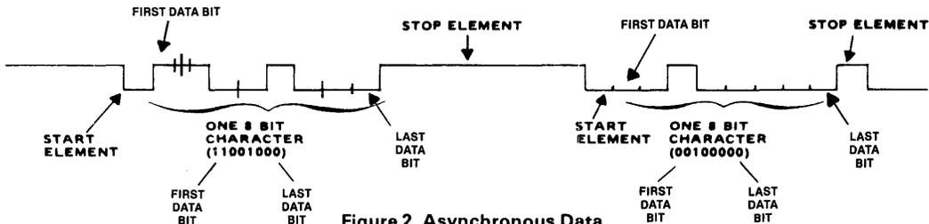
Figure 2. Asynchronous Data
