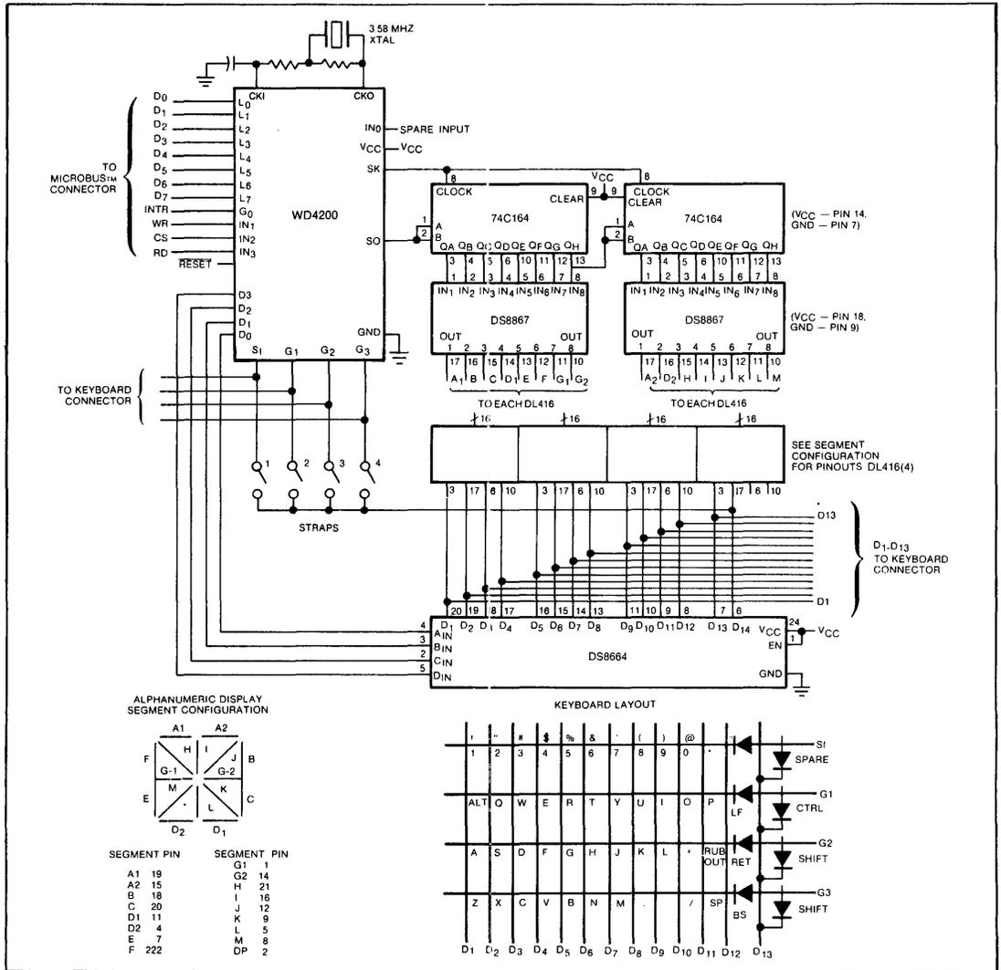
Figure 11 WD4200 KEYBOARD/DISPLAY INTERFACE
