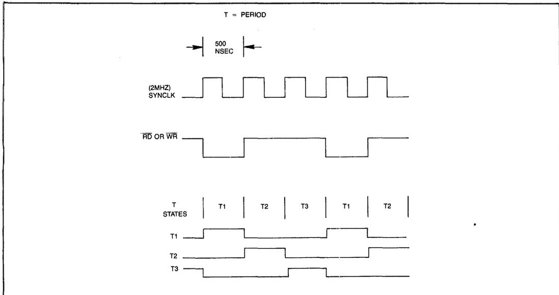
Figure 1 SYNCLK, RD, AND WR TIMING RELATIONSHIPS.
