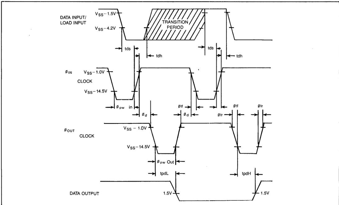
Figure 3 WD5869 TIMING DIAGRAM
