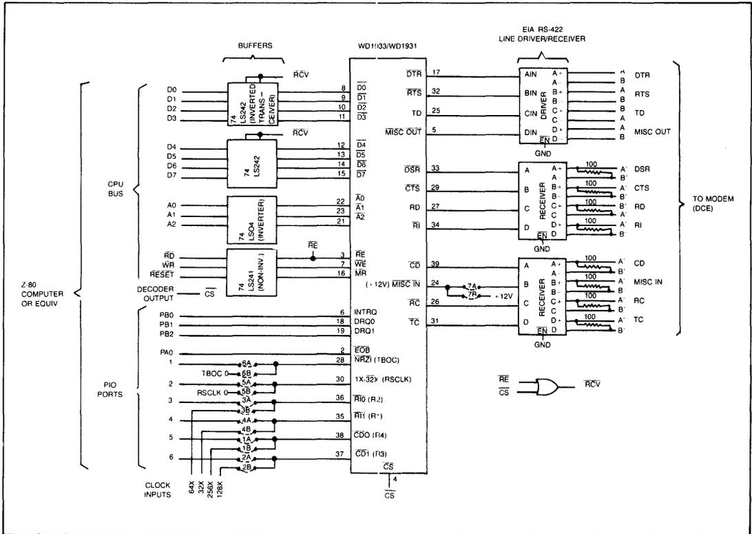
Figure 2. WD1931/1933 AND MICROCOMPUTER. (MULTIPROTOCOL BOARD)
