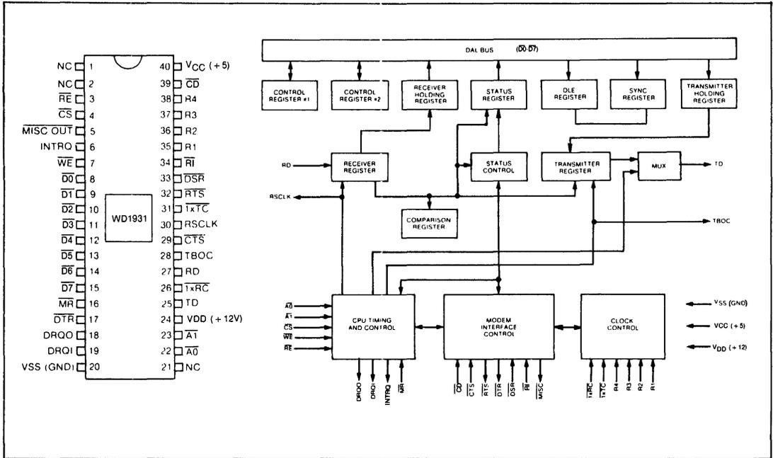
Figure 10. WD1931 PIN CONNECTIONS AND BLOCK DIAGRAM
