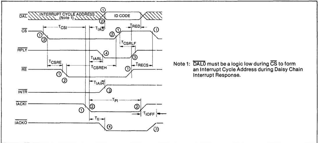
Note 1:  $\overline{DAL0}$  must be a logic low during  $\overline{CS}$  to form an Interrupt Cycle Address during Daisy Chain Interrupt Response.
