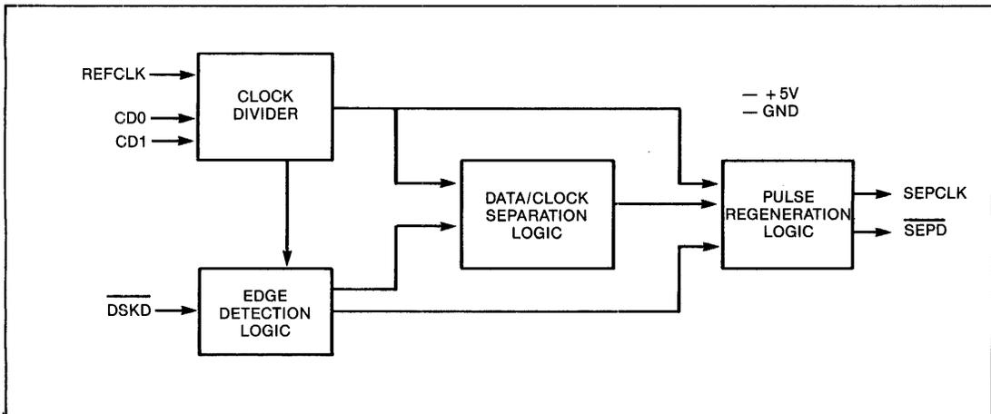
FLOPPY DISK DATA SEPARATOR BLOCK DIAGRAM
