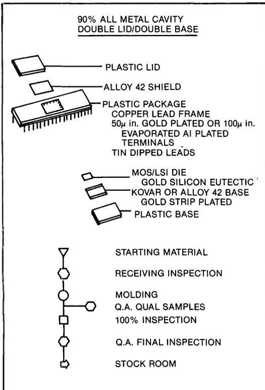
lead frame material we have achieved a true chemical mechanical bond during the molding process. This bond is so strong, we are able to place a device prior to lid seal upside down on a helium leak detector and pass a  $1 \times 10^{-9}$  std cc/sec open face leak test.
