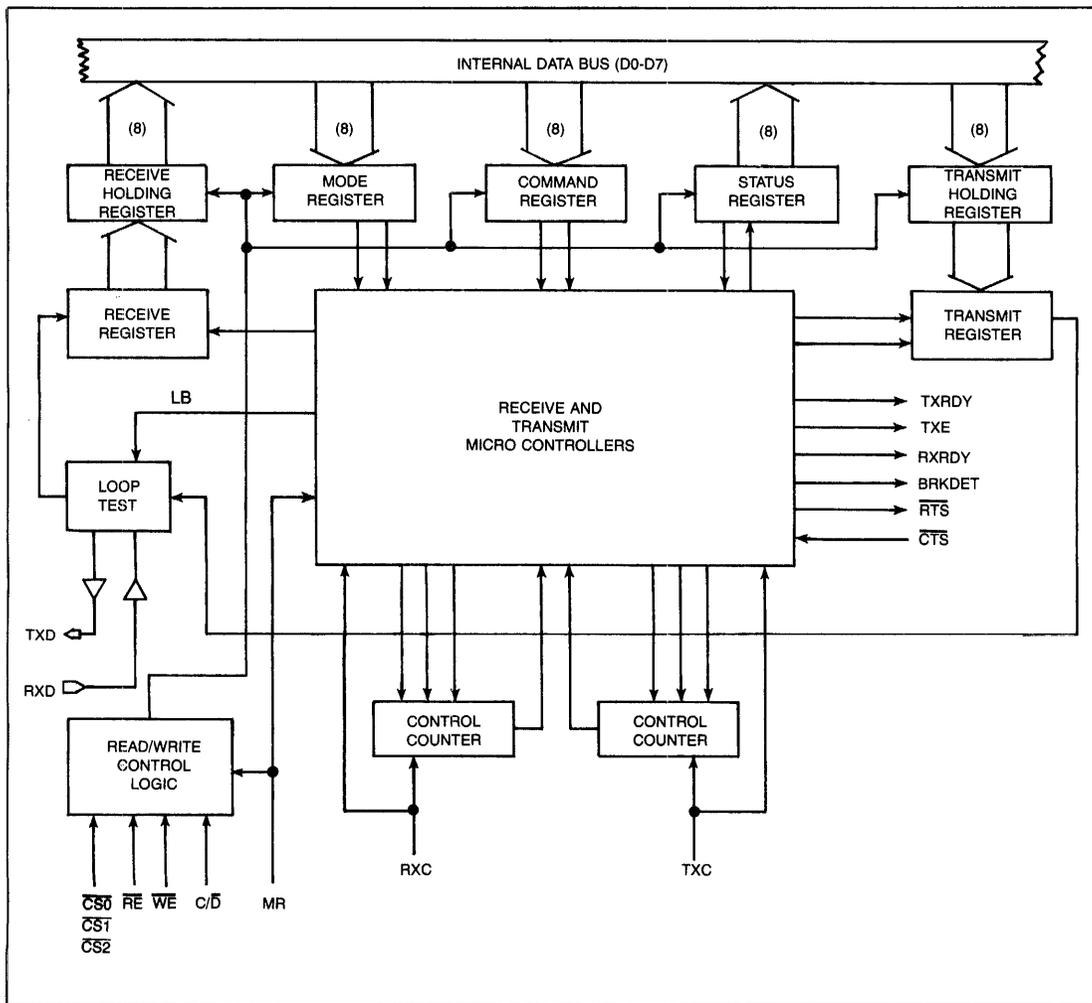
Figure 3. RECEIVE/TRANSMIT COMMUNICATIONS CONTROLLER DIAGRAM
