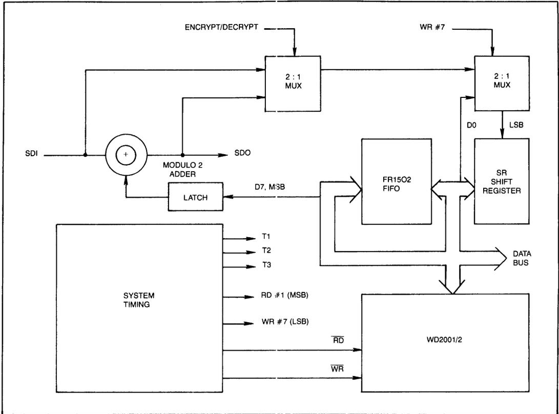
Figure 14 OBCFB SYSTEM BLOCK DIAGRAM
