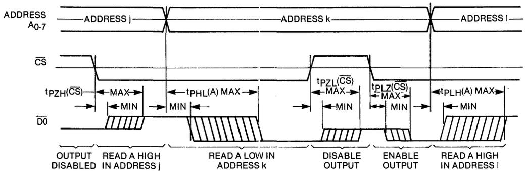
Switching delays from address and chip select inputs to the data output. Disabled output is floating when "OFF," and represented by a single center line.
