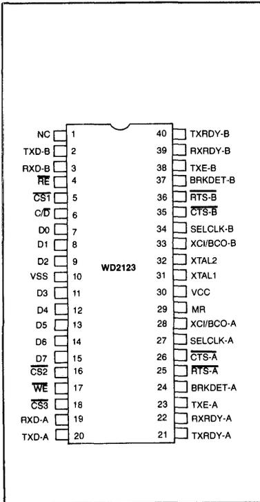
Figure 1. WD2123 PINOUT DIAGRAM
