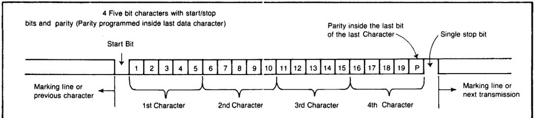
**Figure 13 20 BIT ASYNCHRONOUS**
