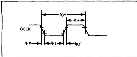
**Input and Output Waveforms for A.C. Tests**
