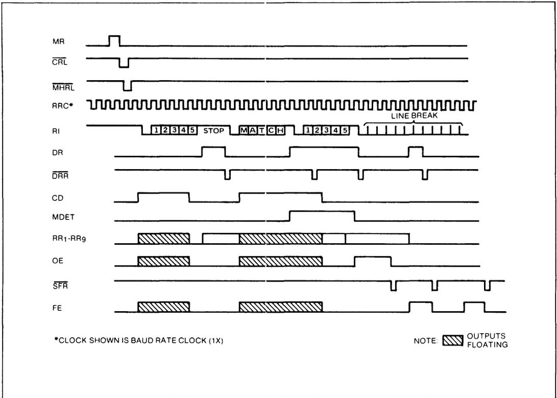
ASYNCHRONOUS & ISOCHRONOUS TIMING EXAMPLE
