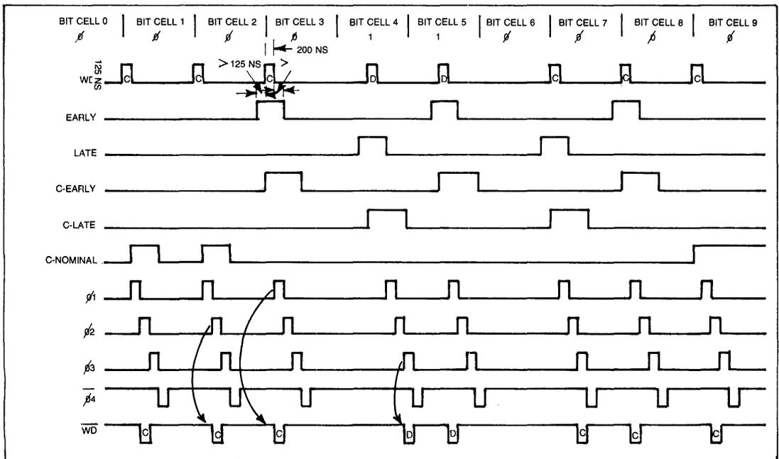
FIGURE 8. PRECOMP TIMING FOR CIRCUIT IN FIGURE 6
