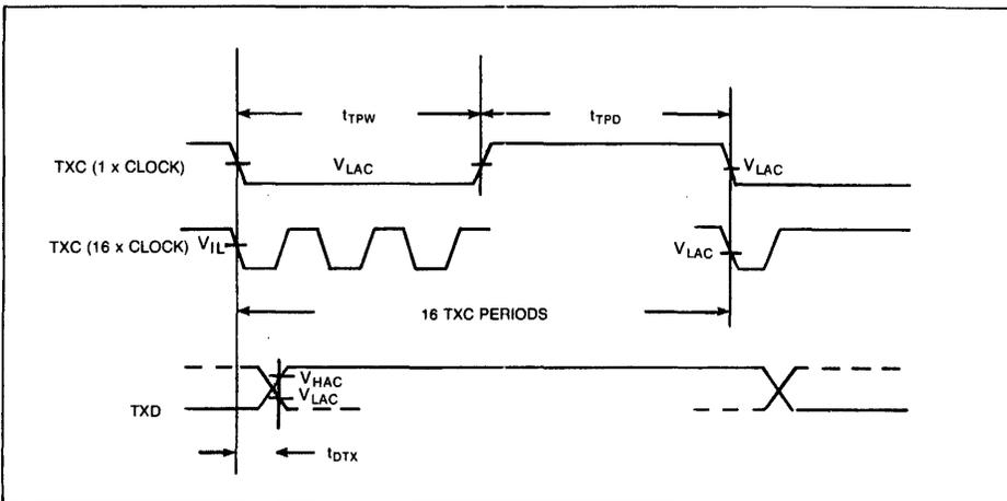
Figure 10 WD2123 TRANSMITTER CLOCK AND DATA TIMING
