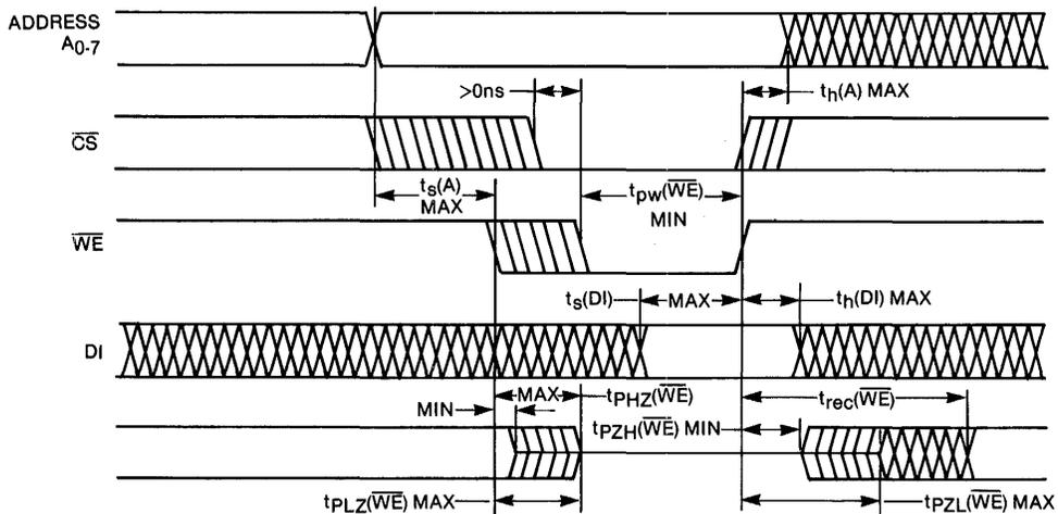
Write Cycle Timing. The cycle is initiated by an address change. After  $t_S(A)$  max, the write enable may begin. The chip select must also be LOW for writing. Following the write pulse,  $t_H(A)$  max must be allowed before the address may be changed again. The output will be floating while the write enable is LOW. Ordinarily, the chip select should be LOW during the entire write pulse.
