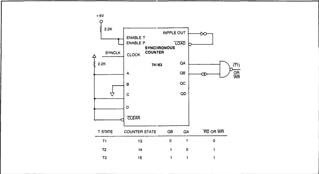
**Figure 2 RD AND WR TIMING GENERATION**
