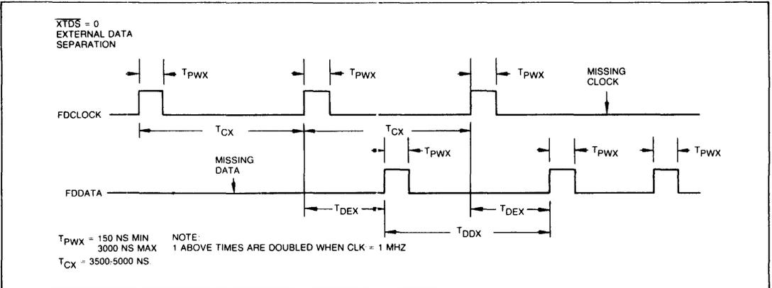
FIGURE 3. EXTERNAL DATA SEPERATOR TIMING.
