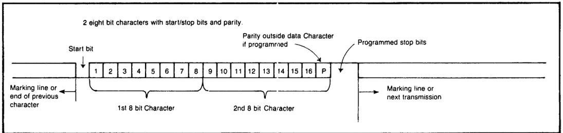
**Figure 12 16 BIT ASYNCHRONOUS**
