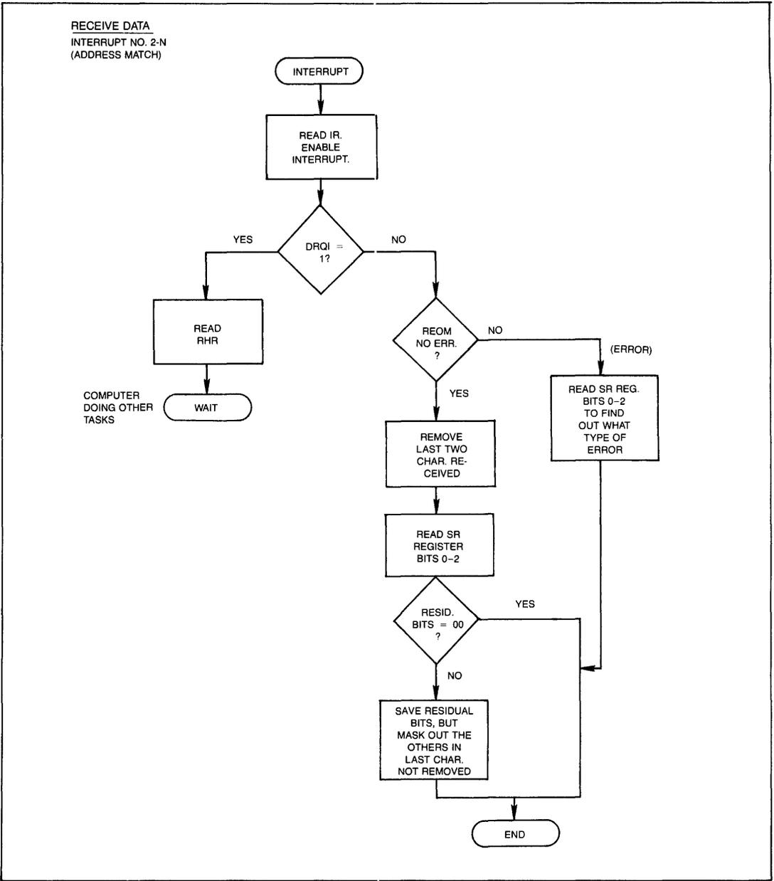
Figure 21. FLOW DIAGRAM OF FRAME RECEPTION
