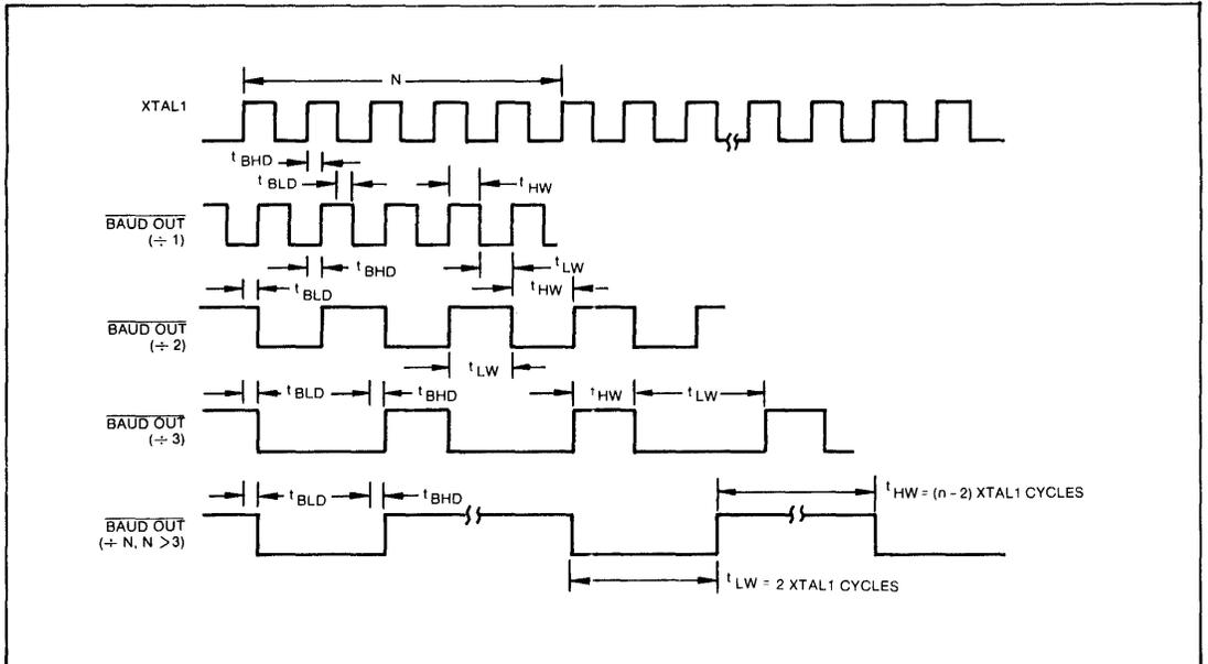
FIGURE 7. BAUDOUT TIMING
