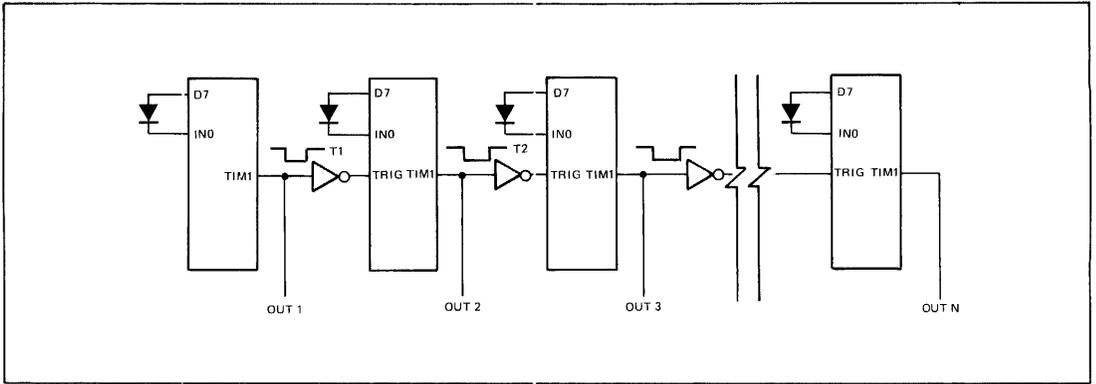
**FIGURE 8. DAISY-CHAIN N-SEQUENTIAL INTERVAL CONTROLLER**
