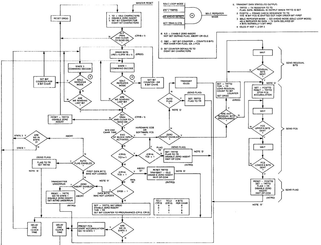
Figure 13. WD193X TRANSMITTER FLOW CHART
