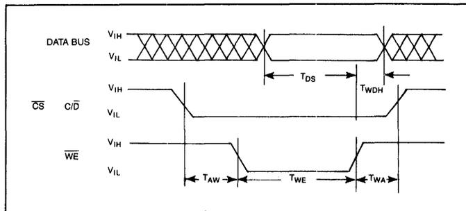
FIGURE 5 WRITE TIMING
