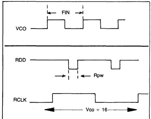
Figure 6 RDD AND RCLK PULSE DIAGRAMS
