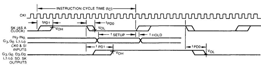
**Figure 14A INPUT/OUTPUT TIMING DIAGRAM (CRYSTAL + 16 MODE)**
