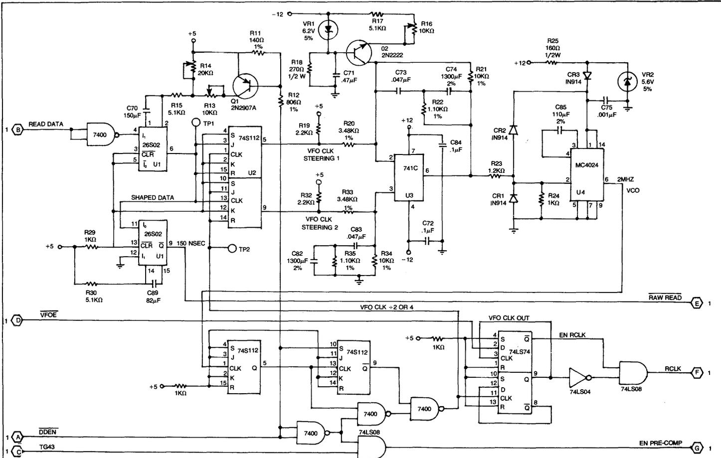
**FIGURE 13. PLL DATA RECOVERY CIRCUIT**
