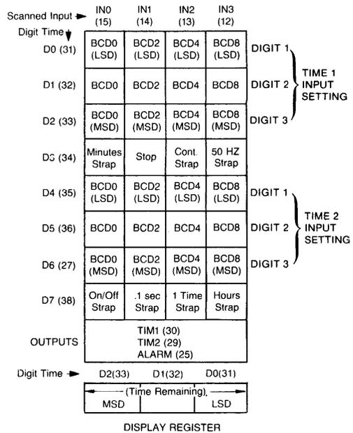
**FIGURE 2. CONFIGURATION TABLE ON/OFF TIMER MODE**
