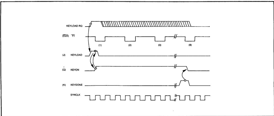
Figure 9 SINGLE KEYLOAD SEQUENCE
