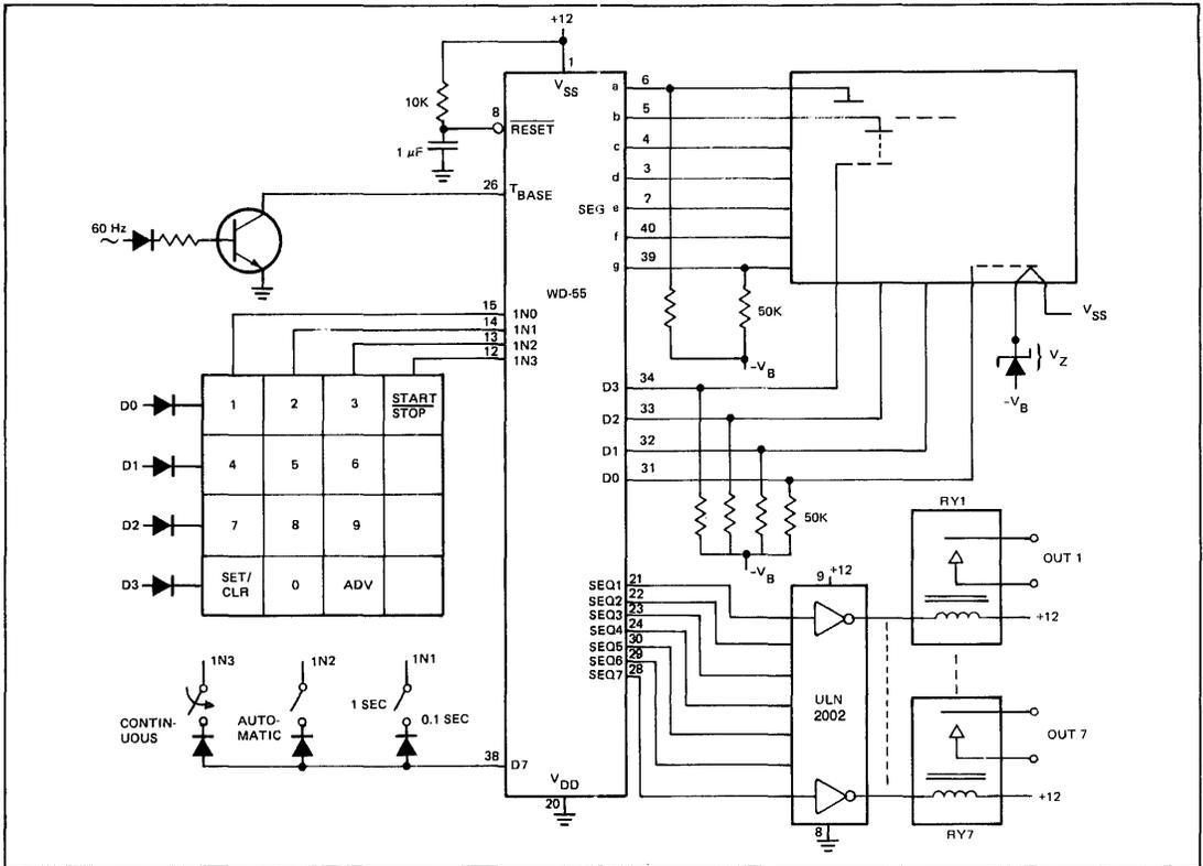
FIGURE 4. SEQUENCER WITH V-F DISPLAY
