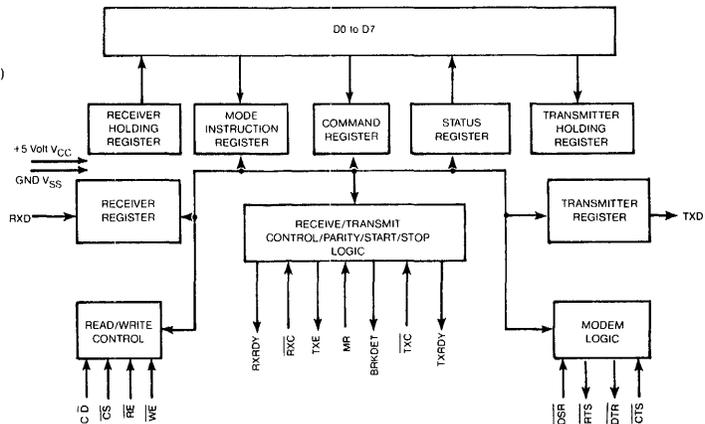
FIGURE 2 WD1983 BLOCK DIAGRAM
