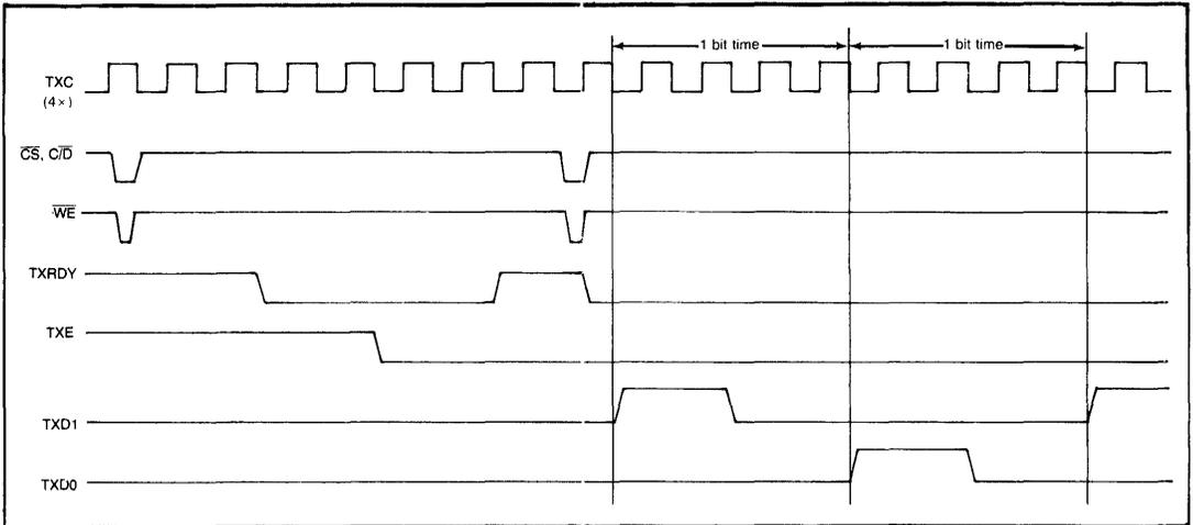
Figure 8 TRANSMITTER TIMINGS (ARINC MODE)
