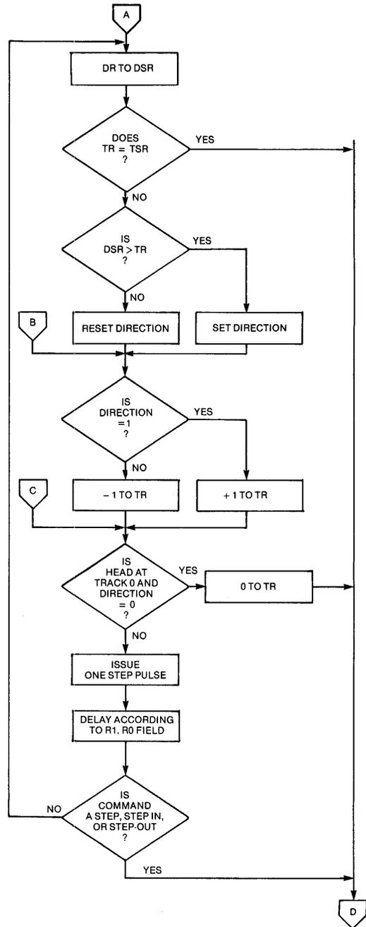
**Figure 5. TYPE I COMMAND FLOW**
