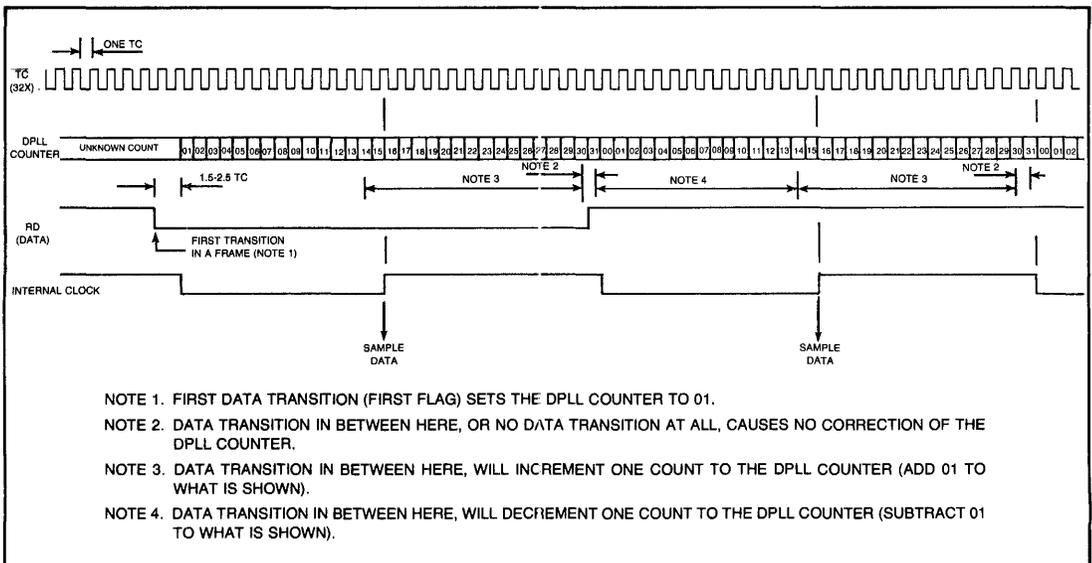
Figure 6. WD193X DPLL TIMING DIAGRAM
