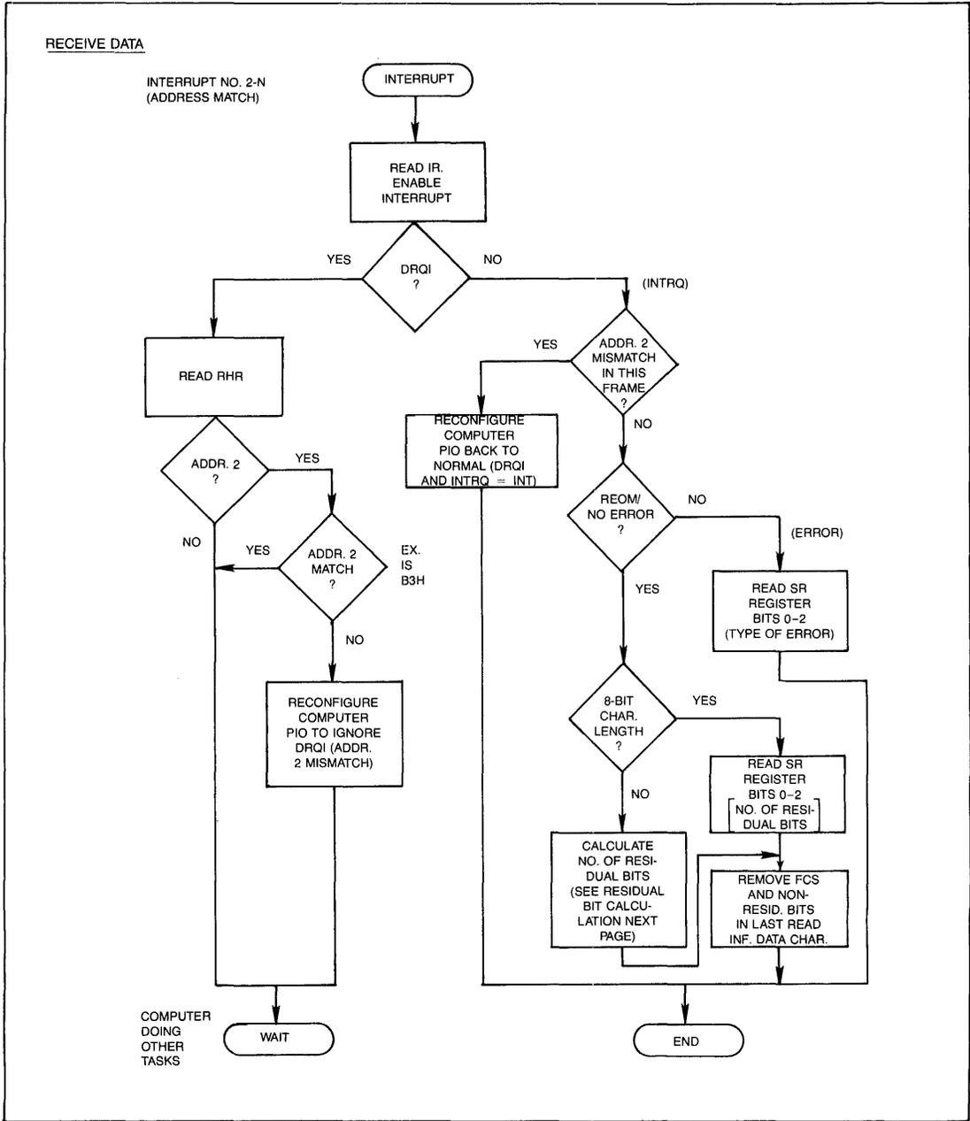
Figure 23. FLOW DIAGRAM OF FRAME RECEPTION
