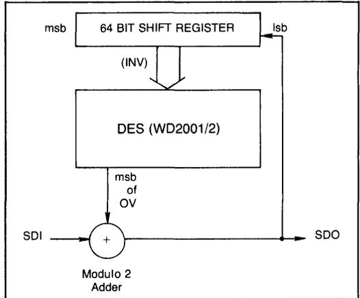
**Figure 11 OBCFB ENCRYPTION BLOCK DIAGRAM**
