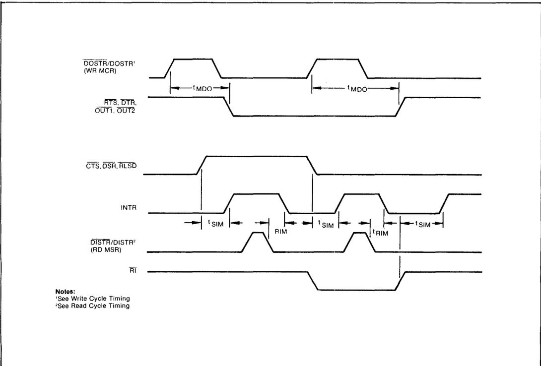
FIGURE 10. MODEM CONTROLS TIMING
