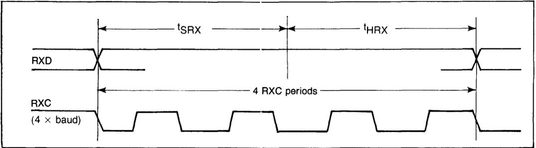
Figure 7 RECEIVER CLOCK AND DATA TIMINGS
