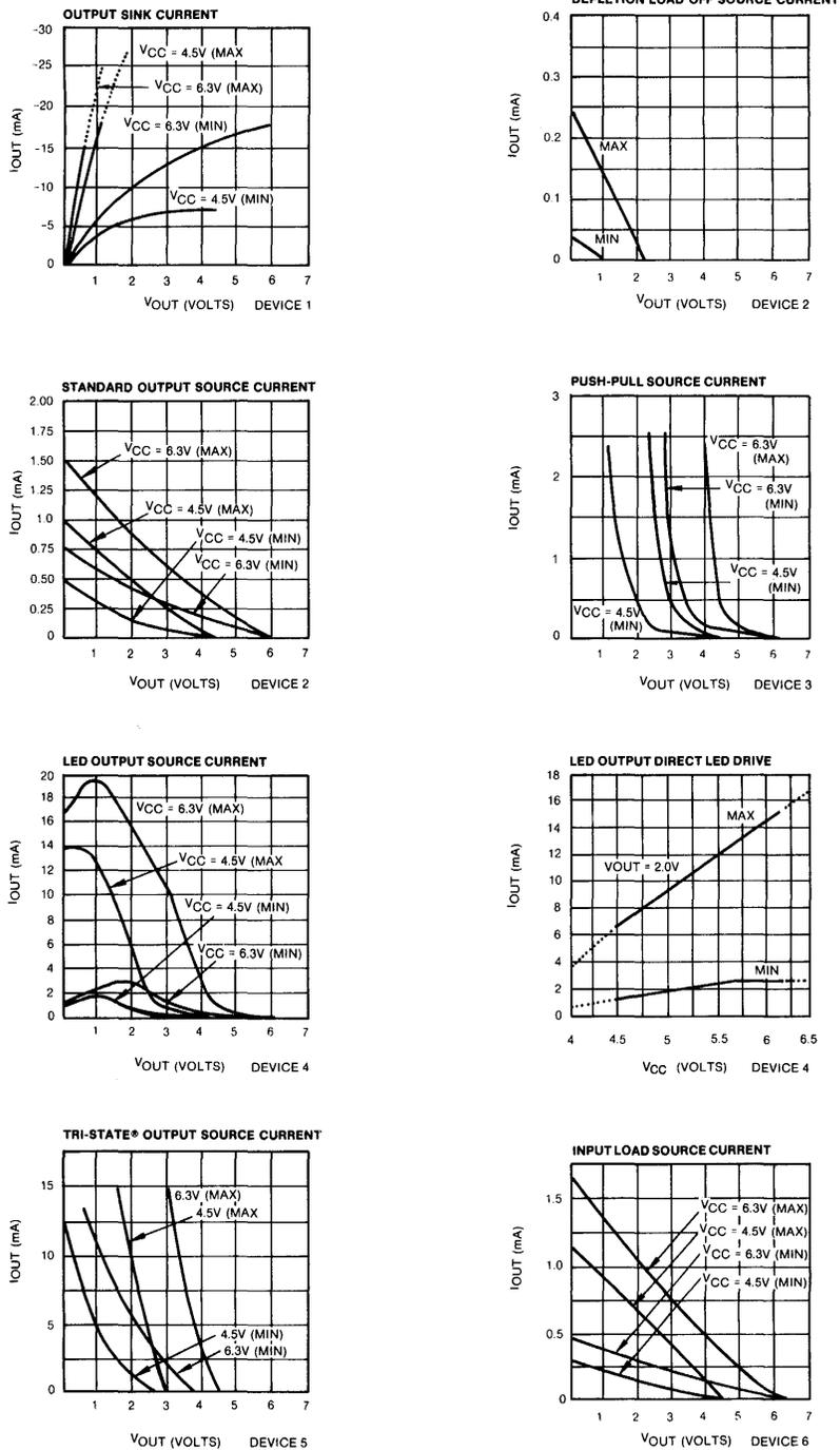
Figure 7 WD4200/4210 OUTPUT CHARACTERISTICS
