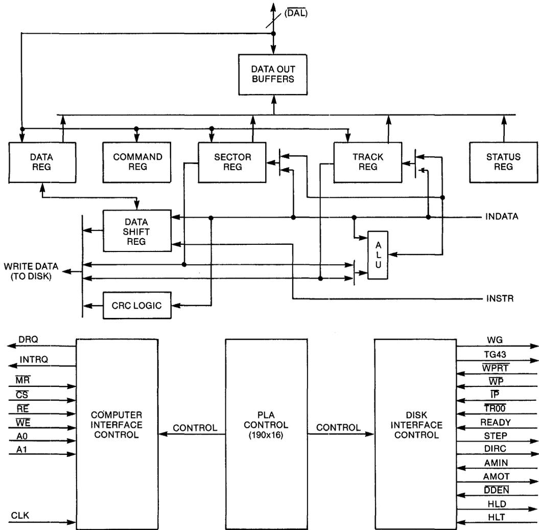
Figure 3. FD1781 BLOCK DIAGRAM
