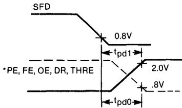
\*OUTPUTS PE, FE, OE, DR, THRE ARE DISCONNECTED AT TRANSITION OF SFD FROM 0.8V TO 2.0V.
