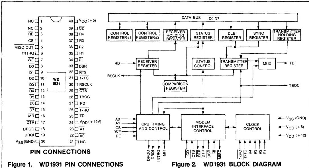
Figure 1. WD1931 PIN CONNECTIONS
