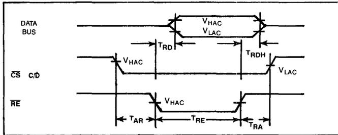
Figure 5 READ CYCLE TIMING
