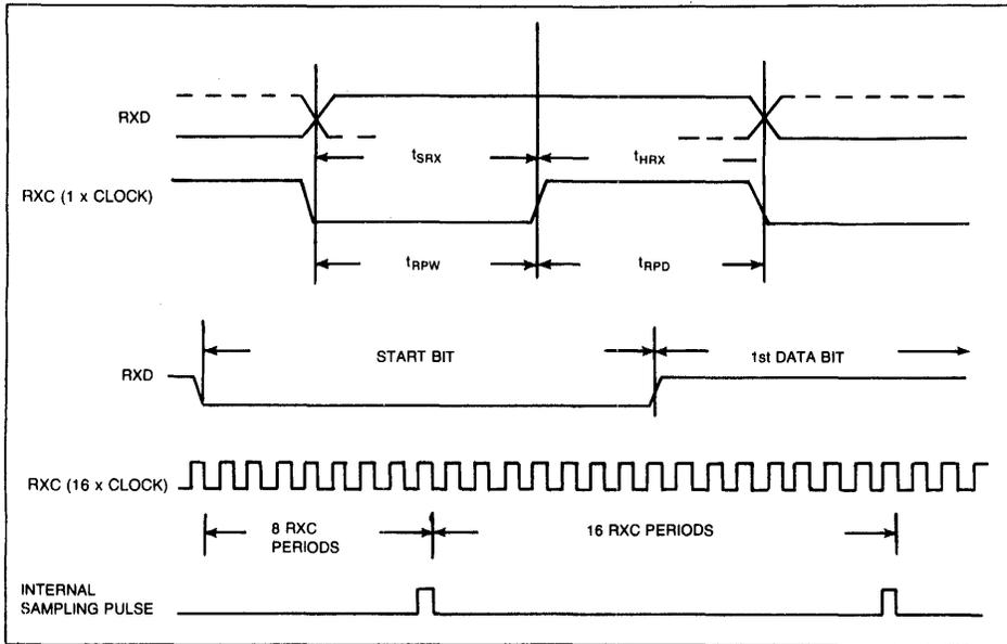
Figure 11 WD2123 RECEIVER CLOCK AND DATA TIMINGS
