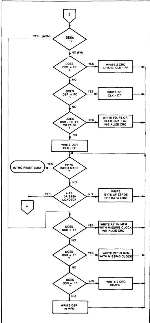
Although the CRC characters are transferred to the computer, the FD176X checks for validity and the CRC error status bit is set if there is a CRC error. The Track Address of the ID field is written into the sector register so that a comparison can be made by the user. At the end of the operation an interrupt is generated and the Busy Status is reset.
