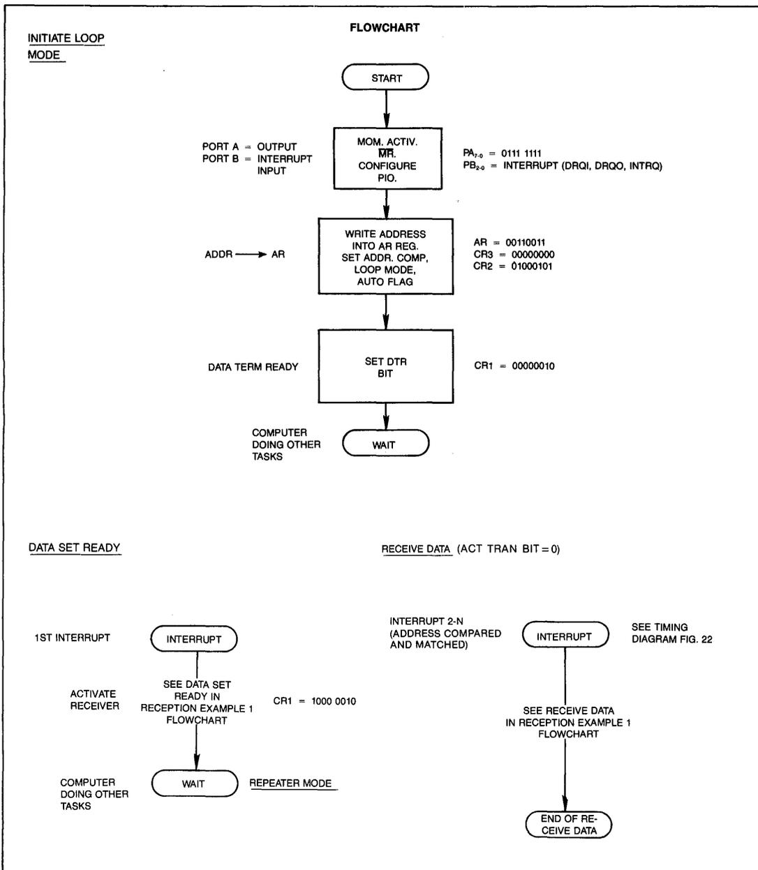
Figure 25. FLOW DIAGRAM OF SDLC LOOP MODE OPERATION
