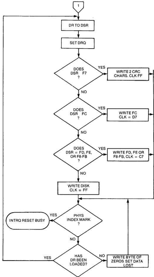
**Figure 12. TYPE III COMMAND WRITE TRACK**
