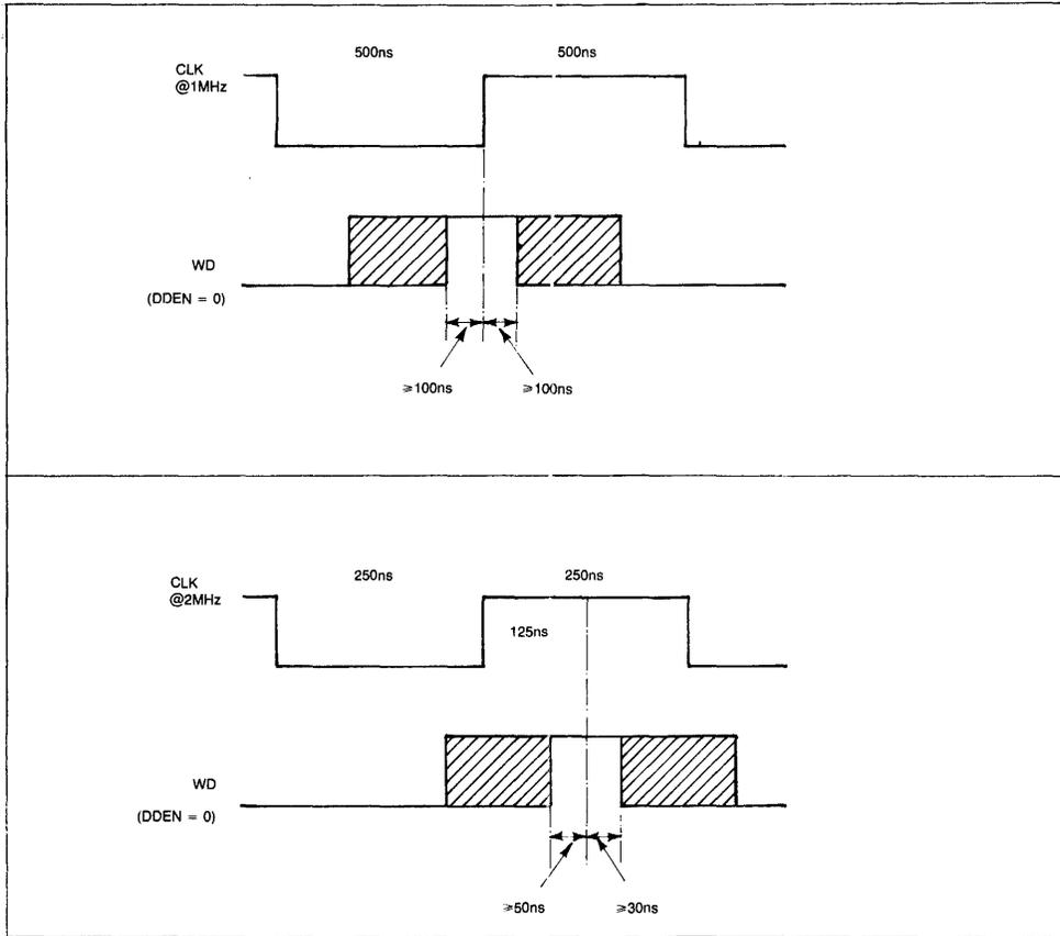
FIGURE 9. WD/CLK RELATIONSHIP FOR WRITE PRECOMP USE
