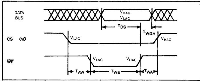
Figure 6 WRITE CYCLE TIMING
