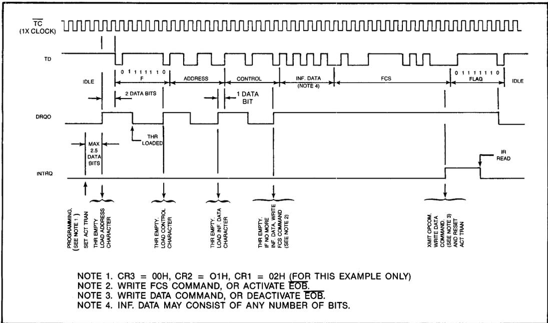
Figure 8. WD193X TRANSMISSION TIMING DIAGRAM
