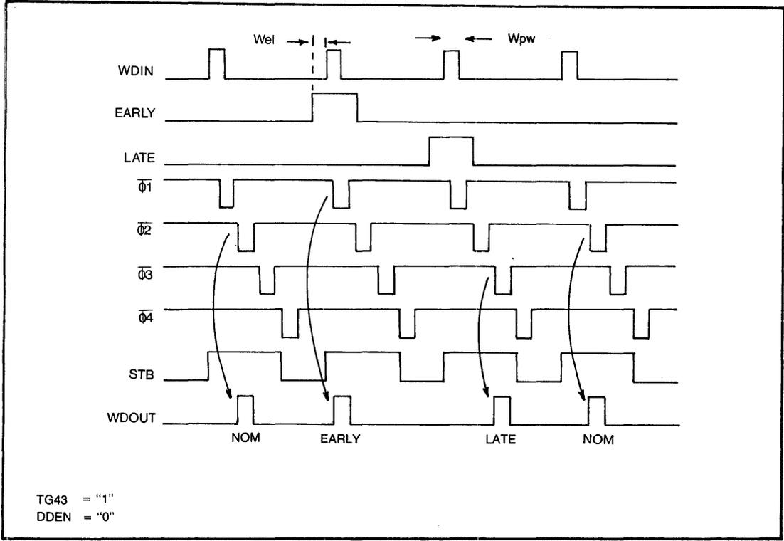
Figure 7 WRITE DATA TIMING (MFM)
