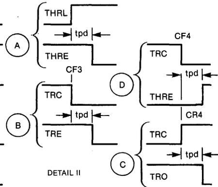
CASE I: IF THE POSITIVE TRANSITION OF THRL OCCURS >500ns PRIOR TO ANY CLOCK FALLING EDGE (CF3 IN SAMPLE) THE A, B, C, AND D SIGNALS WILL BE GENERATED AS SHOWN IN DETAIL II.
