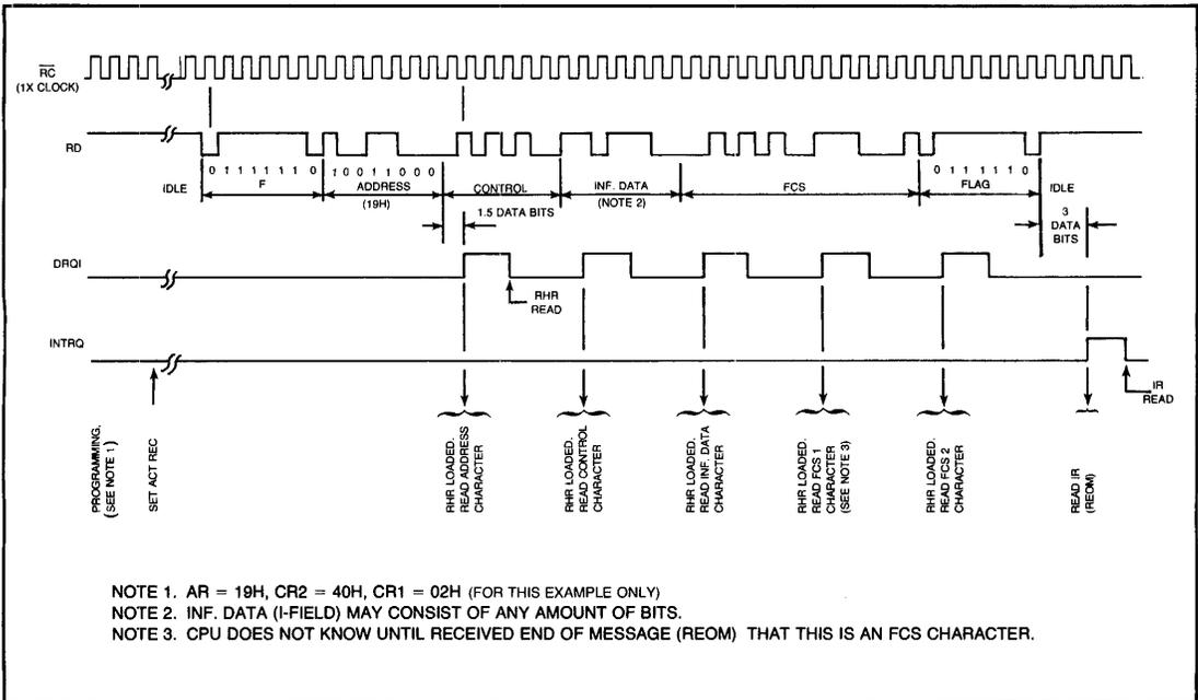
Figure 9. WD193X RECEPTION TIMING DIAGRAM
