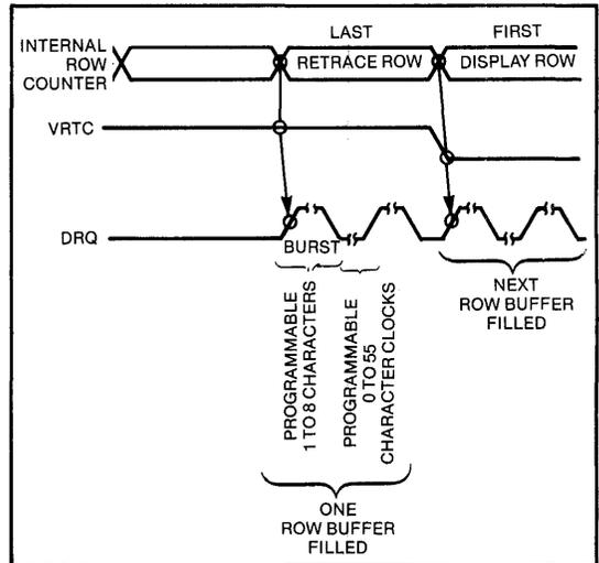
**Figure 20.** **DMA TIMING**
