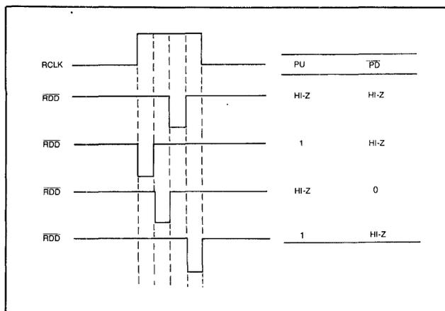
Figure 3 PUMP SIGNAL TIMING DIAGRAM
