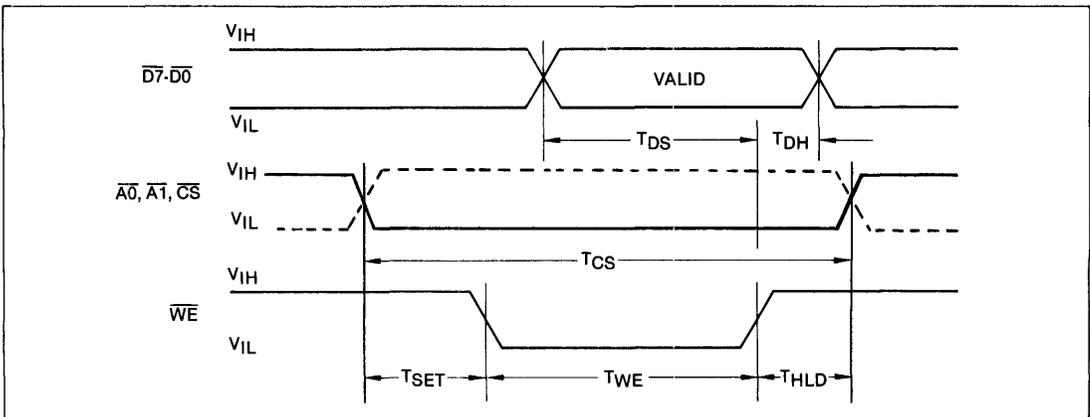
Figure 4. WRITE TIMING
