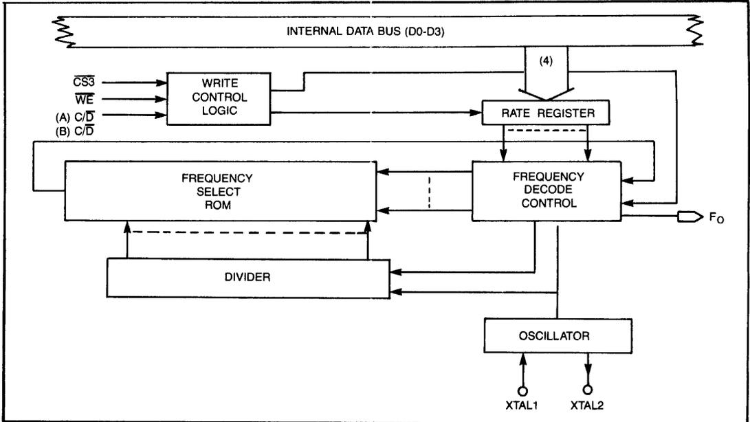
Figure 4 WD2123 BAUD RATE GENERATOR DIAGRAM
