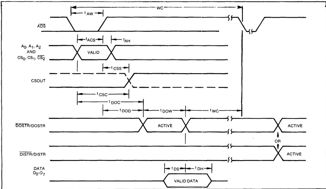
FIGURE 6. WRITE CYCLE TIMING
