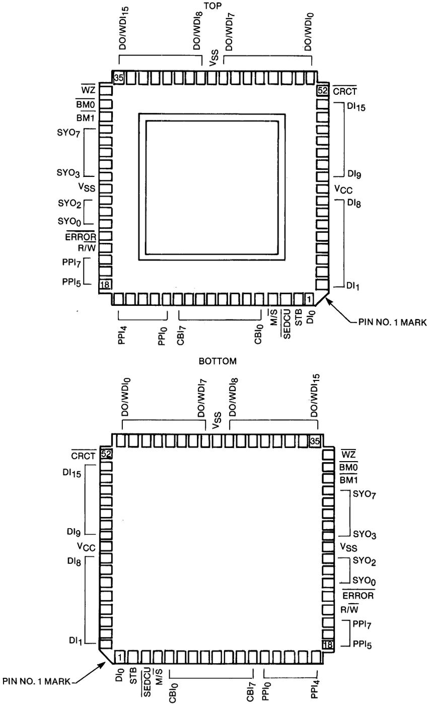
Figure 7. 8206 PINOUT DIAGRAM
