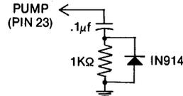
Since 5 1/4" Drives operate at exactly one-half the data rate (250 Kb/sec) the above capacitor should be doubled to .2 or .22  $\mu\text{f}$ .
