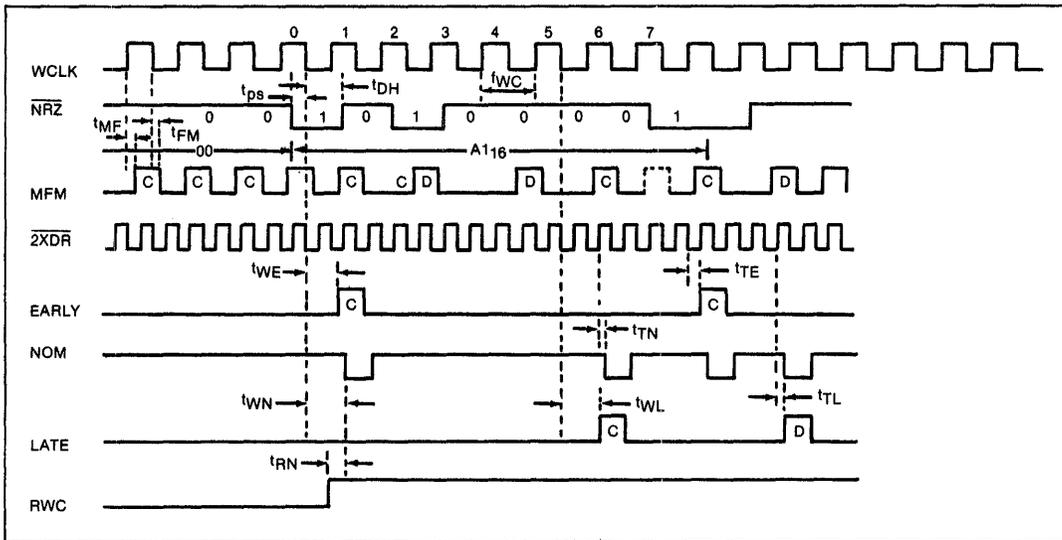
WD1100-12 Figure 4 MFM GENERATOR TIMING
