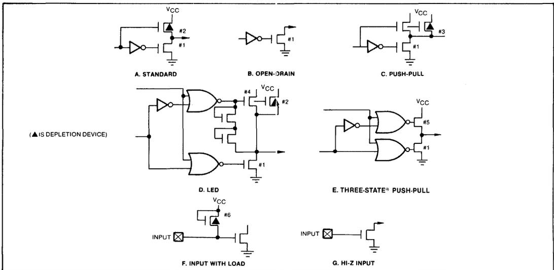
Figure 6 OUTPUT CONFIGURATIONS
