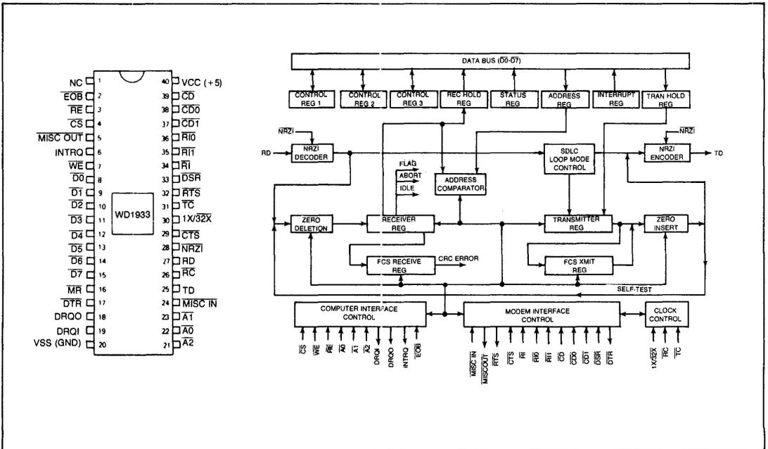
Figure 11. WD1933 PIN CONNECTIONS AND BLOCK DIAGRAM
