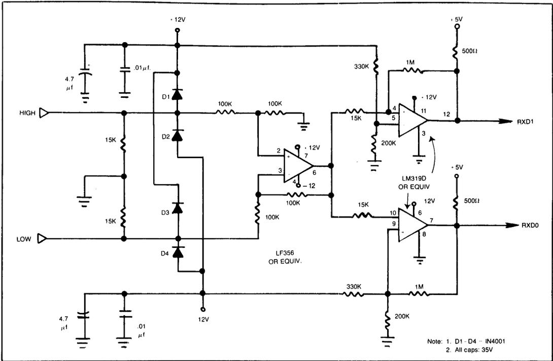
Figure 14 ARINC 429 LINE LEVEL TRANSLATOR (RECEIVER)
