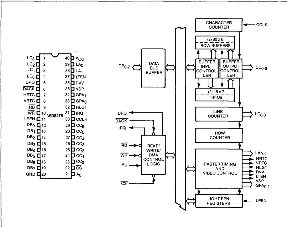
Figure 1. PIN CONFIGURATION
