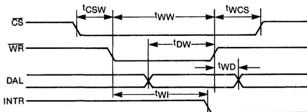
Figure 3 WRITE OPERATION TIMING
