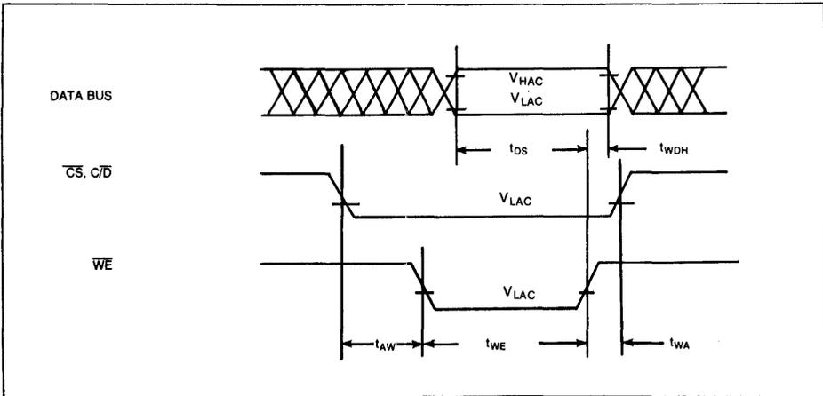
Figure 8 WD2123 WRITE TIMING
