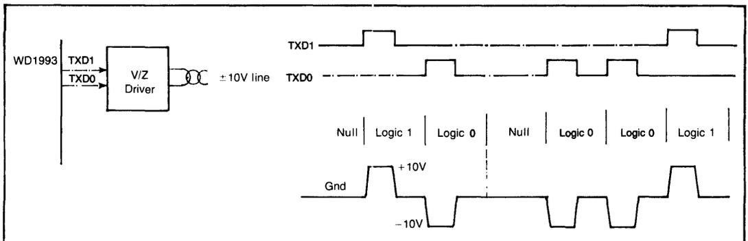
Figure 13 ARINC DRIVER CIRCUIT
