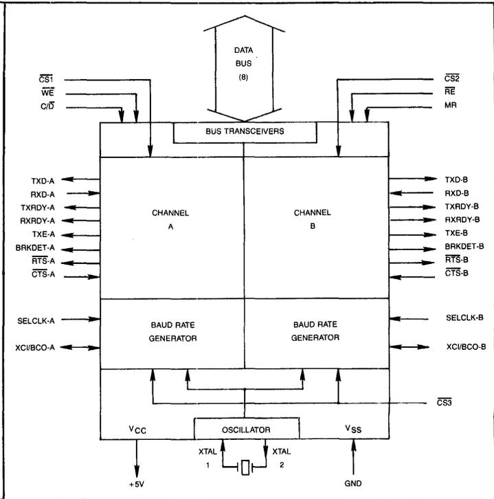
Figure 2. WD2123 BLOCK DIAGRAM
