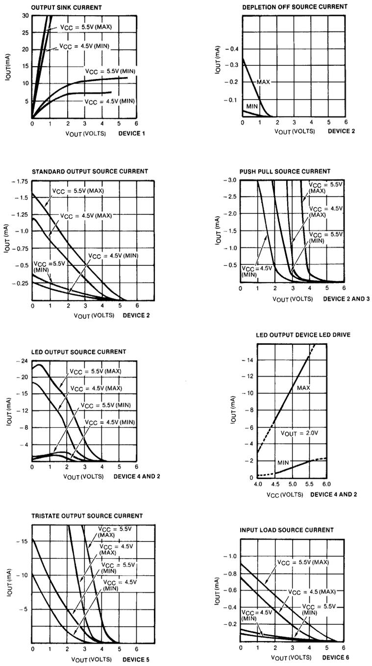
Figure 8 WD4320/4321 OUTPUT CHARACTERISTICS
