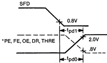
\*OUTPUTS PE, FE, OE, DR, THRE ARE DISCONNECTED AT TRANSITION OF SFD FROM 0.8V TO 2.0V.
