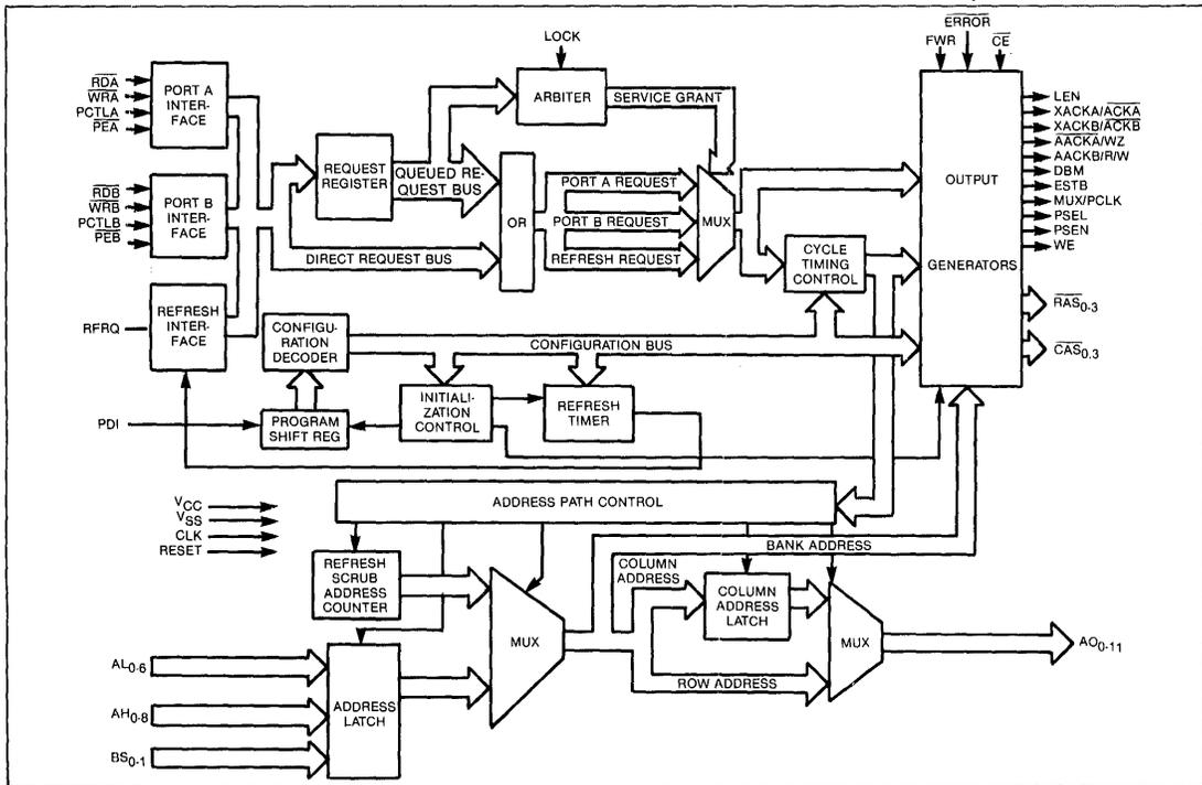
Figure 1. 8207 Block Diagram
