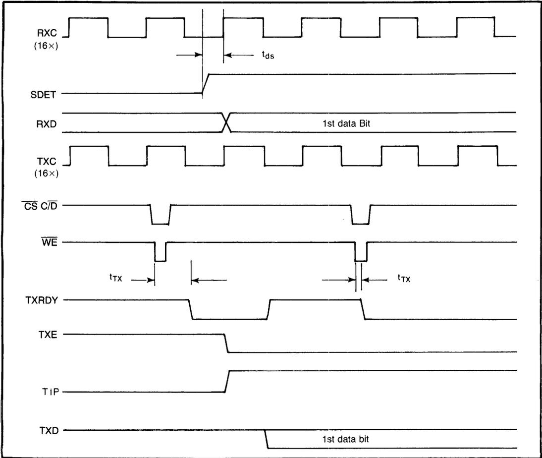
Figure 9 SYNCHRONOUS MODE TIMINGS
