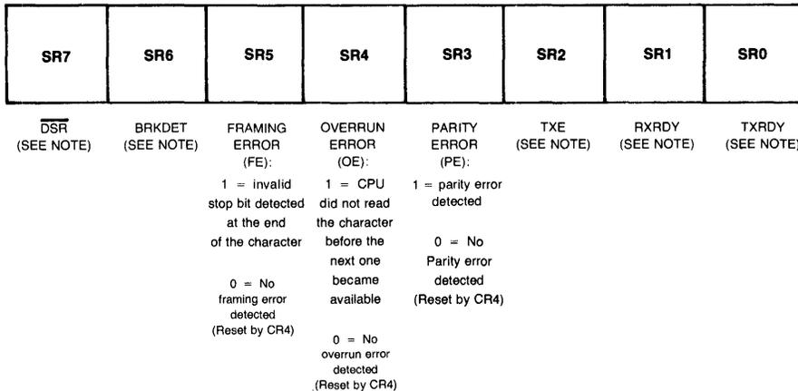
FE, OE & PE FLAGS DO NOT INHIBIT OPERATION.
