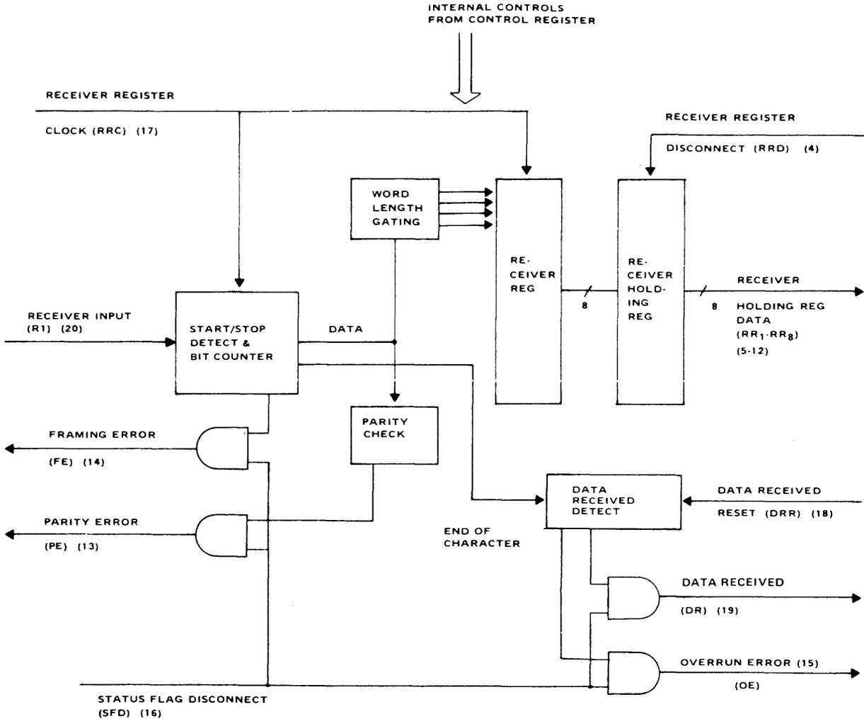
Figure 8. Receiver Block Diagram
