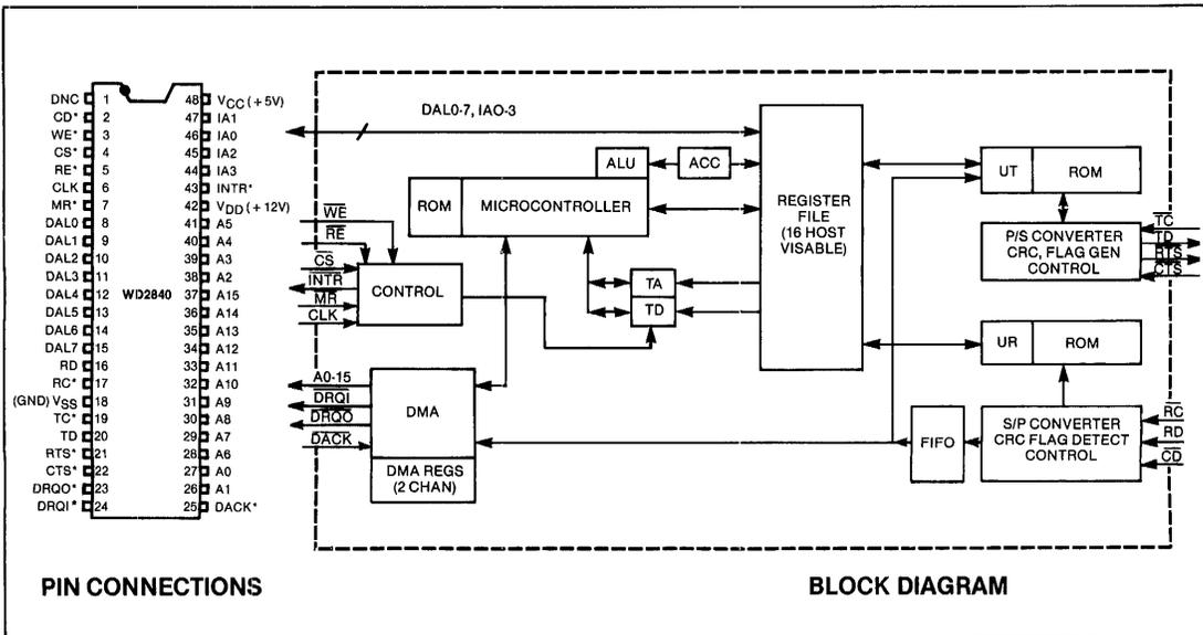
The WD2840 is packaged in a 48 pin DIP. The following is a functional description of each pin. An asterisk after a signal name (SIGNAL\*) means active Low.
