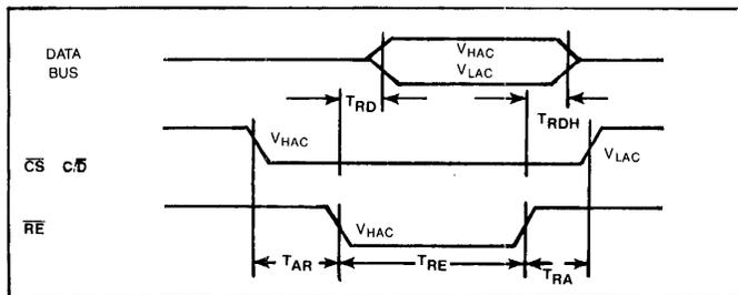
**Figure 5 READ CYCLE TIMING**
