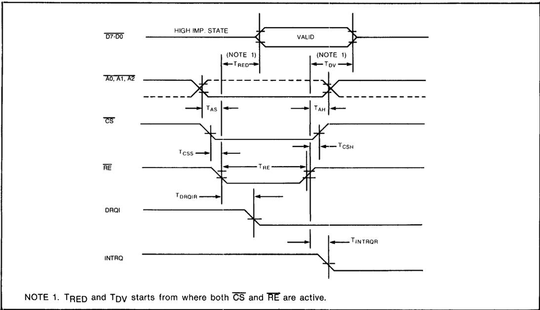
Figure 10. WD193X READ TIMING DIAGRAM
