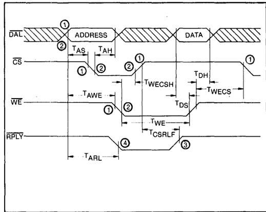
WRITE CYCLE TIMING DIAGRAM
