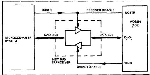
**FIGURE 2. TYPICAL INTERFACE FOR A HIGH-CAPACITY DATA BUS.**
