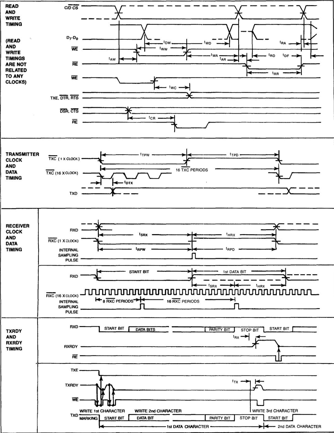
FIGURE 7 SYSTEM TIMING DIAGRAMS
