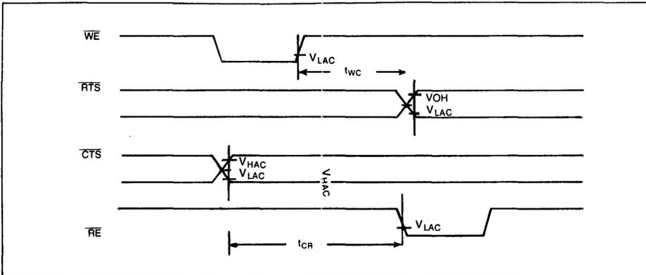
Figure 9 WD2123 INTERFACE CONTROL TIMING
