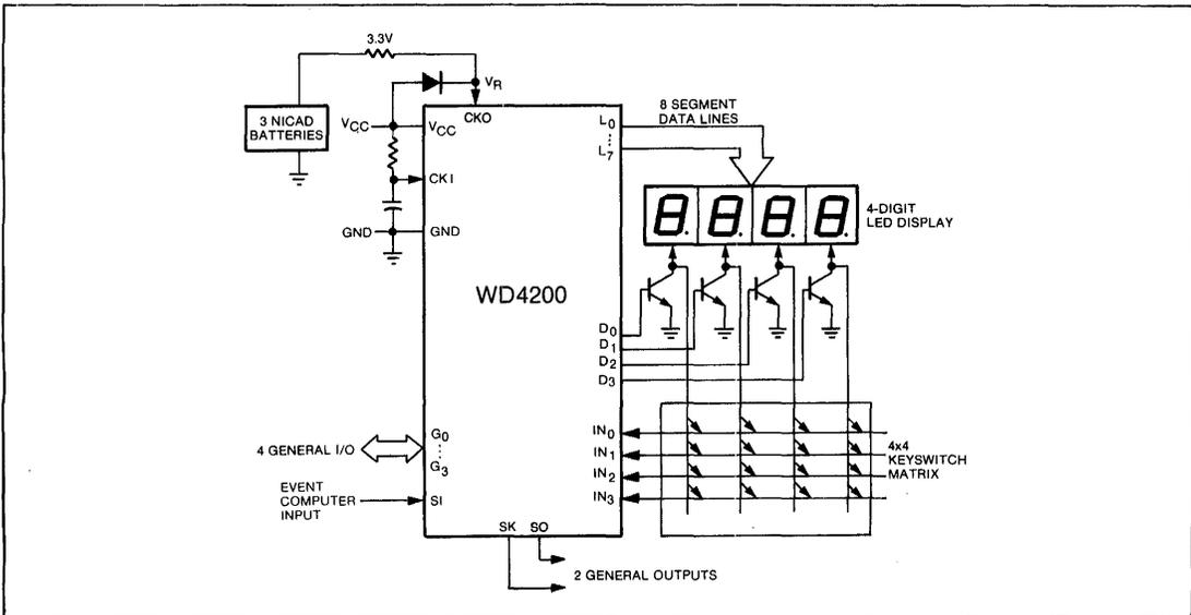
**Figure 10 WD4200 KEYBOARD/DISPLAY INTERFACE**
