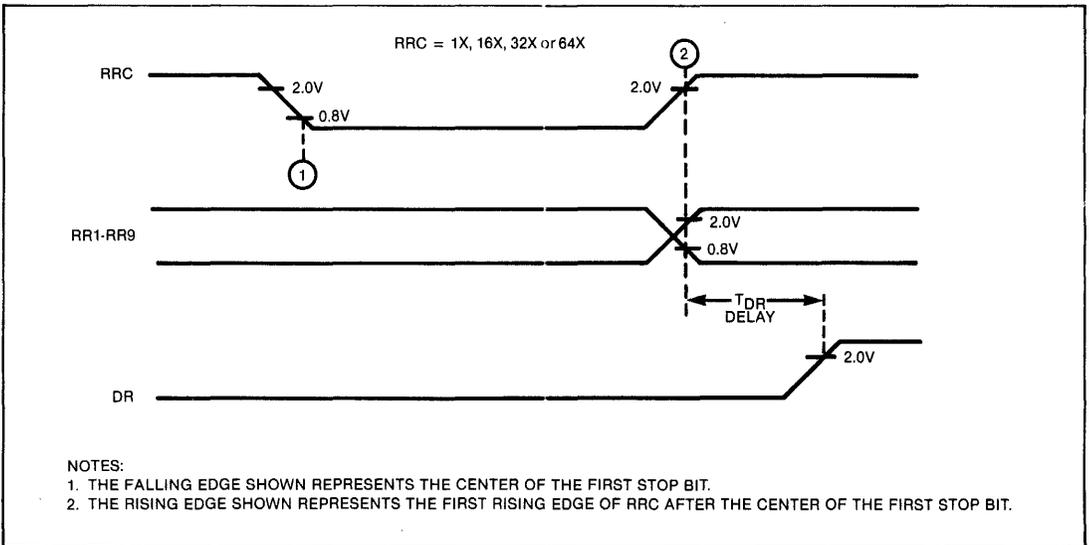
Figure 1 PR1472 TIMING DETAIL
