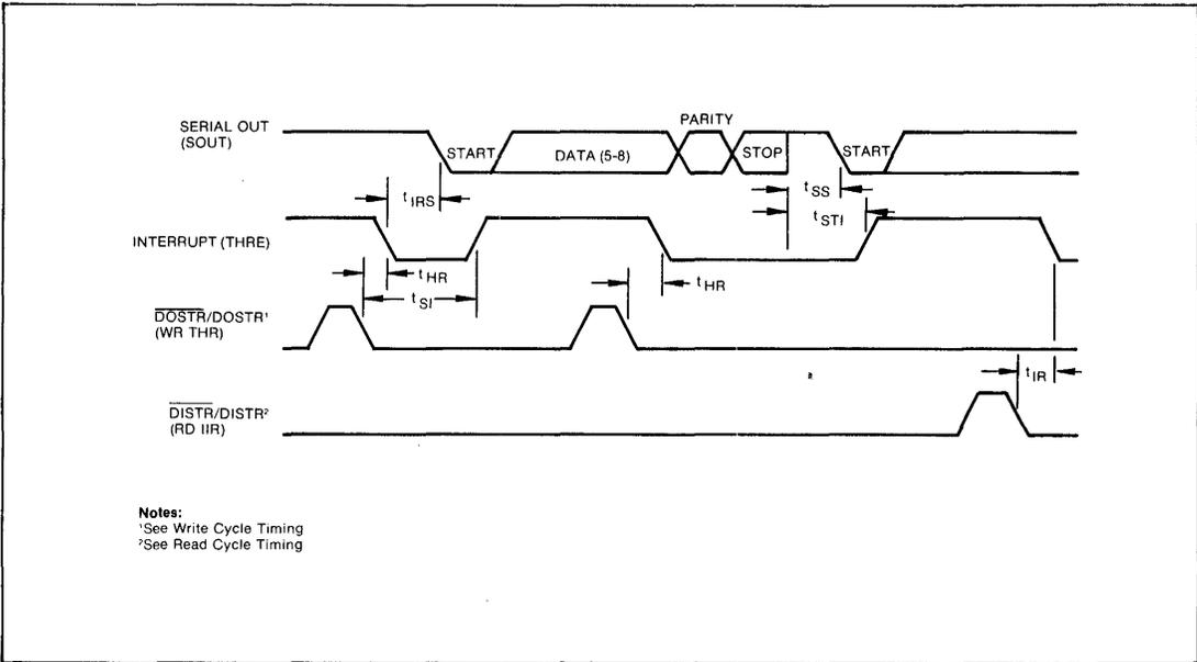
FIGURE 9. TRANSMITTER TIMING
