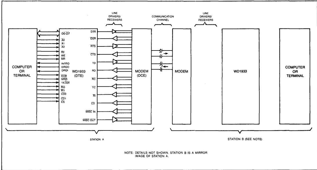
Figure 9. HDLC POINT TO POINT WITH MODEM
