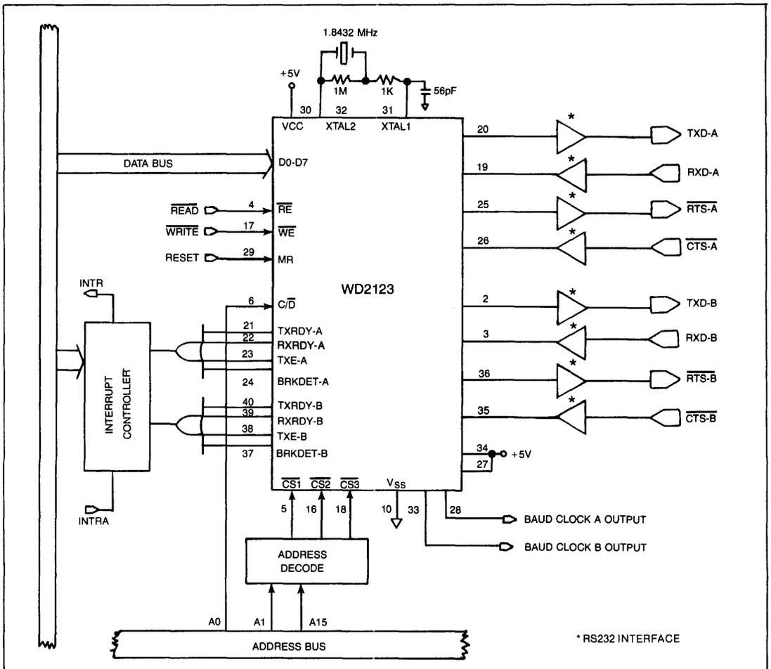
Figure 5 WD2123 MICROPROCESSOR APPLICATION
