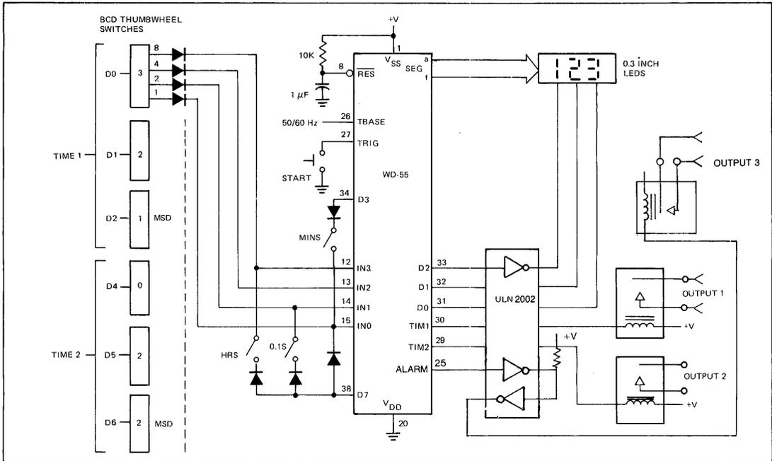
FIGURE 5. THUMBWHEEL PROGRAMMABLE INTERVAL TIMER
