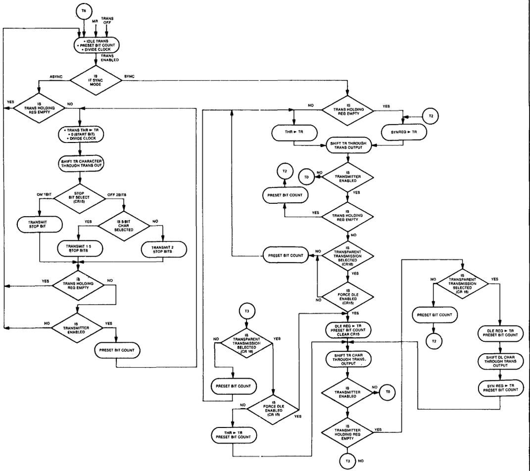
TRANSMITTER SECTION (ASYNCHRONOUS)
