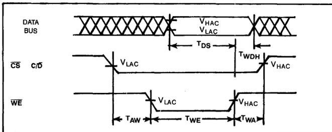
Figure 6 WRITE CYCLE TIMING
