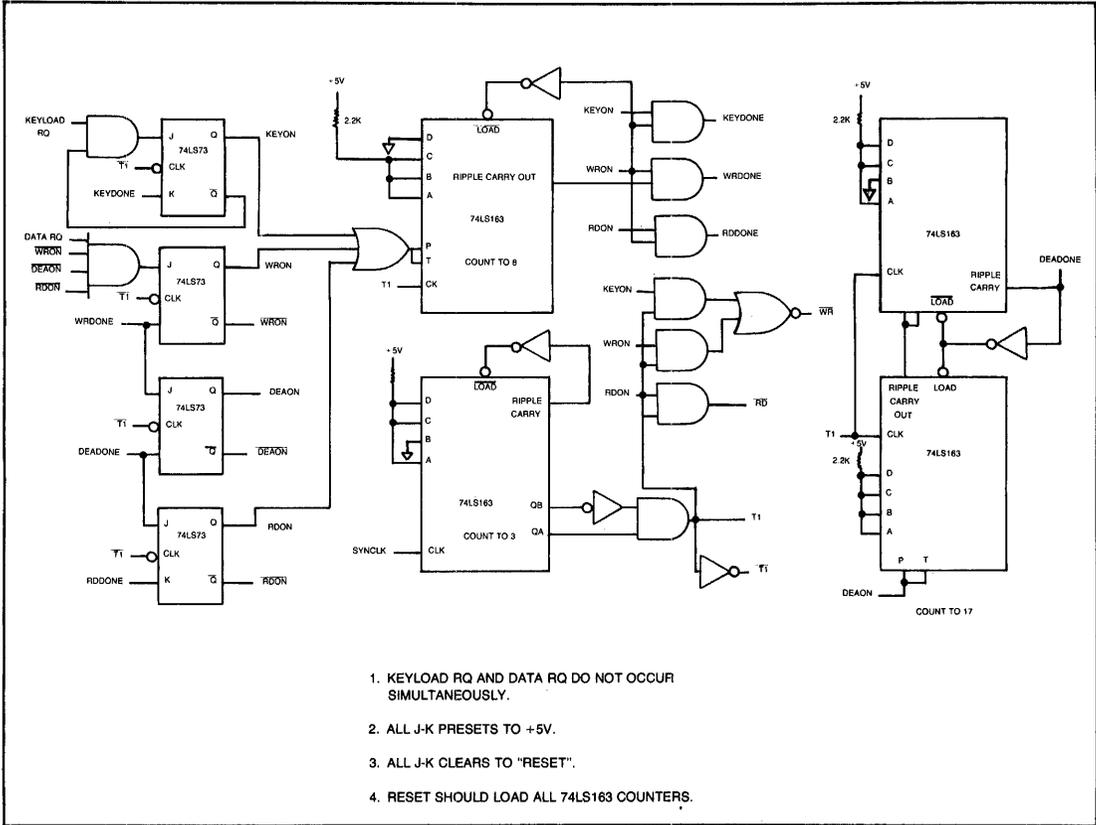
Figure 8 SYSTEM TIMING IMPLEMENTATION
