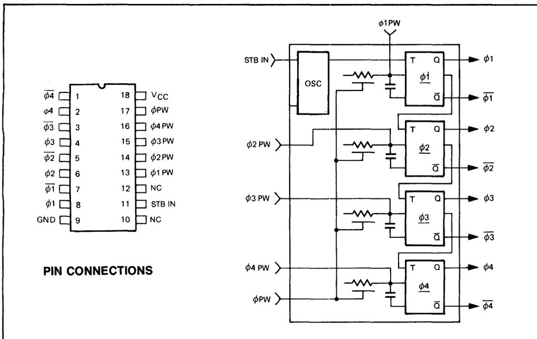
Figure 1 WD2143-03 PIN CONNECTIONS AND BLOCK DIAGRAM
