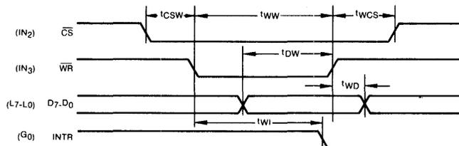
**Figure 13 MICROBUS™ WRITE OPERATION TIMING**
