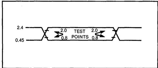
FOR A.C. TESTING, INPUTS ARE DRIVEN AT 2.4V FOR A LOGIC "1" AND 0.45V FOR A LOGIC "0." TIMING MEASUREMENTS FOR INPUT AND OUTPUT SIGNALS ARE MADE AT 2.0V FOR A LOGIC "1" AND 0.8V FOR A LOGIC "0."
