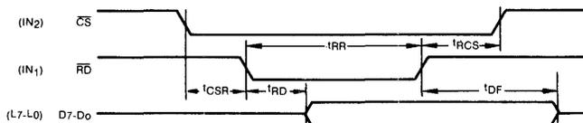
**Figure 12 MICROBUS™ READ OPERATION TIMING**
