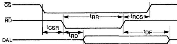
Figure 4 READ OPERATION TIMING
