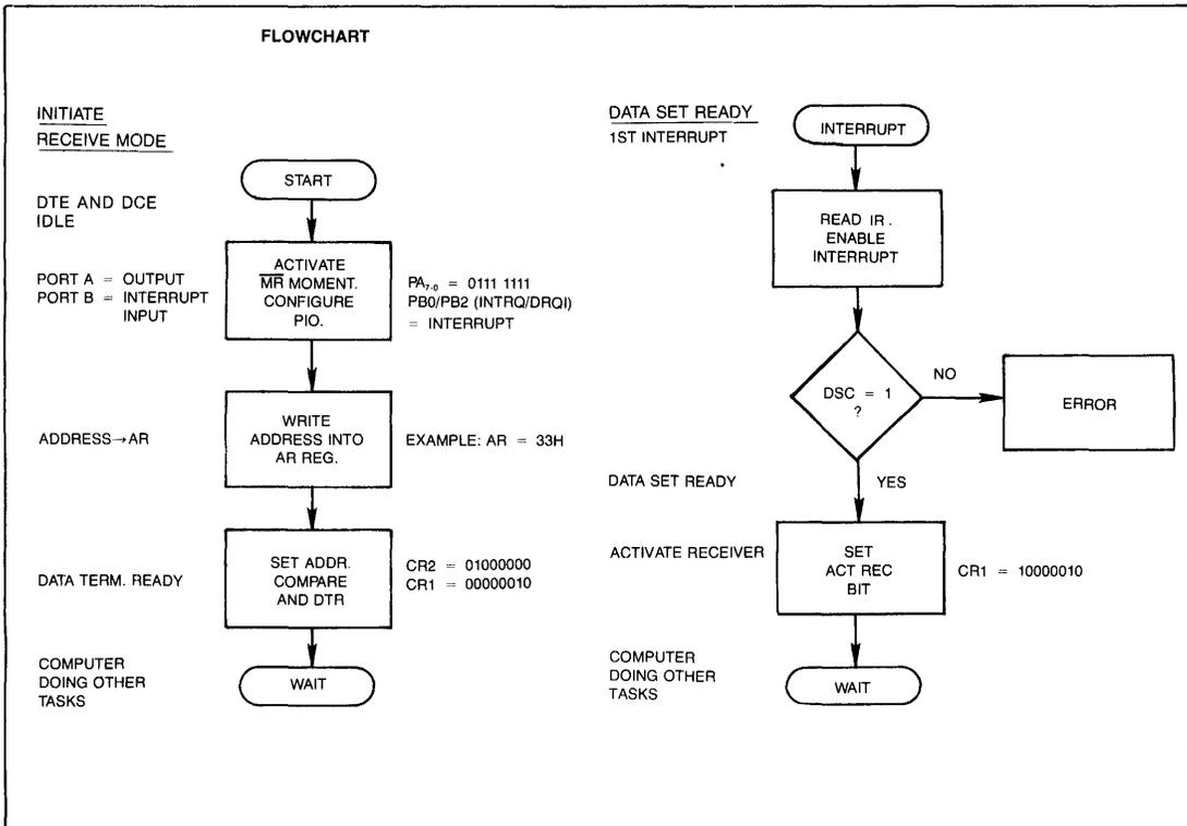
Figure 21. FLOW DIAGRAM OF FRAME RECEPTION (EXAMPLE NO. 1)
