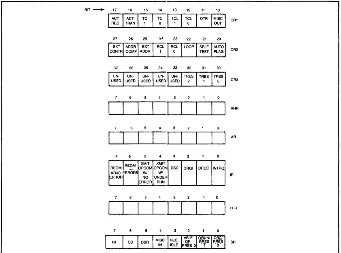
Figure 7. WD193X BIT ASSIGNMENTS
