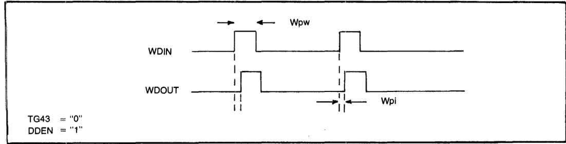
Figure 8 WRITE DATA TIMING (FM)
