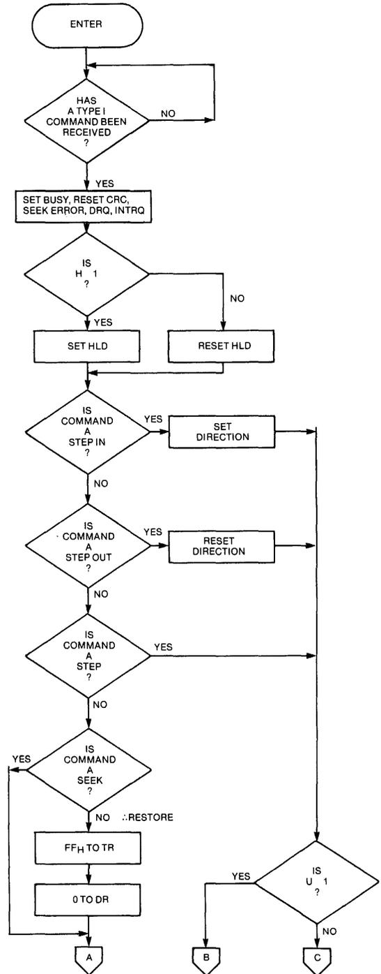
**Figure 4. TYPE I COMMAND FLOW**
