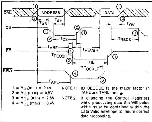
READ CYCLE TIMING DIAGRAM
