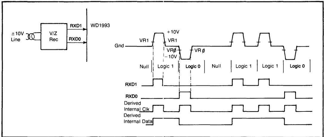
Figure 12 ARINC RECEIVER CIRCUIT
