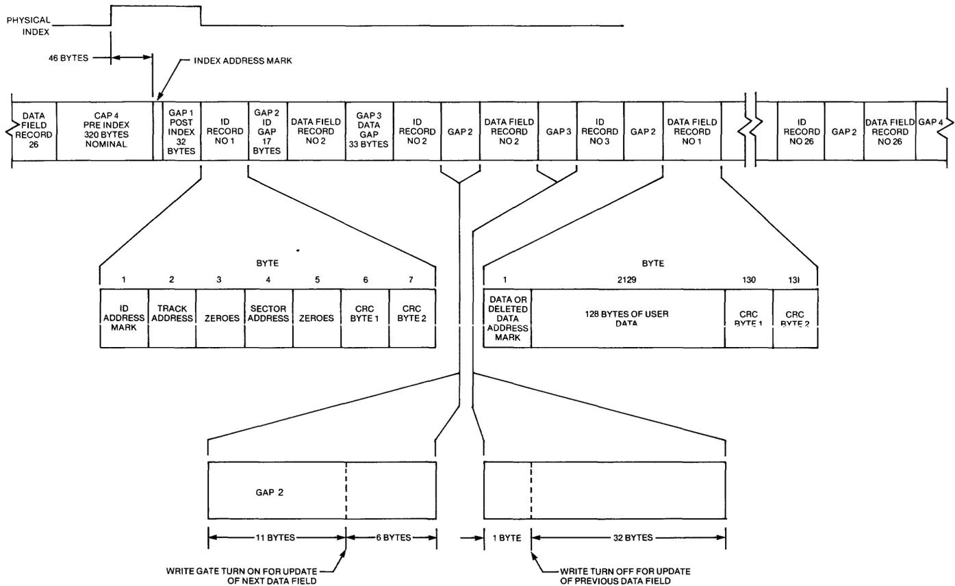
Figure 13. IBM 3740 TRACK FORMAT
