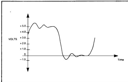
Figure 2 TYPICAL "RINGING" WAVEFORM
