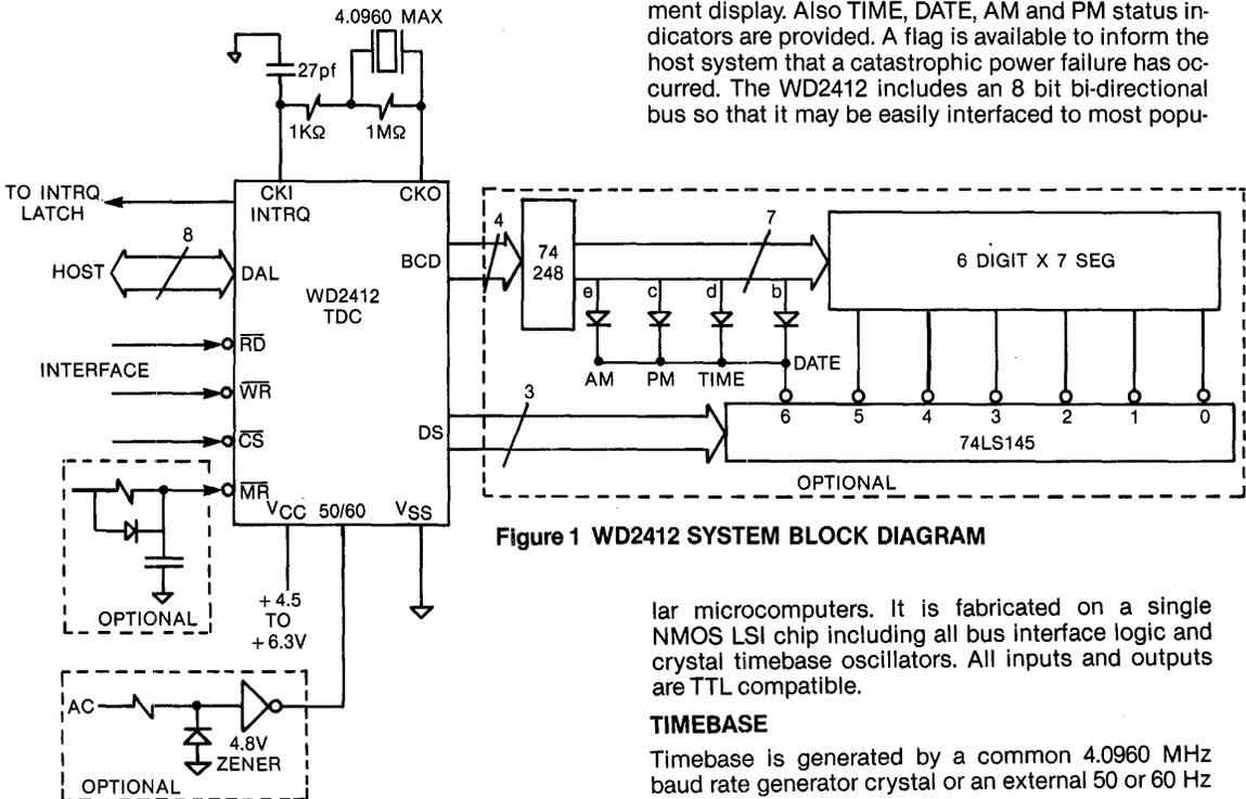
**Figure 1 WD2412 SYSTEM BLOCK DIAGRAM**
