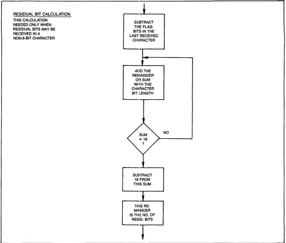
Figure 23. FLOW DIAGRAM OF FRAME RECEPTION
