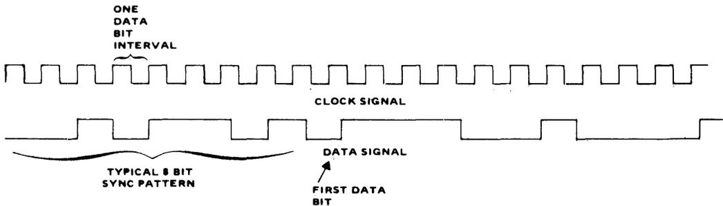
Figure 1. Synchronous Data
