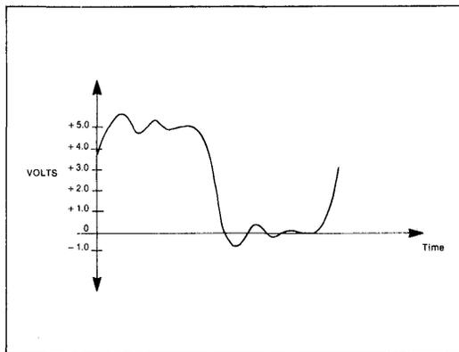
Figure 2. TYPICAL "RINGING" WAVEFORM from TTL INPUT
