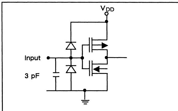
Figure 4. WTL 1232 Input Equivalent Circuit
