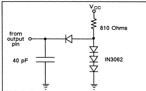
Figure 6. Test Load for Delay Measurement
