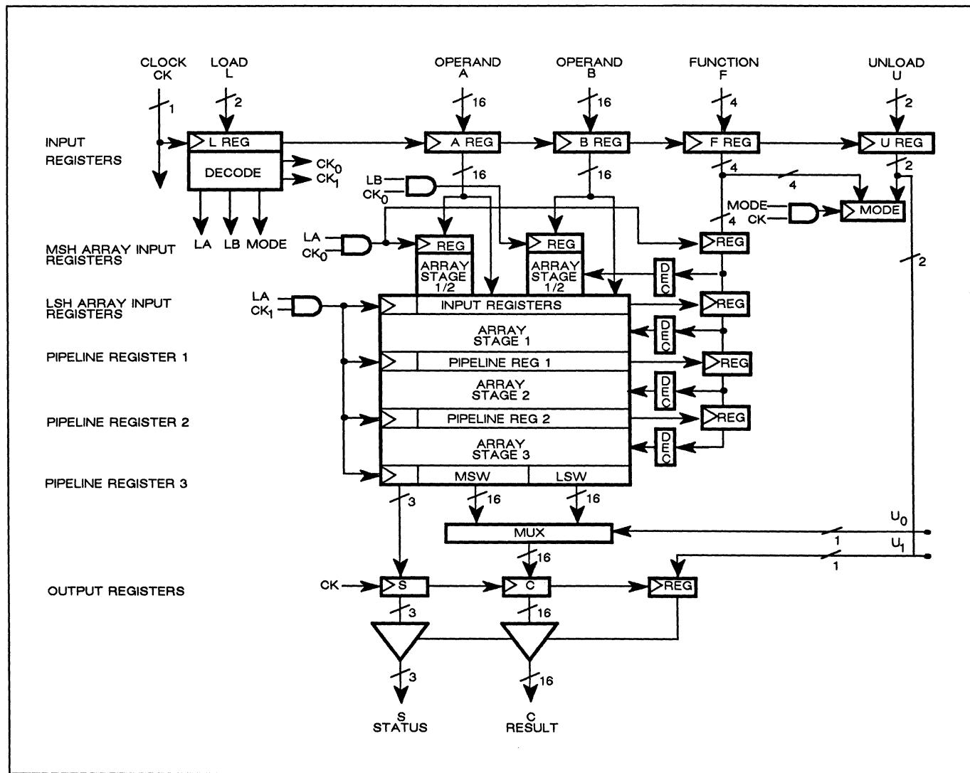
Figure 10. WTL 1232 and WTL 1233 Functional Block Diagram
