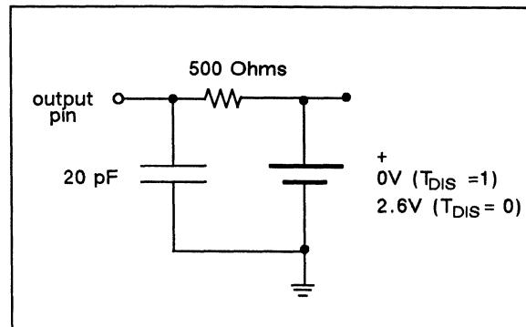
Figure 7. Test Load for Tri-State Delay Measurement
