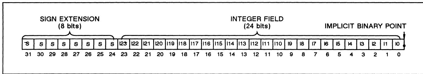
The value of the 24-bit integer field shown above can range from  $2^{23}-1$  to  $-2^{23}$  and must be sign-extended to 32 bits before performing a FLOAT operation, in which the number is converted to floating point format. The eight-bit sign extension field is a repeat of bit 23, the "sign" bit of the two's complement number. When
