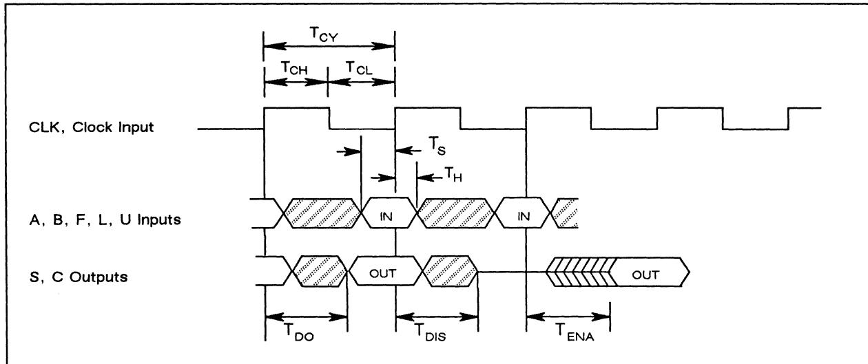
Figure 8. Switching Characteristics
