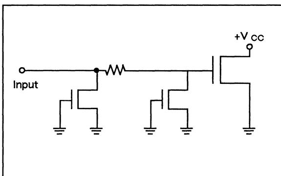
Figure 2. WTL 1233 Input Equivalent Circuit
