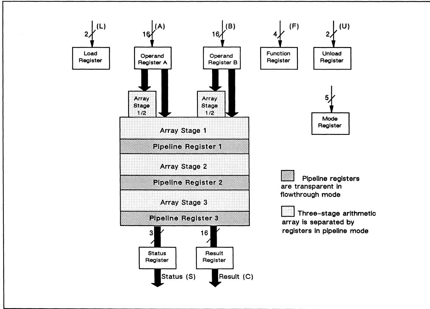
Figure 1. WTL 1232 Multiplier and 1233 ALU Data Path Architecture
