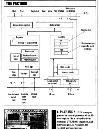
directional I/O lines, scan-test and CASE program test logic, and a 22bit external address bus (Fig. 1, top).
