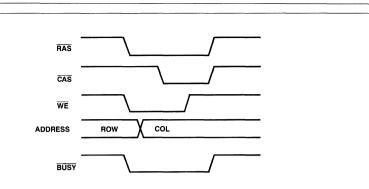
In response to a request to read one early write cycle will take place.  $\overrightarrow{\text{RAS}}$  will latch in the row address and the WE line goes low. The column address is set up followed by the falling edge of  $\overrightarrow{\text{CAS}}$ . The WE input is taken inactive followed by  $\overrightarrow{\text{RAS}}$  and  $\overrightarrow{\text{CAS}}$ . During the whole cycle the busy signal is active.
