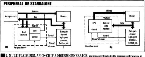
2. MULTIFLE BUSES, AN UN-UHIP ADDKESS GENEKATUK, and sequencer blocks let the microcontroller operate as a memory mapped peripheral to offload the host microprocessor (a). Or it can be operated as a standalone controller (b).
