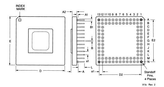
Family: Ceramic Pin Grid Array Package **Millimeters** Inches Symbol Min Max Notes Min Мах Notes 3.30 4.83 0.130 0.190 А A1 1.02 Typical 0.040 Typical A2 2.41 3.43 0.095 0.135 В 0.41 0.51 Diameter 0.016 0.020 Diameter B1 1.02 Typical Dia. 0.040 Typical Dia. D 32.51 33.91 1.280 1.335 1.200 Reference D2 30.48 Reference Е 32.51 33.91 1.280 1.335 E2 30.48 Reference 1.200 Reference 2.54 Reference 0.100 Reference e1 4.32 0.130 0.170 L 3.30 N 88 88
