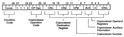
The instruction is executed only if the condition code field is true. The field is described in the Condition Codes section.
