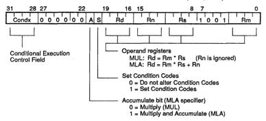
The Multiply and Multiply-Accumulate instructions use a 2-bit Booth's algorithm to perform integer multiplication. They give the least significant 32 bits of the product of two 32-bit operands and may be used to synthesize higher precision multiplications.
