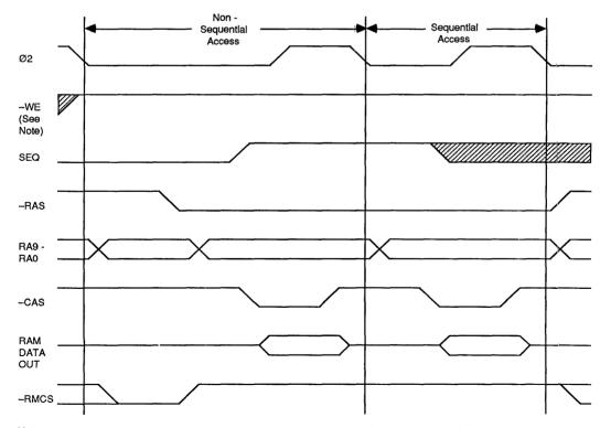
Note: -WE is obtained by passing the DBE signal from the VL86C110 through an external inverter.
