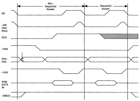
Note: -WE is obtained by passing the DBE signal from the VL86C110 through an external inverter.
