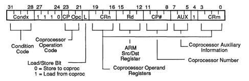
This instruction is executed only if the condition code field is true. The field is described in the Condition Codes Section.
