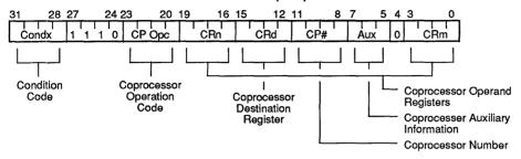
The instruction is only executed if the condition code field is true. The field is described in the Condition Codes Section.
