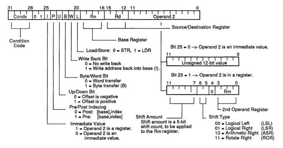
Note: There is no Rs or shift for the LDR/STR class. That is, the shift amount cannot be contained in a register.
