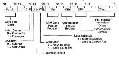
The LDC and STC instructions are used to load or store single bytes or words of data. They differ from MCR and MRC instructions in that they move data between coprocessor registers and a specified memory address. In contrast, the other instructions move data between registers, or move a constant (contained in the instruction) into a register.
