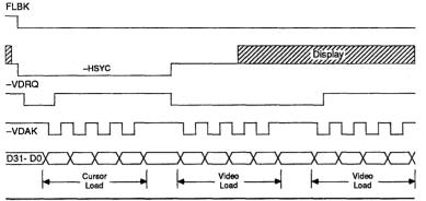
Hence, a VIDC FIFO load cycle consists of 1N + 3S requiring five RCLK clocks (417 ns at 12 MHz).
