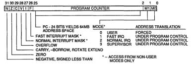
Translate is a control signal provided by the processor for control of an external memory management unit. The translate line is enabled in the user mode and disabled in the supervisor, fast interrupt and normal interrupt modes, since all modes except for the user mode are expected to be running secure code. Translated fetches can be made from the non-user modes by setting an optional bit in the load/store instructions.
