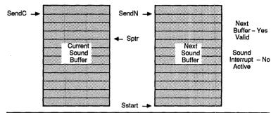
in response to a sound DMA request is held in the sound pointer register, Sptr, and the end of the current sound buffer is delimited by the current sound end register, SendC.
