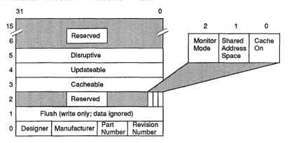
The VL86C020 contains six control registers as shown in Figure 22. These registers are implemented as coprocessor 15, and are accessed using coprocessor register transfer operations, where MRC is a control register read, and MCR is a control register write:
