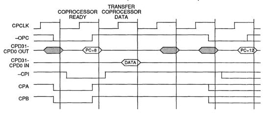
FIGURE 31. COPROCESSOR REGISTER TRANSFER (STORE TO COPROCESSOR)
