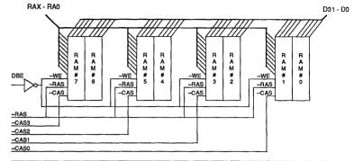
This configuration is essentially the same as used for the 1-bit wide DRAMs. In this case, only eight chips are required for the full 32-bit data bus.
