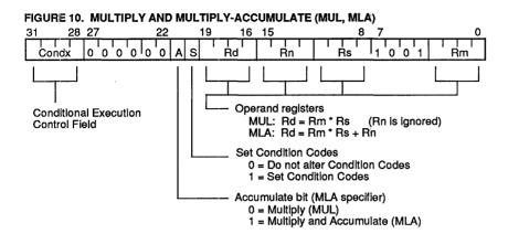
The multiply and multiply-accumulate instructions use a 2-bit Booth's algorithm to perform integer multiplication. They give the least significant 32 bits of the product of two 32-bit operands, and may be used to synthesize higher precision multiplications.
