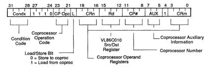
The instruction is executed only if the condition code field is true. The field is described in the Condition Codes section.
