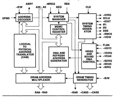
FIGURE 3. VL86C110 MEMORY CONTROLLER (MEMC) PIN DIAGRAM
