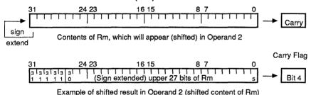
The form of the shift field which might be expected to give ASR 0 is used to encode ASR 32. Bit 31 of Rm is again used as the carry output, and each bit of operand 2 is also equal to the sign bit (bit 31) of Rm. The result is, therefore, all ones or all zeros according to the value of bit 31 of Rm. Rotate Right (ROR) operations reuse the bits which "overshoot" in a logical shift right operation by wrapping them around at the high end of the result. For example, the effect of a ROR 5 is:
