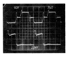
FIGURE 5. TOP: MOSFET V\_DS @ 50V/div. BOTTOM: MOSFET I\_D @ 5A/div.  $2\mu$ s/div.
