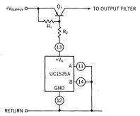
For single-ended supplies, the driver outputs are grounded. The  $V_c$  terminal is switched to ground by the totem-pole source transistors on alternate oscillator cycles.
