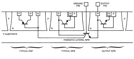
FIGURE 4. PARASITIC NPN TURNS ON WHEN SUBSTRATE - EPI JUNCTION IS FORWARD BIASED.
