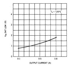
Figure 3. Typical Sink Saturation Voltage vs Output Current
