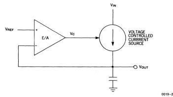
Figure 2. Inductor Looks Like a Current Source to Small Signals
