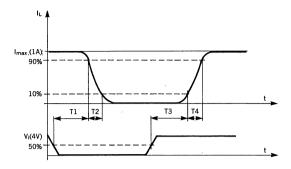
Figure 2a. Sink Current Delay Times vs. Input.
