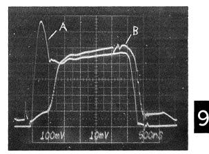
FIGURE 8. A: MOSFET I<sub>D</sub> @ 2A/div. B: CURRENT SENSE (UC2842 — PIN 3) @ 100mV/div. 500ns/div.
