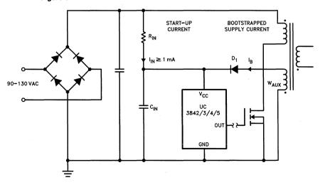
Figure 7. Providing Power to the UC3842/3/4/5
