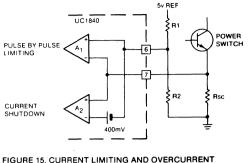
IGURE 15. CURRENT LIMITING AND OVERCURRENT SHUTDOWN ARE IMPLEMENTED WITH COMPARATORS OF DIFFERENT THRESHOLDS AND A SINGLE CURRENT SENSE RESISTOR.
