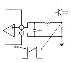
FIGURE 4. RC FILTER FOR REDUCING SWITCH TRANSIENTS
