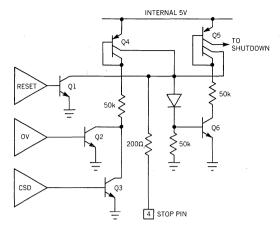
The Error Latch consists of Q5 and Q6 which, when both on, turns off the PWM Output and pulls the Slow-Start pin low. This latch is set by either the Over-Voltage or Current Shutdown comparators, or by a high signal on Pin 4. Reset is accomplished by either the Reset comparator or a low signal on Pin 4. An activation time delay can be provided with an external capacitor on Pin 4 in conjunction with the  $\approx 100\mu$ A collector current from Q4.
