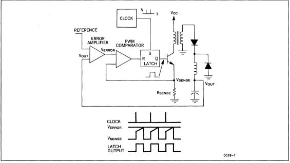
Figure 1. Two-Loop Current-Mode Control System
