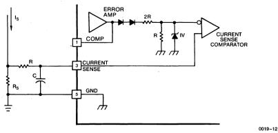
Figure 12. Current Sensing
