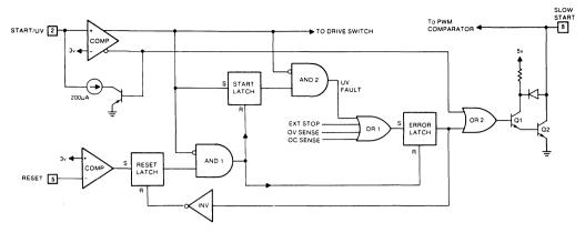
FIGURE 16. FAULT SEQUENCE LOGIC IS DESIGNED TO INSURE A COMPLETE SHUTDOWN AND FULLY CONTROLLED RESTART UPON ANY OF FOUR POSSIBLE FAULT CONDITIONS.
