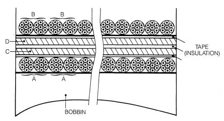
Figure 6. Transformer — Exploded View
