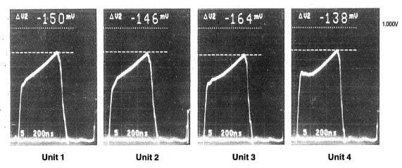
Figure 46. Primary Currents – Parallel Operation
