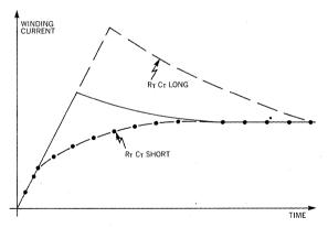
Figure 7. Effects of Different R<sub>T</sub> & C<sub>T</sub> on Bilevel Systems
