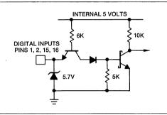
The input zener may be used to clamp input signal voltages higher than 5V as long as the zener current is limited to 10mA max. External pull-up resistors are not required.
