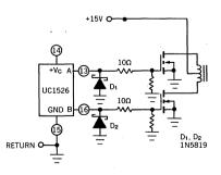
Figure 9. Driving N-Channel Power Mosfets
