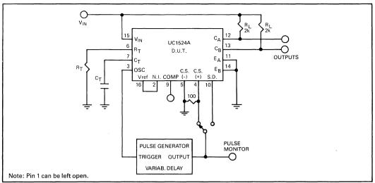
FIGURE 7 — Evaluating the Turn-off Delays of the UC1524A with the Aid of a Triggerable Pulse Generator With Variable Delay.
