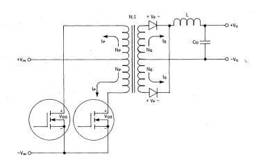
FIGURE 9. BASIC PUSH-PULL POWER CIRCUIT AND FILTER.
