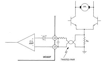
Figure 6. Current Limit Sensing
