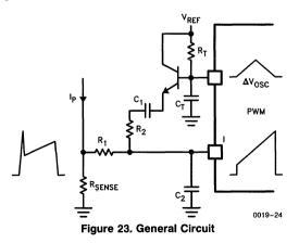
Resistors  $R_1$  and  $R_2$  form a voltage divider from the oscillator output to the current sense input, superimposing the slope compensation on the primary current waveform. Capacitor  $C_1$  is an AC coupling capacitor, and allows the AC voltage swing of the oscillator to be used without adding offset circuitry. Capacitor  $C_2$  forms an R-C filter with  $R_1$  to
