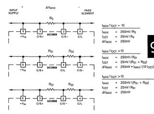
FIGURE 6. Although the ratio of input offset voltages on the current limit and current sense stages is fixed at 10, other ratios for  $|_{MAX}/l_{OCT}$  are easily obtained. Note that a penalty for ratios greater than 10 is increased voltage drop across the sensing network at  $|_{MAX}$ .
