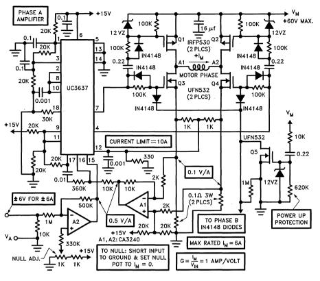
Figure 9. PWM Transconductance Amplifier UC3637
