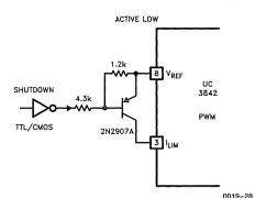
A. NONLATCHING Figure 26A. PWM Shutdown Circuit
