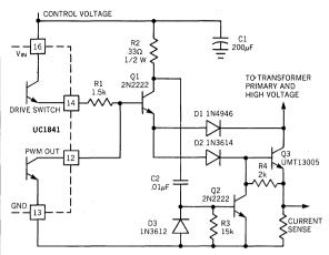
Most high voltage transistors trade both current gain and speed for voltage capability. This circuit provides both high turn-on and turn-off pulse base currents into Q3 as well as a Baker clamp saturation control. This entire drive circuit is held off by the UC1841's Drive Switch for low current drain while the control voltage is rising.
