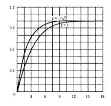
Figure 6. Small Signal Step Response (Normalized Amplitude vs t/R<sub>F</sub>C<sub>F</sub>)
