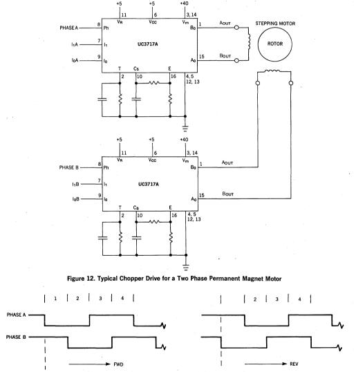
Figure 13. Phase Input Signal for Two Phase Full Step Drive (4 Step Sequence)
