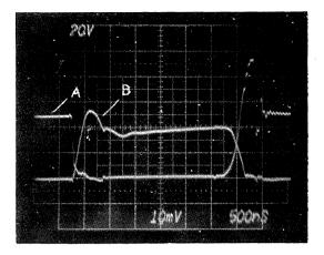
FIGURE 6. A: MOSFET V<sub>DS</sub> @ 20V/div. B: MOSFET I<sub>D</sub> @ 5A/div. 500ns/div.
