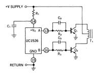
Figure 7. Push-Pull Configuration
