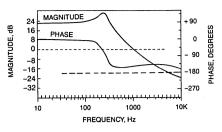
Figure 19. Calculated response plot for the modulator and filter.
