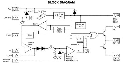
Note: 1. A/B A = DIL-8 Pin Number. B = S0-14 Pin Number. 2. Toggle flip flop used only in 1844 and 1845.
