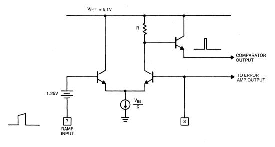
FIGURE 2a. PWM COMPARATOR SCHEMATIC.
