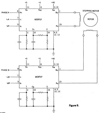
A typical chopper drive for a two phase bipolar permanent magnet or hybrid stepping motor is shown in Figure 9. The input can be controlled by a microprocessor, TTL, LS or CMOS logic. The timing diagram in Figure 10 shows the required signal input for a two phase, full step, stepping sequence. Figure 11 shows a one phase, full step, stepping sequence, commonly referred to as wave drive. Figure 12 shows the required input signal for a one phase-two phase stepping sequence called half-stepping.
