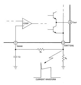
Figure 1. Current Sense Filter
