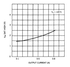
Figure 2. Typical Source Saturation Voltage vs Output Current
