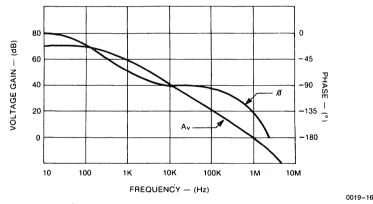
Figure 15. Error Amplifier Open-Loop Frequency Response
