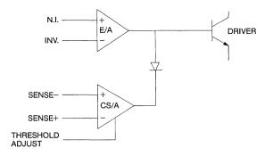
Figure 8. Current Sense Tied to E/A Output
