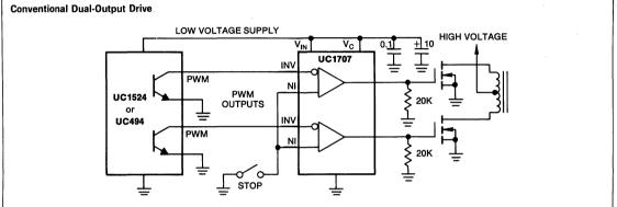
Driving the inverting inputs from open-collector, dual-output PWM Controllers. If unneeded for programming functions, the non-inverting inputs can be left open. Note that the high peak current drive for MOS gates requires good supply decoupling at Vc. VIN and Vc need not be at the same levels. The 20K resistors hold the FETs off during startup when the UC1707 output impedance is high.
