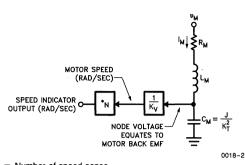
\*N = Number of speed sense cycles per motor revolution
