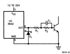
Figure 20. Bipolar Drive with Negative Turn-Off Bias
