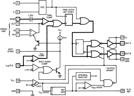
UNITRODE INTEGRATED CIRCUITS 7 CONTINENTAL BLVD. • MERRIMACK, NH 03054 TEL. (603) 424-2410 • TELEX 95-3040 propagation through these subcircuits makes or breaks a design during a fault condition. In the 3825, the propagation delay from either the Ramp input or the Current-limit sense input to the output pins is typically 50ns, very much faster than any chip available today.
