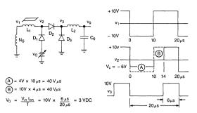
Figure 2. A simplified mag amp regulator and characteristic waveforms.
