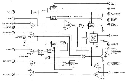
Note: Positive true logic, latch outputs high with set, reset has priority.
