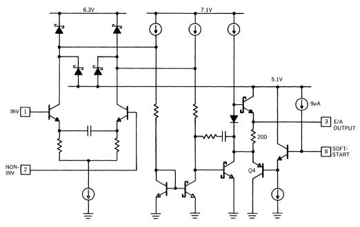
FIGURE 6. SIMPLIFIED SCHEMATIC OF WIDE BAND ERROR AMPLIFIER SHOWING SOFT START CLAMP SCHEME.
