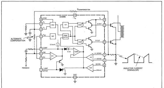
Current loop instability above 50% duty cycle can be corrected using slope compensation derived from the sawtooth oscillator. Compensation magnitude should be greater than  $\frac{1}{2}$  of the down-
