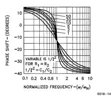
Figure 12. To keep feedthrough of the residual reference frequency at the phase detector output to a minimum, a simple quadratic filter can be used. The design of this filter is easily accomplished with the above equations and response curves.
