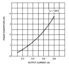
Figure 4. Typical Power Losses vs Output Current
