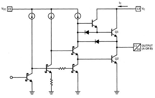
FIGURE 3a. OUTPUT STAGE SIMPLIFIED SCHEMATIC.
