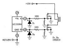
Figure 9. Driving N-Channel Power Mosfets
