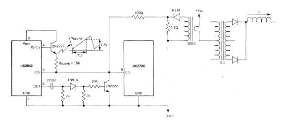
FIGURE 10. CURRENT SENSE WITH SPIKE SUPPRESSION AND SLOPE COMPENSATION.
