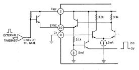
FIGURE 8. SYNCHRONIZING THE 1846 TO AN EXTERNAL TIME BASE
