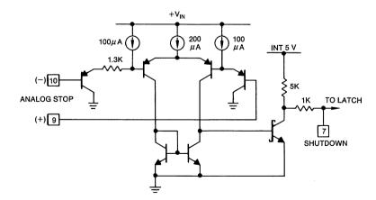
The input common-mode voltage range is from ground to  $(V_{\text{IN}}\text{-}3V).$  When not used both inputs should be grounded. Activate time is a function of overdrive with a minimum value of 160ns. Pin 7 serves both as a comparator output and as a com-
