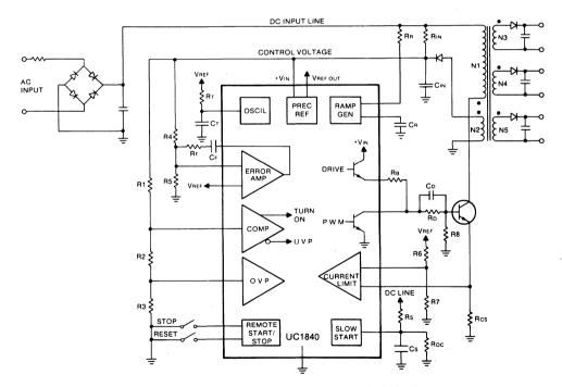
FIGURE 2. A FULLY PROTECTED, ISOLATED FLYBACK POWER SUPPLY CAN BE IMPLEMENTED WITH THE UC1840, A HIGH-VOLTAGE POWER SWITCH, THE TRANSFORMER, AND A SMALL HANDFUL OF PASSIVE COMPONENTS.
