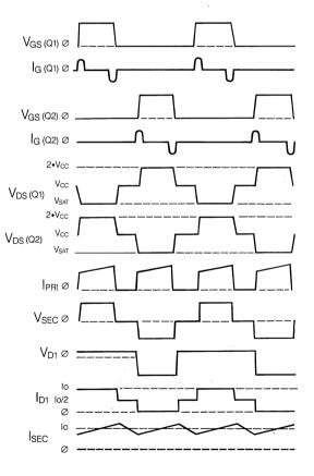
Figure 3. Basic Push-Pull Waveforms
