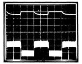
Top: V<sub>OUT</sub>,  $2V \times 20$  ms/div. Bot: Inductor current,  $2A \times 20$  ms/div.
