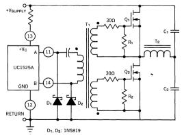
Low power transformers can be driven by the UC1525A. Automatic reset occurs during dead time, when both ends of the primary winding are switched to ground.
