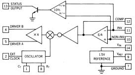
FIGURE 4. UC2901 BLOCK DIAGRAM
