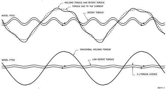
Figure 1. Static Torque Curves of Two Hybird Steppers
