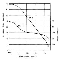
FIGURE 11. THE UC1840 ERROR AMPLIFIER HAS A DC GAIN OF 67 db, A 2 MEGAHERTZ BANDWIDTH, AND PHASE MARGIN OF APPROXIMATELY 45°
