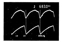
Top Trace Ramp Voltage TP 'H', 1 v/cm Bottom Trace CT Waveform, TP 'D', 1 v/cm
