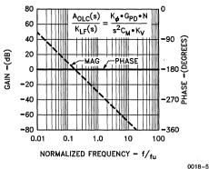
Figure 5. A Bode plot of the combined gain and phase response of the motor, motor drive, and phase dectector is useful in determining the requirements on the loop filter. This plot is normalized to the desired open loop unity gain frequency.
