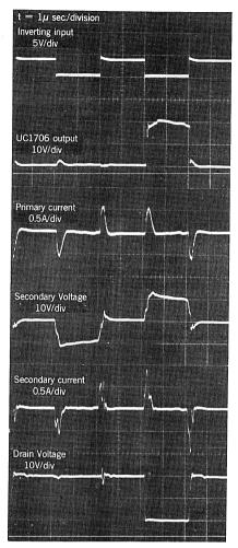
FIGURE 24 - BALANCED PUSH-PULL TRANSFORMER COUPLING PERFORMANCE.
