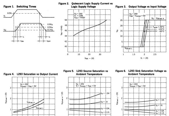
Io – (A) NOTE: For L293D curves, multiply output current by 0.6
