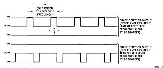
Figure 11. The phase detector on the UC3633 is a digital circuit that responds to phase error with a pulsed output at the reference frequency rate. The width and polarity of the pulses depend respectively on the phase error magnitude and polarity. If any static frequency error is present, the detector will respond with a constant 0 Volt or 5 Volt signal depending on the sign of the error present.
