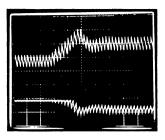
Top: Inductor current,  $2A \times .1$  ms/div. Bot: V<sub>OUT</sub> of C.L. amp (pin 1),  $2V \times .1$  ms/div.
