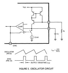
Referring to Figure 5, an external resistor R<sub>T</sub> is used to generate a constant current into a capacitor C<sub>T</sub> to
