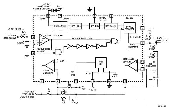
Figure 10. Phase locking the motor to a precision reference frequency is achieved with the UC3633. The double edge sensing option on this device doubles the loop gain and allows twice the reference frequency to be used for a given motor RPM by forcing the phase detector to respond to both edges of the Hall feedback signal.
