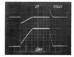
FIGURE 7. LARGE-SIGNAL OUTPUT SLEW RATE. TOP: OUTPUT VOLTAGE @ 11/div. BOTTOM: OUTPUT CURRENT @ 5A/div. 200µs/div.
