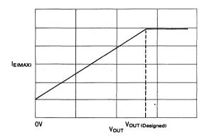
Figure 13. Foldback Current Limiting Characteristic
