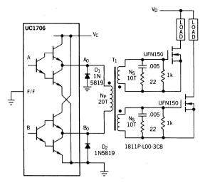
FIGURE 23 BALANCED PUSH-PULL TRANSFORMER COUPLING
