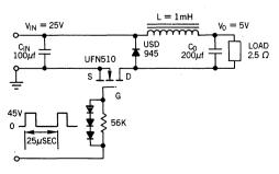
FIGURE 2 - SWITCHING TIME EVALUATION CIRCUIT.
