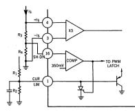
FIGURE 12. OVER CURRENT SENSING WITH THE SHUTDOWN CIRCUIT PRODUCES A SHUTDOWN — SOFT RESTART CYCLE TO PROTECT OUTPUT DRIVERS
