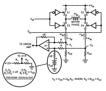
Figure 6. H-Bridge Configuration with Bidirectional Current Sensing
