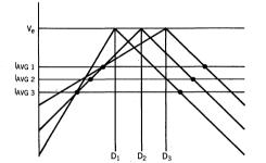
FIGURE 8 – PEAK CURRENT SENSING WITHOUT SLOPE COMPENSATION ALLOWS AVERAGE INDUCTOR CURRENT TO VARY WITH DUTY CYCLE
