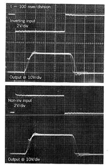
FIGURE 12- SWITCHING RESPONSE WITH OUTPUT CAPACITANCE OF 0, 1000, AND 2200 PF.
