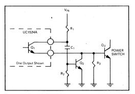
FIGURE 10 — The addition of C<sub>1</sub> and Q<sub>2</sub> Uses the Collector Signal of the UC1524A to Generate an Enhanced Turn-off Command for Q<sub>3</sub>
