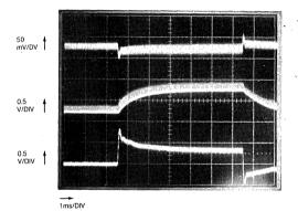
FIGURE 11: The Transient Response of the 5V Output (Top Trace), to a 3.0A Step Load Change Reflects the Extended Bandwidth of the 5V Loop. The Open-Loop 12V Output (Middle), Responds to the Effects of Cross Regulation. The Feedback Error Signal (Lower) Coupled Through the UC1901 is Measured at the UC1840 Error Amp. Output.
