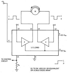
INPUTSFUNCTION $V_{En} = H$ C = H; D = LTurn rightC = L; D = HTurn leftC = DFast motor stop $V_{En} = L$ C = X; D = CFree running<br/>motor stop
