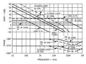
FIGURE 11. SMALL SIGNAL FREQUENCY RESPONSE.
