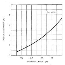
Figure 4. Typical Power Dissipation vs Output Current
