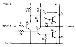
FIGURE 6 - A SIMPLIFIED SCHEMATIC OF THE DS0026 DRIVER IC
