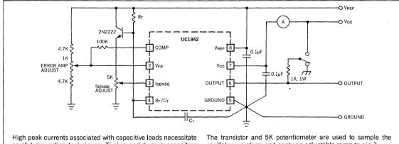
careful grounding techniques. Timing and bypass capacitors should be connected close to pin 5 in a single point ground.
