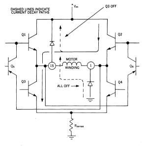
Figure 7. Simplified Schematic of Output Stage
