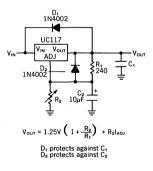
Figure 2. Regulator with Protection Diodes
