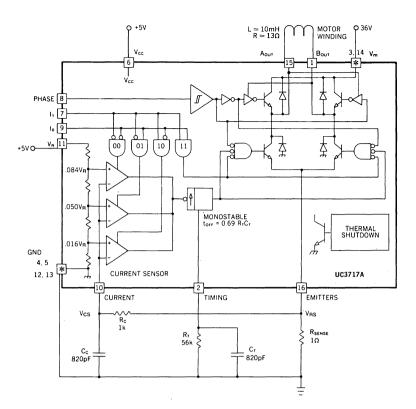
Figure 6. UC3717A Test Circuit
