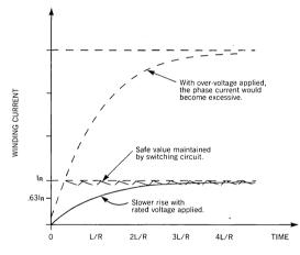
Figure 9. With rated voltage applied, winding current does not exceed rated value, but takes L/R seconds to reach 63% of its final value—probably too long. Increased performance requires an increase in applied voltage, or overdrive, and therefore a means to limit current. The UC3717A motor driver performs this task efficiently.
