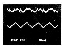
**Top Trace** Output Voltage Ripple & Noise TP 'W', 100 mv/cm Bottom Trace AC Output Current J2, 2 A/cm
