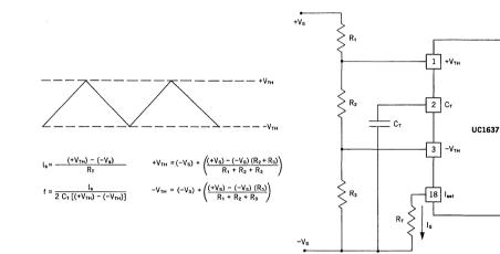
Figure 1. Oscillator Set Up
