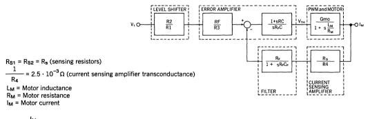
$G_{mo} = \frac{I_{M}}{V_{TH}}|_{s} = 0$  (DC transfer function from the input of the comparator (V\_{TH}) to the motor current (I\_{M})).
