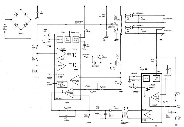
FIGURE 9: The UC1901 Combines With an Advanced PWM Controller in a 60W Off-Line Converter.
