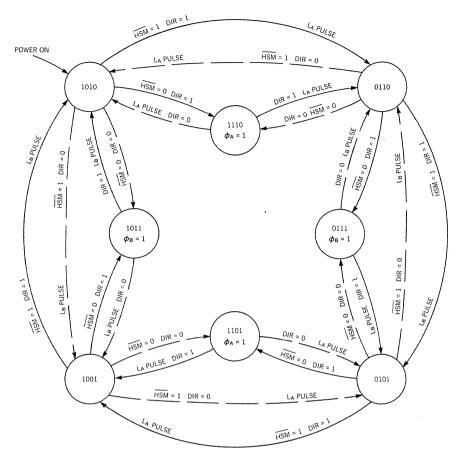
Figure 5. Logic Flow Graph
