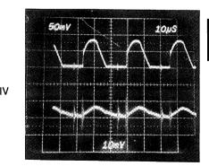
Upper trace: +5V charging current Lower trace: +5V output ripple voltage
