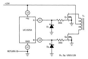
The low source impedance of the output drivers provides rapid charging of power FET input capacitance while minimizing external components.
