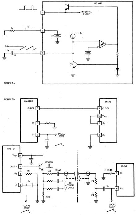
FIGURE 5. OSCILLATOR SIMPLIFIED SCHEMATIC (a) AND TWO SYNCHRONIZATION METHODS (b).
