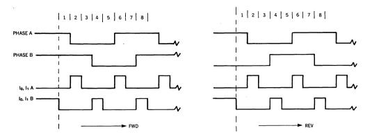
Figure 14. Phase and Current-Inhibit Signal for Half-Stepping (8 Step Sequence)
