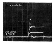
FIGURE 20- CURRENT LIMITING WITH THRESHOLD SET FOR 2 amps
