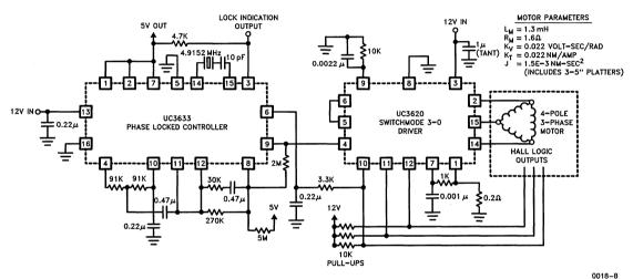
Figure 8. A precision speed control loop uses the UC3620 Switchmode 3-phase Driver and the UC3633 Phase Locked Controller to spin a DC brushless motor at 3600 rpm, ±60 ppm.
