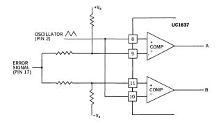
Figure 2. Comparator Biasing
