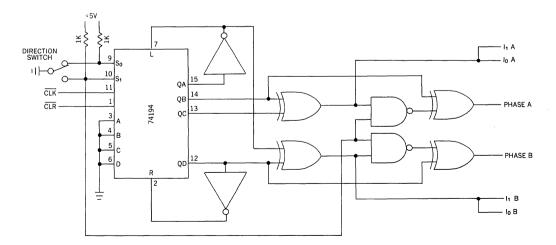
Figure 16. Half Step, Bidirectional Drive Logic
