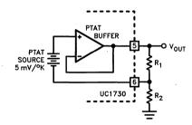
$V_{OUT} = 5 \times \left(1 + \frac{R_2}{R_1}\right) mV/^{\circ}K$  (Recommended Range for R<sub>1</sub> is 2K to 4K)
