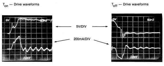
Upper trace:  $Q_1$  — Gate to source voltage Lower trace:  $Q_1$  — Gate current
