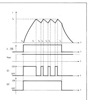
Figure 2. Load current waveform with external R-C network connected between pin 9 and ground
