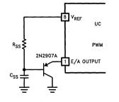
Figure 29. Soft Start Circuit
