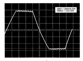
Figure 8. A typical winding current waveform. Winding current rises exponentially to a selected peak value. The peak value is limited by switched mode operation producing a ripple in winding current. A phase polarity reversal command is given and winding current decays to zero, then increases exponentially in the reverse direction.
