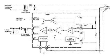
FIGURE 2: With a Precision Reference, and a Complete Amplitude Modulation System, the UC1901 Lets Isolated Feedback Loops be Closed Using a Small Signal Transformer.
