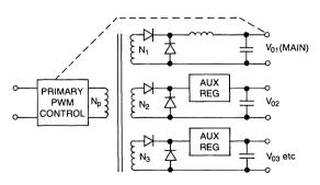
Figure 1. A typical multiple output power supply architecture with overall control from one output.
