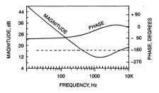
Figure 20. Compensated amplifier response.
