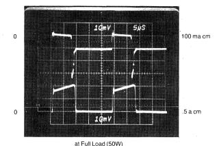
FIGURE 17 — Base Current (Upper Trace) and Collector Current for the UMT 13005 of Figure 16. The Time Base is 5µs per Division.
