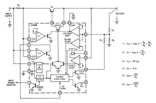
FIGURE 4. Using a few external parts and following simple design equations the UC3906 can be configured as a dual level float charger.
