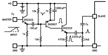
Figure 35. Sync Pulse Generator Circuit
