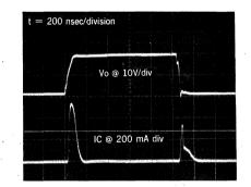
FIGURE 8 - CROSS-CONDUCTION CURRENT IN THE 1525A OUTPUT STAGE
