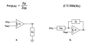
Figure 21. E/A Compensation (a.) Without and (b.) With Local Feedback
