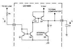
FIGURE 9. CURRENT MIRRORS Q1-Q4 ARE USED TO MAKE THE RAMP CHARGING CURRENT I2, LINEARLY PROPORTIONAL TO THE DC.INPUT LINE
