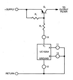
Figure 10. A single-ended, ground-referenced power stage for a flyback or boost regulator.
