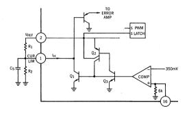
FIGURE 11. SHUTDOWN CIRCUITRY
