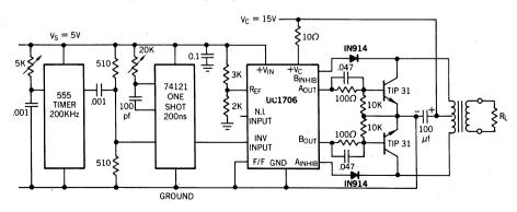
FIGURE 25 - A SQUARE WAVE INVERTER CIRCUIT USING THE UC1706 TO DRIVE BIPOLAR TRANSISTOR SWITCHES.
