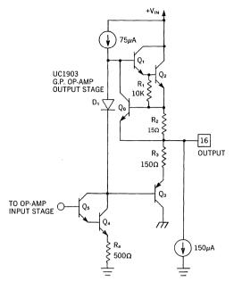
Figure 5. The G.P. op-amp on the UC1903 has a high source current (≥20mA) capability and enhanced transient sinking capability through substrate device Q<sub>3</sub>.
