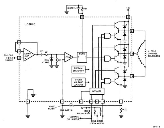
Figure 9. The UC3620 is a current mode fixed off-time driver. This device includes all the drive and commutation circuitry for a three phase brushless motor. The 0.2Ω current sense resistor and the internal divide by five sets the transconductance of this power stage to 1 Amp/Volt.
