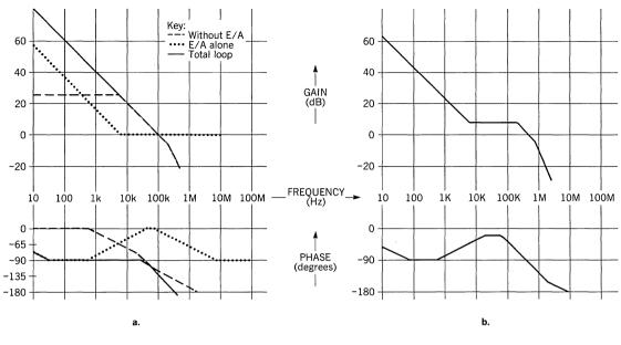
Figure 18. Loop Responses for Circuit of Figure 17 a. Voltage Loop b. Current Loop
