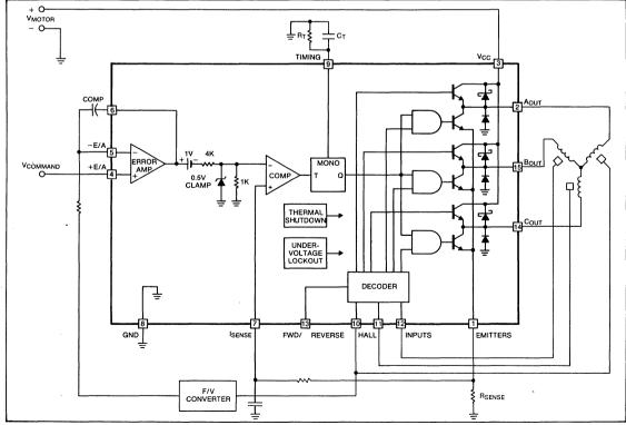
3- $\phi$  BRUSHLESS DC OPEN LOOP MOTOR DRIVE WITH CURRENT LIMIT
