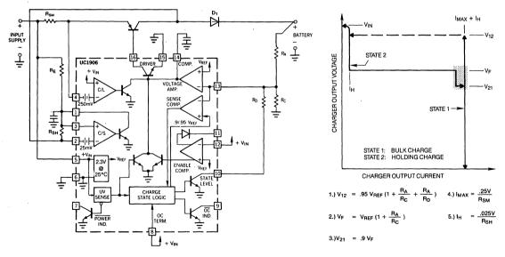
FIGURE 10. A dual step current charger has some advantages when large series strings must be charged. This type of charger maintains constant current during normal charging that results in equal charge distribution among battery cells.
