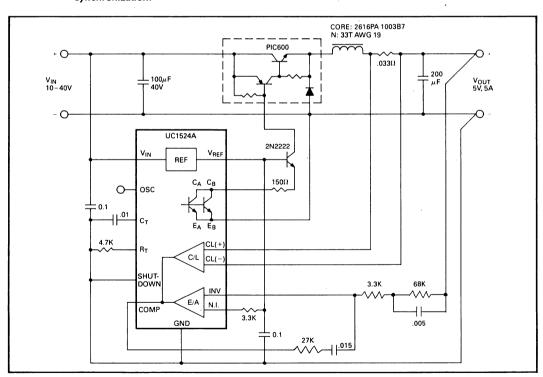
FIGURE 12 — The UC1524A Combines With the PIC 600 Hybrid Switch to Form A Simple But Powerful Buck Regulator.
