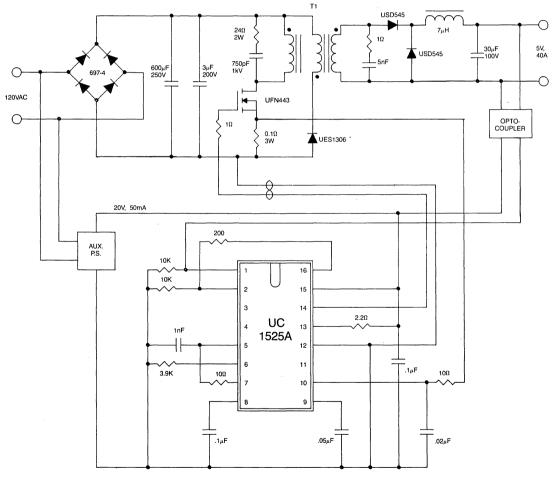
Figure 13. 200W, Off-Line Forward Converter.
