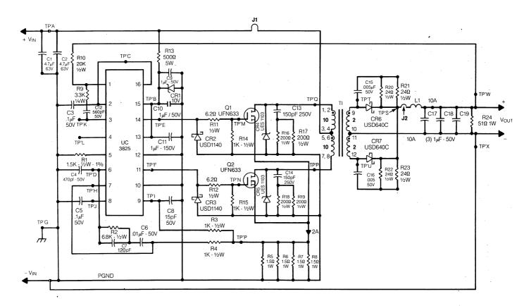
Figure 1. 1.5 MHz Push-Pull Converter Schematic Diagram
