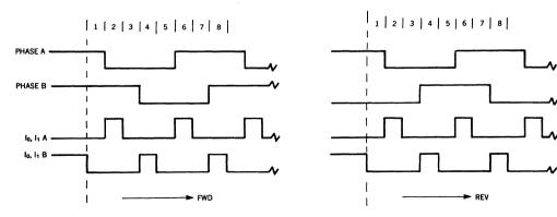
Figure 12. Phase and Current-Inhibit Signal for Half-Stepping (8 Step Sequence)
