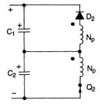
Figure 44. Transistor Q2 On
