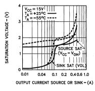
Figure 17. Output Saturation Characteristics
