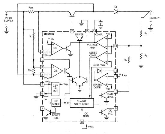
Figure 4. The UC2906 in a Dual Step Current Charger
