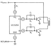
In conventional push-pull bipolar designs, forward base drive is controlled by R<sub>1</sub>-R<sub>3</sub>. Rapid turn-off times for the power devices are achieved with speed-up capacitors C<sub>1</sub> and C<sub>2</sub>.
