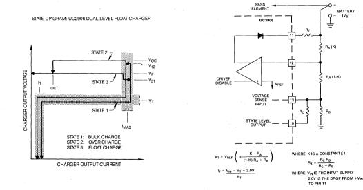
FIGURE 7. The charge enable comparator, with its trickle bias output, can be used to build protection into the charger. The current foldback at low battery voltages prevents high current charging of batteries with shorted cells, or improperly connected batteries, and also protects the pass element from excessive power dissipation.
