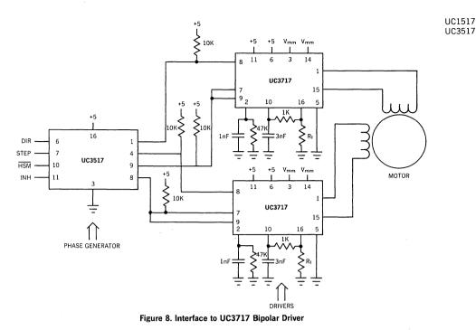
In this application, the  $\phi_A$  and  $\phi_B$  outputs of the UC3517 are connected to the current program inputs of the UC3717. This allows the UC3517 inhibit signal to inhibit the UC3717, and also allows half-step operation of the UC3717. Peak motor winding current will be limited to approximately .42V/R<sub>I</sub> by chopping.
