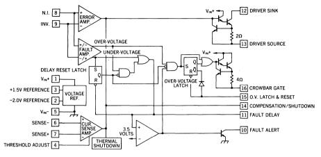
Figure 2. UC1834 Block Diagram
