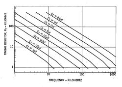
FIGURE 6. OSCILLATOR FREQUENCY AS A FUNCTION OF  $$R_{T}$$  AND  $C_{T}$
