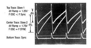
Figure 26. CT Ramp Amplitude Waveforms
