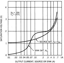
Figure 5. The ouput saturation characteristics of the UC1525A provide both high drive current and low hold-off voltage.
