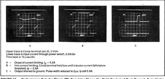
FIGURE 13 — Performance Data for Figure 13's Regulator Shows the Tight Control of Peak Current, Even Under Shorted Output Conditions.
