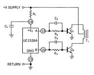
Figure 7. Push-Pull Configuration
