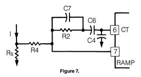
For the purposes of determining the resistor values, capacitors C4 (timing), C6 (ac coupling) and C7 (filtering) can be removed from the circuit schematic. The simplified model represented in figure 8 is used for the calculations. These calculations can be applied to all Current Mode circuits using a similar scheme.
