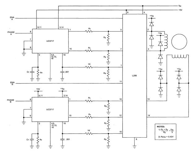
Figure 15 - UC3717 with L298 Power Amplifier.
