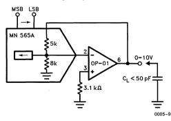
10 Hz to 10 kHz Square Wave Generator
