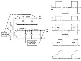
Figure 4. Control waveforms for a typical two-output, secondary regulated, forward converter.
