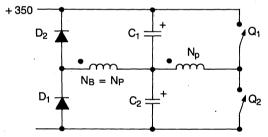
Figure 42. Schematic – Balancing Winding
