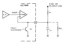
FIGURE 6. PIN 8 ON THE UC1840 CAN BE USED FOR BOTH . SLOW TURN-ON AND DUTY-CYCLE LIMITING AS WELL AS A PWM SHUTDOWN PORT.
