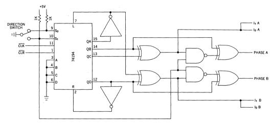
Figure 14. Half Step, Bidirectional Drive Logic
