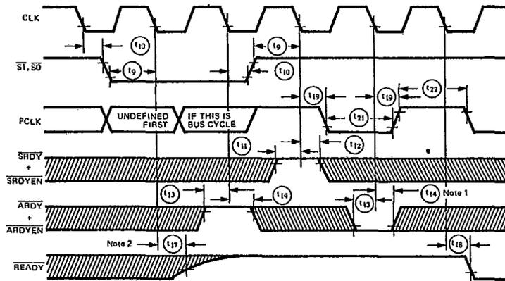
Note 1: This is an asynchronous input. The setup and hold times shown are required to guarantee the response shown.
