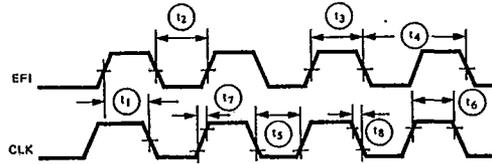
Note: The EFI Input LOW and HIGH times as shown are required to guarantee the CLK LOW and HIGH times shown.
