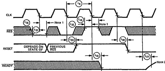
Note 1: This is an asynchronous input. The setup and hold times shown are required to guarantee the response shown.
