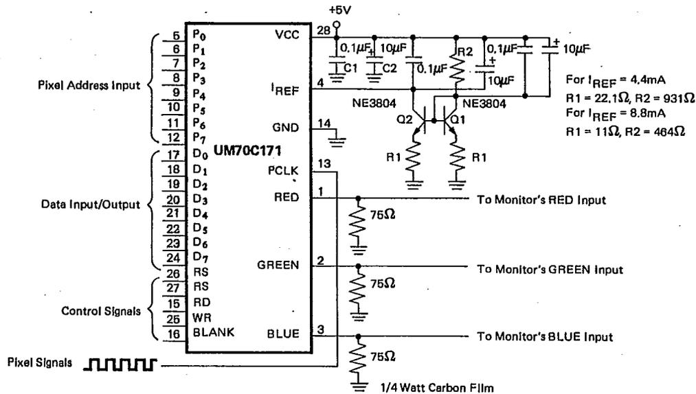
Note: Bead-style tantalum capacitors should be used for the 10 $\mu$ F devices
