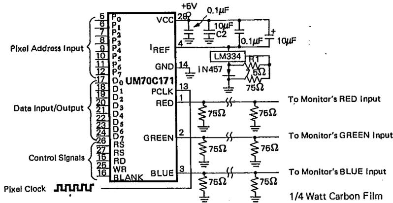
Note: Bead-style tantalum capacitors should be used for the 10μF devices.
