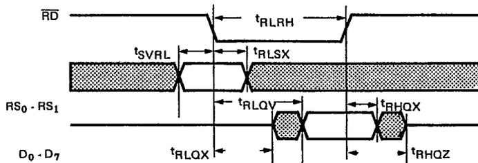
Figure 4. Basic Read Cycle Timing Diagram.
