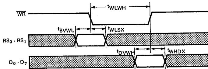
Figure 3. Basic Write Cycle Timing Diagram.
