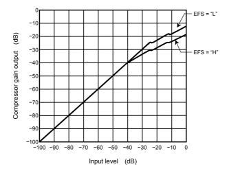
Figure 7 Dynamic Digital Bass Boost Compressor I/O Characteristics
