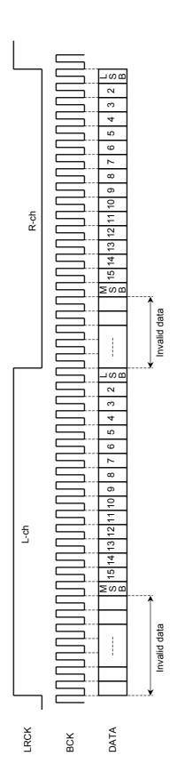
Figure 2b Example of Input Timing Chart
