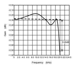
Figure 3 Digital Filter Frequency Characteristics
