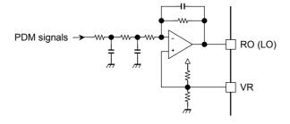
Figure 11 Analog Filter Circuit
