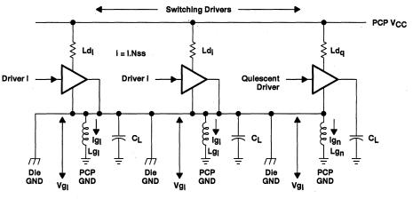
Figure 2. Simultaneous Switching<sup>2</sup>
