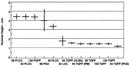
Figure 7. Typical Package Height Versus Height Variance
