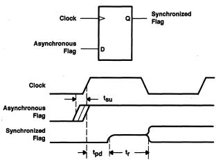
Figure 2. Single-Stage Synchronizer
