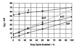
Figure 5. I<sub>CC</sub> Versus Duty Cycle Enabled (25 MHz)
