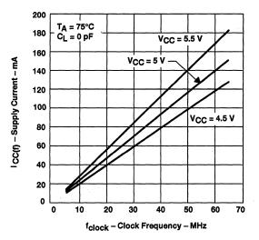
Figure 1. SN74ACT7804 Supply Current Versus Clock Frequency
