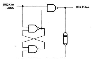
Figure 4. 'ALS2232A and 'ALS2233A Clock Input Circuit
