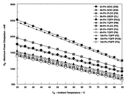
Figure 10. R<sub>OJA</sub> for FIFO Packages in Still Air
