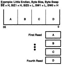
Figure 5. Little-Endian Data-Output Structure
