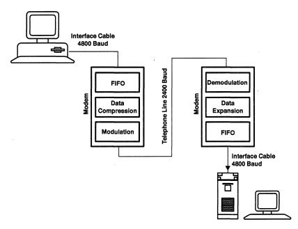
Figure 16. Data Transmission by Modem With Data Compression
