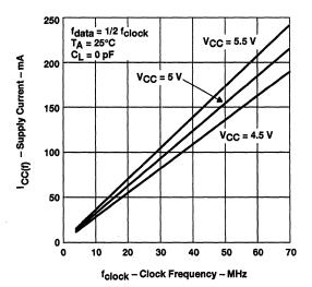
Figure 2. SN74ACT3638 Supply Current Versus Clock Frequency
