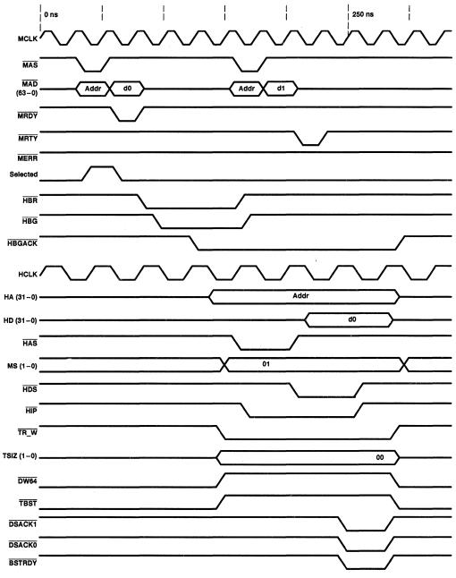
Figure 8. MBus-Word Write to HIF Single-Write Transaction
