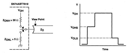
Figure 4. Shelf Voltage When Switching a Transmission Line
