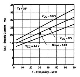
Figure 5. SN74ABT3614 Idle Current With CLKA Switching, Other Inputs at 0 or  $V_{CC}$  – 0.2 V and Outputs Disconnected
