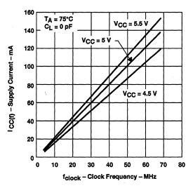
Figure 1. SN74ACT7807 Supply Current Versus Frequency
