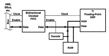
Figure 3. Bidirectional Clocked FIFO Used for Bus-Speed Matching
