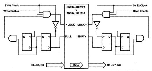
Figure 5. Clock Generation With Two-Stage Synchronization of FULL and EMPTY
