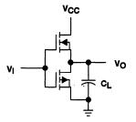
Figure 1. Gate Model of a CMOS Inverter
