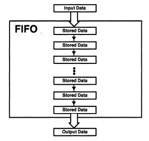
Figure 1. FIFO Data Flow
