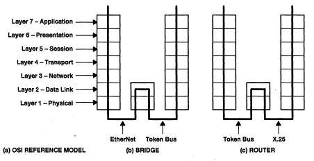
Figure 15. Bridge and Router Devices
