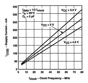
Figure 2. SN74ABT3612 Supply Current Versus Clock Frequency
