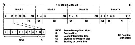
Figure 7. Frame Structure of the 8448-kbit/s Multiplex Signal (Second Hierarchy Level)
