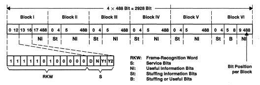
Figure 9. Frame Structure of the 139264-kbit/s Multiplex Signal (Fourth Hierarchy Level)
