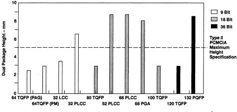
Figure 6. Type II PCMCIA Package Height Versus Dual Package Solutions<sup>†</sup>
