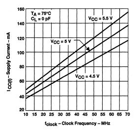
Figure 1. SN74ABT7819 Supply Current Versus Clock Frequency
