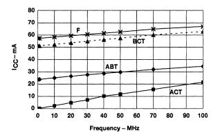
Figure 2. I<sub>CC</sub> Versus Frequency (One Switching, Unused Outputs Low)
