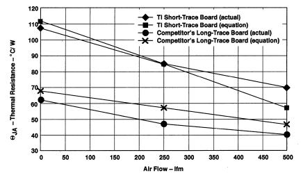
Figure 3. 52-Pin MQFP (actual versus equation)
