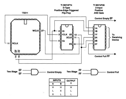
Figure 5. Resolving Metastability of a Synchronous FIFO
