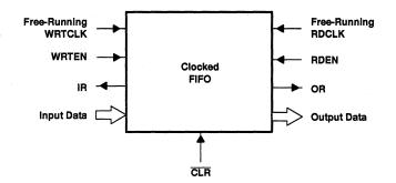
Figure 3. Connections of a Clocked FIFO
