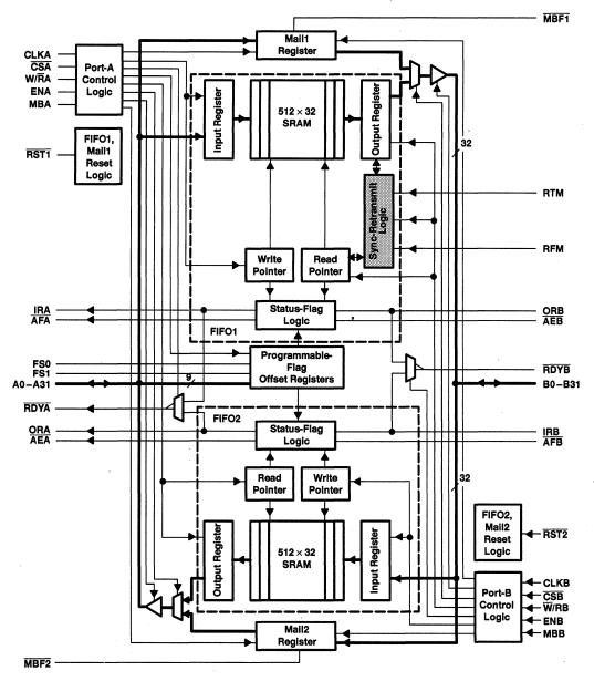
Figure 1. SN74ACT3638 Functional Block Diagram
