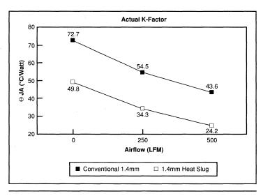
Figure 10. Thermal Impedance of Conventional vs. Heat Slug Packages.
