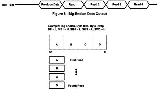
Figure 7. Big-Endian Data-Output Structure
