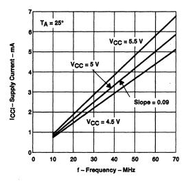
Figure 3. SN74ACT7807 Idle Current With RDCLK Switching, Other Inputs at 0 or V<sub>CC</sub> – 0.2 V and Outputs Disconnected
