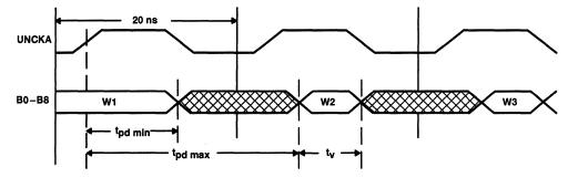
For SN74ACT2235-20:  $t_{pd min}$  = 12 ns,  $t_{pd max}$  = 25 ns,  $t_{v}$  = 7 ns
