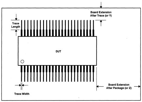
NOTE: Y and Z are used for PLCC and QFP packages.
