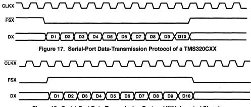
Figure 18. Serial-Port Data-Transmission Protocol With Inverted Signals
