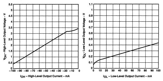
Figure 3. Output Characteristics of the SN74ABT7819 ( $V_{CC} = 5 V$ ,  $T_A = 25^{\circ}C$ )
