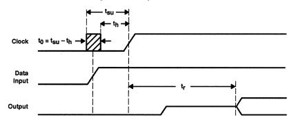
Figure 2. Output at Intermediate Level Due to Data Edge Within to Aperture
