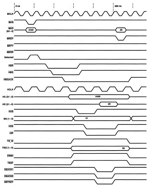
Figure 7. MBus-Word Read to HIF Single-Read Transaction
