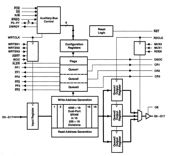
Figure 4. Multi-Q FIFO Functional Block Diagram
