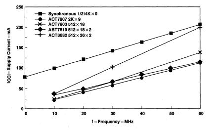
Figure 8. Active I<sub>CC</sub> Versus Frequency
