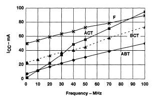
Figure 4. I<sub>CC</sub> Versus Frequency (All Switching, 50% Duty Cycle Enabled)
