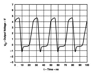
Figure 2. Output Waveform at 80-MHz Clock (CL = 50 pF)
