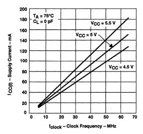
Figure 3. SN74ACT7814 Supply Current Versus Clock Frequency
