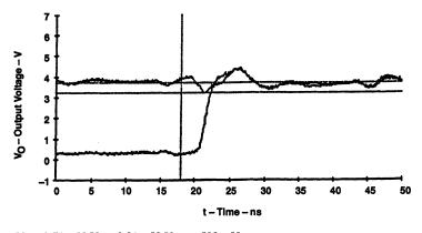
$V_1 = 3.71 \text{ mV}, V_2 = 3.21 \text{ mV}, V_D = -500 \text{ mV}$
