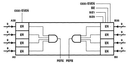
Figure 13. Parity-Checking Block Diagram
