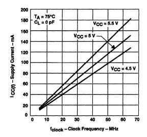
Figure 7. SN74ACT7813 Supply Current Versus Clock Frequency
