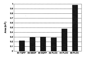
Figure 4. Surface-Mount Package Area Comparison
