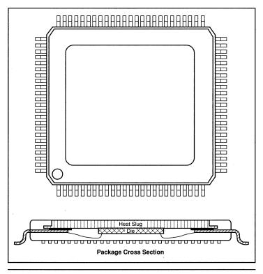
Figure 2. Package Outline Drawing — 100 TQFP TEP.
