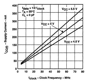
Figure 4. SN74ABT3614 Supply Current Versus Clock Frequency
