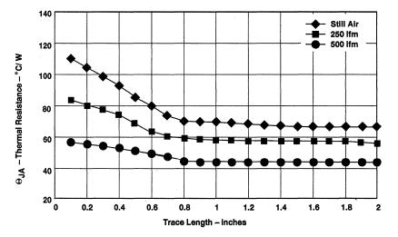
Figure 4. 52-Pin MQFP (trace length effect)
