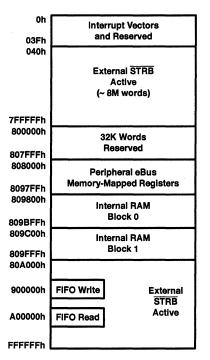
Figure 3. TMS320C31 Memory Map in Microprocessor Mode Showing Mailbox-Bypass Register and FIFO SRAM Addresses
