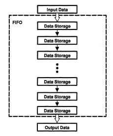
Figure 1. First-In, First-Out Data Flow
