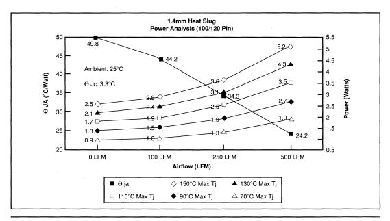
Figure 9. Power Dissipation at Selected Maximum Junction Temperatures.
