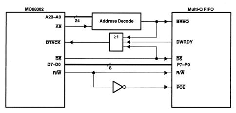
Figure 11. Connection of a Microcontroller to the Auxiliary Bus
