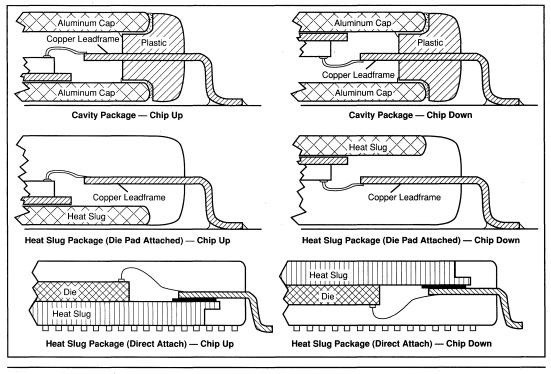
Figure 1. Package Configurations Considered.
