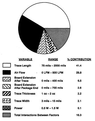
Figure 8. 48-/56-Pin SSOP K-Factor Board Modeling
