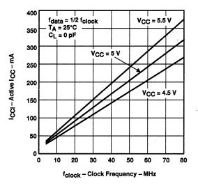
Figure 5. SN74ABT3614 Active I<sub>CC</sub> With CLKA and CLKB Switching, Simultaneous Read/Write and CLKB as Data Output
