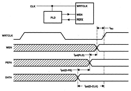
Figure 4. Parity-Error Exception Circuit
