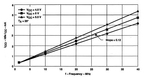
Figure A–1. SN74ACT7811 Idle I<sub>CC</sub> With RDCLK or WRTCLK Switching
