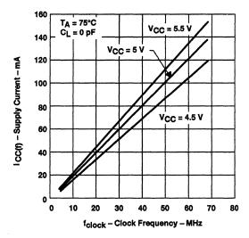
Figure 4. SN74ACT7808 Supply Current Versus Frequency
