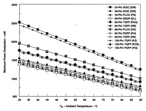
Figure 1. Comparison Summary of Advanced Packaging Derating Curves (in still air)
