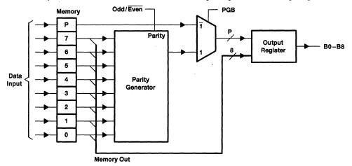
Figure 1. Parity-Generate Circuit
