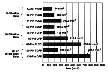
Figure 2. Surface-Mount Package Area Comparison
