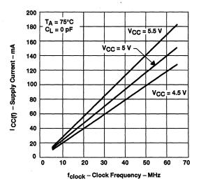
Figure 2. SN74ACT7806 Supply Current Versus Clock Frequency
