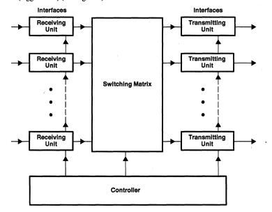
Figure 2. ATM Telecommunications Exchange System Block Diagram
