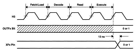
Figure 6. Retransmit Timing for Interconnection Example
