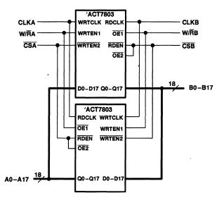
Figure 5. Bidirectional Configuration for the SN74ACT7803
