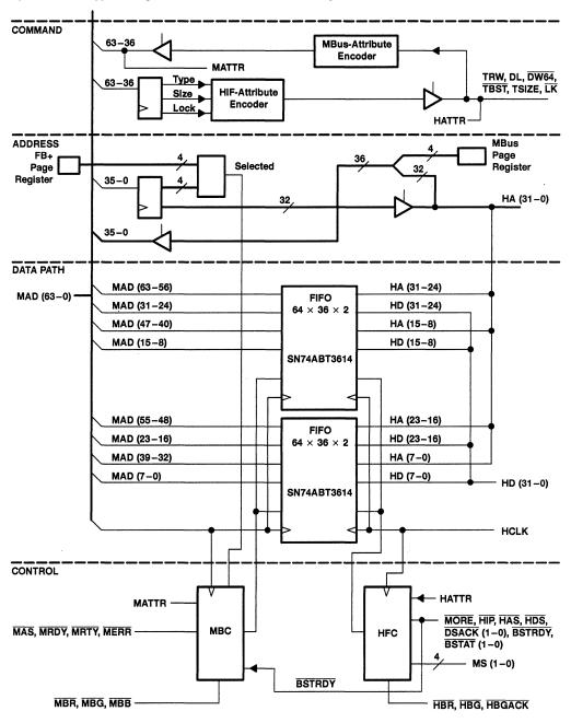
Figure 2 shows suggested implementation of the MBus to HIF bridge.
