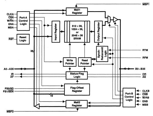
Figure 1. SN74ACT3641 FIFO Functional Block Diagram
