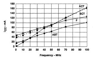
Figure 3. I<sub>CC</sub> Versus Frequency (All Outputs Switching)
