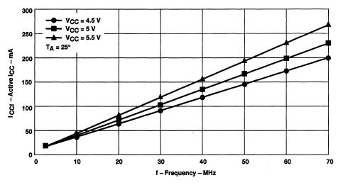
Figure 4. SN74ACT3632 Active I<sub>CC</sub> Versus Frequency
