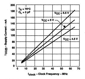
Figure 6. SN74ACT7805 Supply Current Versus Clock Frequency
