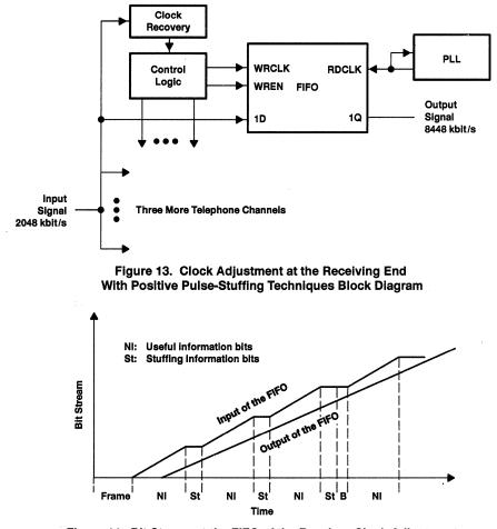
Figure 14. Bit Stream at the FIFO of the Receiver-Clock Adjustment
