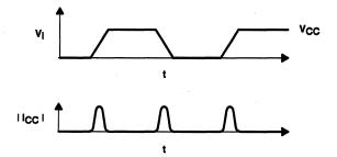
Figure 2. Current Waveform Supplied by V<sub>CC</sub> to a CMOS Gate
