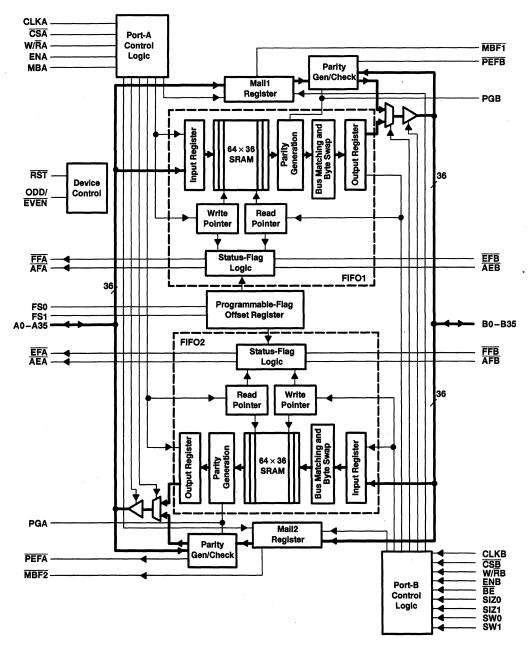
Figure 1. SN74ABT3614 Functional Block Diagram
