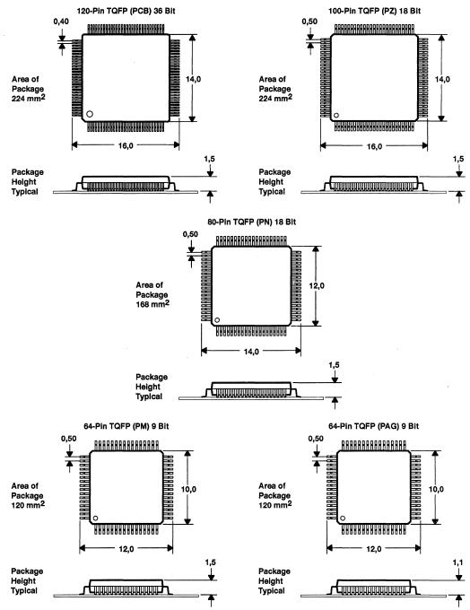
NOTE: Dimensions are in millimeters.
