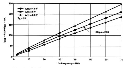
Figure A–5. SN74ACT3641 Active I<sub>CC</sub> With CLKA and CLKB Switching, Simultaneous Read/Write and CLKB as Data Output
