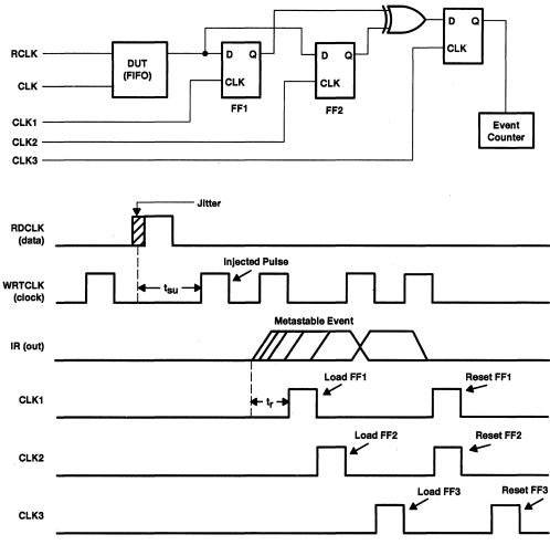
Figure 4. Metastable Event Counter and Input Waveforms
