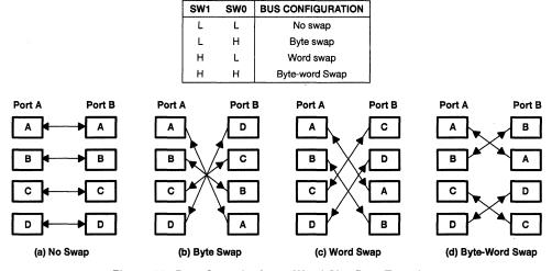
Table 2. Control of Byte-Swap Operation on Port B Using SW1 and SW0
