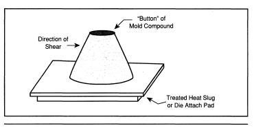
Figure 4. "Button" Shear Test Setup.
