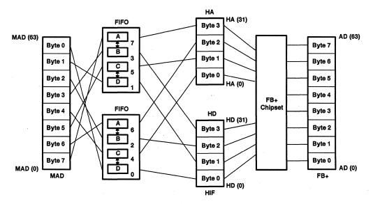
Figure 5. Byte-Lane Mapping for a 64-/32-Bit System
