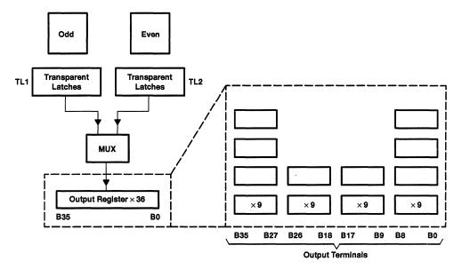
Figure 5. Pipeline Registers
