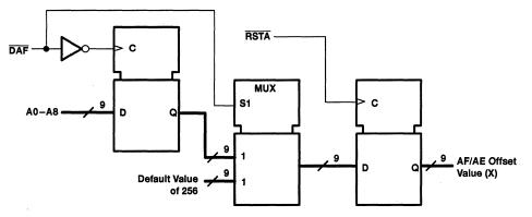
Figure 4. AF/AEA Flag-Programming Logic for FIFOA
