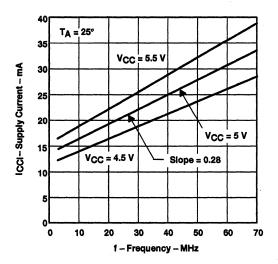
Figure 6. SN74ABT3614 Idle Current With CLKB Switching, Other Inputs at 0 or  $V_{CC}$  – 0.2 V and Outputs Disconnected
