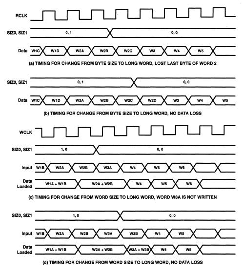
Figure 10. Dynamically Changing Byte-/Word-Size Transfers to Long-Word Data Transfers
