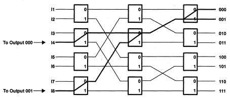
Figure 21. Switching Matrix With Bottleneck Between Two Switching Elements
