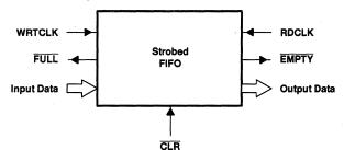
Figure 2. Connections of a Strobed FIFO
