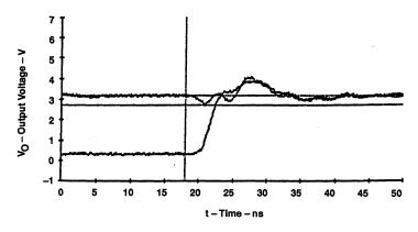
$V_1 = 3.18 V, V_2 = 2.71 V, V_D = -468.75 mV$
