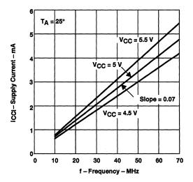
Figure 2. SN74ACT7807 Idle Current With WRTCLK Switching, Other Inputs at 0 or  $V_{CC}$  – 0.2 V and Outputs Disconnected
