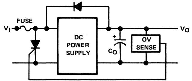
Figure 6-71. Typical Crowbar Circuit
