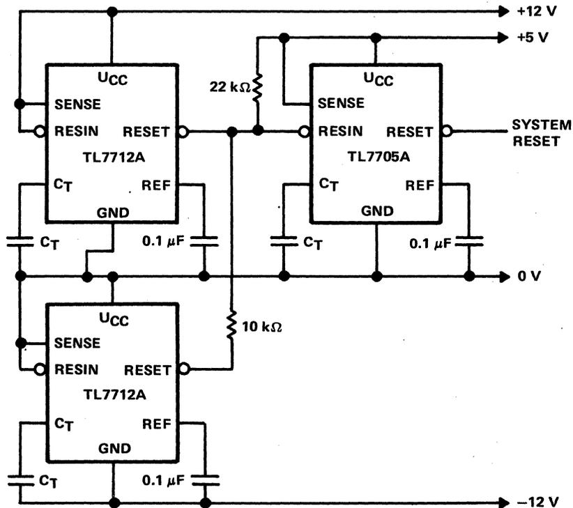
Figure 6-60. Voltage Supervision of a Multiple Power Supply
