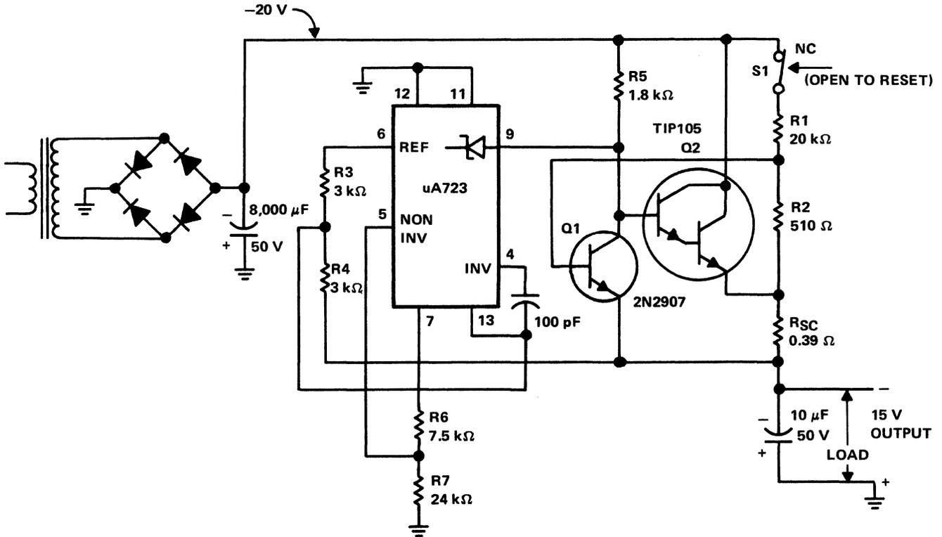
Figure 6-69. -15-Volts at 1.0-Amp Regulated Power Supply
