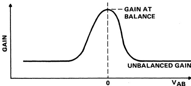
Figure 3-4. Gain as a Function of  $V_{AB}$
