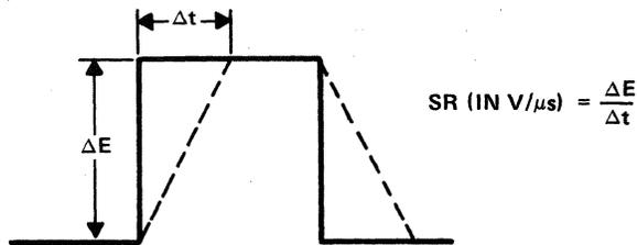
NOTE: Solid line is a square-wave input. Broken line is slewed output.
