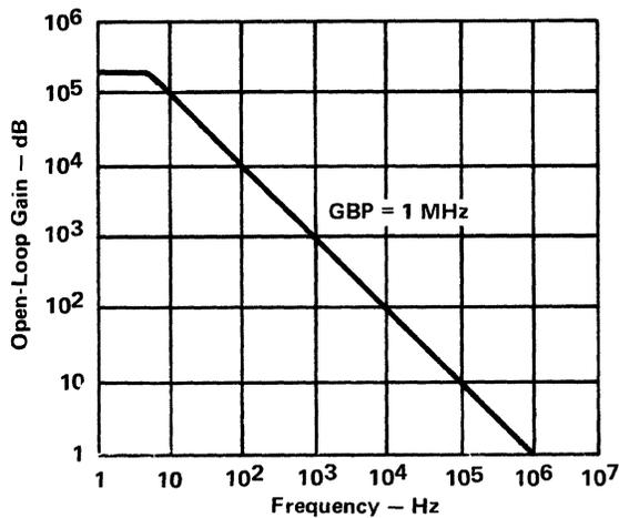
Gain-Bandwidth Product = Closed-Loop Gain X Frequency Response
