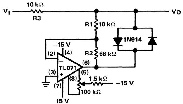
Figure 3-7. Low-Voltage Shunt Limiter
