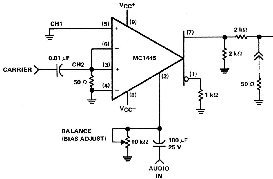
Figure 4-8. Balanced Modulator
