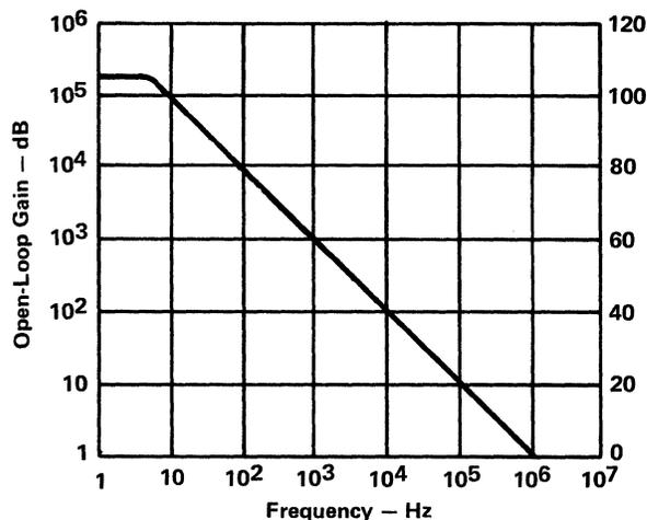
Figure 2-3. TL321 Operational Amplifier Bandwidth
