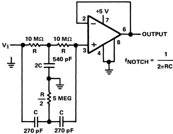
Figure 3-42. Twin-T Notch Filter for 60 Hz
