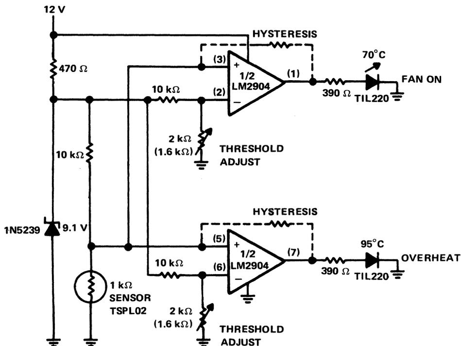
Figure 3-11. PTC Sensor Automotive Temperature Control Circuit
