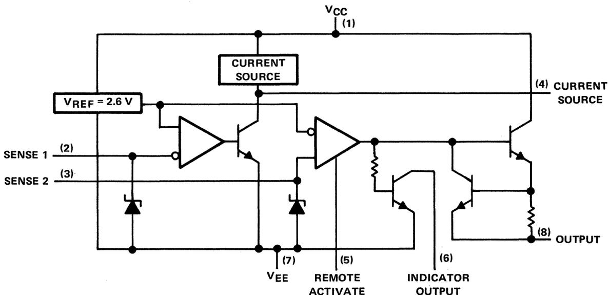
Figure 6-70. MC3423 Overvoltage Crowbar Sensing Circuit Block Diagram
