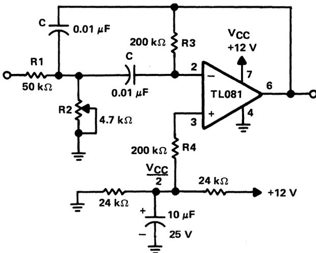
Figure 3-15. Two Pole Active Band-Pass Filter
