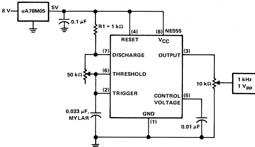
Figure 7-21. Oscilloscope Calibrator
