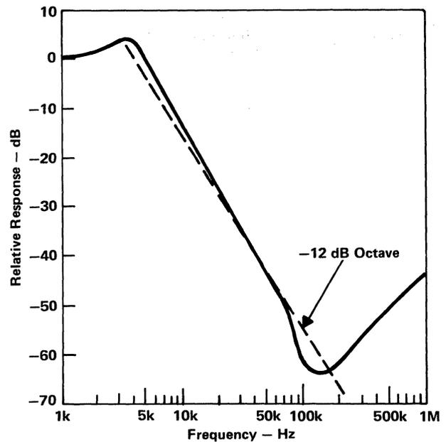
Figure 2-27. Response Curve of a Low-Pass Active Filter
