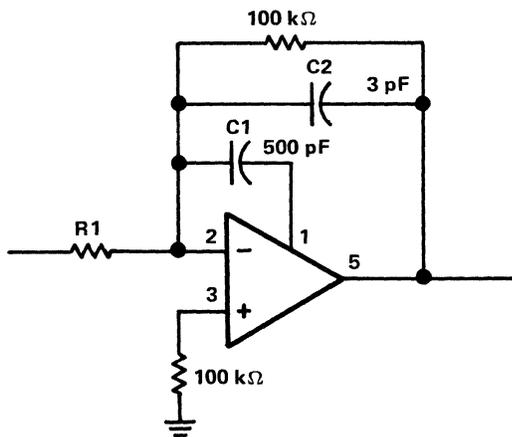
Figure 2-13. Feed-Forward Compensation
