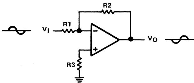
Figure 2-18. Inverting Amplifier with DC Offset Correction
