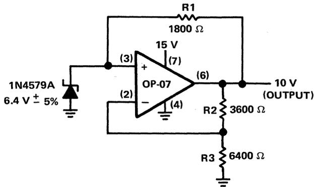
**Figure 3-12. Accurate 10-Volt Reference Circuit**
