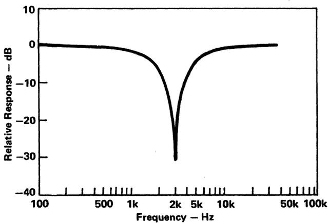
Figure 2-31. Response Curve of Band-Reject Active Filter
