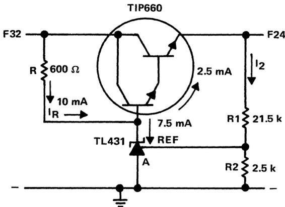
Figure 6-43. Series Regulator Circuit
