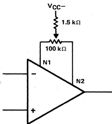
Figure 2-7. Null Pins Connected to Emitters
