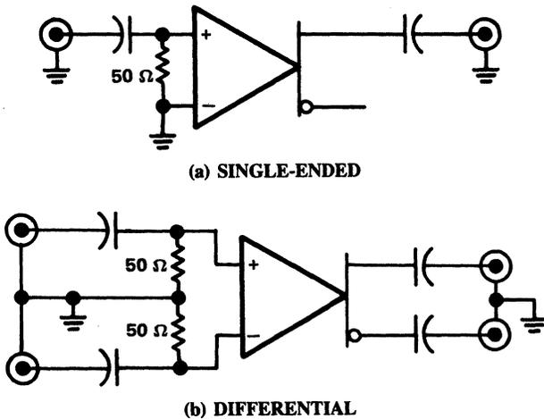
Figure 4-4. Coupling Methods
