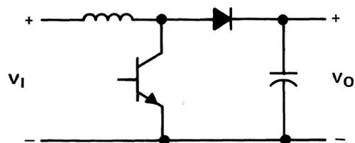
Figure 6-3. Step-Up or "Boost" Switching Regulator Circuit
