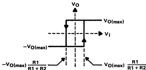
Figure 3-9. Voltage-Follower Schmitt Trigger
