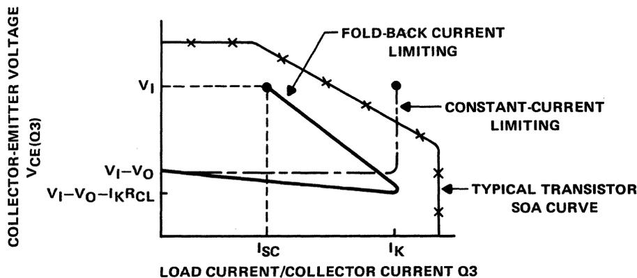
Figure 5-35. Fold-Back Current Limit Safe Operating Area
