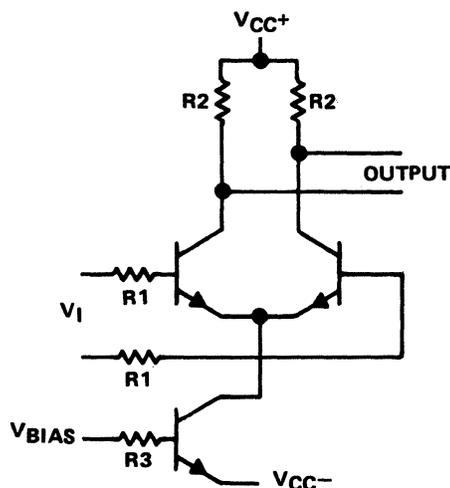
Figure 4-1. Basic Video Amplifier Circuit
