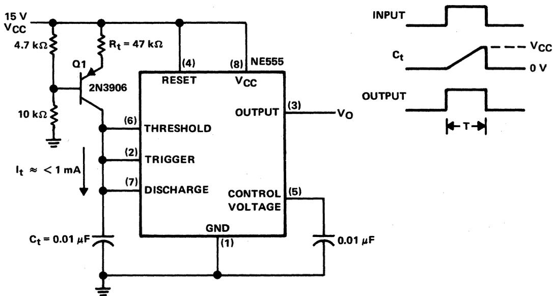
Figure 7-25. Linear Ramp Generator
