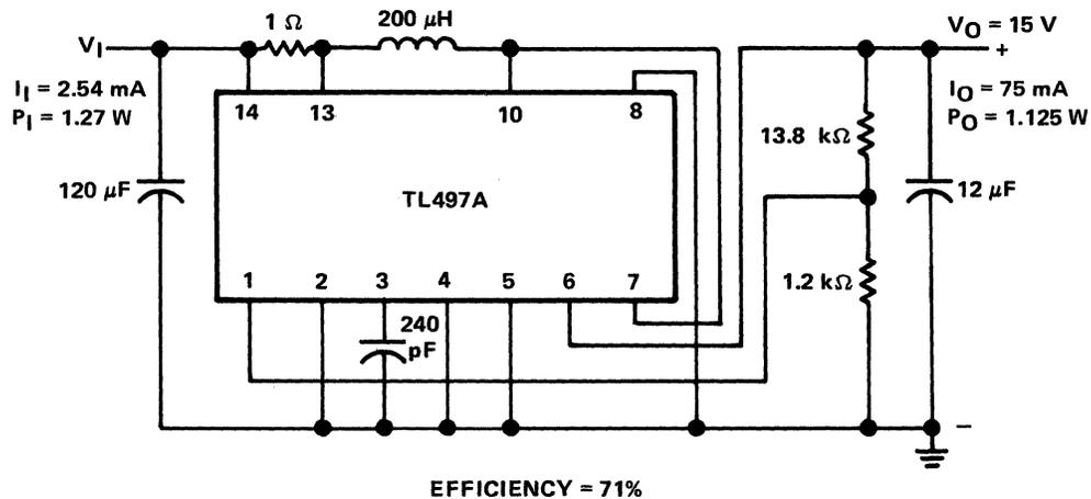
Figure 6-37. 5-Volt to 15-Volt Switching Regulator
