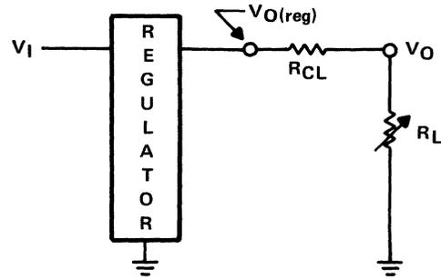
Figure 5-28. Series Resistance Current Limiter
