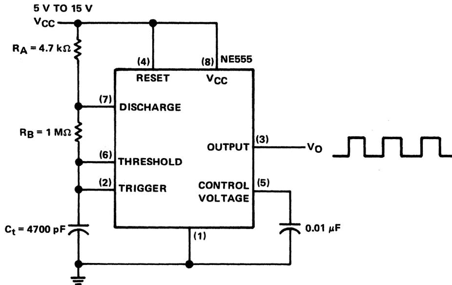
Figure 7-24. Basic Square Wave Oscillator
