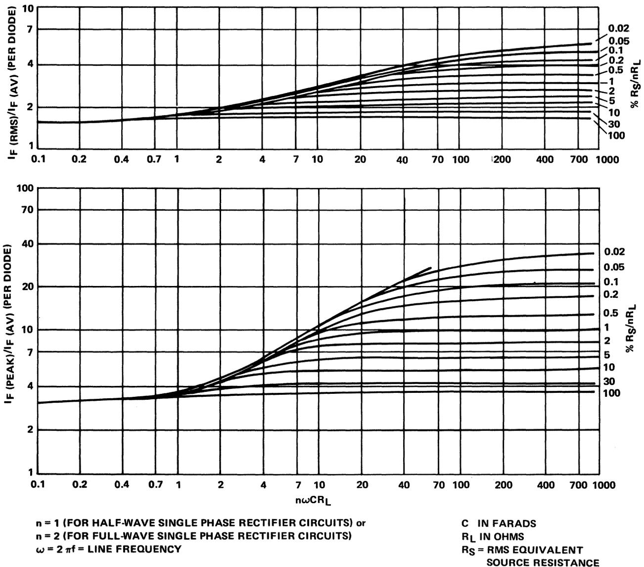
Figure 5-47. Relation of RMS and Peak to Average Diode Current in Capacitor Input Circuits
