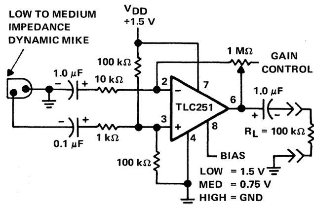
Figure 3-37. Microphone Preamplifier
