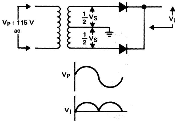
Figure 6-49. Full-Wave Rectifier Section of Circuit
