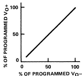
Figure 5-16. Dual Tracking Regulator
