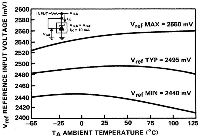
Figure 6-41. Reference Input Voltage Versus Ambient Temperature
