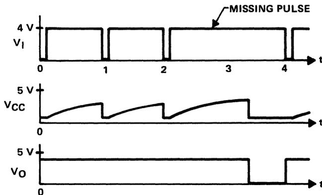
Figure 7-18. Missing Pulse Detector Waveforms
