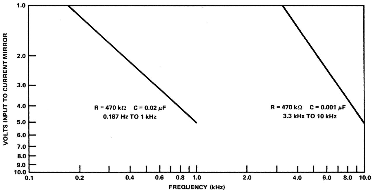
Figure 7-31. Voltage-Controlled Oscillator Frequency vs Voltage
