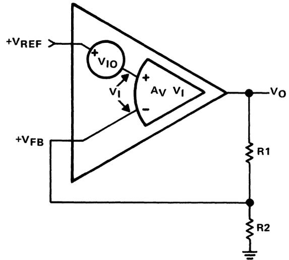
Figure 5-11. Amplifier Model Showing Input Offset Voltage Effect
