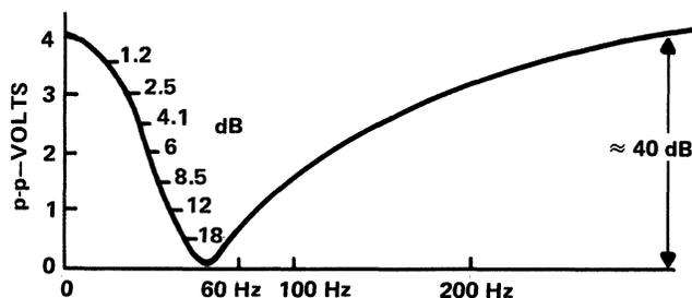
Figure 3-25. 60 Hz Twin-T Notch Filter Response
