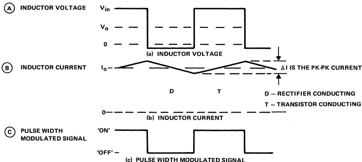
Figure 6-12. 12-Volt to 5-Volt Series Switching Regulator Waveforms
