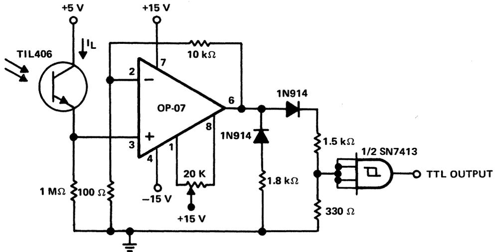
Figure 3-1. Optical Sensor to TTL Interface Circuit
