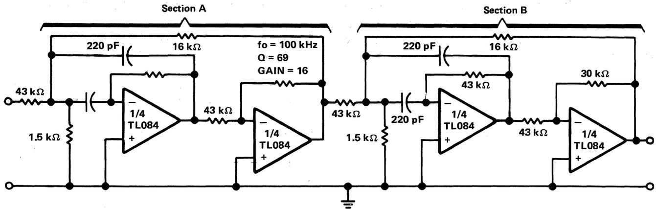
Figure 3-21. Positive Feedback Band-Pass Filter
