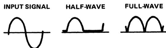
Figure 5-44. Rectifier Output-Voltage Waveforms
