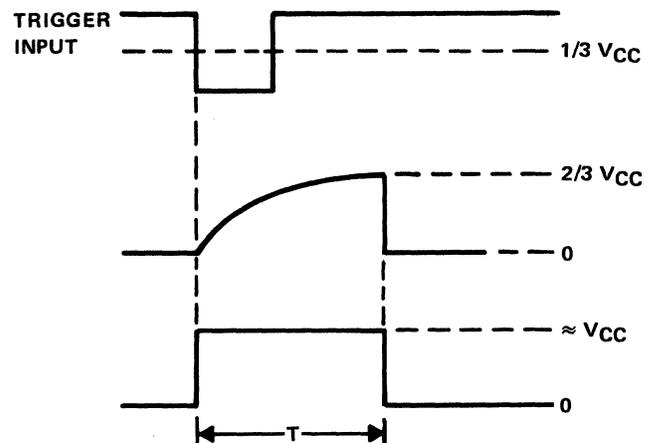
Figure 7-20. NE555 One-Shot Timing Diagram
