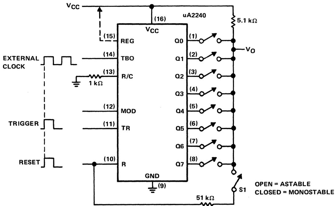
Figure 7-44. Operation with External Clock
