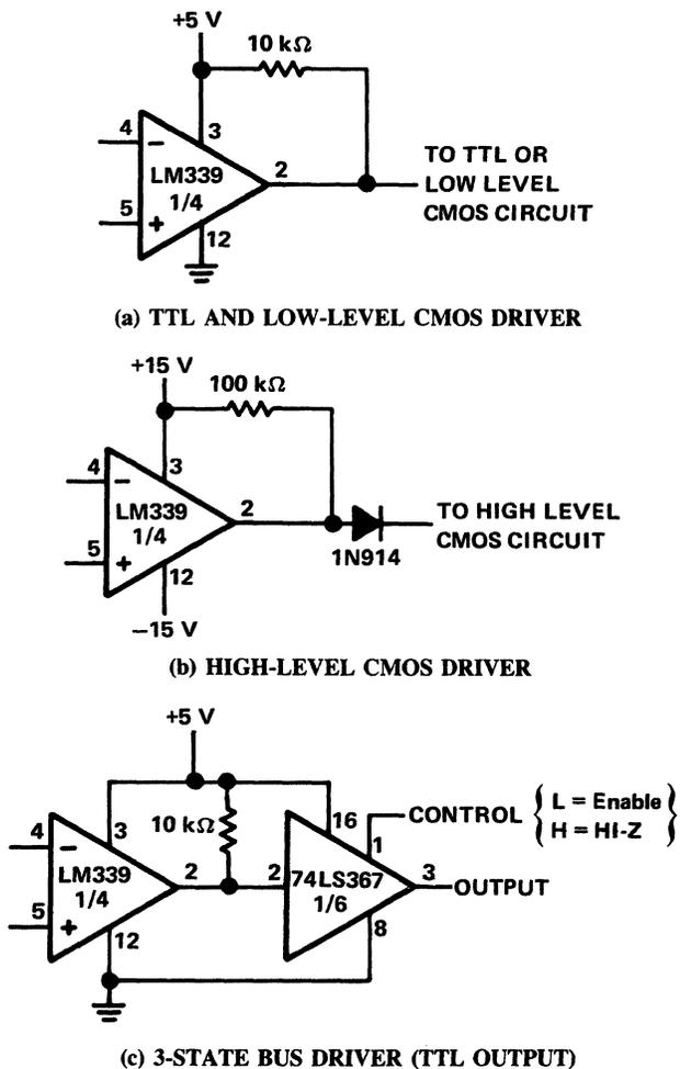
Figure 3-50. Comparator Logic Interface Circuits
