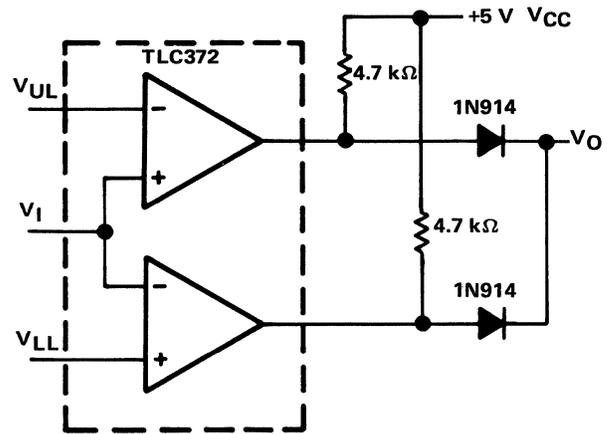
Figure 3-46. Basic Window Comparator
