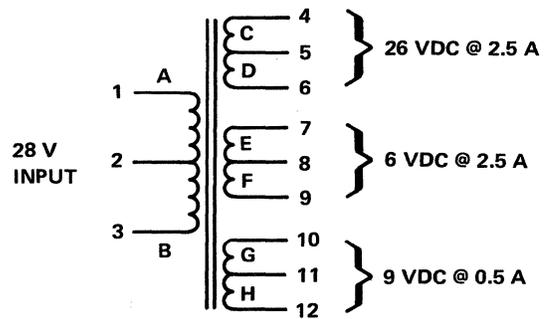
Figure 6-10. Transformer Winding Layout
