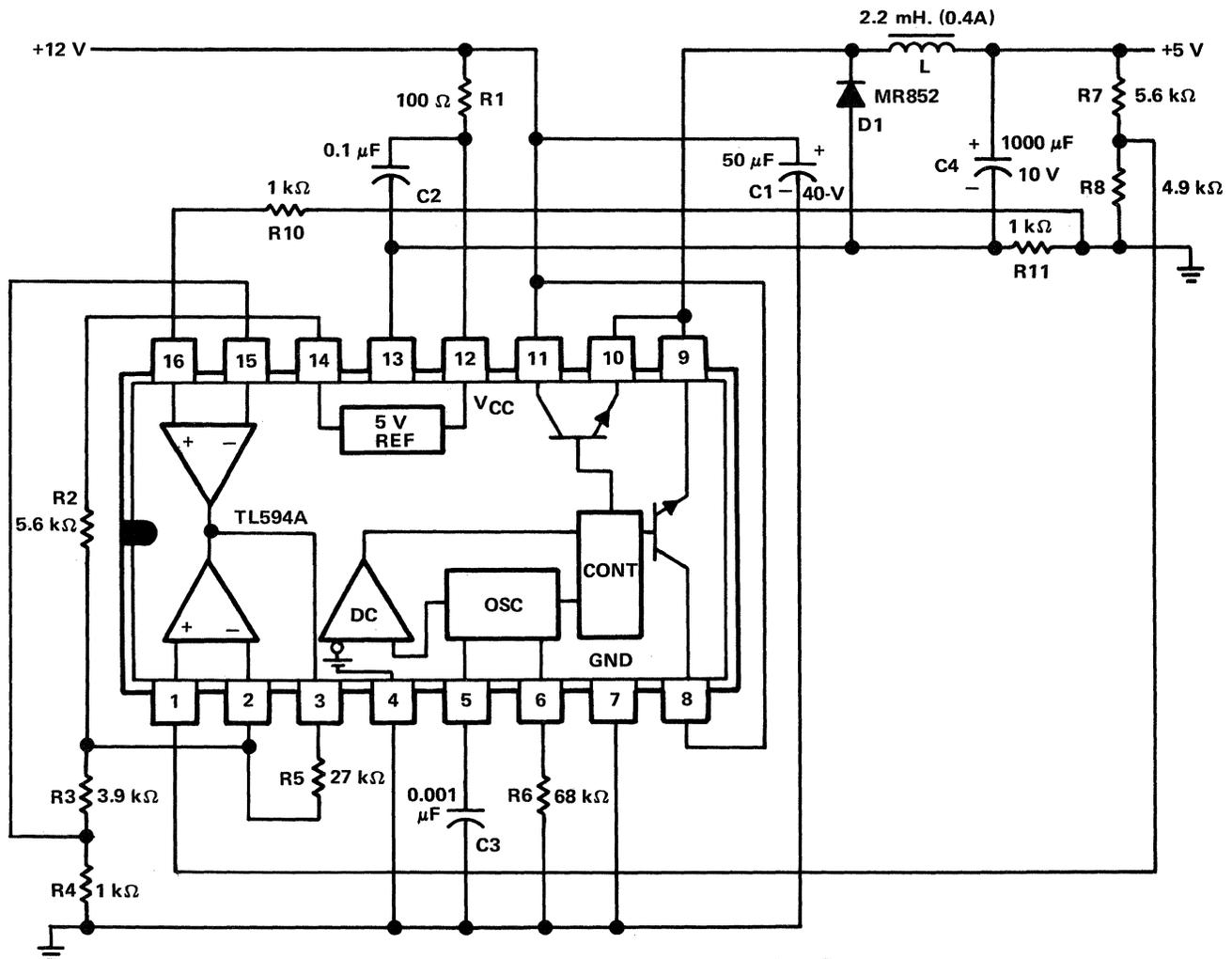
Figure 6-11. TL594 12-Volt to 5-Volt Step-Down Regulator
