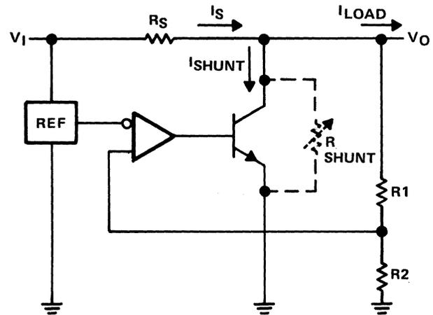
Figure 5-4. Basic Shunt Regulator
