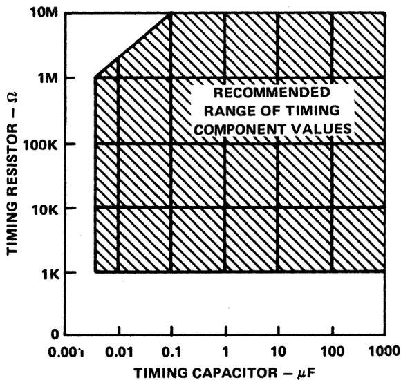
Figure 7-10. Recommended Range of Timing Component Values
