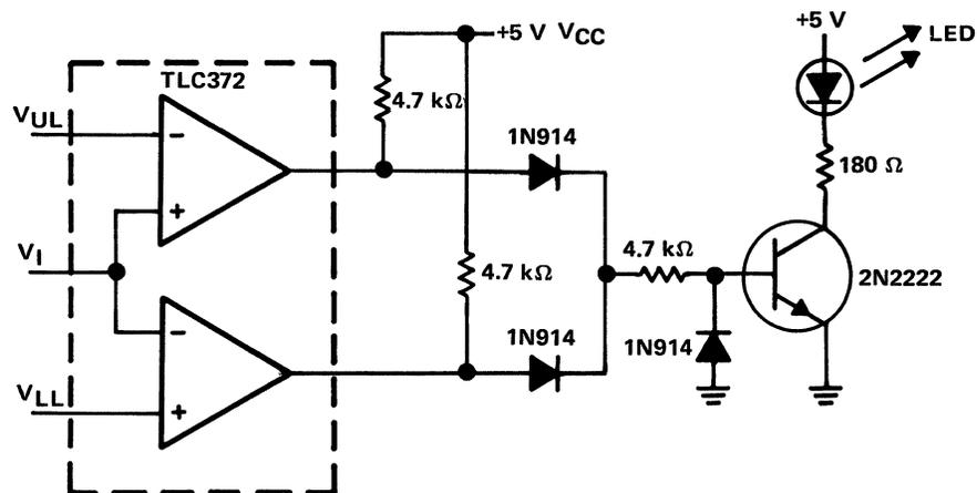
Figure 3-47. Window Comparator with LED Indicator
