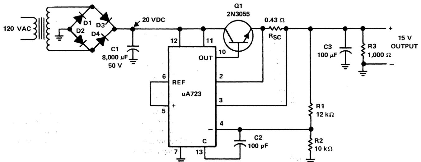
Figure 6-68. +15-Volts at 1.0-Amp Regulated Power Supply
