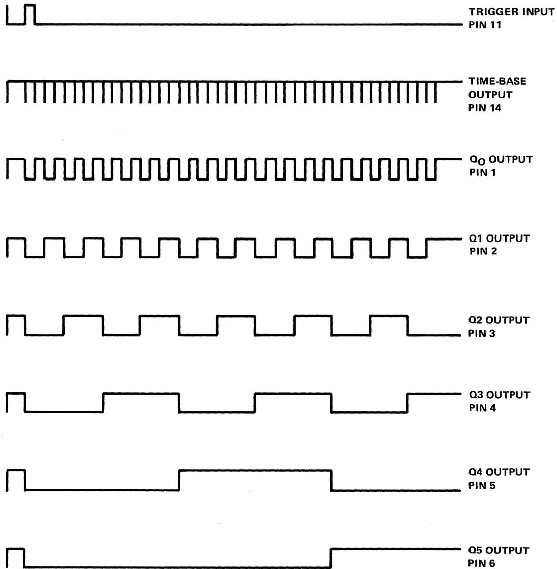
Figure 7-14. Timing Diagrams of Output Waveforms
