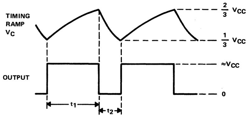
Figure 7-5(b). NE555 Astable Timing Diagram
