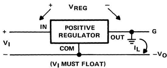
Figure 5-14. Positive Regulator in Negative Configuration ( $V_1$  Must Float)
