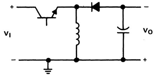
**Figure 6-4. Inverting or “Flyback” Switching Regulator Circuit**
