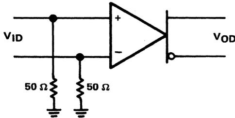
Figure 4-2. Differential Voltage Gain
