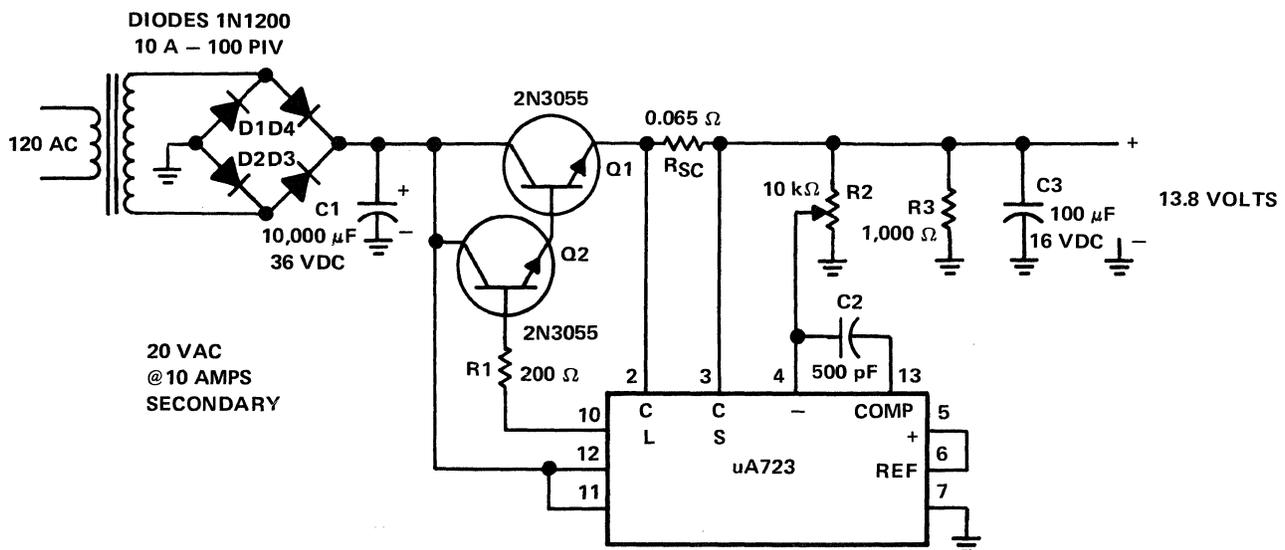
Figure 6-67. 8-Amp Regulated Power Supply
