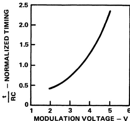
Figure 7-40. Modulation Voltage Control of Time-Base Period
