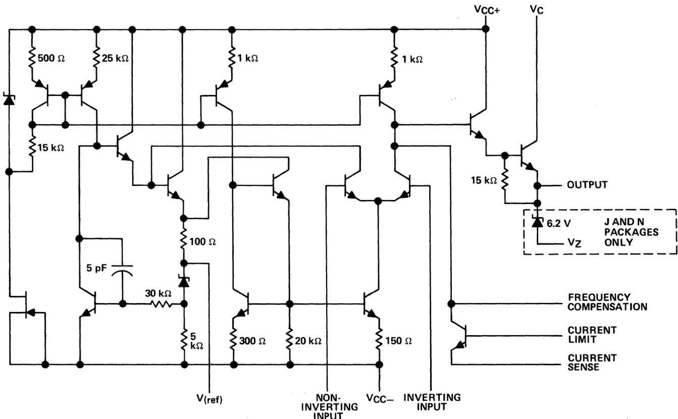
Figure 6-64. uA723 Schematic
