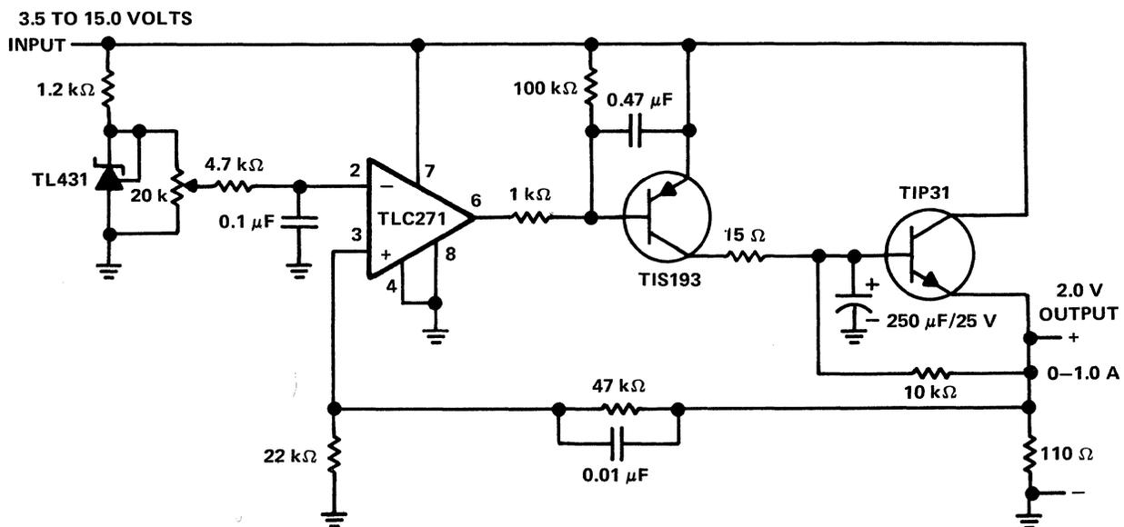
Figure 3-41. TLC271 Logic Array Power Supply
