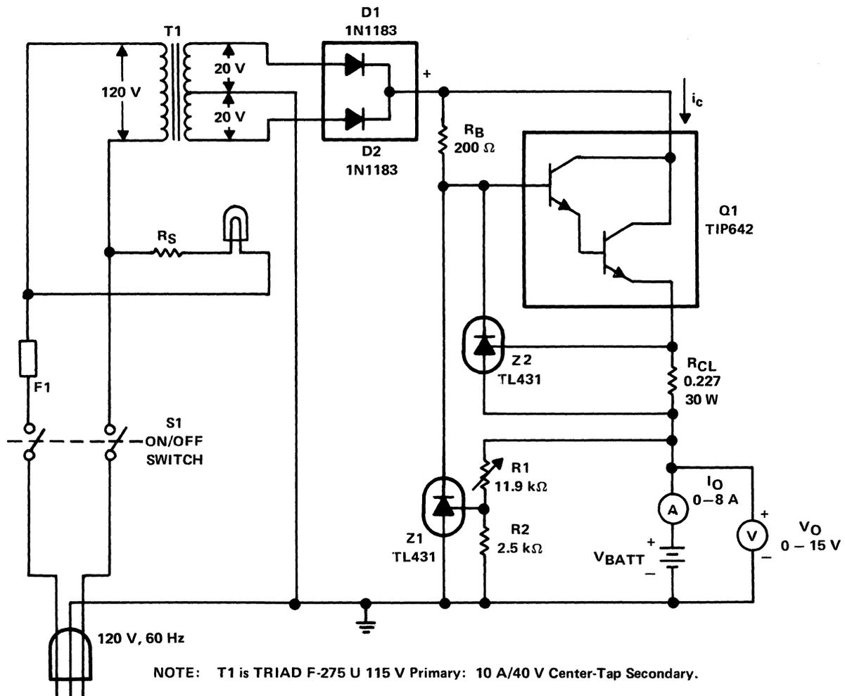
Figure 6-48. Current Limited and Voltage Regulated Battery Charger
