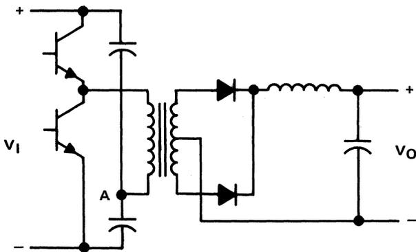
Figure 6-7. Half Bridge Converter Circuit
