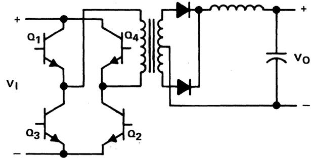
Figure 6-8. Full Bridge Converter Circuit
