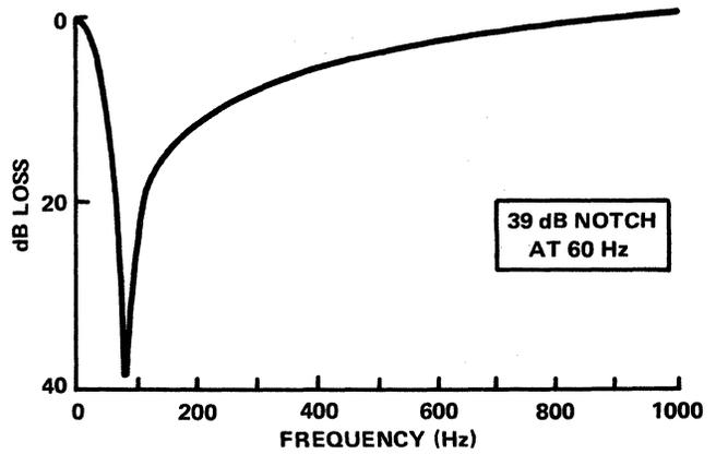
Figure 3-43. TLC271 Twin-T Notch Filter Frequency Response
