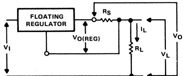
Figure 5-19. Floating Regulator as a Constant-Current Regulator
