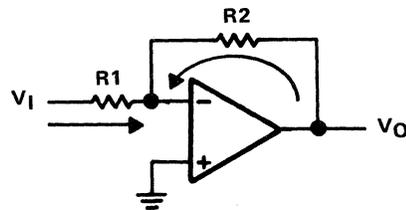
Figure 2-17. Inverting Amplifier with Input Bias Currents
