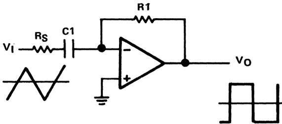
Figure 2-23. Differentiator with High Frequency Noise Correction
