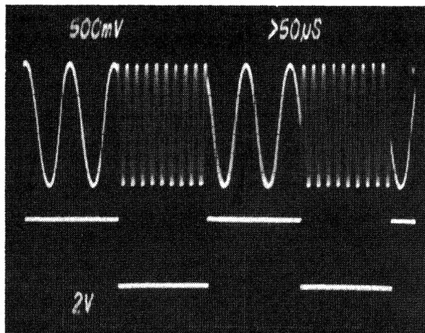
Figure 4-13. FSK Output and Gate Input Signal Waveforms
