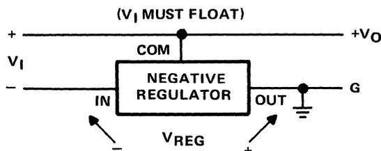
Figure 5-15. Negative Regulator in Positive Configuration ( $V_1$  Must Float)
