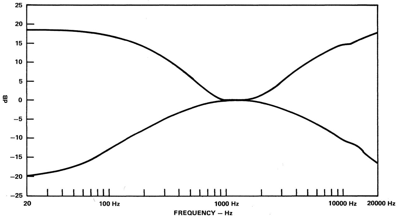
Figure 3-27. Preamp Frequency Response
