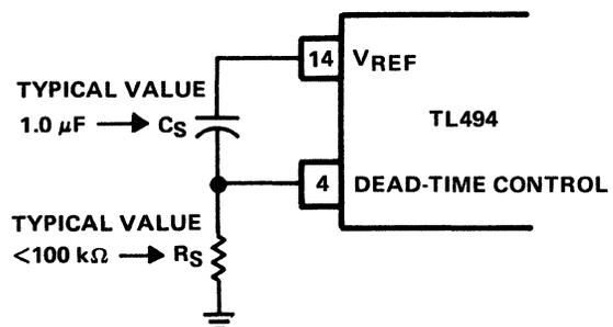
Figure 6-17. Soft-Start Circuit
