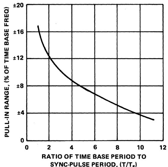
Figure 7-12. Typical Pull-In Range for Harmonic Synchronization
