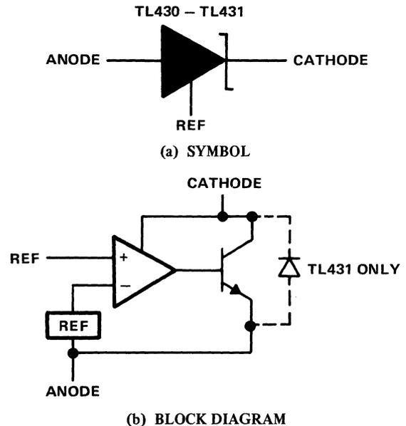
Figure 6-39. TL430/TL431 Adjustable Shunt Regulators
