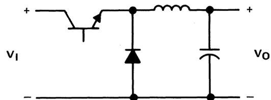
Figure 6-2. Step-Down or "Buck" Switching Regulator Circuit
