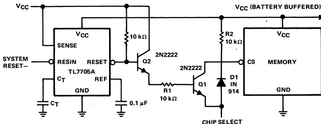
Figure 6-62. Circuit Diagram for Memory Protection
