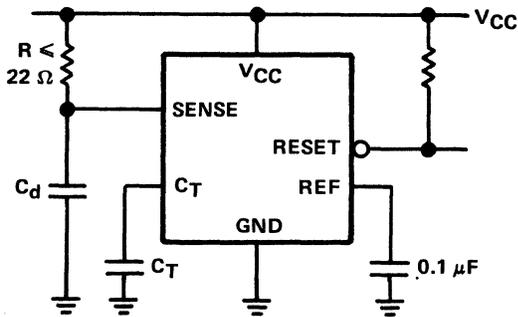
Figure 6-61. Delayed Triggering
