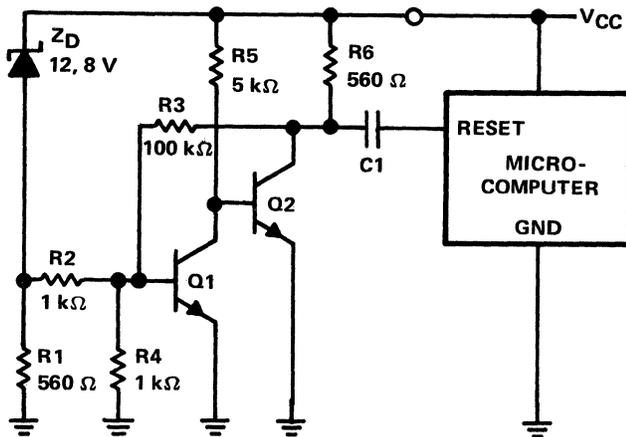
Figure 6-54. Discrete Solution of a Voltage Supply Supervisor
