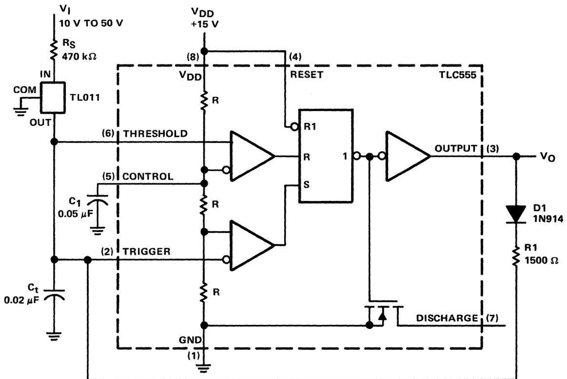
Figure 7-30. Voltage-Controlled Oscillator
