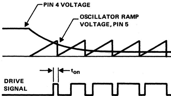
Figure 6-23. Soft-Start Circuit
