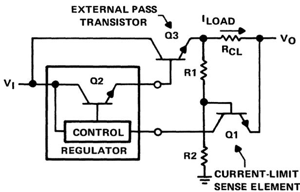
Figure 5-34. Fold-Back Current Limit Configuration
