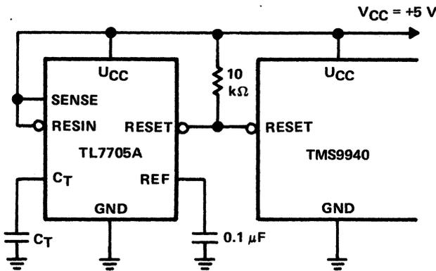
Figure 6-58. TL7705A in 5-Volt Microcomputer Application
