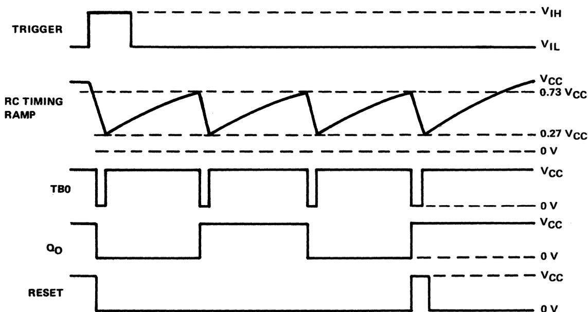
Figure 7-13. Timing Diagram
