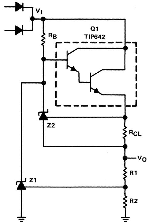
Figure 6-52. Series Pass Element
