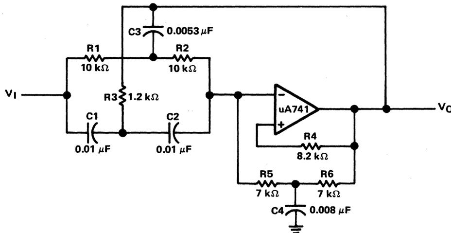
Figure 2-30. Band-Reject Active Filter
