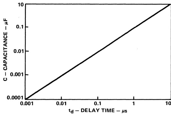
Figure 6-74. Capacitance vs Minimum Overvoltage Duration
