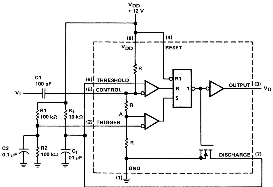
Figure 7-29. Positive-Triggered Monostable
