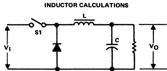
Figure 6-24. Switching Circuit
