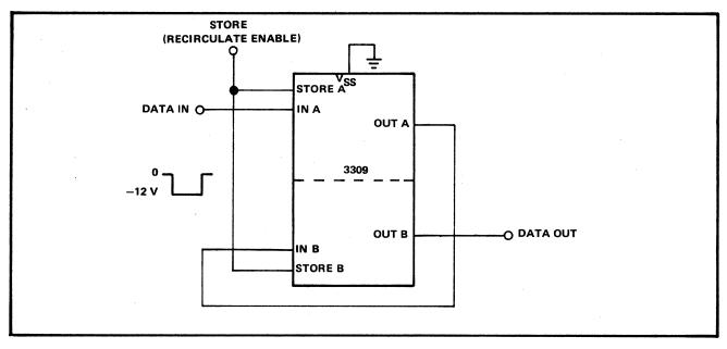
NOTE: In this figure the register has been connected as a 1024-bit shift register.
