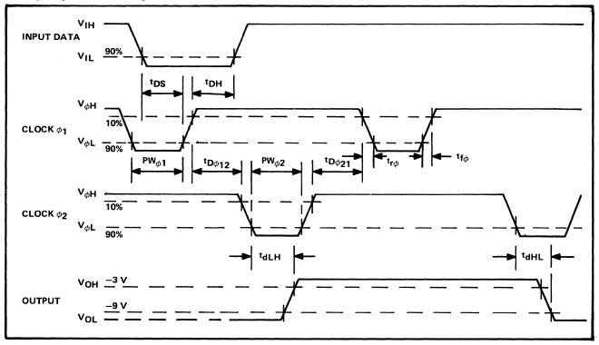
timing diagram and voltage waveforms
