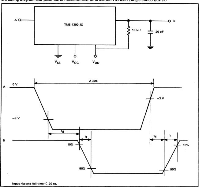
switching diagram and parametric measurement information RC load (single-ended buffer)
