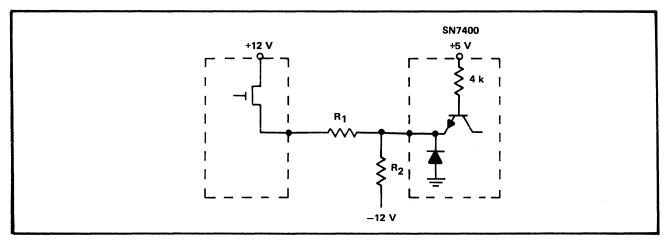
$R_2$  provides the necessary current sink for the TTL input,  $R_1$  limits the positive excursion to +5 V. If used for low threshold MOS,  $V_{SS}$  is translated up to +5 V instead of +12 V and  $R_1$  can be eliminated. If  $R_2$  is on the chip no external components are necessary.
