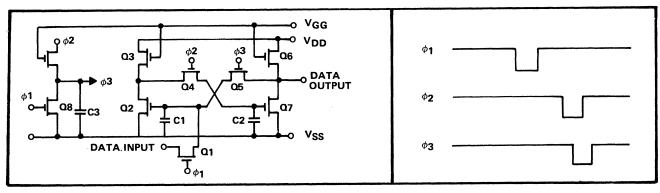
Basic cell of static shift register and  $\phi$ 3 internal generation
