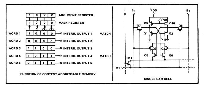
A content-addressable memory (CAM) is one in which the words it contains can all be matched simultaneously against an argument word and outputs given wherever a true match is obtained. Each word has a Write input which can also be used to interrogate that word for a match. Two bit lines run through each column of cells allowing the word data to be written in. They may also be used for reading the contents of a word or for masking parts of the argument word where a Don't Care state exists.
