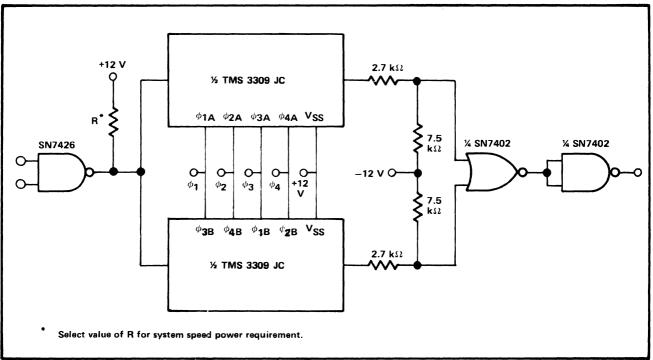
twin 512-bit dynamic shift register/accumulator multiplexing of TMS 3309 JC, 10-MHz operation
