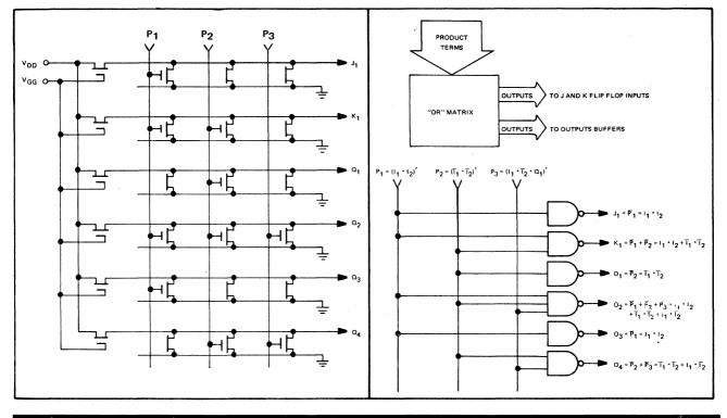
The AND matrix feeds into the OR matrix. The OR matrix generates sums of product terms. Some of the outputs of the OR matrix are fed to the outside while others are fed back to the first matrix (AND) through flip-flops.
