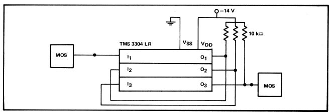
To demonstrate MOS interface the register has been connected as a 198-bit shift register.
