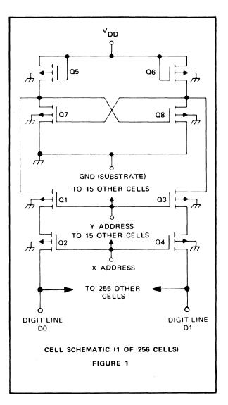
synchronously or asynchronously pulsing the  $V_{DD}$  power supply. This feature is a result of the temporary data storage provided by the gate capacitance of transistors Q7 and Q8.
