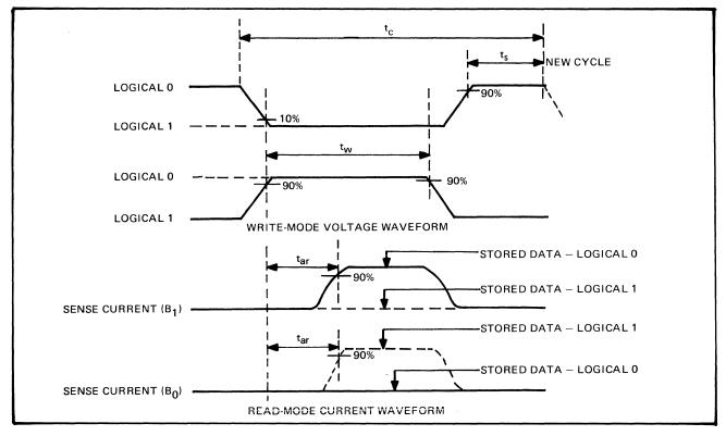
typical switching waveforms (read and write)
