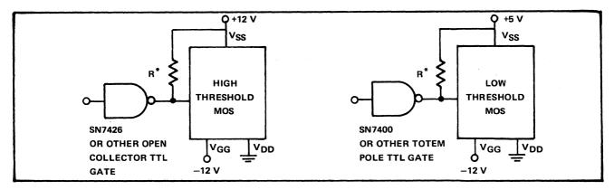
The value of the R\* resistor varies depending on speed-power requirements. In many cases this resistor is diffused on the MOS chip. For low threshold MOS this resistor assures that the worst case TTL output (2.4 V) is pulled up to at least 3.5 V for proper MOS circuit operation.
