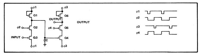
4 phase shift register basic cell and timing diagram
