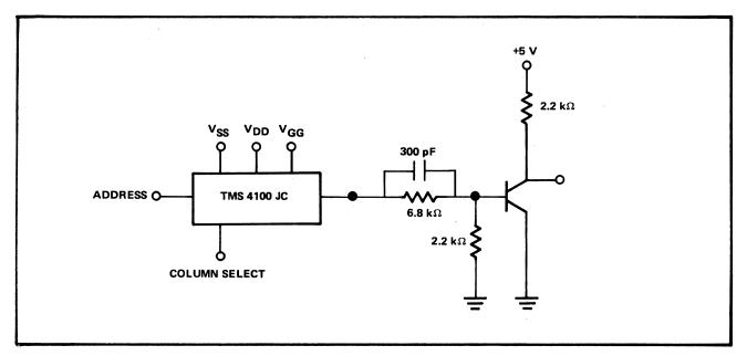
Address column select input voltage
