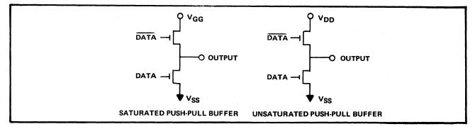
The unsaturated push-pull buffer is the most commonly used for low threshold circuits. It permits direct TTL compatibility without external components.
