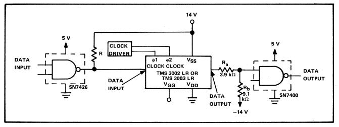
An input pull-up resistor is required to provide the necessary input voltage swing. The value of this resistor (R) depends on the actual circuit requirements – values as low as 1 k $\Omega$  can be used for high-speed operation while values as high as 15 k $\Omega$  can be used when low power consumption is important rather than high-speed.
