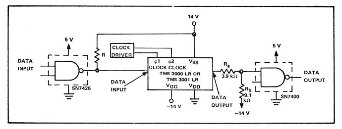
An input pull-up resistor is required to provide the necessary input voltage swing. The value of this resistor (R) depends on the actual circuit requirements – values as low as 1 k $\Omega$  can be used for high-speed operation while values as high as 15 k $\Omega$  can be used when low power consumption is important rather than high-speed.
