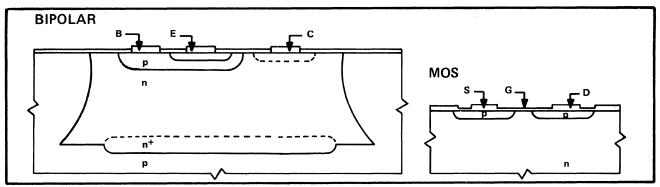
COMPARISON OF TRANSISTOR CROSS SECTIONS
