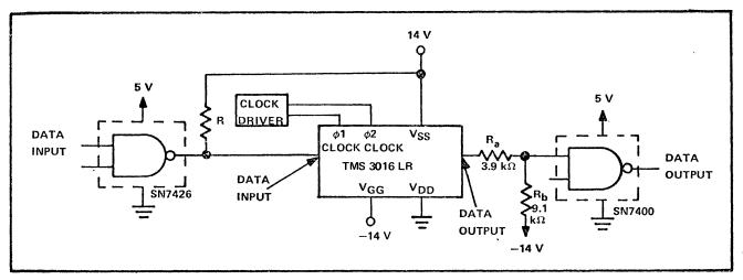
An input pull-up resistor is required to provide the necessary input voltage swing. The value of this resistor (R) depends on the actual circuit requirements – values as low as  $1 \text{ k}\Omega$  can be used for high-speed operation while values as high as  $15 \text{ k}\Omega$  can be used when low power consumption is important rather than high-speed.
