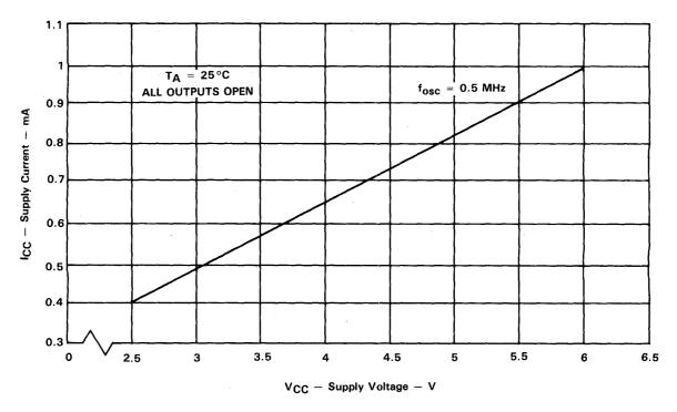
Figure 4-42. Typical Operating ICC vs. Oscillator Frequency
