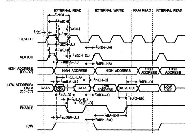
Figure 4-17. Read and Write Cycle Timing
