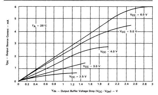
Figure 4-44. Typical Output Source Characteristics
