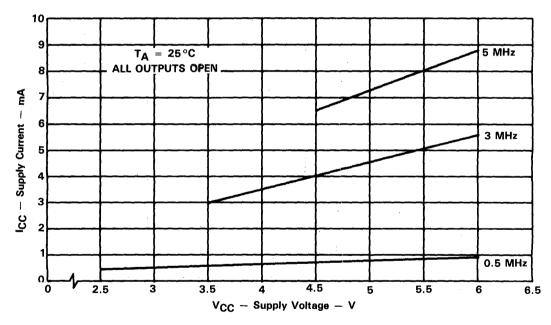
Figure 4-28. Typical Operating Current vs. Supply Voltage
