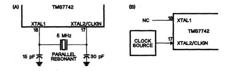
Figure 4-16. Recommended Clock Connections
