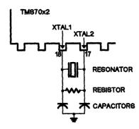
Figure 4-12. Ceramic Resonator Circuit
