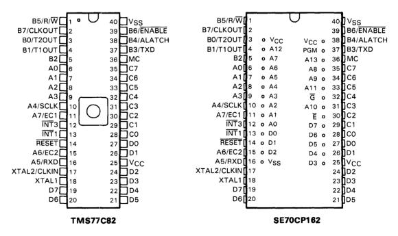
Figure 2-6. Prototyping Devices Available for TMS70Cx2 and TMS77C82 Devices
