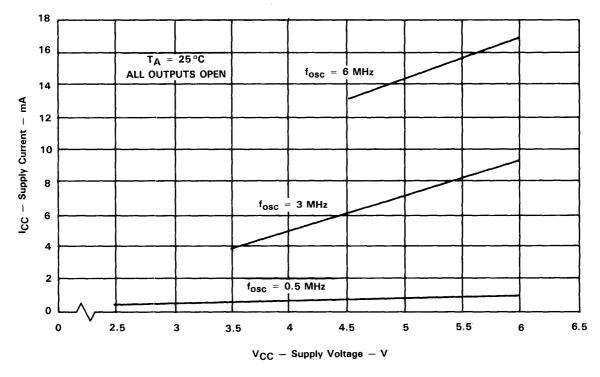
Figure 4-41. Typical Operating Current vs. Supply Voltage
