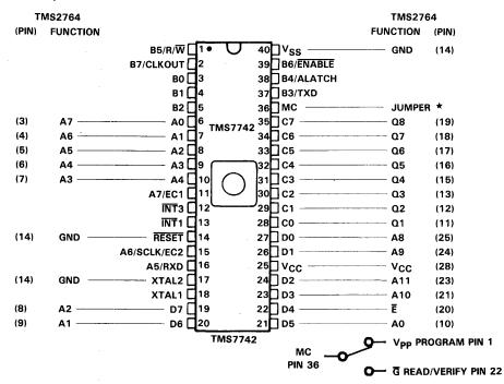
Figure 9-3. RTC/EVM7000 40-to-28-Pin Conversion Socket
