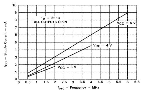
Figure 4-30. Typical Operating ICC vs. Oscillator Frequency
