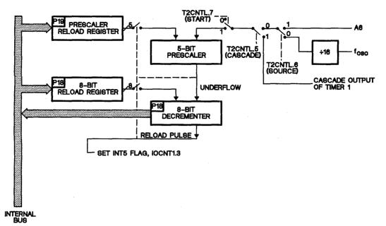
Figure 3-23. 8-Bit Programmable Timer/Event Counters - Timer 2 (TMS70x2)
