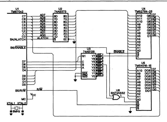
Figure 9-1. TMS70x2 Microprocessor Interface Sample Circuit
