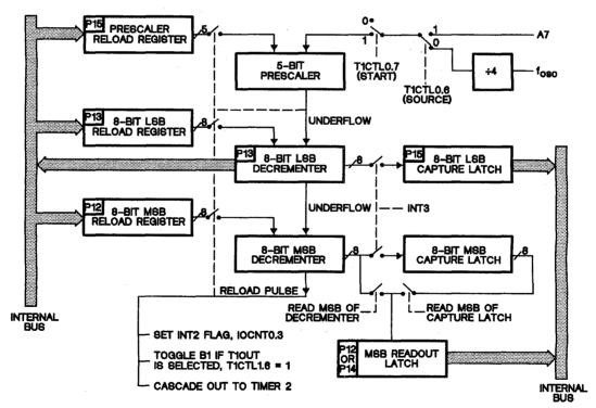
Figure 3-20. 16-Bit Programmable Timer/Event Counters - Timer 1 (TMS70Cx2)
