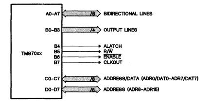
Figure 3-9. I/O Ports - Full-Expansion Mode
