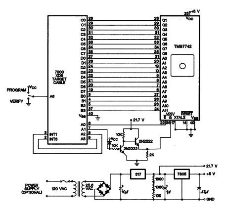
Figure 9-4. Interface Circuit for Programming the TMS7742 with the TMS7000 XDS
