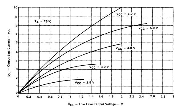
Figure 4-45. Typical Output Sink Characteristics
