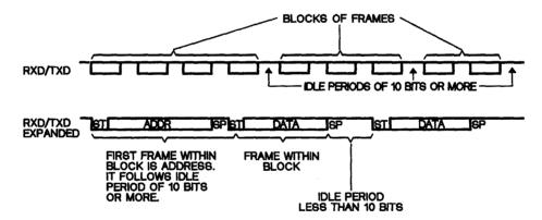
Figure 3-39. Motorola Multiprocessor Communication Format
