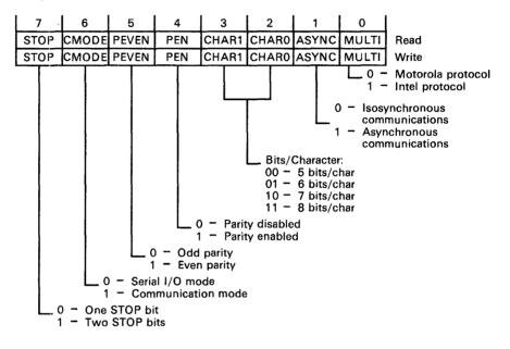
Figure 3-28. Serial Mode Register - SMODE
