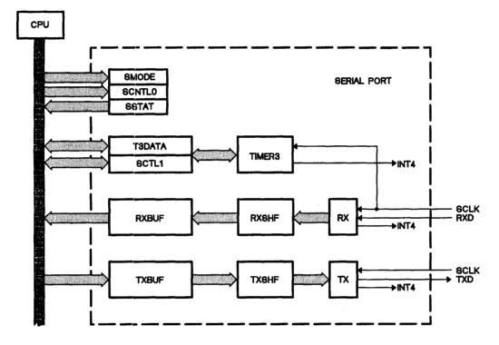
Figure 3-27. Serial Port Functional Blocks
