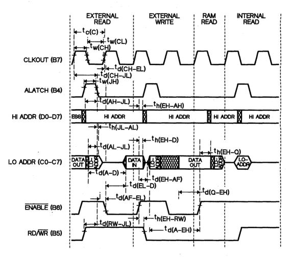
Figure A-1. Read and Write Timing Diagram
