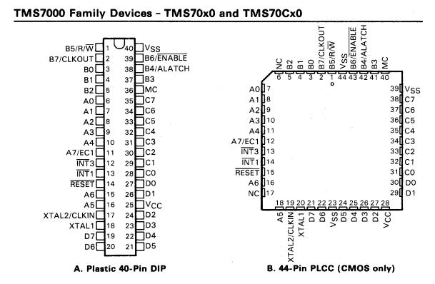
Figure 2-1. Pinouts for TMS7000, TMS7020, TMS7040, TMS70C00, TMS70C20 and TMS70C40
