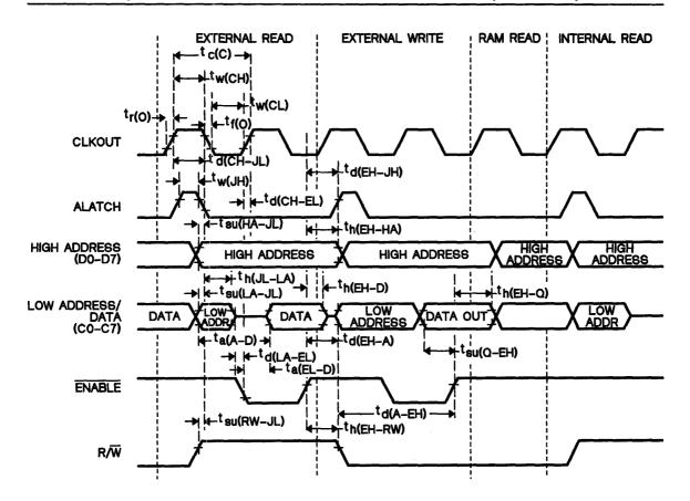
Figure 4-50. Read and Write Cycle Timing
