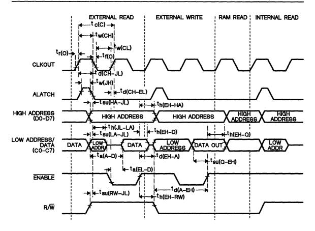
Figure 4-37. Read and Write Cycle Timing
