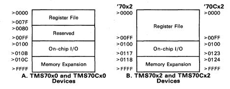
Figure 3-11. Microprocessor Mode Memory Map
