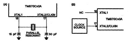
Figure 4-26. Recommended Clock Connections
