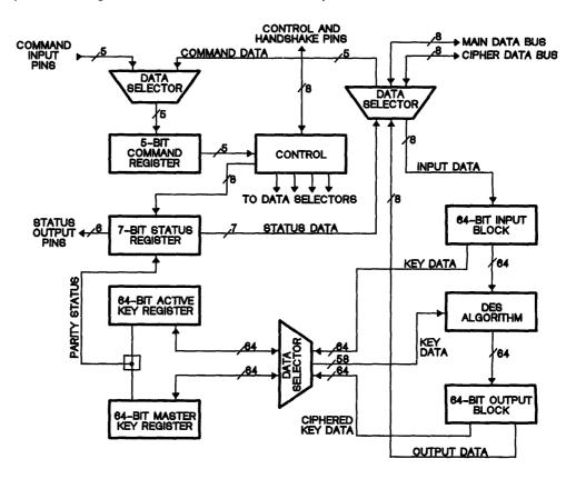
Figure B-1. TMS7500 Functional Block Diagram
