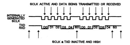
Figure 3-37. Serial I/O Communication Format
