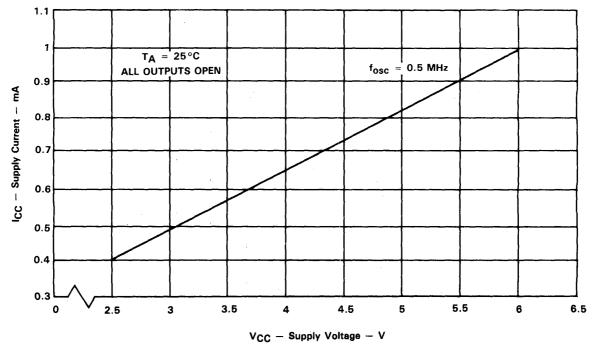
Figure 4-43. Typical Operating Current vs. Supply Voltage
