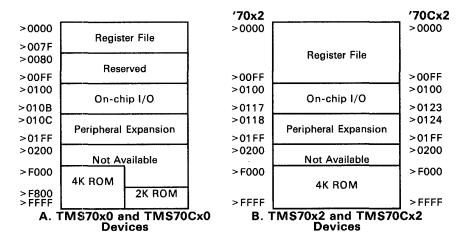
Figure 3-8. Peripheral-Expansion Mode Memory Map
