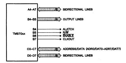
Figure 3-7. I/O Ports – Peripheral-Expansion Mode
