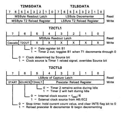
Figure 3-26. Timer 2 Data and Control Registers (TMS70Cx2)
