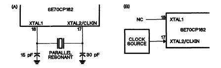
Figure 4-54. Recommended Clock Connections
