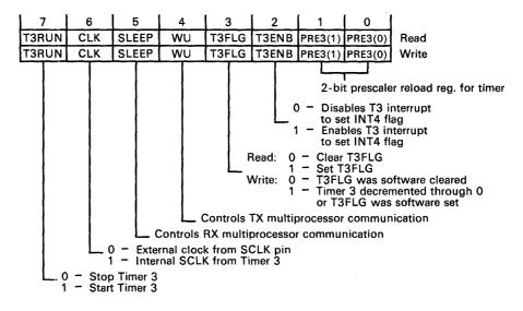
Figure 3-31. Serial Port Control 1 Register - SCTL1
