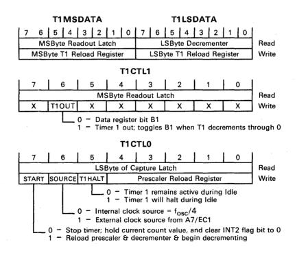
Figure 3-22. Timer 1 Data and Control Registers (TMS70Cx2)
