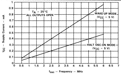
Figure 4-29. Typical Power-Down Current vs. Oscillator Frequency
