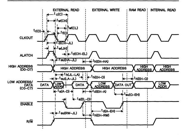
Figure 4-5. Read and Write Cycle Timing
