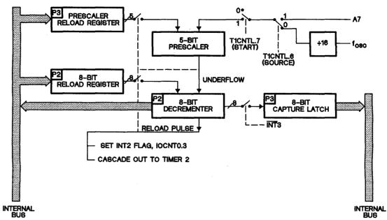
Figure 3-19. 8-Bit Programmable Timer/Event Counters - Timer 1 (TMS70x0, TMS70x2, and TMS70Cx0)
