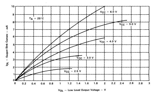
Figure 4-32. Typical Output Sink Characteristics
