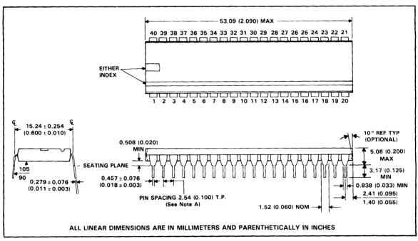
NOTE A: Each pin centerline is located within 0,254 (0.010) of its true longitudinal position.
