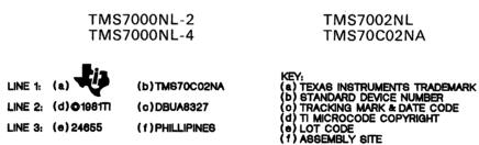
Figure 12-10. TI Standard Symbolization for Devices without On-Chip ROM
