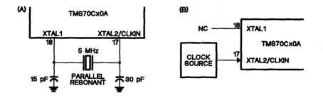
Figure 4-36. Recommended Clock Connections
