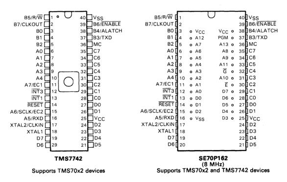
Figure 2-4. Prototyping Devices Available for TMS70x2 and TMS7742 Devices
