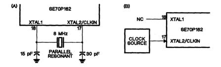
Figure 4-23. Recommended Clock Connections
