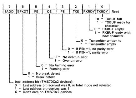
Figure 3-30. Serial Port Status Register - SSTAT
