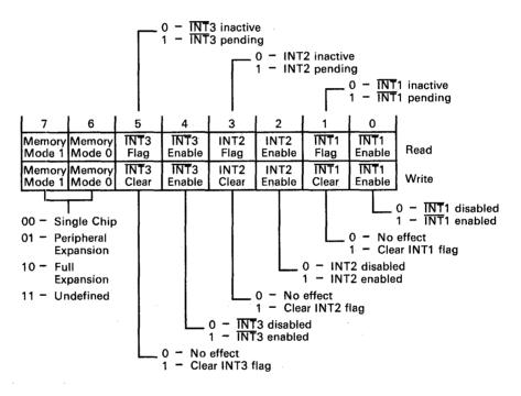
Figure 3-16. IOCNT0 - I/O Control Register 0 (P0 for All Devices)
