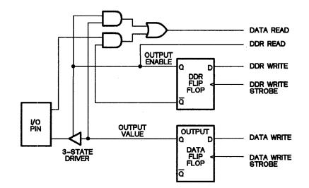
Figure 3-4. Bidirectional I/O Logic
