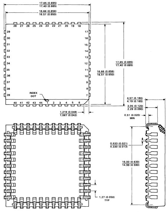
ALL DIMENSIONS ARE IN MILLIMETERS AND PARENTHETICALLY IN INCHES
