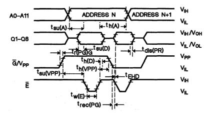
Figure 4-18. Program Cycle Timing
