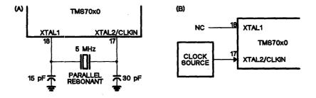
Figure 4-4. Recommended Clock Connections
