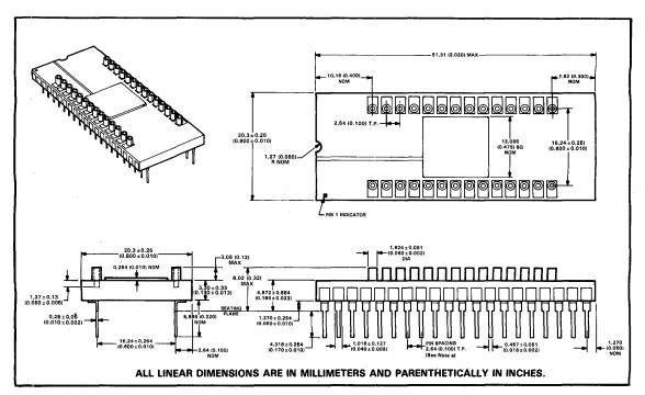
NOTE A: Each pin centerline is located within 0,254 (0.010) of its true longitudinal position.
