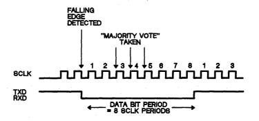
Figure 3-35. Asynchronous Communication Format
