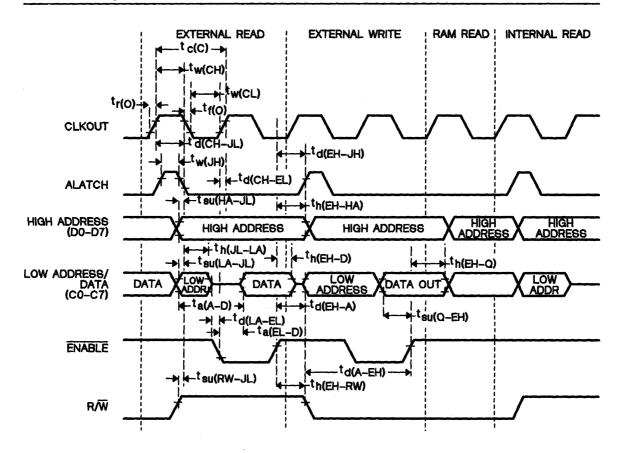
Figure 4-11. Read and Write Cycle Timing
