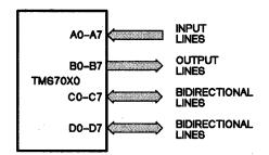
Figure 3-5. I/O Ports - Single-Chip Mode
