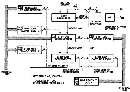
Figure 3-24. 16-Bit Programmable Timer/Event Counters - Timer 2 (TMS70Cx2)
