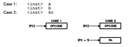
Figure 6-1. Single Register Addressing Mode Object Code
