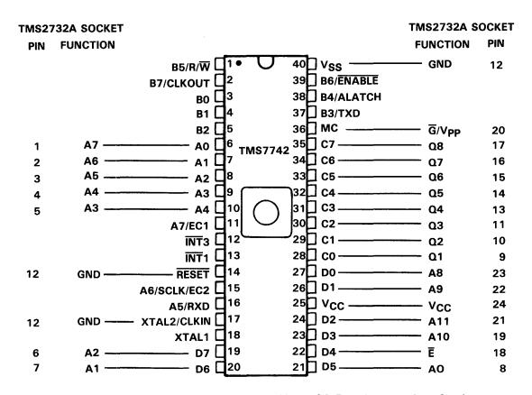
Figure 9-2. PROM Programmer 40-to-24-Pin Conversion Socket
