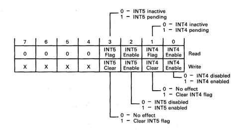
Figure 3-17. IOCNT1 - I/O Control Register 1
