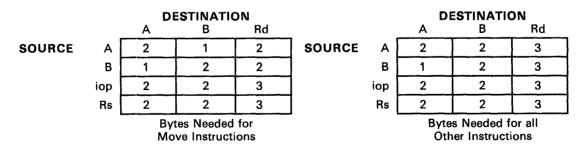
Figure 6-2. Dual Register Addressing Mode Byte Requirements
