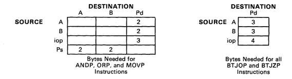
Figure 6-3. Peripheral-File Addressing Mode Byte Requirements
